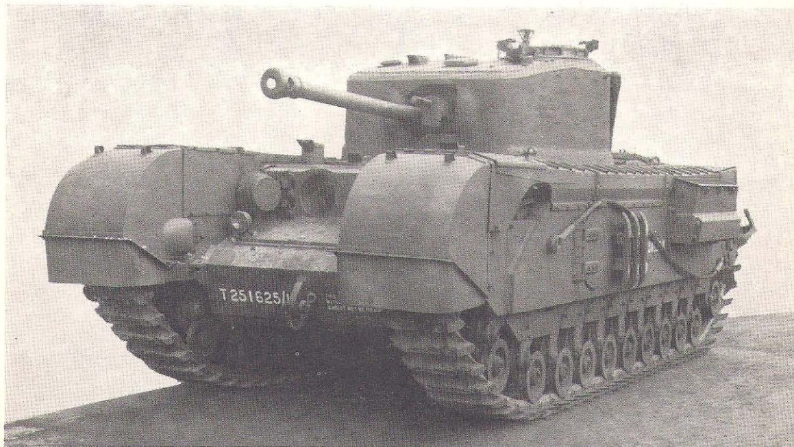
Two views of the Churchill VII show the new turret, the commander's cupola, the 75 mm. gun, the round escape hatches and armoured covers on the exhaust manifolds, all introduced on this mark. Note also the new side appearance, the bolts having "disappeared" due to the integral armour plating on the hull. (Imp. War Mus.)
