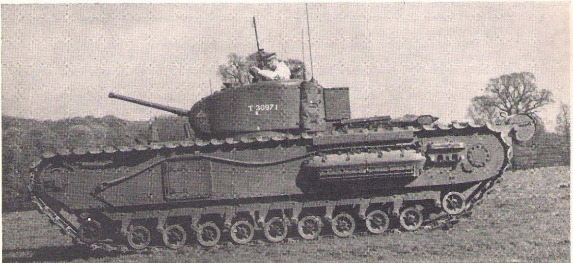
His Majesty the late King George VI inspects the first production model of the Churchill I, then still known only as the Infantry Tank Mk. IV, in March, 1941. Ordered straight off the drawing board, this was also the "pilot" model, and was made of mild steel.
