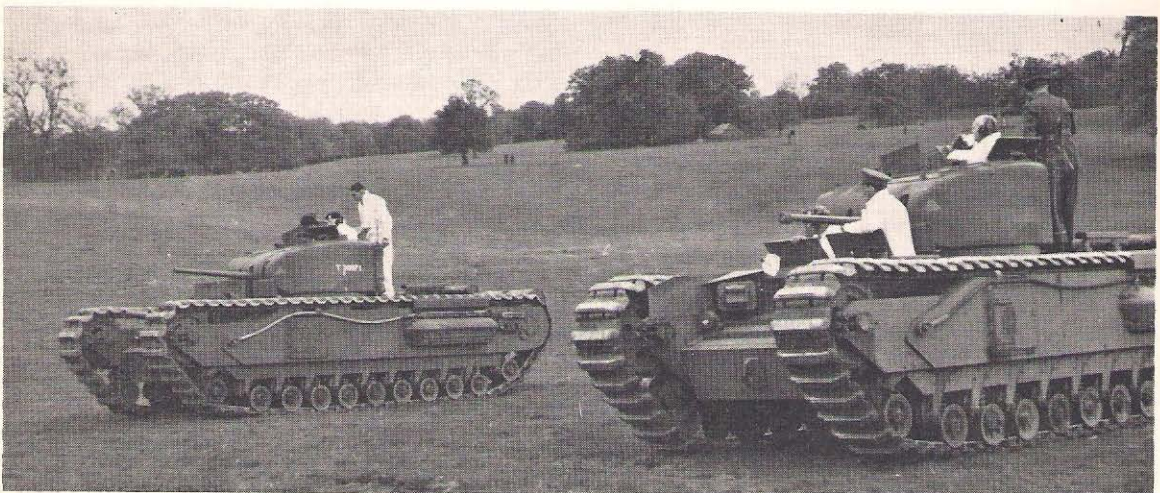
Mr. Winston Churchill, the Prime Minister, paid a visit to Vauxhall in 1941 to see the tank which later took his name. He is seen here in the second production vehicle (nearest the camera) talking by R/T to General Sir John Dill, C-in-C Home Forces, in the first production machine. Note the triangular warning plate on the turrets indicating mild steel construction. (Imp. War Mus.)
