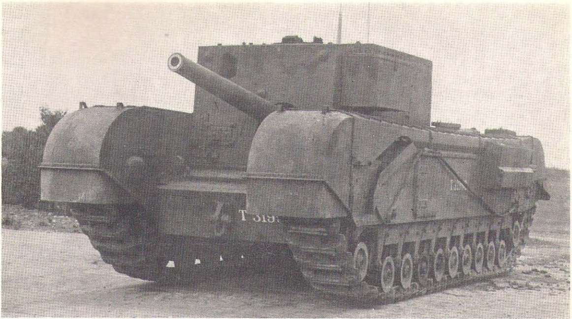
Two views of the Gun Carrier, 3-inch Churchill Mk. 1, showing the new superstructure and the limited traverse mount for the 3-inch gun. This particular vehicle is the pilot model built by Vauxhall. Production vehicles were built by Beyer Peacock. (Peter Chamberlain Collection)
