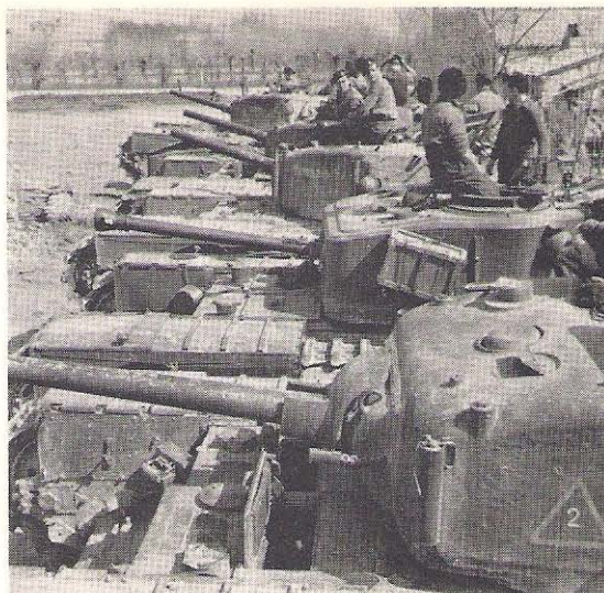
Four Churchills lined-up in Italy show clearly the difference between the Mk. IV (NA 75s) with 75 mm. gun from Sherman tanks, compared to a Churchill VII with 75 mm. gun, which is the second vehicle in the line. Note the commander's cupola in this later vehicle. This picture was taken in April, 1945, when NA 75s were still in service. (Imp. War Mus.)
