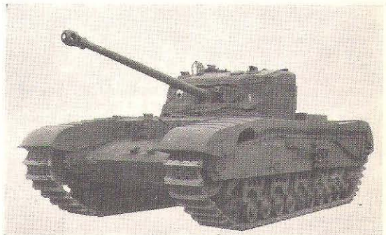
The A43 Black Prince (sometimes known as the "Super Churchill") was essentially similar to the Churchill VII, scaled-up to take a 17 pdr. gun. Note that the intake louvres were moved to the hull top, however, and the exhaust was led to the rear. Increased width of this vehicle to take the wider turret is noticeable. In the Black Prince, also, the commander's position was moved to the right as the gun was turned sideways for left-hand loading. Only six vehicles were built and the Black Prince never entered full production. (Peter Chamberlain Collection)
