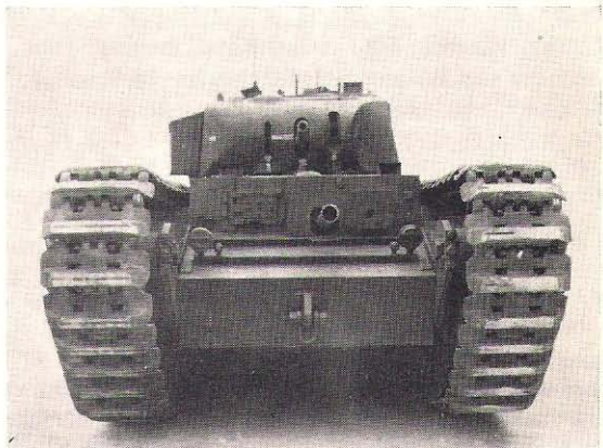
Three views of one of the first production Infantry Tank, Mk. IV taken at Luton May 9, 1941, show the characteristics of the Churchill I, including the 3-in. howitzer in the hull front, small cast turret with pistol ports and 2 pdr. gun, brackets for long range fuel tank at rear, lack of track covers, unarmoured exhaust manifolds and the original type of intake louvre. (Imp. War Mus.)
