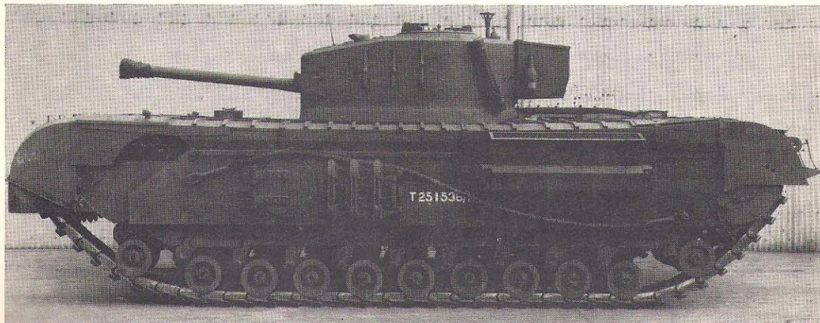
Two views of the Churchill VII show the new turret, the commander's cupola, the 75 mm. gun, the round escape hatches and armoured covers on the exhaust manifolds, all introduced on this mark. Note also the new side appearance, the bolts having "disappeared" due to the integral armour plating on the hull. (Imp. War Mus.)
