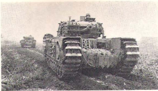
A Churchill VI, which was essentially a Mk. IV re-armed with a 75 mm. gun, seen in North-West France in October, 1944. Note the use of Sherman track shoes for added protection.
