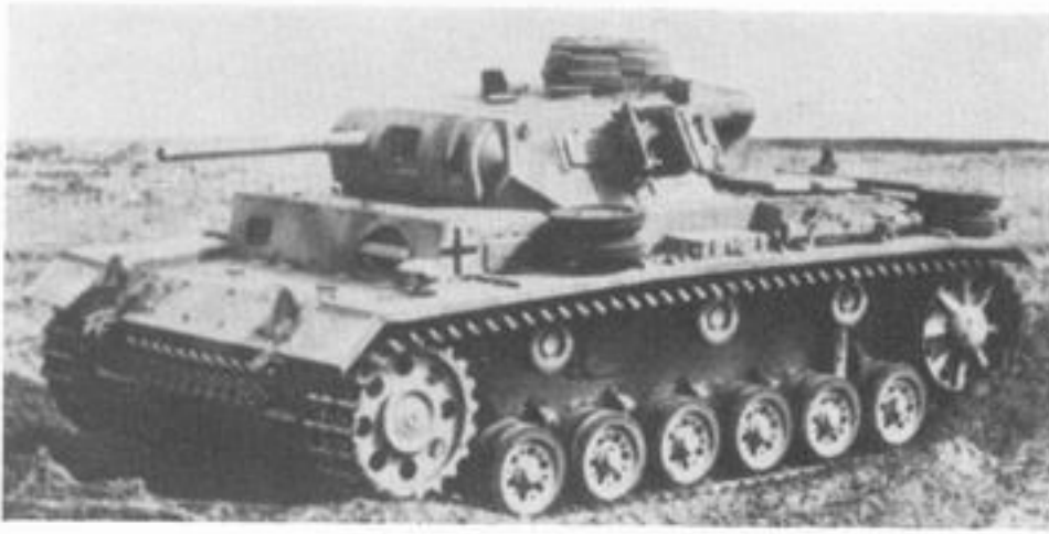
The Pz.Beob.Wg III (armoured observation post) had a dummy wooden gun barrel and a central ball-mounted machine gun in the mantlet to serve observation officers for motorized artillery units. This one is based on a Panzer III Ausf H. Turret was fixed. (Imp War Mus.)
