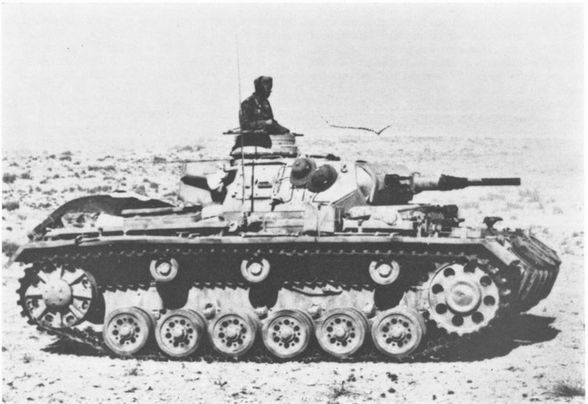
A Panzer III Ausf F or G with the Afrika Korps in late 1941. It has the early cupola but re-spaced return rollers, plus the short 5 cm. gun. (Imp. War Mus.)
