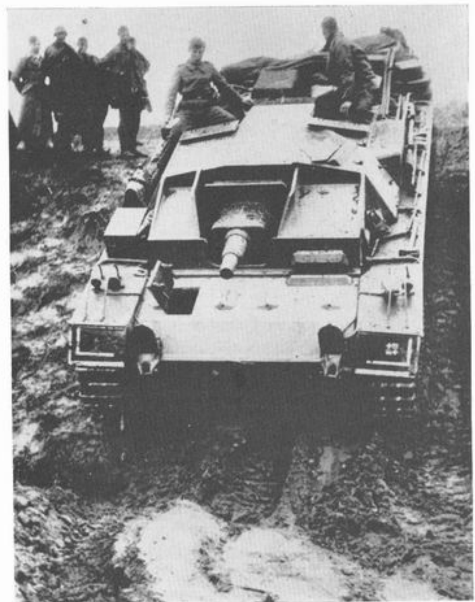
Another view, of a StuG III Ausf C with short 75 mm. gun, shows how the conversion was simply made on the basic Panzer III design by producing a completely new superstructure. Hull sub-assemblies did not require changing. Projection on left of superstructure (right) housed radio equipment. (Imp. War Mus.)
