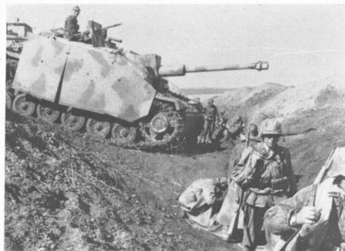
A StuG III Ausf G negotiates an anti-tank ditch on the Orel Front, Russia, in support of advancing infantry. Note the machine-gun and shield, and the commander's binocular sight raised in the cupola. Skirt armour was a usual fitting by this period, July 1943. (Imp. War Mus.)
