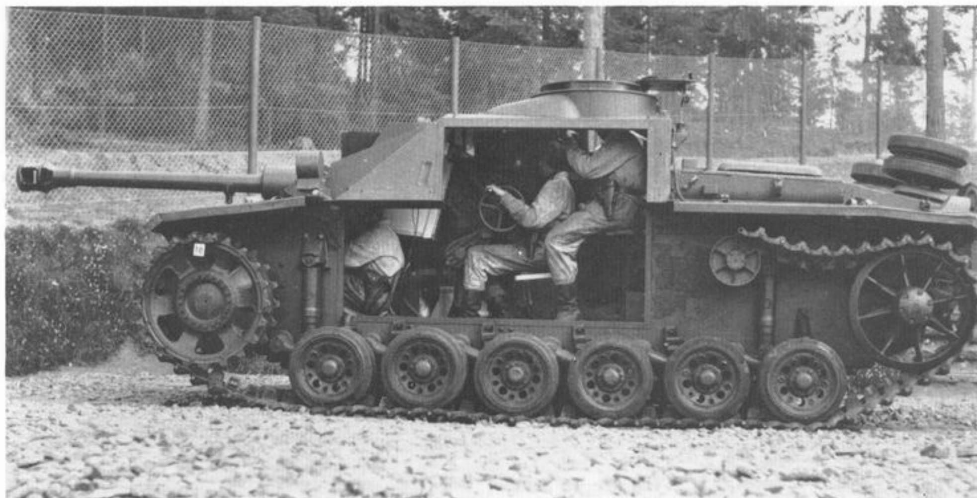
A late model StuG III Ausf G at the Finnish Army Museum with its side cut away to show interior layout and crew positions. This also gives an excellent view of the Panzer III torsion bar suspension. (Chamberlain Collection.)
