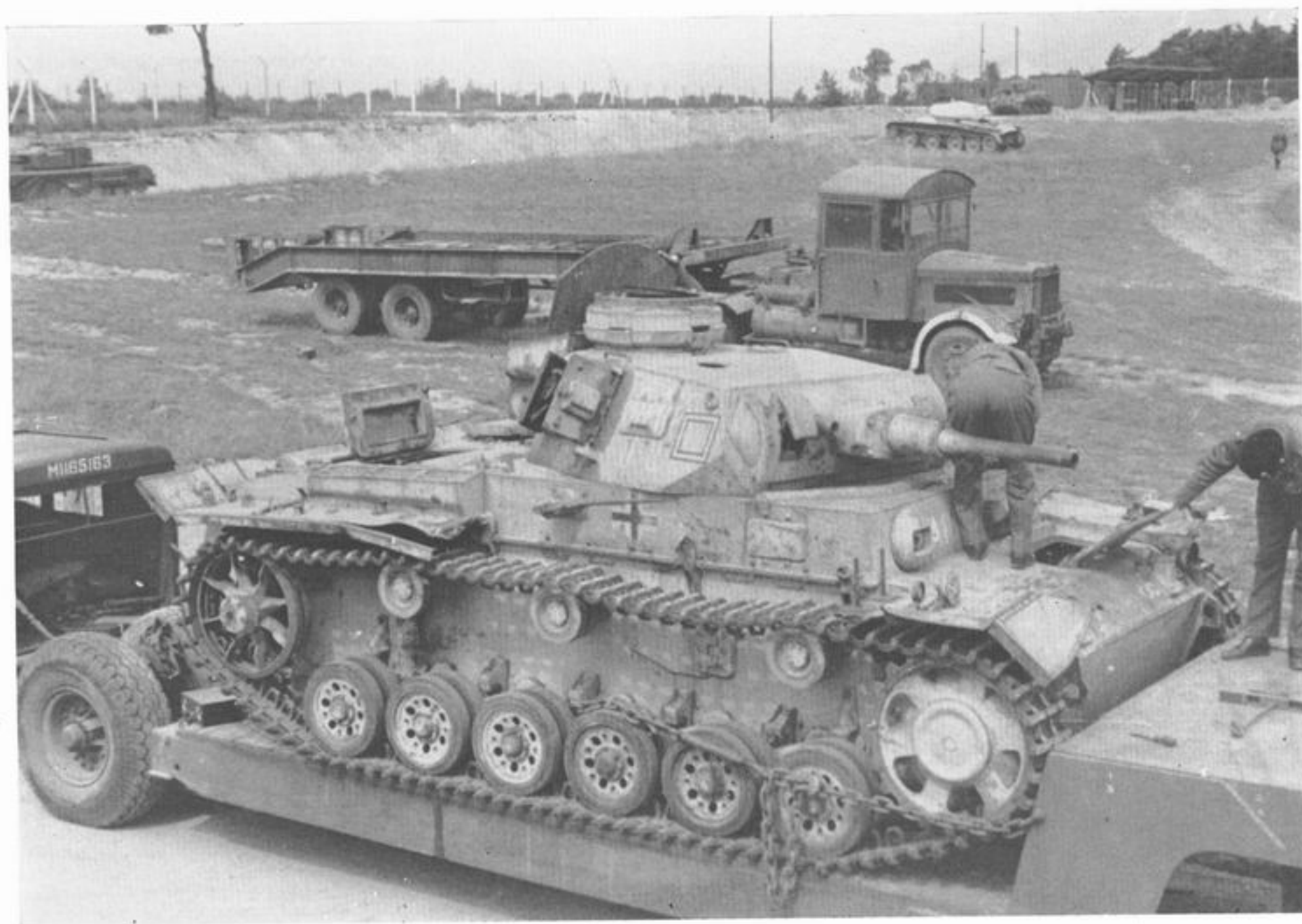
A captured Afrika Korps Panzer III Ausf J seen on arrival in Britain where it was examined by British intelligence authorities. Note movable twin covers over vision ports in cupola. (Imp. War Mus.)
