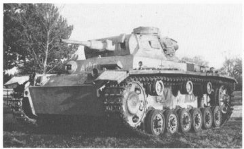
Another view of an early Ausf J, clearly shows the wider spaced return rollers. (Warpics.)
