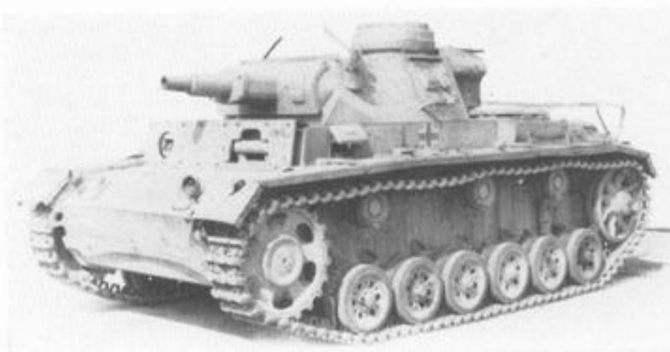
Above: Model N had the short L/24 75 mm. gun from the Panzer IV, and appeared in late 1942 and 1943 for the 'close support' role. It was sometimes called Sturmpanzer III. This is one of the Model Ns converted from a Model L. Others were built as Ns. (Imp. War Mus.)
