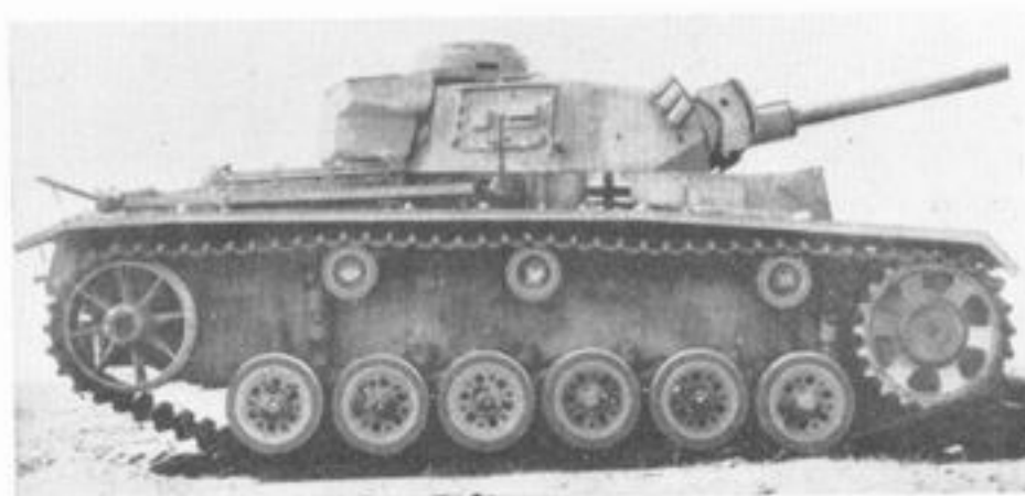
In 1942 a total of 100 Panzer III Ausf M were converted to Flammenwerfer-Panzer III by replacing the 5 cm. long gun with a flame projector which resembled the gun barrel except for lack of taper. 1000 litres of flame fuel were carried in the hull in containers which replaced the ammunition racks, and on one loading 70-80 shots were possible. Range was 55-60 metres. Note the triple smoke dischargers on turret side. (Chamberlain Collection.)
