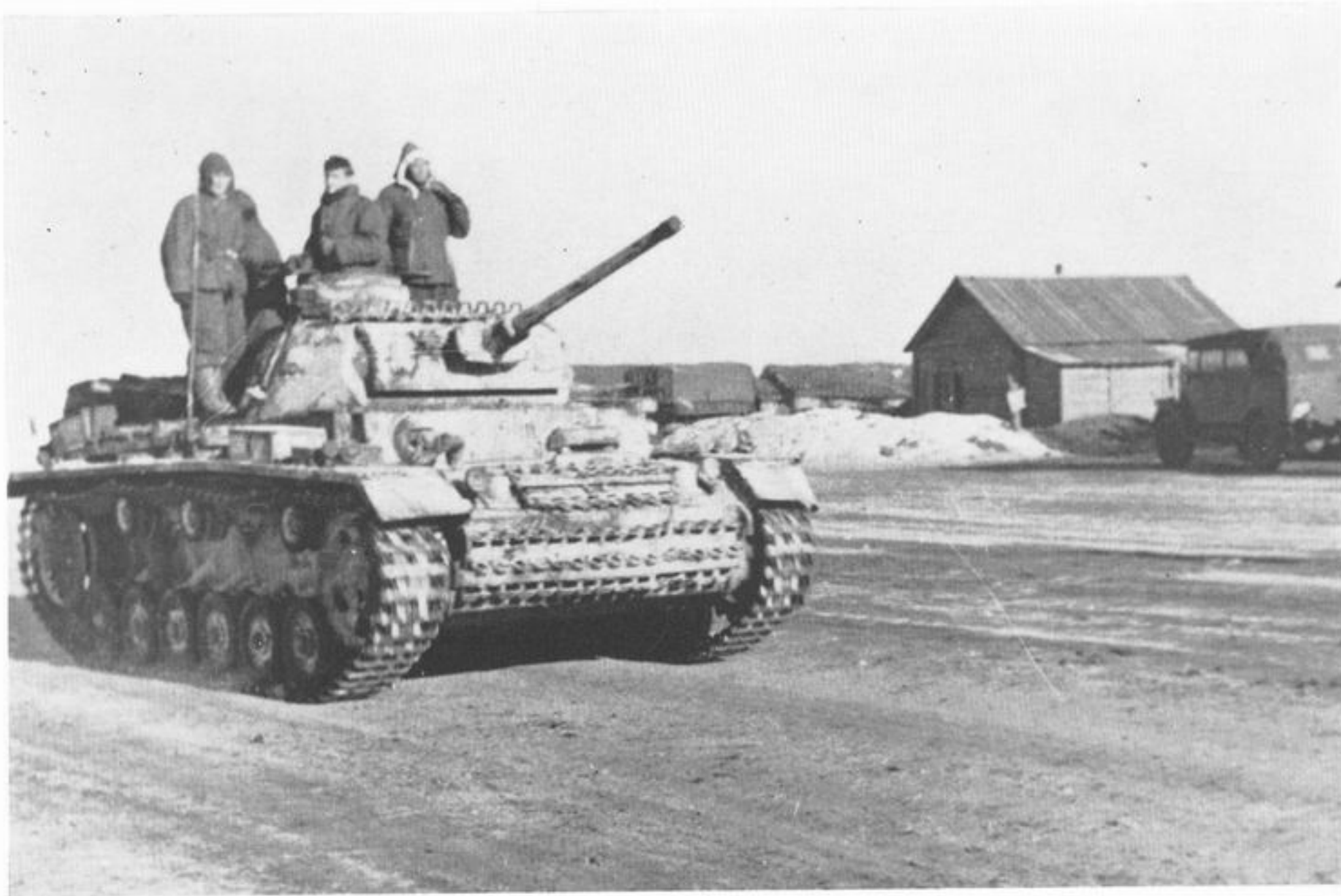
Panzer III Ausf J with long 50 mm. gun, shown in Russia in 1942 with winter camouflage and trackshoes on nose and turret top for added protection. (Warpics.)
