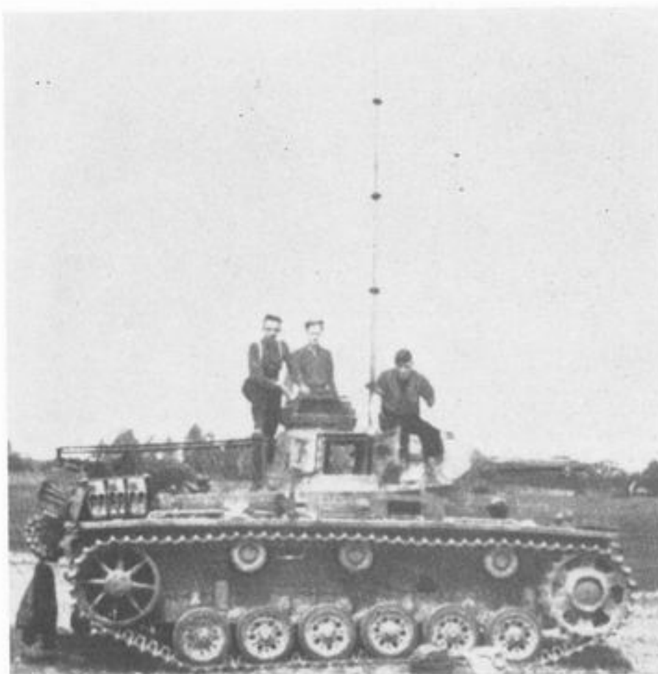
Rare view of a Pz.Bef.Wg III Ausf H (formerly Ausf C) in service, with 9 metre aerial erected. (Axel Duckert.)
