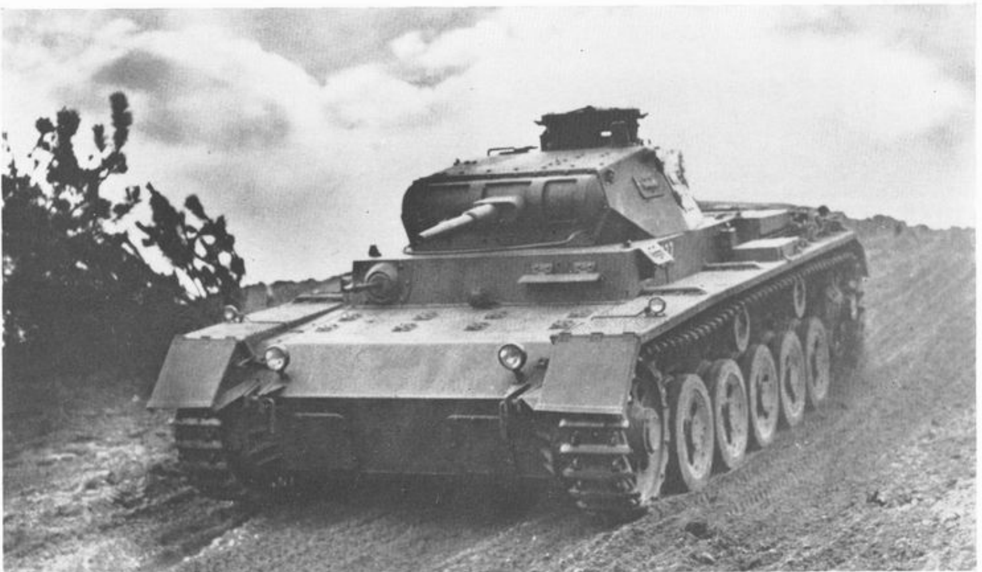
Below: A fine view of one of the Panzer III Ausf A development vehicles on test, showing the large bogie wheels used in this first model. (Chamberlain Collection.)
