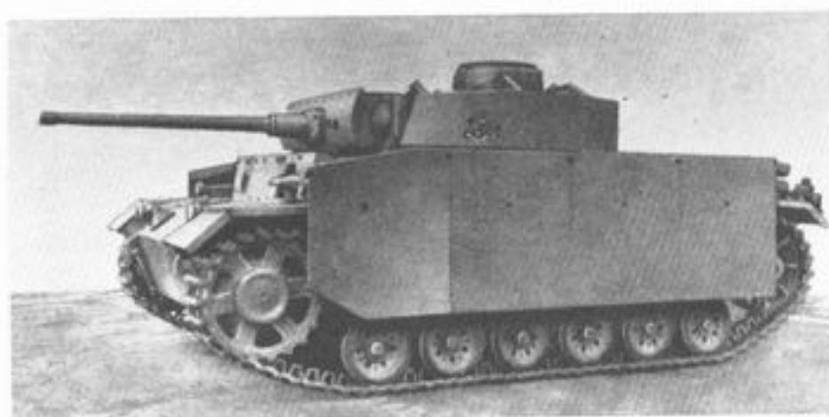
Below: Another Model M this time fitted with full skirt armour for hull and turret, a 1943 feature. (Chamberlain Collection.)
