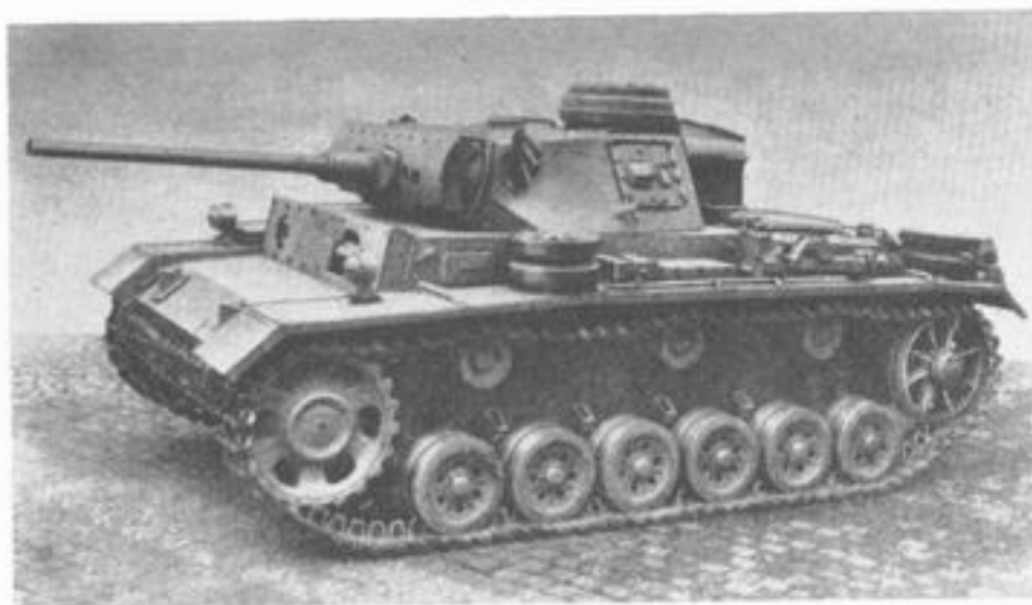
Above: Ausf M had all the visible external features of the L but the pistol ports in the turret side were omitted as were the hull side escape hatches. Another prominent feature were the triple 90 mm. Nb.Kwg. smoke dischargers on the turret sides, replacing the tail smoke dischargers. (Chamberlain Collection.)
