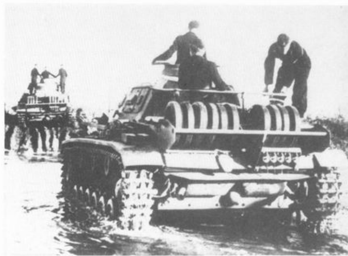
A Pz.Bef.Wg III fords a river during the initial stages of the invasion of Russia in 1941. Note the frame aerial, spare wheels, and tail smoke dischargers in a rack on the right rear. (Imp. War Mus.)
