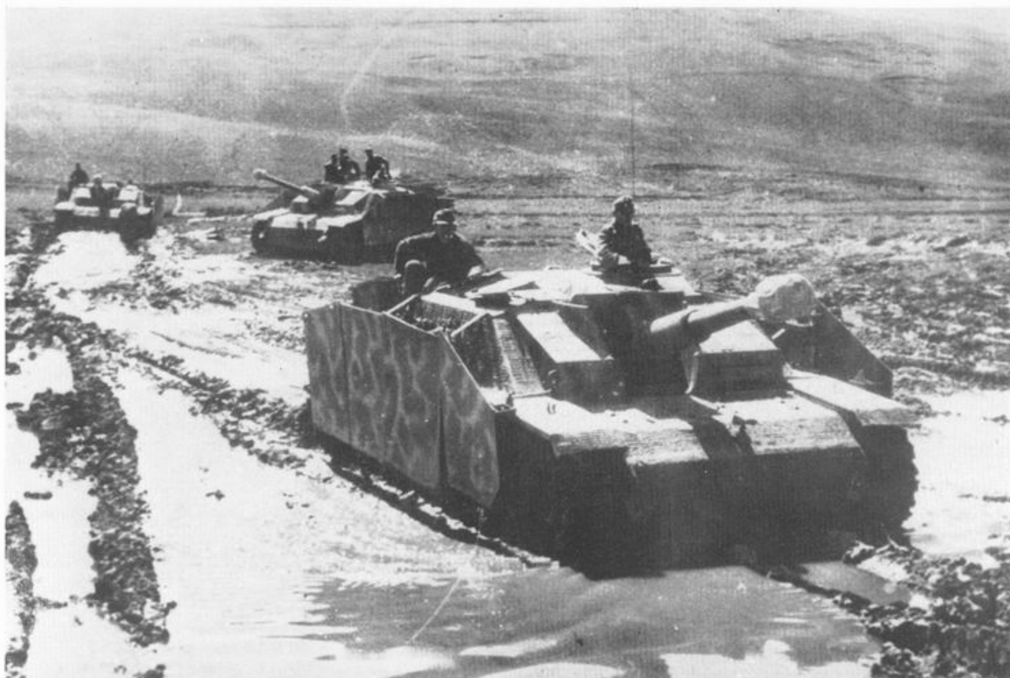
One in every nine StuG IIIs from 1942 onwards had the 10.5 cm. howitzer (and were classified 'Sturmhaubitze'). Otherwise they were identical to the StuG III Ausf G with the 75 mm. gun. This vehicle is shown in Northern Italy in July 1944. It is typical of very late StuG IIIs with Zimmerit anti-magnetic paste covering clearly visible. (Imp. War Mus.)
