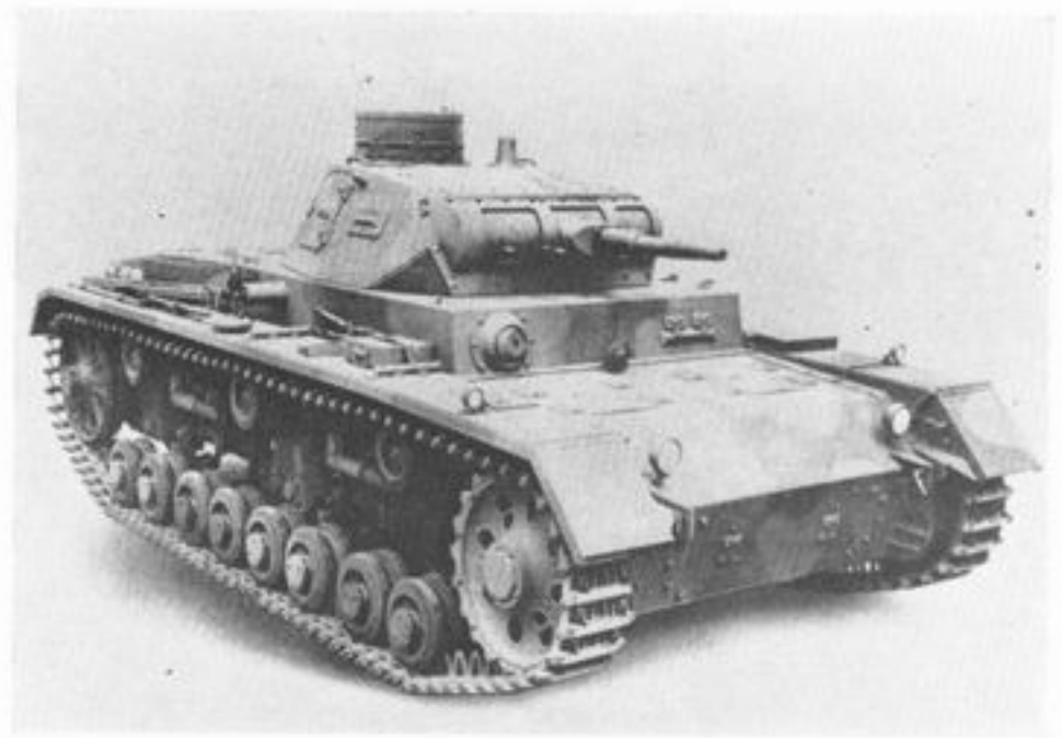
The Panzer III Ausf B differed from the A in having eight small bogie wheels. Note in particular the plain 'dustbin' type cupola with eight peep slots and the horn type periscope on the turret top. Model C was externally identical. (Imp. War Mus.)
