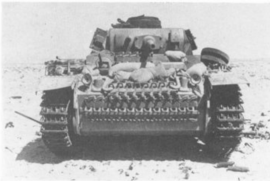
Major distinguishing feature of Ausf J was the new ball mount for the hull machine gun and thicker armour. This is an early production vehicle with the 5 cm. L/42 gun – later vehicles had the long L/60 weapon. Note track shoes and sandbags used for extra frontal protection. (Imp. War Mus.)
