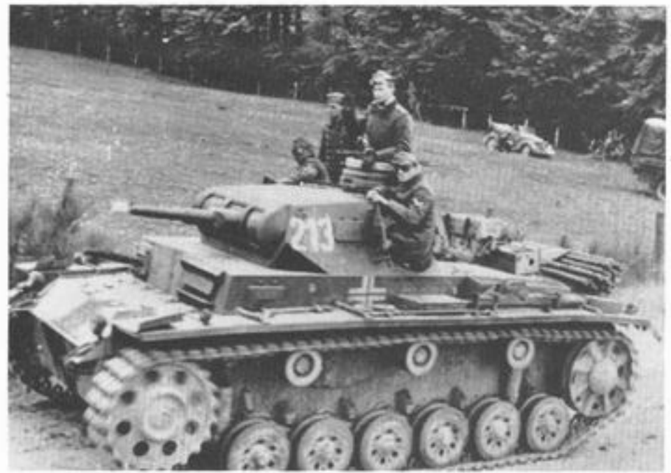
Panzer III Ausf E was the last model in the development series and had the torsion bar suspension adopted for all subsequent production models. Driver's visor cover and the machine-gun mount were also improved. This is an Ausf E in France, May 1940. It is evidently a vehicle brought from Poland since the cross shows evidence of being 'modified' from plain white. (Imp. War Mus.)
