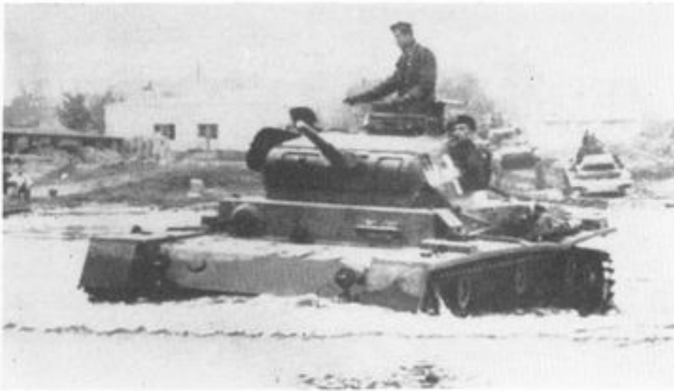
First campaign involving the Panzer III, though only in relatively small numbers, was the invasion of Poland, September 1939. This is one of the Ausf D development models, distinguished by its front visor plate fittings (in this view), fording a river on the approach to Warsaw. Plain white cross was standard recognition mark for this campaign. (Chamberlain Collection.)
