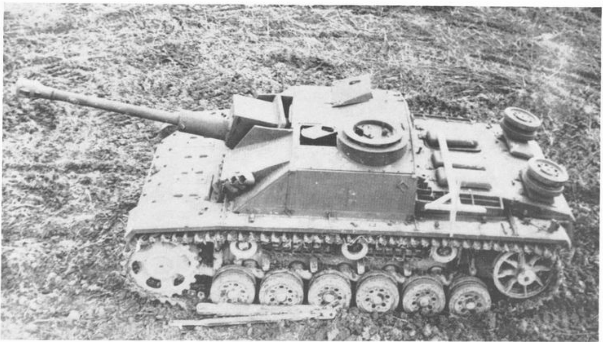
From 1942 the StuG III had the potent long L/48 75 mm. gun. This official recognition shot shows the Ausf G model, complete with machine-gun shield on the roof, vision cupola, smoke dischargers and improved superstructure with increased 80 mm. armour maximum. (US Signal Corps.)
