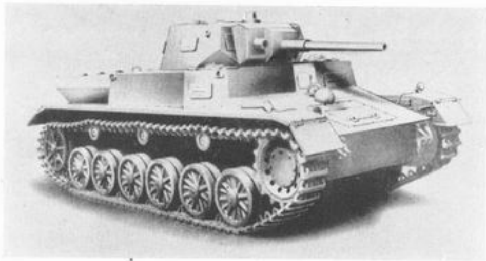
Above: The Krupp prototype for the ZW requirement. This vehicle was not adopted as the basis of the Panzer III but Krupp incorporated many of its features in the Panzer IV later. (Imp. War Mus.)
