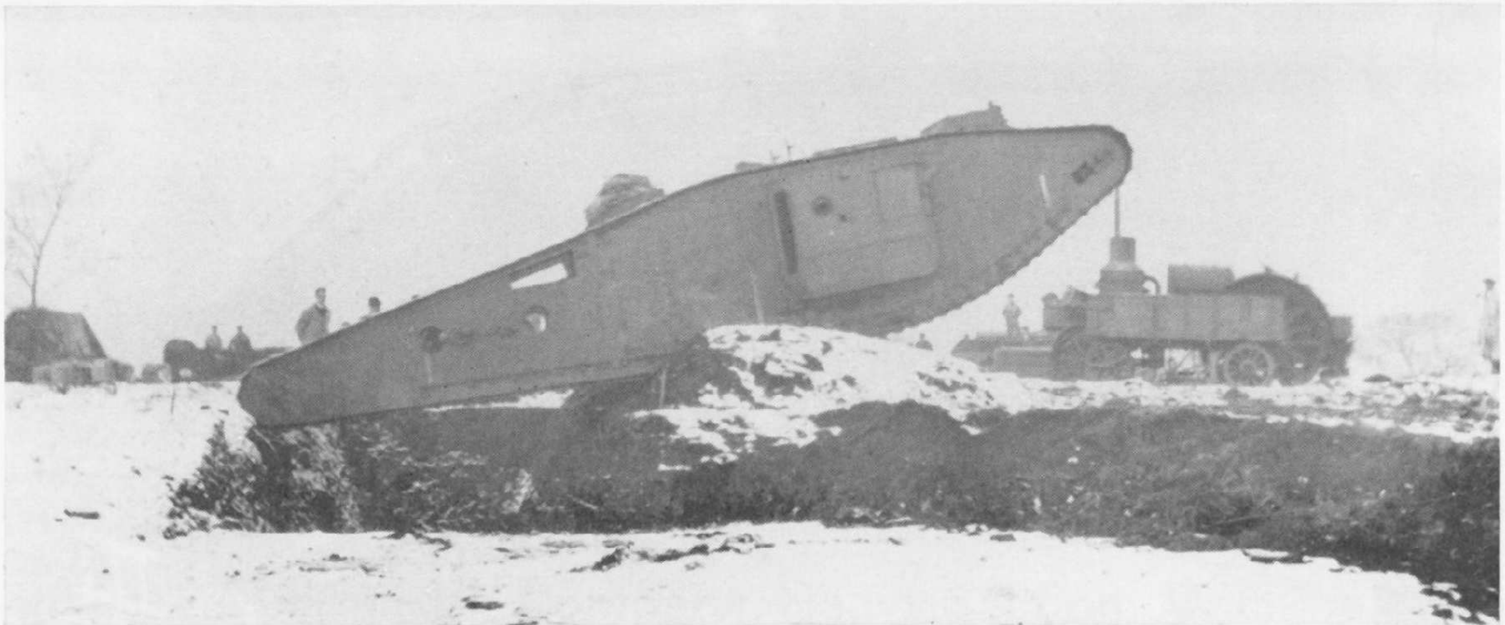
The increased trench crossing ability of the "Tadpole Tail" on a Mk. IV being demonstrated at the Tank Supply Department's test ground, Wembley Park. (Imperial War Museum)
