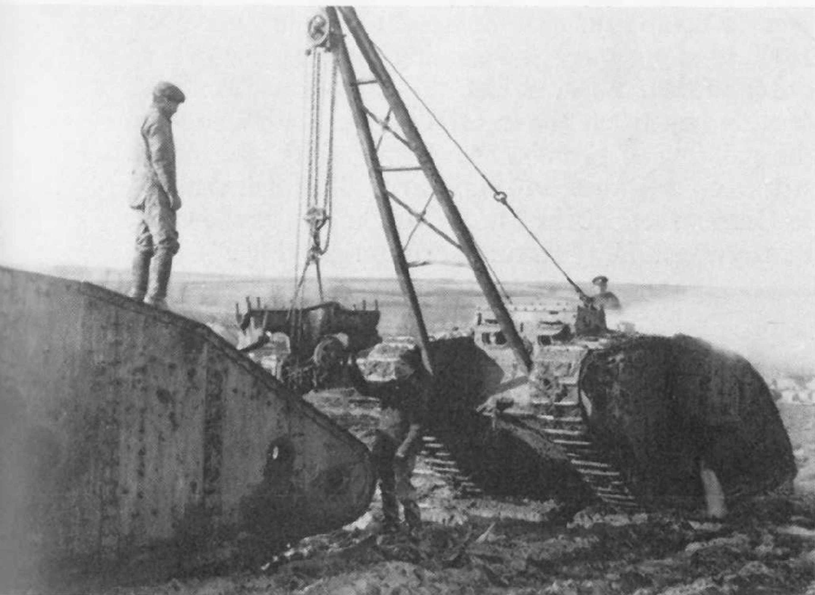
A few Mk. IV's were converted to Salvage Tanks by the addition of sheerlegs and Westons purchase. They were used mainly at the tank parks and at the Erin depot for maintenance work on damaged tanks. (Imperial War Museum)
