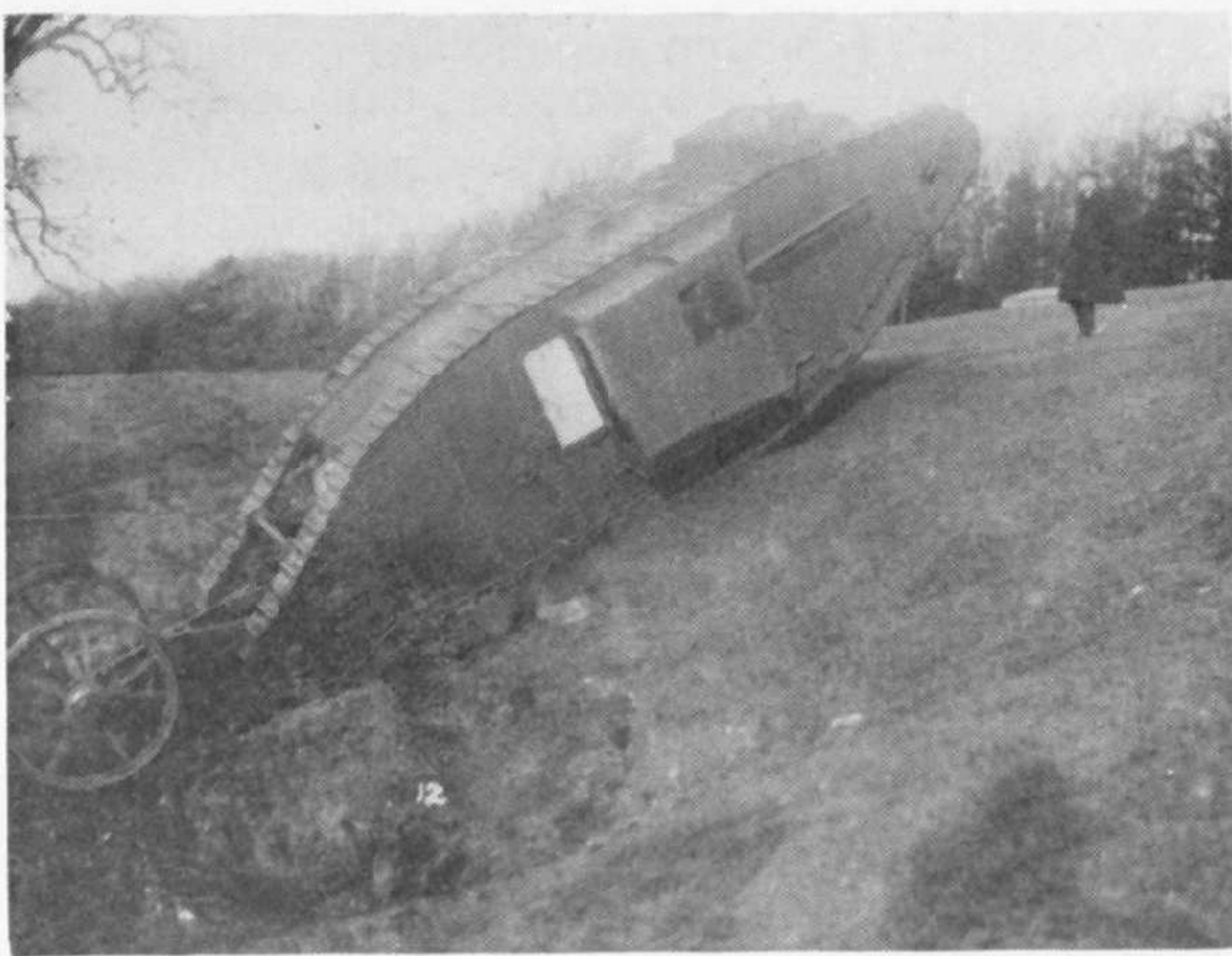
"Mother" shows its capabilities on an initial test run before the official demonstration. Note access door in sponson. (Imperial War Museum)
