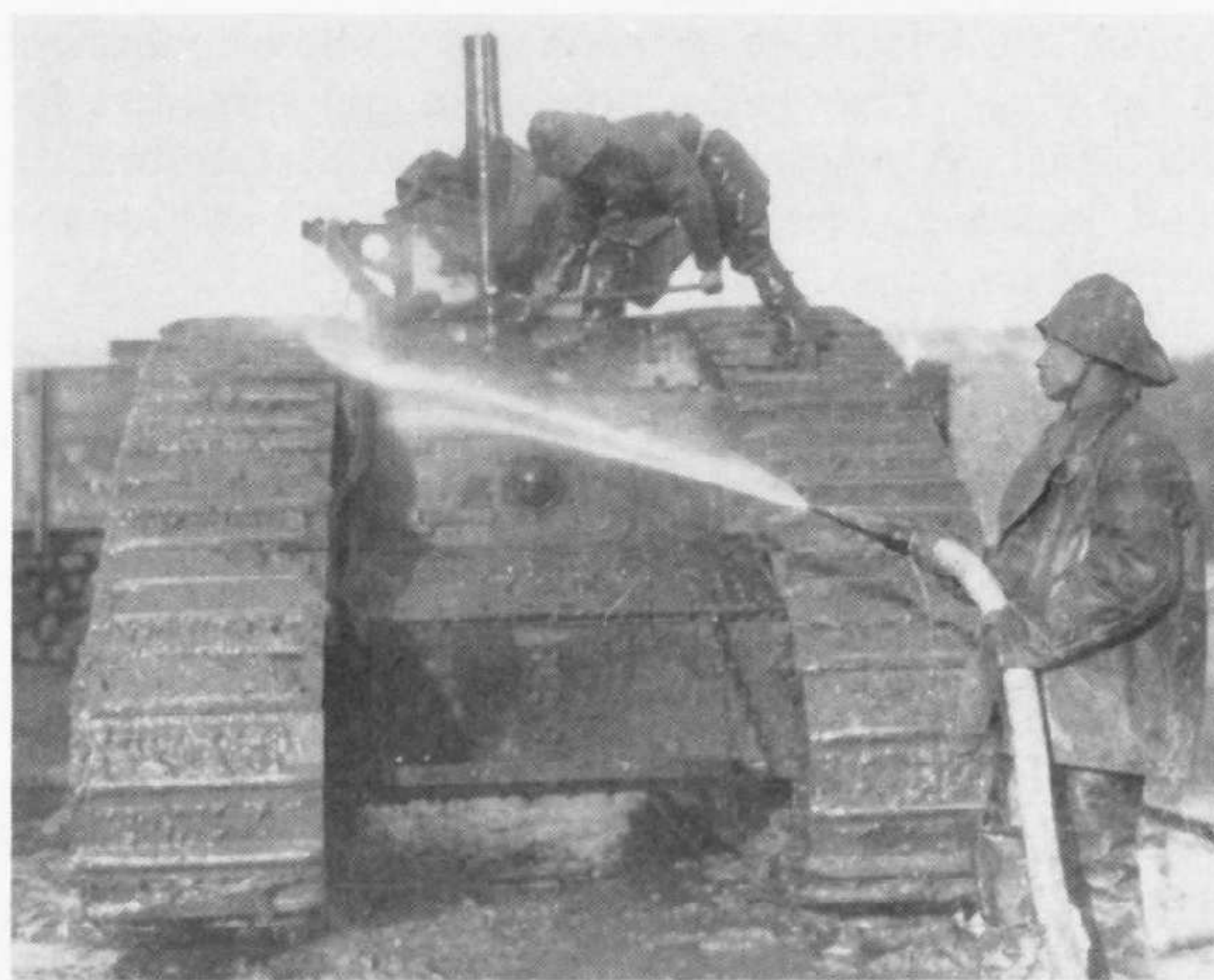
Chinese labourers hosing down a Mk. V in for repair at the Erin depot. Note the ball mount for the rear machine-gun, the external armoured fuel tank, and the post with semaphore arms for signalling. (Imperial War Museum)
