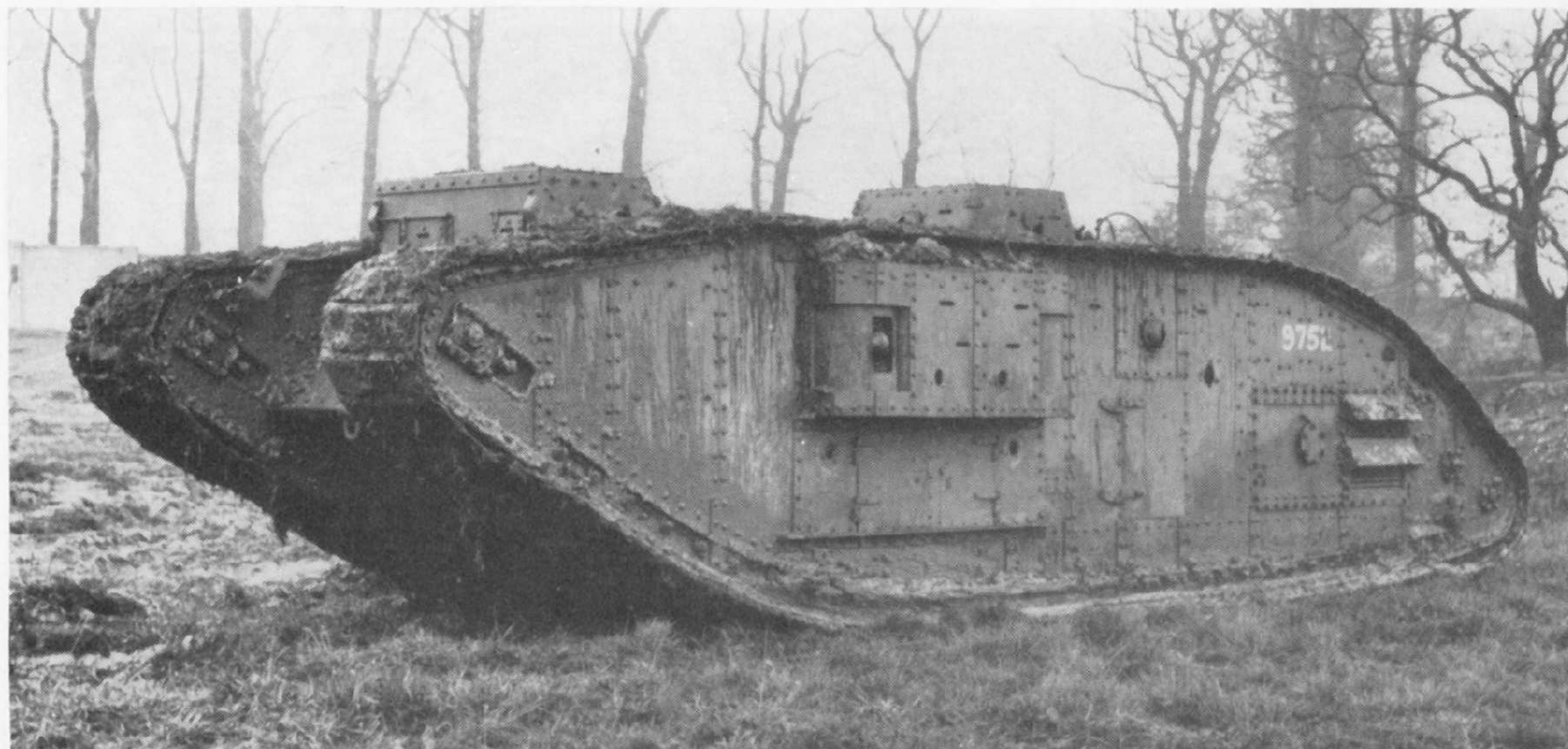
The Mk. V* showing the lengthened hull. This is a female. (Imperial War Museum)
