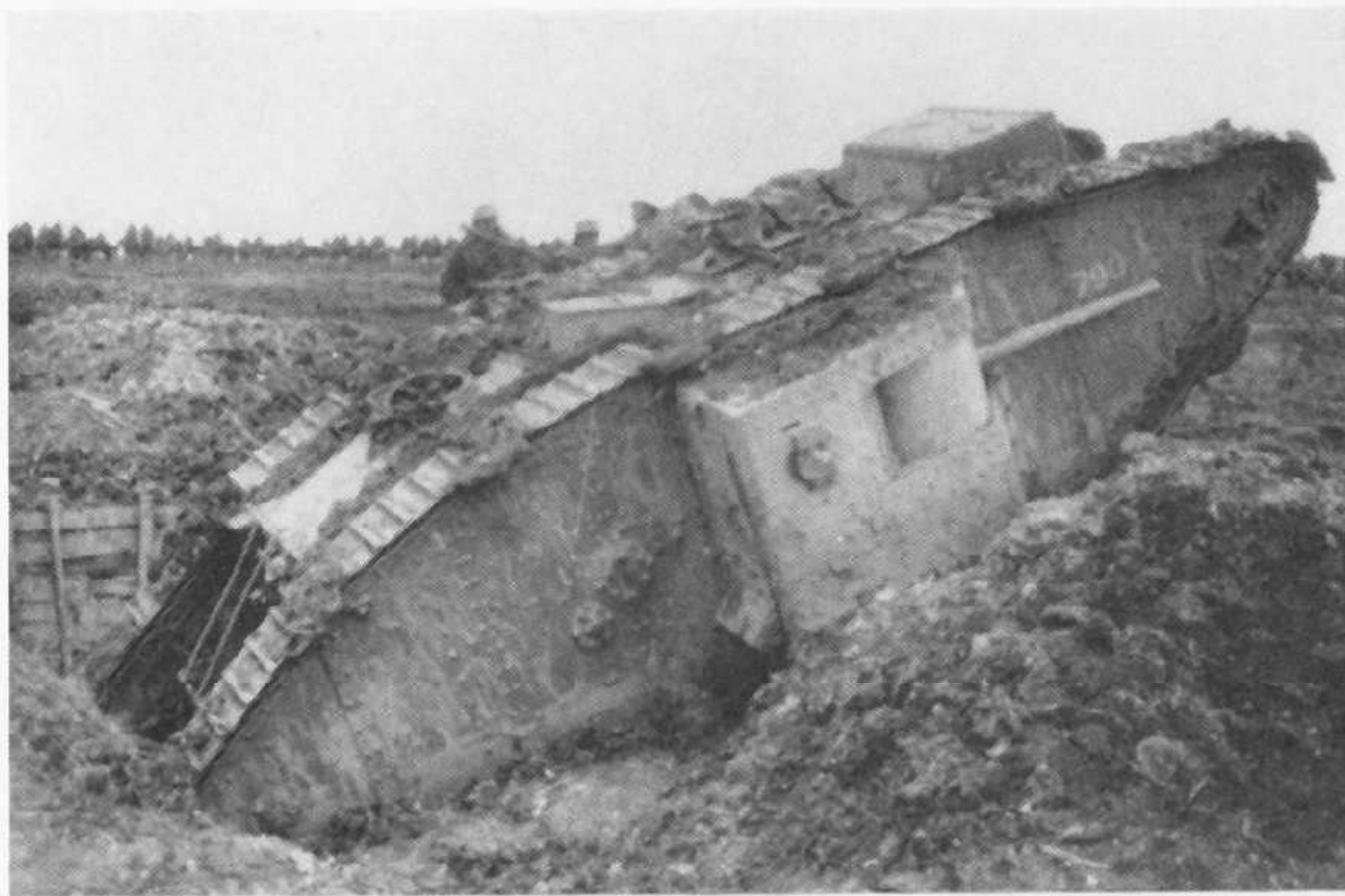
Fine view of a Tank Mk. II male at Arras, April 13, 1917, shows the modified hatchway in hull top and the widened track shoes. Note the cavalry on the horizon. (Imperial War Museum)
