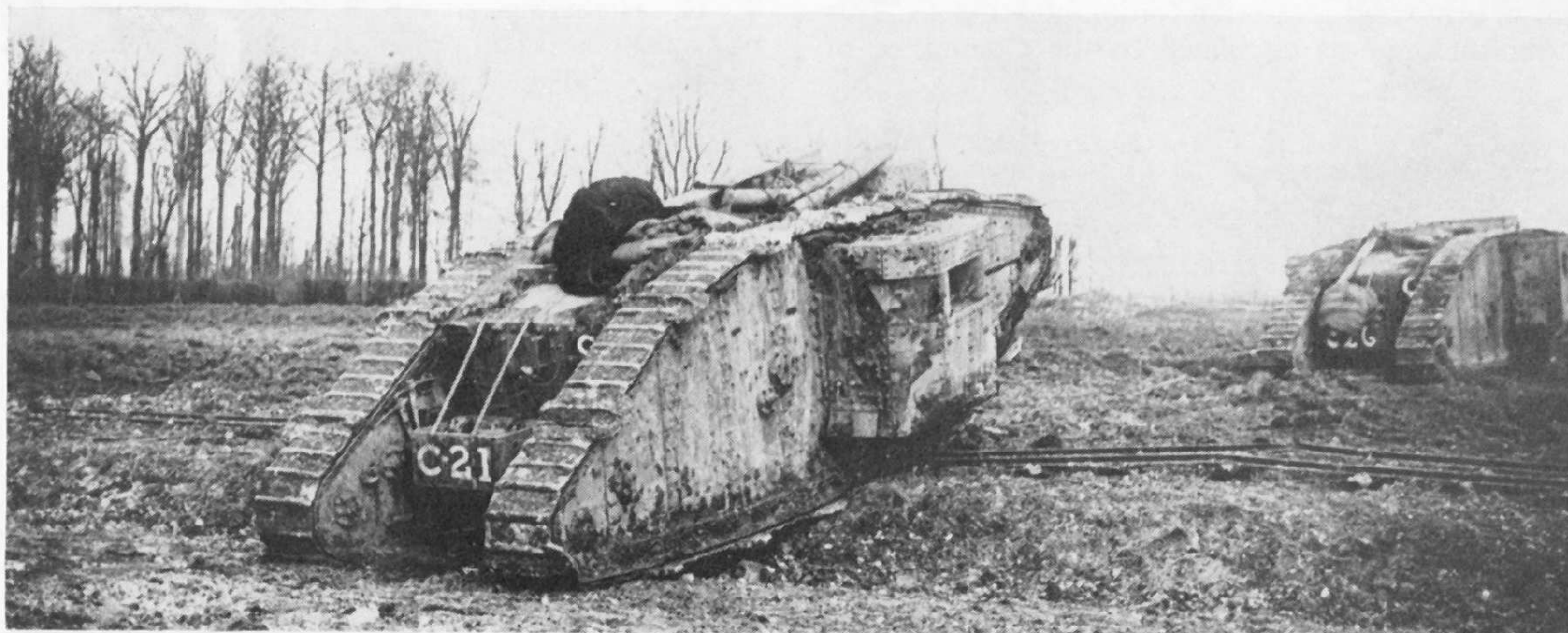
A Mk. I female in December 1916 after the tail and bomb roof had been removed, showing addition of the stowage tray at the rear. (Imperial War Museum)
