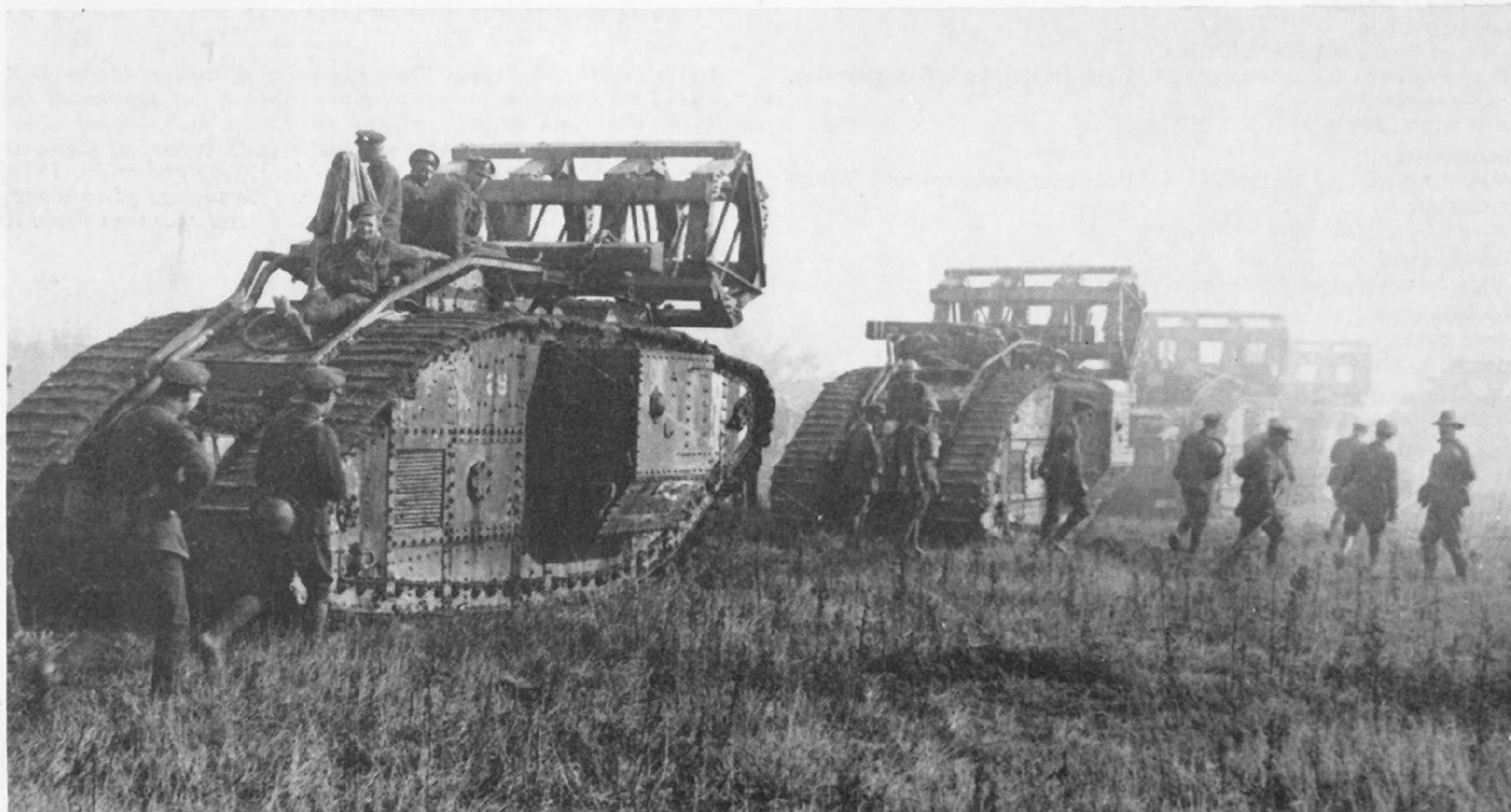
Mark V tanks move forward with cribs to cross the tributaries of the Selle river during the final stages of the War, October 1918, when Britain's tank force was at a peak of 25 battalions, 18 of them in France including one armoured car battalion. (Imperial War Museum)
