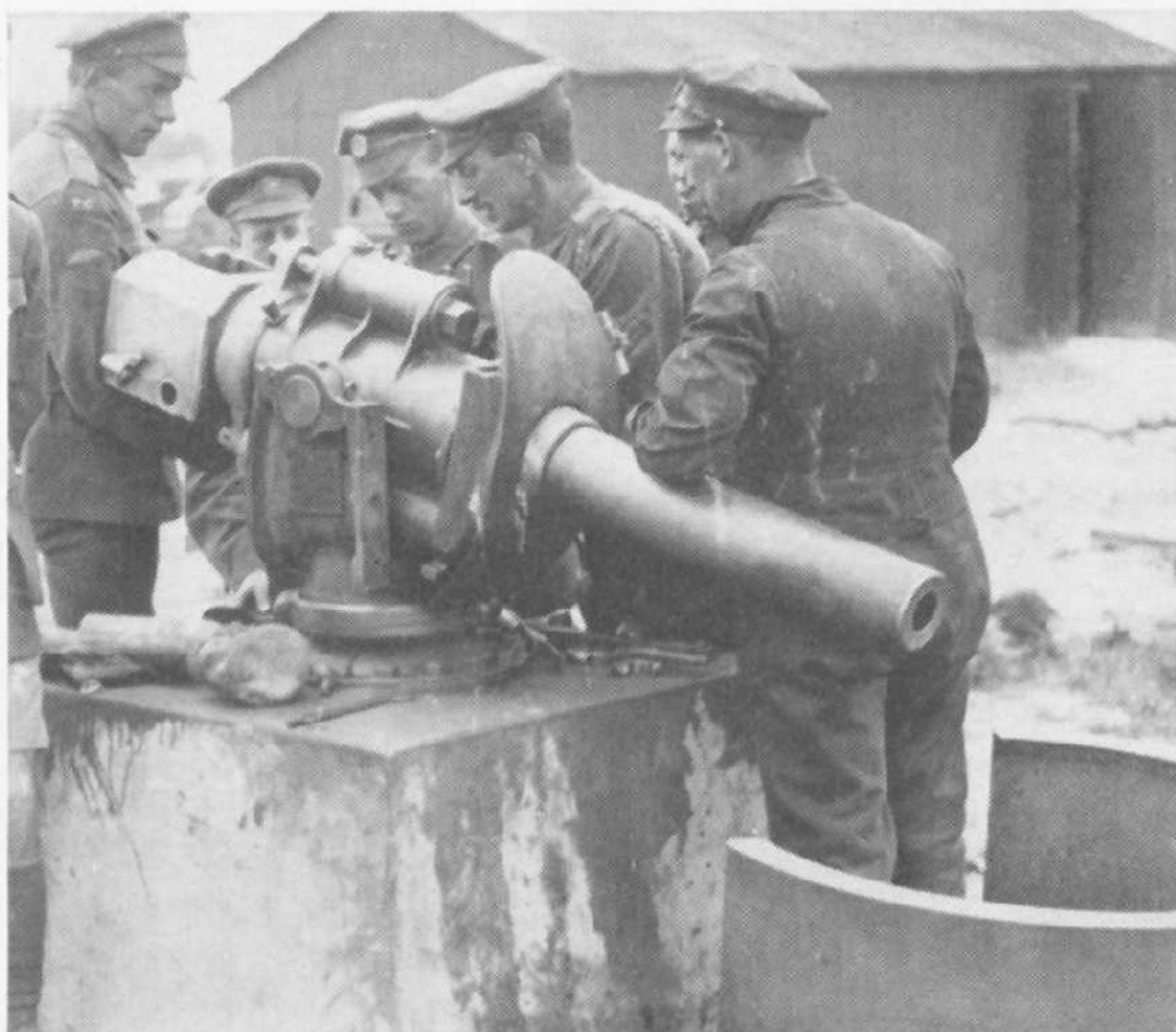
The 23 calibre 6 pdr. Hotchkiss naval gun which formed the main armament of the Mk. IV and V male tanks, seen with tank gunners under instruction. Note Tank Corps Arm Badge on left-hand man. (Imperial War Museum)
