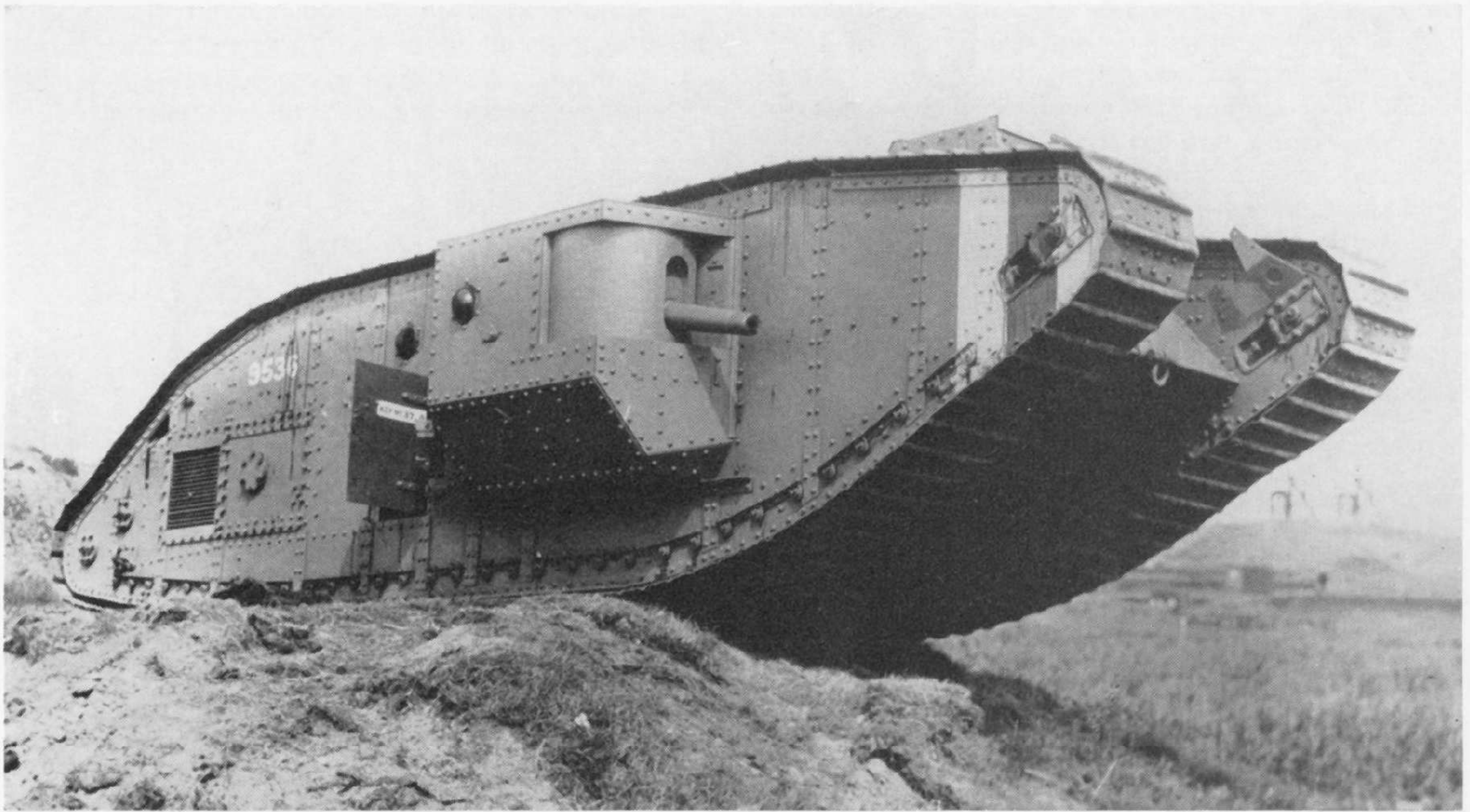
A Mk. V* male complete with recognition stripes. Note side door in lengthened section. The 6 ft. long extension was made up of three additional standard 2 ft. wide side panels.
