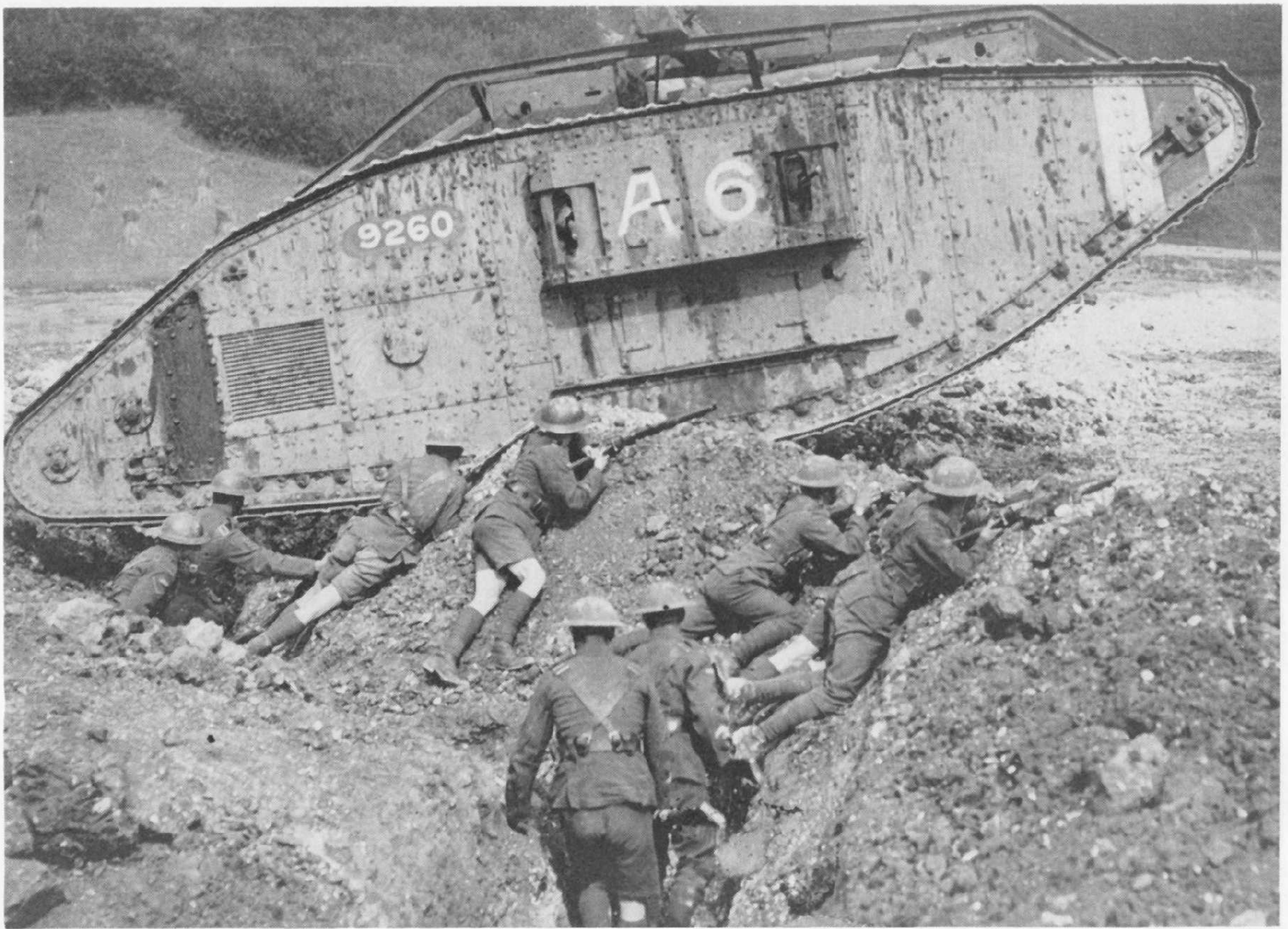
The features of the Mk. V are well shown in this posed "propaganda" picture of a vehicle crossing a British trench, manned for the occasion by Tank Corps men. This Hotchkiss-armed female shows the radiator intake louvres, the rear cupola, and the unditching beam. It is a 1st Battalion (formerly "A" Battalion) vehicle. (Chamberlain Collection)
