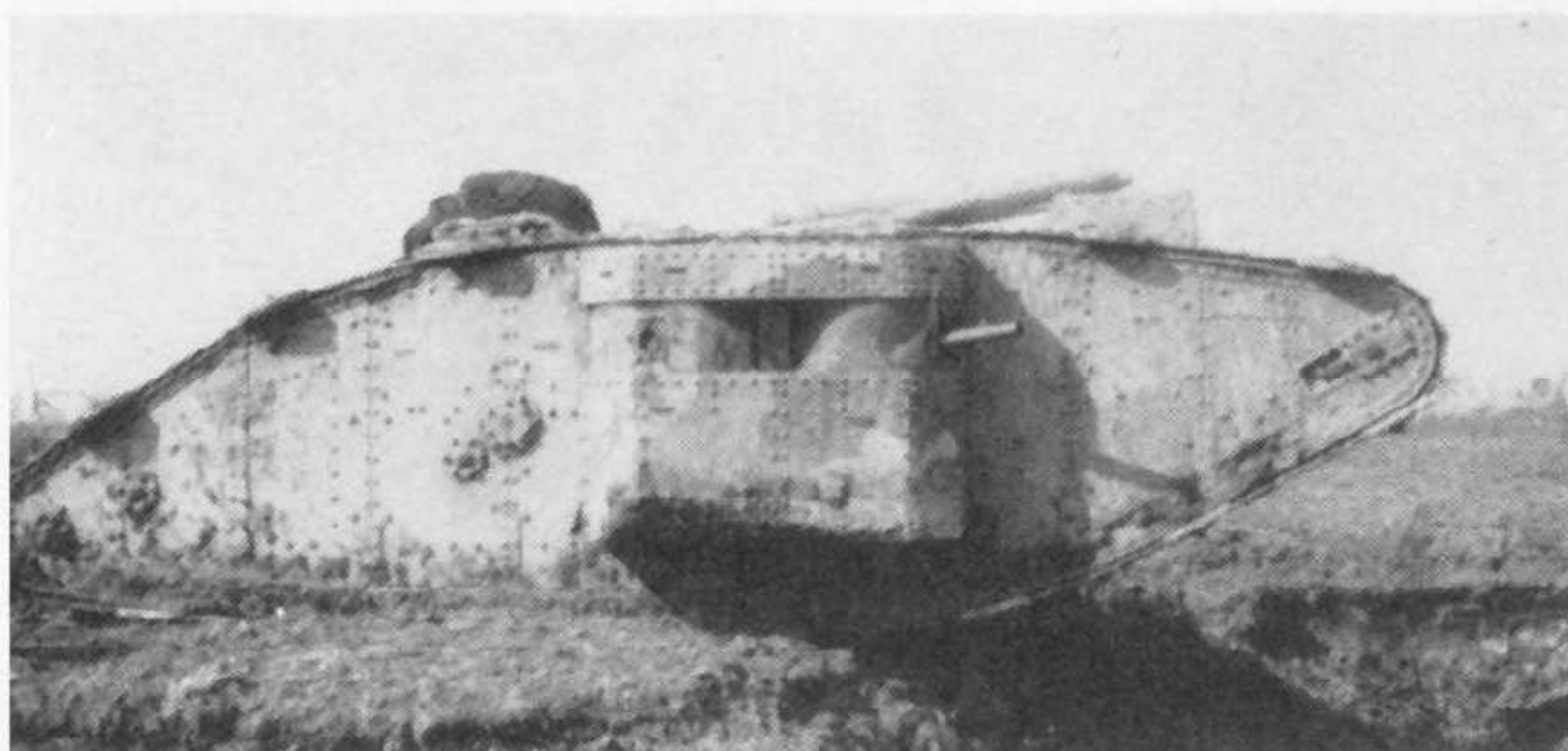
A Mk. II female ("The Perfect Lady") seen during the Battle of Cambrai, on November 20, 1917. The Mk. IV had by this time largely replaced the earlier Marks. (Imperial War Museum)
