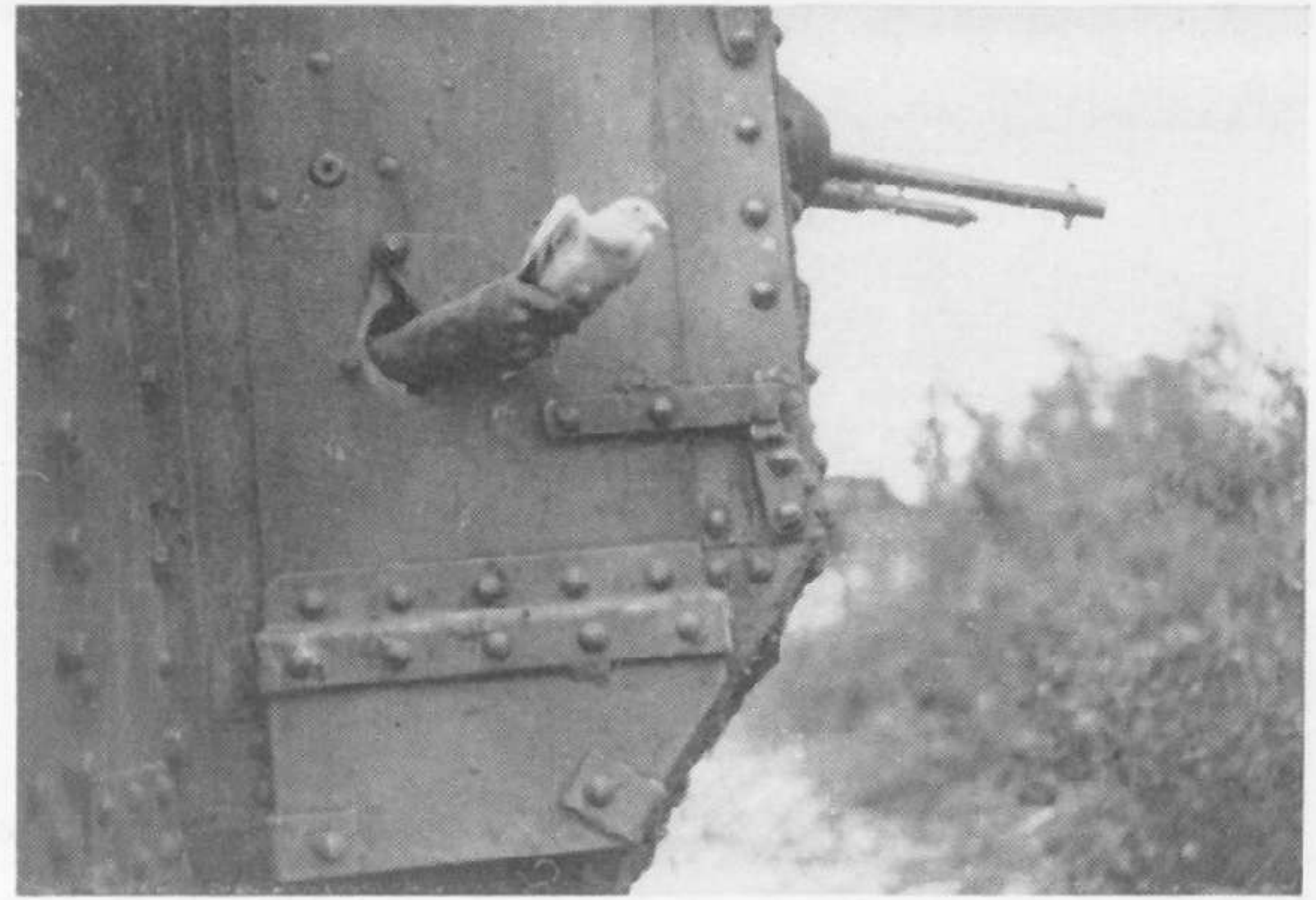
Tank communication: releasing a pigeon from the vision flap in the sponson of a Mk. V tank. Note the Hotchkiss machine-gun in its ball mount. (Imperial War Museum)
