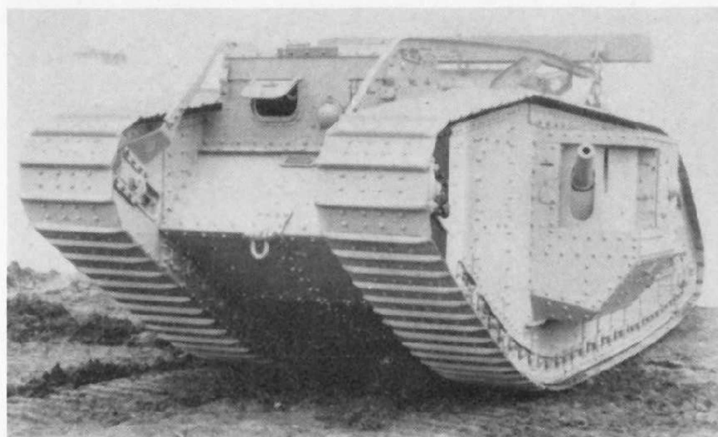
Fine view of a Mk. V male in "mint" condition shows the unditching beam on its rails and the ball mount in the front cupola for the machine-gun.
