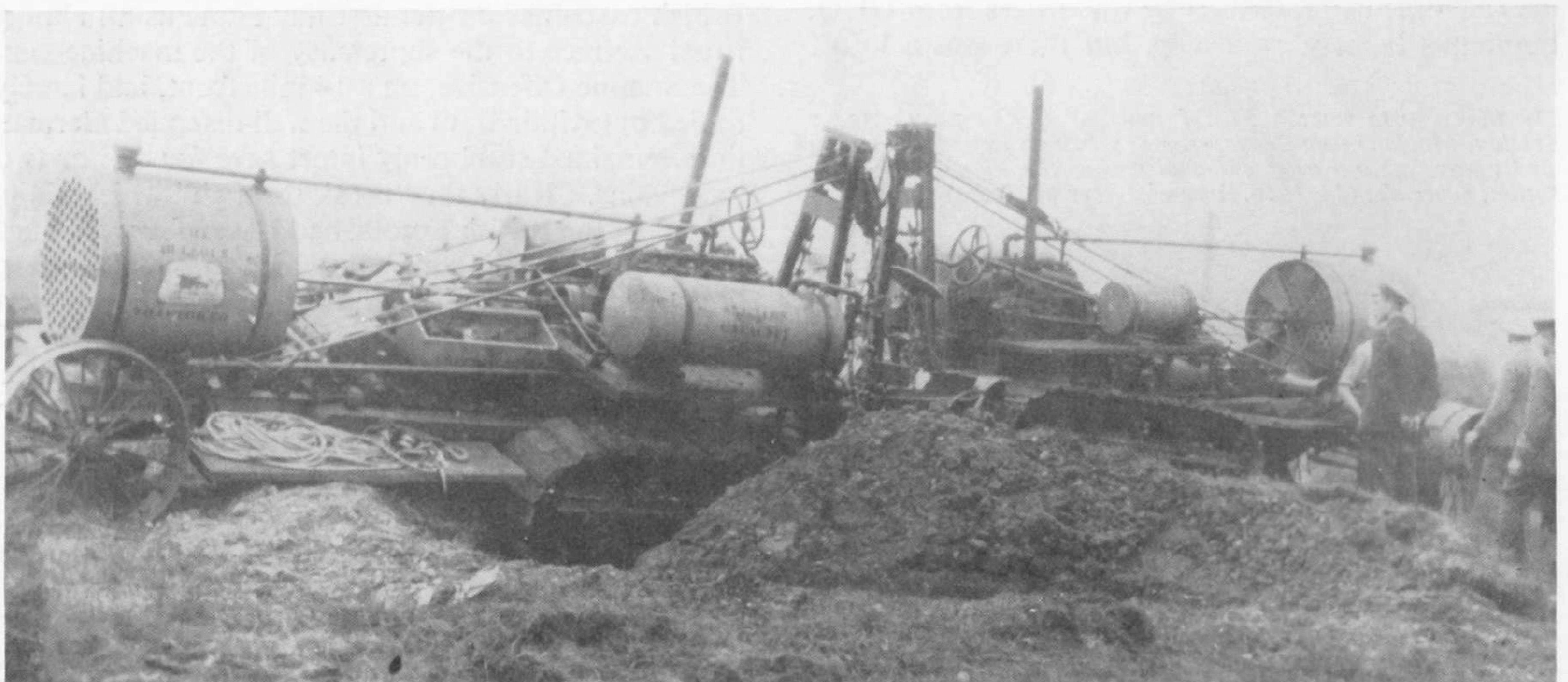
Progenitors of the Tank 2: the two Bullock Creeping Grip tractors which were to form the basis of the projected articulated "landship", seen on test by the RNAS at Burton-on-Trent, July 1915. When this was abandoned, Bullock tracks were used on the experimental "No. 1 Lincoln Machine". (Imperial War Museum)
