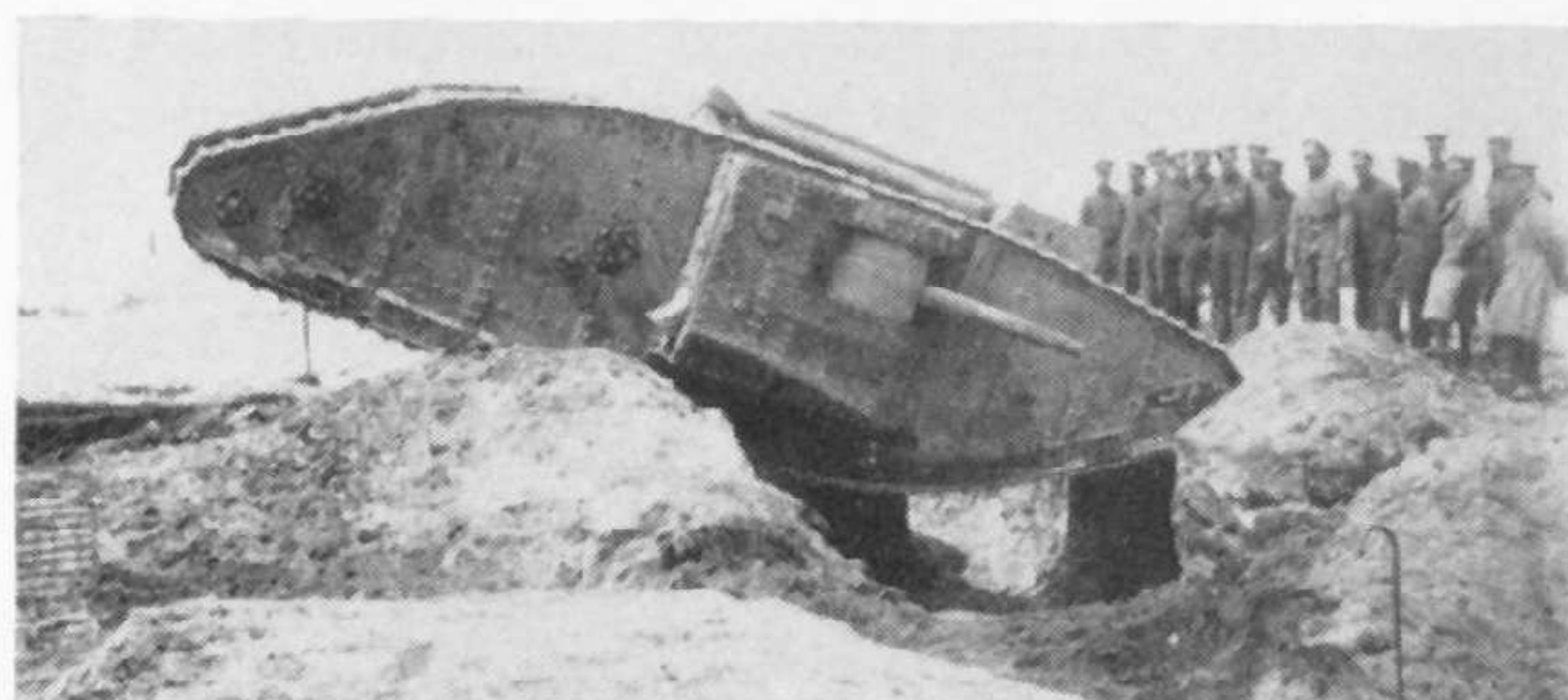
An old Mk. I in use for training at the Tank Corps depot in France in 1917 demonstrates trench-crossing techniques to pupil drivers. (Imperial War Museum)
