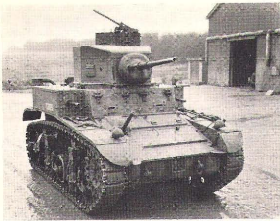
An absolutely standard M3 light tank, Stuart I, with welded turret, showing all the .30 machine-guns in place. Picture taken on delivery of the vehicle to Britain. (Imperial War Museum)
