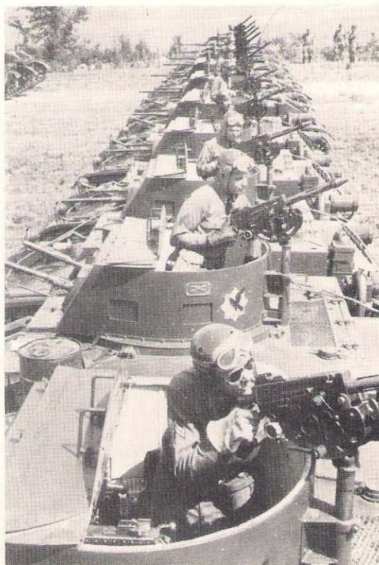
Close view of a company of M1 Combat Cars of 1st U.S. Cavalry in 1939. Note the simplicity of the traversing turret with its vision ports and machine-guns. (Chamberlain Collection)
