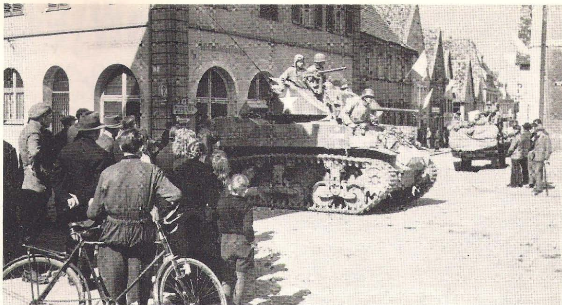
An M5A1 of 43rd Tank Battalion, 12th Armored Div, XXI Corps, 7th Army, accompanies half-tracks (background) into the town of Neustadt, Germany, which has just been surrendered to U.S. forces, April 16, 1945. Armoured fairing over AA machine-gun pintle is clearly shown here. (U.S. Official)
