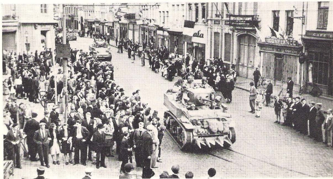
M5A1 light tanks of a U.S. armoured division move through the French village of St Amand to cross the Belgian border, September 1944. Leading vehicle is fitted with “prongs”—the Cullin Hedgerow Device—more usually fitted to medium tanks to cut through hedges and foliage in close country. (U.S. Official)
