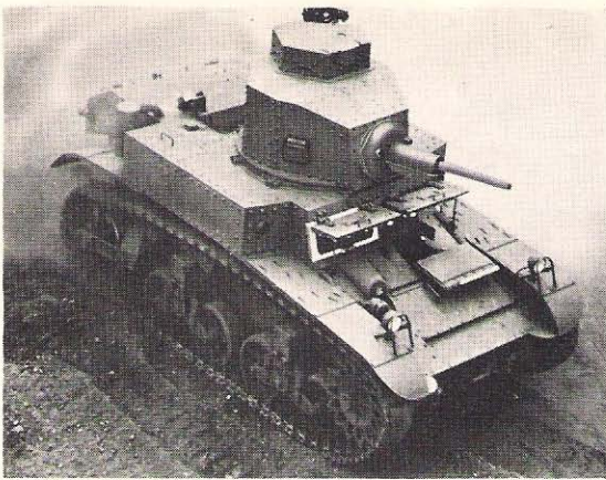
An early production M3 light tank, showing the all-riveted construction. This is an early trials vehicle with the machine-guns not fitted. (Chamberlain Collection)
