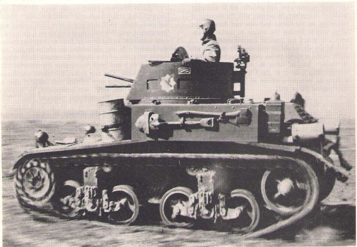
A Combat Car M1 of the U.S. 1st Cavalry Regt, 7th Cavalry Brigade, seen at high speed during 1939 manoeuvres. (Chamberlain Collection)
