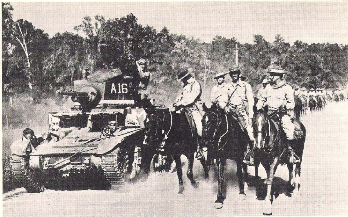
Into the mechanised age; an almost symbolic scene during the U.S. Army Summer exercises of 1940 as a M2A4 light tank of the 7th Cavalry Brigade (Mechanised) overtakes a horsed squadron of the U.S. Cavalry. The M2A4 was the first U.S. tank to be built in quantity in the 1940-45 period. (Chamberlain Collection)
