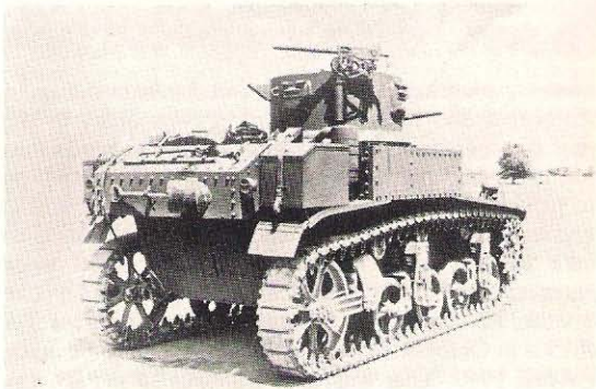
Pilot model of the M3A1 light tank which dispensed with the cupola. Early vehicles still had the riveted hull. (U.S. Official)
