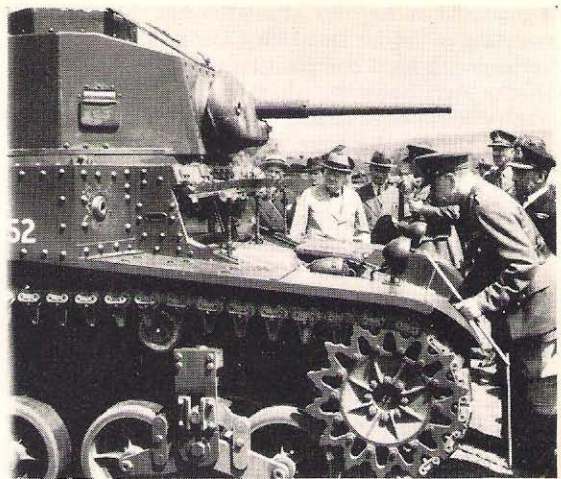
Prime Minister Winston Churchill and Defence Staff chiefs inspect a brand new M3 light tank equipping a U.K.-based armoured division in late Summer 1941. This vehicle has the welded turret. Note driver's vision slit, and the mount for the sponson machine-gun which has been removed. (Imperial War Museum)
