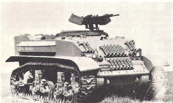
Above and below: Two views of the T8E1 Reconnaissance Vehicle, which was converted from the M5A1 light tank. Note stowage box for carrying landmines on hull side. Same vehicle also has a twin .50 Browning instead of a single mount. (Chamberlain Collection)
