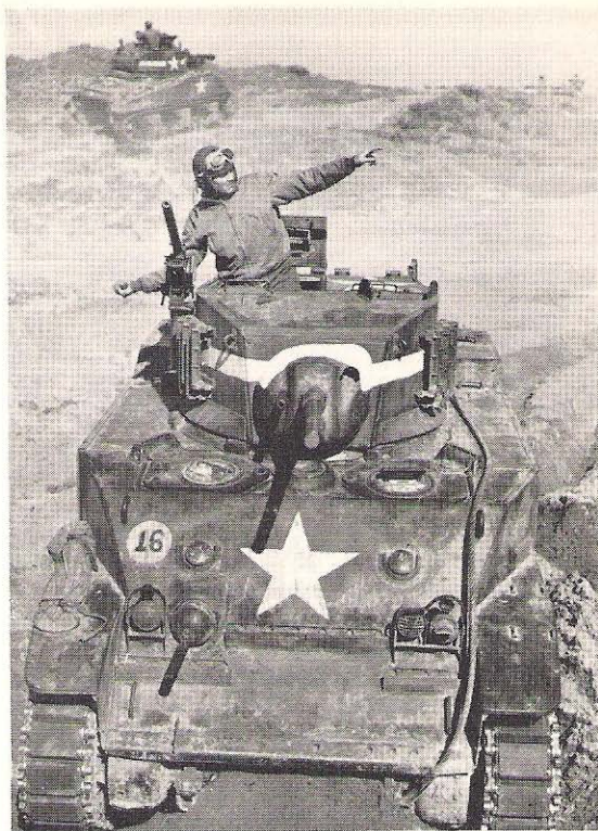
Fine view of a U.S. Army M5A1 (in this case also with the pintle fairing removed) on pre-invasion training exercises in Britain, 1944. Direct sighting telescope aperture is clearly visible to right of mantlet. (Chamberlain Collection)
