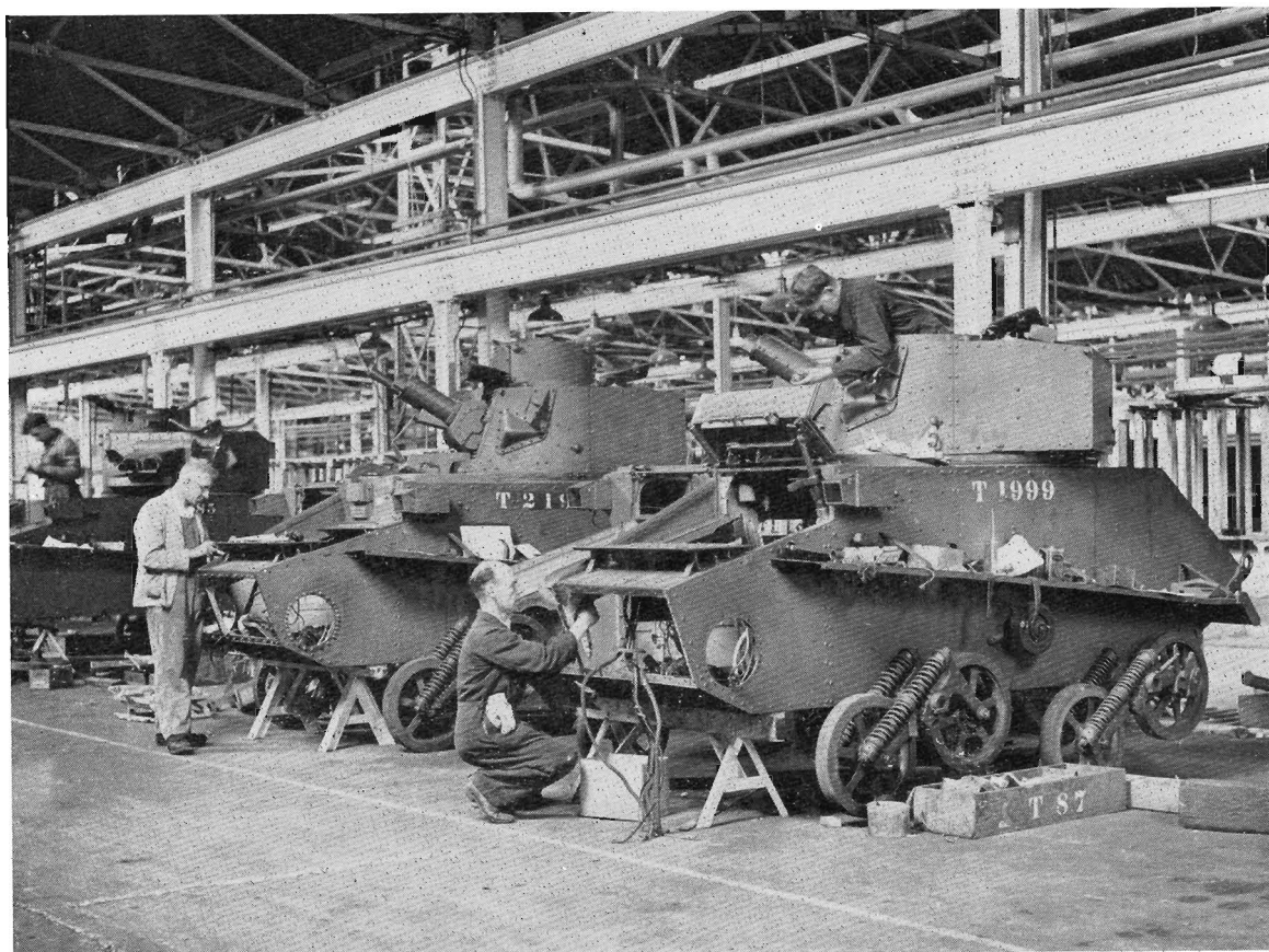
Another view of light tanks, Mk. VIBs in this case, being "re-manufactured" at the MG works, showing the simple lines of the Vickers design. The twin coil springs of the "four pair" Horstmann suspension are clearly shown. (Imperial War Museum)
