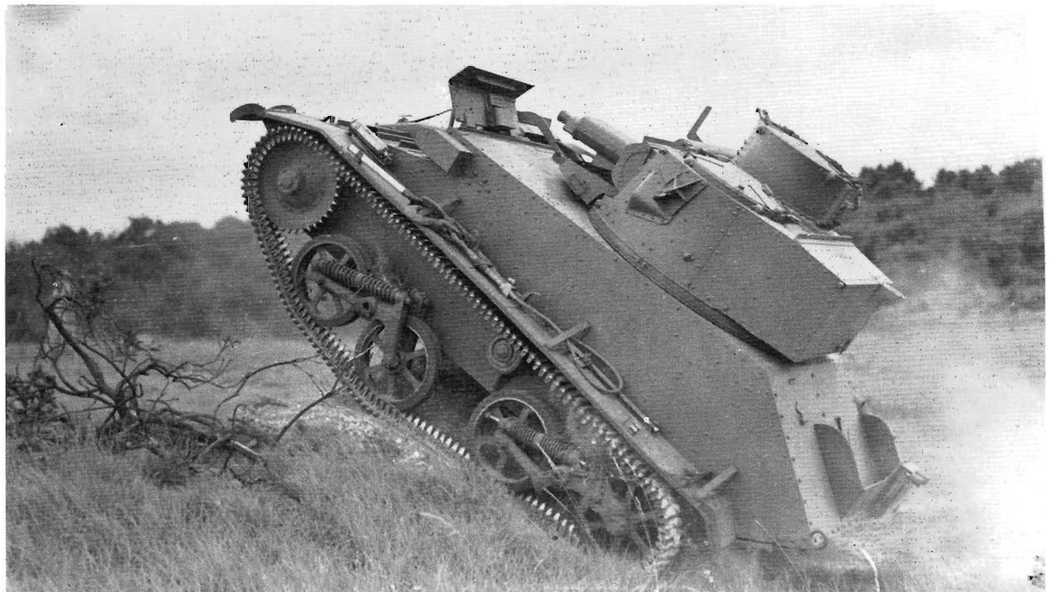
Refurbished vehicles were thoroughly tested before being re-issued "as new" to units. Stowage of the tow rope and tools on the track cover is here shown. (Imperial War Museum)
