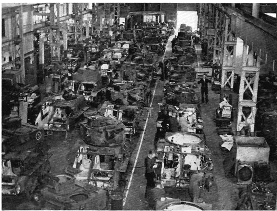
The MG Car Co., Abingdon, Berks., part of the Nuffield Organisation, was responsible for the "re-manufacture" of over 100 light tanks from mid-1940 onwards, refurbished vehicles going initially to armoured divisions in Britain and the Libyan desert and latterly to training units. This general view of the MG assembly shed, summer 1940, shows ex-1st Armoured Division vehicles salvaged from France being stripped and overhauled. (Imperial War Museum)
