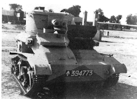
Light Tank Mk. VIB Indian pattern was distinguished from the standard VIB by the absence of the cupola. Some VIBs in Britain were later modified to this standard. (Imperial War Museum)
