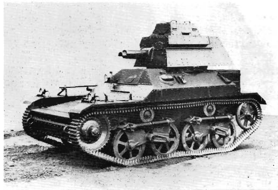
Left: Light Tank Mk. IIA . Note bullet-proofed air louvres on turret and air hatch to engine beyond driver's loop-hole. (RAC Tank Museum.) Right: Light Tank Mk. IIB—Indian pattern with cupola . (RAC Tank Museum)
