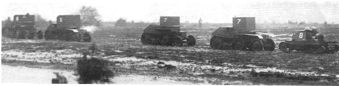
Four Morris-Martels followed by a Carden Loyd marching past, Salisbury Plain, 1929. The Carden Loyd is an original two-man vehicle, very low in build and thus inconspicuous, and armed with a light machine rifle. (RAC Tank Museum)
