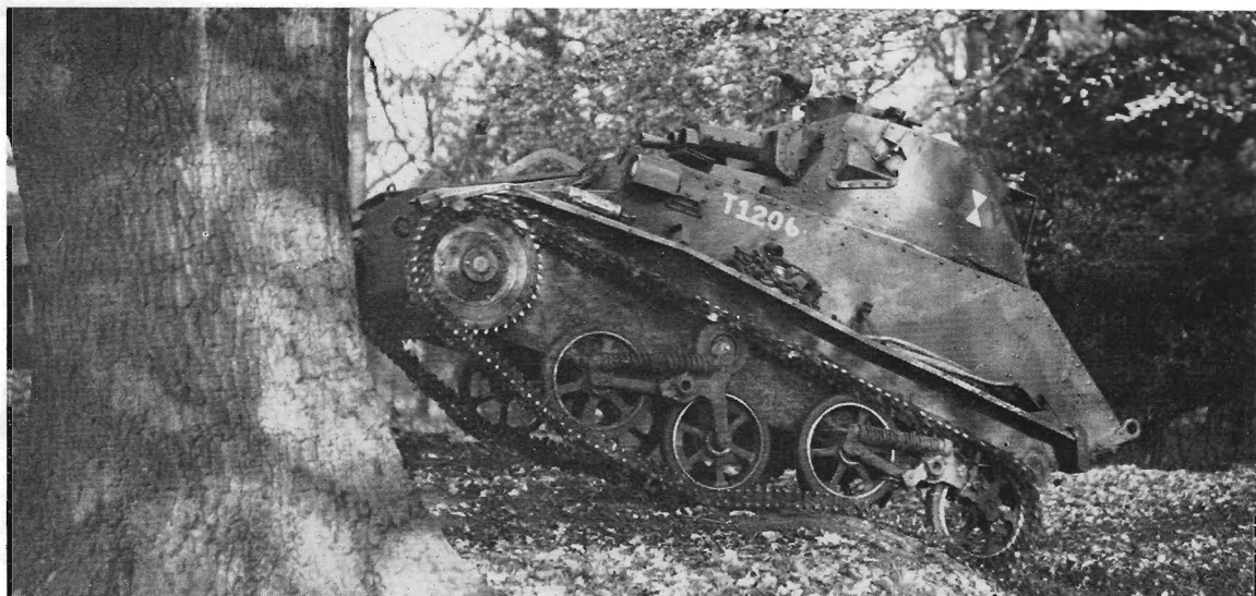
Light Tank Mk. V showing the sloping back turret plate. The return roller on the front bogie (see also the Mk. IVs illustrated) gave continual track trouble, accentuated no doubt by having the rear suspension wheel on the ground which seemed to transmit "shakes" in the top run of the track and make it come off. This tank is being used for training at Catterick, October 1940. (Chamberlain Collection)
