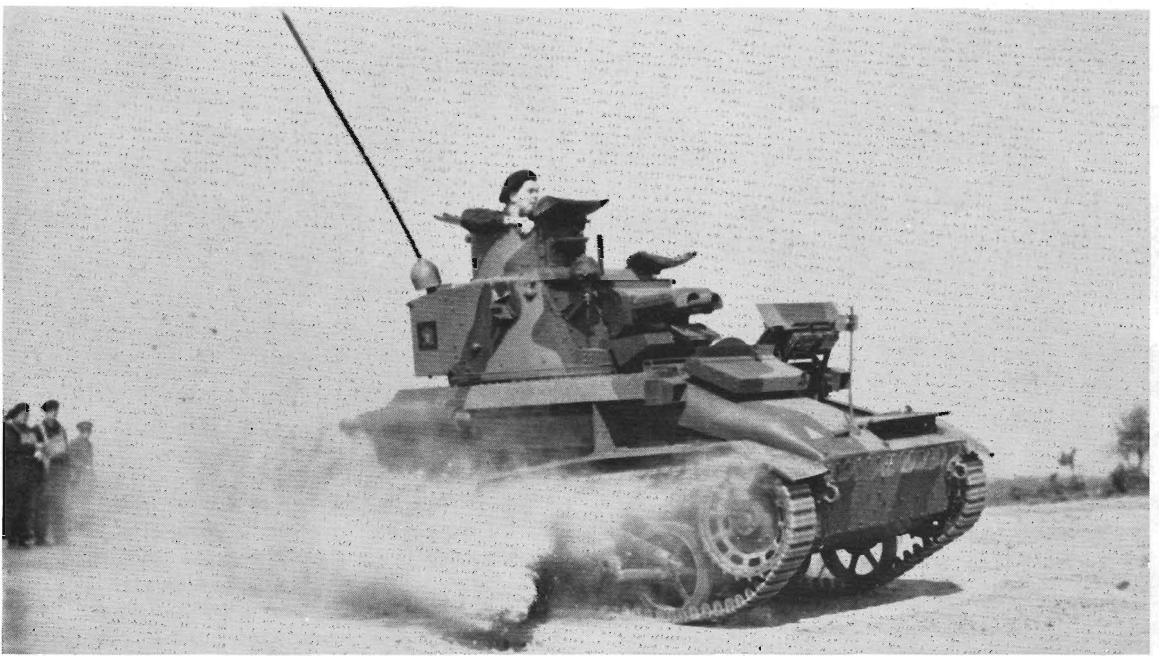
A few Mk. VIs were modified by the provision of larger diameter sprocket wheels, as shown on this VIB at 102nd OCTU, Blackdown, August 1940. The badge painted on the turret below the wireless aerial is of the Westminster Dragoons. (Chamberlain Collection)
