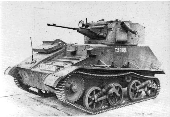
Last of the Vickers light tank models stemming from the Carden Loyd was the Mk. VIC which had a 15 mm. Besa and 7.92 mm. Besa armament. (RAC Tank Museum)
