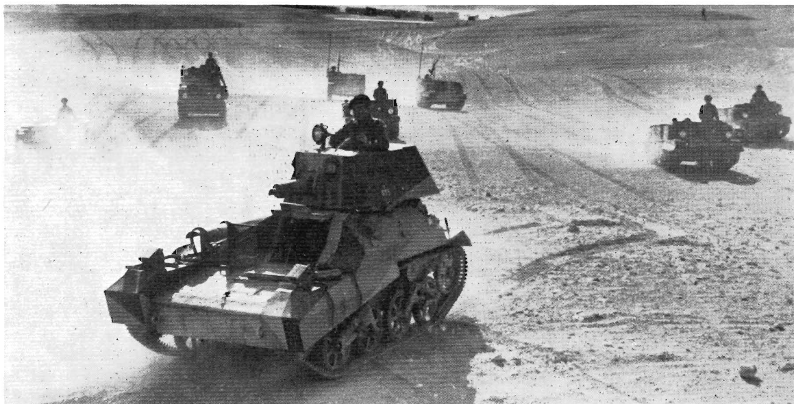
A Light Tank Mk. IIA, with revised Horstmann suspension, and an assortment of Bren Carriers form the motley equipment of an Australian-manned light tank squadron in training in Egypt in summer 1940. (Imperial War Museum)
