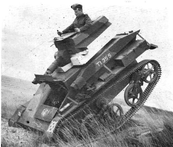
Light Tank Mk. IV in use for training in summer 1940. Note hand-grips for commander (also fitted in Mk. II and III). (Chamberlain Collection)
