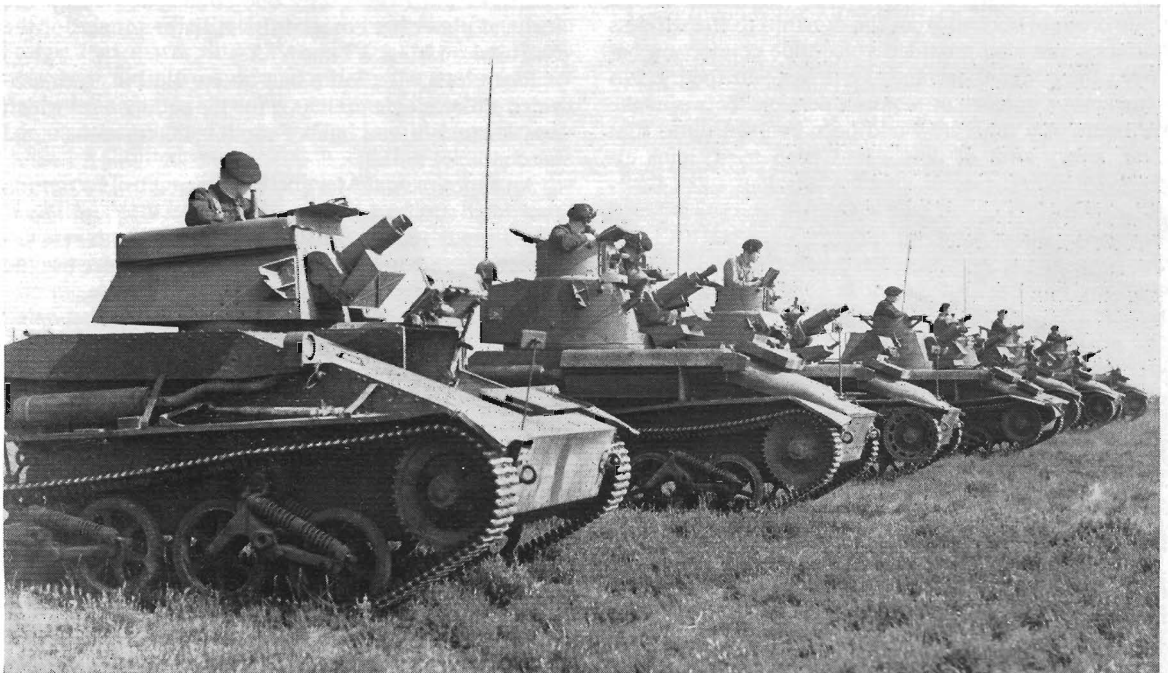
Line up at 102nd OCTU in August 1940 shows some of the external differences between Vickers light tank models. Mk. IV is nearest, then come two Mk. VIBs, then a Mk. V. Note the trays in each case for empty shell cases. (Chamberlain Collection)
