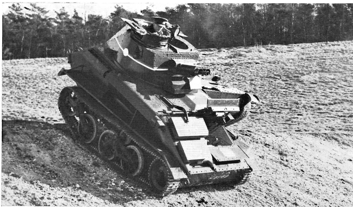
Light Tank Mk. V (with another just behind it) was the model which introduced the longer, deeper hull and a two-man turret with twin machine-gun armament. (Chamberlain Collection)
