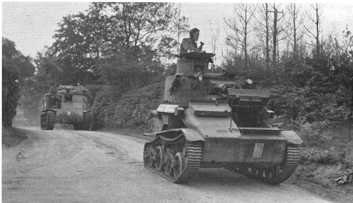
A battered Light Tank Mk. VIB still in use for training seen in company with a Grant in August 1942 at Catterick. The light tank, fitted with No. 19 set, is probably from 51st Training Regiment.
