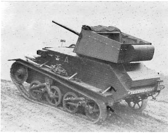
Left: Based on the Mk. V, this experimental "tank destroyer" model with 2 pdr. gun developed by Vickers was tested by the army in 1938 but never went into production. (Imperial War Museum.) Right: A fine view of a Light Tank Mk. VIB showing all the standard fittings of the 1939 period, including spotlight on turret, smoke discharger, and headlights in armoured housings.
