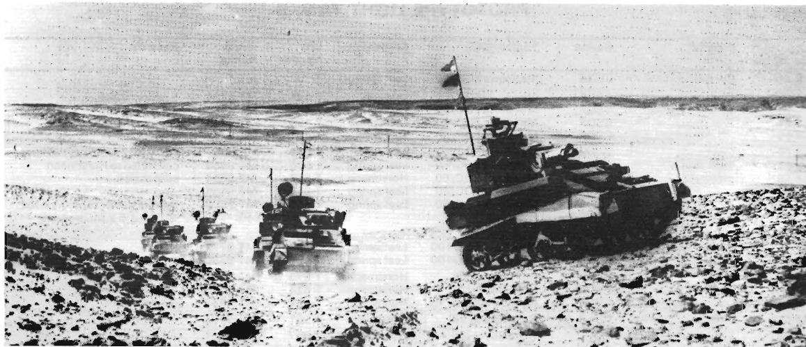
Mk. VIBs in the Western Desert, 1940. Sandshields have been fitted over front of tracks.
