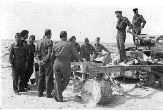
Valentine with Anti-Mine Roller Attachment Mk. 1B. The equipment has been damaged in exploding a mine. (Imp. War Mus.)
