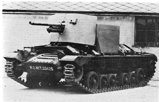
Self-propelled 6 pdr. mounting on Valentine I—experimental only. (RAC Tank Mus.)
