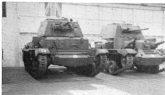
Cruiser Mark IIA CS (left) in the R.A.C. Tank Museum, Bovington, Dorset. The 3.7 in. howitzer of the close support tank can be compared with the 2 pdr. (40 mm.) gun of the A.9 alongside. (B. T. White.)
