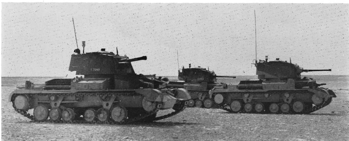
Cruiser Mark I CS (left) and two Cruiser Mark IIAs on patrol in the Western Desert in 1940. This picture brings out the chief external differences between the A.9 and the A.10, including the engine air louvres. (Imp. War Mus.)
