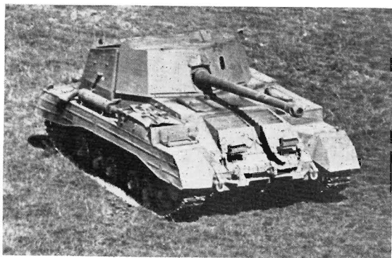
Rear view of an Archer. Note how engine air louvres differ from those of the Valentine tanks. (Imp. War Mus.)
