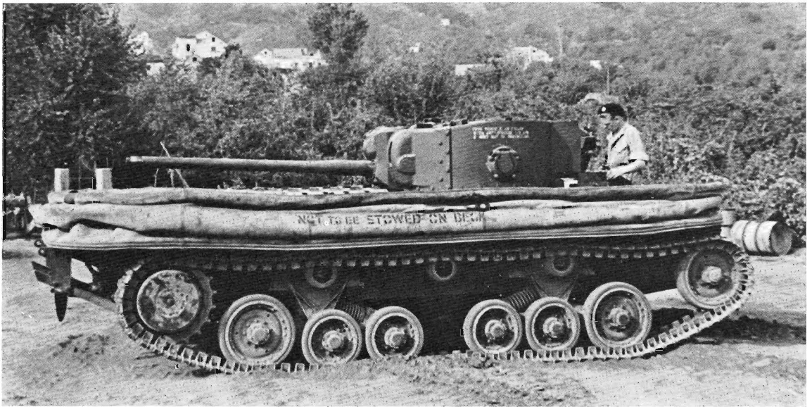
Valentine IX DD tank with the flotation screen folded. (Imp. War Mus.)
