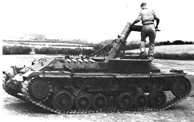
Valentine with a 9.75 in. mortar mounted in the fighting compartment. This mortar fired a combustible projectile. Experimental vehicle only. (Imp. War Mus.)
