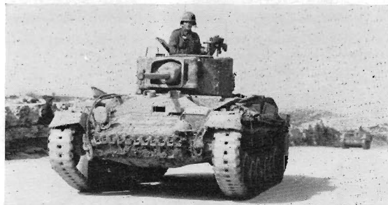
Left: Valentine IV. This Mark was externally identical to the AEC-engined Valentines I and II. (B. T. White.) Right: Valentine V in Tunisia, January 1943. Note the Bren gun with drum magazine mounted on the turret for anti-aircraft use. (Imp. War Mus.)
