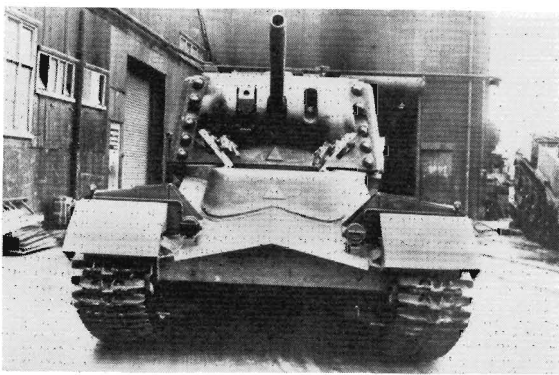
Valiant—front view. Note inverted-V top surface of cast nose plate. (Imp. War Mus.)
