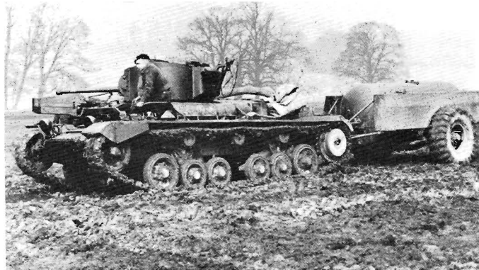
Valentine with gas pressure system flamethrower. This experimental vehicle, built by A.E.C. Ltd. in conjunction with the Petroleum Warfare Department, formed the basis of the later Crocodile flamethrower system. (Imp. War Mus.)
