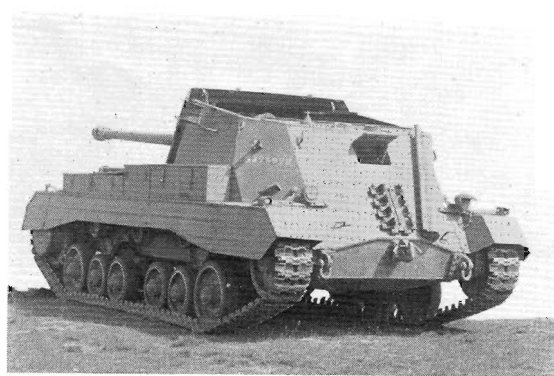
Front view of S.P. 17 pdr., Valentine—an Archer. Note spare track plates, the front towing hook and the cable bracket on the right-hand side of the hull. (Imp. War Mus.)
