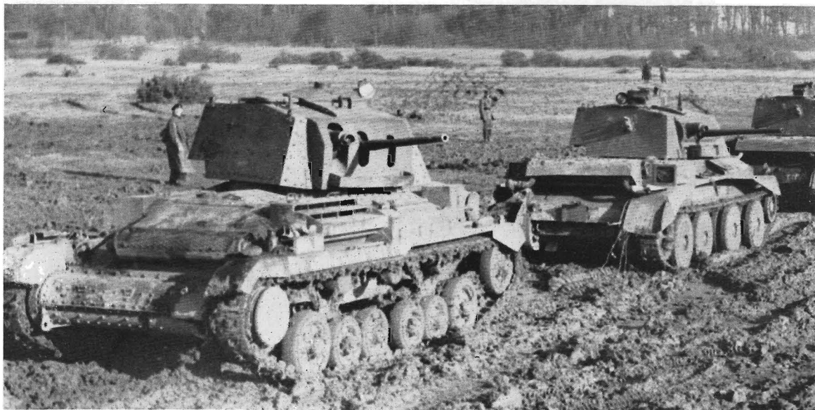
An A.10 with 2 pdr. gun and coaxial Vickers machine-gun in the turret. On the right is an A.13, a Cruiser Mark III. (Imp. War Mus.)
