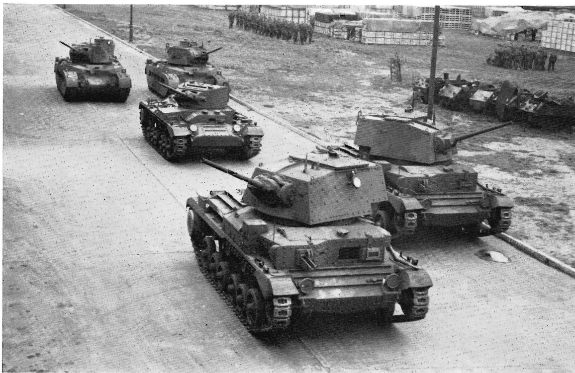
Two Cruiser Mark IIAs followed by a Valentine. The similarities and the differences between the two types are apparent in this view. In the rear are two Matildas, Infantry Tank Mk. II. (Imp. War Mus.)
