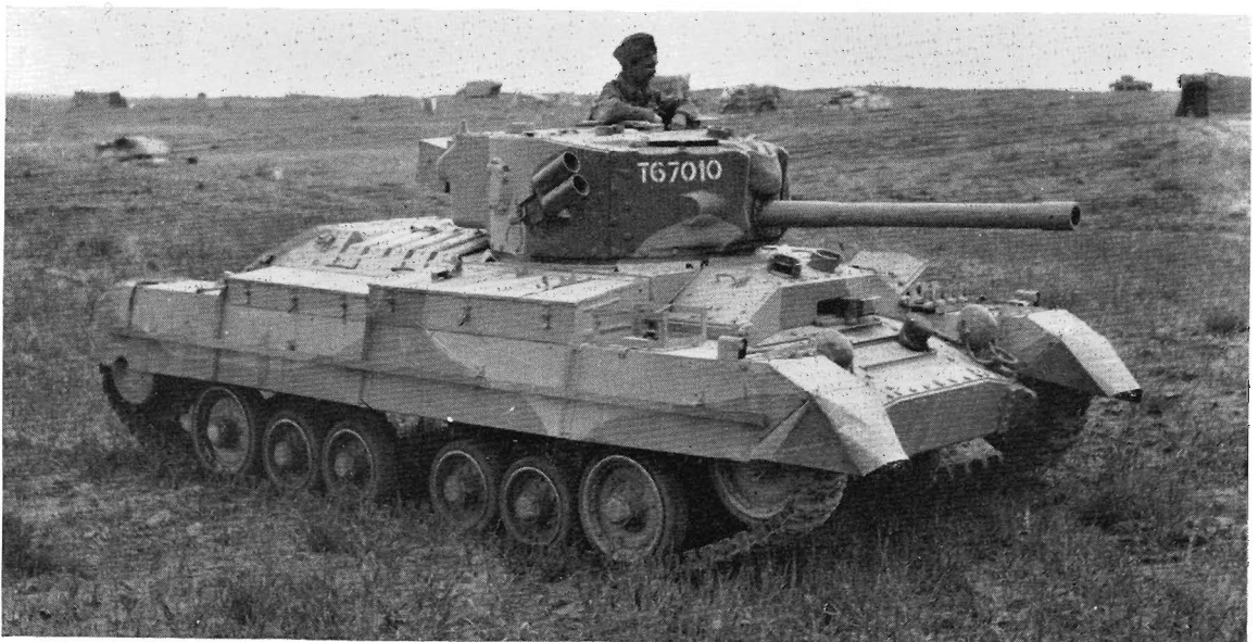
Valentine VIII—the Mark IX was externally identical and had the same turret armament of a 6 pdr. without a coaxial machine-gun. This tank is equipped with two 4 in. smoke dischargers mounted on the side of the turret. (Imp. War Mus.)
