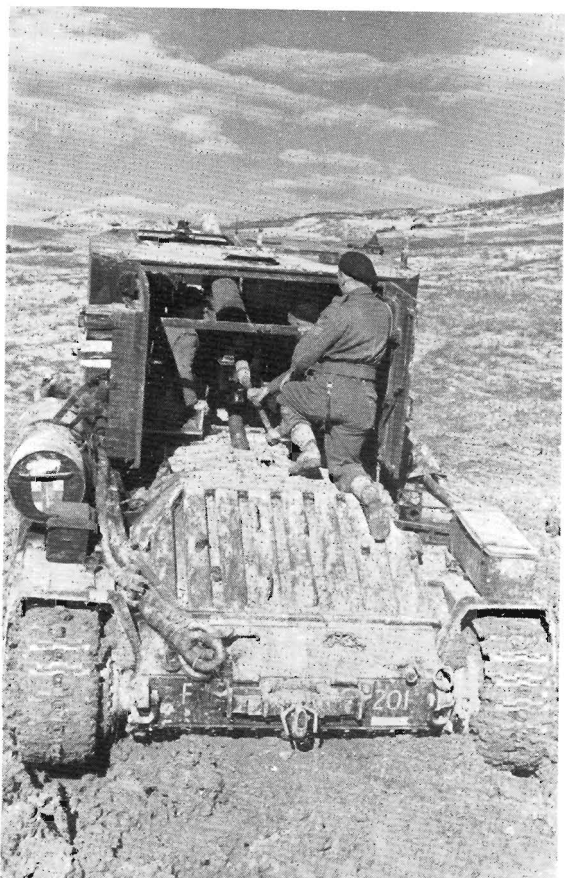
Rear view of a Bishop. Note towing hook, used for towing 25 pdr. field artillery limber. (Imp. War Mus.)
