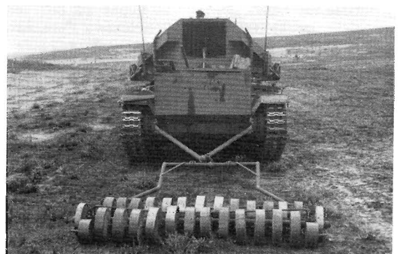
Left: Valentine Scorpion flail tank. Right: Valentine Scorpion towing a Centipede for dealing with anti-personnel mines. (Imp. War Mus.)
