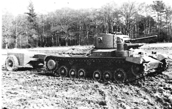
Valentine with cordite-operated flamethrower—experimental vehicle built by the Ministry of Supply. (Imp. War Mus.)
