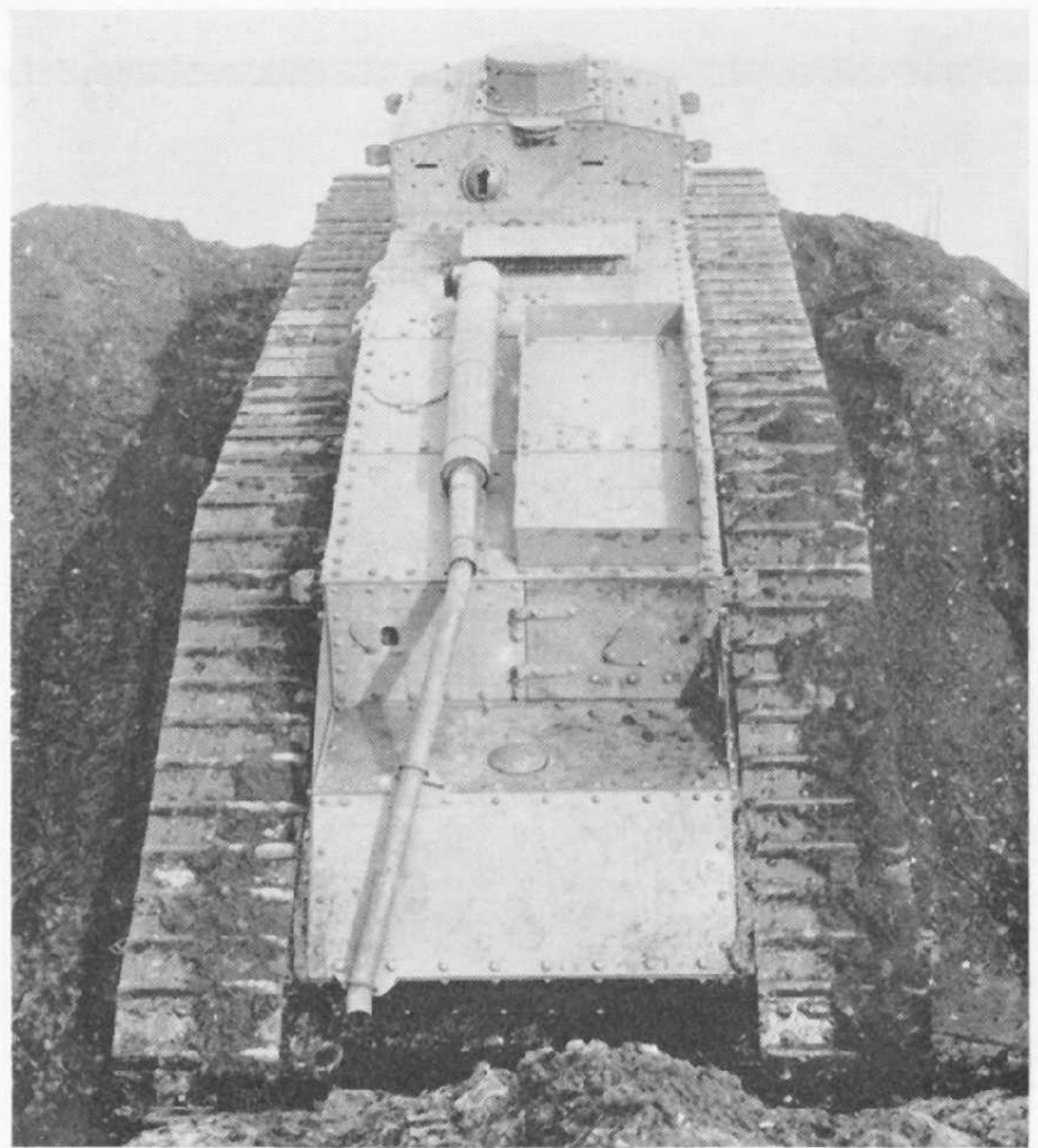
Medium C top decking. Armoured fuel tank is between rear horns and the panel with the radiator grille was a complete one-piece assembly. (Imperial War Museum)
