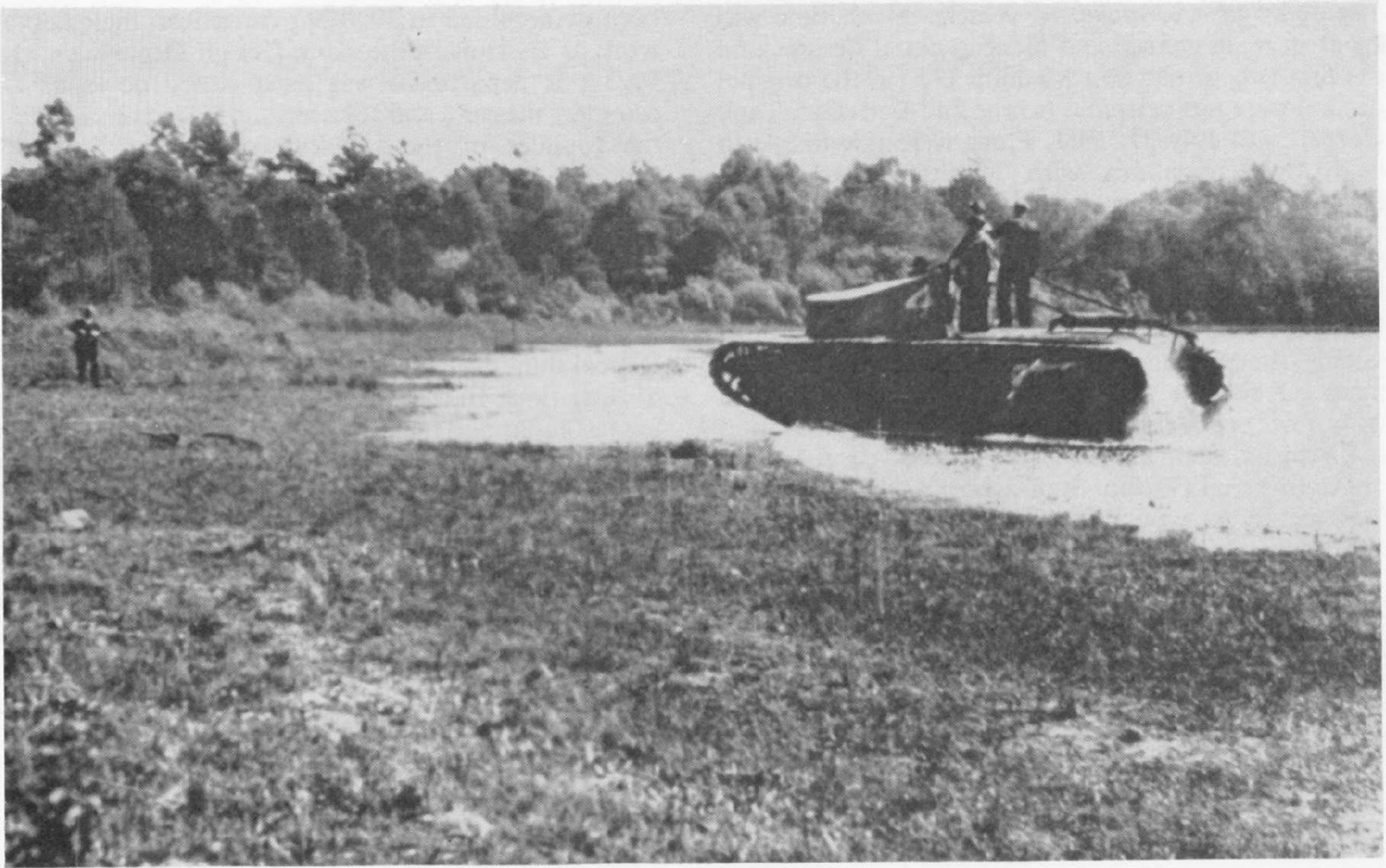
Rare picture of Johnson's Light Infantry Tank on amphibious trials in Fleet Pond, near Aldershot, 1922. (R.A.C. Tank Museum)
