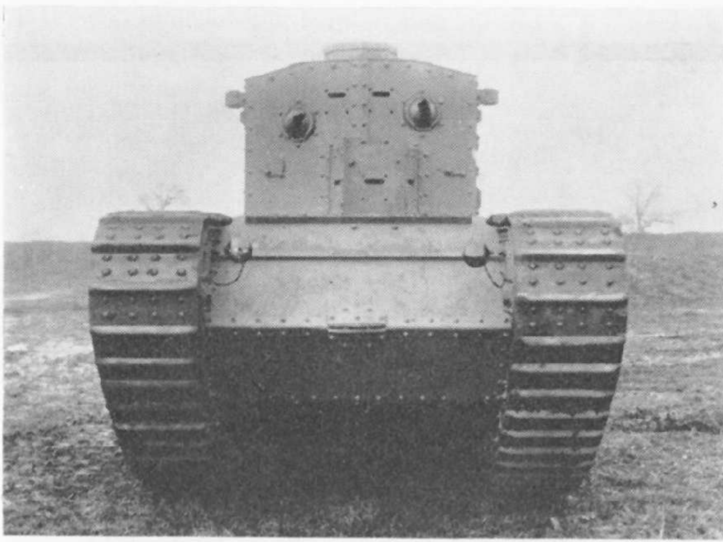
Medium Mark C from front shows disposition of ball-mounts for guns and the numerous vision slots and pistol ports. Note also the refinement of hooded electric headlights. (Imperial War Museum)
