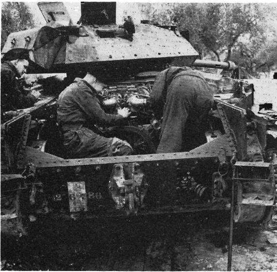
Repairs to a Crusader III of 6th Armoured Division in Tunisia. Holders for smoke dischargers, known as rear smoke emitters, can be seen on each side. This tank mounts a substantial towing hook. (I.W.M.)
