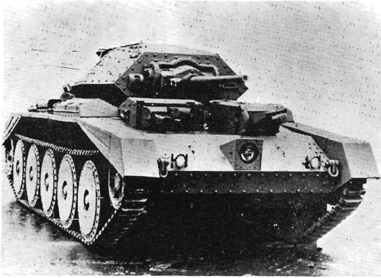
Crusader prototype which mounted a Besa machine-gun in the front of the driver's hood. This gun was removed and a revolver port fitted in place. (R.A.C. Tank Museum)
