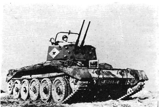
Crusader III AA Mark II, with twin 40 mm. Oerlikon. The sign on the turret is that of a trials establishment. (R.A.C. Tank Museum)
