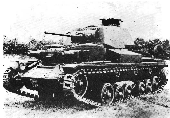
The A9 E2, mounting Vickers MGs in two forward sub-turrets. (R.A.C. Tank Museum)
