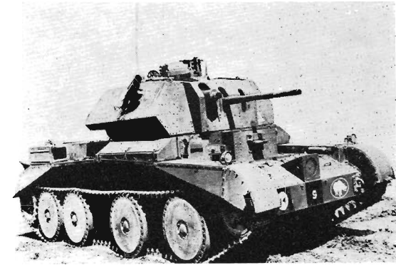
A13, Mark II, Cruiser Mark IV, the up-armoured version of A13 with spaced armour on the turret. This mark carries the Vickers machine-gun. (I.W.M.)
