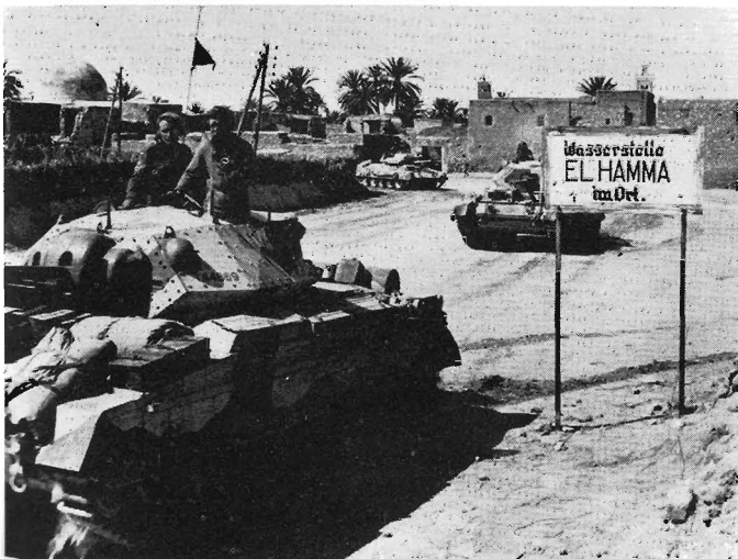
Crusader II followed by Crusader III advancing in Tunisia with Eighth Army, near the end of the Battle of Mareth, March 19-29, 1943. These are tanks of the 9th Queen's Royal Lancers, 1st Armoured Division. (I.W.M.)
