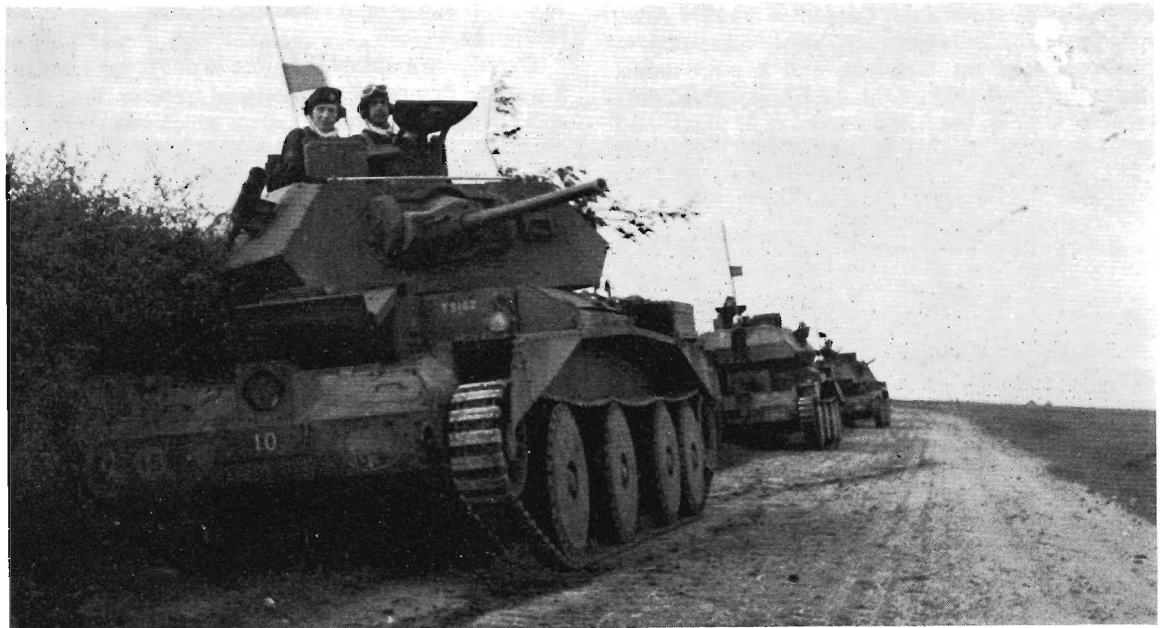
A13s, Mk IIA, of the 5th Royal Tank Regiment taking cover beside a hedge in France, 1940. On the side of the turret are the smoke dischargers which projected a 4-inch smoke canister about 150 yards. The furthest tank is a Mk I, without the extra armour on the turret. Mk IIA mounted the Besa machine-gun. (I.W.M.)
