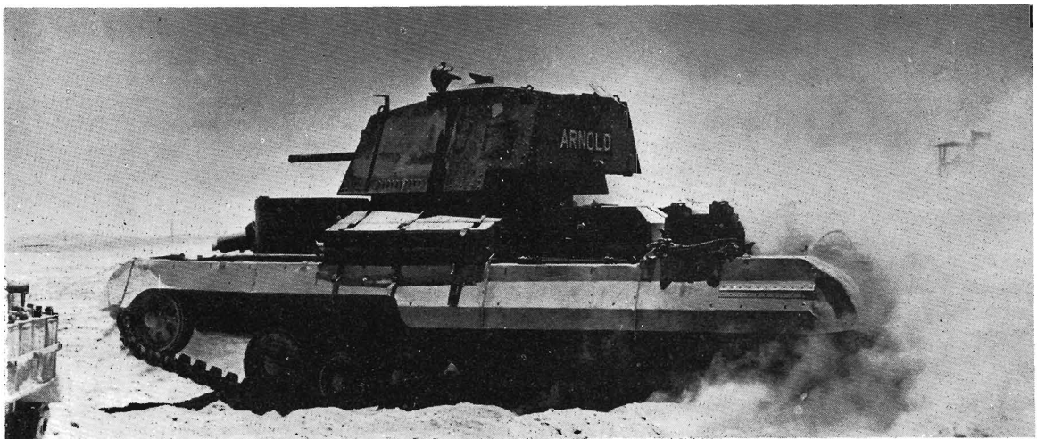
An A9 of the 1st Royal Tank Regiment in Egypt in 1940, with sand guards over the tracks for desert operations. (I.W.M.)
