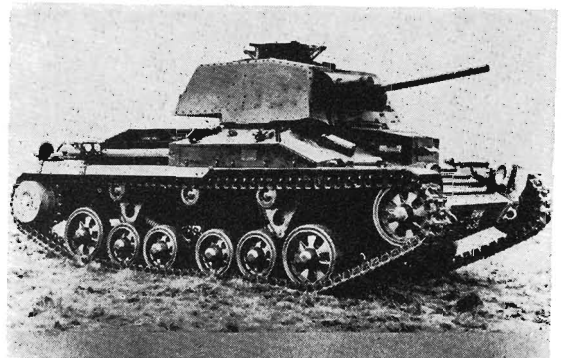
The A10 E1, with dummy guns in the turret and no place for any machine-gun in a hull mounting. (R.A.C. Tank Museum)
