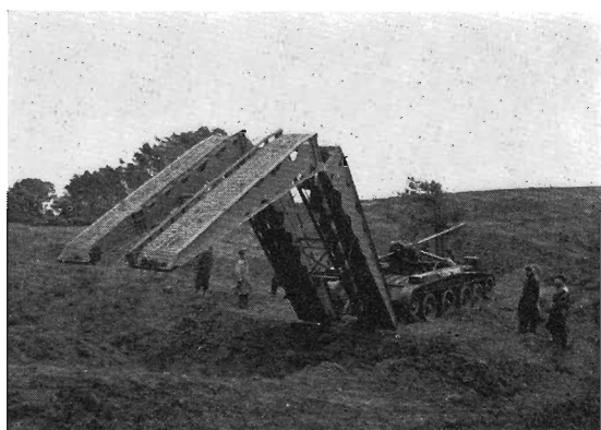
The Covenanter III Bridgelayer could lay, and recover, its Scissors Bridge over a 30 ft. gap for a tracked vehicle load of 30 tons. (I.W.M.)
