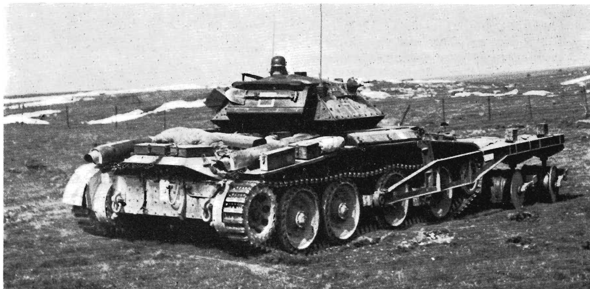
The Anti-Mine Roller Attachment, mounted here on a Covenanter, consisted of a framework carrying spring-mounted and castoring rollers wide enough to cover the track path of the tank. (I.W.M.)
