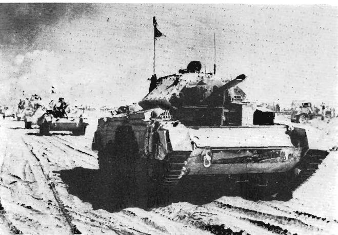
Crusader II Close Support in a tank column with Shermans moving up at El Alamein. This tank has had extra armour plates bolted on the glacis and nose plates, an unusual addition. (I.W.M.)
