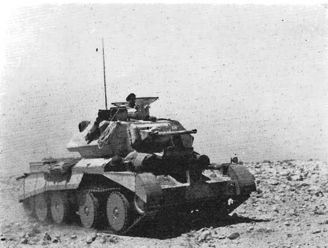
An A13, Mk IIA, of the 2nd Royal Tank Regiment in the desert. A later version with an external gun mantlet. (I.W.M.)
