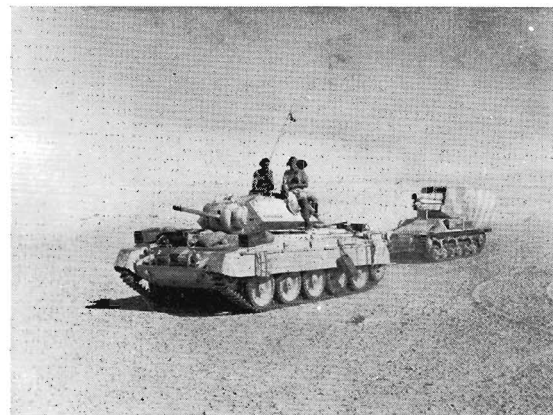
A Crusader I towing a captured SP 15 cm. howitzer Lorraine Schlepper (SdKfz 135/1), a German conversion of the French Lorraine tractor. (I.W.M.)
