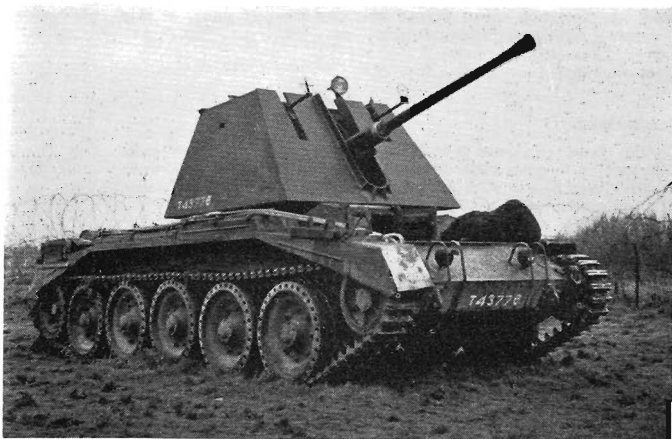
Crusader III AA Mark I with 3-man crew, mounting the 40 mm. Bofors gun, used by light anti-aircraft artillery units. Normally operated by hydraulic power in traverse and elevation by joystick from the gunlayer's seat. (I.W.M.)
