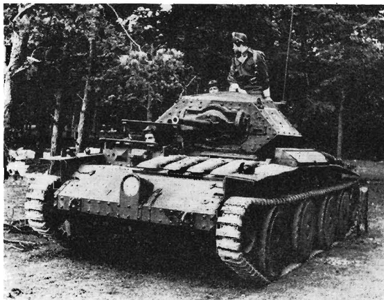
A Covenanter I, in which the crew are wearing the protective helmet introduced in the early part of the war but which was seldom, if ever, worn in action. (I.W.M.)
