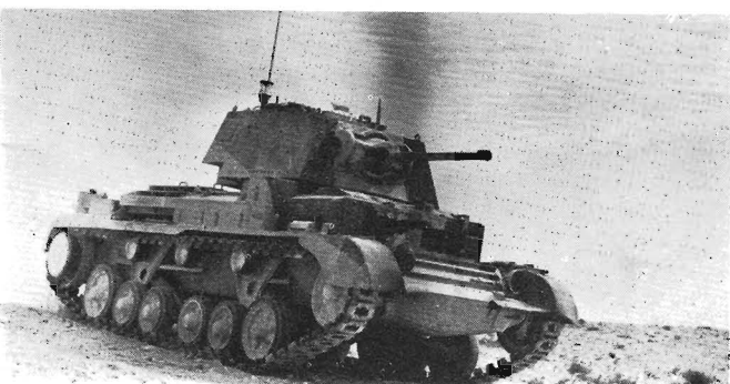
The A10 in desert camouflage. The signalling lamp raised through the roof was similar to one mounted on the Matilda infantry tank. (I.W.M.)
