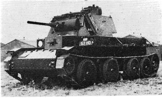
A13 E2, with a heavier hull than the original Christie 1932 prototype, but running on the same type of track. (R.A.C. Tank Museum)
