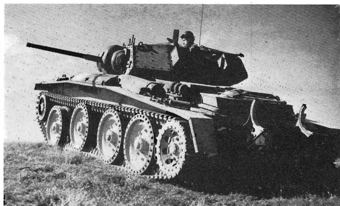
Covenanter IV in September 1942, showing air vents in the hull side below the track guard. The air louvres were similar to those on Mark III but the front stowage bins were removed and others mounted on the turret sides. (I.W.M.)
