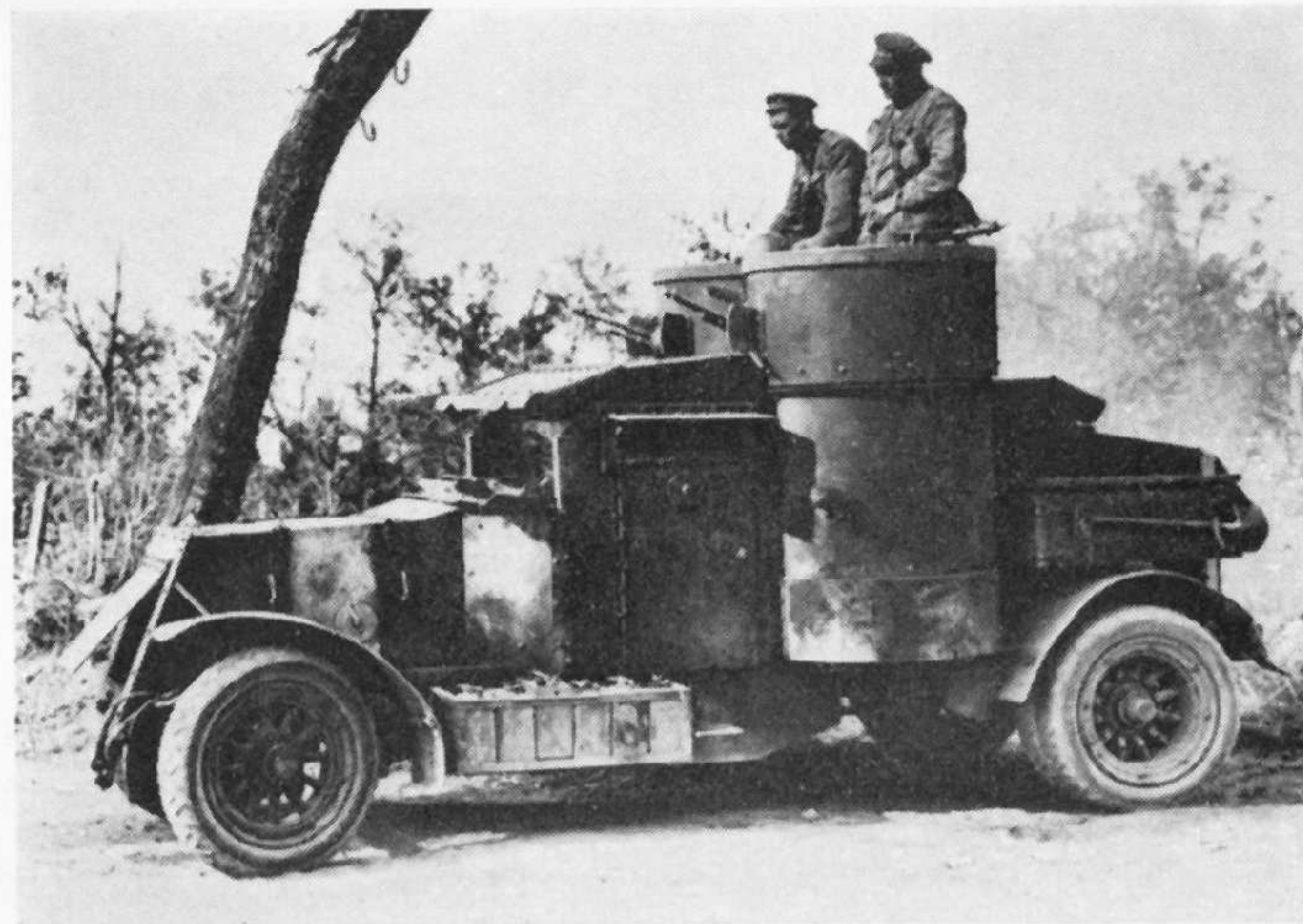
Austin of 17th (Armoured Car) Bn. Tank Corps. The height of the driver's cab has been lowered giving wider traverse to the two Hotchkiss machine-guns. (R.A.C. Tank Museum)
