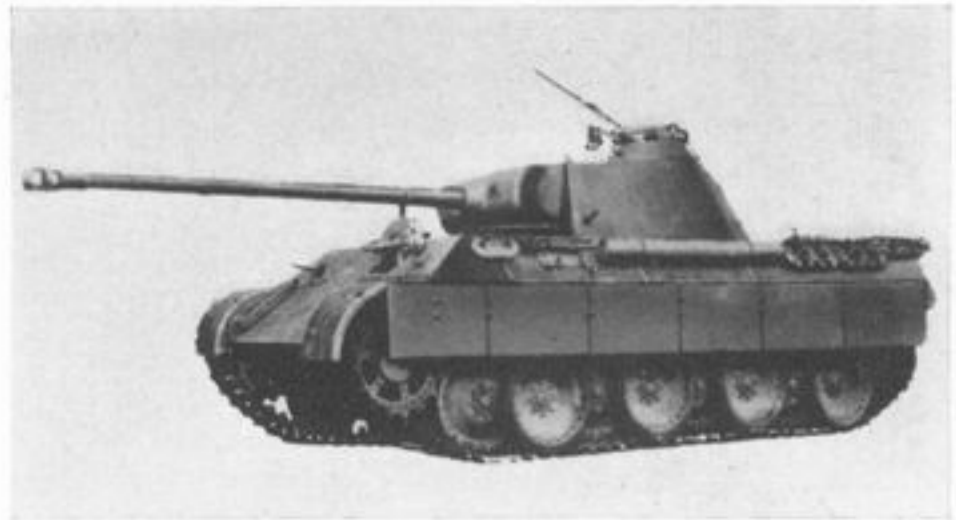
Panther Ausf A had a ball mount for the hull machine-gun and the later type of cupola which featured a ring mount for an AA machine-gun. (IWM)
