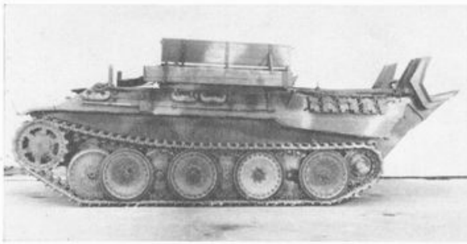
Above and Right: The Bergepanzer Panther (Panther ARV) was an important special purpose type with winch and recovery gear. The earth anchor was raised and lowered from the winch. The light jib could be erected either side for lifting components. (IWM)
