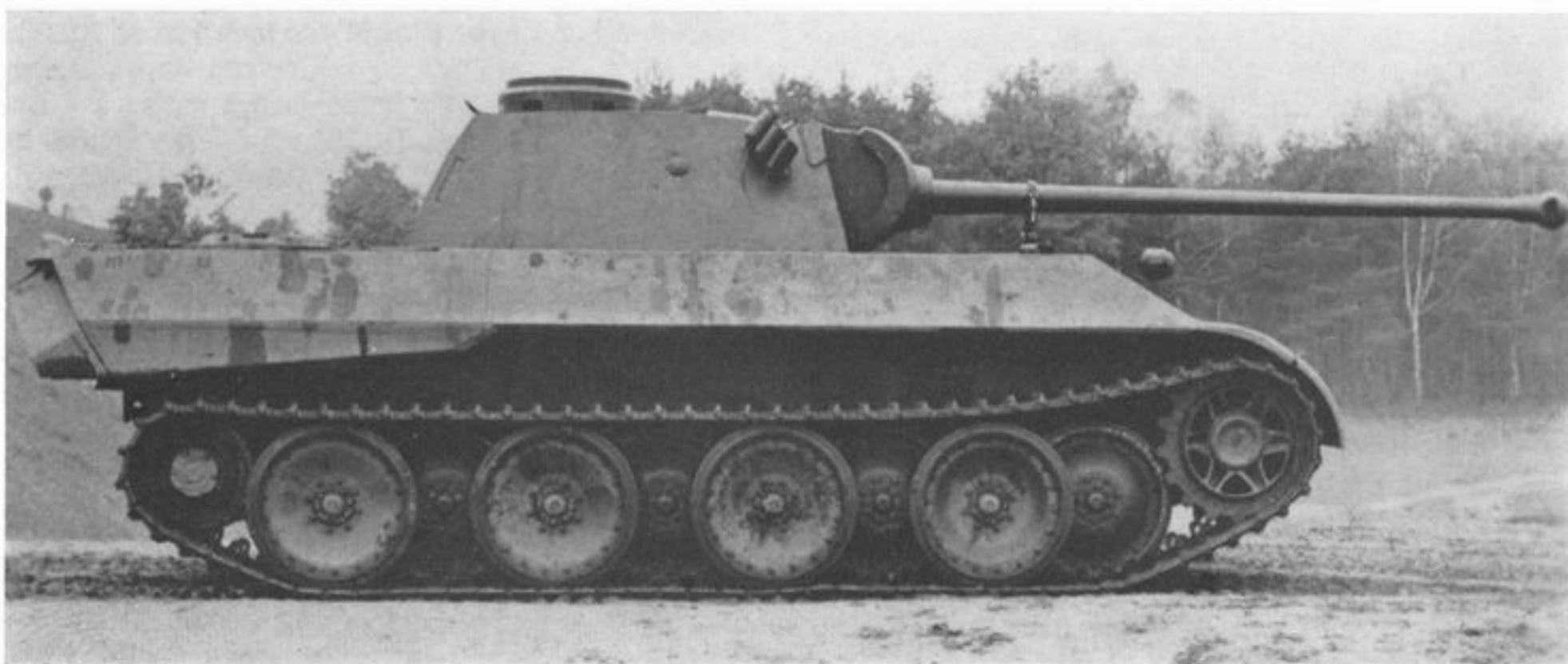
An early production Panther Ausf D with single baffle muzzle brake and smoke dischargers on turret side.
