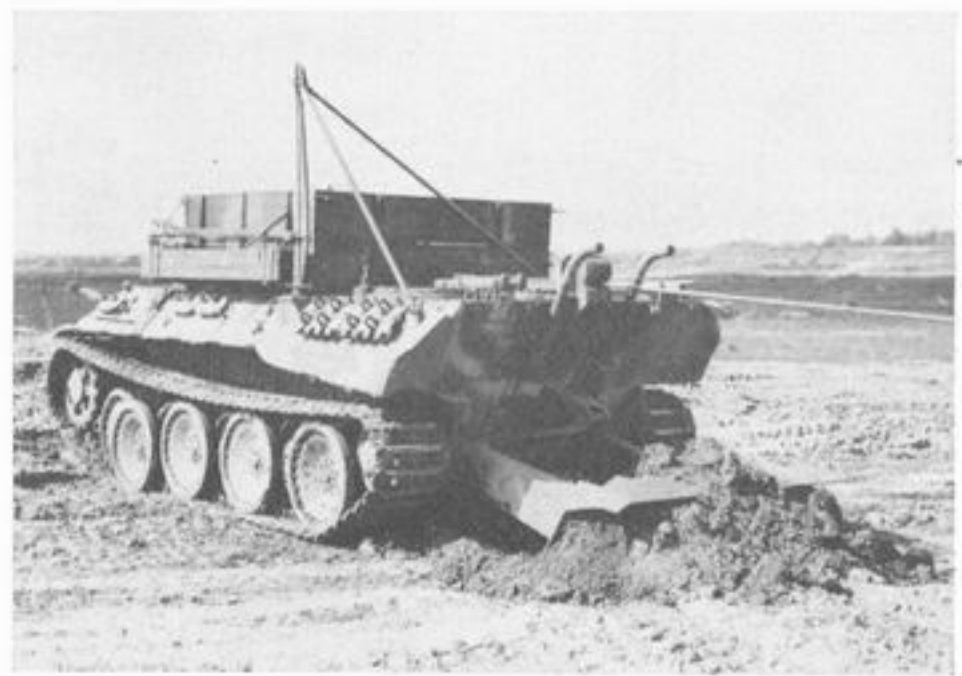
Above and Right: The Bergepanzer Panther (Panther ARV) was an important special purpose type with winch and recovery gear. The earth anchor was raised and lowered from the winch. The light jib could be erected either side for lifting components. (IWM)
