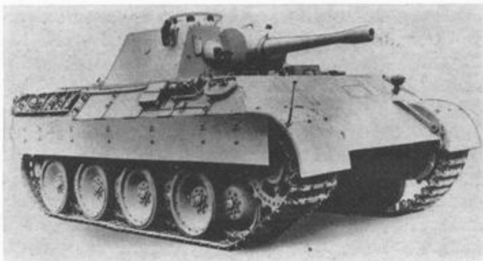
The Beobachtungspanzer Panther (Sd Kfz 172) was an old Panther D converted as an OP vehicle or command vehicle for SP artillery battalions. The "gun" was a wooden dummy and main armament (for self-defence) was the ball-mounted machine-gun. (IWM)
