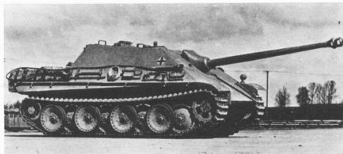
Below and Right: Views of a standard early production Jagdpanther with narrow cast collar round mantlet and one-piece gun barrel. Note the moving arc on the roof and slot for the sighting telescope.
