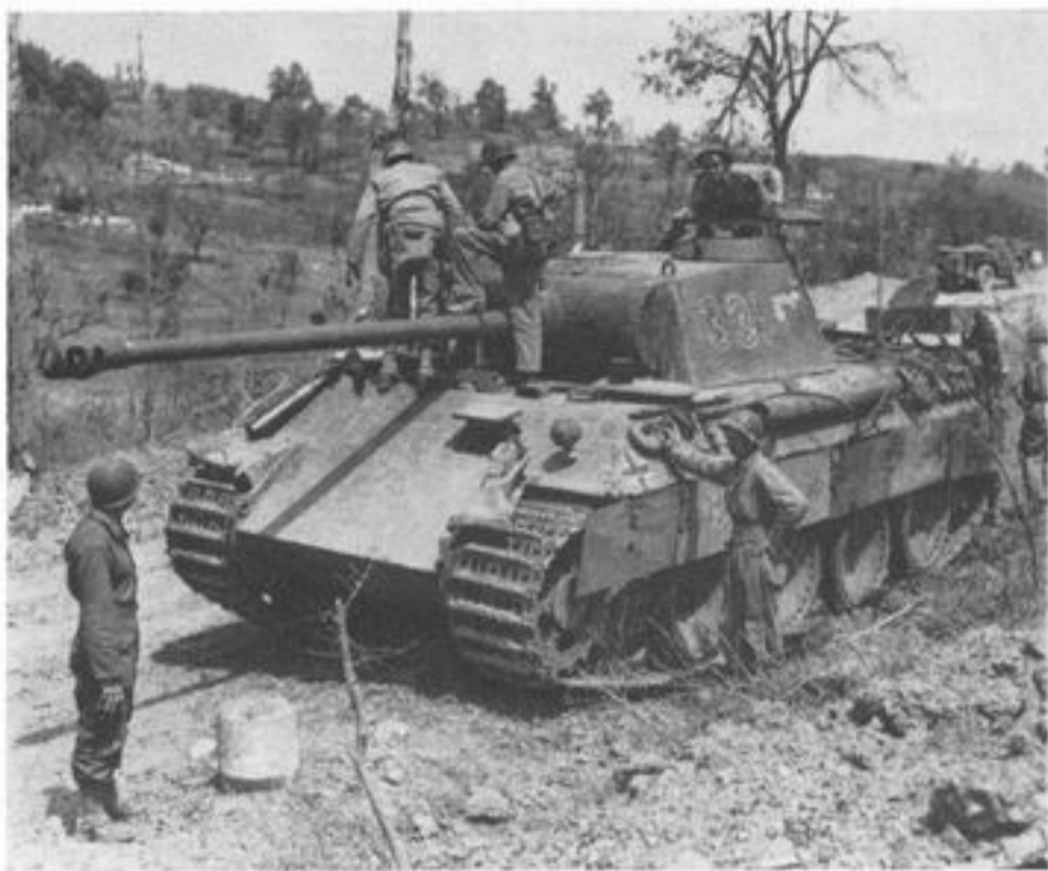
Late production Panther Ds had the improved pattern cupola with periscopes and MG ring. It was also fitted retrospectively to some earlier models. This Ausf D, knocked out in Italy in 1944, also has Zimmerit anti-magnetic coating and side skirts. A 75mm shell can be seen on the glacis plate. (IWM)
