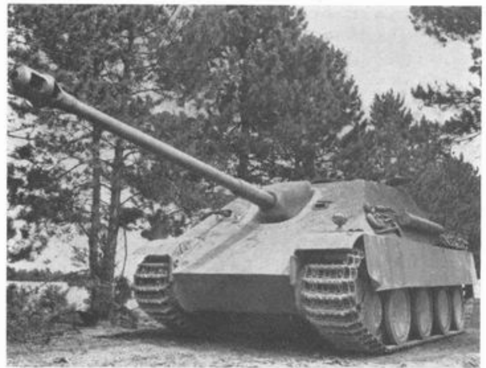
These three illustrations show the later production Jagdpanther with the two-piece barrel of the later 8.8 cm. gun. This simplified barrel changing. Note the Zimmerit anti-magnetic paste and the side skirts. (Chamberlain Collection)
