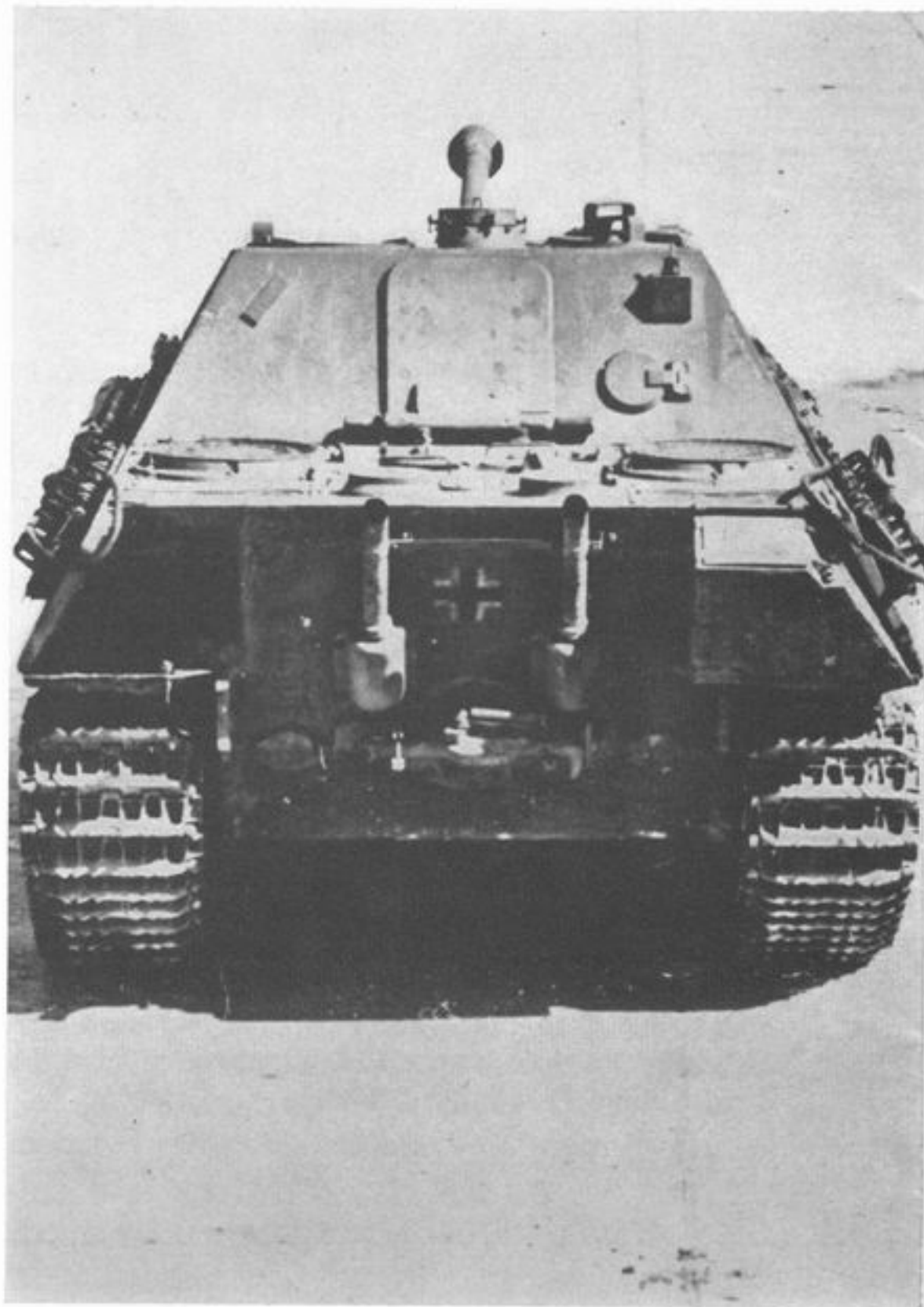
A rear view of an early production Jagdpanther which shows the large escape hatch and the small hatch for re-ammunitioning and discarding empty cases. (IWM)
