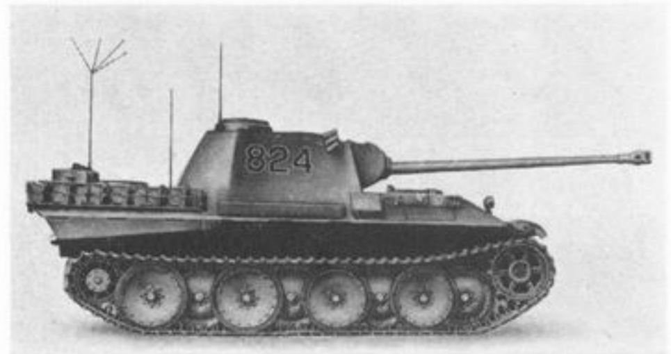
The Befehlspanzer Panther was a standard vehicle (in this case an Ausf D) fitted with extra radio for the use of unit commanders. It was distinguished by the extra aerials. (IWM)
