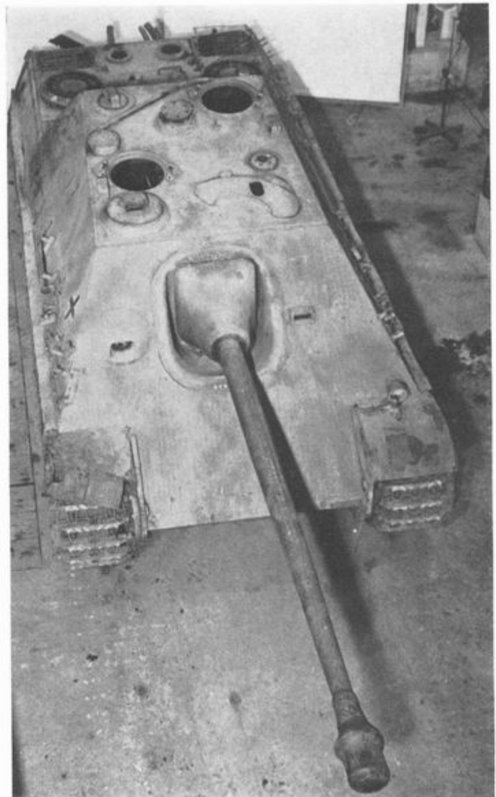
Below and Right: Views of a standard early production Jagdpanther with narrow cast collar round mantlet and one-piece gun barrel. Note the moving arc on the roof and slot for the sighting telescope.
