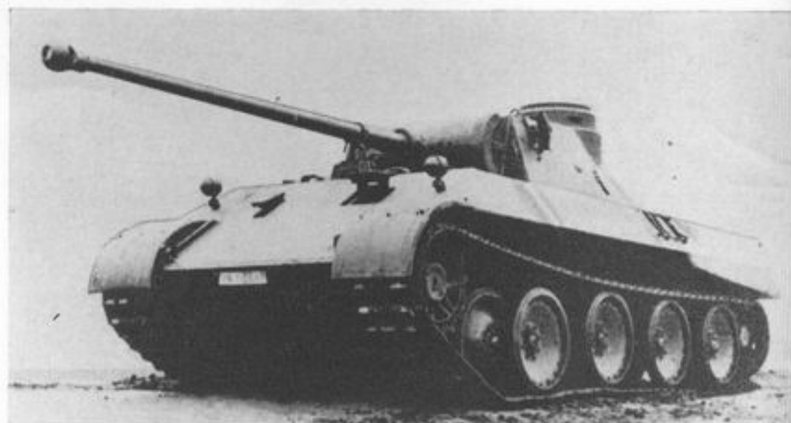
One of the first 20 Panthers produced, originally designated Ausf A, later classed as Ausf D, and known as the D 1 . Major distinguishing feature is the cupola protruding through the turret side, but the single baffle muzzle brake and smoke dischargers on the turret side are other early features to note.
