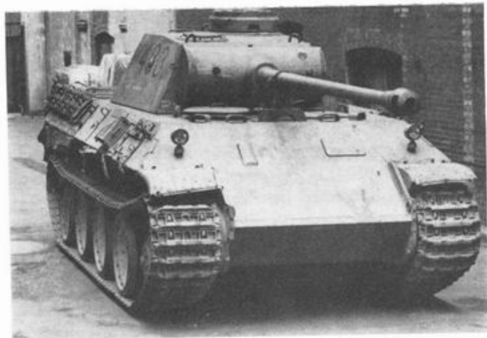
A later production Panther Ausf D which shows the dustbin-type cupola and the vision port and machine-gun port on the glacis. (Chamberlain Collection)
