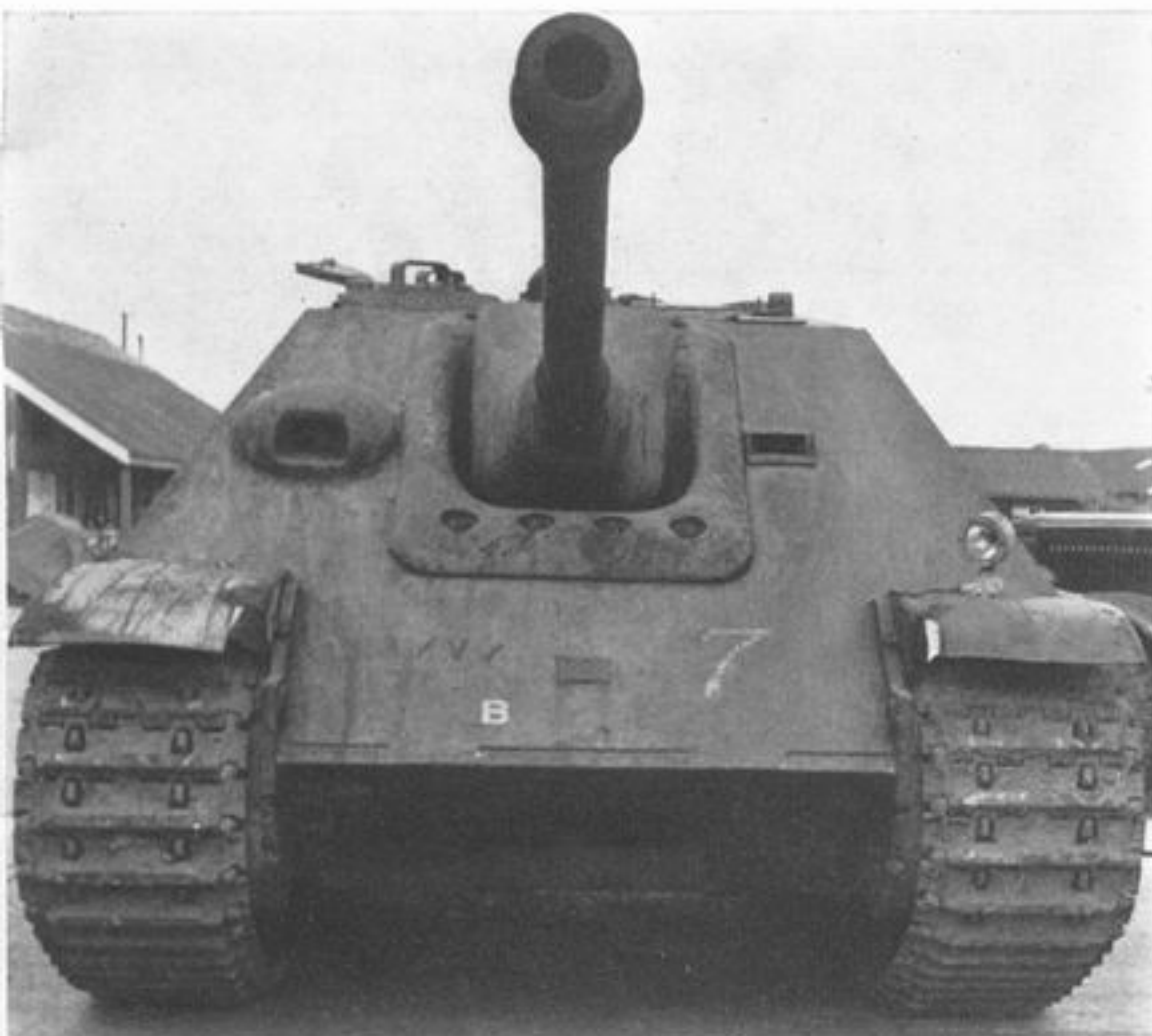
Final production model of the Jagdpanther had a wider, squarer collar which was bolted in place to simplify production. (IWM)
