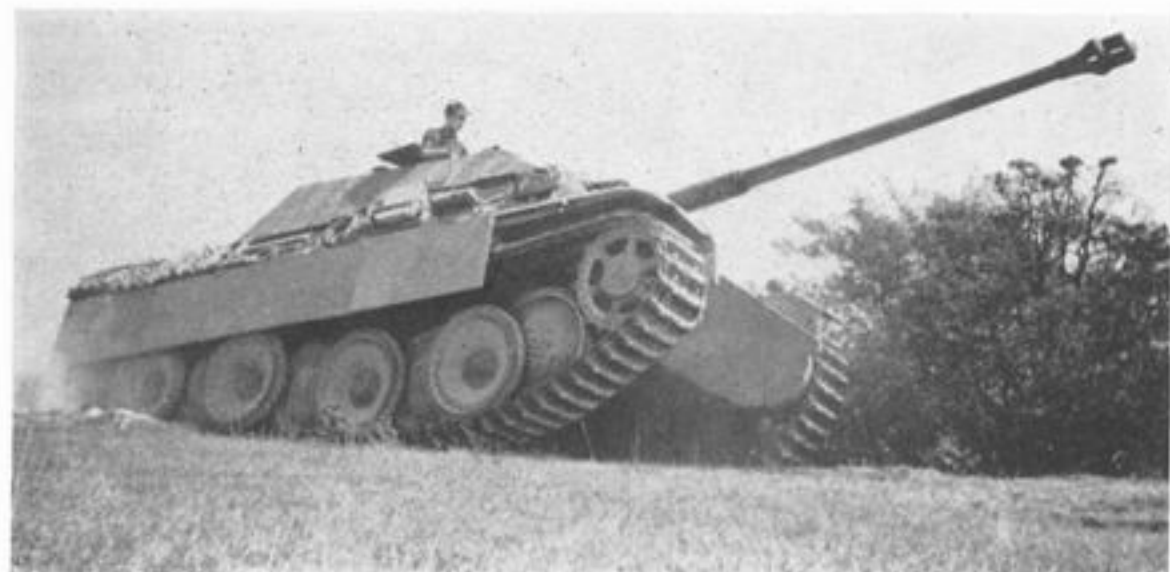
These three illustrations show the later production Jagdpanther with the two-piece barrel of the later 8.8 cm. gun. This simplified barrel changing. Note the Zimmerit anti-magnetic paste and the side skirts. (Chamberlain Collection)
