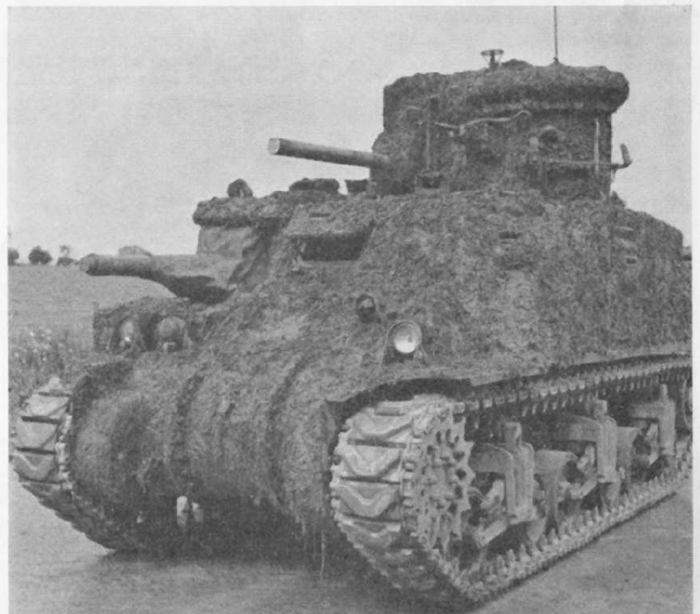
A well-camouflaged Grant CDL in 1944 during exercises in Britain prior to D-Day. Note the dummy gun on the searchlight turret and the later type of rubber chevron-pattern tracks.
