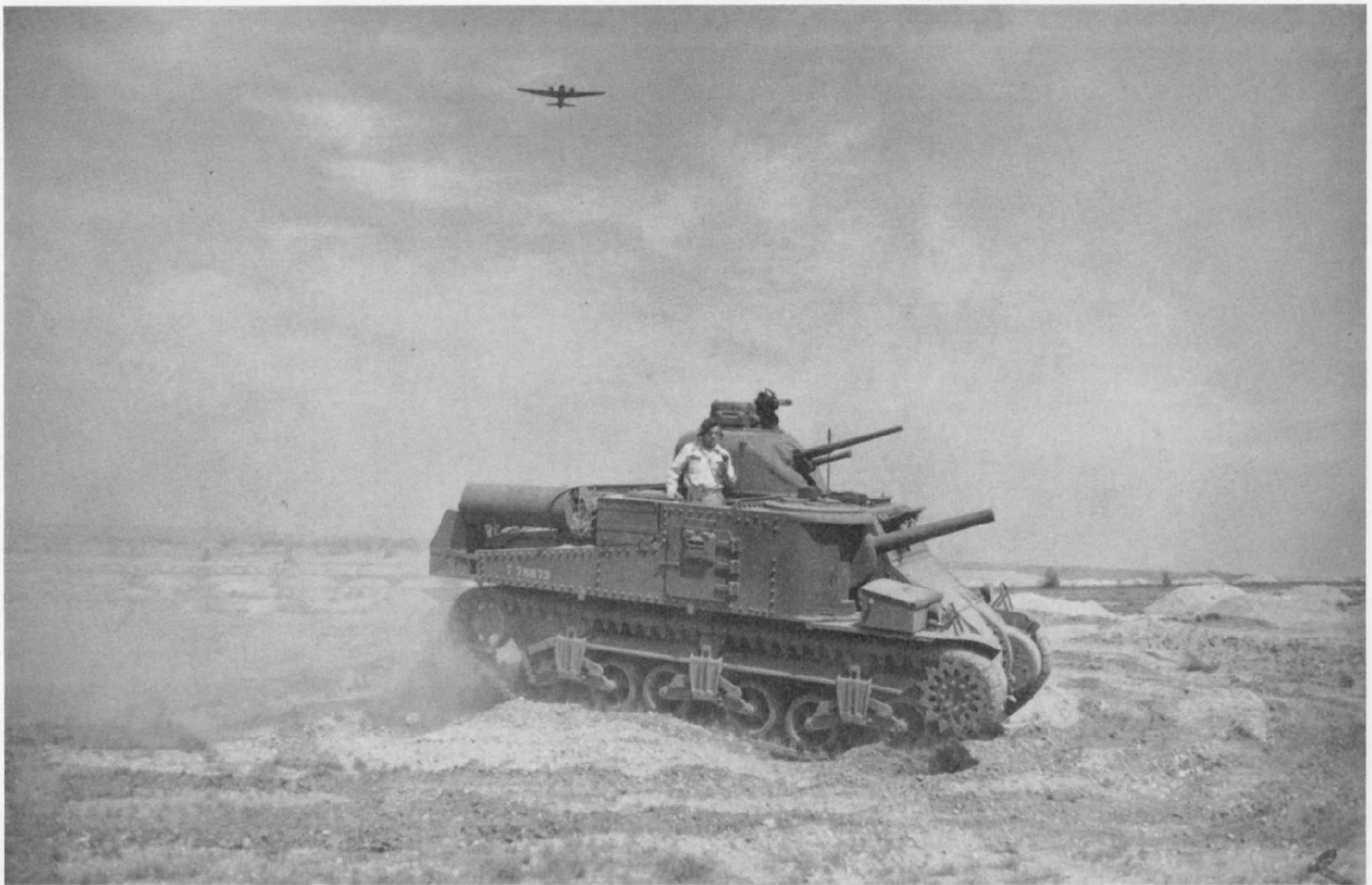
M3 in Canadian service had local modifications including jettisonable fuel tanks and mud chutes beneath the top run of the track. (Canadian Official)
