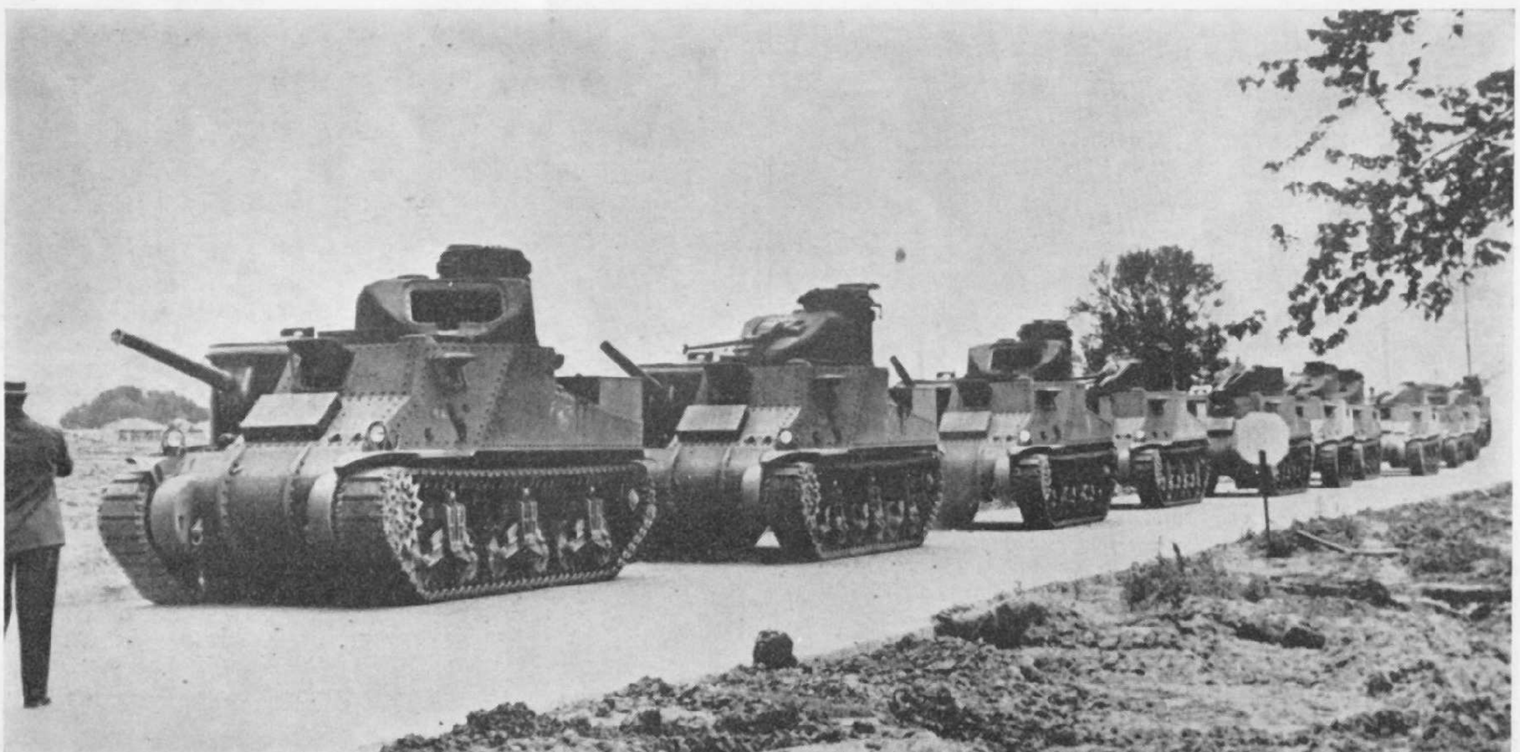
Late production M3A4s on the test track at Detroit Arsenal in the fall of 1942. All have the M3 75 mm. gun, but on most the turret guns are yet to be fitted. (U.S. Official)
