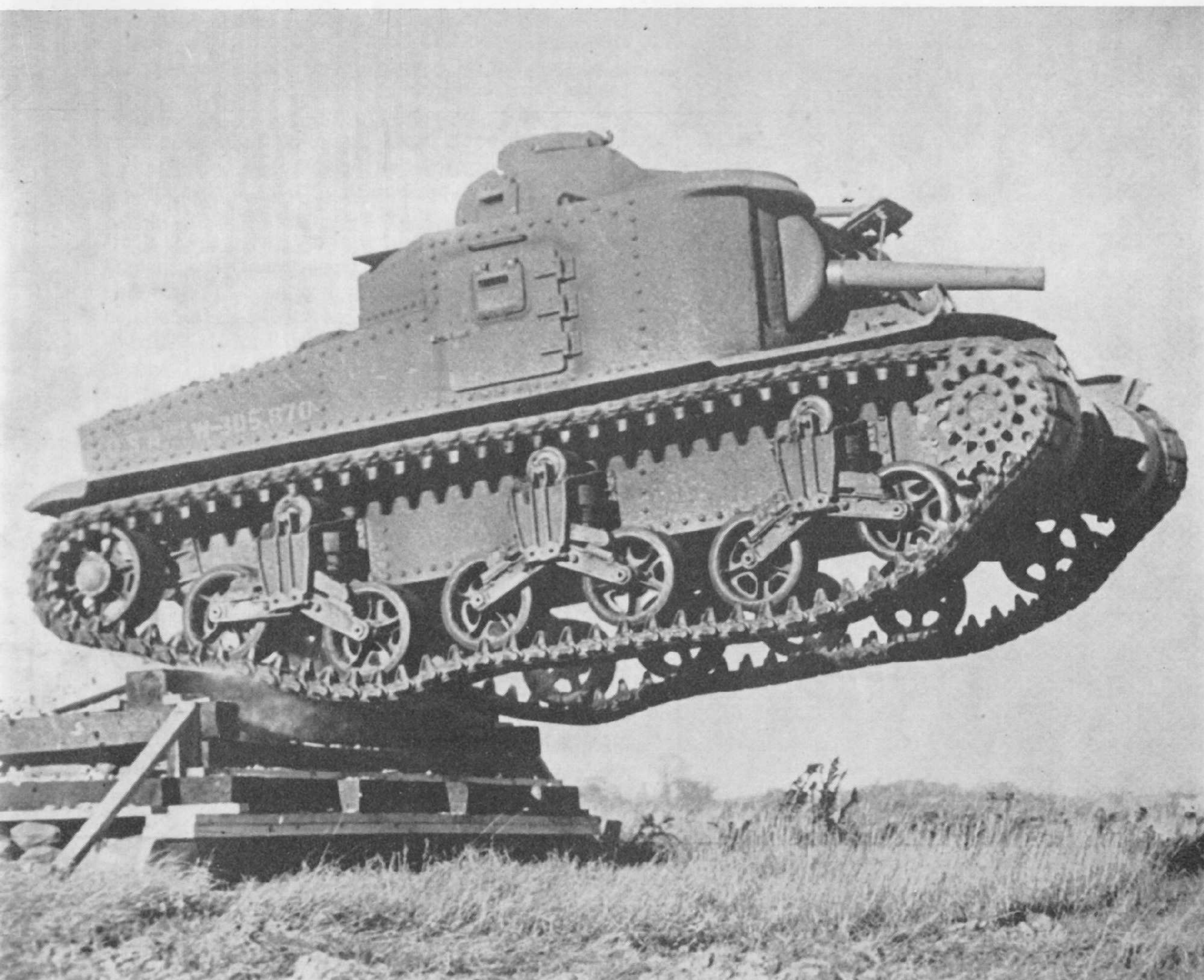
An early production M3 being put through its paces at Aberdeen Proving Ground in 1941 shows to advantage the flexibility of the simple vertical volute spring suspension. (U.S. Official)
