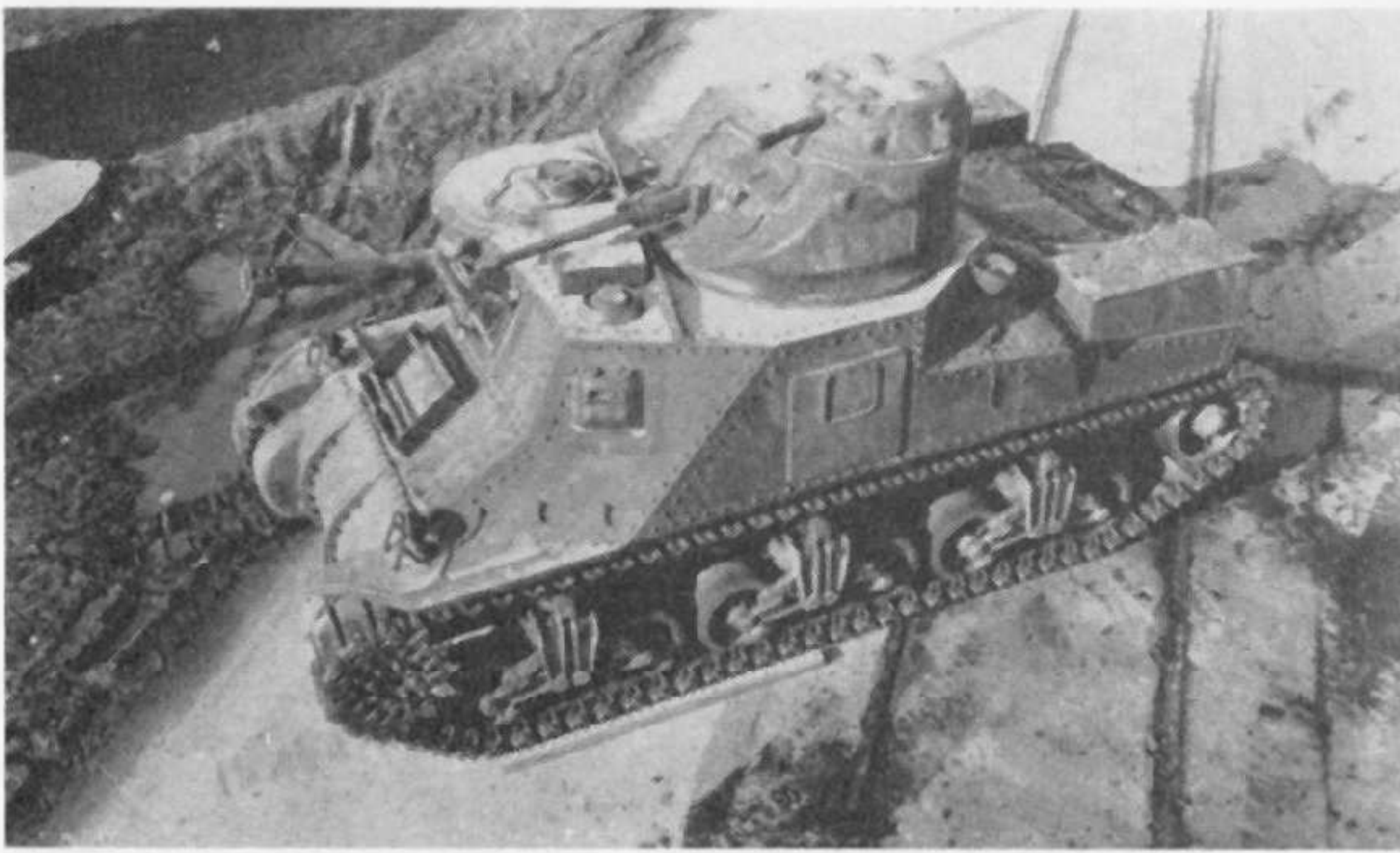
The M3A5 had twin GM diesel motors. This view shows the M2 gun with added counterweight, welded up side doors, and the deeper rear housing for the engines. (U.S. Official)
