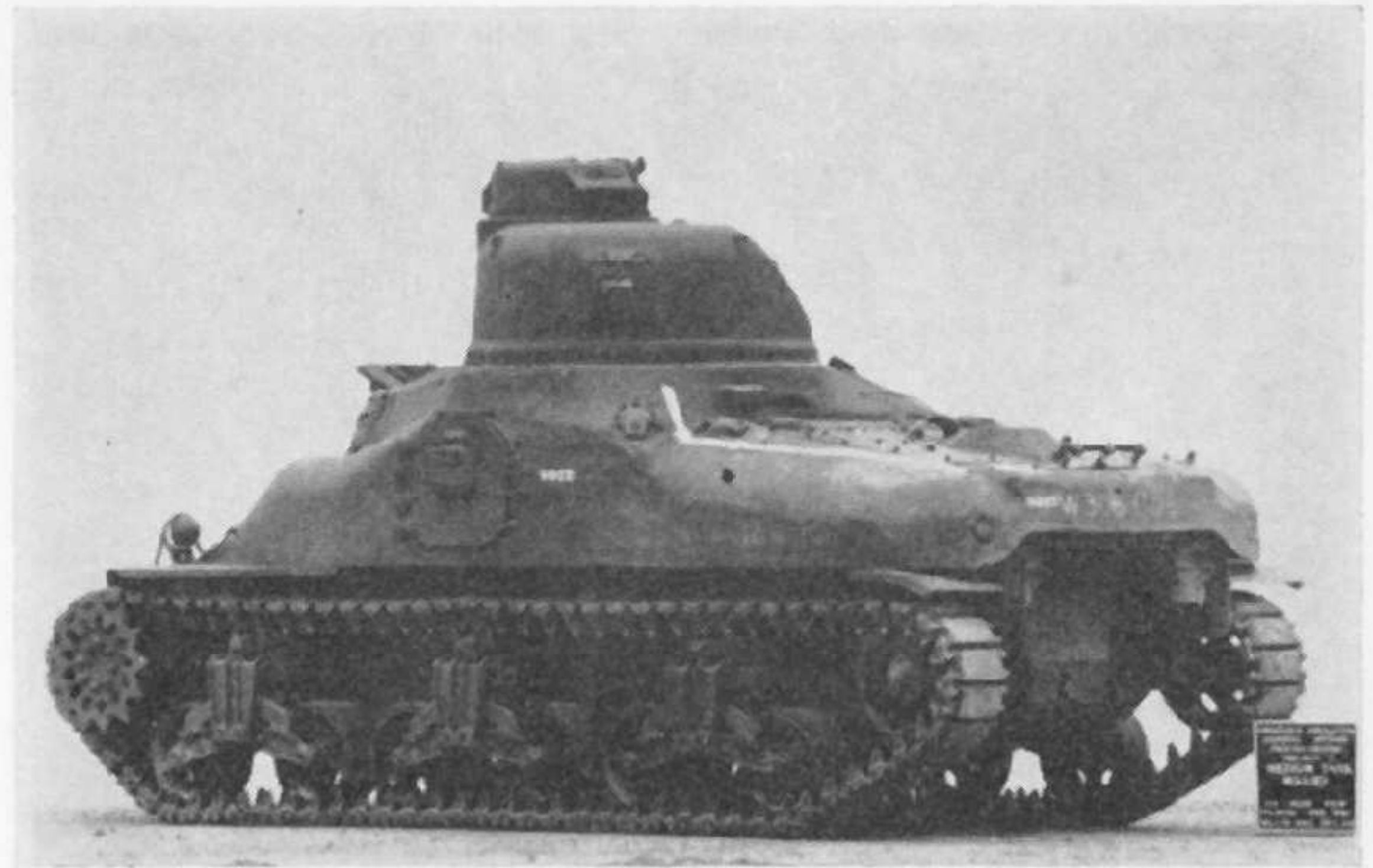
The M3A1E1 was one of many project test vehicles. It was tried with triple Lycoming aero engines in May 1942 when alternative power plants were being sought for M3 series vehicles. (U.S. Official)
