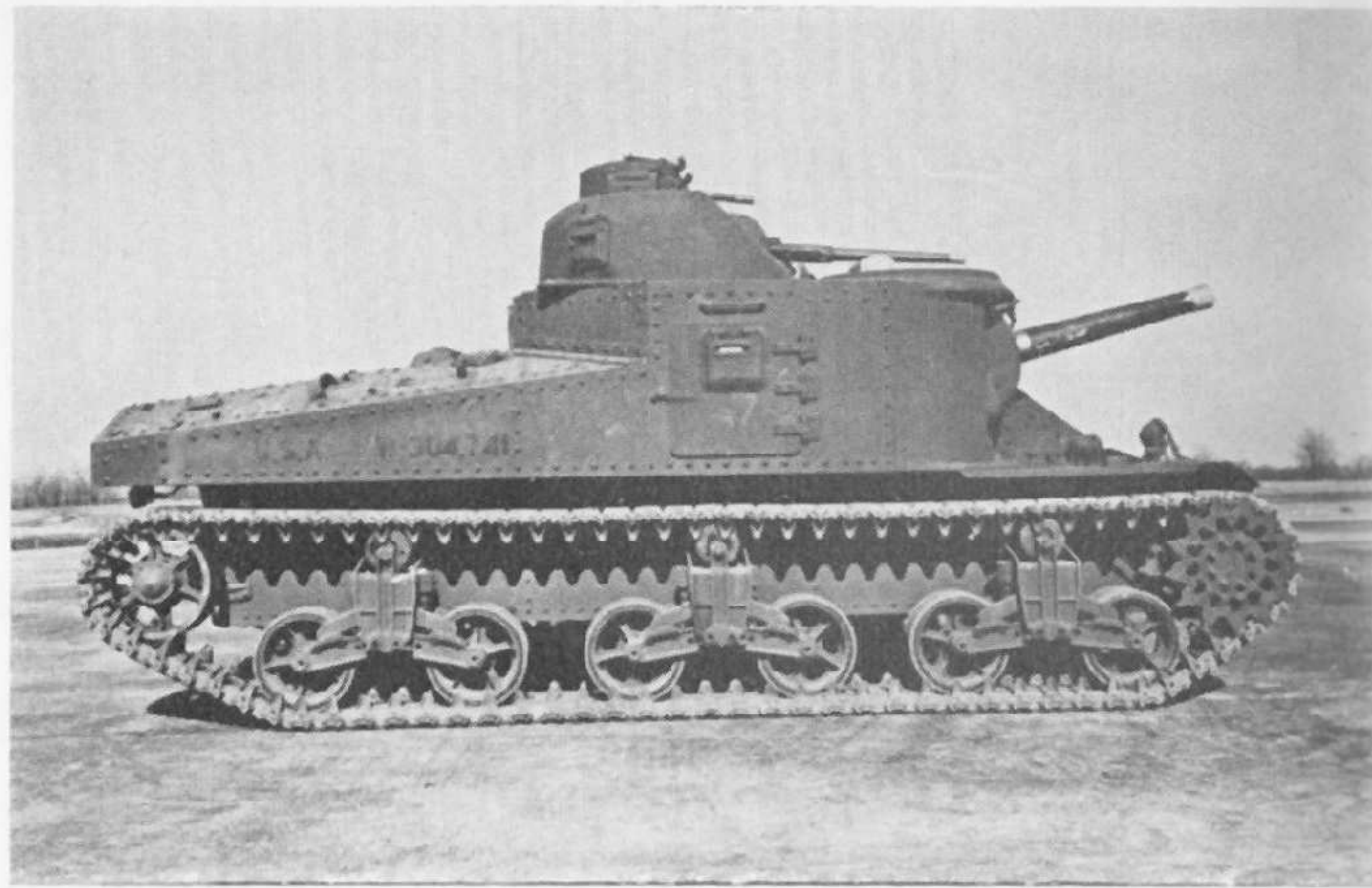
The M3A4 had the Chrysler Multibank engine which necessitated lengthening the hull and chassis to accommodate it. Wider spaced bogies and the extended rear can be seen clearly in this view. British designation was Lee VI. (U.S. Official)
