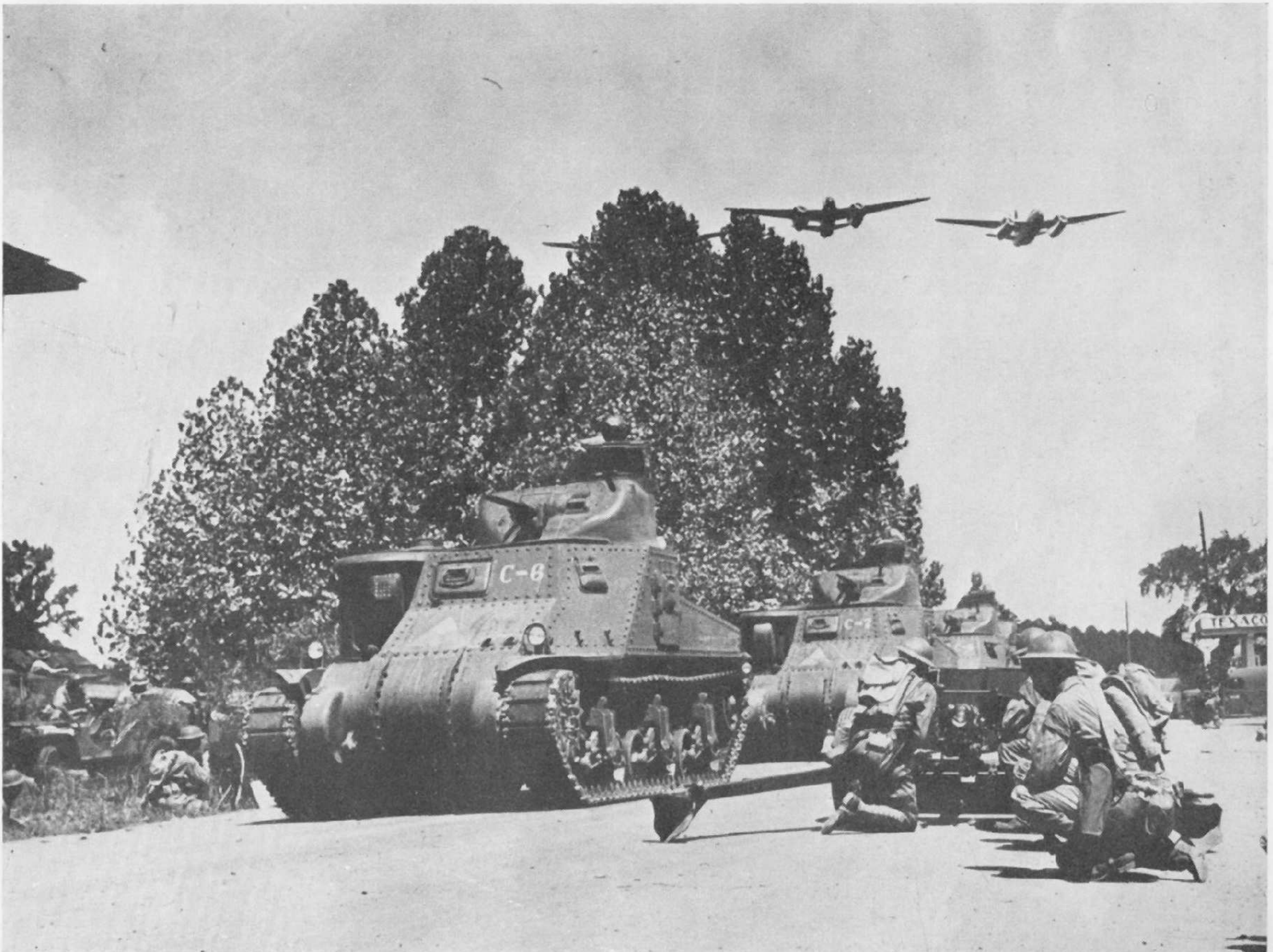
Early M3s in U.S. Army service take part in exercises in October 1941. Note that they lack the 75 mm. gun, still in short supply at this period. Troops are still wearing 1918 type steel helmets. (U.S. Official)
