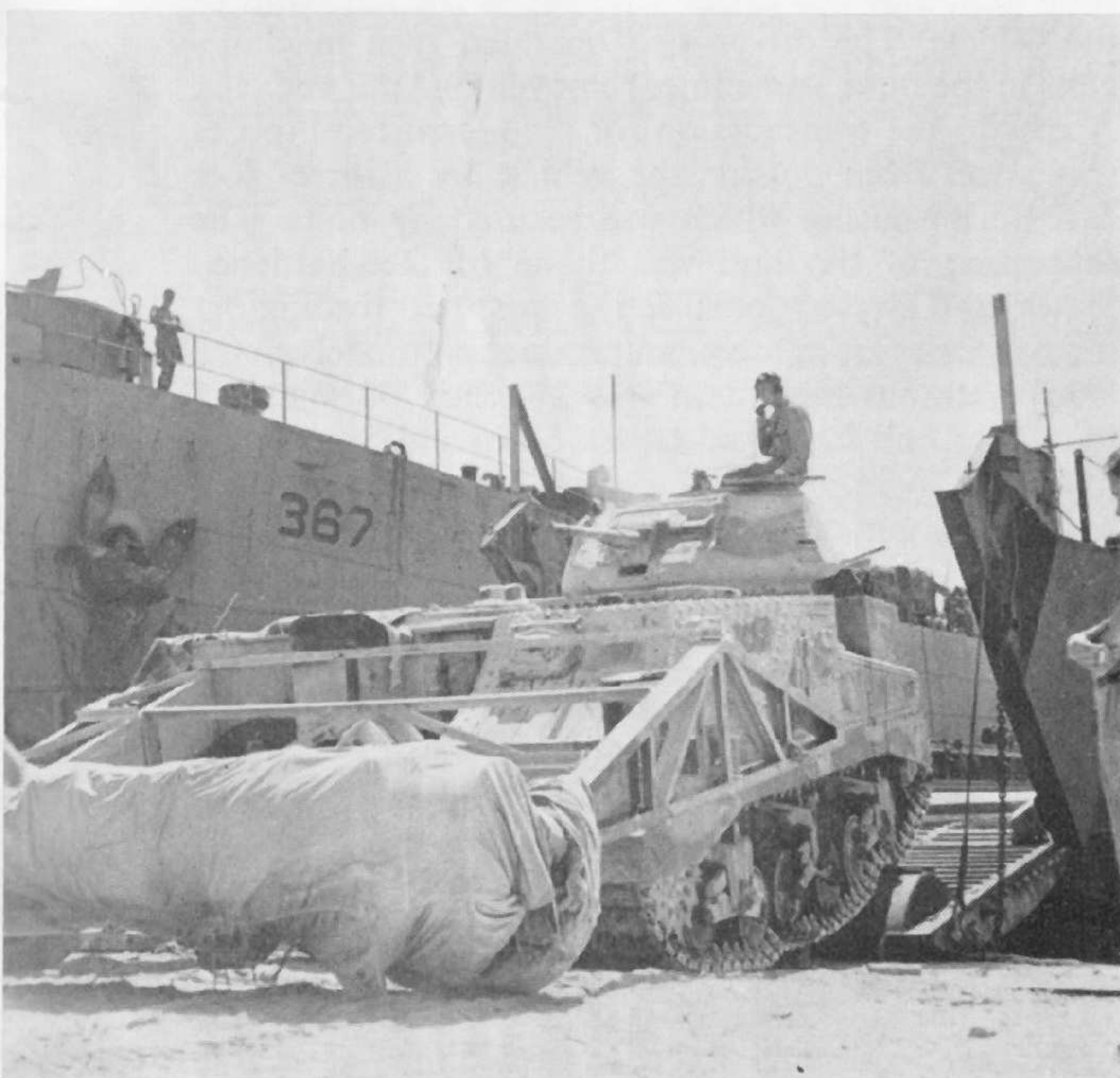
Grant Scorpion III leaves a LCT during training for the Anzio landings. (Imperial War Museum)
