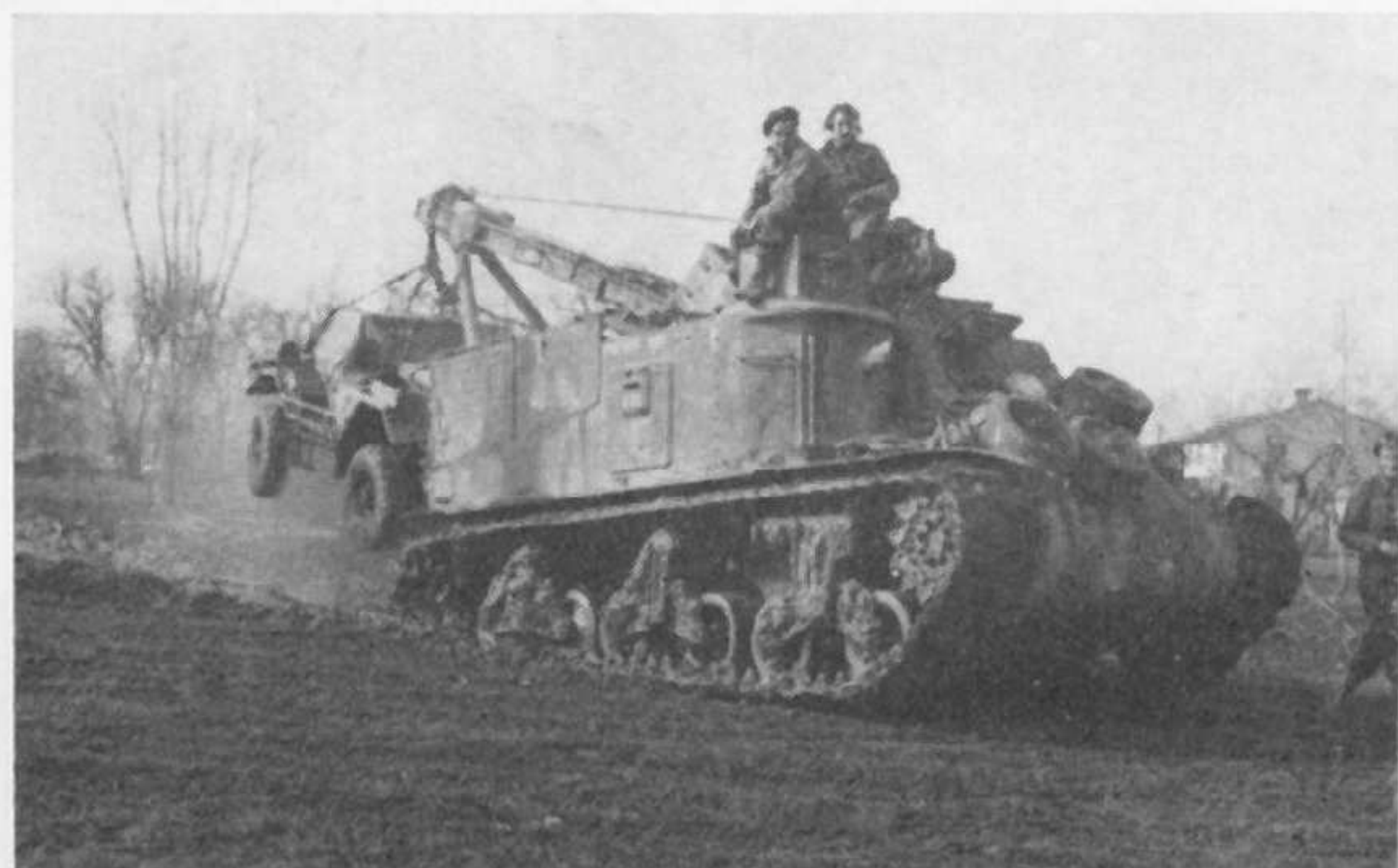
M31 TRV (based on M3 tank) seen in British service as a Grant ARV II carrying a scout car slung from its boom. M31B1 was similar vehicle based on the welded M3A3.
