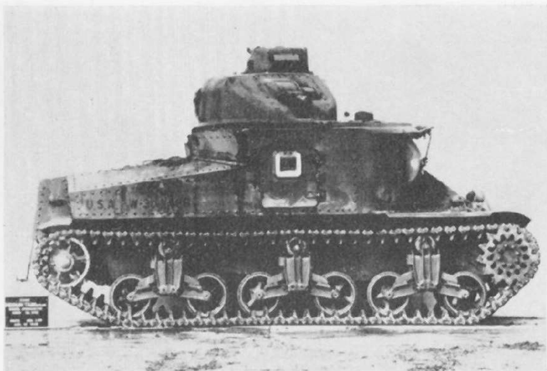
The M3A5E1 was yet another trials vehicle, this time to test the possible installation of Hydramatic transmission. Note the extended rear hull to house it. (U.S. Official)
