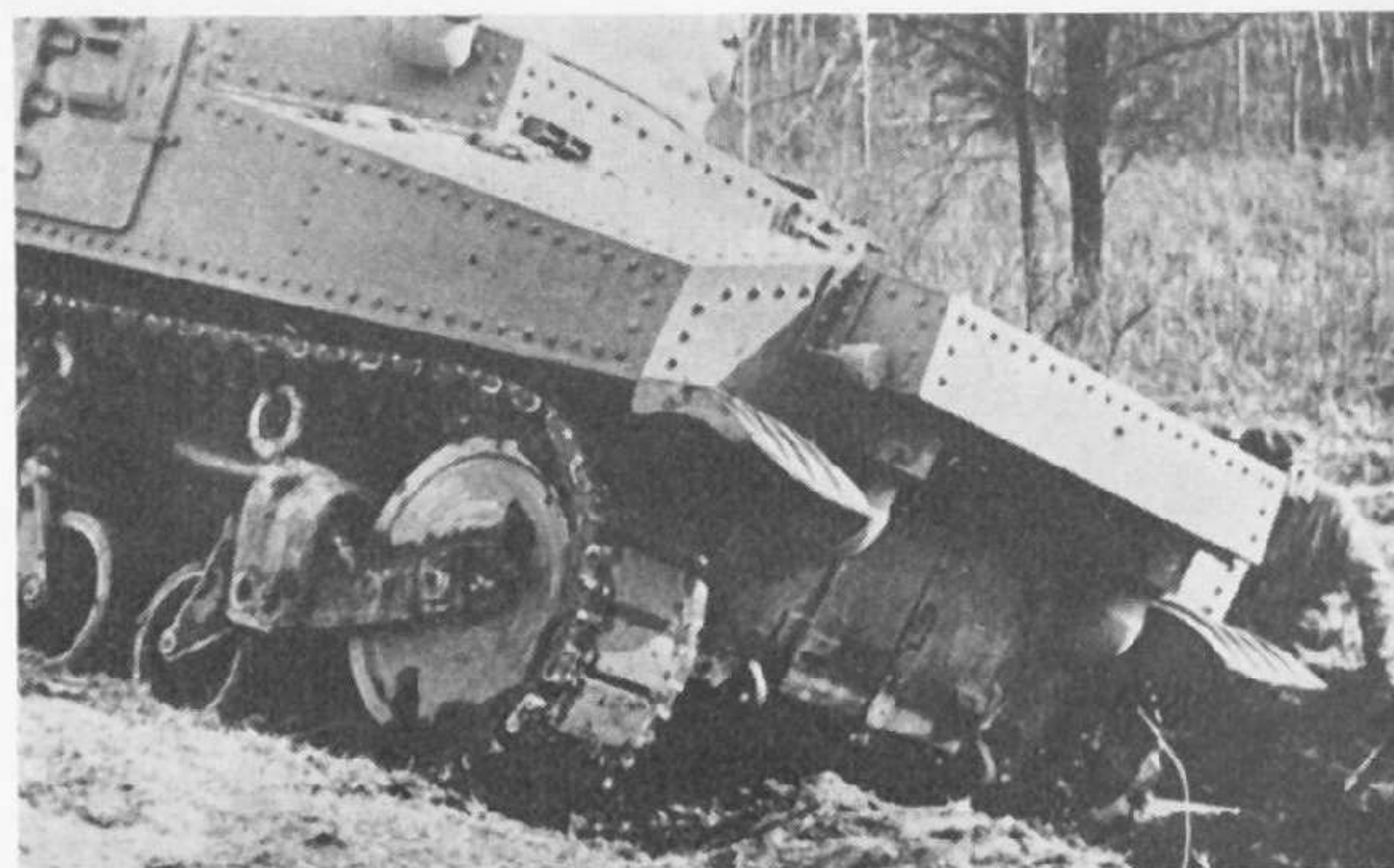
Yet another test vehicle was used with experimental trailing rear idlers. This is the Wright-engined M3. (Chamberlain Collection)
