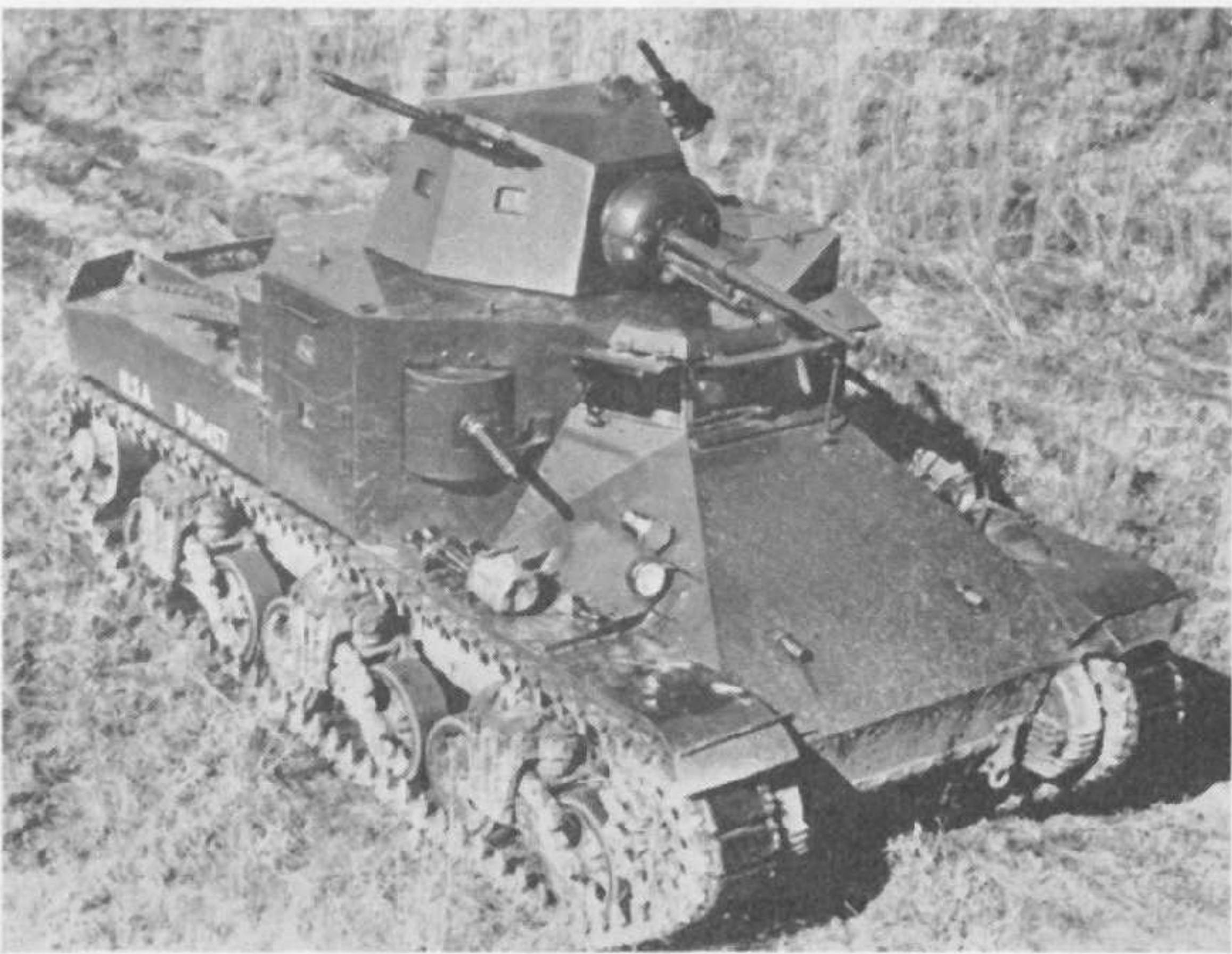
Medium Tank M2 (and its similar but improved successor the M2A1) were the designs which formed the mechanical basis for the M3 Mediums. Note the numerous machine-guns, the single 37 mm. gun in the turret, and the deflector plates for enfilading trenches in line with the rear-firing machine-guns. (Imperial War Museum)
