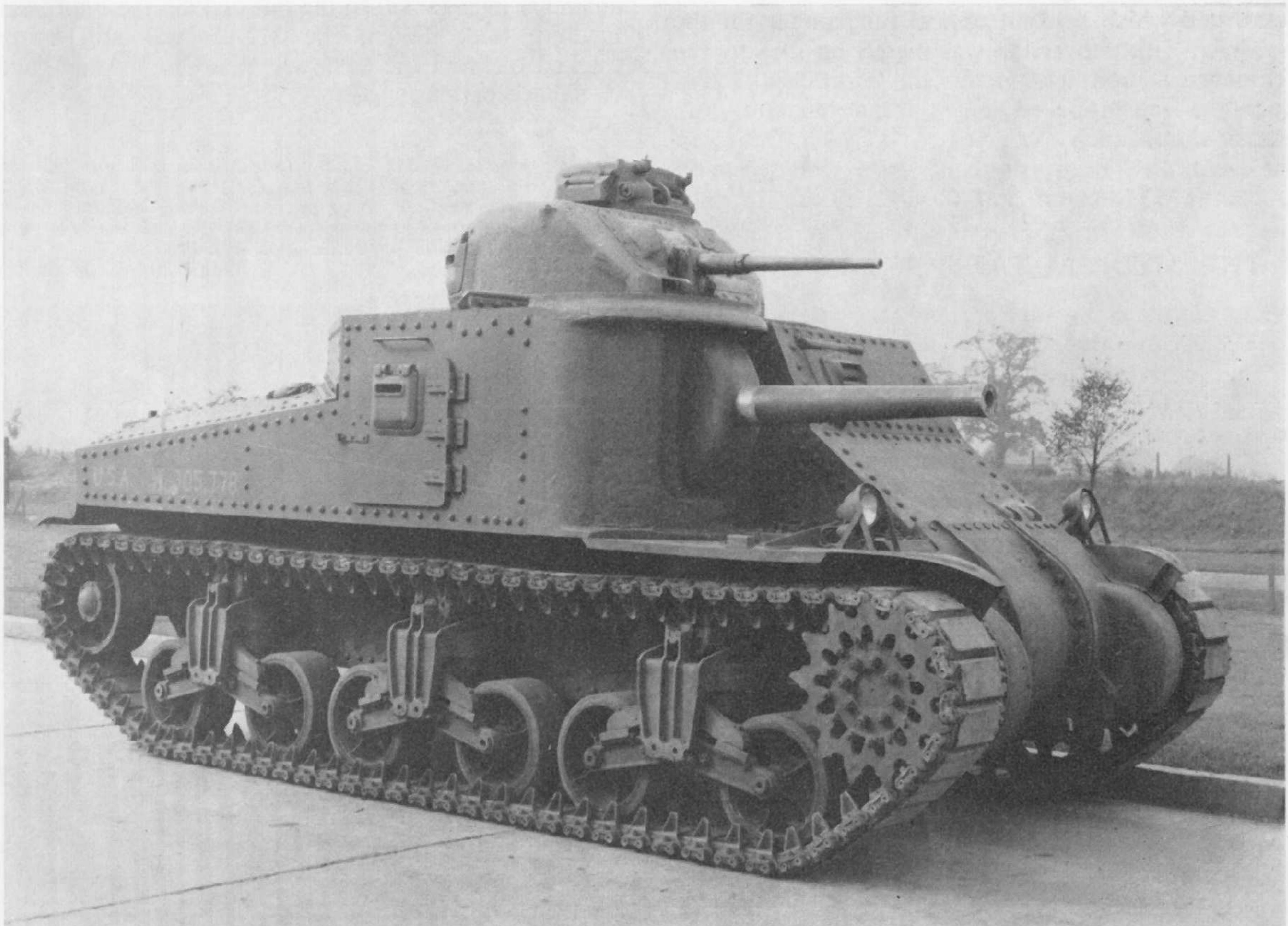
A standard early production M3 (Lee I) with the short M2 75 mm. gun and M5 37 mm. gun.
