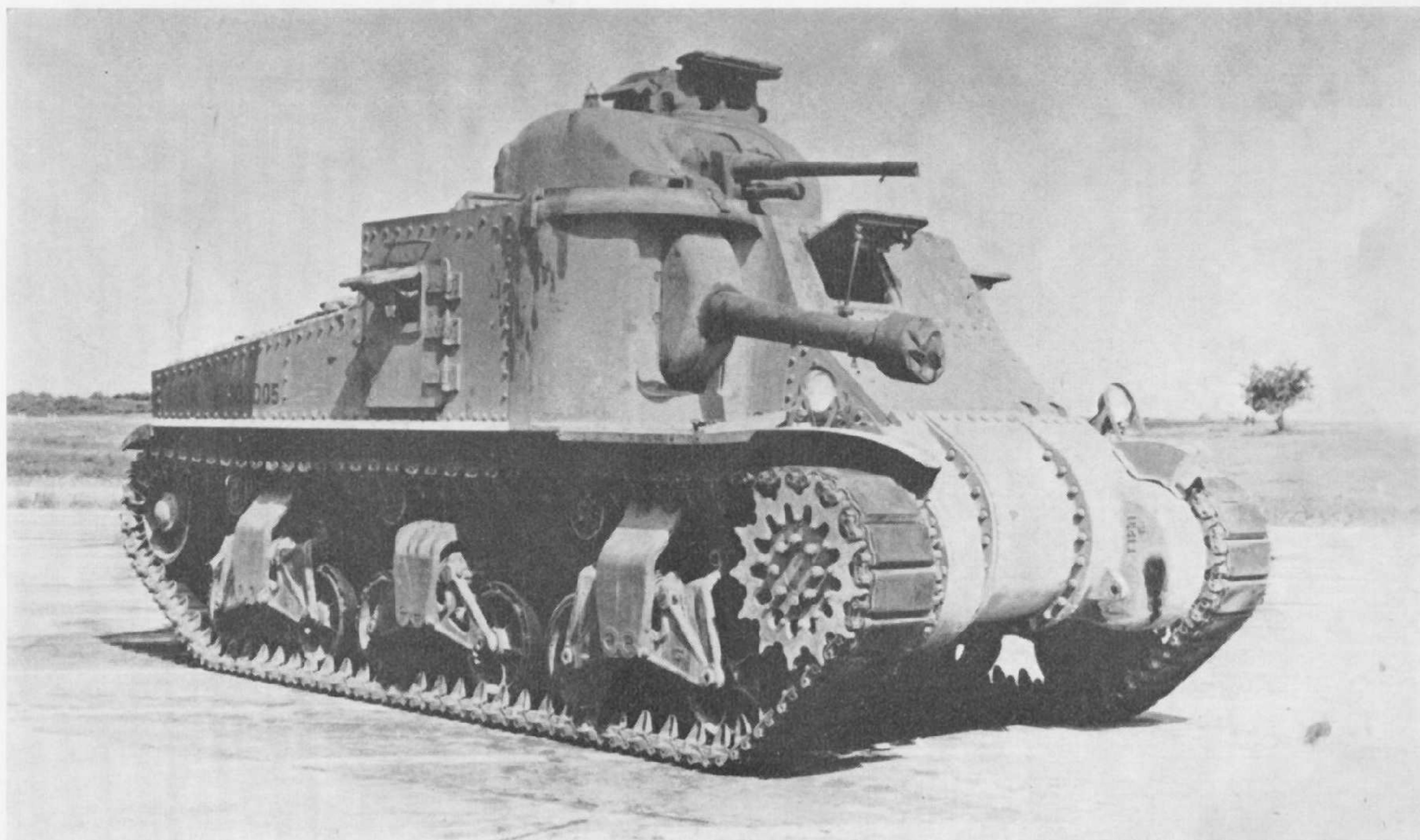
A trials model of the M3A4 used for experiments with horizontal volute spring suspension, April 1942. Shown here in its early form, HVSS was later fitted on the Sherman tank. (U.S. Official)
