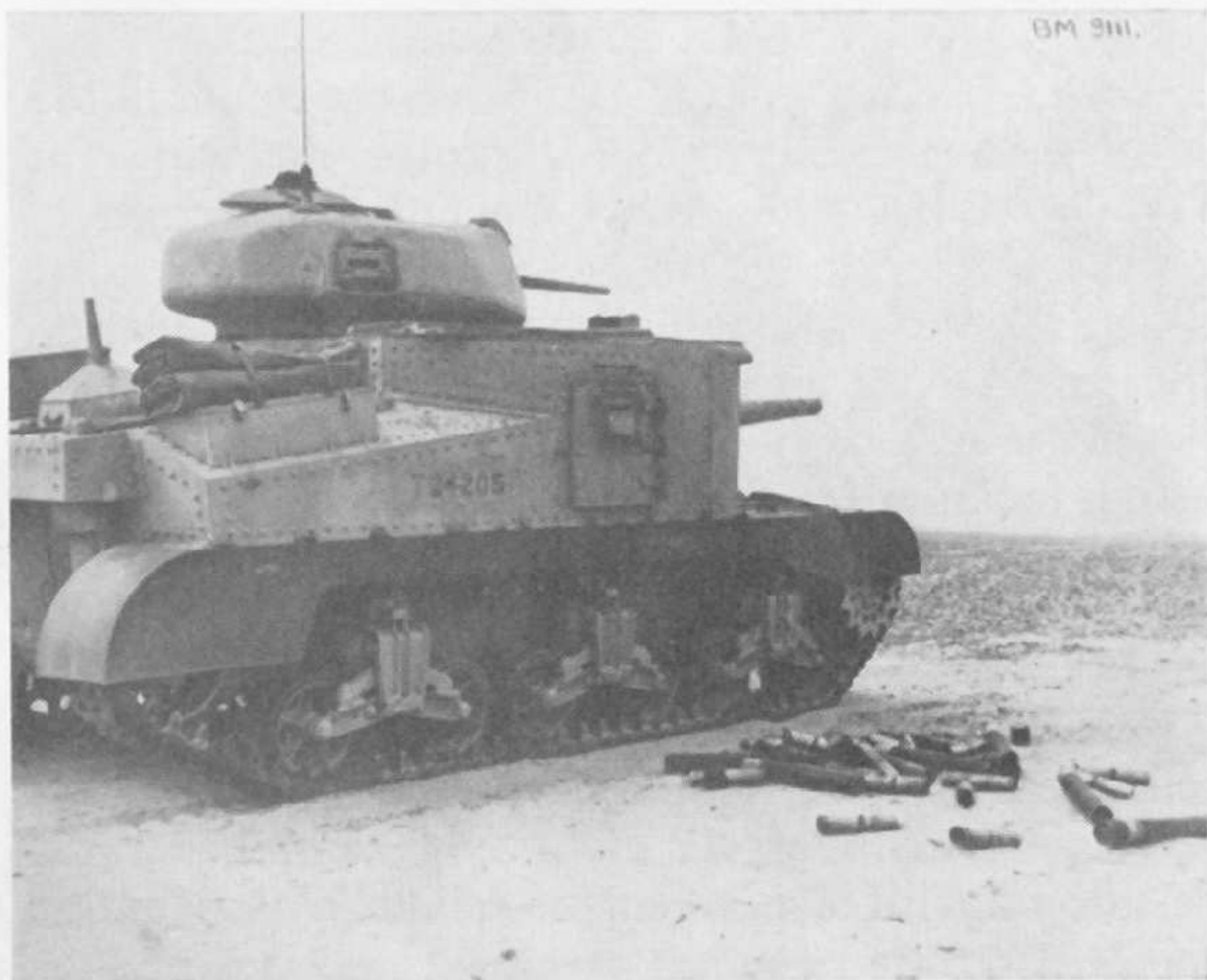
A Grant in the desert at the time of Alamein, while engaging distant targets. Note the upended fabricated funnel on the rear decking used for re-fuelling. (Imperial War Museum)
