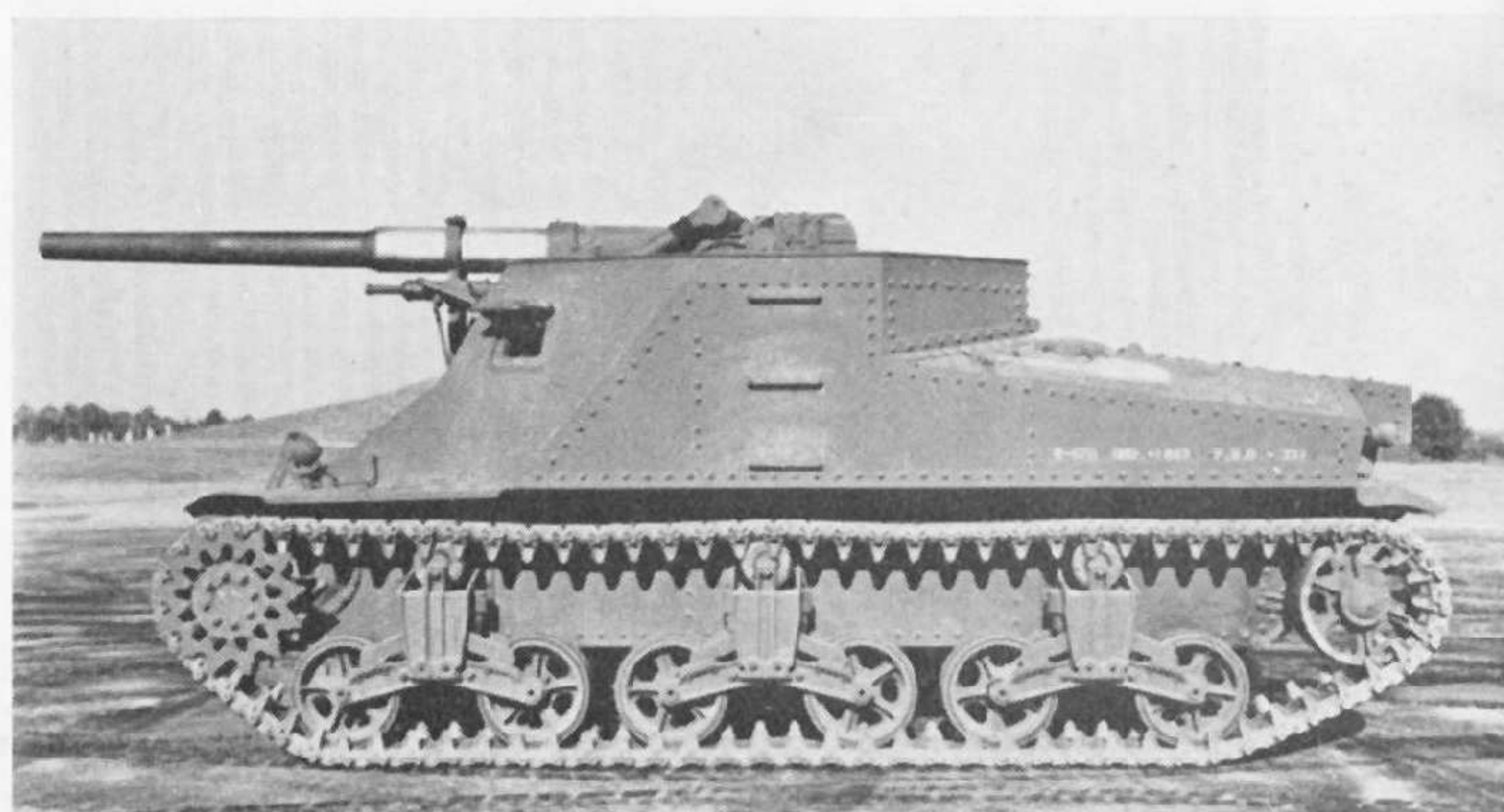
The T24 3-inch Gun Motor Carriage was an early attempt to produce a SP version of the M3. It was a prototype only. (U.S. Official)
