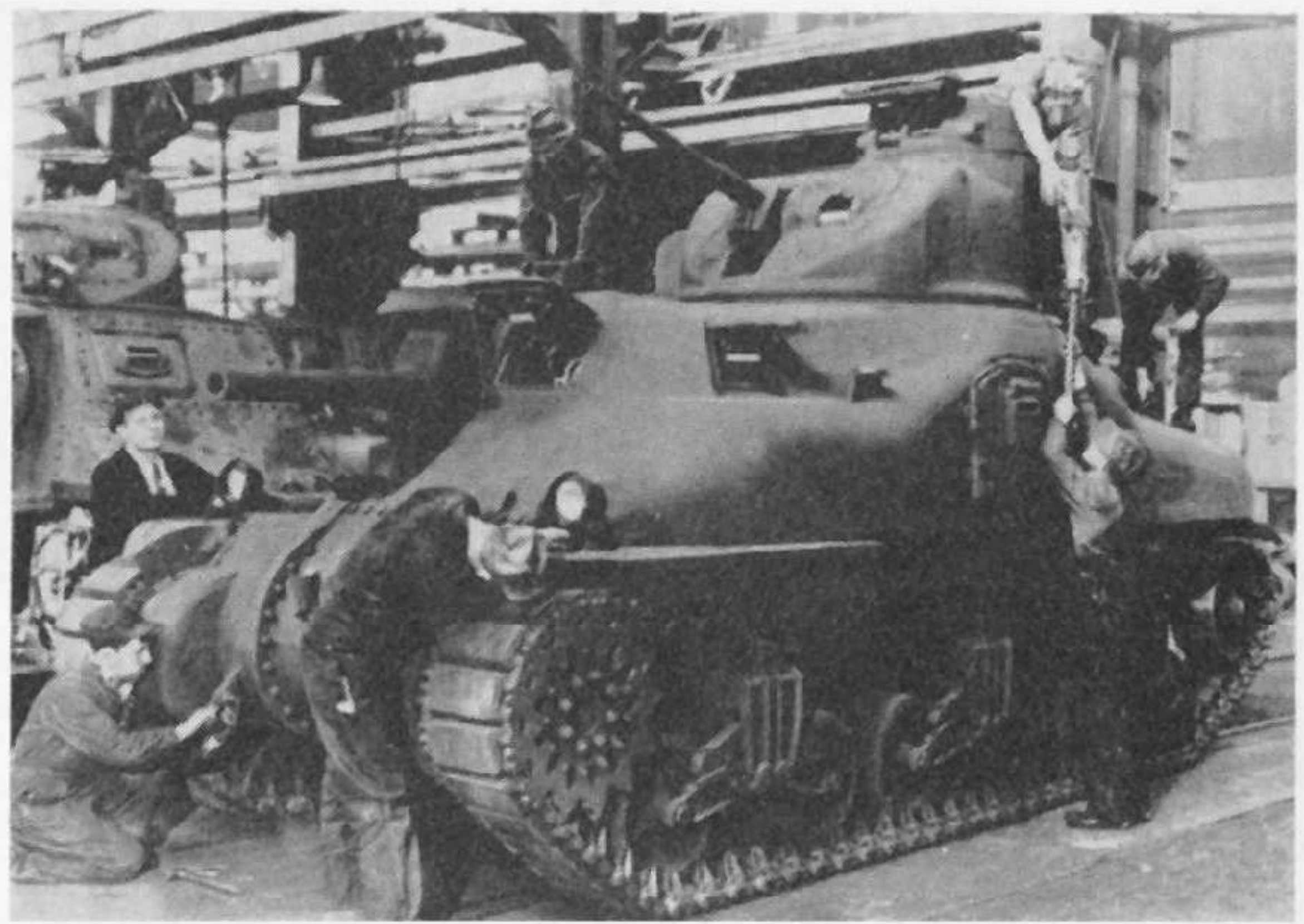
The M3A1 was distinguished by its cast hull. Here the pilot model is seen being completed at American Locomotive Works in February 1942. (U.S. Official)
