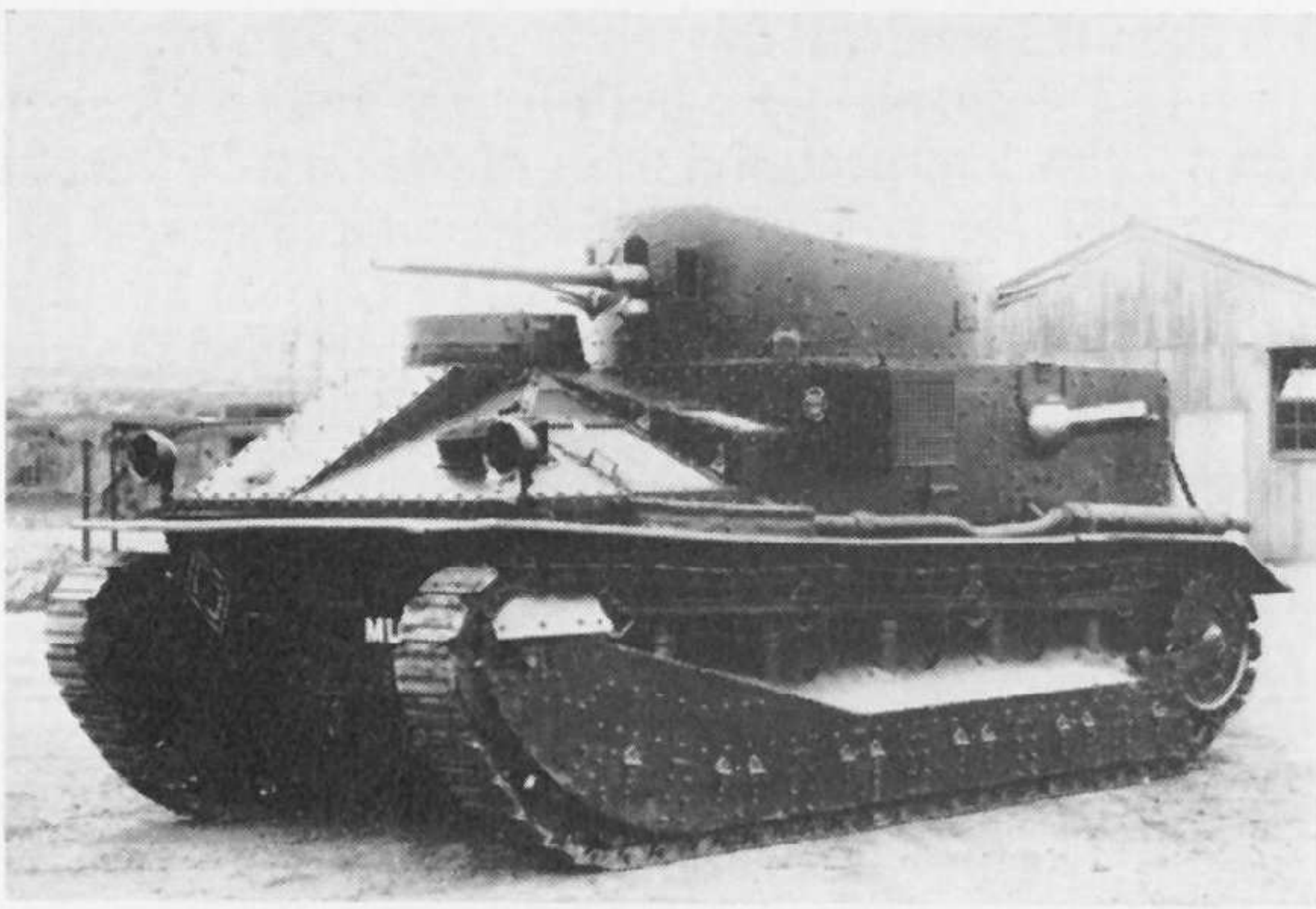
Mark II. Note driver's hood proud of superstructure, one of the recognition points of all Mark IIs and variants. This vehicle was later converted to a Mark II*. The tracks are No. 1 pattern without recesses in the plates. (R.A.C. Tank Museum)
