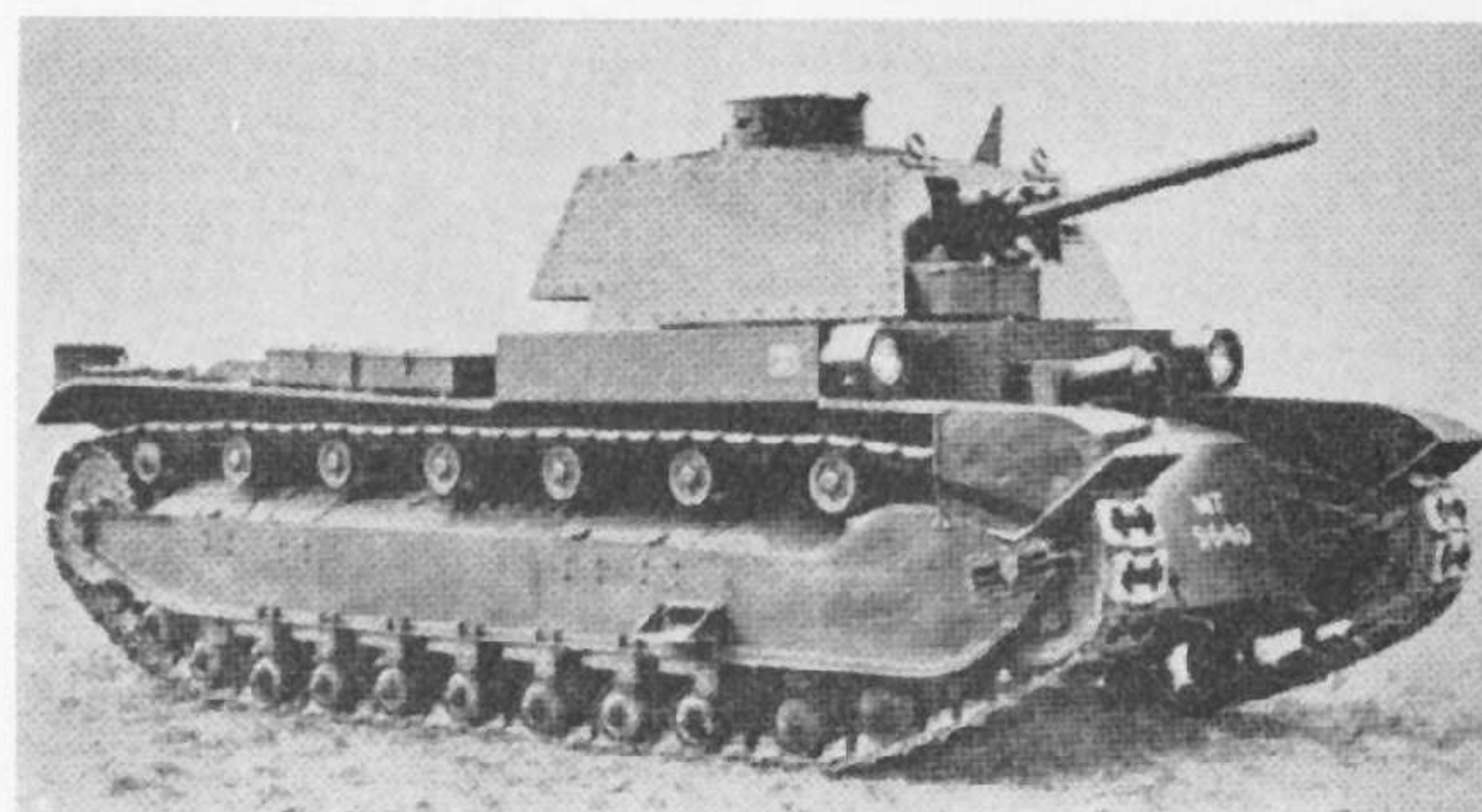
Medium Tank A7E2. Development work on the A7 14-tonners was stopped in 1937 but they contributed different points to the A12 (Matilda), the Churchill, the A9 and the A10.
