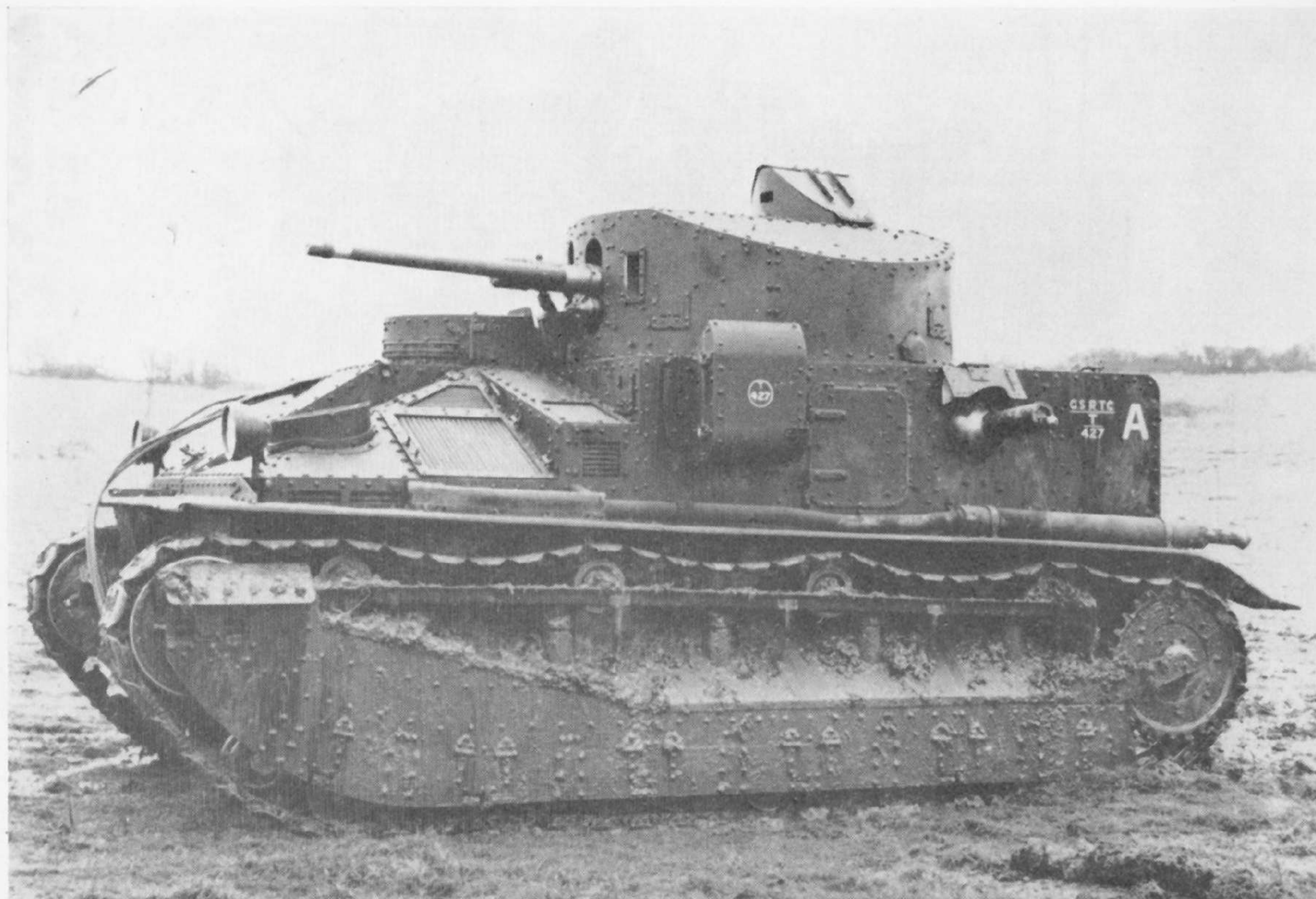
Mark IIA, showing the armoured box which protected the electrically operated ventilating fan on the port side just forward of the side door. Mark IIA had the "Bishop's Mitre" and coaxial Vickers machine-gun like the Mark II*. (R.A.C. Tank Museum)
