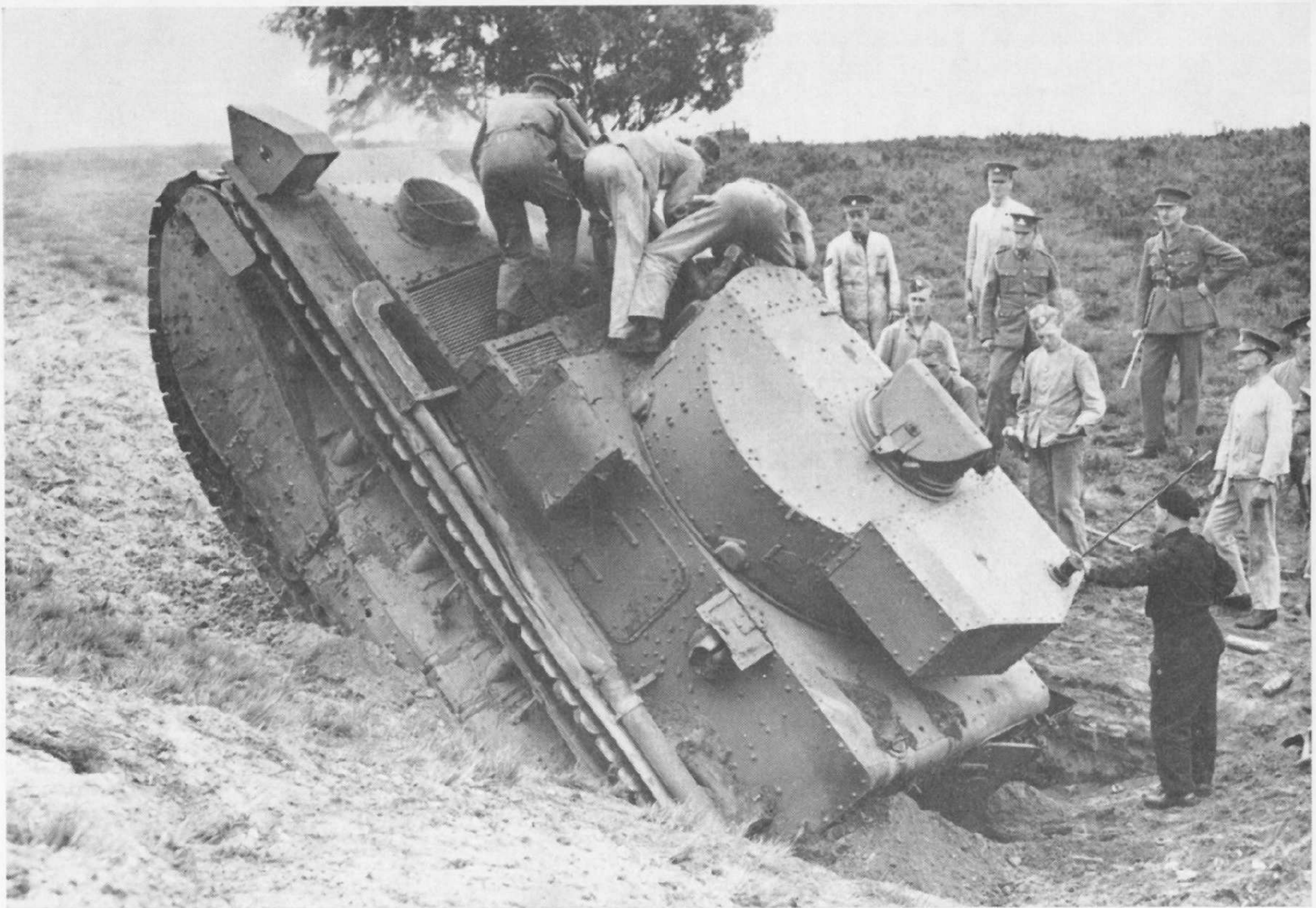
Mark IIA* in difficulties—caught in a pit dug by sappers to test tank stopping techniques.
