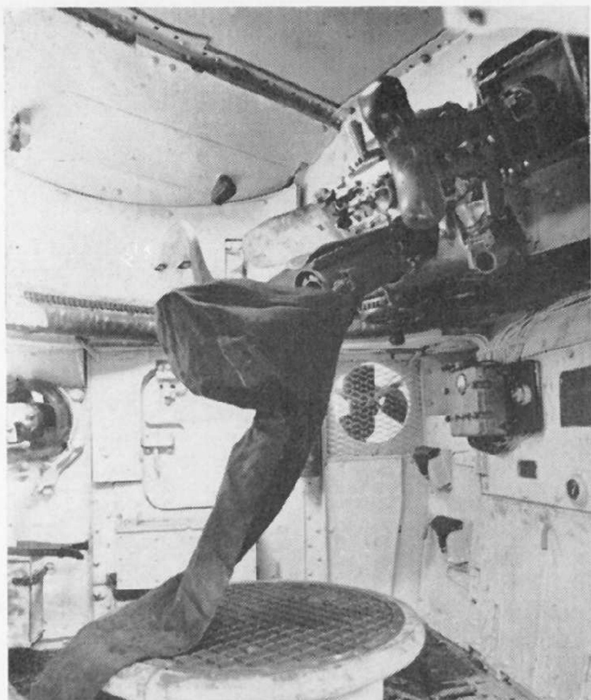
Interior of Mark IIA showing coaxial mountings and ventilating fan. (Imperial War Museum)
