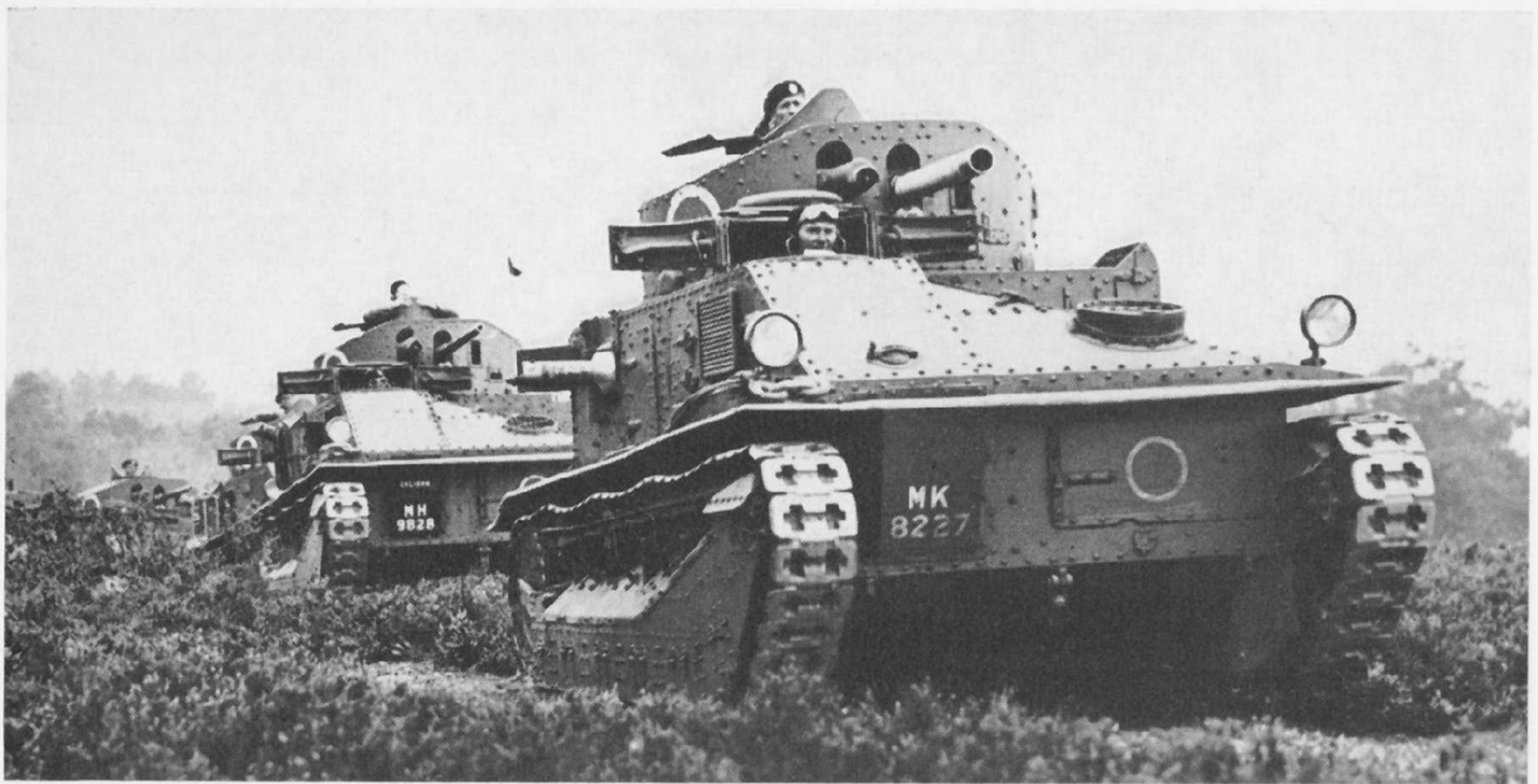
Mark II A CS. Note driver's hood open, with vizor divided in two and top hinged back—an arrangement common to all Mark IIs and variants. Because of Britain's tank shortage in 1940, especially after the fall of France, Mediums were brought back into service with operational units for a time. The tanks in this photograph, taken in England in autumn 1940, are probably of C Squadron, 3rd. Royal Tanks, part of 1st. Armoured Brigade, 2nd. Armoured Division, which sailed for the Middle East in November of that year.
