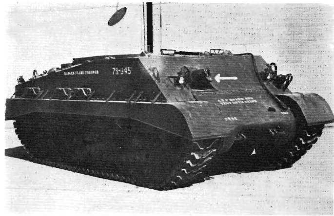
The Badger was a Kangaroo with Wasp flame-throwing equipment replacing the hull machine-gun. This picture shows the same conversion on a Canadian Sherman just post-war with the flame projector arrowed. (Canadian Official)
