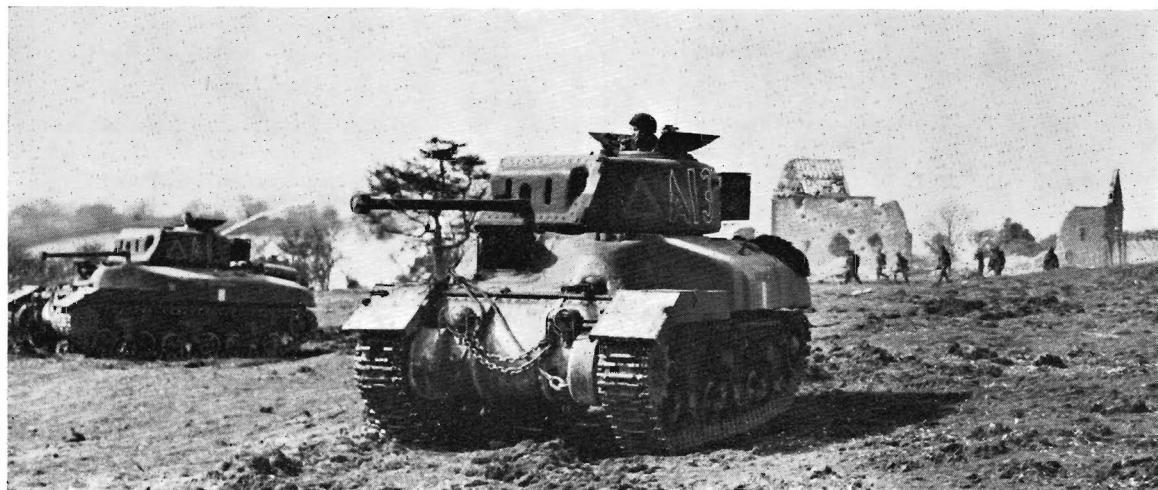
Another view of a very late production Ram Mk. II, this time fitted with C.D.P. steel tracks. Note the Mk. V 6-pdr. gun and the absence of the auxiliary turret. Date: May 1944.
