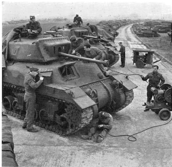
A late production Ram II in 1944 exhibiting all the final modifications. The auxiliary machine-gun turret is eliminated as are the side doors and the pistol ports in the turret. It has U.S. type steel tracks and bogies with trailing return rollers as fitted to the Sherman tank. Note the long Mk. V 6-pdr. gun with muzzle counterweight. Vehicle at rear is the earlier production type with pistol ports, auxiliary turret and Mk. III 6-pdr. gun.
