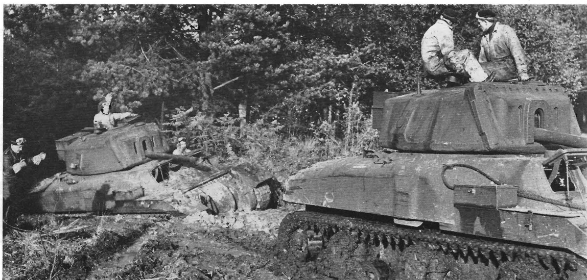
Late production Ram IIs displaying the absence of side openings in hull and turrets. These are on exercises in England in December 1943. (Imperial War Museum)
