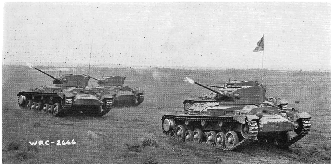
The first 30 Canadian-built Valentines were kept in Canada for training where three of them are seen here at Camp Borden. These very early vehicles had fabricated noses of riveted construction, though most Canadian Valentines had the cast nose. (Canadian Official)
