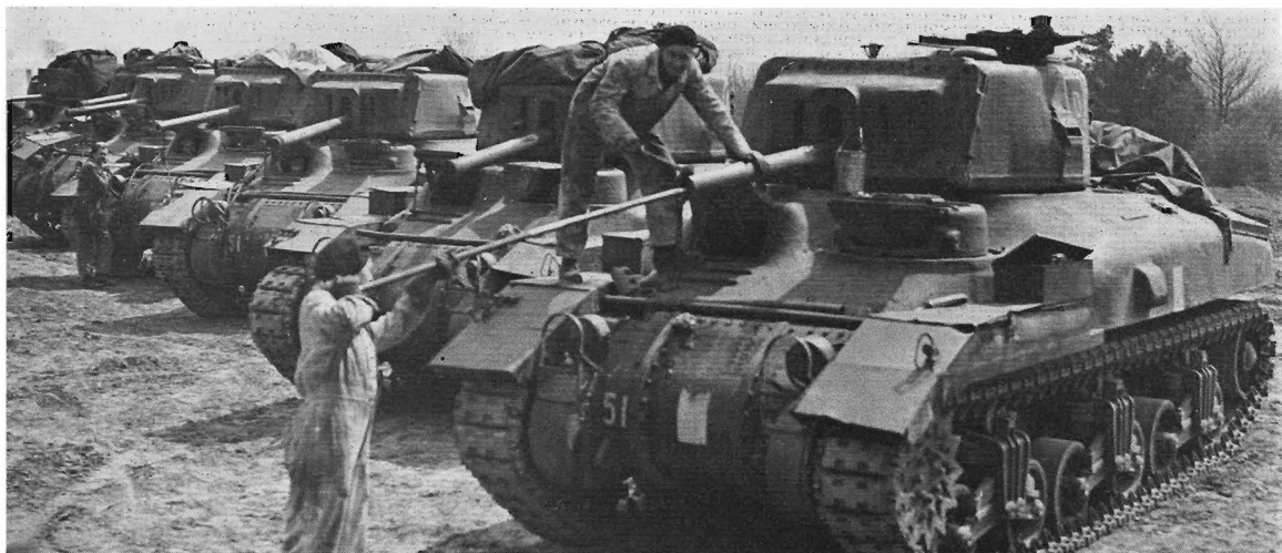
A fine line-up of Ram IIs from one of the Canadian armoured regiments in Britain in April 1944. The nearest three vehicles have the Mk. III 6-pdr. gun and the next two have the longer Mk. V 6-pdr. gun but with the usual muzzle counterweights removed. Note that the nearest vehicle is a late production Mk. II with the sponson doors eliminated but retaining the ventilator and the auxiliary machine-gun turret. (Canadian Official)
