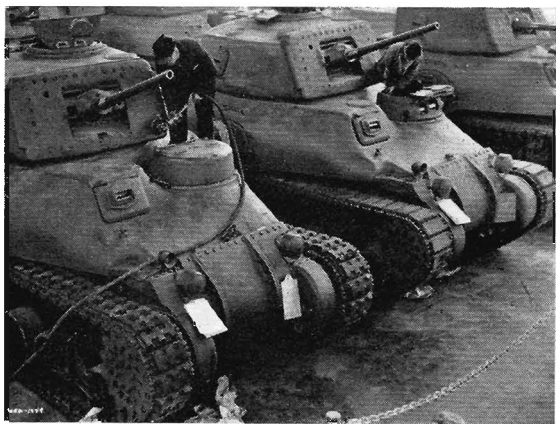
A view which contrasts the two types of American rubber shoe tracks used on most Rams. (Canadian Official)
