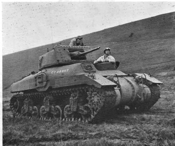
This view of a production Ram I with the Fort Garry Horse shows very clearly the origin of the 2-pdr. mantlet which was taken straight from the Valentine tank. (Chamberlain Collection)
