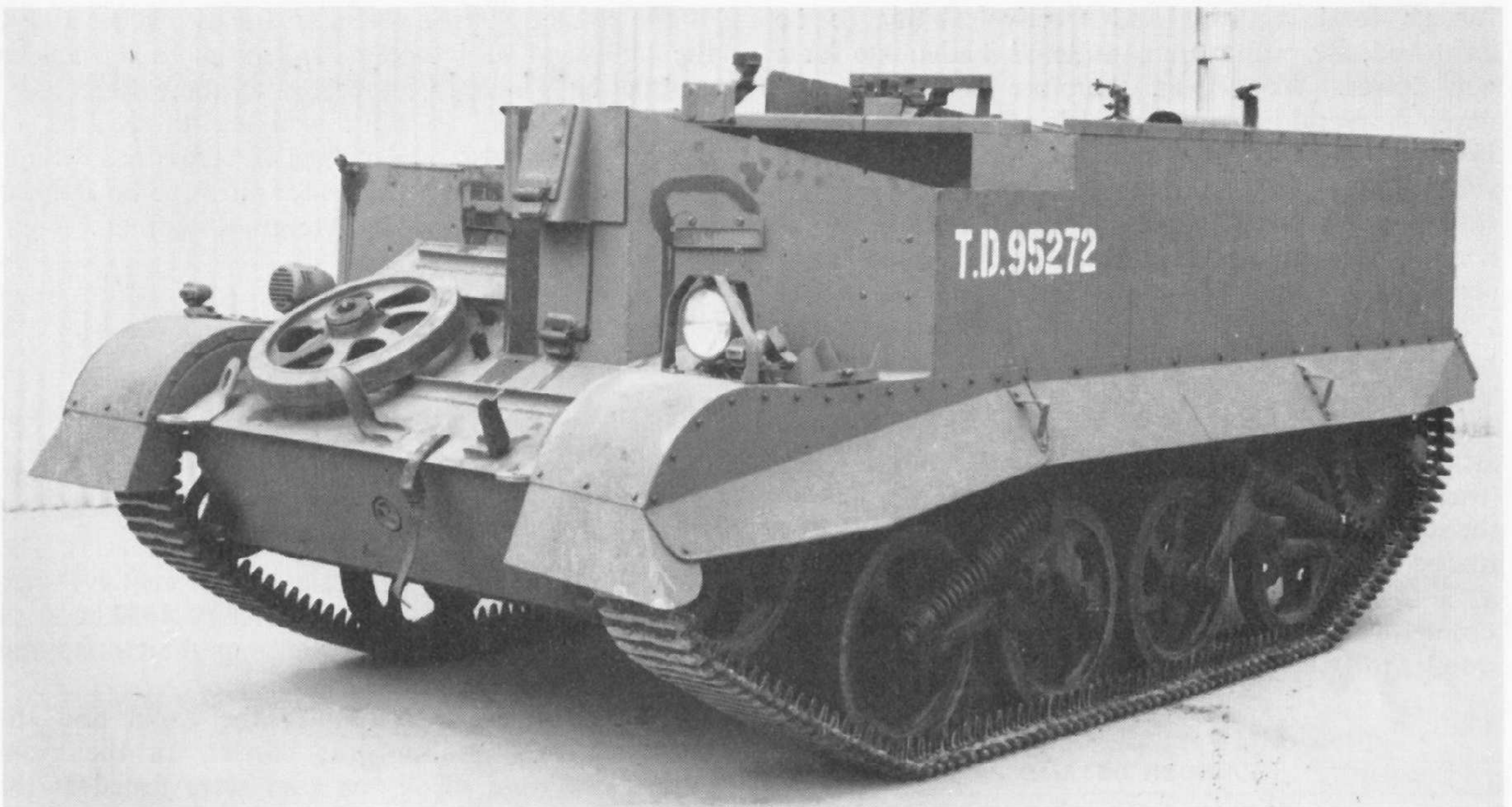
Carrier, Universal, T.16. Designed and built in the United States, this was an attempt to develop a more satisfactory vehicle than the Universal Carrier. The principal changes in design were the use of the controlled differential steering system, Ford Mercury engine, two two-wheeled bogies on each side, refinement of the track and suspension, and a lengthened welded hull structure.
