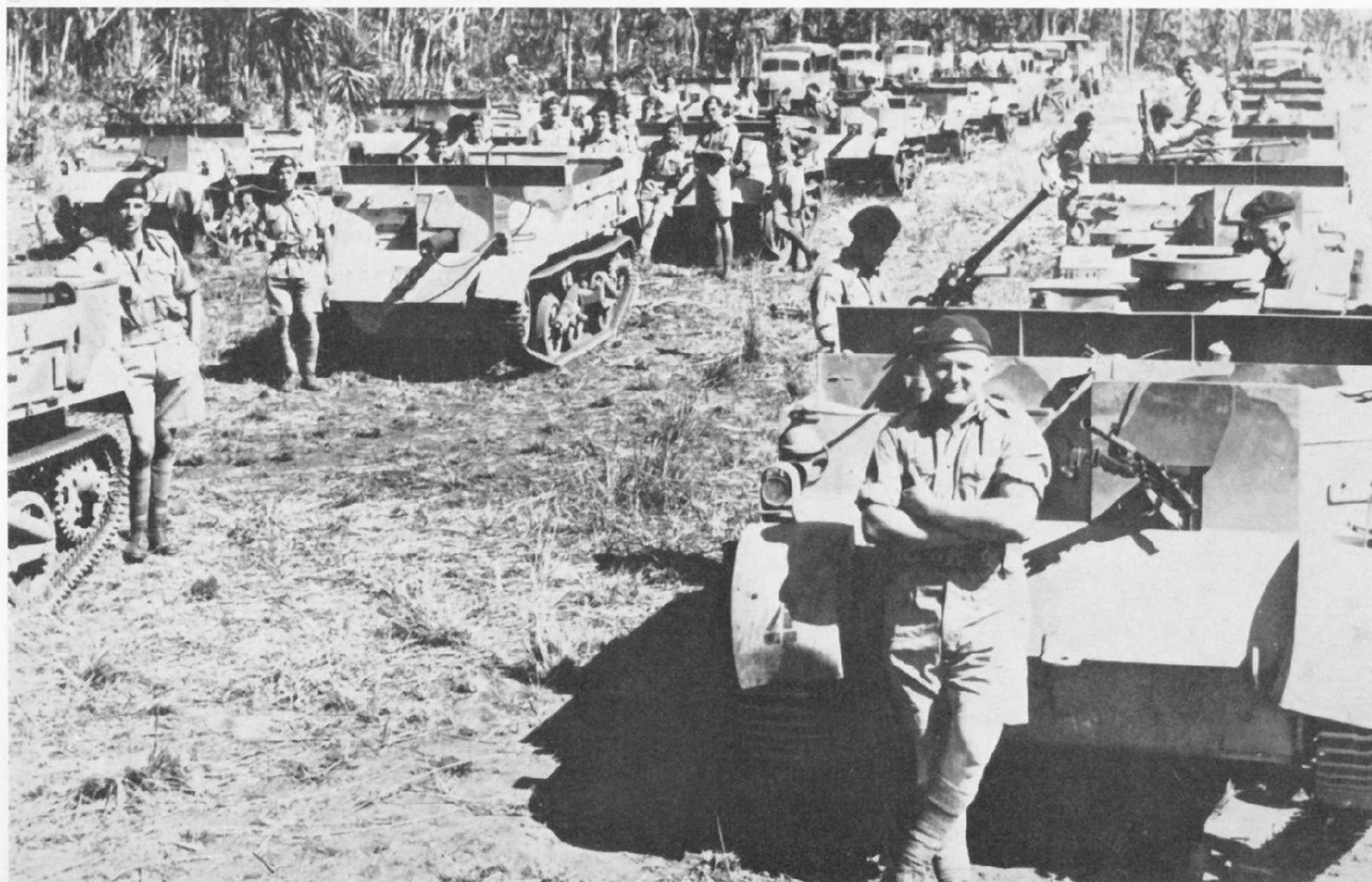
Universal Carrier, MG, Local Pattern, No. 2, Australian-built, all welded and Australian manned.
