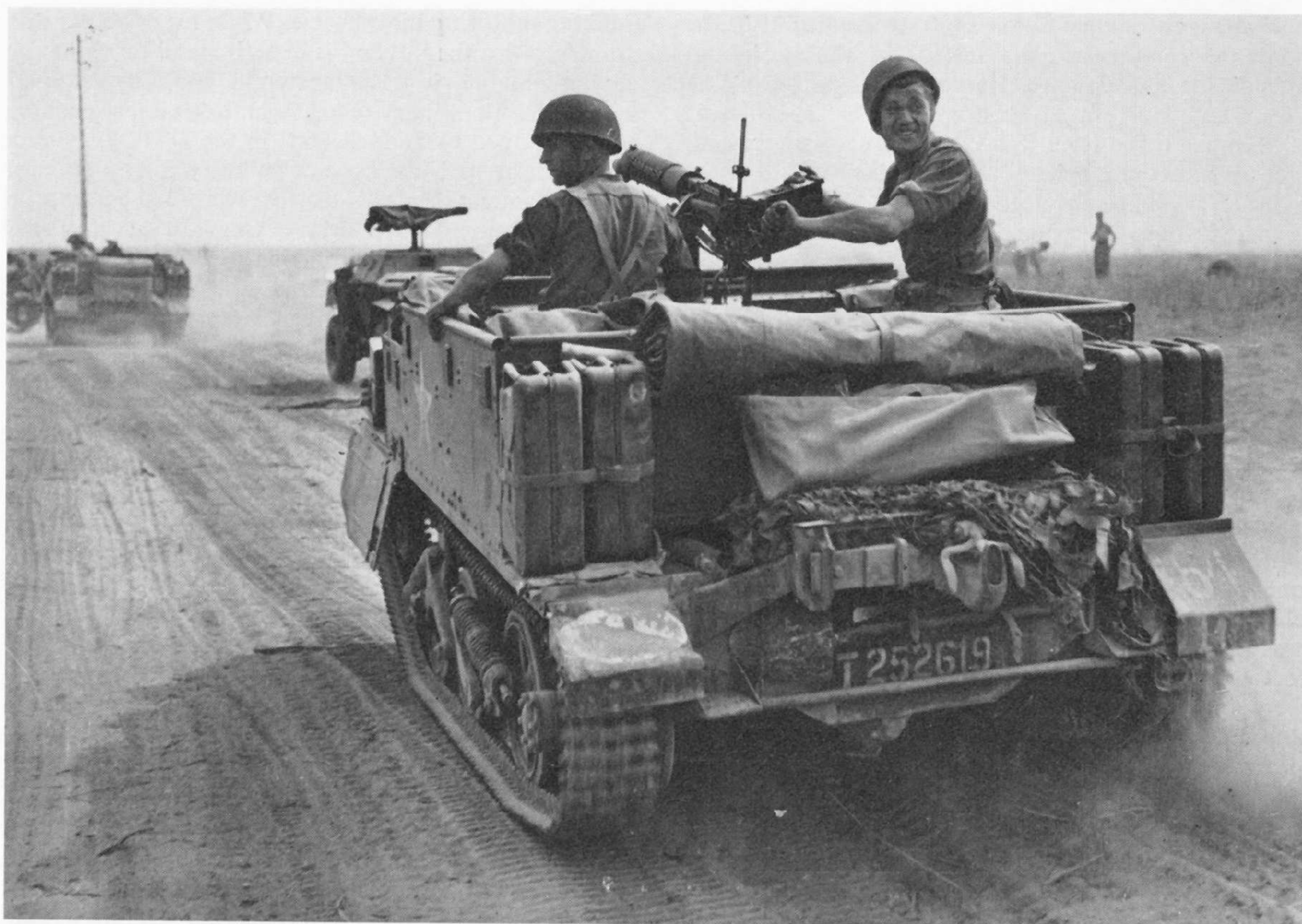
Universal Carrier Mark II with Canadian crew south of Caen in the battle for Falaise, August 9, 1944. Note mudguard shape and Stacey towing attachment. Vehicle has been modified as a medium machine-gun carrier.
