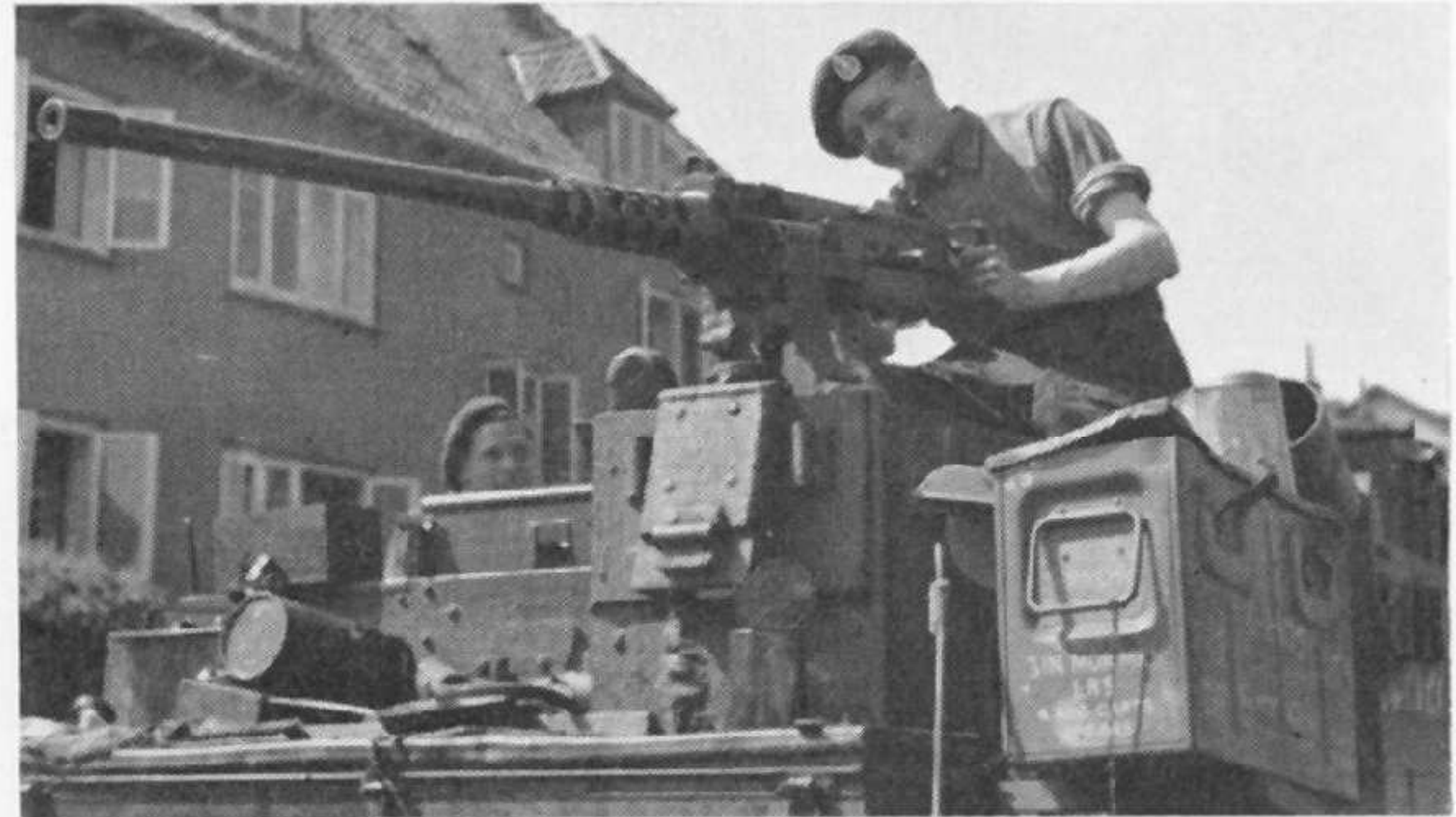
Three-inch mortar Carrier, Mark II, with .50 Browning machine-gun mounted in front.
