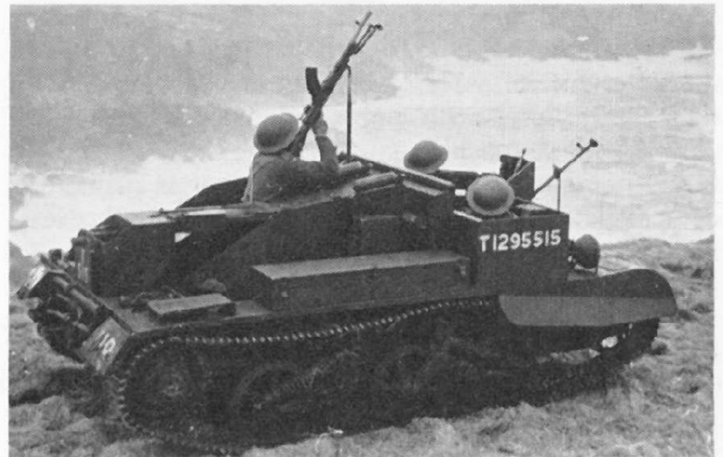
Below: Carrier, Scout Mark I, showing the pedestal-mounted Bren gun, with an alternative anti-aircraft mount. On this class of vehicle the built-up superstructure was reversed from that on the Bren Carrier.
