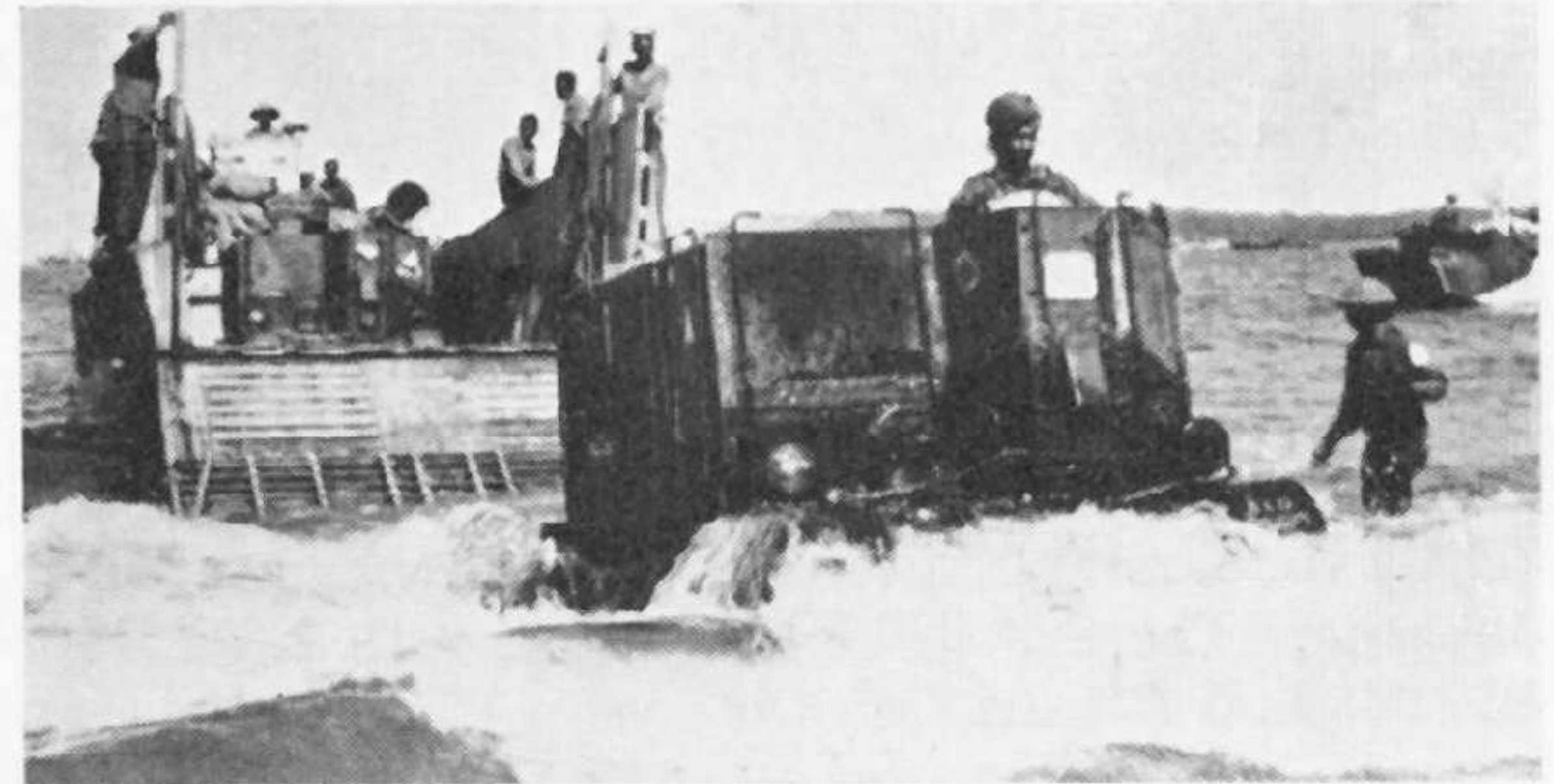
Universal Carrier fitted for wading with heightened hull disembarking on Ramree Island, Arakan, January 1945.
