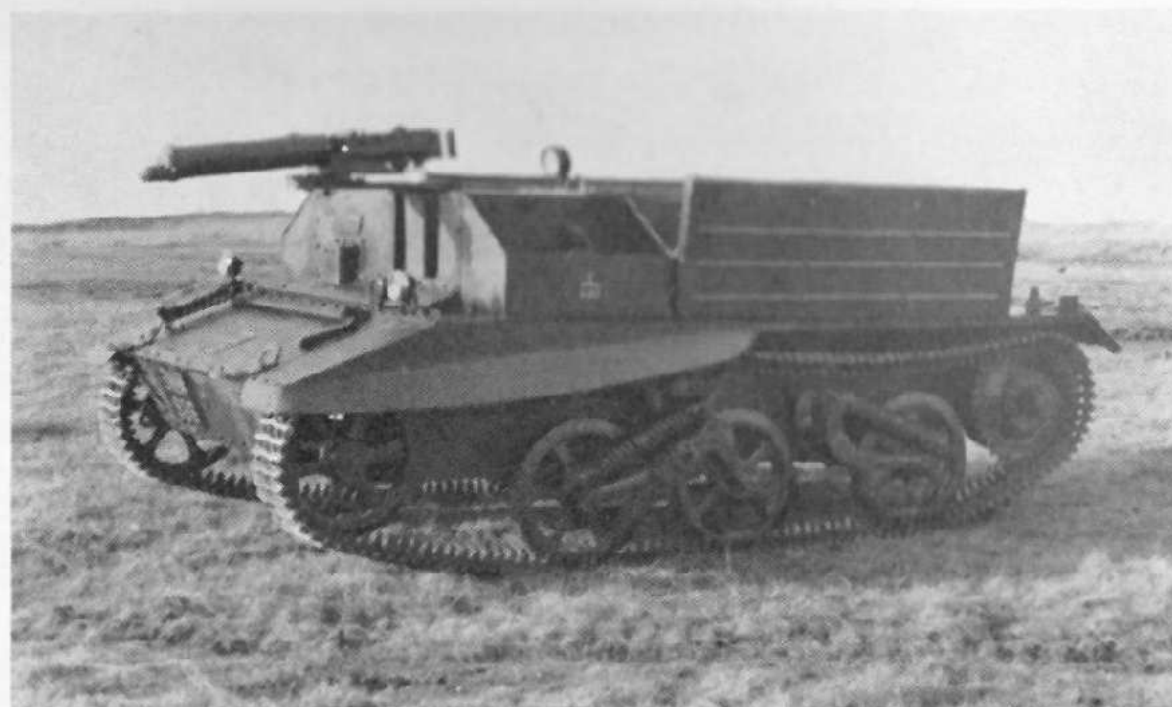
The second experimental machine, designated Carrier, Machine-Gun, with same type of chassis as that of Light Dragon Mk. III but with superstructure adapted for its rôle of machine-gun carrier. Note stowage bin and folding armoured side, and one of the methods of mounting the machine-gun.
