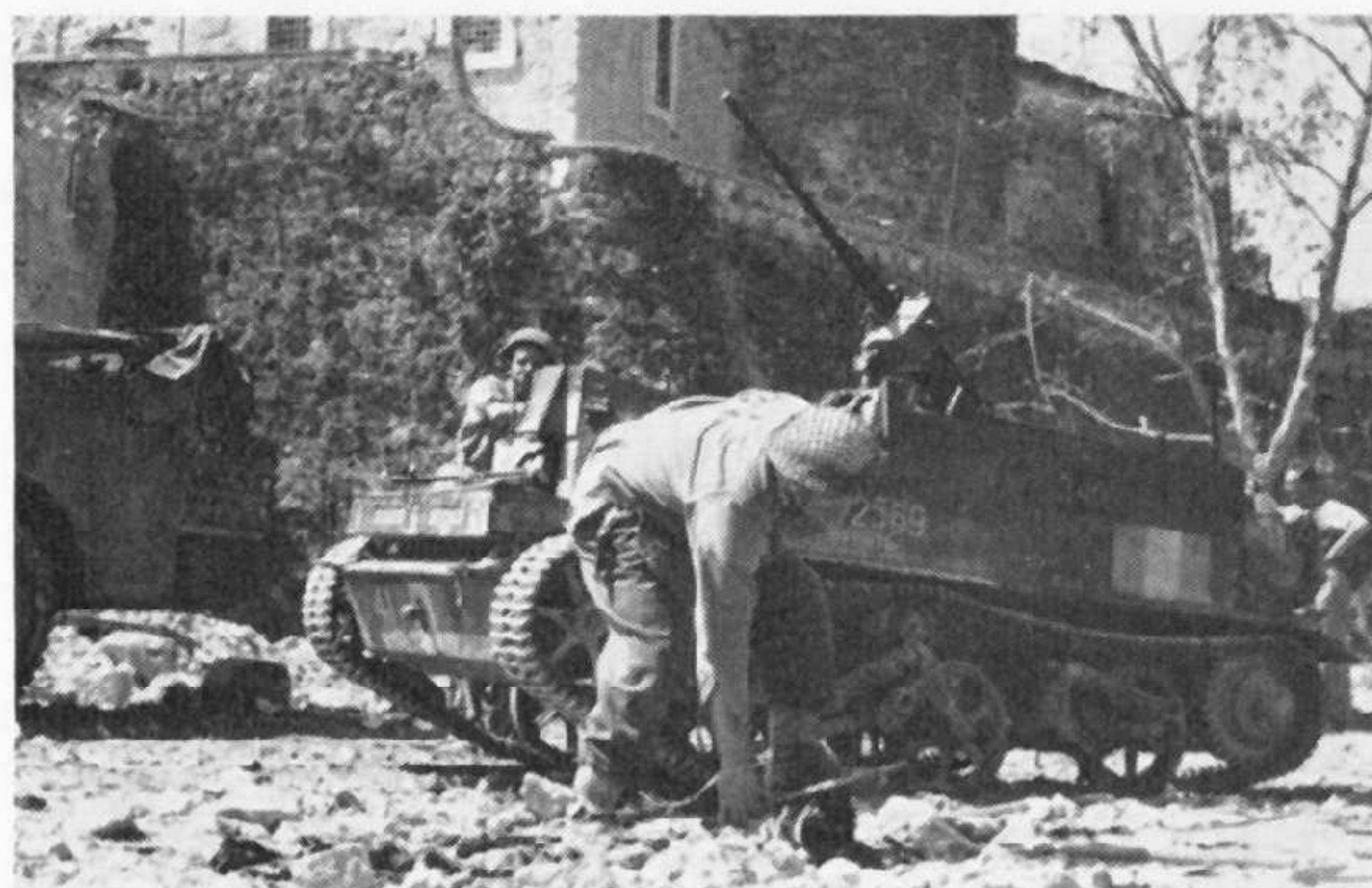
Universal Carrier in Italy fitted with .50 Browning machine-gun in rear compartment.
