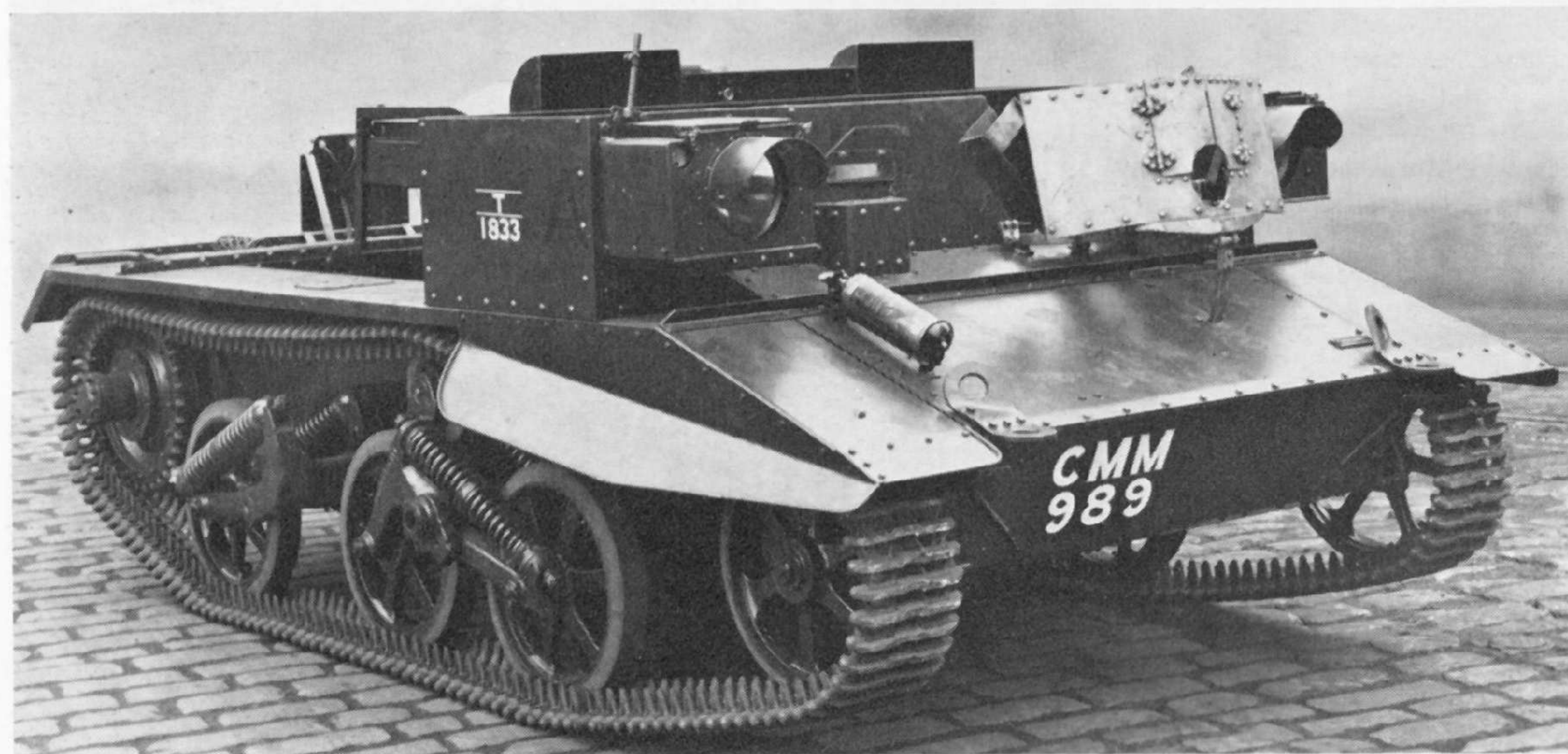
Carrier, Machine-Gun, No. 1, Mark I. Developed from the Experimental Machine-Gun Carrier, this was the prototype of the carriers of the Machine-Gun and Bren series. The view shows the armoured box front headlamps and the small armoured shield for the machine-gun.
