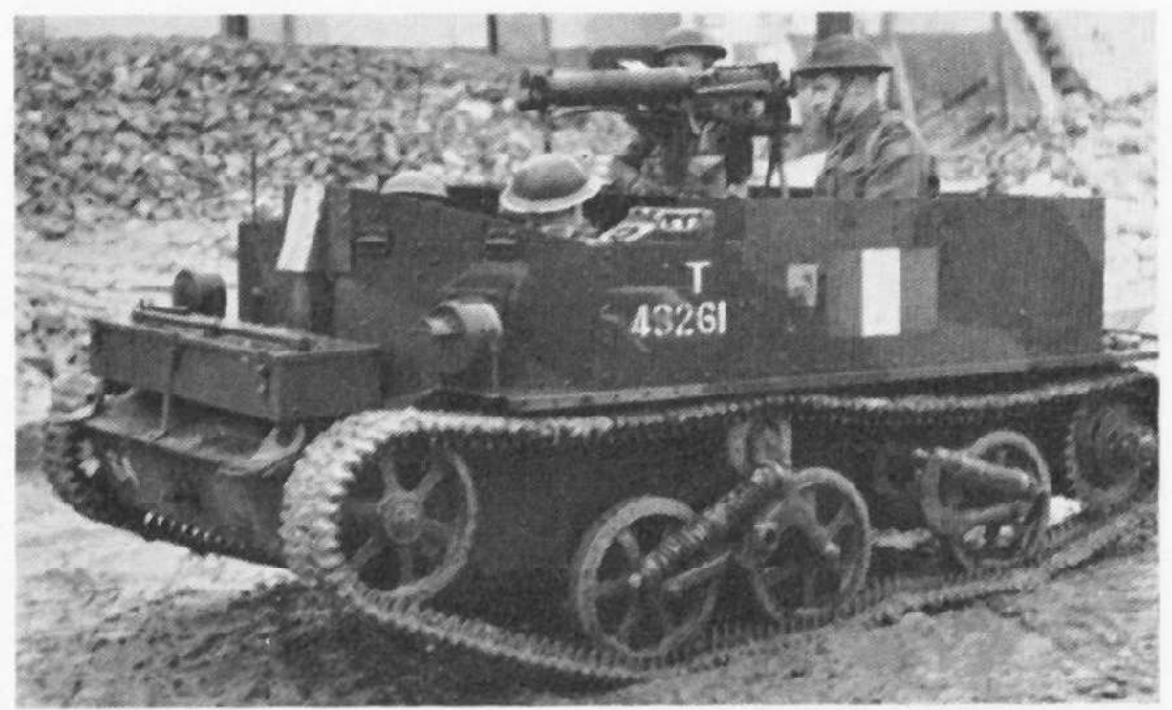
Carrier, Medium Machine-Gun No. 3, Mark I. Canadian built Universal Carrier adapted to the MMG rôle.
