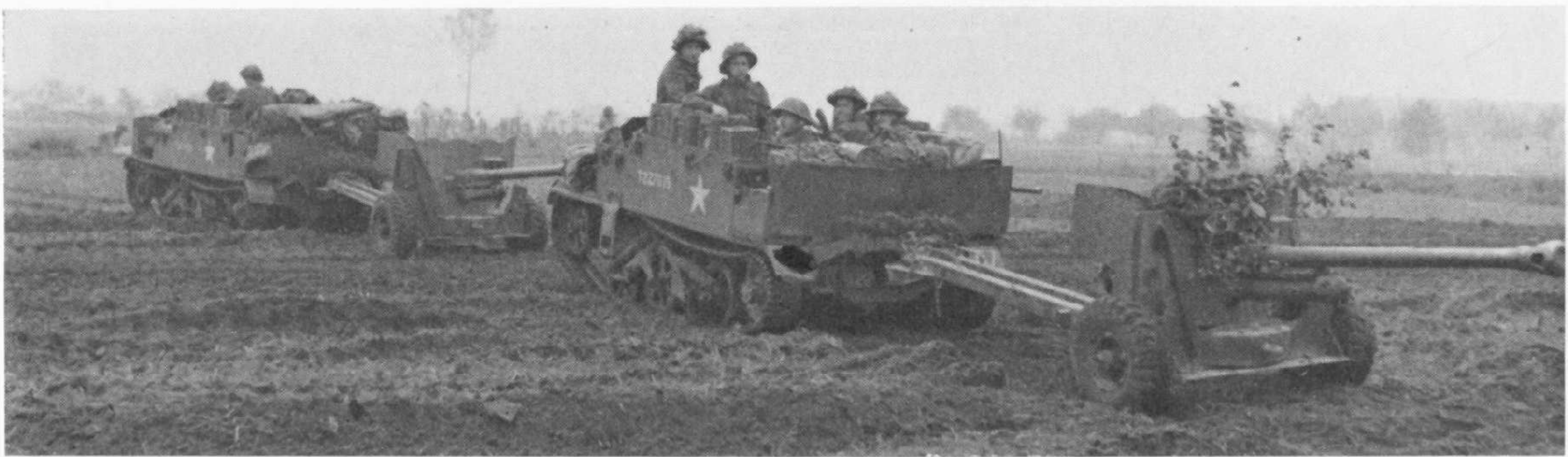
Universal Mark IIs towing 6-pdr. anti-tank guns in Holland, October 1944.
