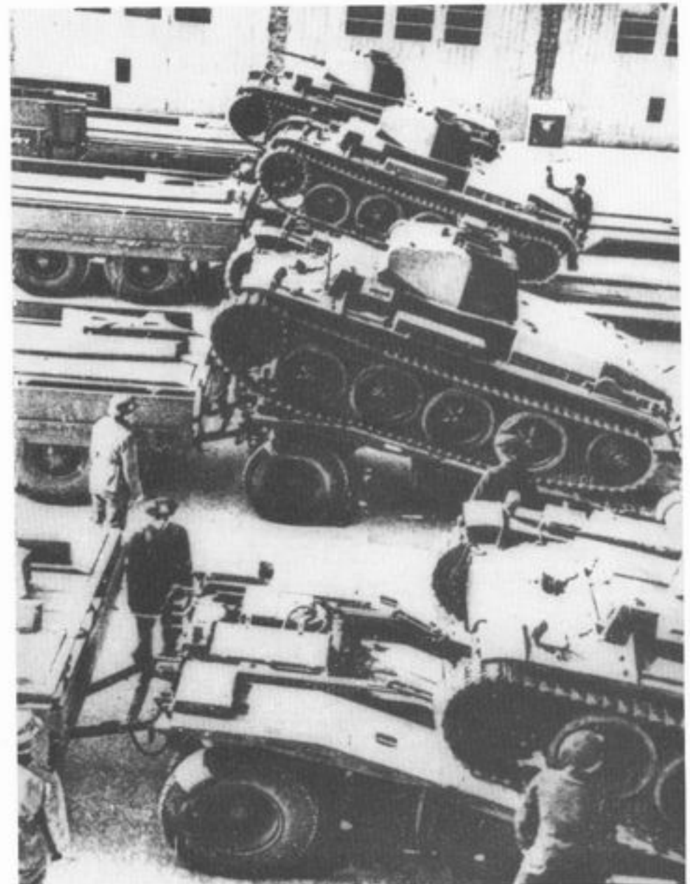
Panzer II Ausf. D and E being loaded on to transporters. Note large Christie-type suspension wheels. (Photo: R.A.C. Tank Museum)
