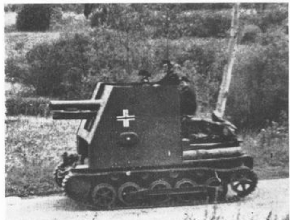
150-mm. infantry support gun (Infanteriegeschütz 33) on a Panzer I Ausf. B chassis. (Photo: Imperial War Museum)
