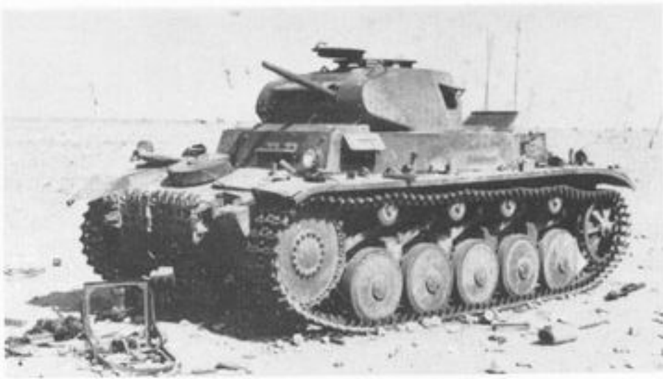
Panzer II Ausf. B (note cupola and absence of horn-type periscope) knocked out in the Western Desert fighting. (Photo: Imperial War Museum)
