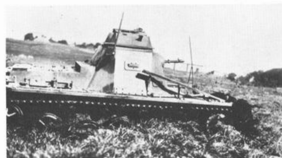
Right side view of Kleiner Panzer Befehlswagen. Panzer I Command Tank with non-rotating turret and single MG. (Photo: Imperial War Museum)
