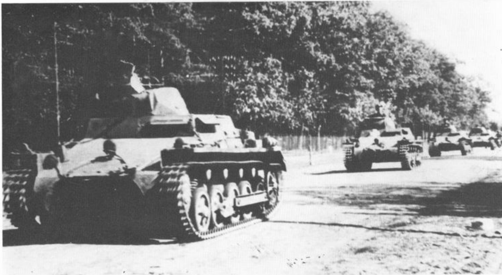
Panzer I Ausf. Bs entering Warsaw after it had been forced to capitulate on September 27, 1939. Note five suspension wheels and four return rollers. (Photo: Imperial War Museum)
