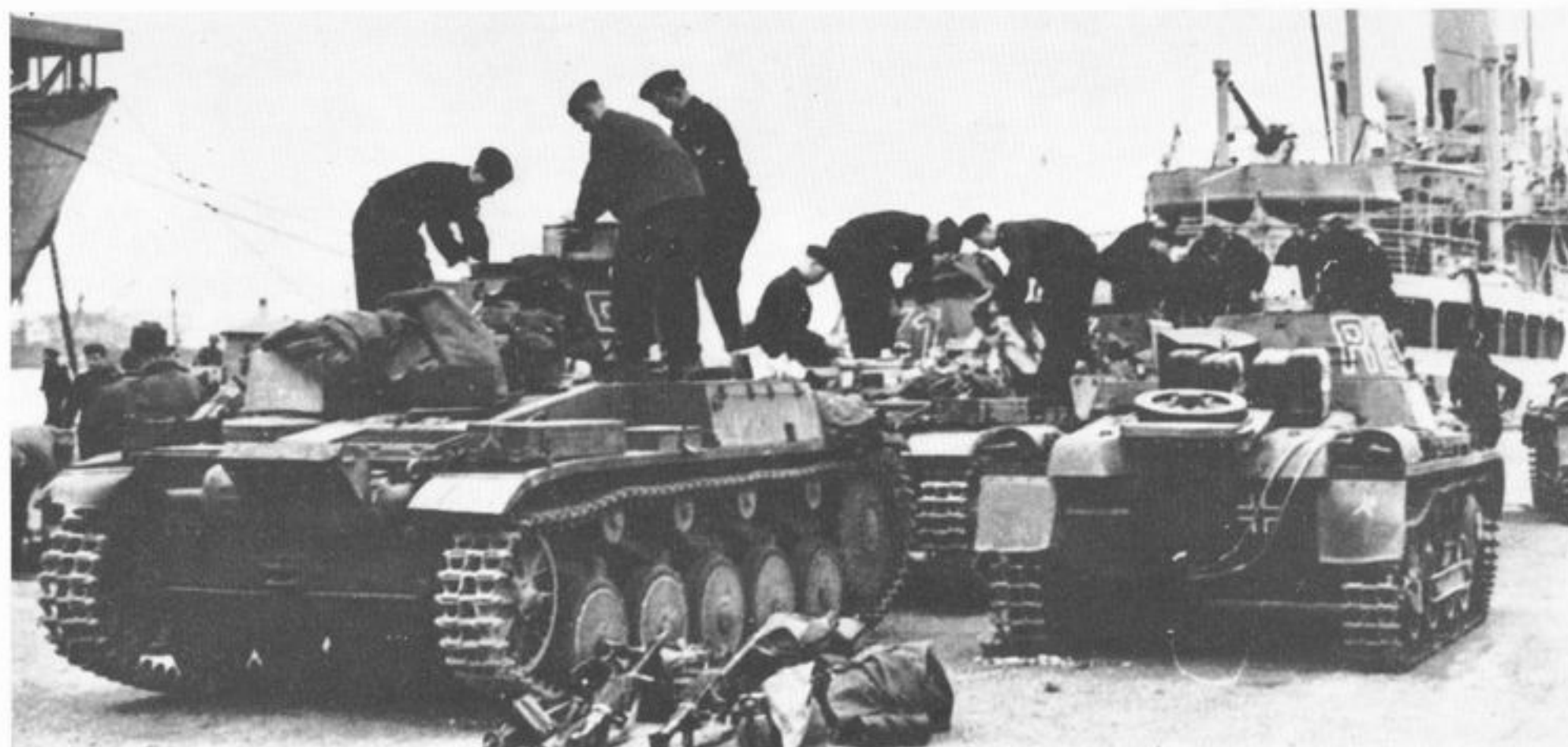
Panzers I and II being prepared for embarkation. Apparatus for discharging smoke is fitted at tail. Note divisional sign on right-hand mudguard of right-hand tank and on tool chest of left-hand tank. (Photo: Imperial War Museum)
