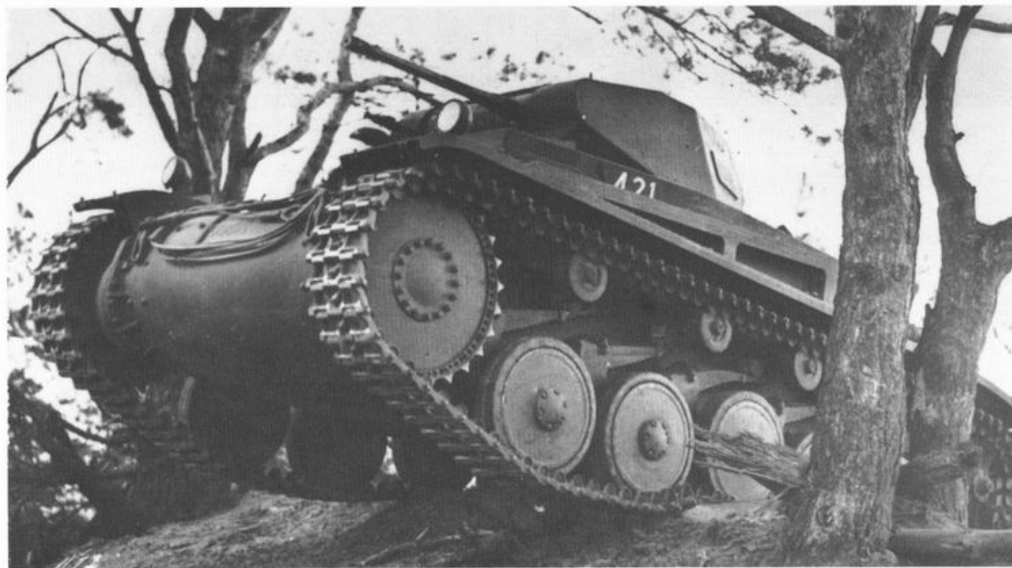
Pz Kpfw II Ausf. c in November 1939. Note cast rounded nose plate and medium-sized suspension wheels which identify it. Compare angular welded nose plate of subsequent Ausf. A. (Photo: Imperial War Museum)
