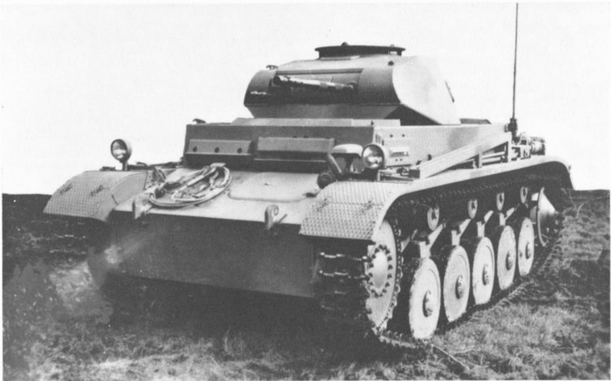
Panzer II Ausf. F which was up-armoured on turret and nose. The visor beside the driver's true visor (under the 20-mm. gun) was a dummy, presumably to confuse enemy anti-tank gunners. To complete the illusion there was also a vision slit on the off-side superstructure to match the one seen here on the near-side. Conical idler wheel was also a feature of Ausf. F.
