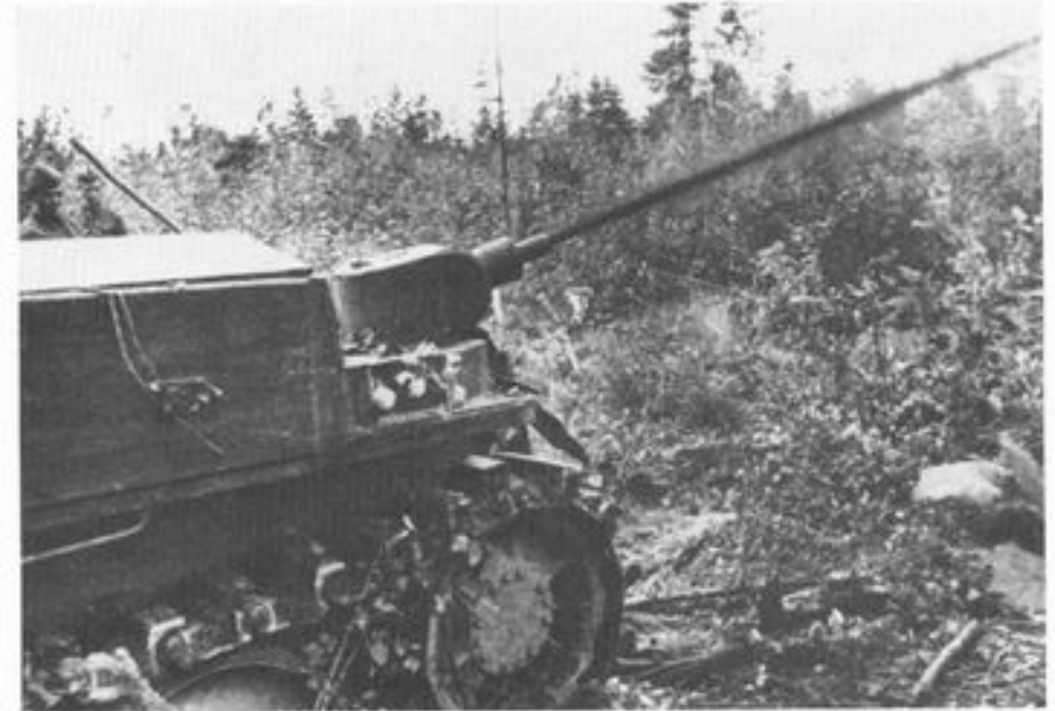
Flammpanzer II—Ausf. D or E modified as flame-thrower, showing location of flame-gun and rod of fuel which has apparently not ignited. Vehicle is in Russian hands having been captured on Leningrad front. (Photo: R.A.C. Tank Museum)
