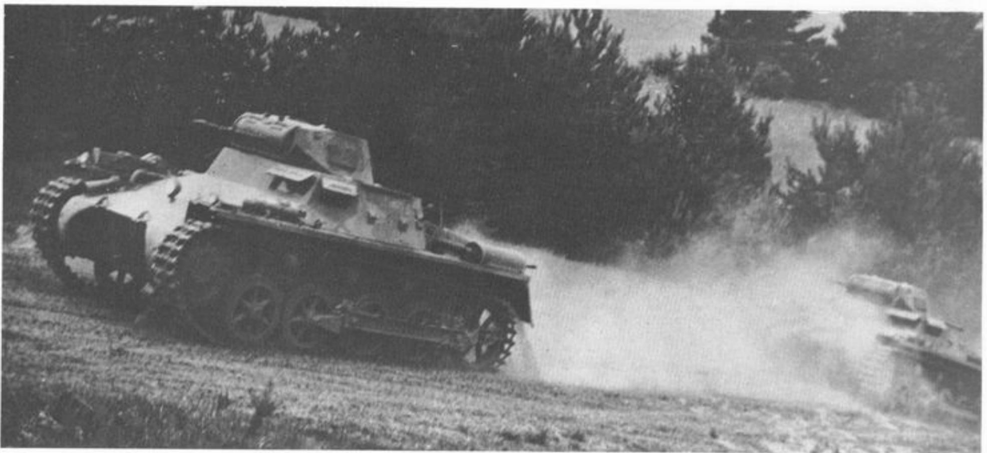
Pz Kpfw I Ausführung (model) A distinguished from Ausf. B by the four suspension wheels and three return rollers. (Photo: Imperial War Museum)
