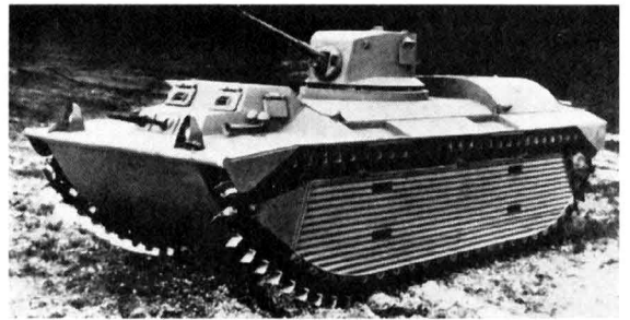
Borg-Warner Experimental Model A, the forerunner of the LVT (A) 1 and LVT (A) 4, constructed of aluminum and fitted with M3 Light Tank turret and gun.
