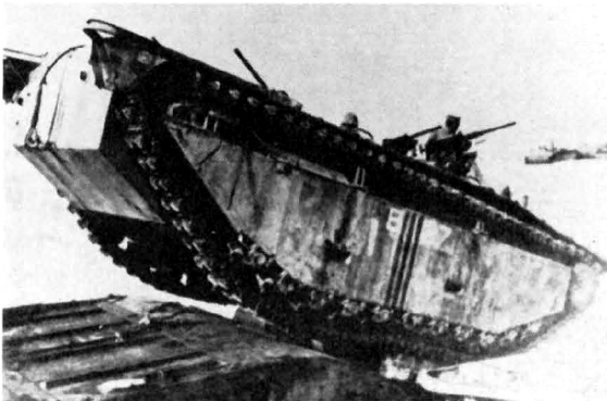
An LVT 2 going down the ramp of a landing craft to take to the water.
