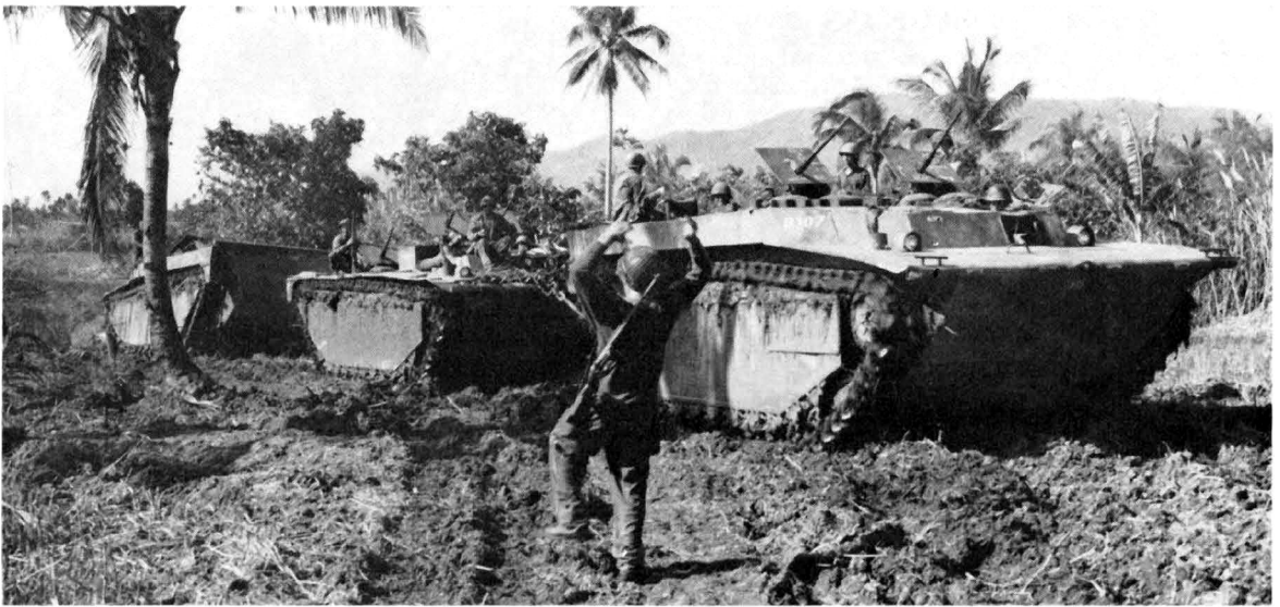
An LVT 4 and an LVT 2 with bolt-on armor pulling a disabled LVT 4 on Leyte Island.
