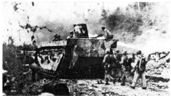
The LVT 3 fitted with Ronson Flamethrower was of considerable use on Peleliu.
