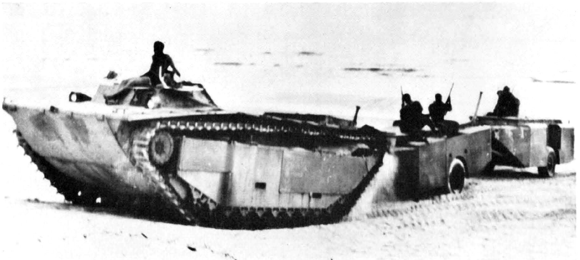
LVT 2 pulling two of the special amphibious trailers found so useful for carrying supplies.
