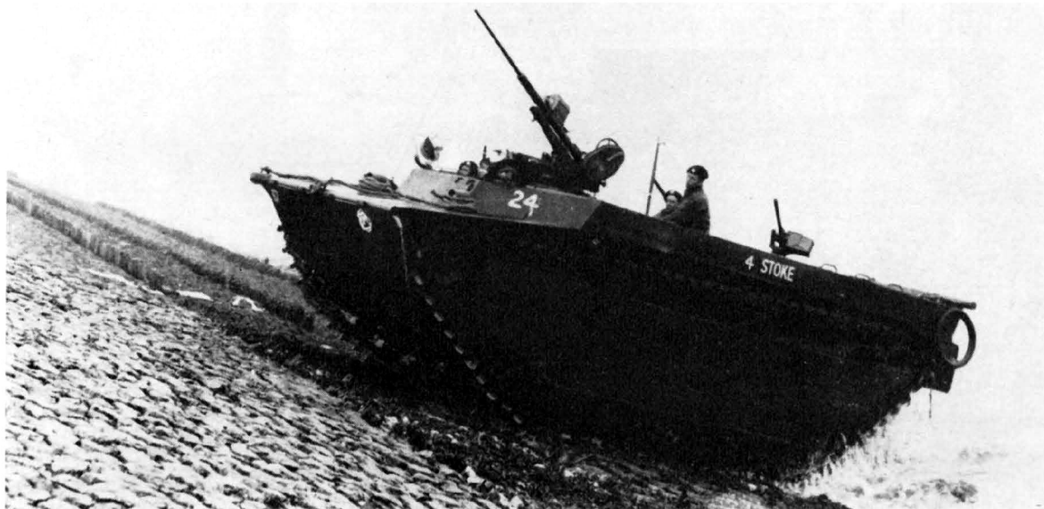
British Amphibian, tracked, 2TG, 5 (LVT (A) 2), armed with 20 mm. Polsten cannon.
