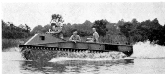
LVT 1 Prototype undergoing tests at Aberdeen proving ground. (Photo: U.S. Ordnance Dept.)
