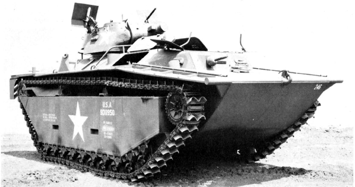
LVT (A) 5 with stabilized M8 Howitzer carriage power traverse turret.
