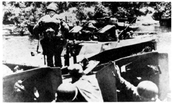
Another type of shield for LTV armament was common. (Photo: U.S. Marine Corps)
