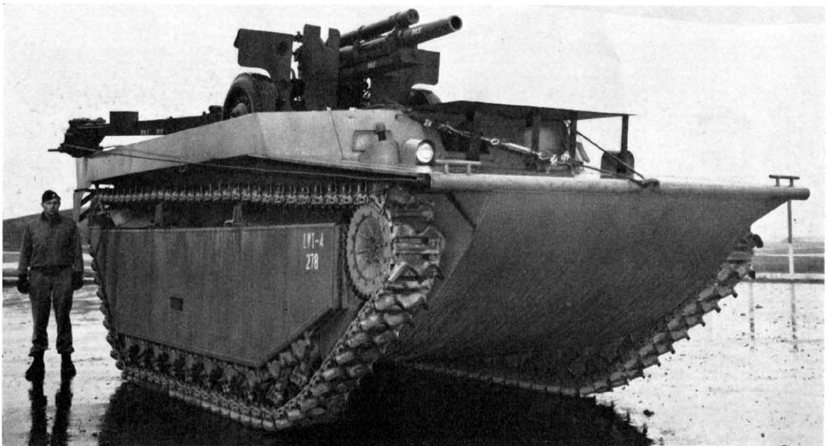
LVT 4 modified to carry a 105 mm. Howitzer on standard field carriage. (Photo: U.S. Ordnance Dept.)
