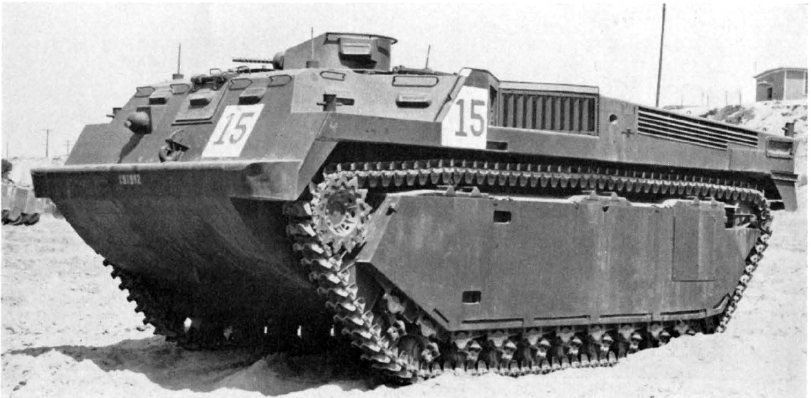
Standard LVT 3C as modified after World War II to cover top and add MG cupola.
