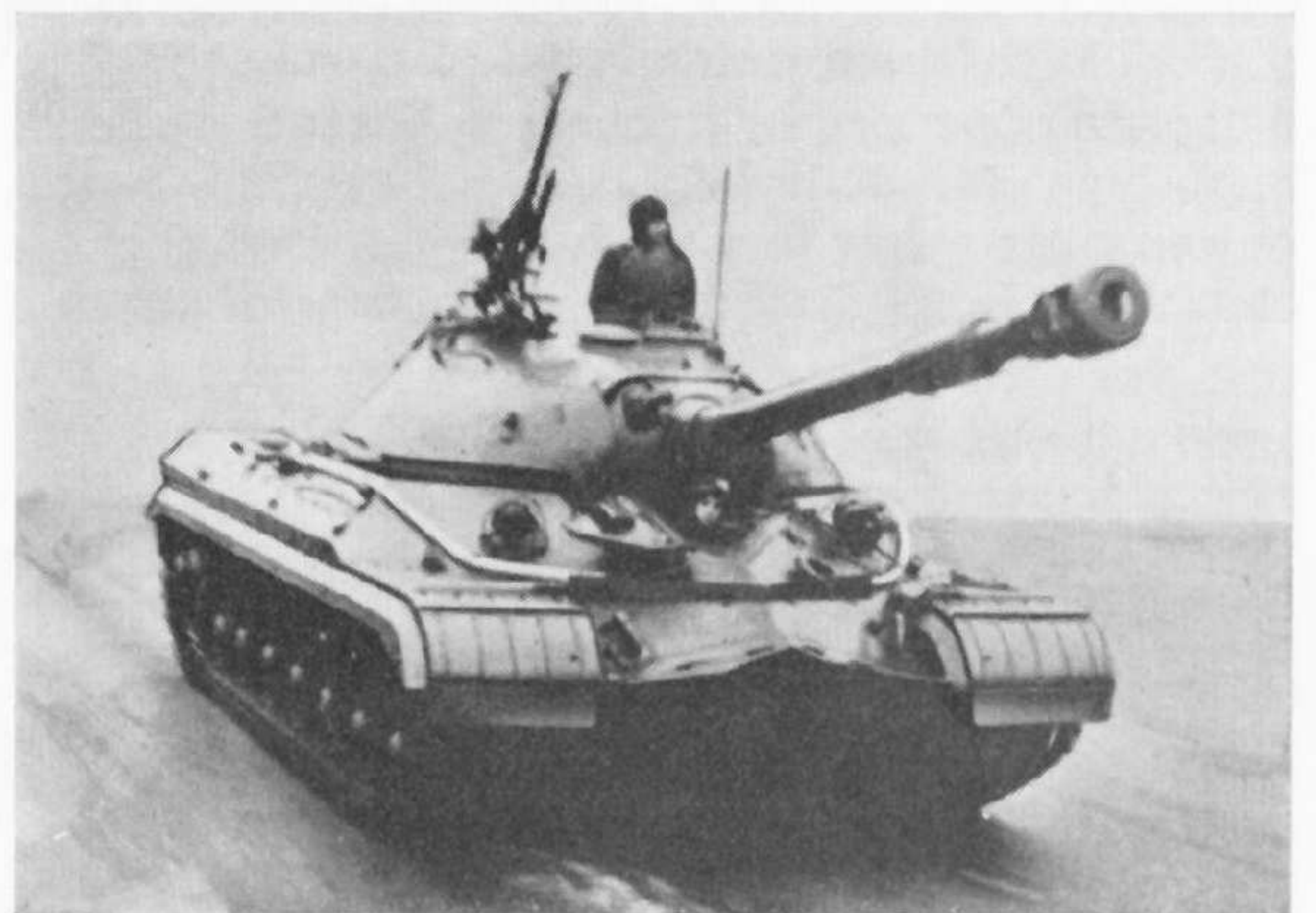
T-10. Its derivation from the basic IS-3 design can be seen clearly. The new 122 mm. has a fume extractor as well as a muzzle brake. (Crown Copyright Reserved)
