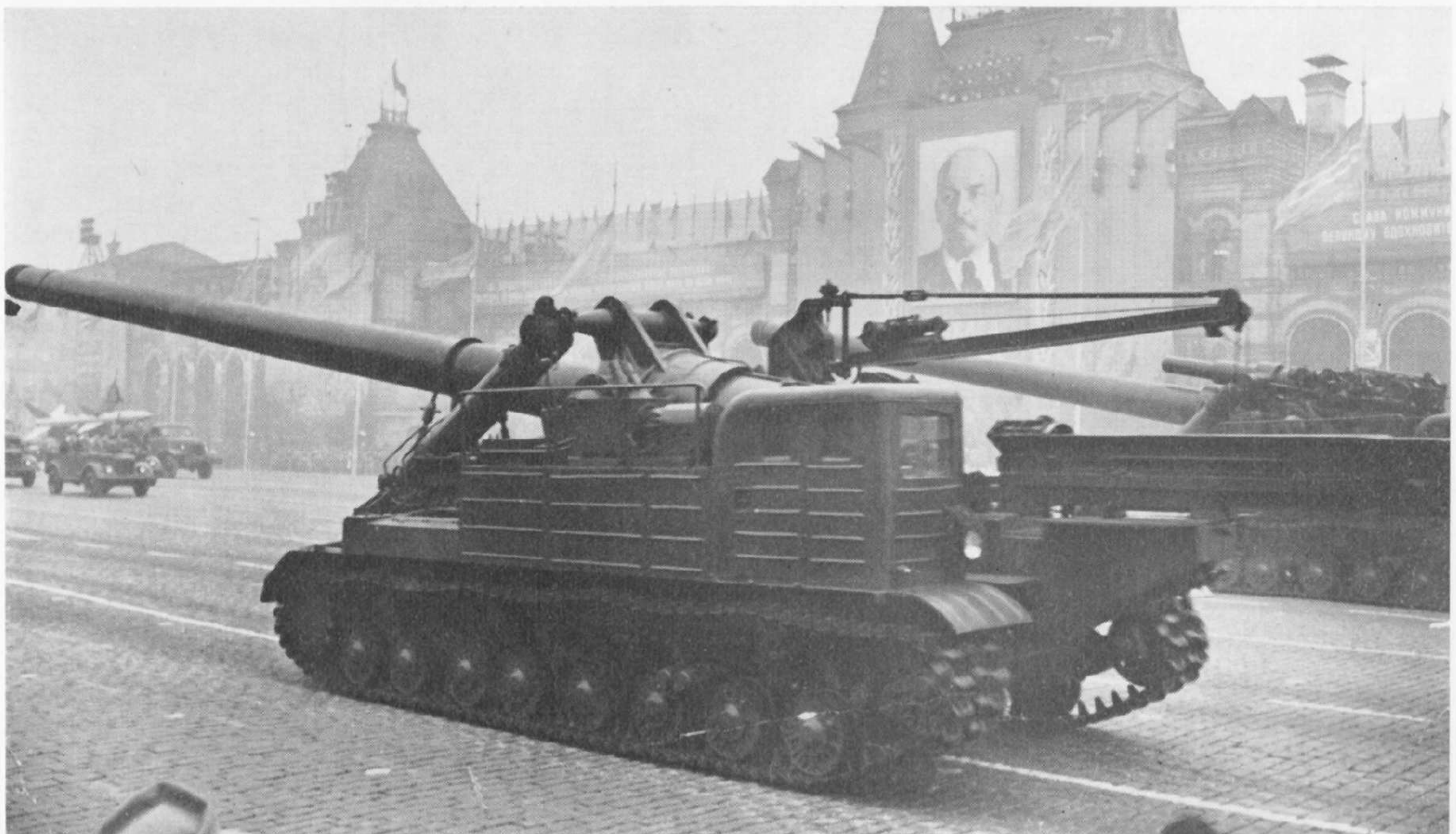
IS/C, a lengthened and much modified IS chassis mounting a 300 mm. tube launcher, on parade in Moscow in 1957.
