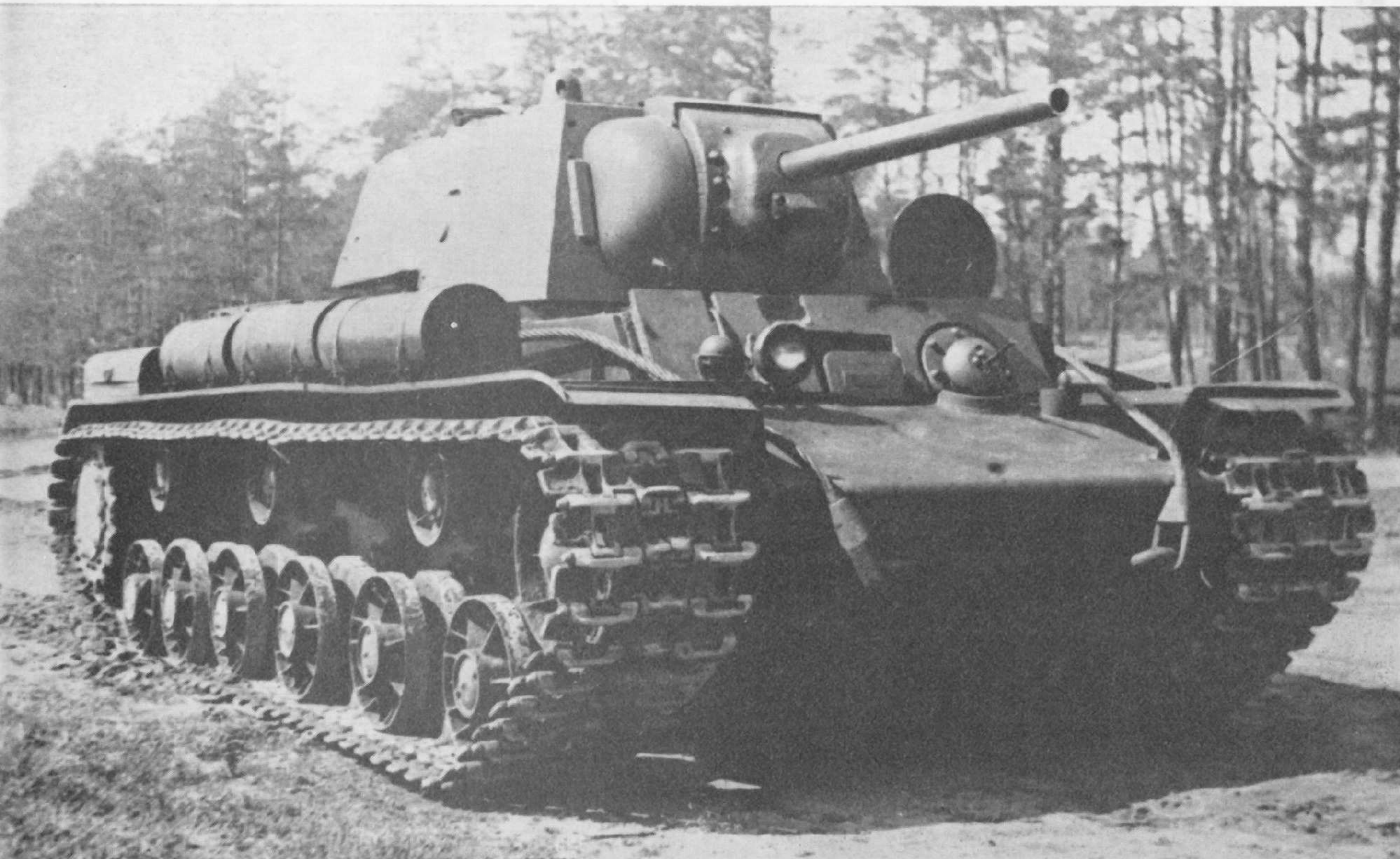
A KV-1A. The upward continuation of the front plate to protect the turret ring and the bar welded to the turret front to protect the trunnions can be seen clearly. (Crown Copyright Reserved)
