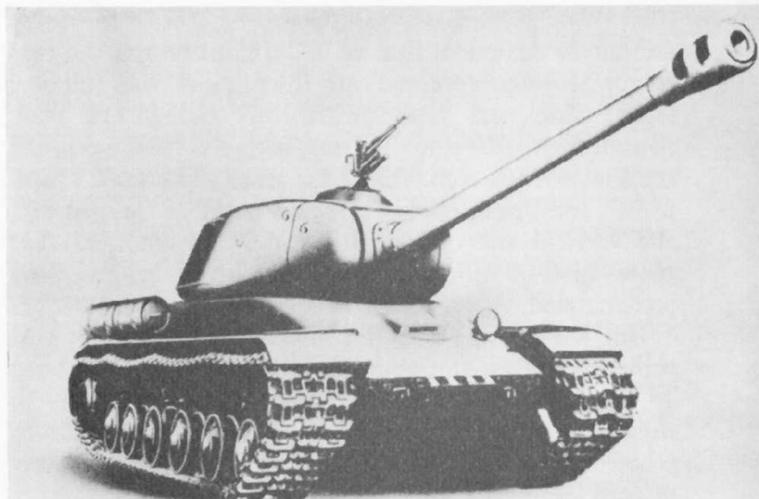
The IS-2 with a uniformly sloping glacis plate compared with the bent plate on the IS-1. Note also the change in the driver's vision device. (Crown Copyright Reserved)
