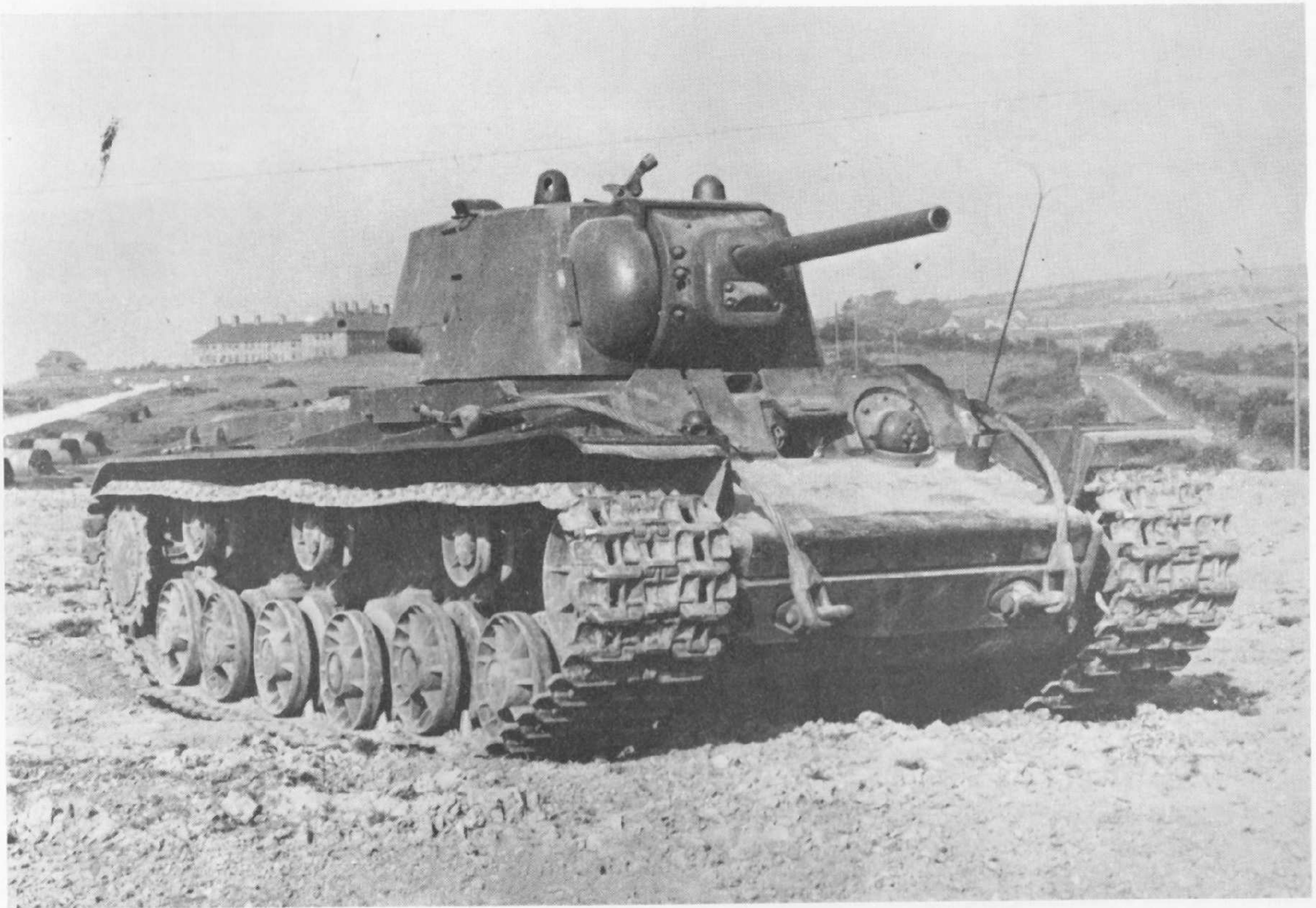
A KV-1C on test in England during World War II. Note the unusual design and mounting of the radio antenna on the glacis plate. This vehicle is now on display in the R.A.C. Tank Museum in Bovington. (R.A.C. Tank Museum)
