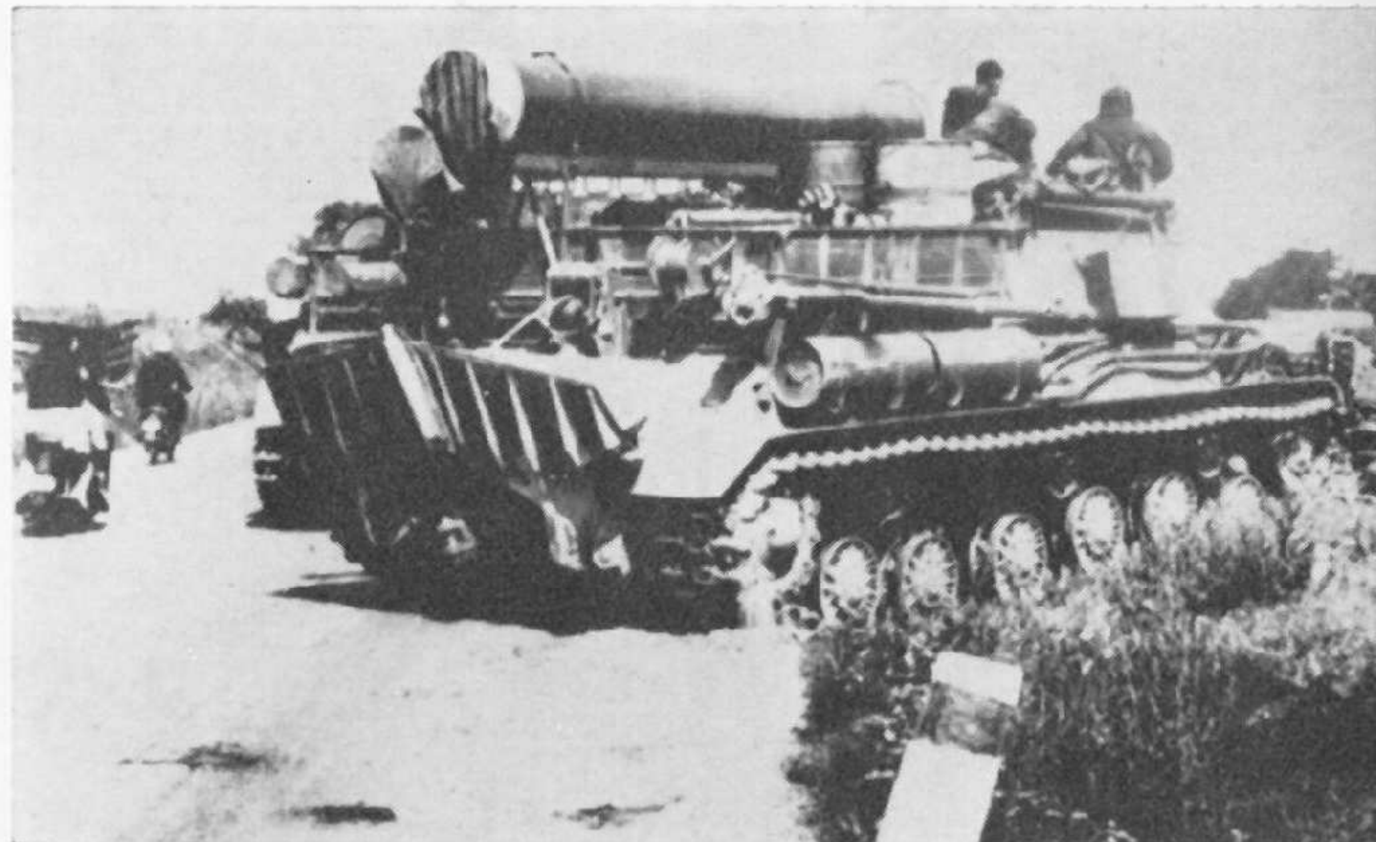
An ISU-TD recovery vehicle in Czechoslovakia in August 1968. The snorkel tube stowed horizontally and the large anchoring spade at the rear can be seen clearly. (dpa)
