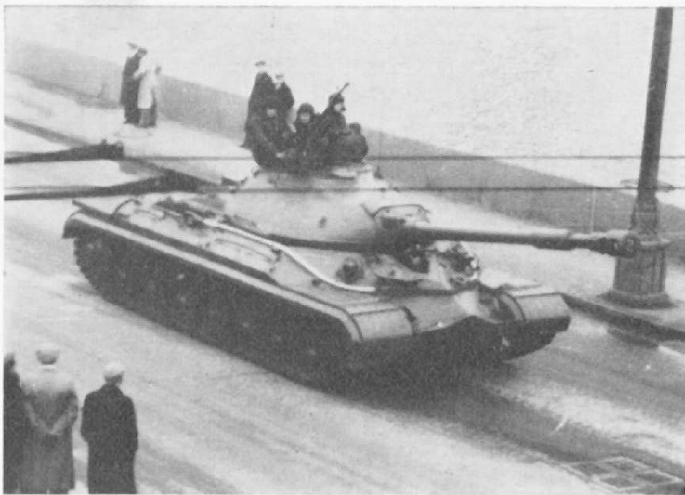
A T-10. The relative size of the turret compared with its three occupants indicates the cramped conditions in which they work. (R.A.C. Tank Museum)
