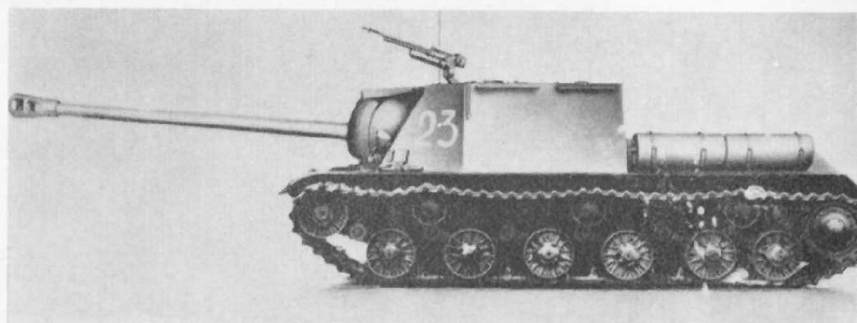
ISU-122A (or SU-249) mounting the D-25S 122 mm. gun as used in IS-3. (Imperial War Museum)
