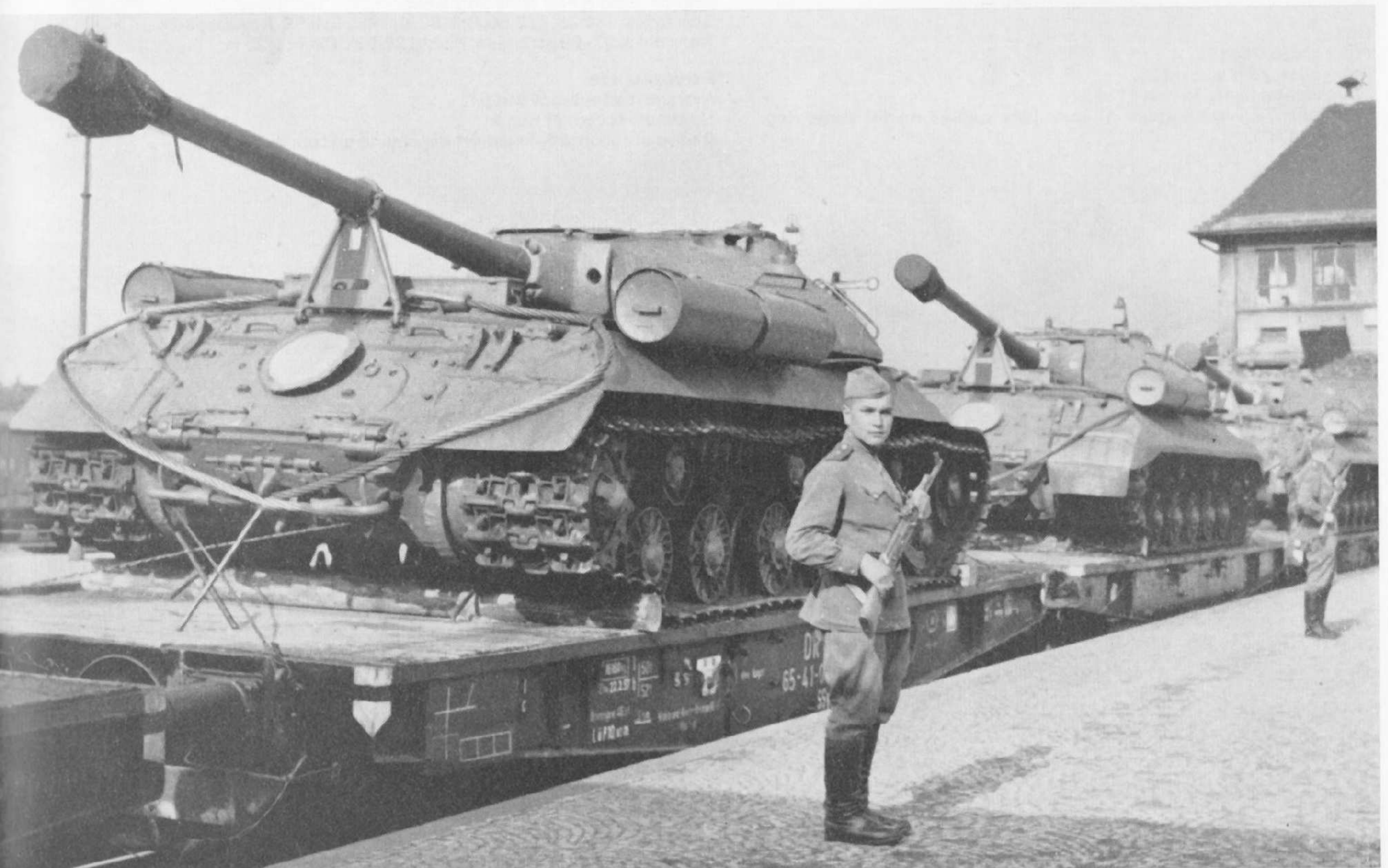
IS-3 tanks loaded on rail flats in East Germany in 1956. The discs on the rear of the hulls were probably road safety signs. Note the gun travelling clamp and the unused brackets—possibly for smoke canisters—to its left and right. (dpa)
