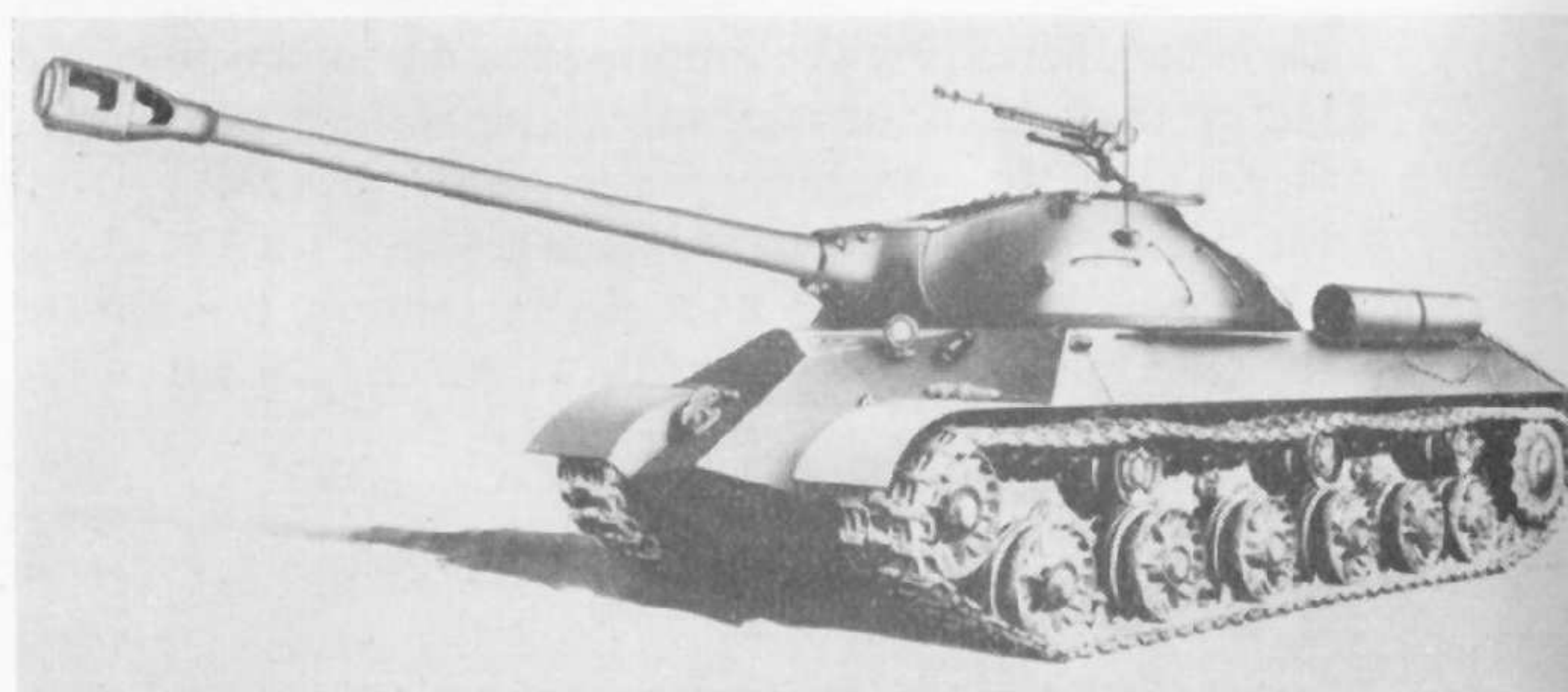
The radical redesign of the hull front and turret are clearly visible in this IS-3. (Crown Copyright Reserved)
