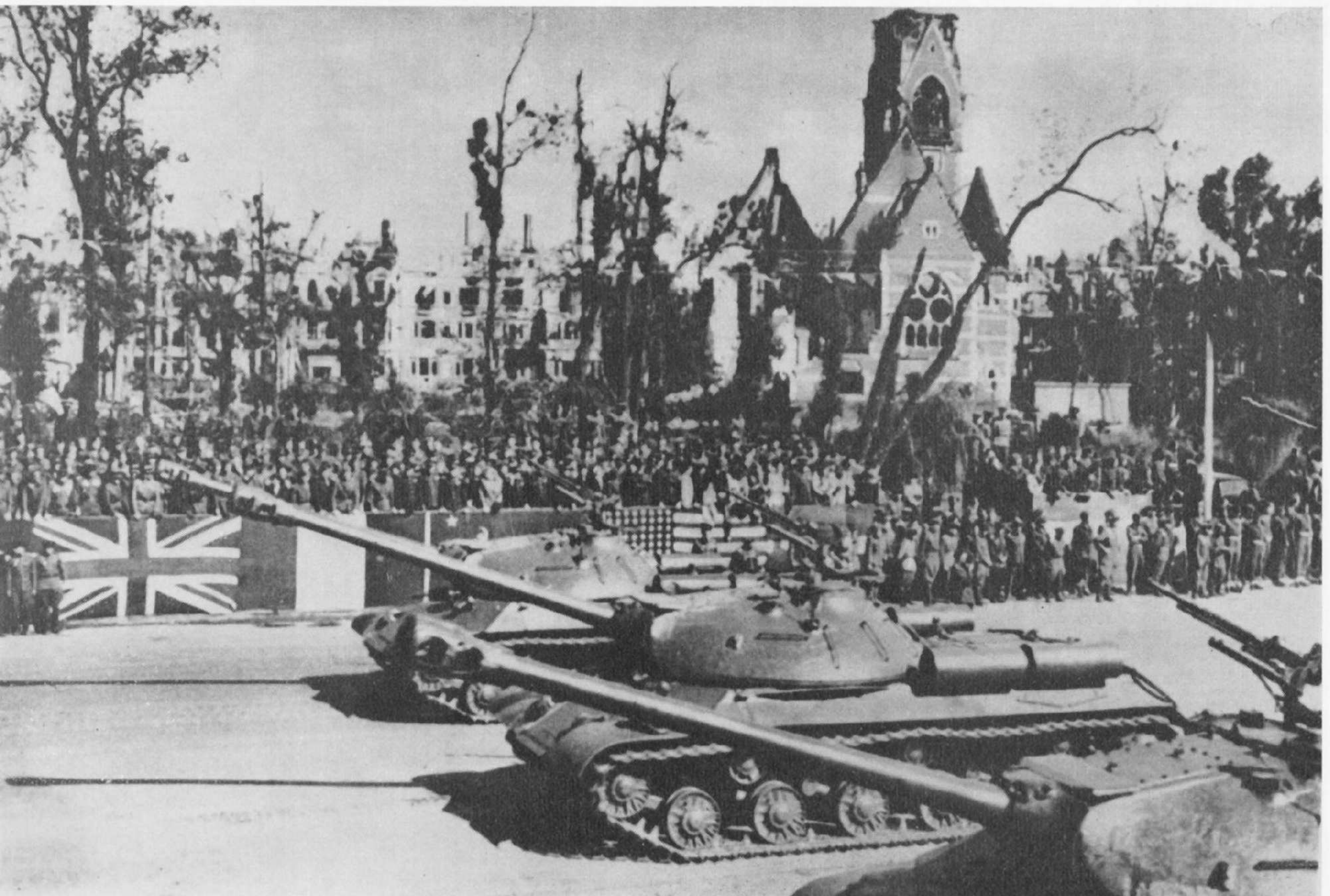
IS-3 marching past on the Victory Parade in Berlin in September 1945. The lifting flap to allow full elevation of the 122 mm. gun can be seen on the nearest tank. (Burroughs/A.P.)
