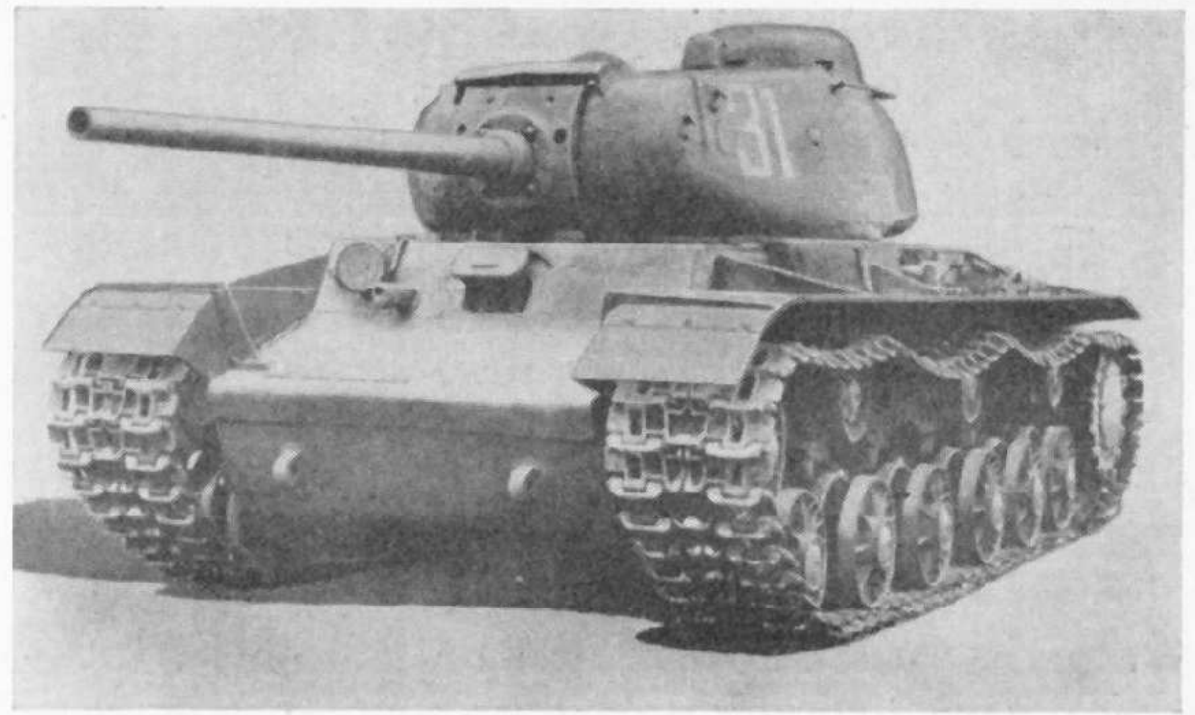
Note the changes in the hull front of this interim KV-85 and the similarity to the IS-1 which followed soon afterwards. (Crown Copyright Reserved)
