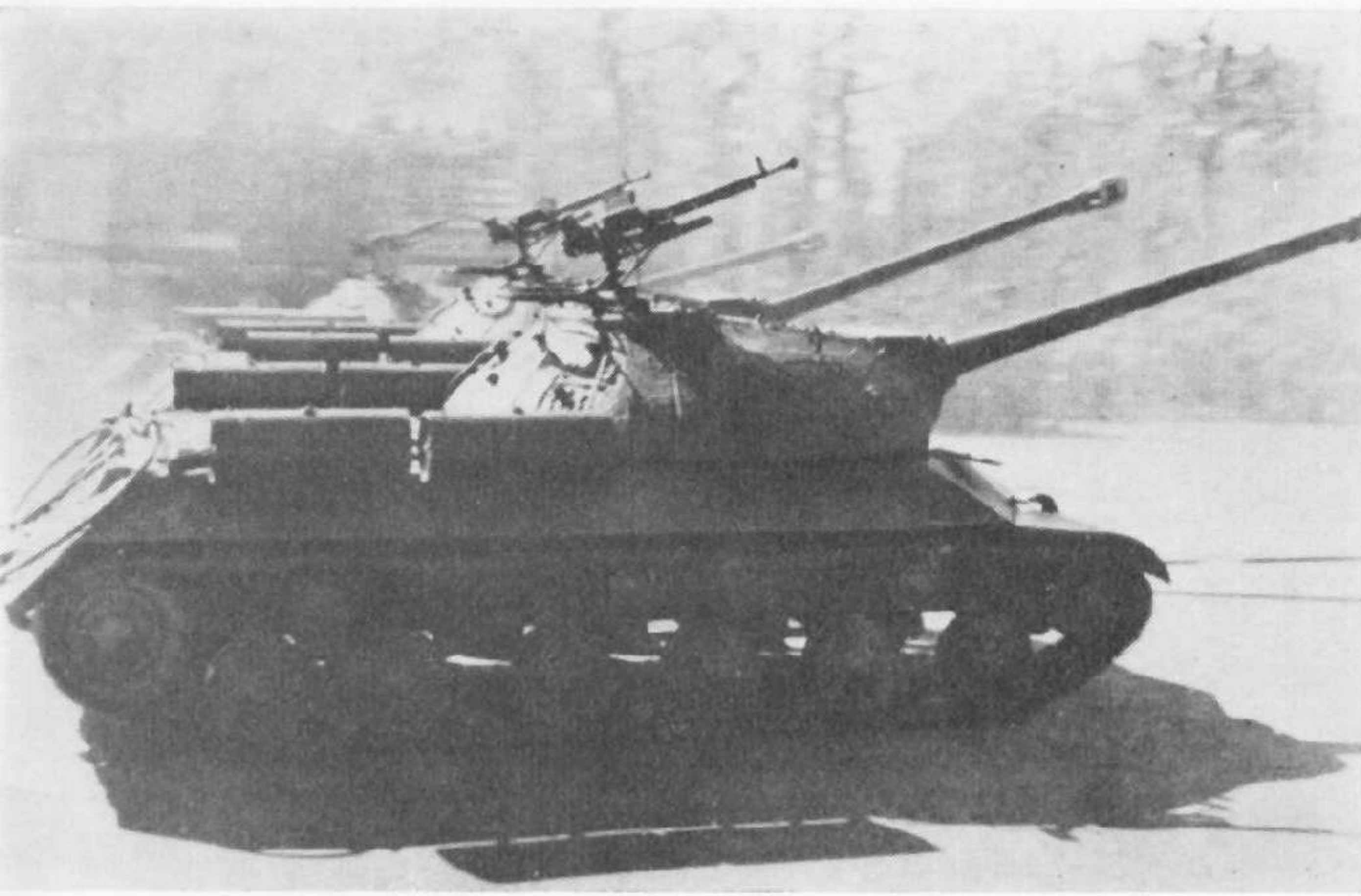
IS-3 on the Victory Parade in Berlin. The remarkable configuration of the armour and the mounting of the 12.7 mm. AAMG can be clearly seen. (Crown Copyright Reserved)
