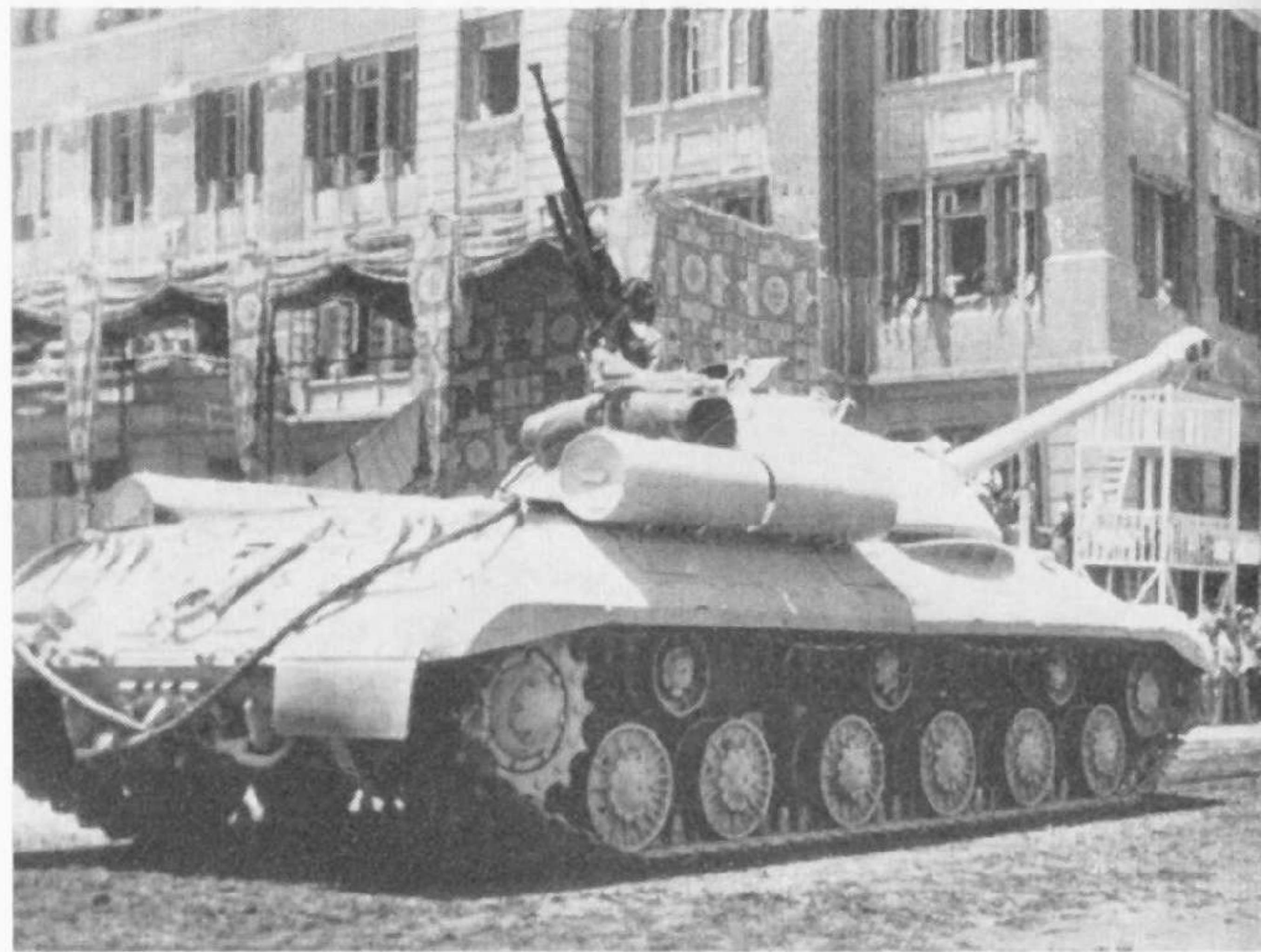
One of the few IS-3 tanks to be exported taking part in the Independence Day parade in Cairo in June 1956. The semi-circular plate on the hull may have partially protected the turret race which would be vulnerable at this point. (dpa)
