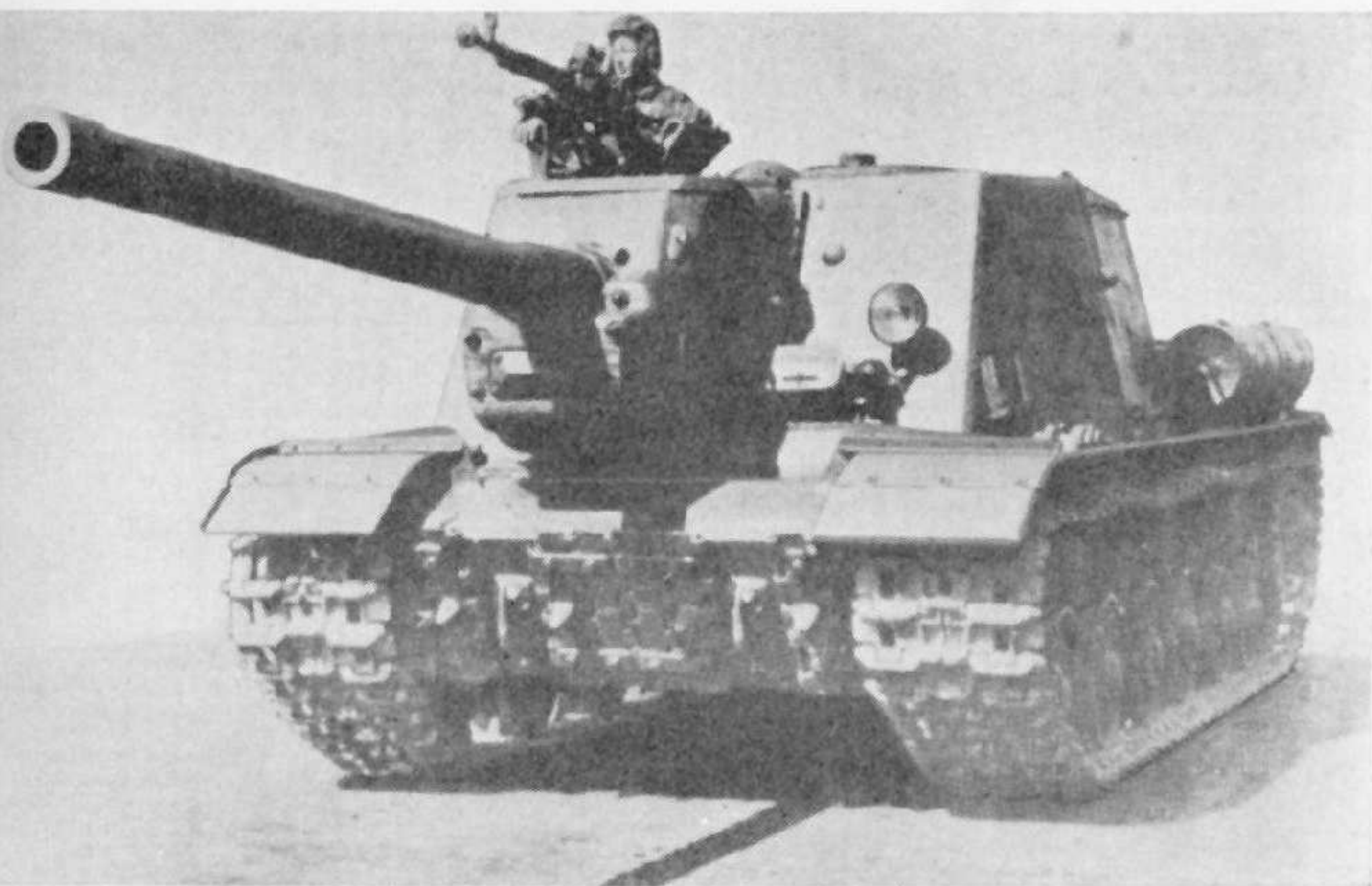
The ISU-122 had the same superstructure and automotive design as ISU-152 but is recognizable by the smooth tube of the M-1944 A-19S 122 mm. gun. (Crown Copyright Reserved)
