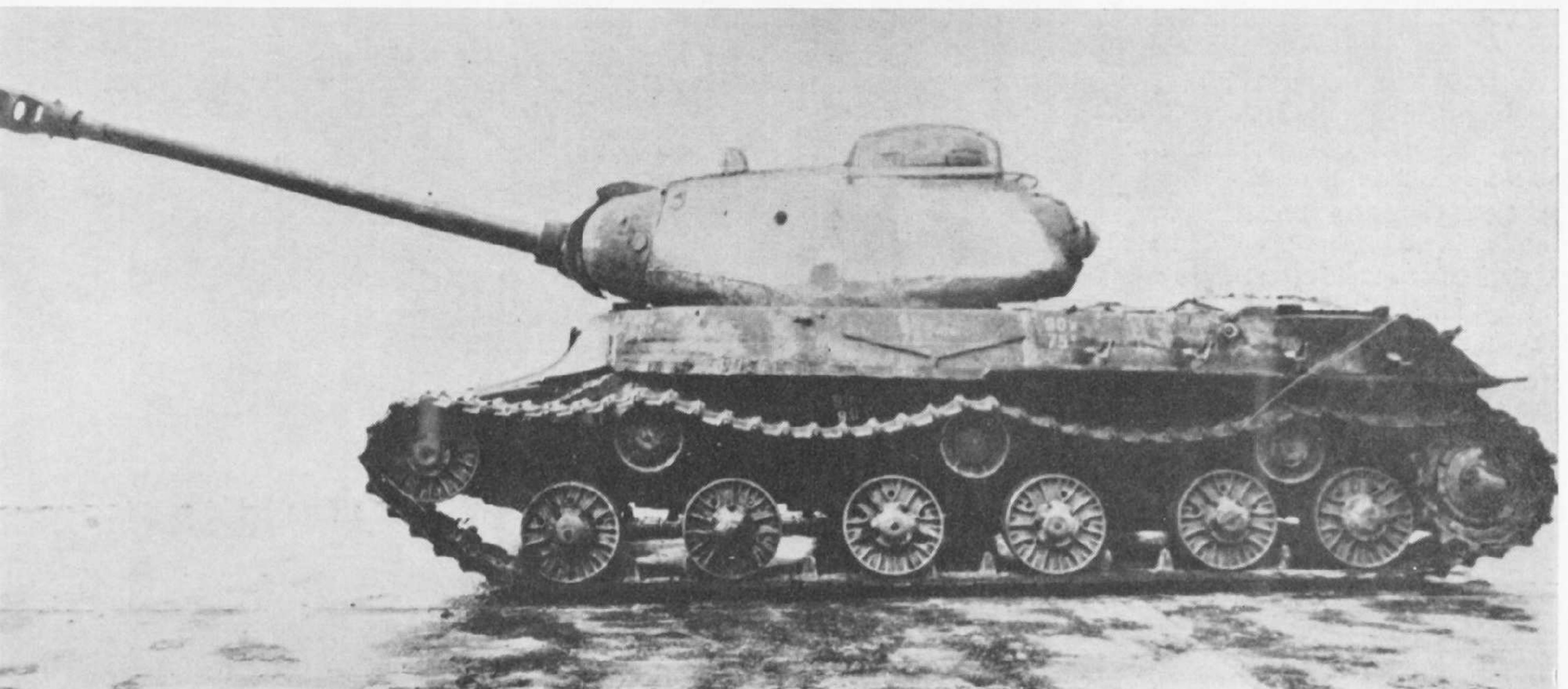
A battered IS-1. Note the lowering of the top suspension units compared with the KV design, necessary in order to accommodate a turret ring of a wider diameter on a hull of roughly the same width. (Crown Copyright Reserved)
