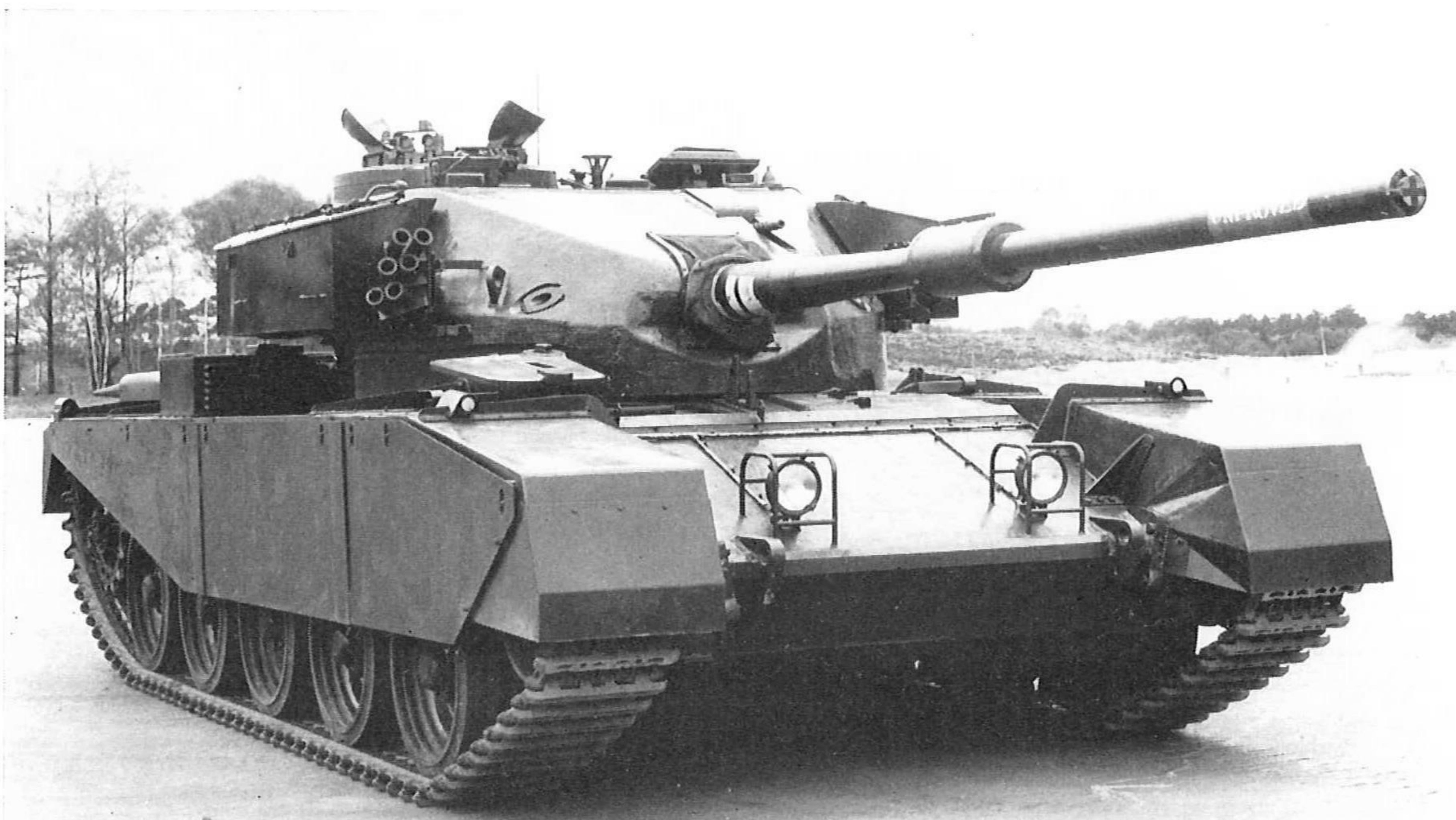
Above and below: FV 4202 ; the so-called 40-ton Centurion built by Leyland Motors to provide practical experience of a number of concepts intended for FV 4201 , including the reclining position for the driver and the mantlet-less turret. (FVRDE, CCR)
