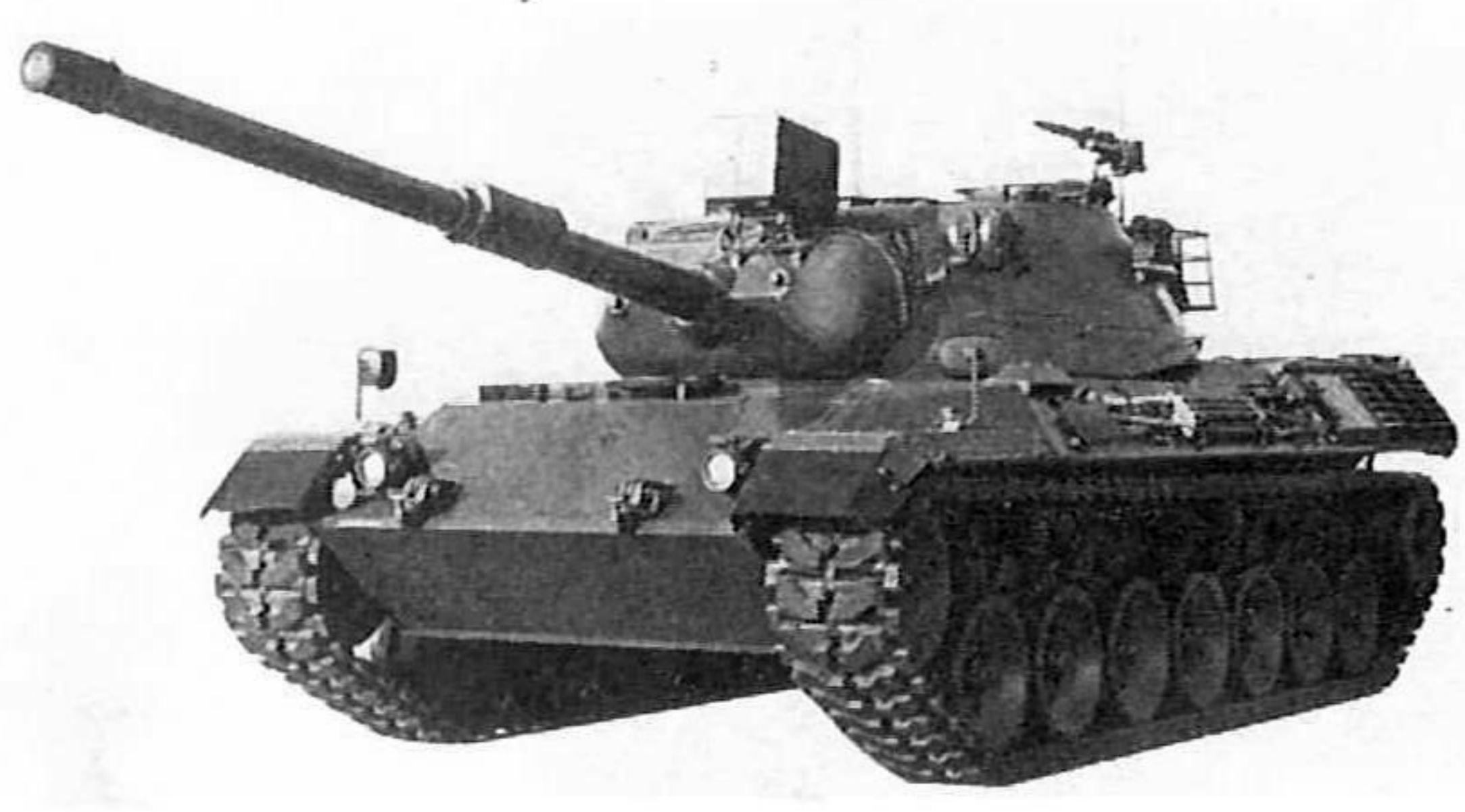
Production versions of Leopard. Among the number of changes visible note the moving of the smaller searchlight to the left of the mantlet to avoid back-scatter of light into the sights.
