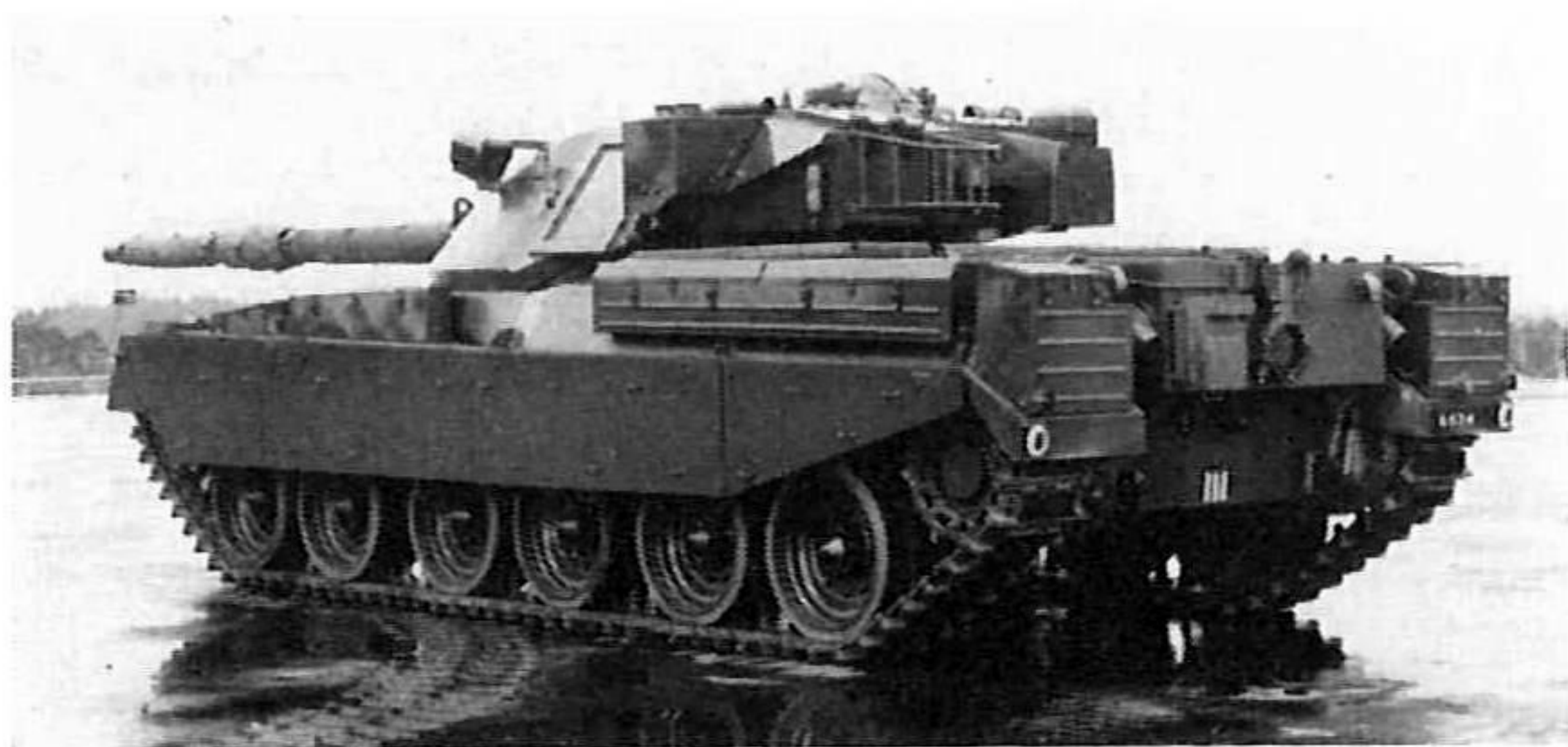
A prototype modified with the raised suspension system and incorporating the armored cover for the exhausts. (FVRDE, CCR)
