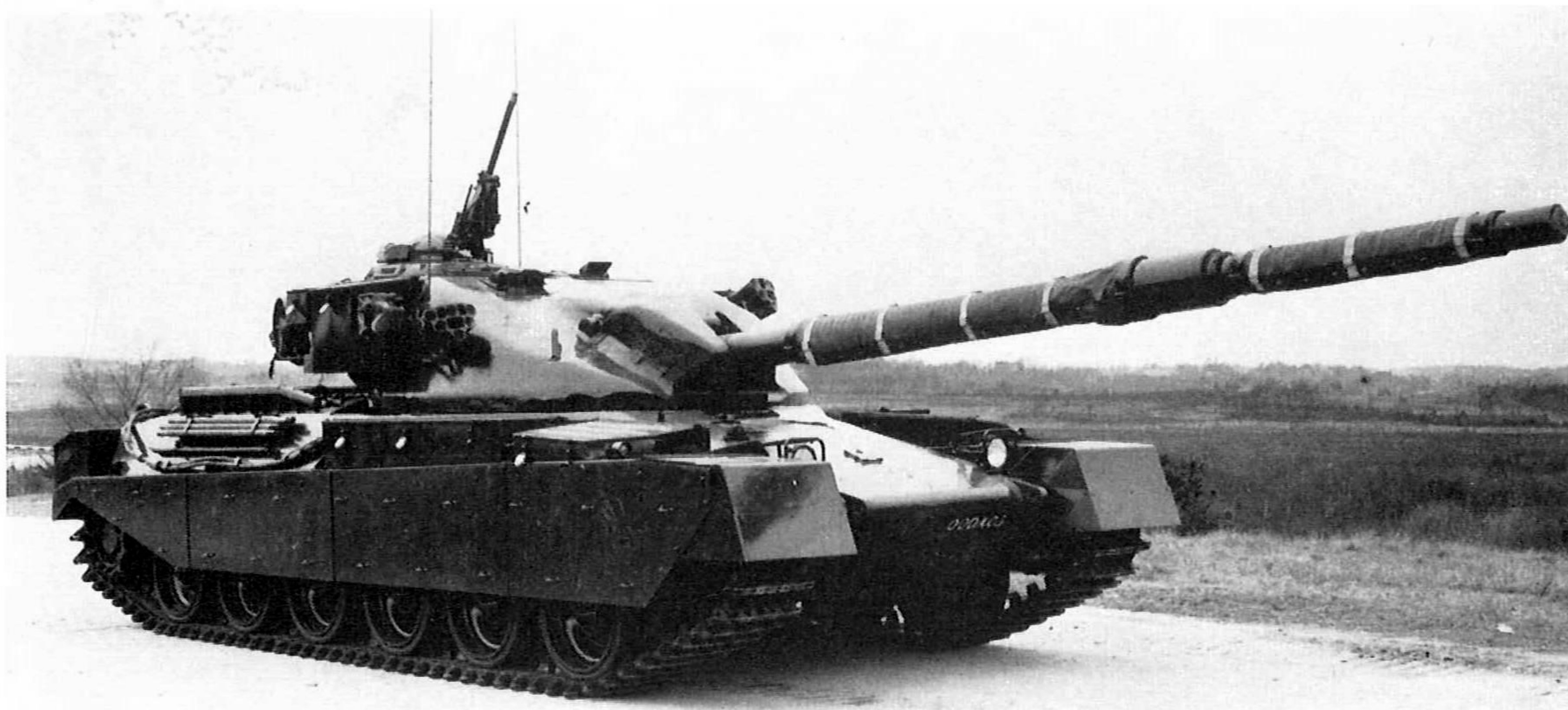
One of the first prototypes of Chieftain having the original low suspension.
