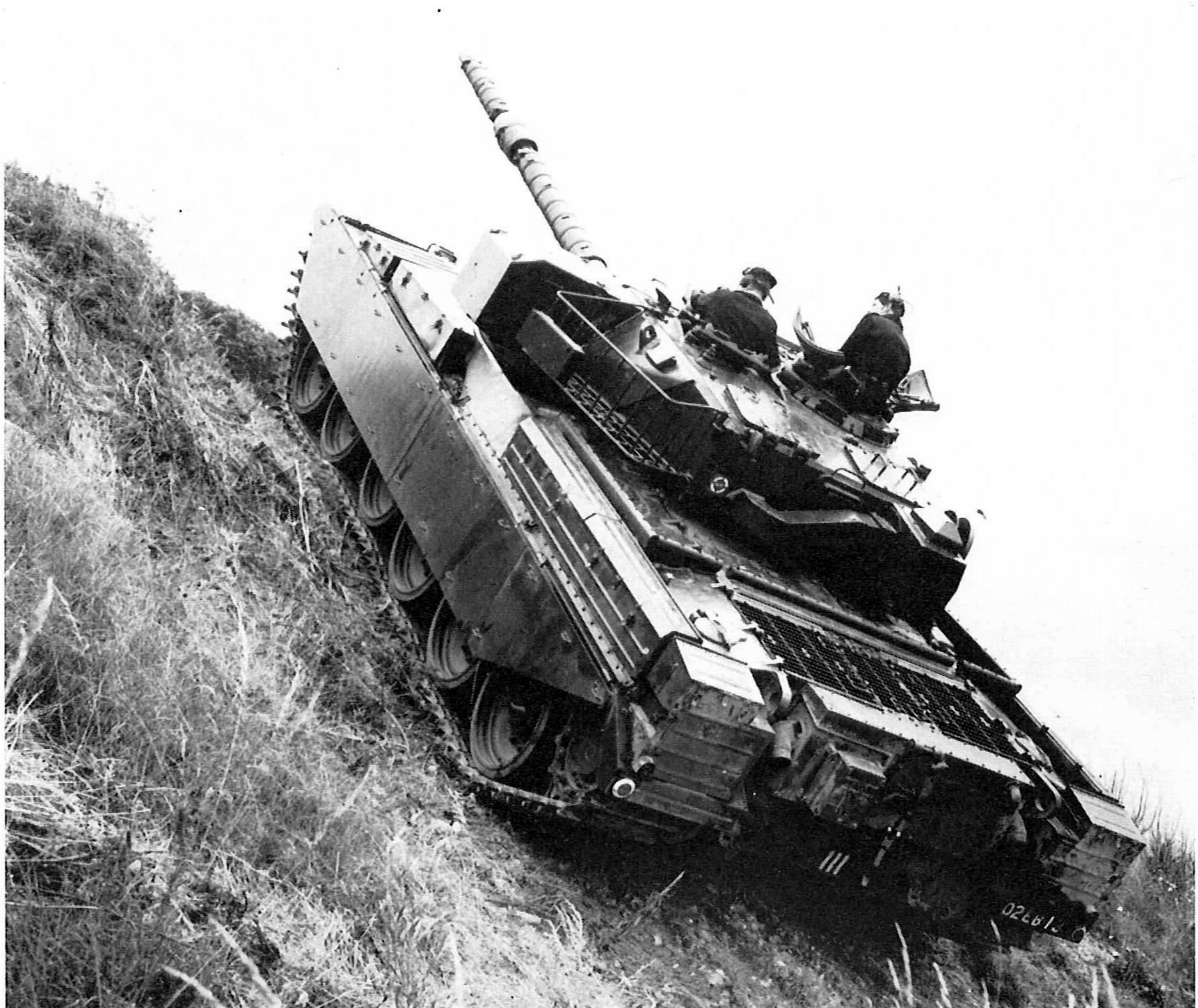
Mark 1 Chieftain. The external components of the ventilation equipment are fitted and a new stowage rack has been fitted on to the left rear of the turret. The split covers on the commander's cupola are open. None of the comparatively few Mark 1 versions was issued to the Service. (CCR)
