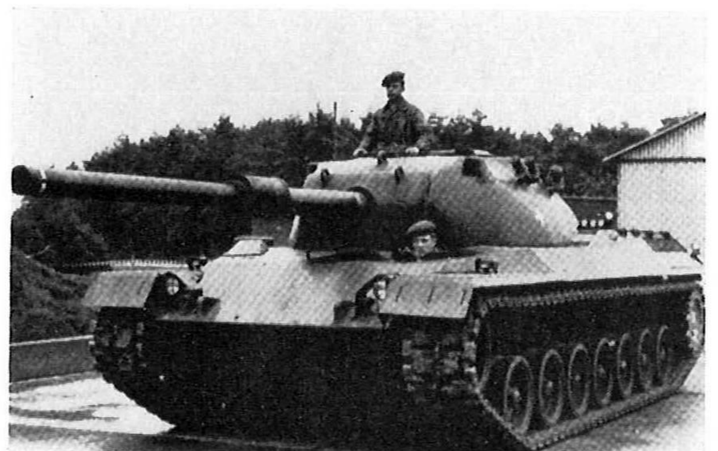
Prototype I of Group A mounting the British 105-mm. L7 gun. The driver's compartment had to be moved subsequently to the other side of the hull to make way for ammunition stowage for the gun which is loaded from the left. (Soldat und Technik)
