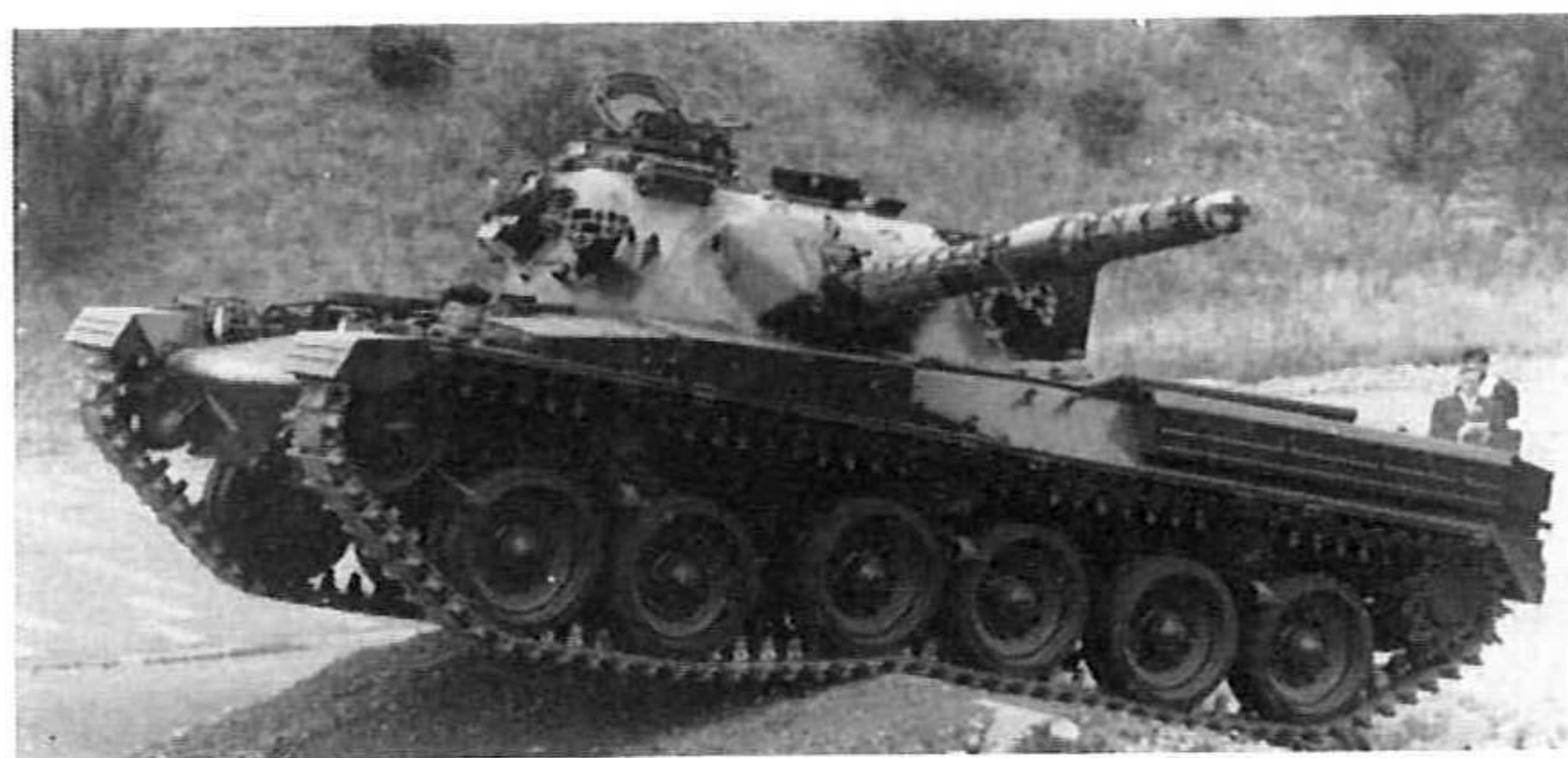
Mark 2 negotiating a minor obstacle during a demonstration. This tank has the much-improved commander's cupola and the new hatch cover is apparent. (FVRDE, CCR)
