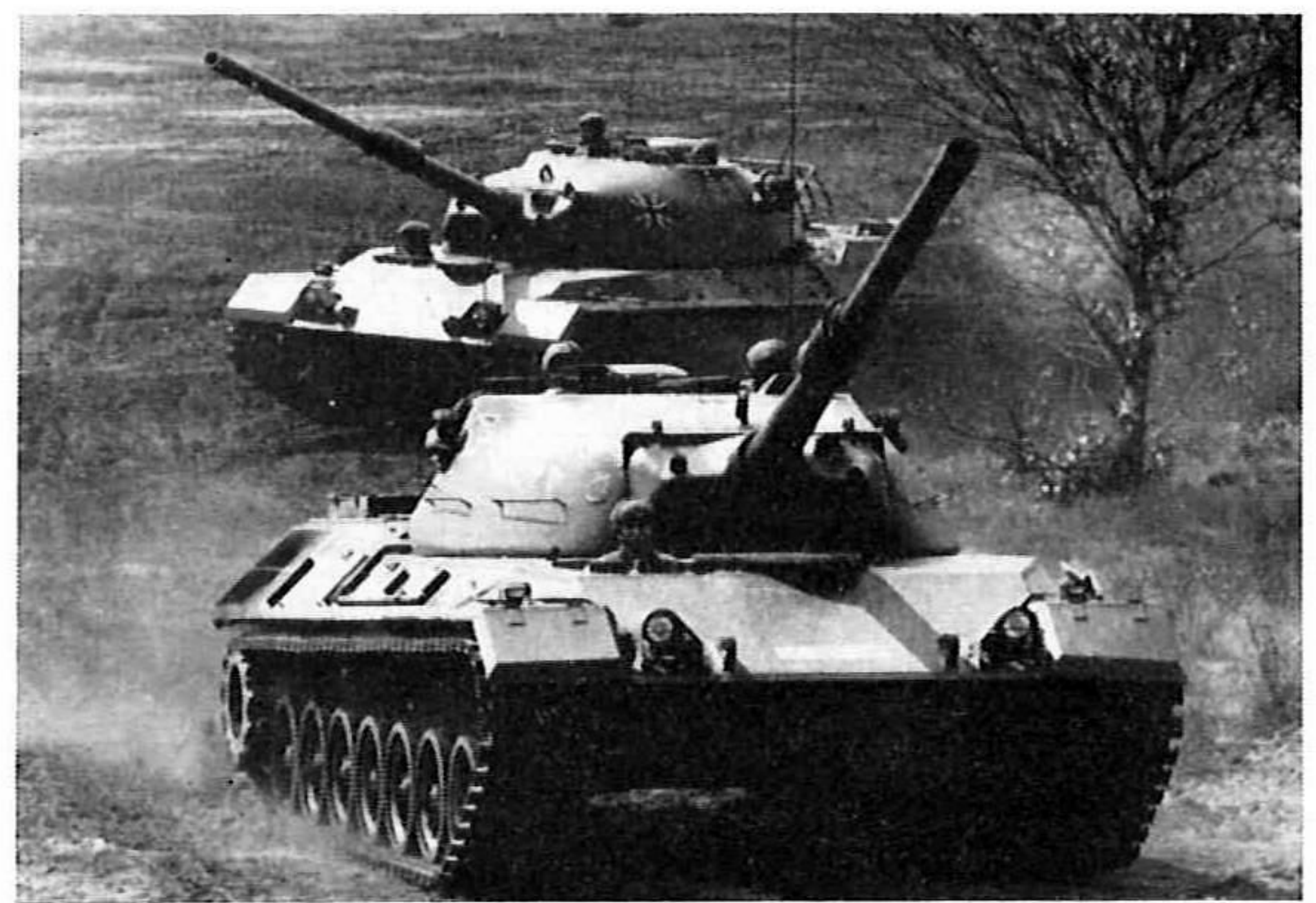
Prototype IIA Leopards at the first public demonstration in July 1963. Note the re-positioning of the driver's compartment. (Associated Press)
