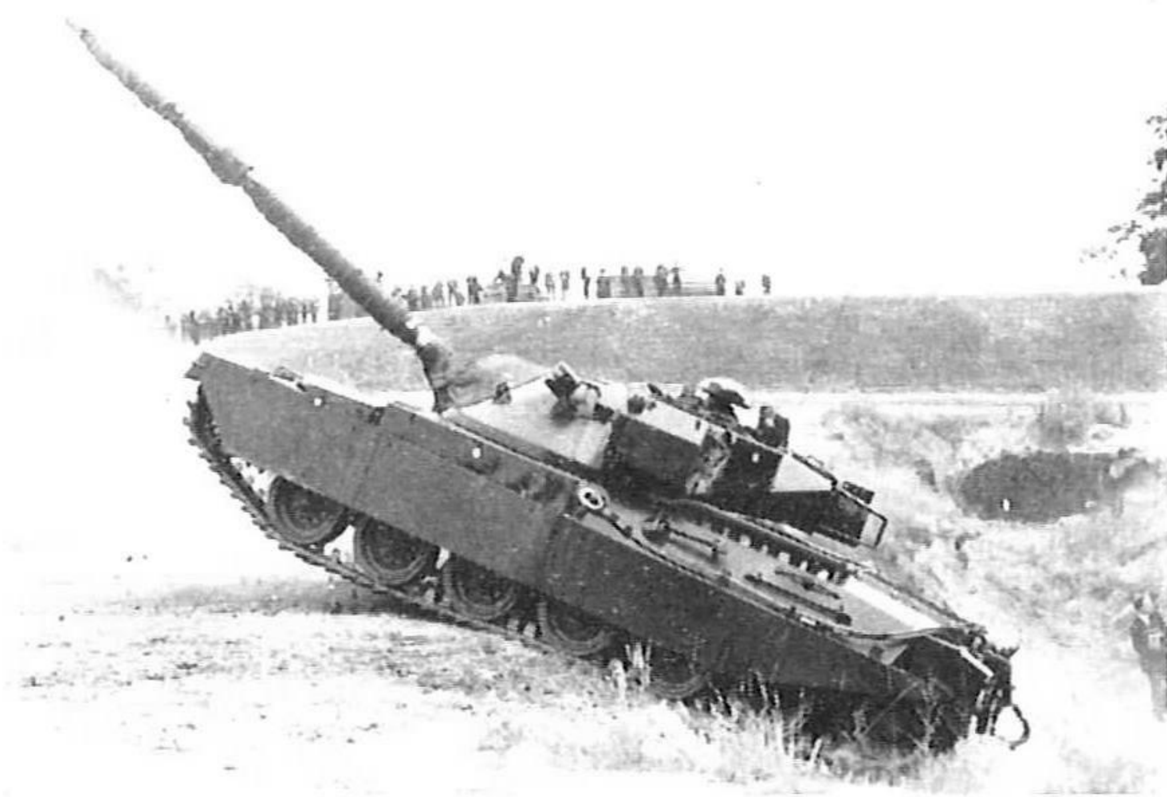
An early prototype showing its paces during a demonstration in August 1963. The cupola hatches are in the "umbrella" position to give the commander some degree of overhead protection and a better field of view than was possible with the early design of vision devices. (Keystone)
