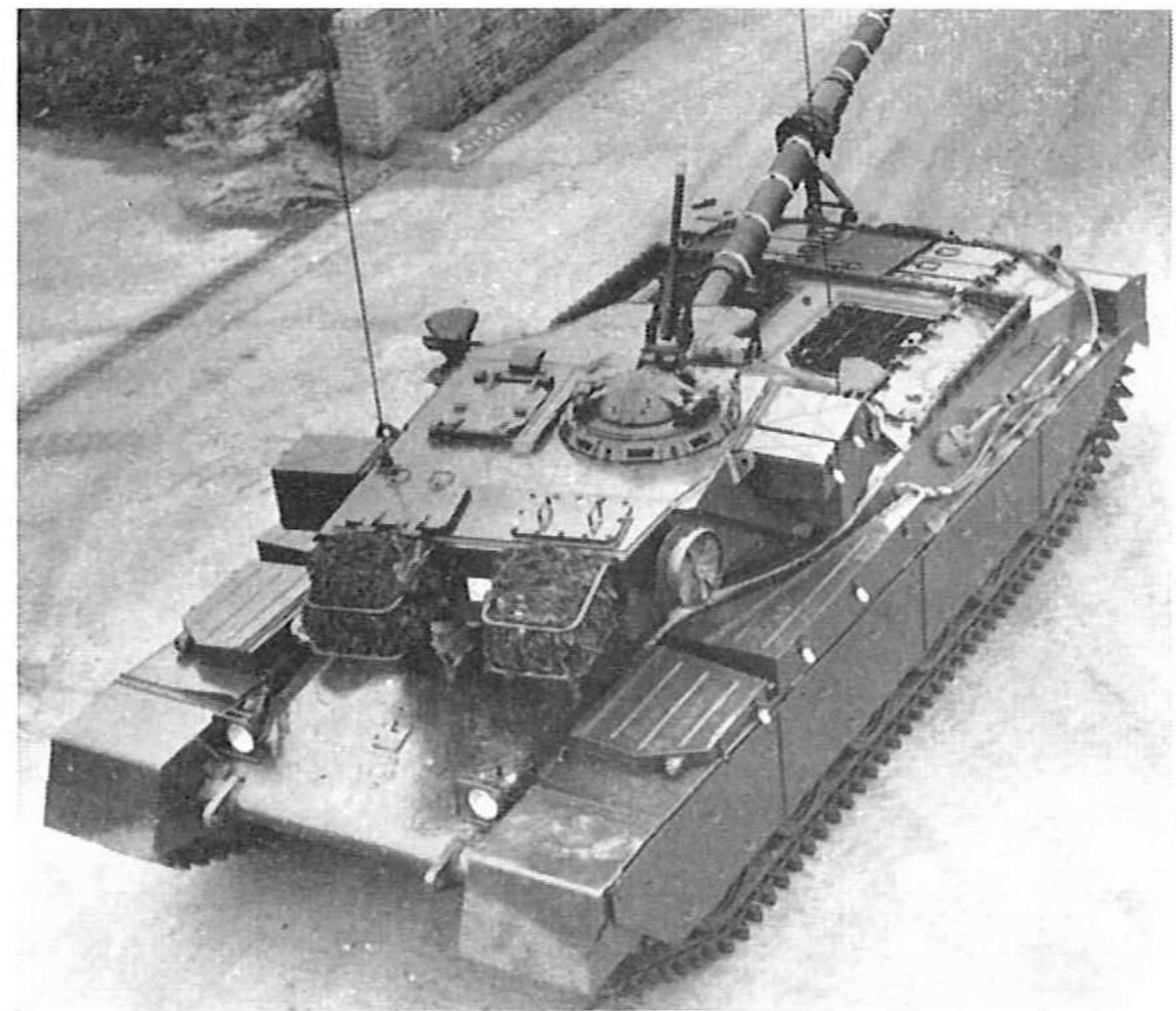
A prototype prepared for troop trials. Note the changes in the cupola assembly and the stowage racks on the rear of the turret. (FVRDE, CCR)
