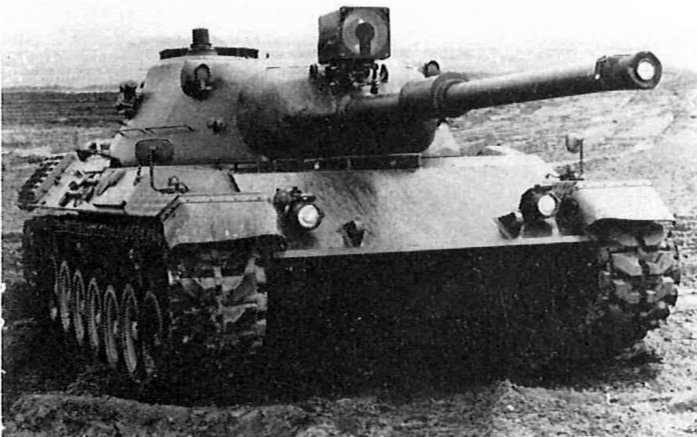
Left: Preproduction version of Leopard with the commander's panoramic periscope installed and a coaxially-mounted IR searchlight on the centre of the mantlet. (RAC Centre)
