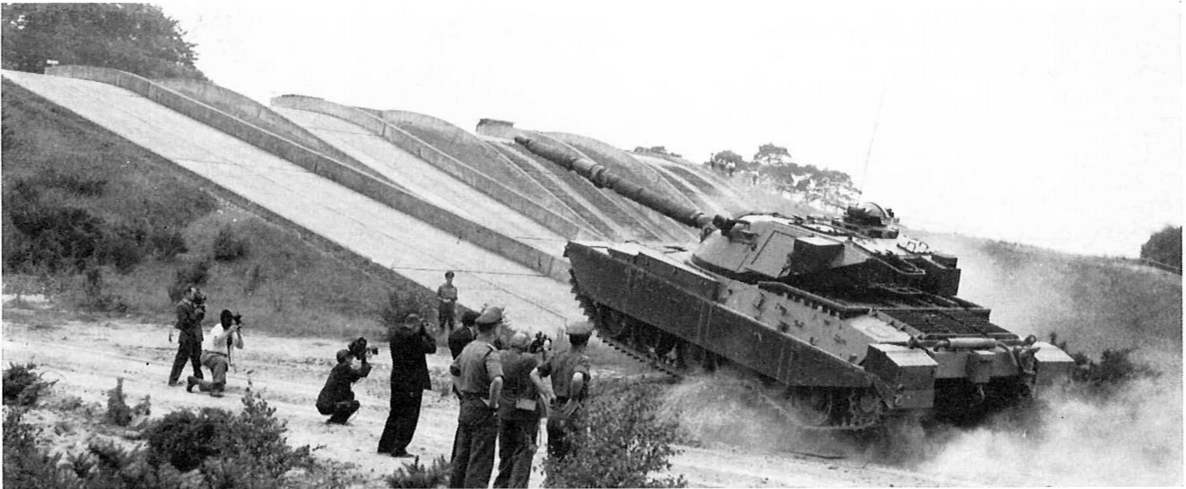
A prototype Chieftain starting a hill climb. One of the rear turret stowage racks has been replaced by part of the ventilation equipment, the exhaust system is still in the development stage and the light projector is not fitted. (FVRDE, CCR)
