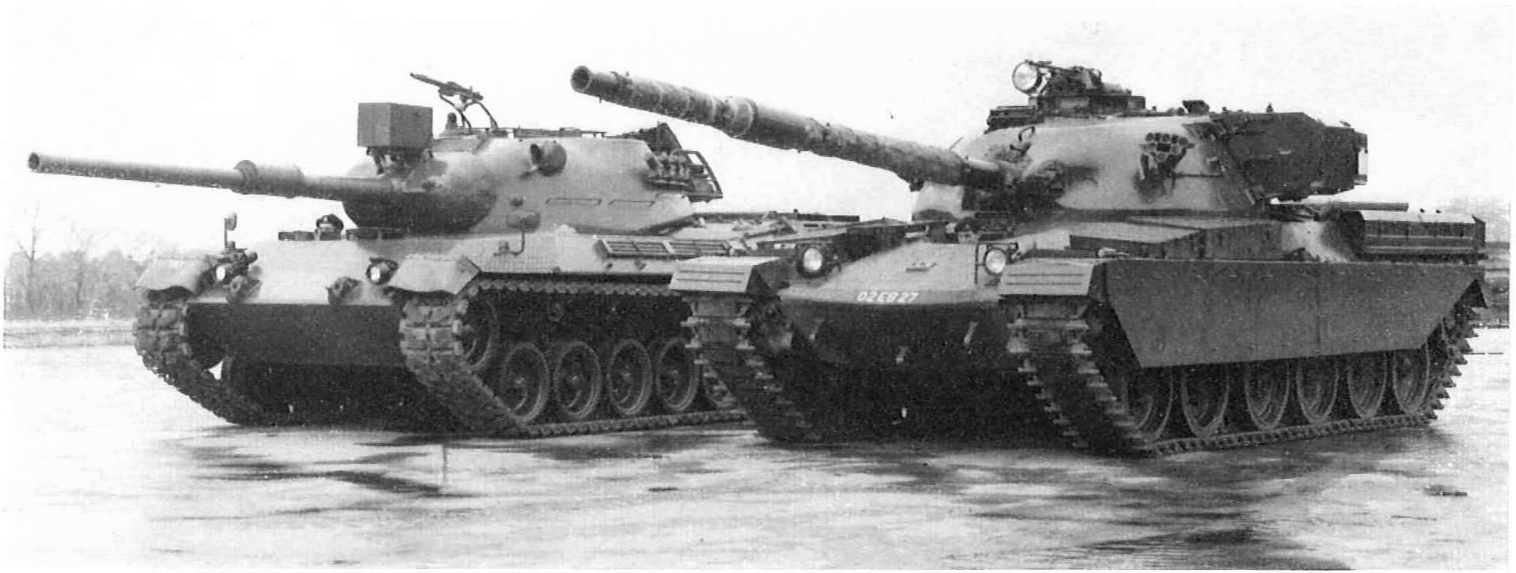
Above and below: A Chieftain Mark 2 (right) and a pre-production Leopard together for comparative trials. (FVRDE, CCR)
