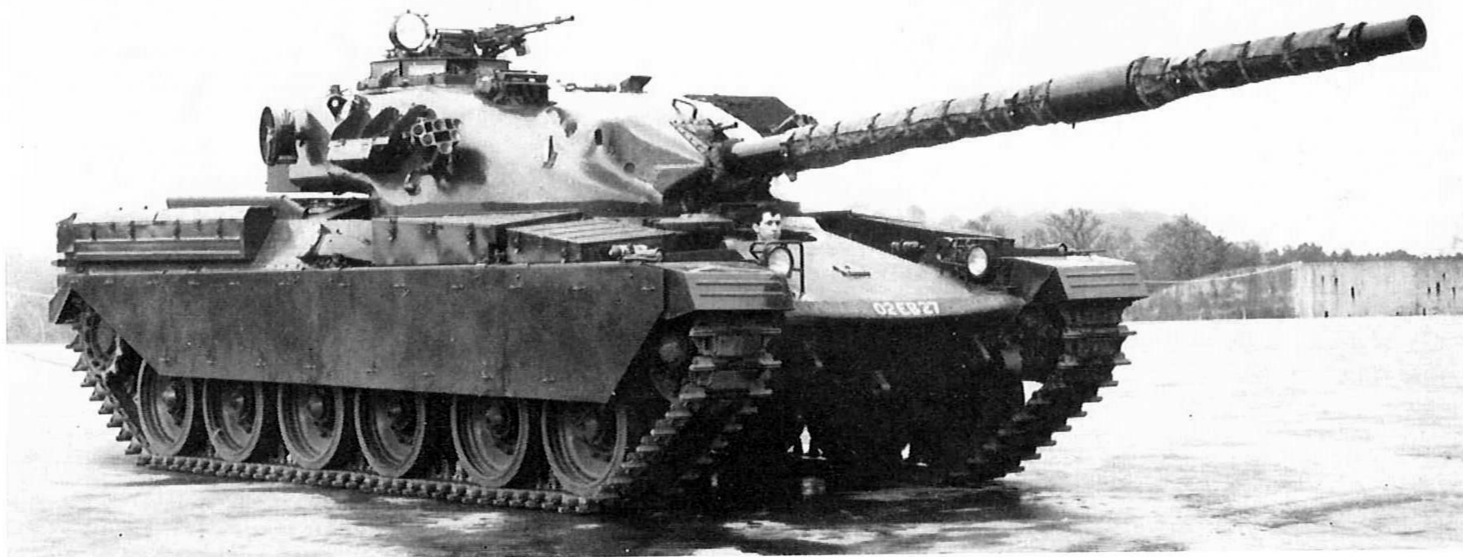
The new periscopes in the commander's cupola and changes to the stowage on the turret are shown in this Mark 2. (FVRDE, CCR)
