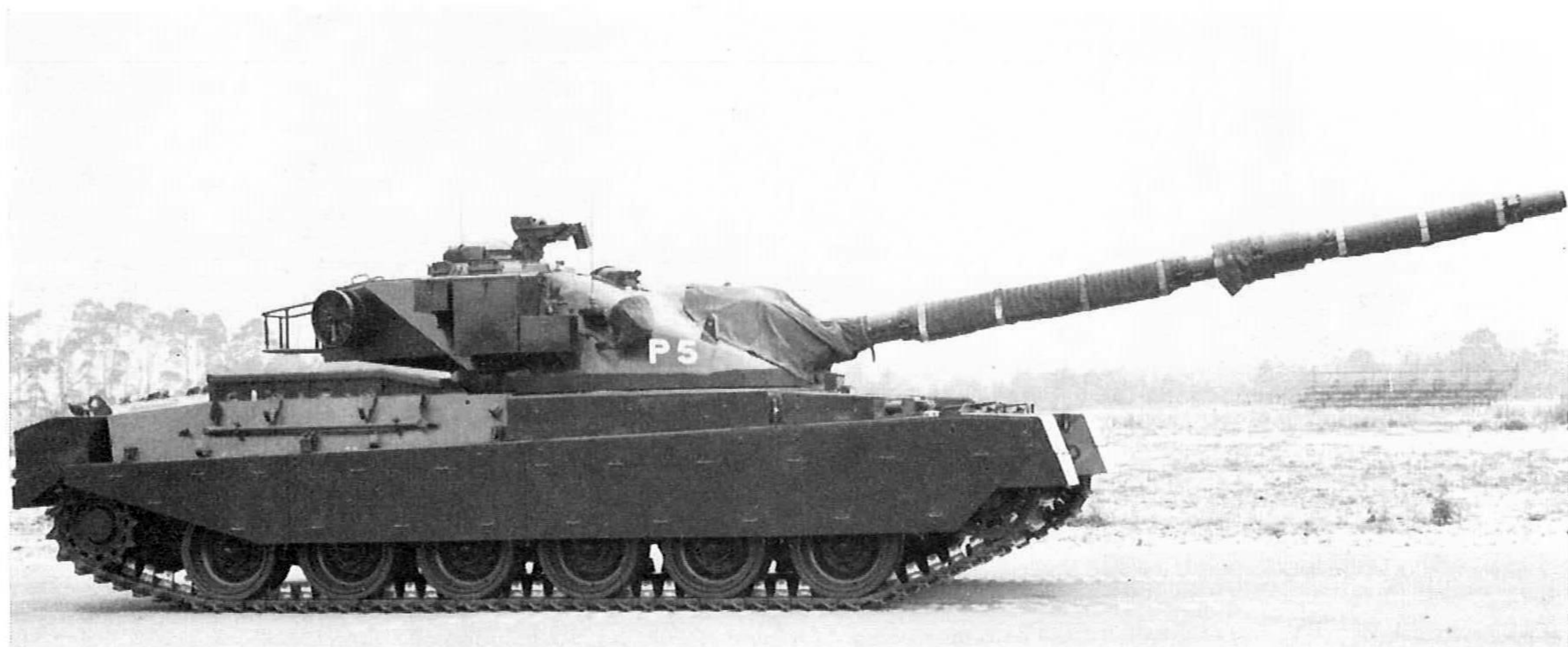
Prototype P5 completed in early 1962. Note the thermal sleeve fitted on the 120-mm. gun barrel.
