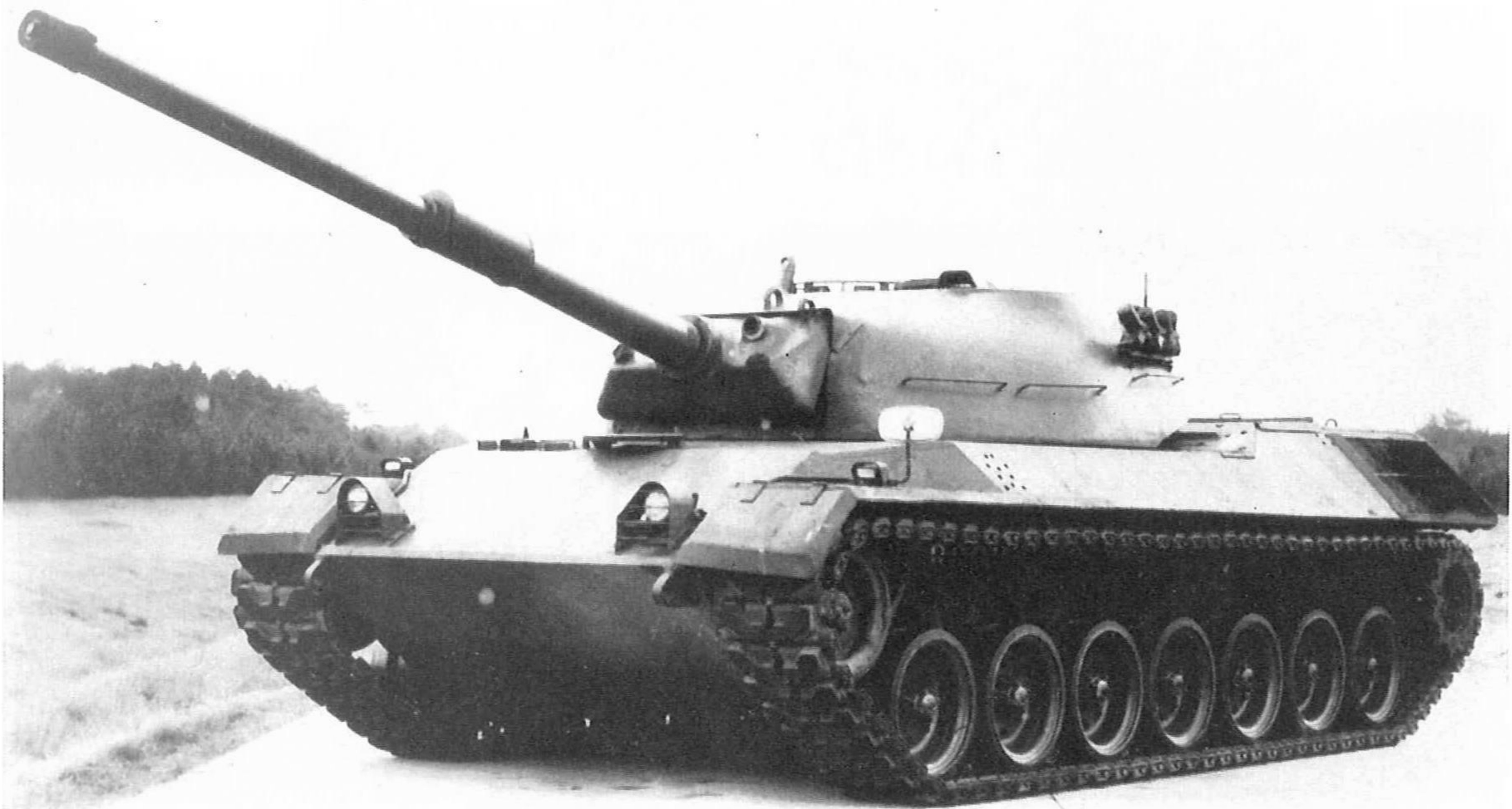
Top right and below: Prototype type IIA with the cross turret rangefinder removed in favour of the 0.5-in. ranging gun. (German MOD)
