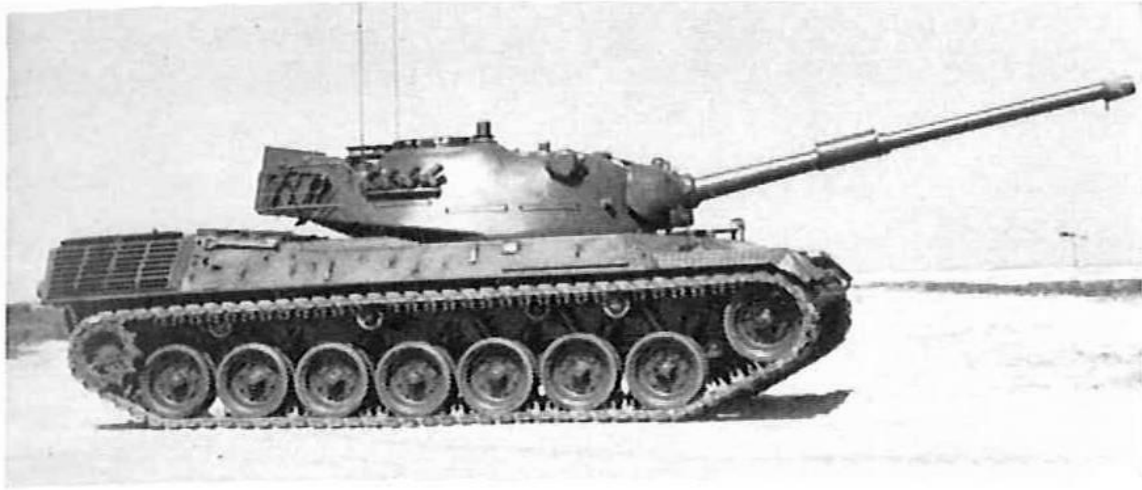
Above and below: Preproduction version of Leopard with the commander's panoramic periscope installed. (RAC Centre)
