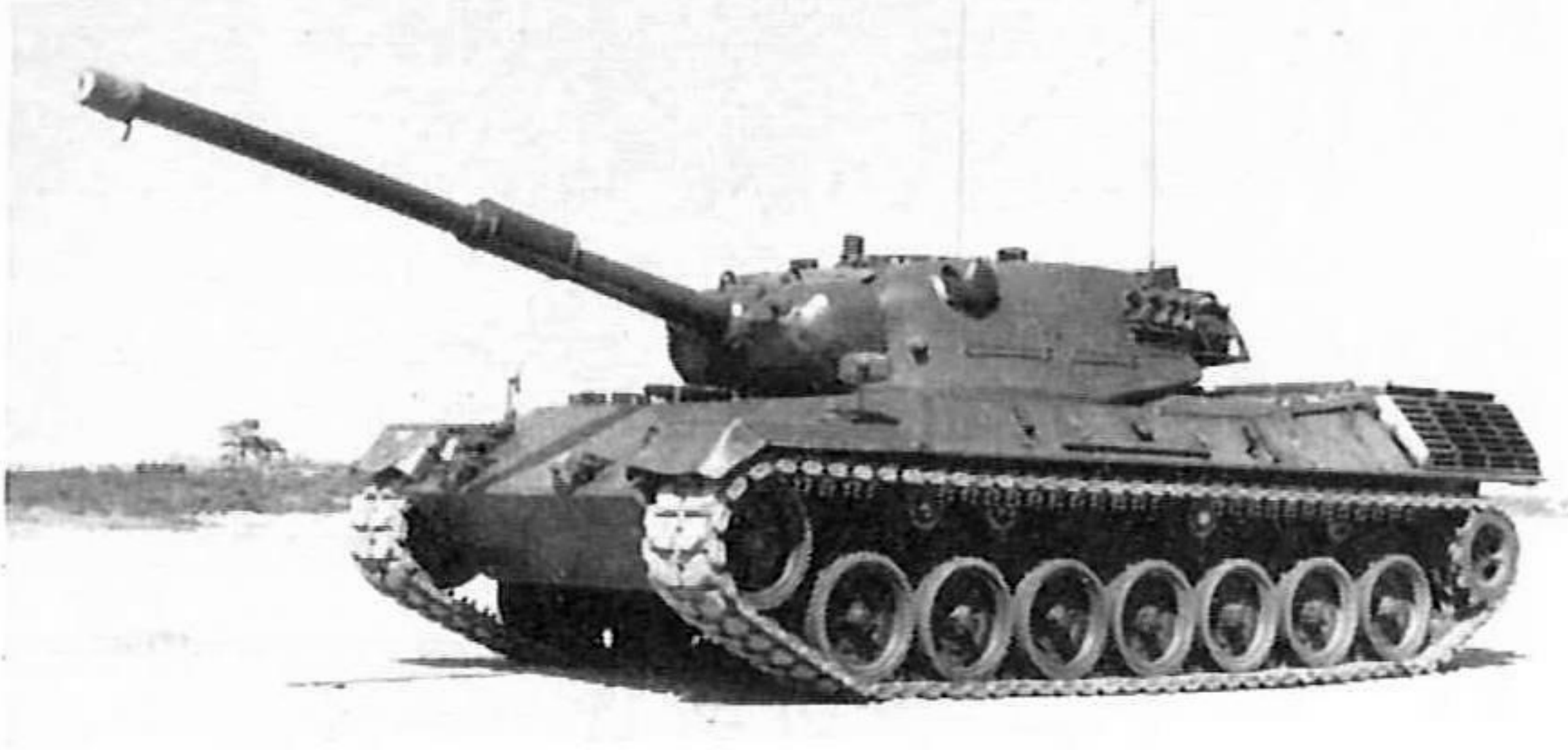
Above and below: Preproduction version of Leopard with the commander's panoramic periscope installed. (RAC Centre)
