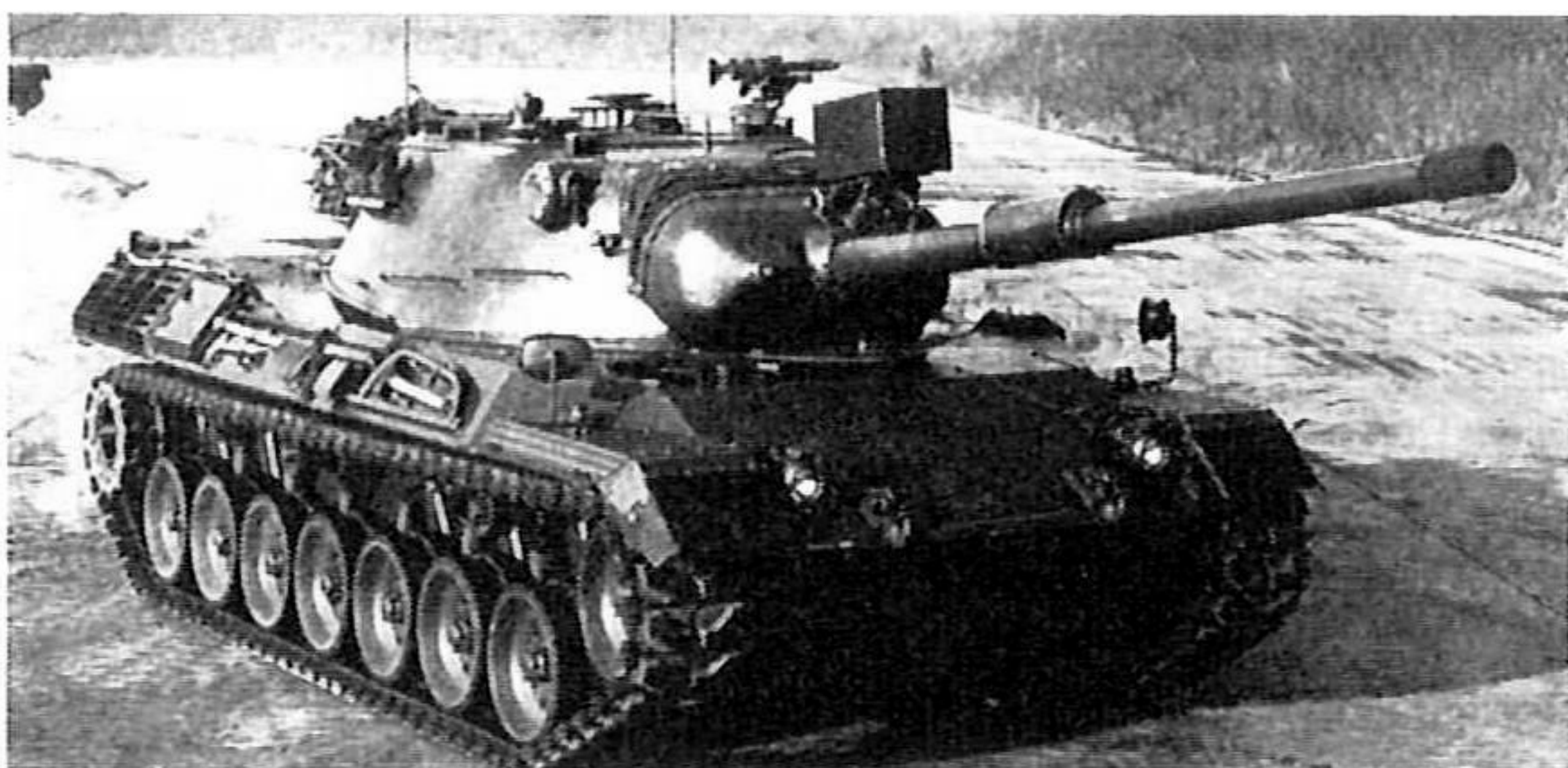
Three pictures show production versions of Leopard. Among the number of changes visible note the addition of a stowage bin at the rear of the turret where previously there had been an ammunition loading hatch. (Soldat und Technik)
