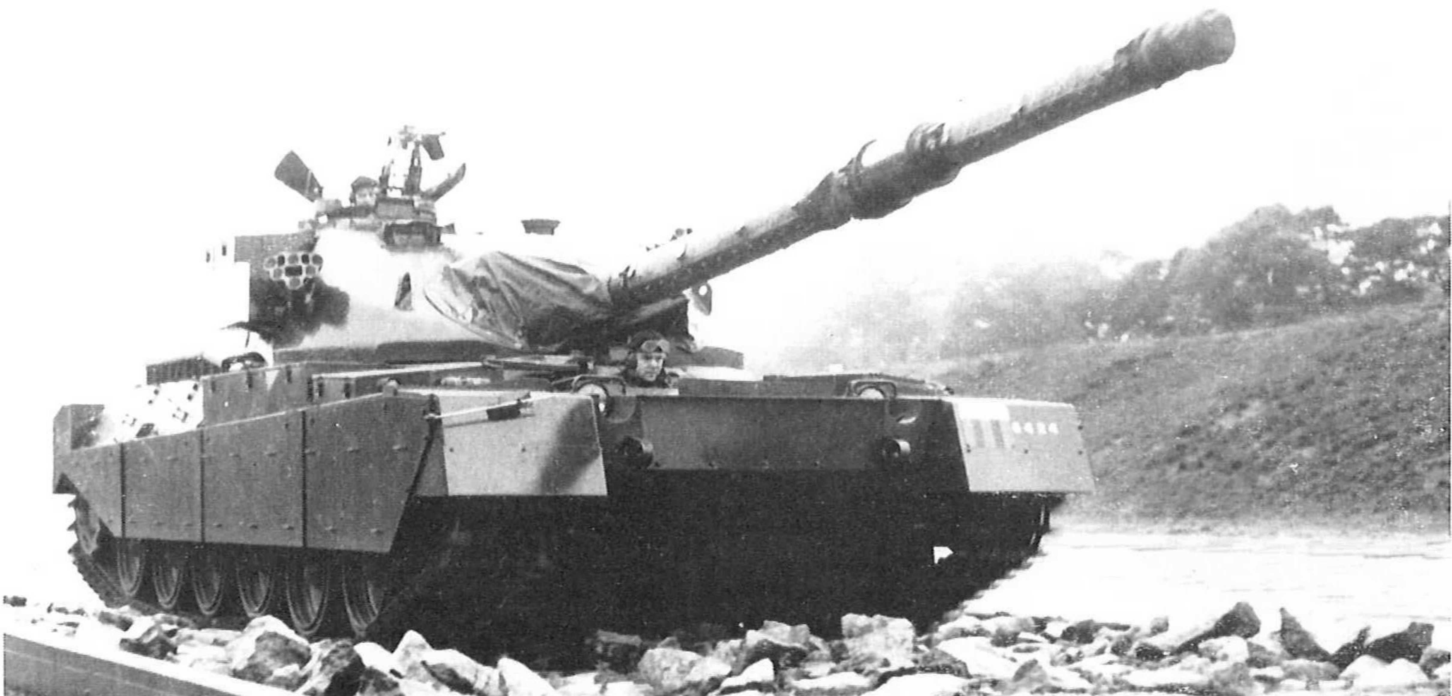
An early prototype negotiating a rough test track at FVRDE. The dummy bin on the front of the glacis plate and the cover on the nose of the turret were fitted during the first public appearance of the vehicle. (Keystone)
