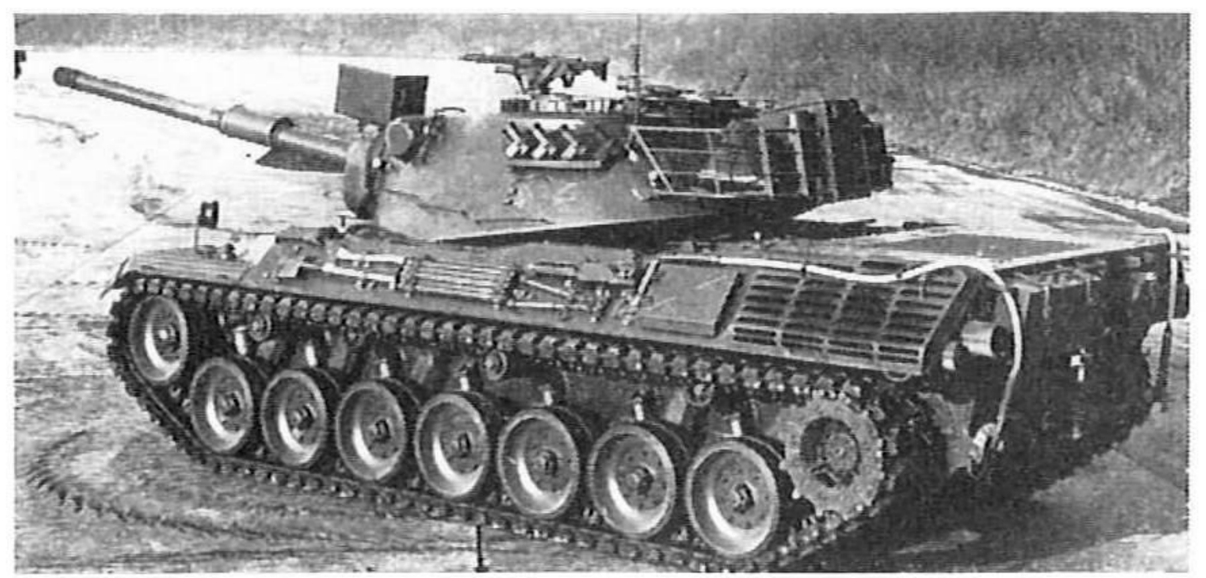
Three pictures show production versions of Leopard. Among the number of changes visible note the addition of a stowage bin at the rear of the turret where previously there had been an ammunition loading hatch. (Soldat und Technik)
