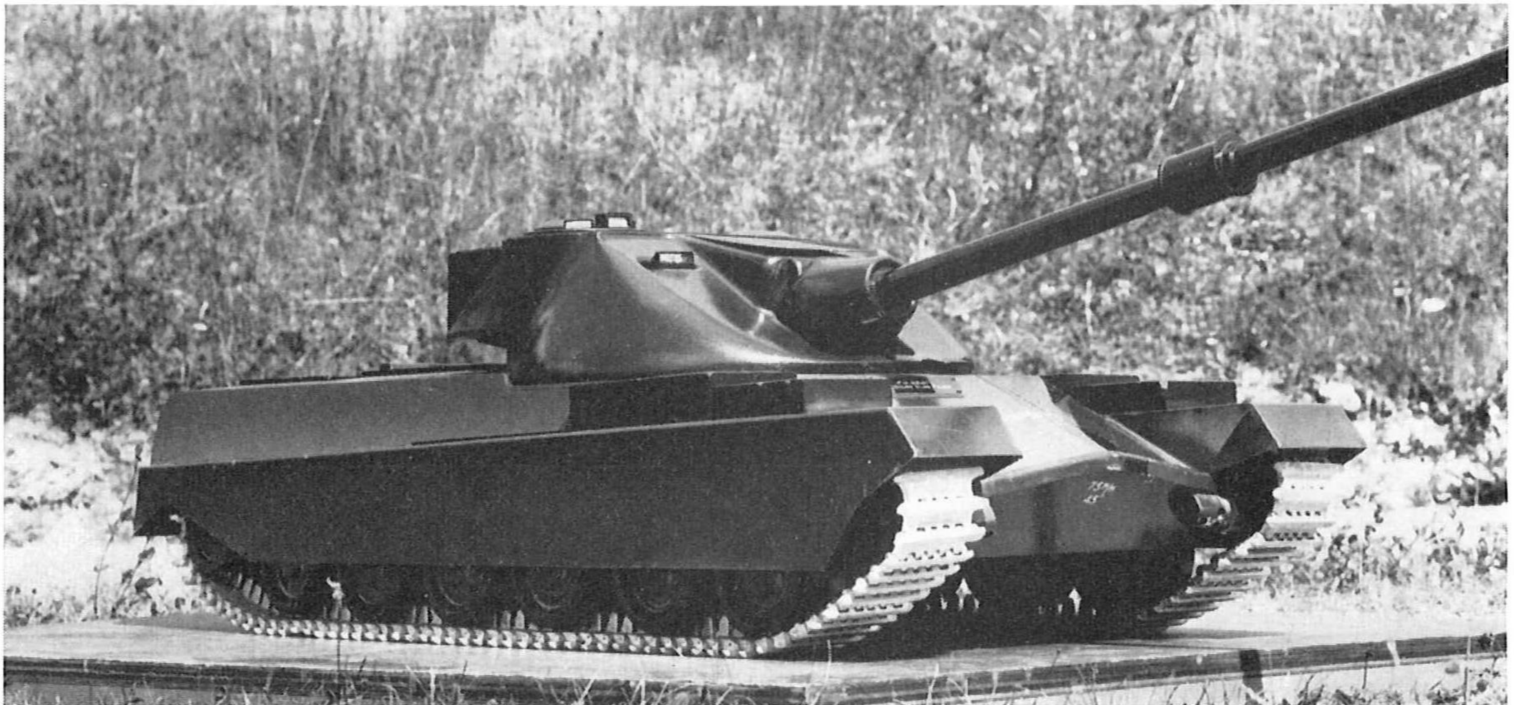
Above and below: A small scale model of an early design for FV 4201 Medium Gun Tank No. 2. Note the similarity of the turret design to that on FV 214 Conqueror and the complex sloping of the glacis plate. (FVRDE, CCR)
