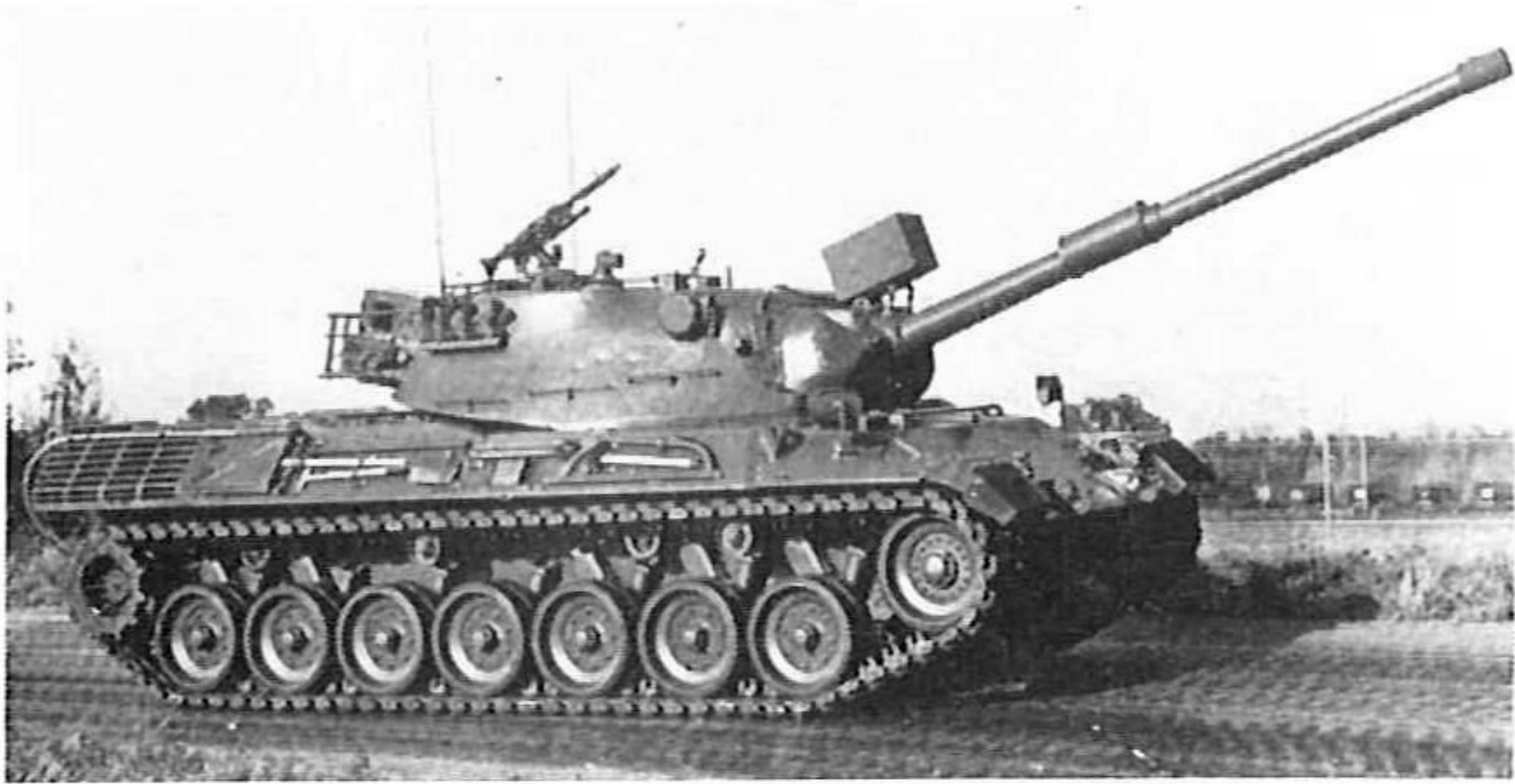
Production versions of Leopard. Among the number of changes visible note the moving of the smaller searchlight to the left of the mantlet to avoid back-scatter of light into the sights.
