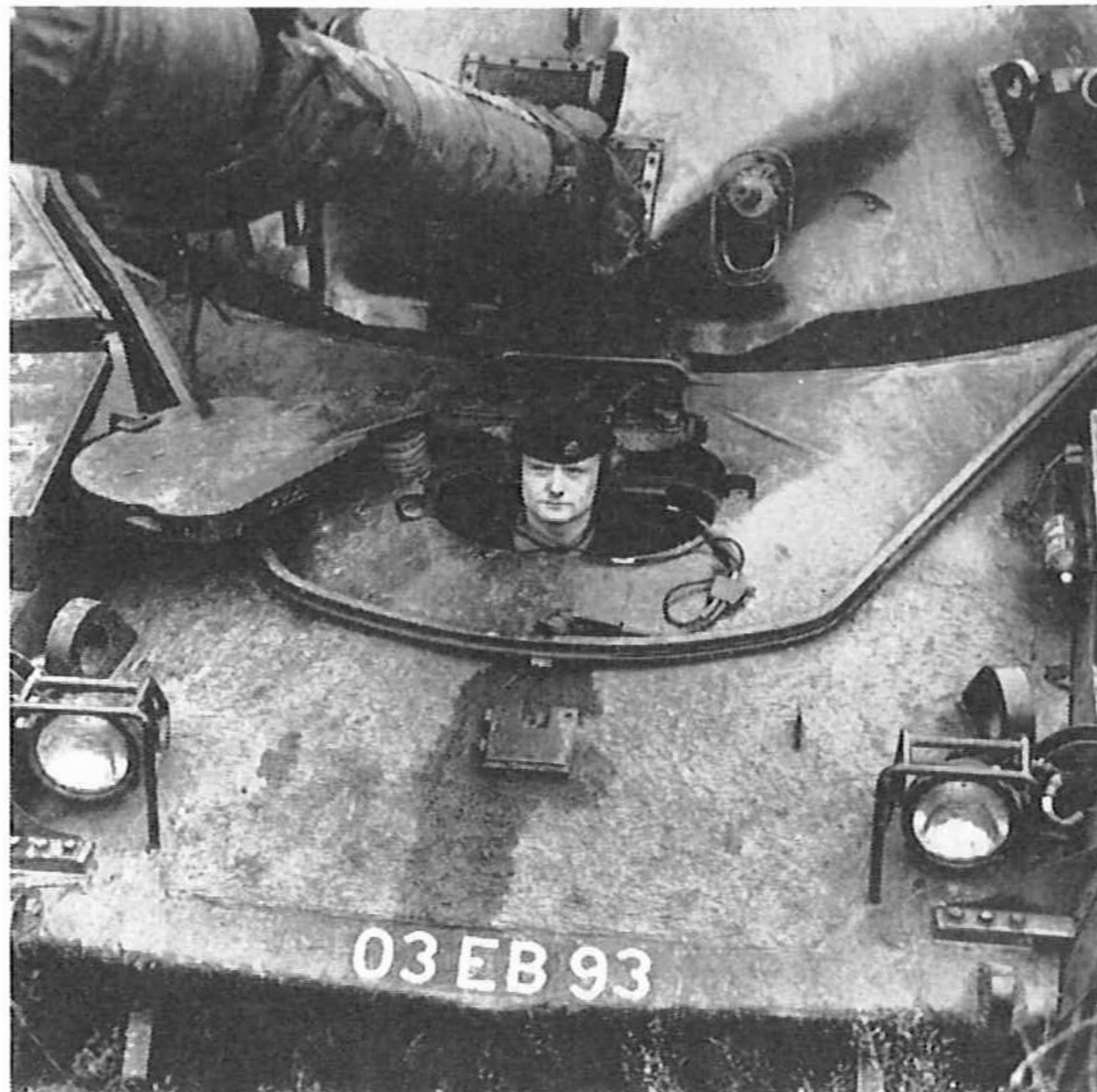
Above: Standardpanzer prototype with Type II turret mounting the 12.7-mm. ranging gun, later to be replaced by the cross-turret optical range finder. (German MOD)
