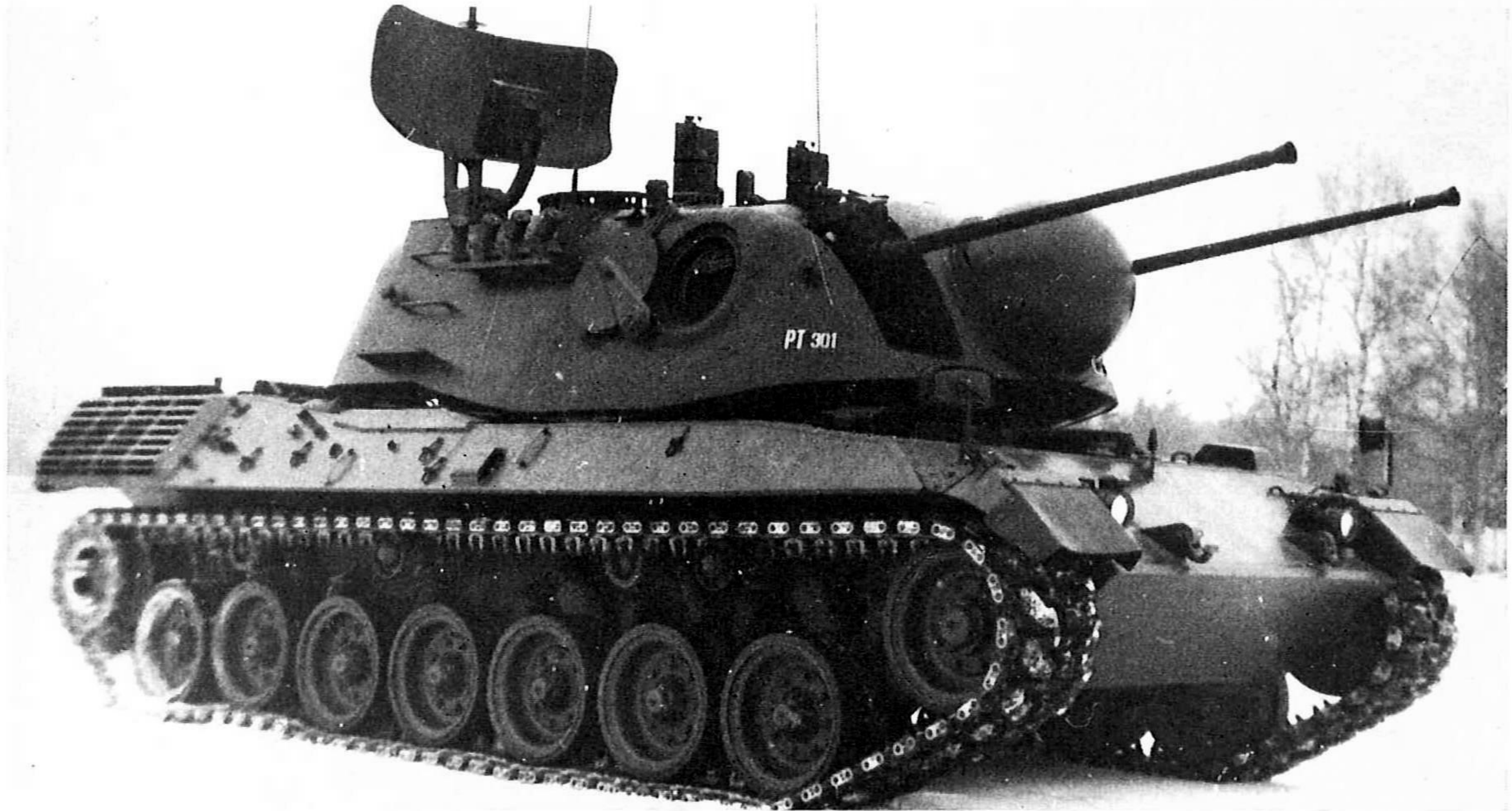
The Rheinmetall anti-aircraft Leopard with twin 30-mm. guns.
