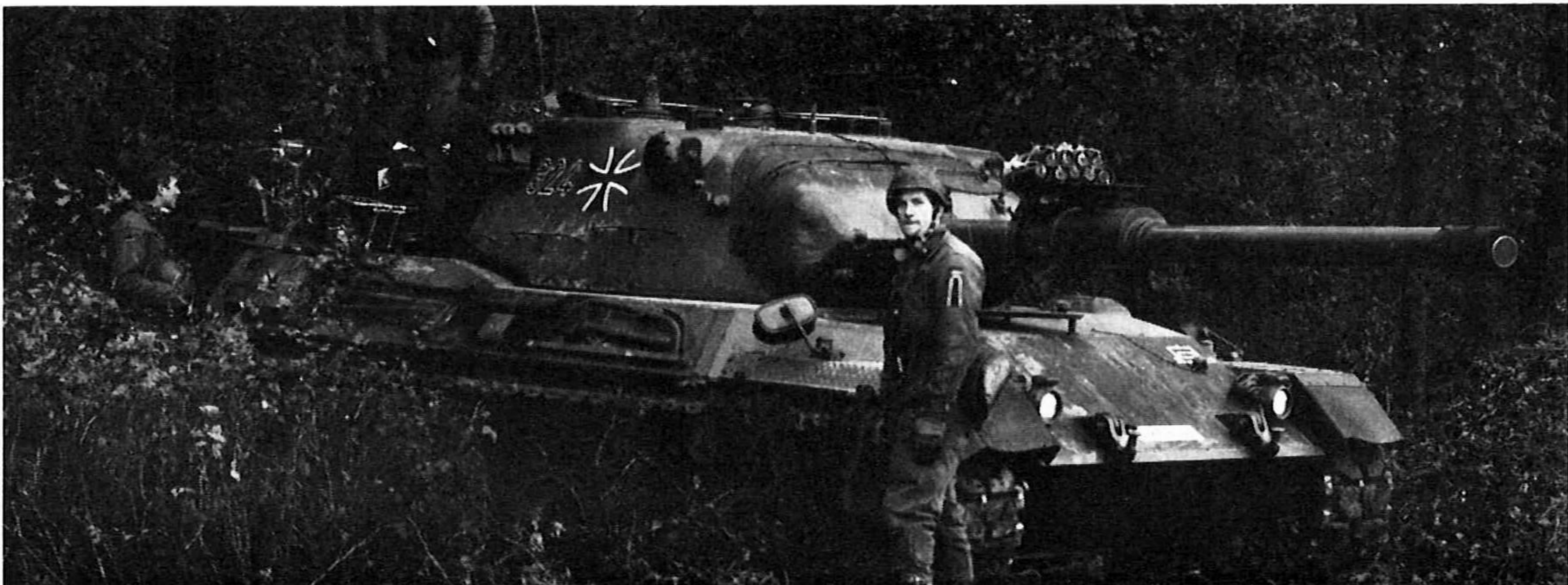
Leopard with a gunfire simulator mounted on the 105-mm. barrel.
