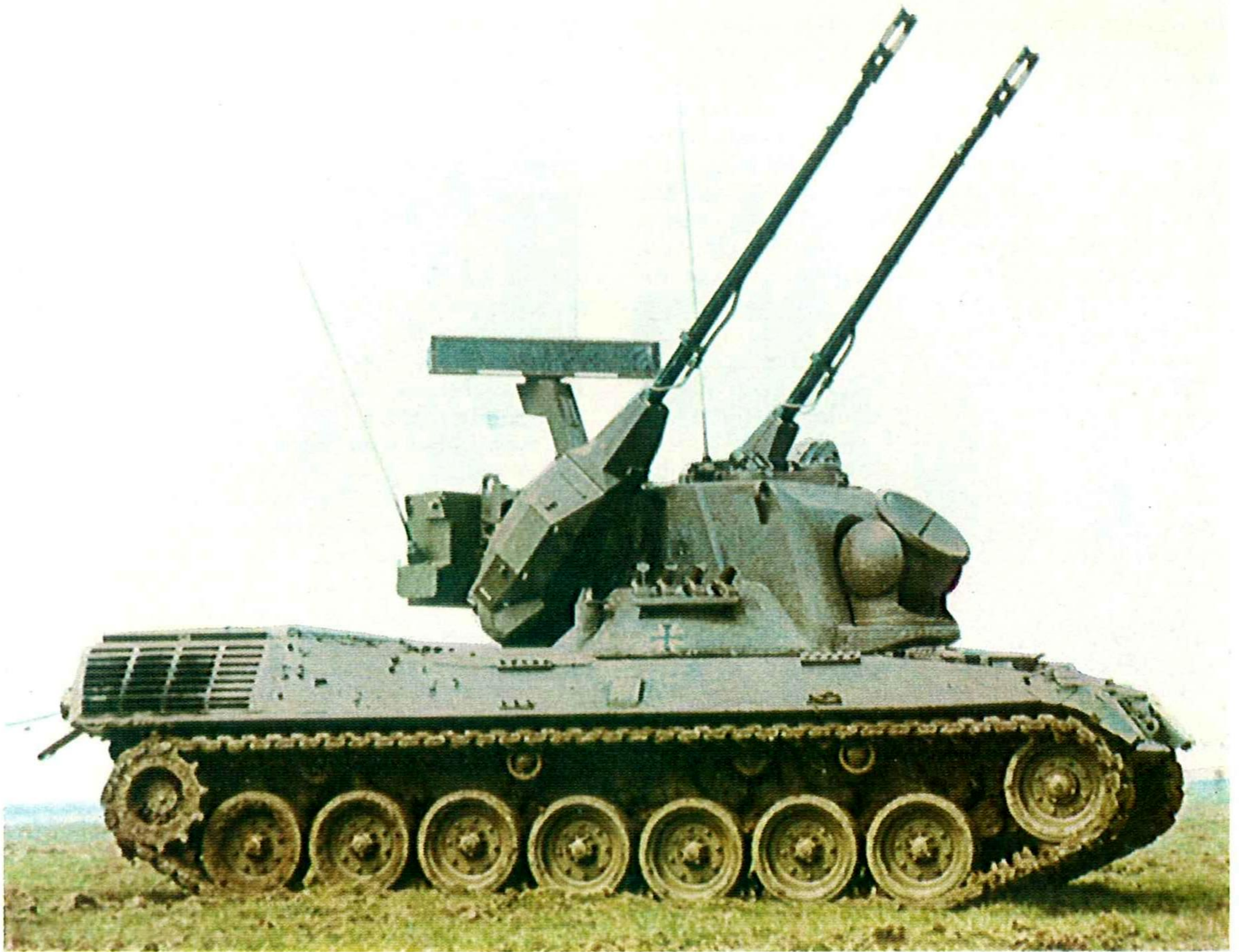
Leopard Anti-Aircraft Tank, Oerlikon-Contraves version with twin 35-mm guns and radar fire control equipment.
