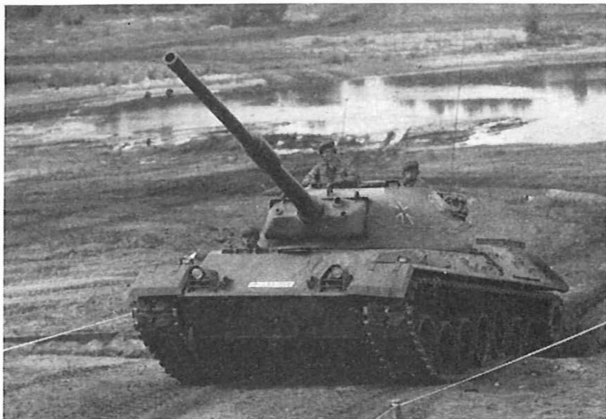
Above: Standardpanzer prototype with Type II turret mounting the 12.7-mm. ranging gun, later to be replaced by the cross-turret optical range finder. (German MOD)
