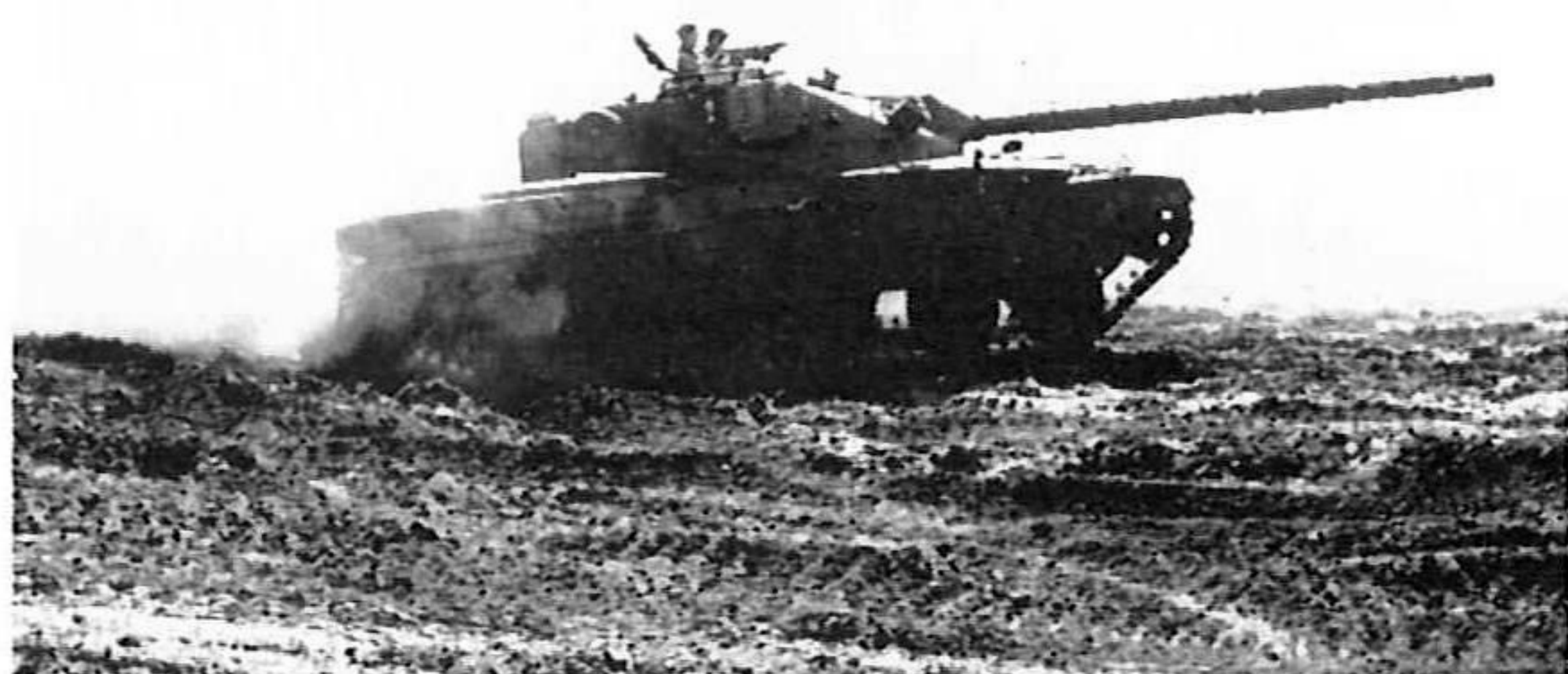
Though slower on the road than Leopard, Chieftain Mark 2's sustained cross country speed is not significantly different. (Army PR)
