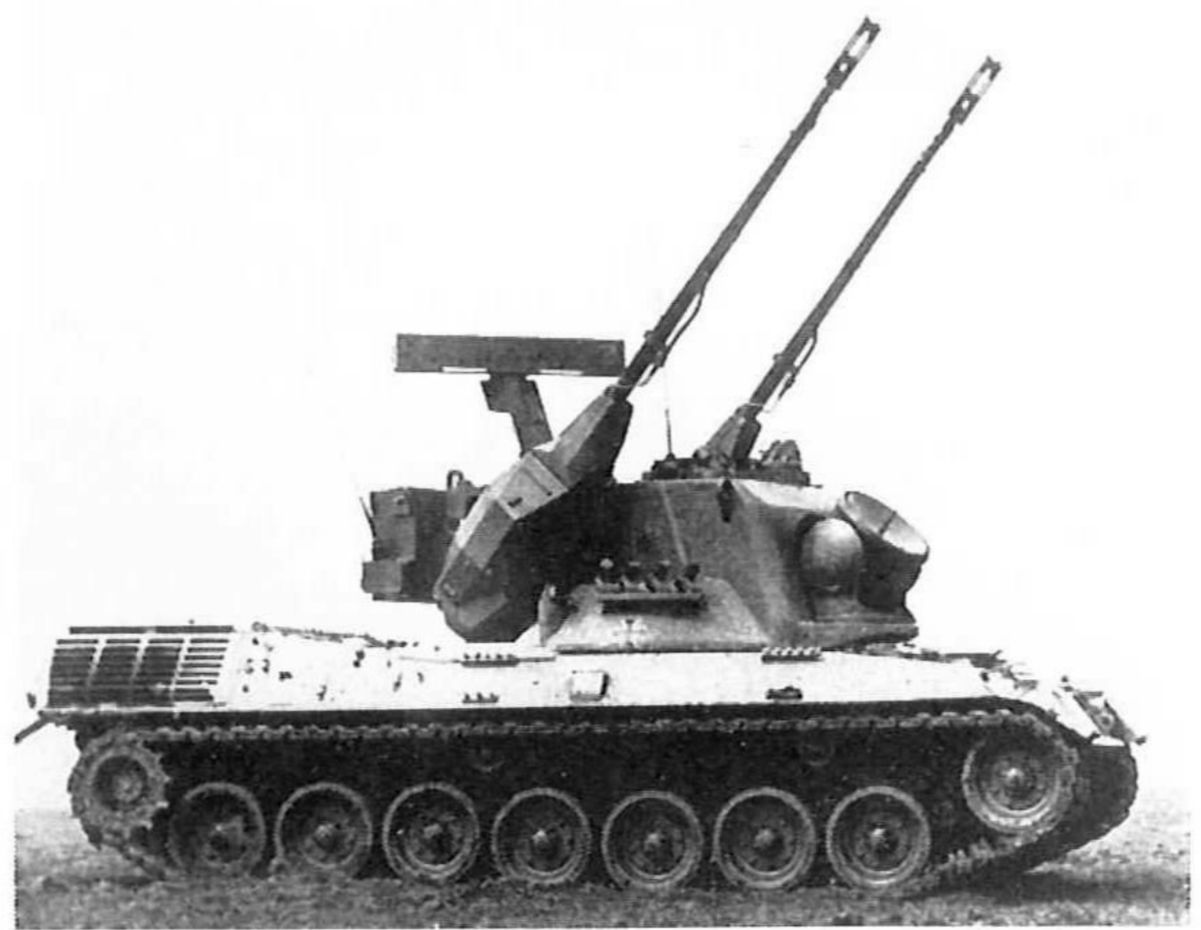
An anti-aircraft version of Leopard designed by Oerlikon-Contraves, mounting two 35-mm. guns under radar control. (Oerlikon)
