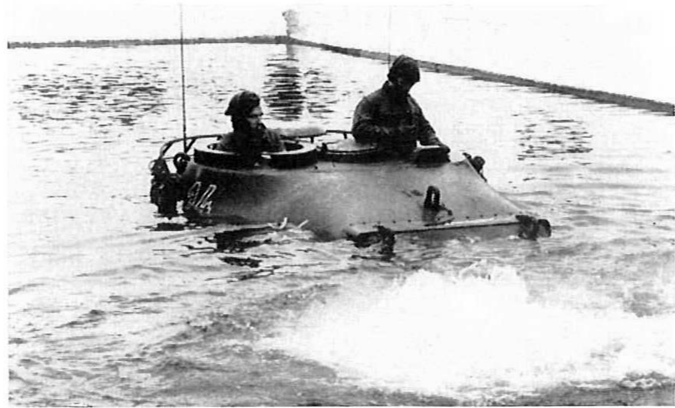
An early Leopard undergoing deep-wading tests which include stopping and re-starting the engine while submerged.
