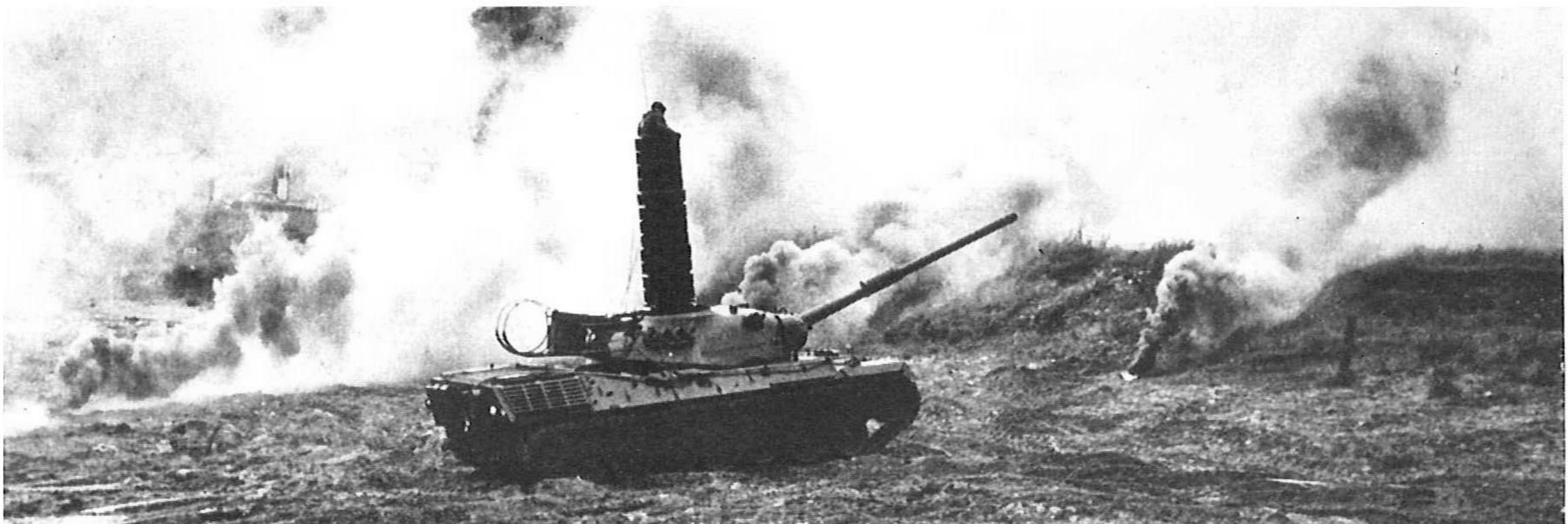
Leopard with schnorkel tower in place advancing through smoke to river crossing.
