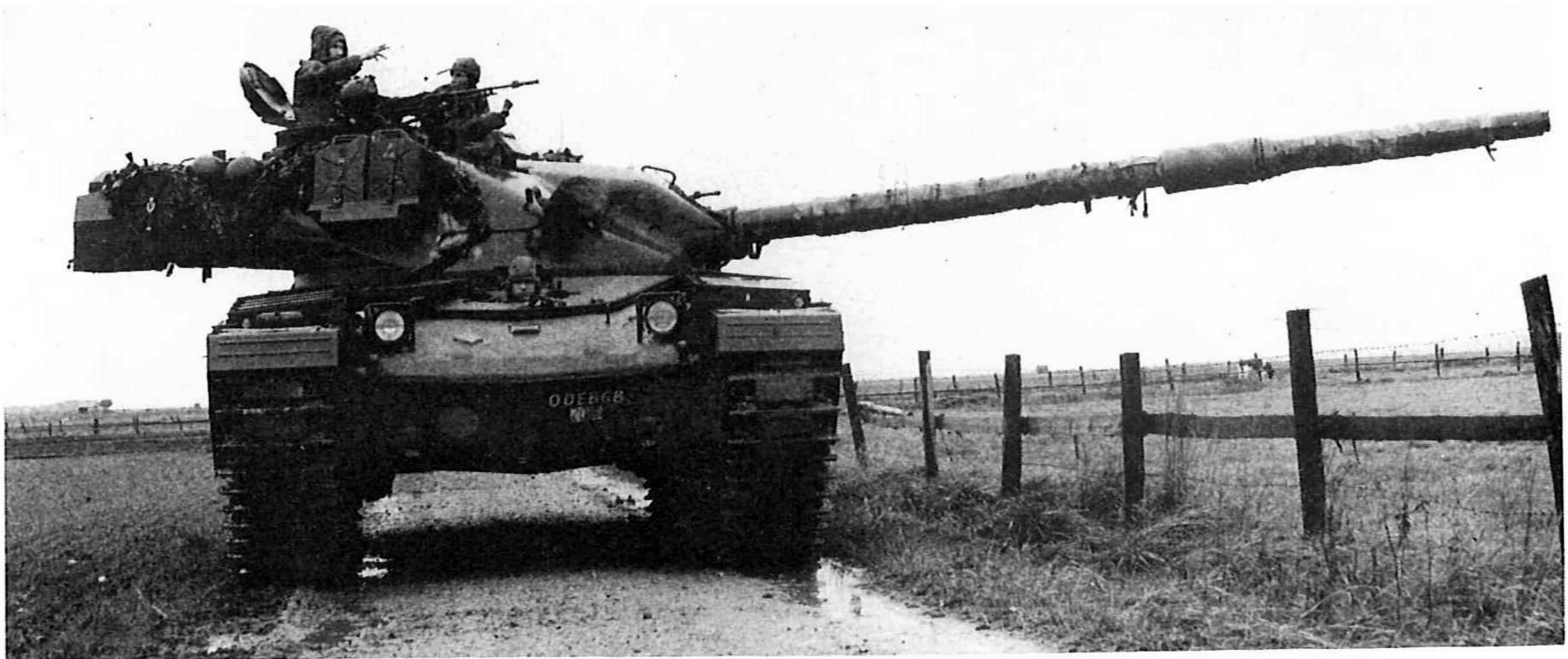
Chieftain with turret traversed, showing extent of rear bulge.
