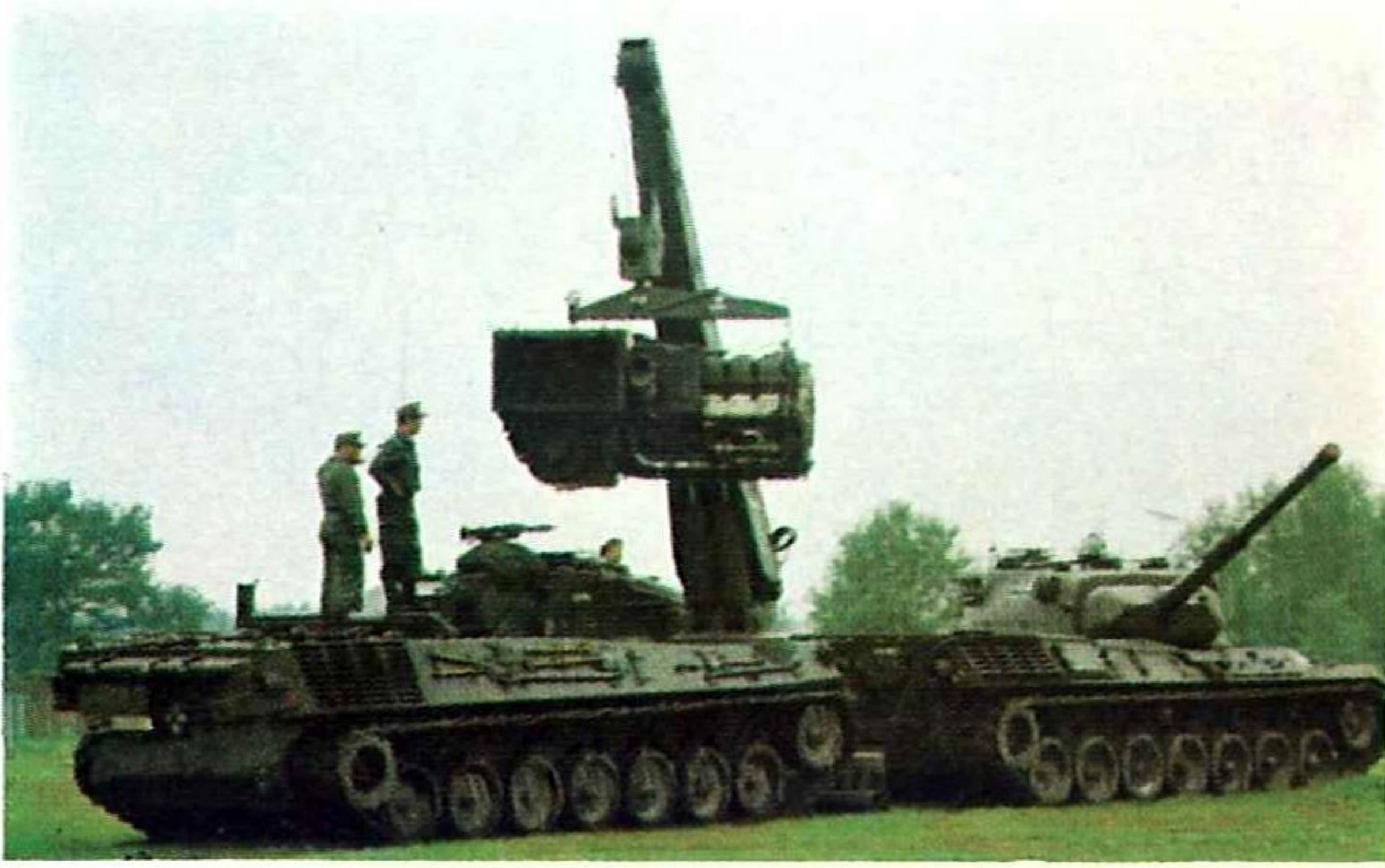
Bergepanzer standard lifting, and carrying, a complete Leopard power unit.
