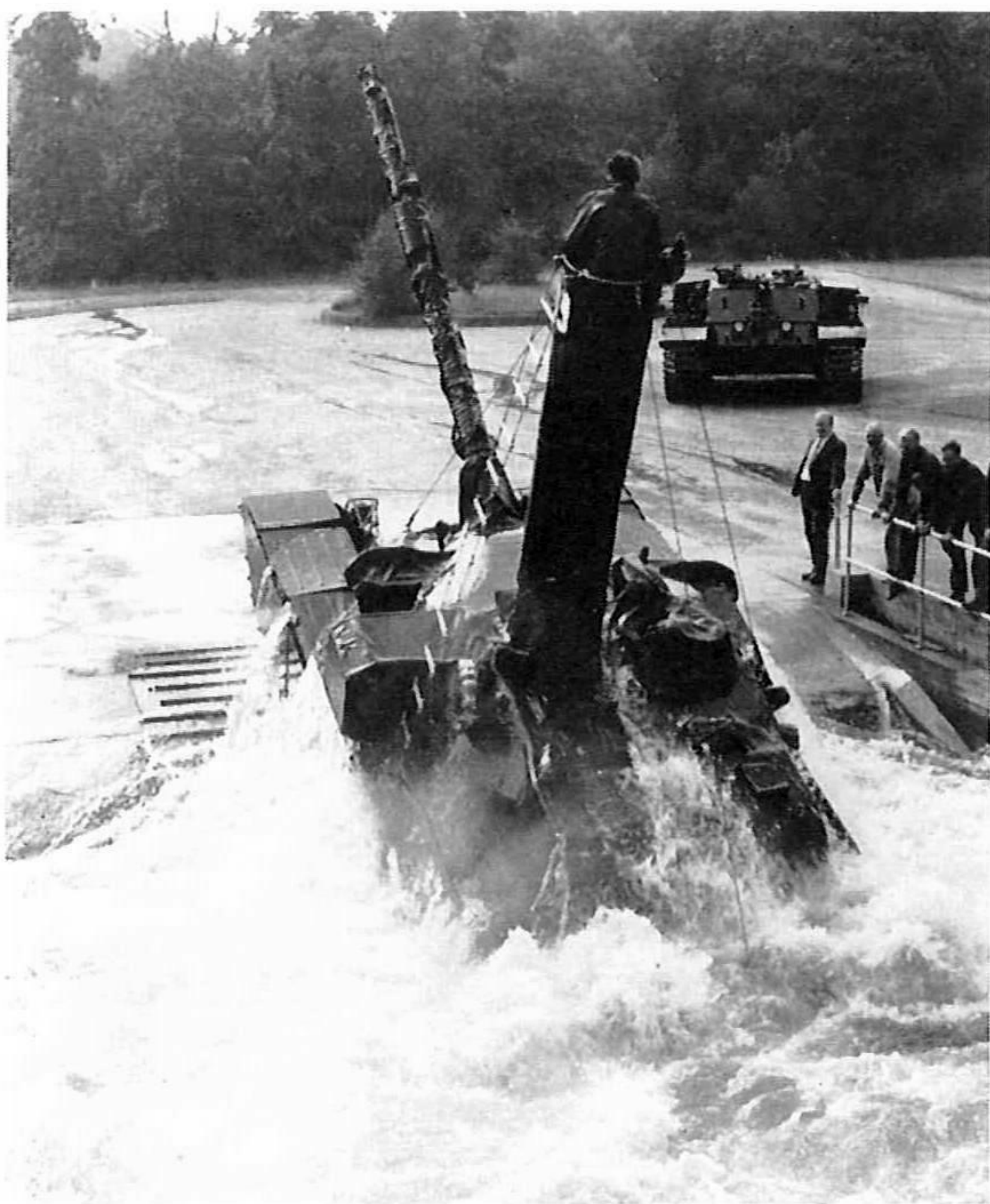
Chieftain emerging from a deep-wading pit. The commander is standing at the top of the schnorkel tower. (Keystone)
