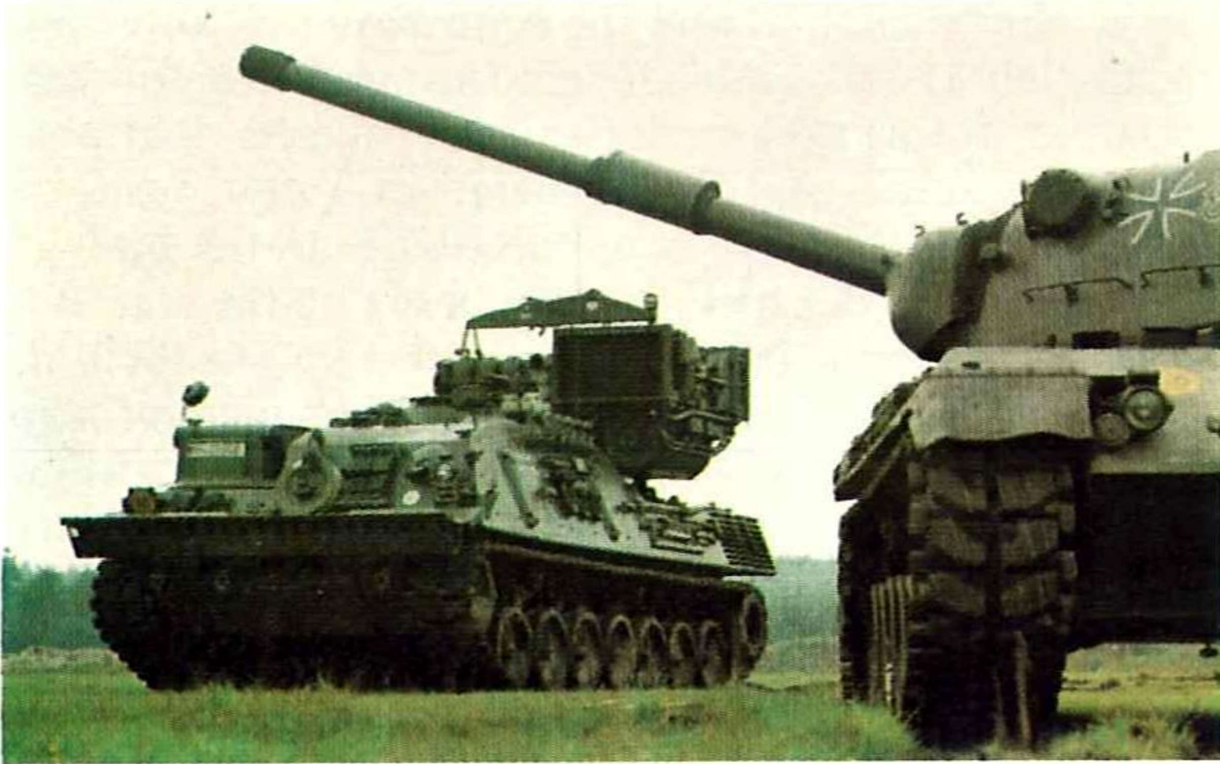
Bergepanzer standard lifting, and carrying, a complete Leopard power unit.
