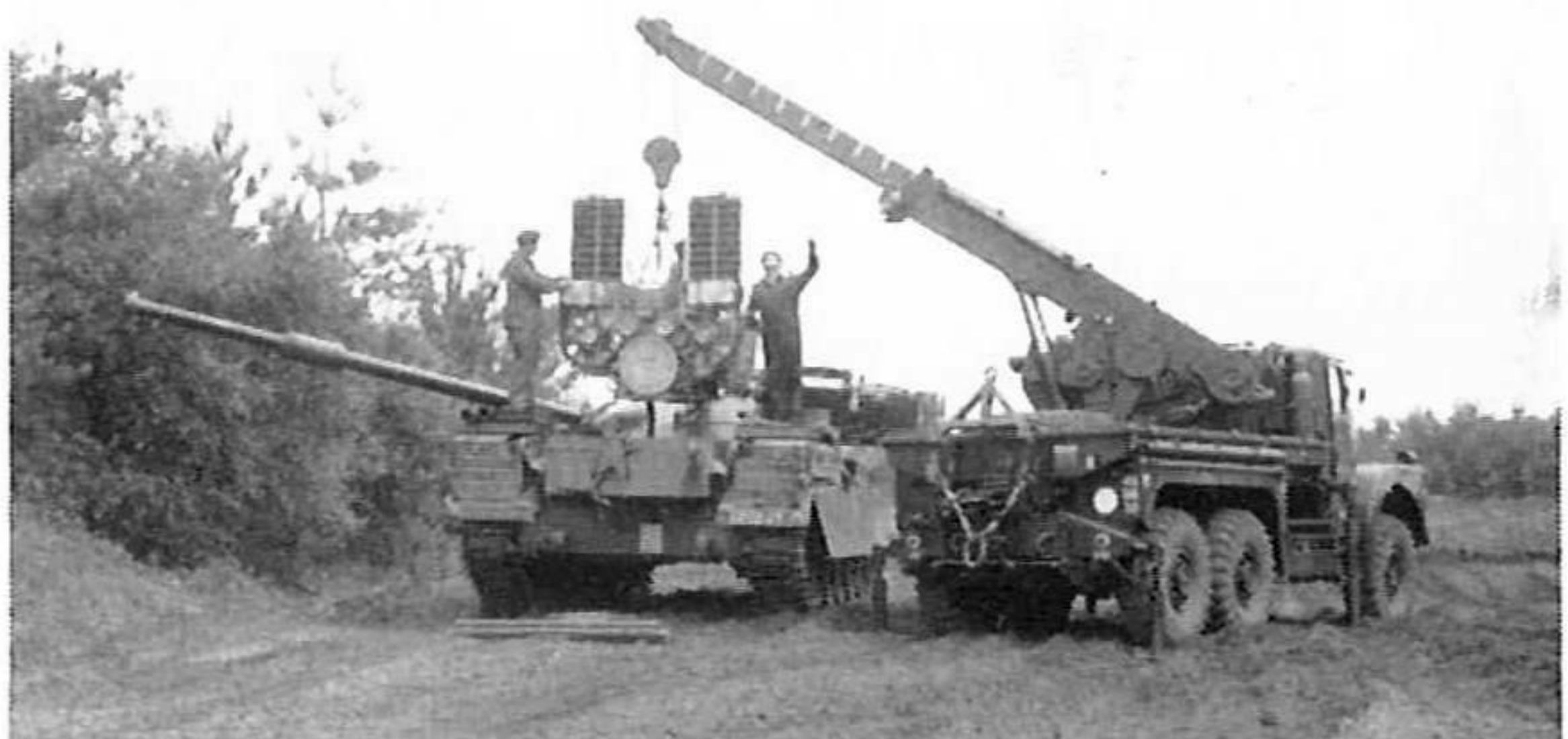
Above: The power pack of Chieftain being lifted out by REME fitters. The two cooling fans can be seen with, immediately above, the radiators that have been raised to the vertical position. (FVRDE, CCR)
