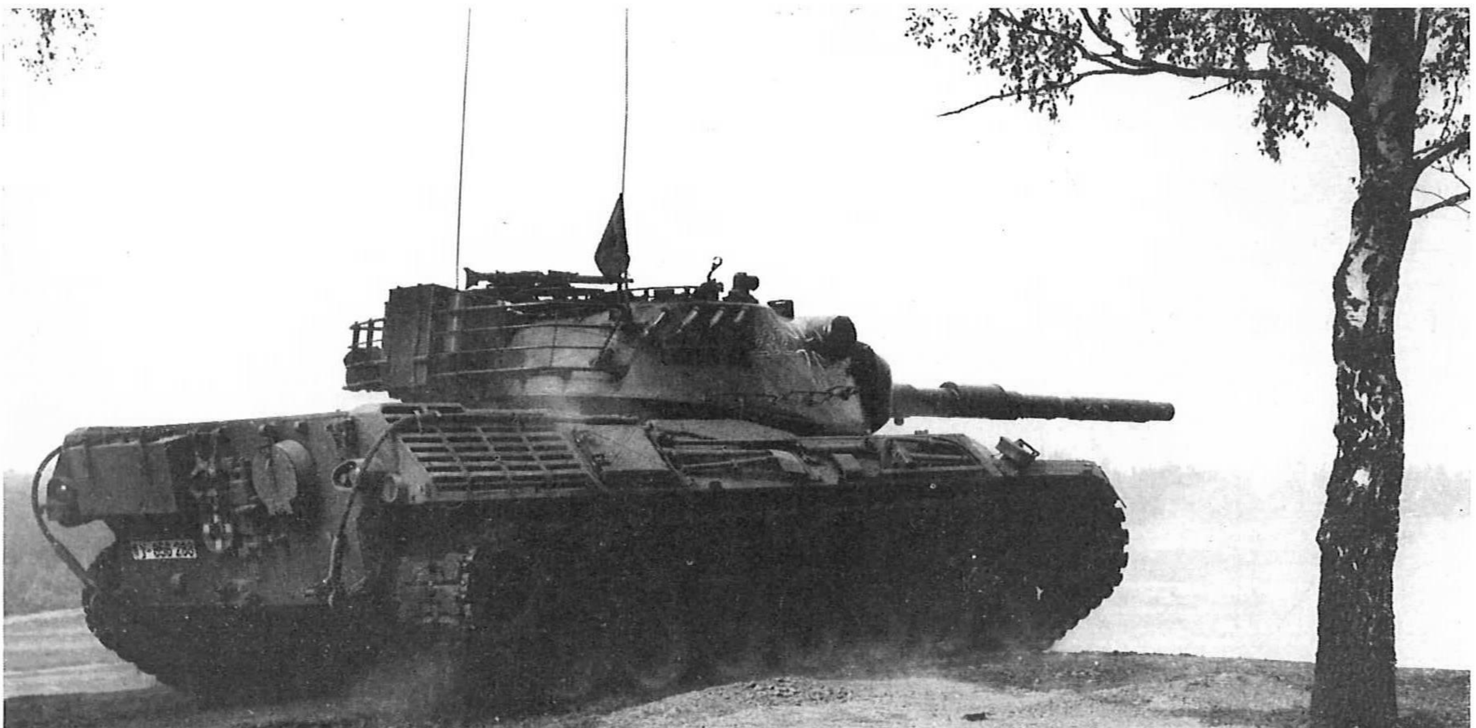
A production Leopard fitted with a thermal sleeve on the 105-mm. barrel.
