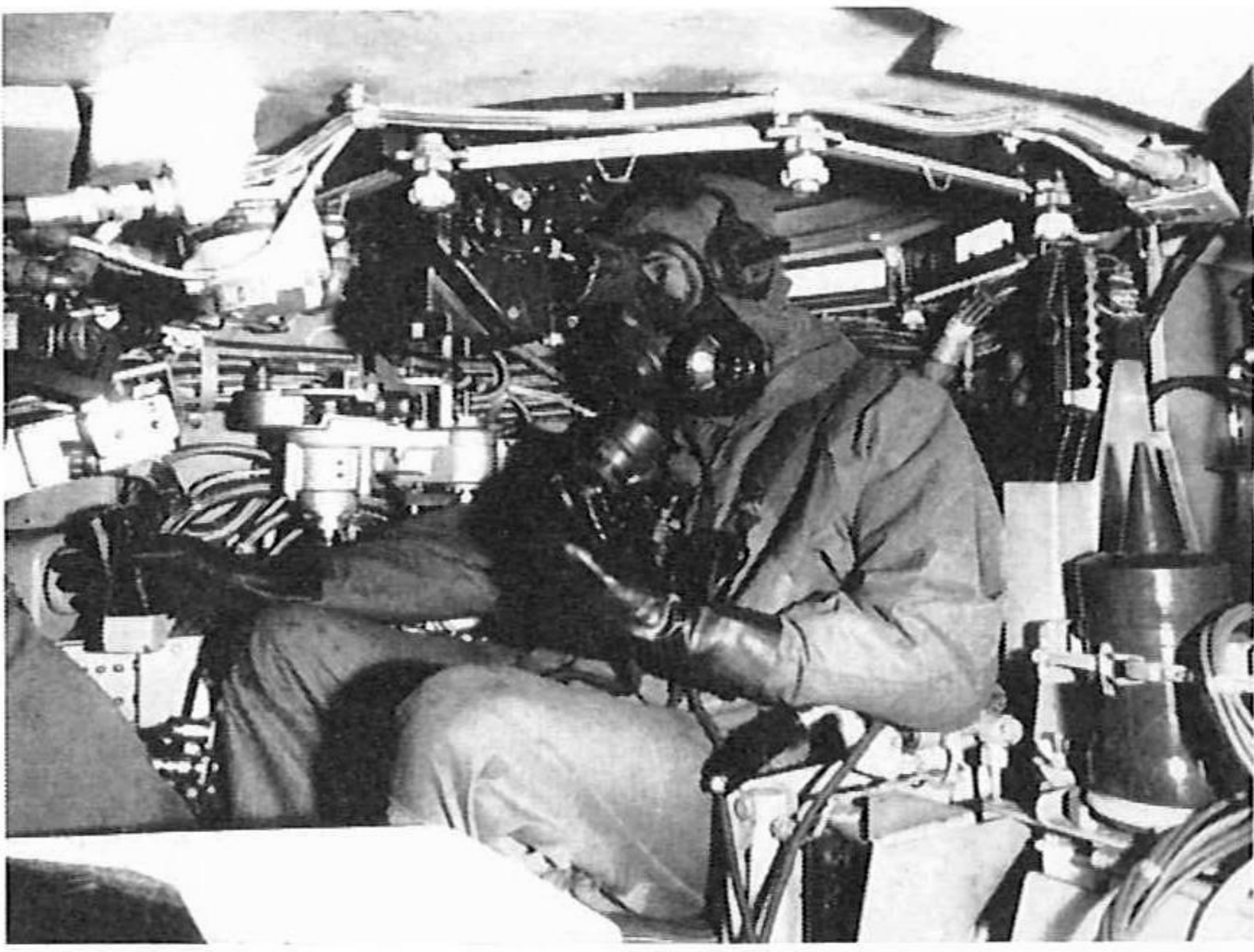
A tank commander of The Blues and Royals wearing a respirator and protective clothing. He is observing through his binocular sight and grasping his controller for powered elevation and traverse with his right hand. (CCR)
