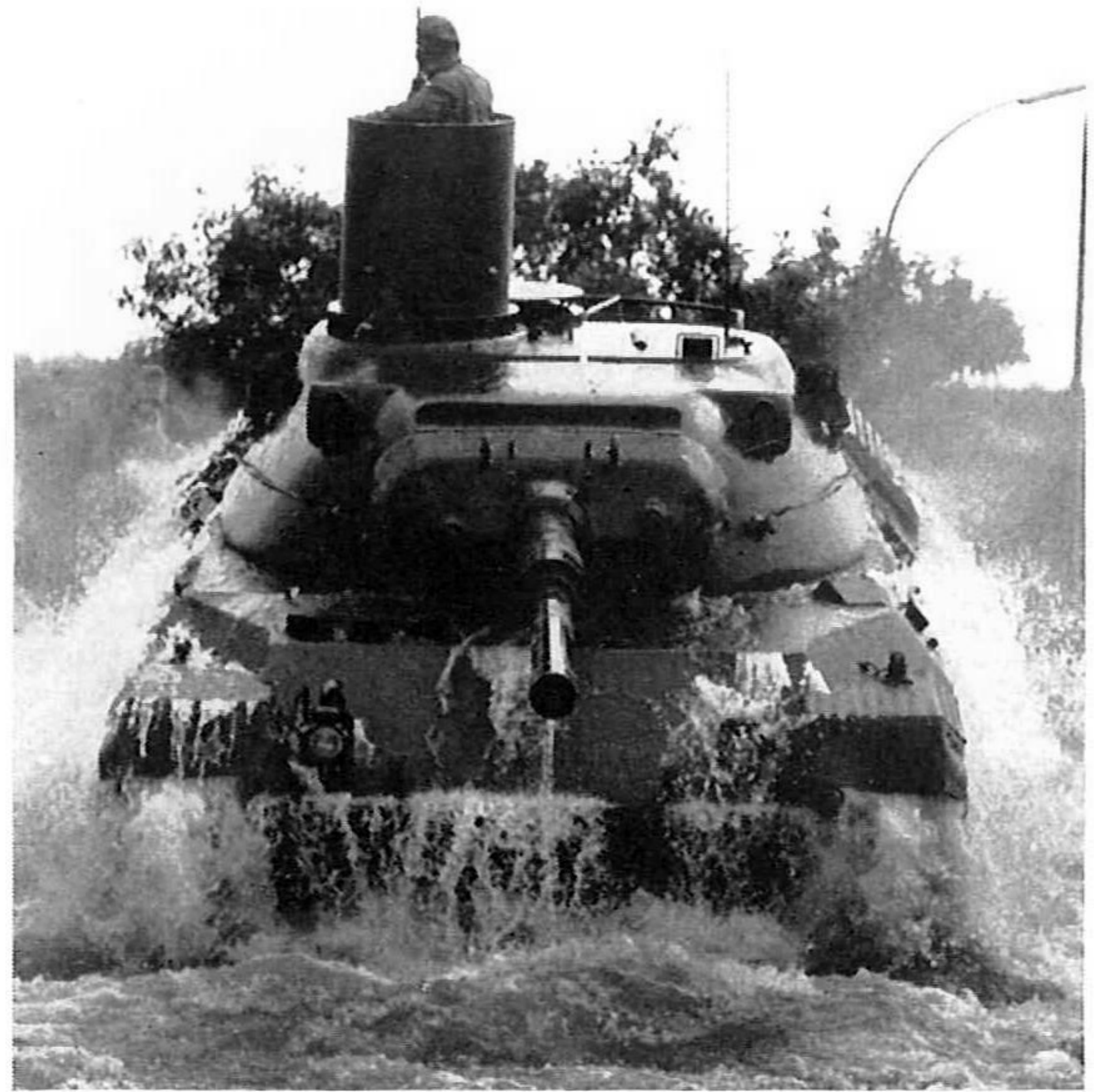
Pre-production Standardpanzer, with the bottom section of the schnorkel tower only fitted, reversing at speed from a wading tank. (German MOD)
