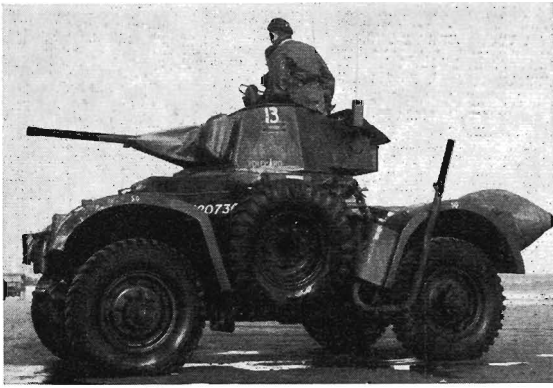
A Daimler Armoured Car of the 2nd Household Cavalry Regiment waterproofed for deep wading trials in 1944. (Imperial War Museum)
