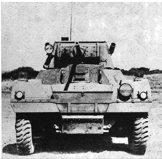
Daimler Light Tank (Wheeled)—second prototype. This car has the turret and armament as used on the production vehicles, but there are several differences in the hull details. (Imperial War Museum)
