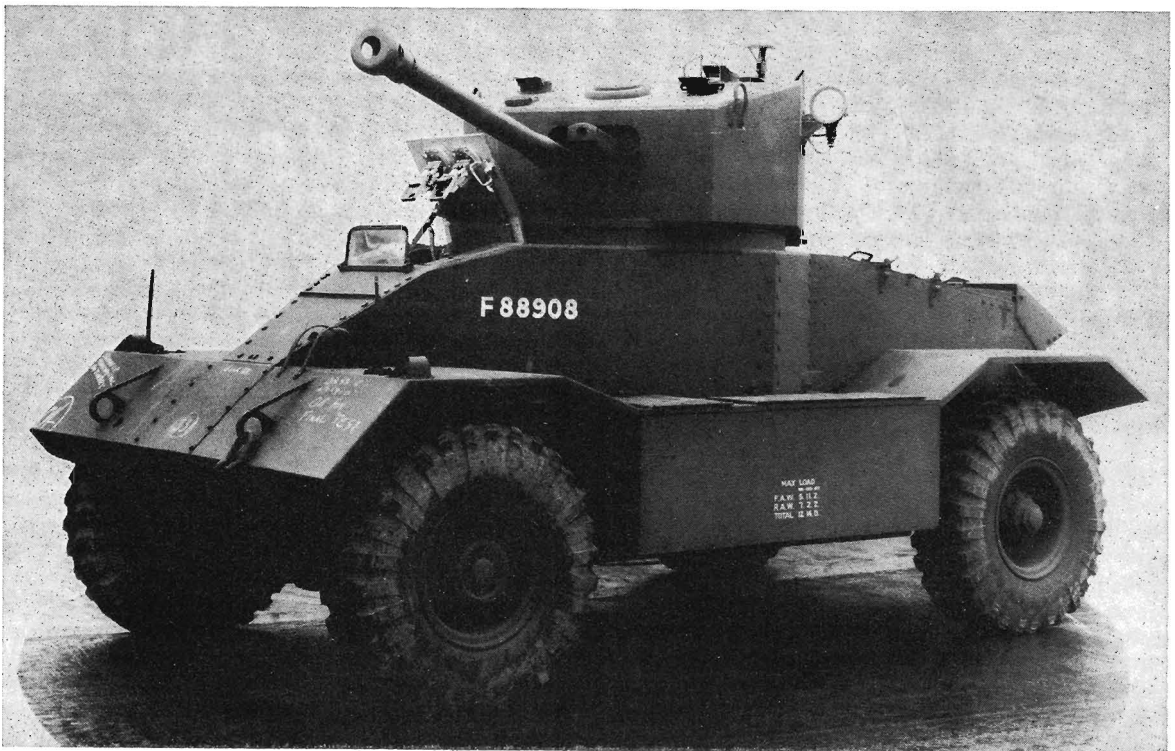
Armoured Car, A.E.C., Mark II. The Besa machine-gun is not fitted in this car and the driver's hatch is open and the windscreen erected. (A.E.C. Ltd.)
