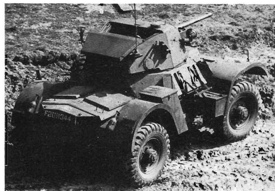
Above: Armoured Car, Daimler Mark I H.A. An experimental modification carried out in the Middle East to produce extra high elevation of the main armament. A special sight, with linkage to the mounting, was mounted on top of the turret.
