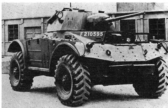
Armoured Car, Coventry Mark I. The Daimler influence in the parentage shows up clearly in this view. The weights bolted on to the nose plate are for trials purposes only.
