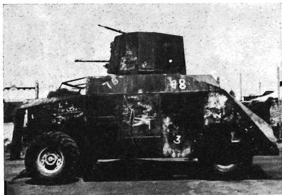
Experimental armoured car on modified front-engine A.E.C. Matador chassis. This work was carried out in Egypt in 1941. (British Official)
