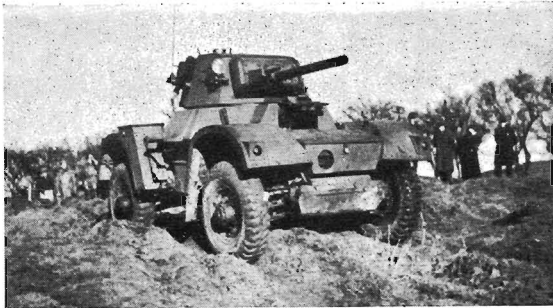
An Armoured Car, Daimler Mark I CS in which the 2-pdr. gun has been replaced by a 3-in. howitzer. (The Daimler Co.)
