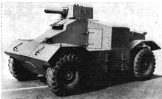
Basilisk flamethrower armoured car. A small turret for a flame projector mounted on a hull adapted from that of the basic armoured cars. This vehicle was intended to accompany armoured car units in the field but did not get beyond the experimental stage because the requirement for this particular type of vehicle was cancelled. (A.E.C. Ltd.)
