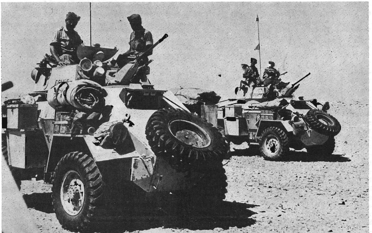
Below: Humber Mark II Armoured Cars of the 12th Royal Lancers on patrol in the desert in the region of the Qattara Depression, 1942. Much extra equipment had to be carried on these long range patrols and the cars have fittings, including a sun compass on the turret side and a spare wheel, which were not on Home service. (Imperial War Museum/Jaguar Cars Ltd.)
