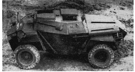
Car, Scout Humber Mark I. A view from above showing the fixed roof with two sliding hatches. (Tank Museum)
