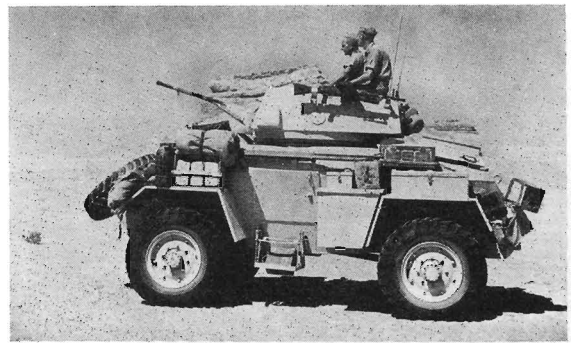
Armoured Car, Humber Mark III. This side view (of a car with full Desert equipment on patrol near the Qattara Depression) shows the new form of turret with increased head room. (Imperial War Museum)
