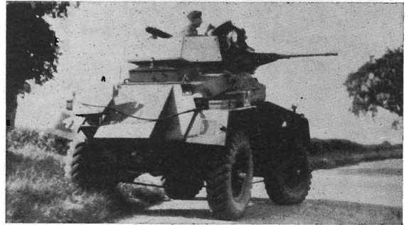
A rear view of an Armoured Car, Guy Mark IA. This shows clearly the "solid" rear plate, with air intake underneath. This car is of the 2nd Derbyshire Yeomanry on an exercise in 1941.
