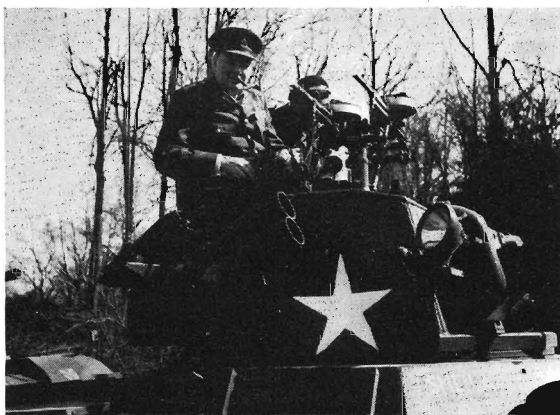
Daimler Mark I Armoured Car. A good close-up of Winston Churchill and also a clear view of turret details of his car, including the twin smoke dischargers, the gun mounting and the P.L.M. mounting on top for two 0.303-in. Vickers "K" machine-guns.
