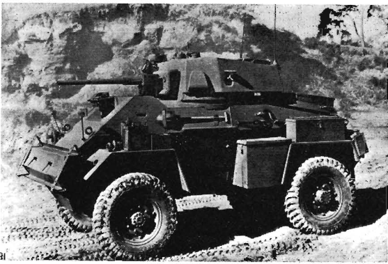
Armoured Car, Humber Mark IV. Apart from the 37-mm. gun, this model was similar in most respects, externally, to the Mark III. Note the un-ditching channel carried across the front glacis plate. (Rootes Ltd.)
