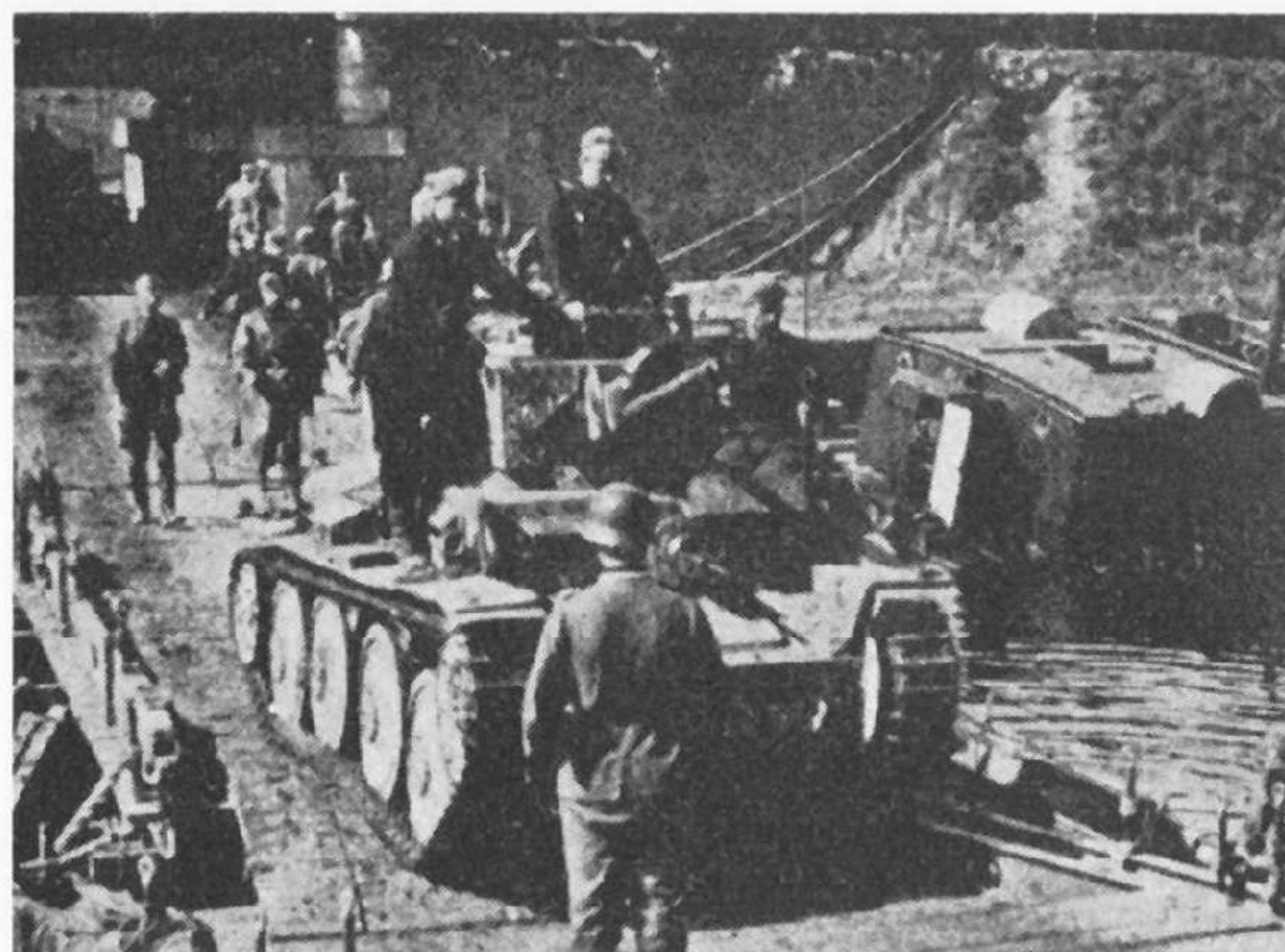
Above and right: The final production model of the TNHP (Model H). This vehicle has the increased armour thickness and other minor alterations. (Milsom Collection)
