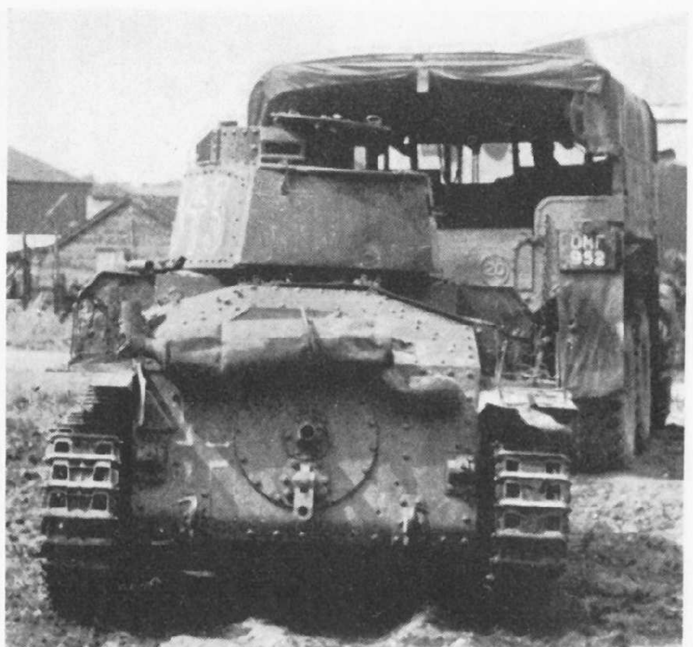
Rear view of the Model E; compare the exhaust pipe arrangement with the Model F. (Chamberlain Collection)
