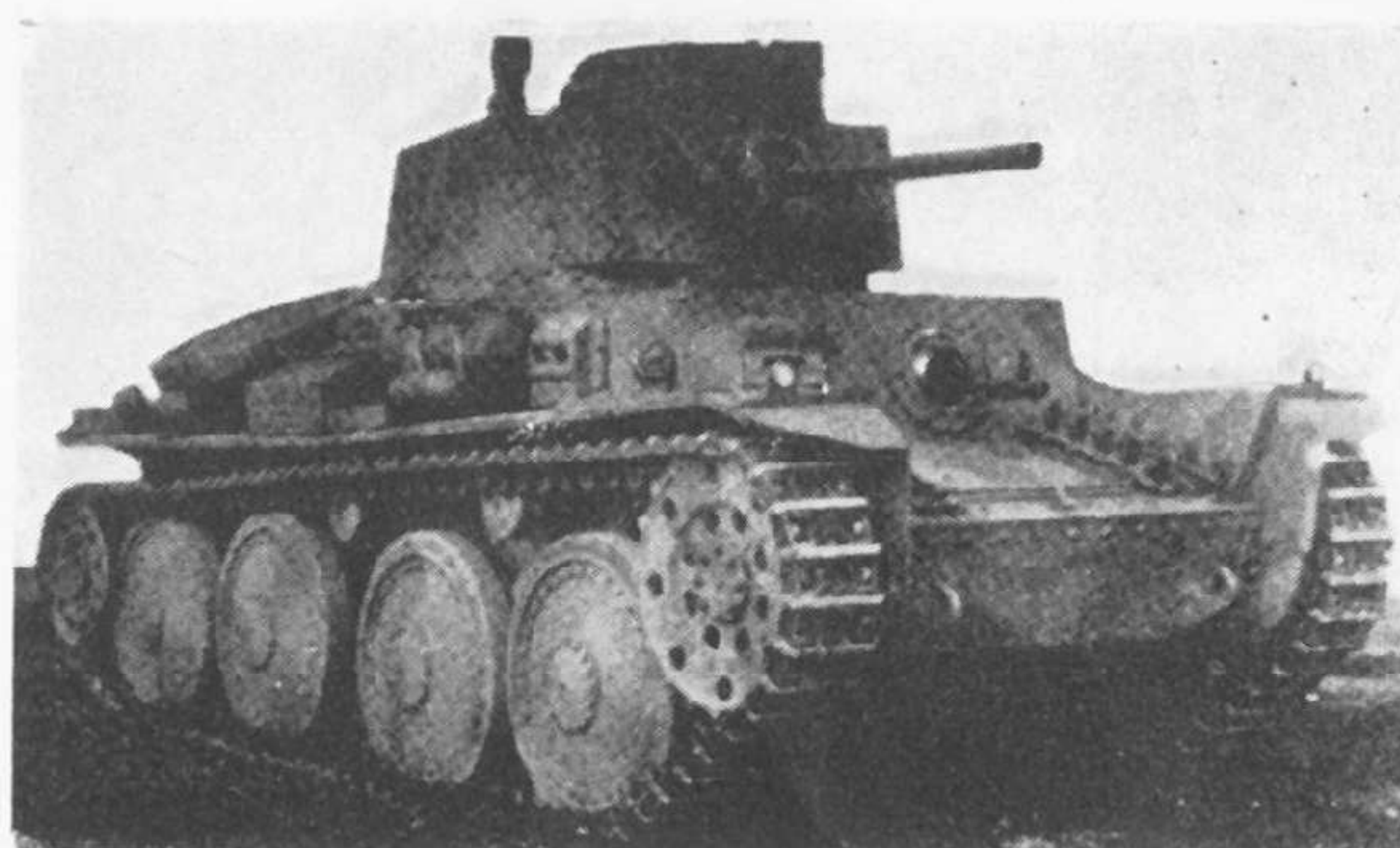
The seventh production model TNHP (Model S), originally built for Sweden. Note the cylindrical device (function unknown) on the RHS behind the driver's episcopes. Photos are of the Swedish vehicle (Strv m/41).
