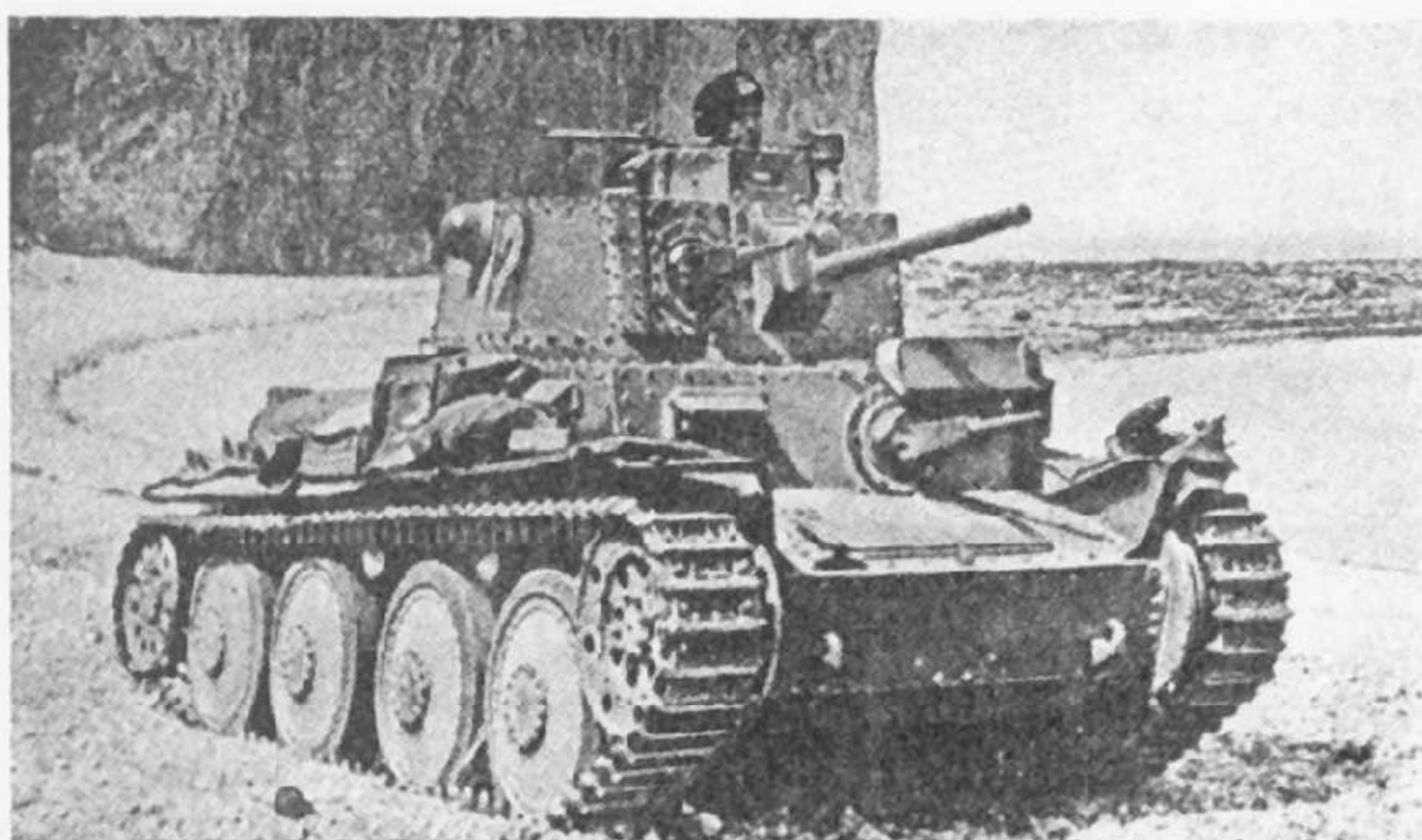
Above and right: The final production model of the TNHP (Model H). This vehicle has the increased armour thickness and other minor alterations. (Milsom Collection)
