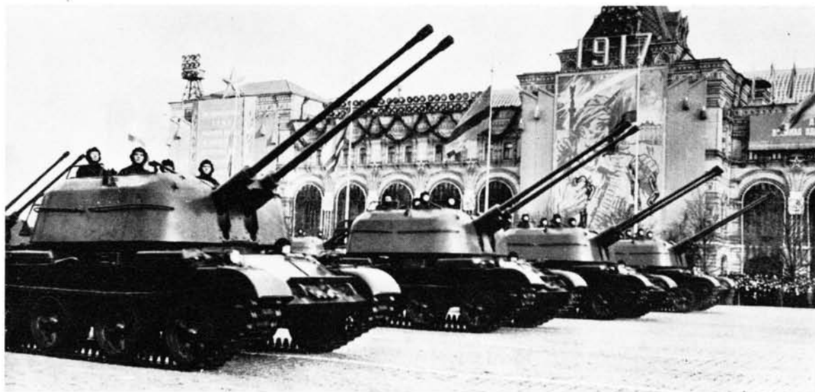
ZSU-57-2 self-propelled AA guns based on a shortened T-54 chassis with four instead of five road wheel positions.
