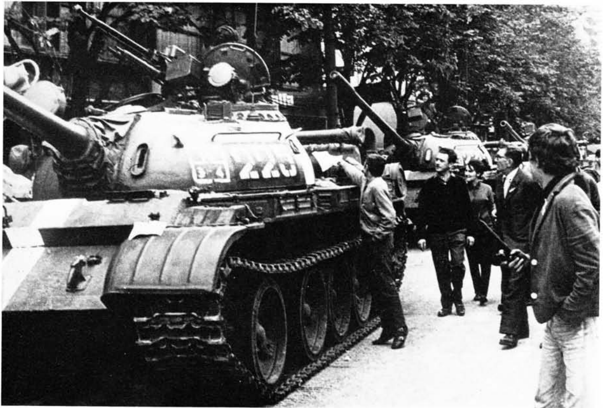
A T-54A(M) in Prague 1968. The long equilibrator tubes needed to balance the 12.7 mm. AAMG are visible under the barrel. (Photo: Keystone)
