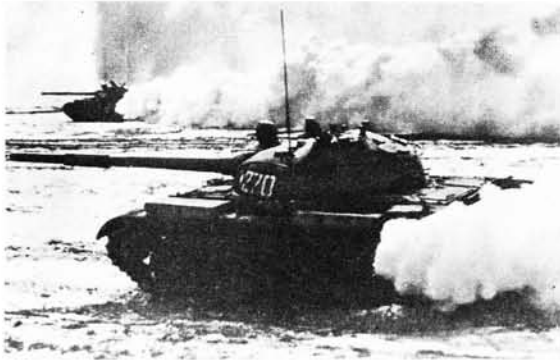
Top left: T-62 tanks discharging a dense screen of partially burnt fuel oil from their exhausts.
