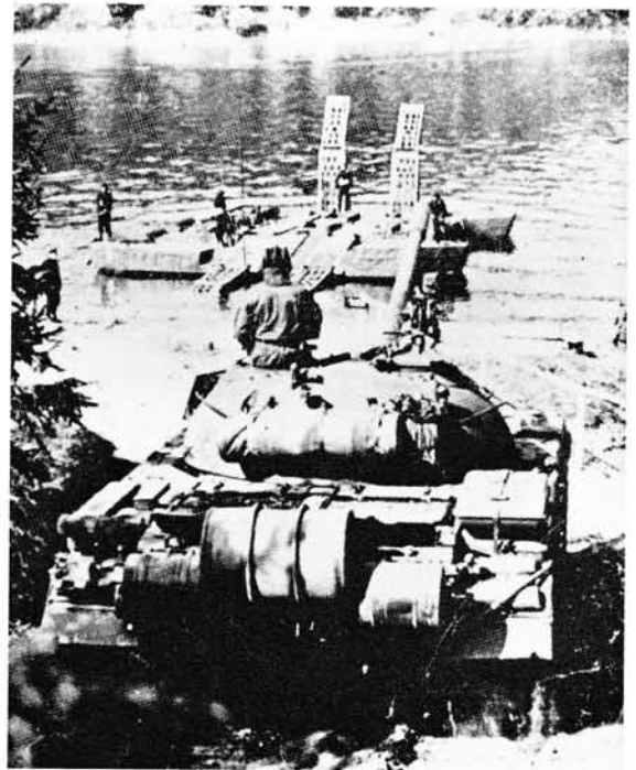
T-55 tanks wading a river during an exercise. The disturbance to the water surface caused by the engine exhaust gases can be seen to the left of the tubes of the two leading tanks.
