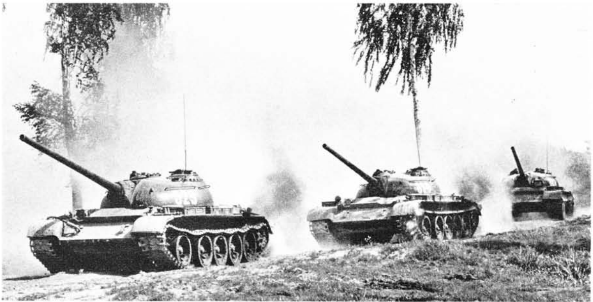
A platoon of the first version of the T-54 tank to be produced in quantity on exercise manned by the Soviet Taman Guards. The design of the turret has been altered but the early 100-mm. gun, with its plain section barrel without a fume extractor, has been retained. (Photo: Camera Press)
