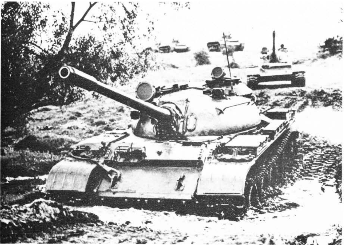
A T-55 fording a shallow stream. As well as the absence of the loader's cupola and the ventilation dome, note the change in design of the commander's cupola and his new sight.
