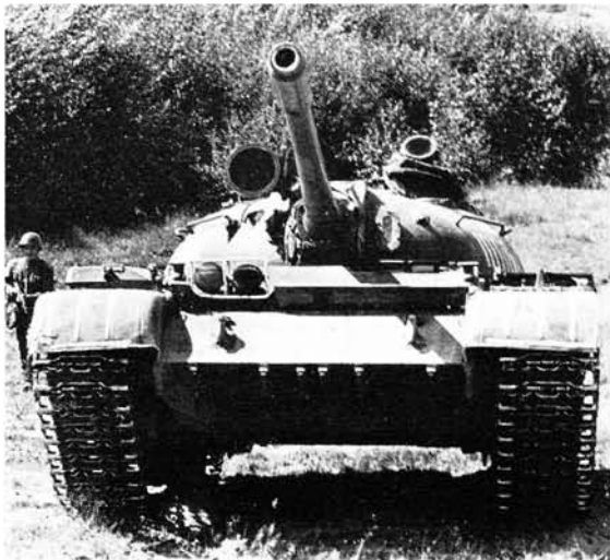
A Soviet T-54(X), recognizable by its flush loader's hatch and by the fact that the main IR searchlight is attached to the gun barrel itself. The T-54B is similar except it has the normal cupola for the loader. (Photo: Camera Press)
