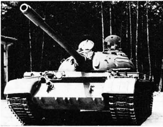
T-54A showing the mounting lugs welded on the nose plate for the attachment of a dozer blade, as well as the splash board on the glacis which was first introduced on the T-44. Note fume extractor fitted near the gun muzzle.
