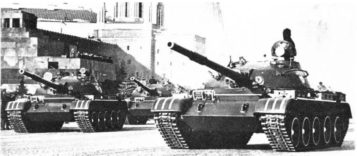
T-62 tanks in parade livery marching past Lenin's tomb in Moscow. The change to a circular aperture for the gunner's sighting telescope can be seen on the nearer vehicle.
