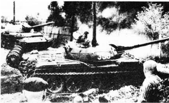
Czech T-54 tanks moving forward to a river crossing site with the folding schnorkel tube erected over the loader's periscope housing and with waterproofing equipment installed. The loader's cupola and the rear brackets for fuel drums appear to be different to those on T-54 tanks in Soviet service. (Photo: Soldat und Technik)
