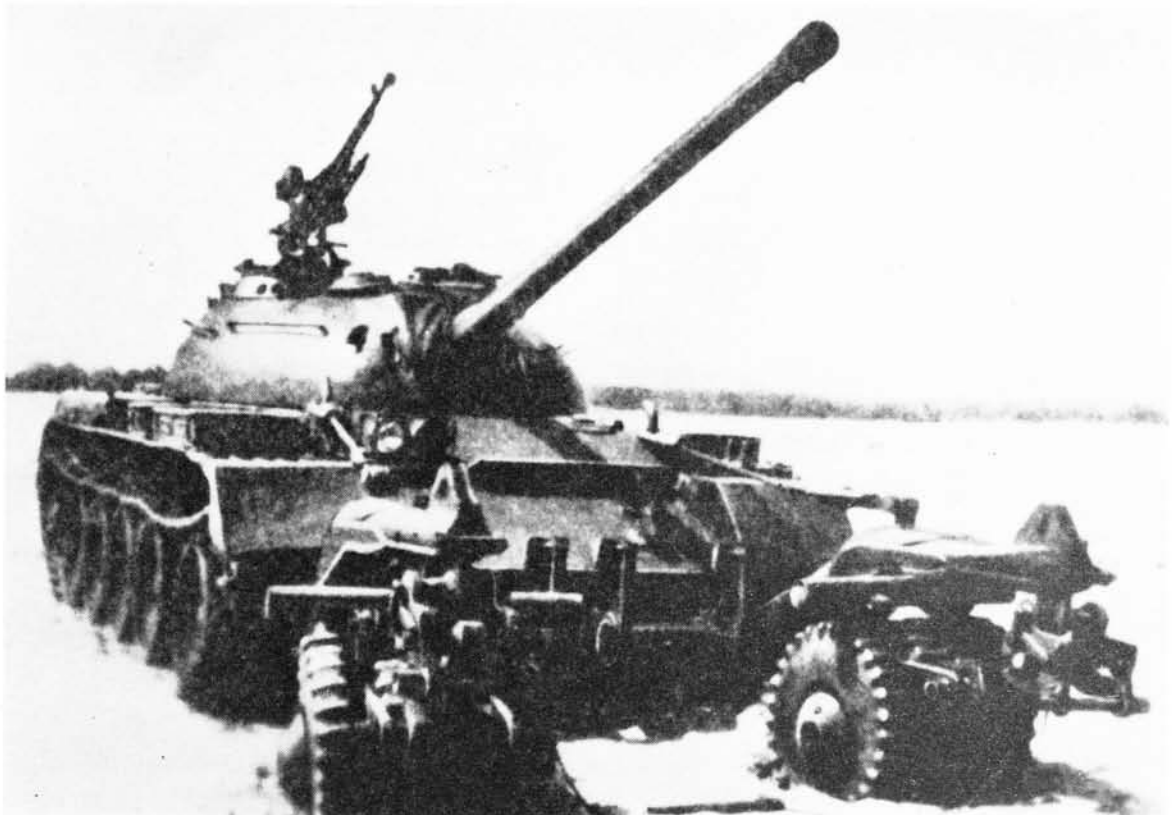
The PT-54 mine roller equipment based on an obsolescent T-54.
