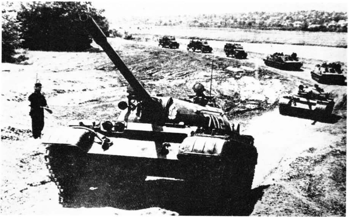
Two T-55 tanks from the Kiev Military District lead a column of motorised infantry which includes two BTR-50p APCs. An additional small IR projector can be seen to the left and below the main searchlight.
