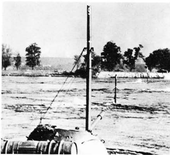
T-55 tanks wading a river during an exercise. The disturbance to the water surface caused by the engine exhaust gases can be seen to the left of the tubes of the two leading tanks.
