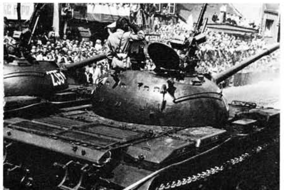
Polish T-54A tanks showing the excellent ballistic shape of the turret without the cut-away portion of the earliest version. The 12.7-mm. DShK anti-aircraft MG is mounted prominently in front of the loader's hatch. Note also the lightly armoured fuel tanks on the rear of the track guard and the hand-rails on the turret for use by mounted infantry.
