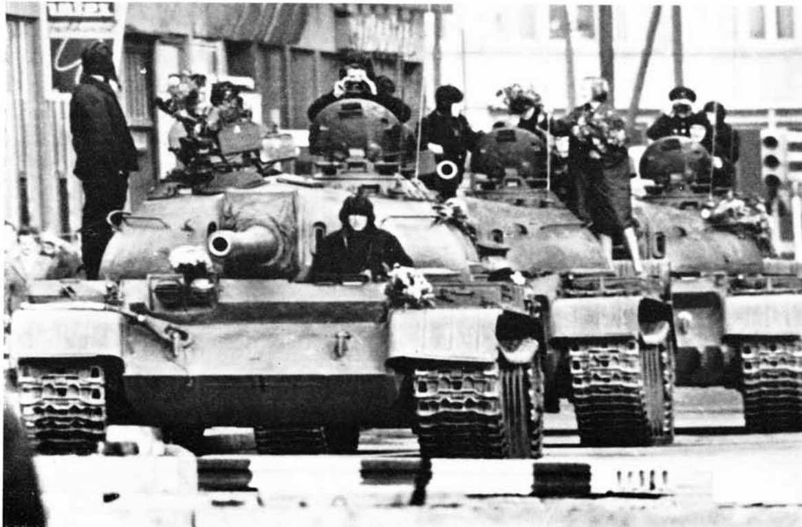
T-54A tanks at Check-point Charlie in Berlin in October 1961. A presentation of bouquets to the tank crews is in progress. The ventilation dome in front of the loader's cupola is a distinctive feature of the T-54 series. (Photo: Associated Press)
