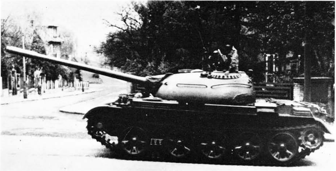
A T-54A. Note the prominent gap between the first and second road wheels. The exhaust cowl is visible as the narrow oblong shape on the track guard just to the rear of the long stowage bin.
