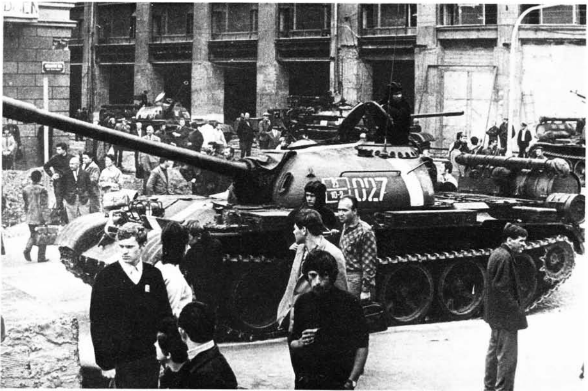
A Soviet T-54A used in the occupation of Prague in August 1968. The radio antenna is on the left of the commander's cupola. Two large fuel drums are carried in addition to the smoke canisters with the schnorkel tube secured across the top. (Photo: Keystone)
