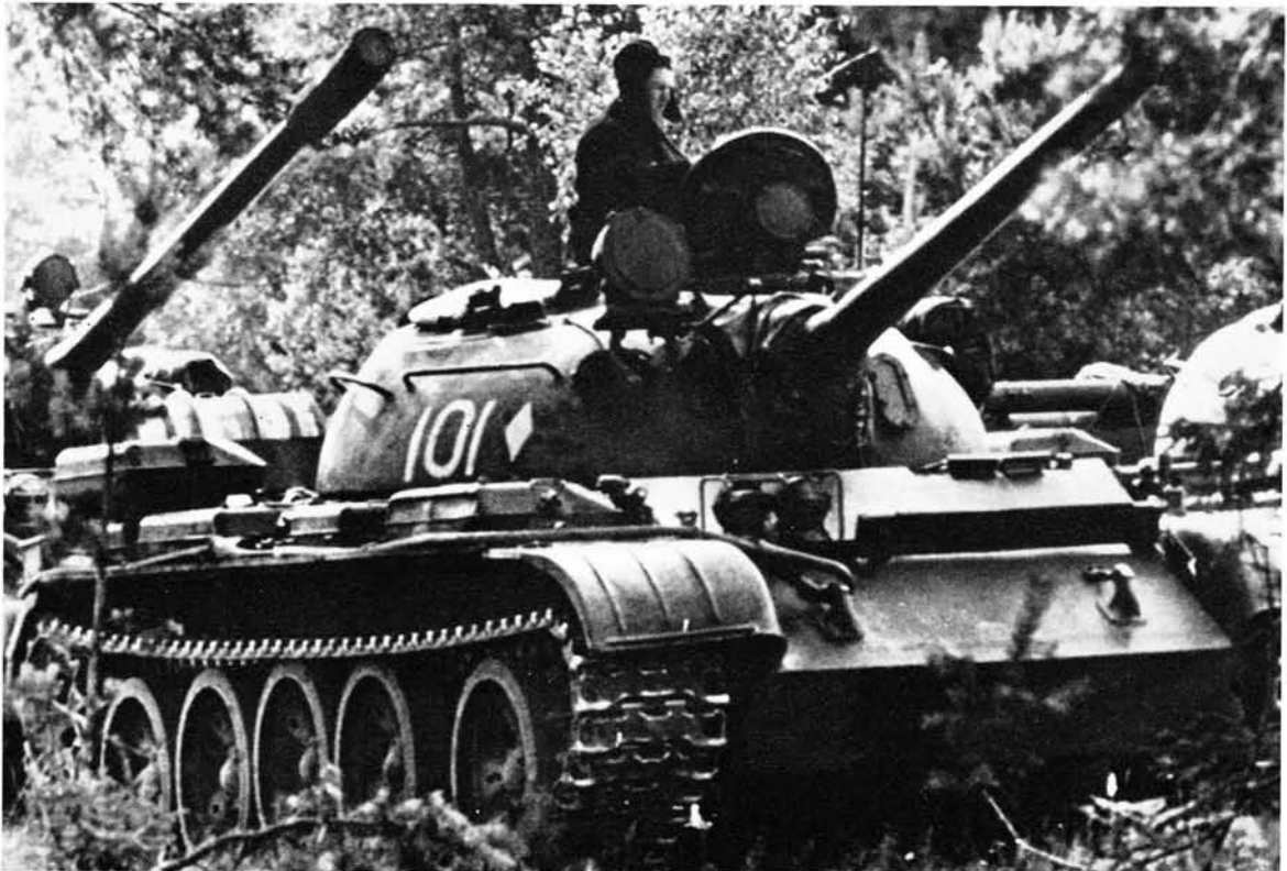
A T-55, successor to the T-54 series, on exercise prior to the invasion of Czechoslovakia in 1968. Note the absence of the loader's cupola with its AAMG. (Photo: dpa)
