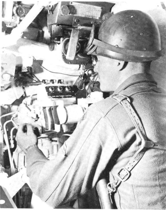
The gunner in the M48A3 has his controls compactly arranged. Photo—U.S. Army
