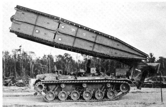
The M60 AVLB like its M48 predecessor was a conventional type of scissors bridgelayer.
