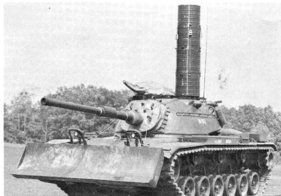
An M60A1 tank equipped with dozer blade and snorkel indicating a maximum depth of 17 feet which could be forded.
