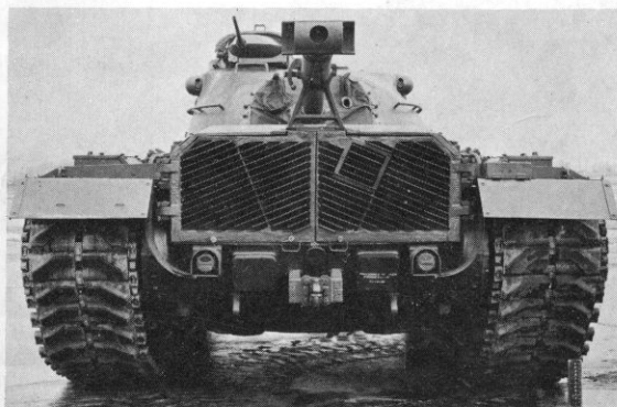
The rear view of the M48A2 shows the major redesign of the engine compartment, new louvers, travel lock, pintle and inside telephone box of changed design. Photo—U.S. Ordnance Corps.
