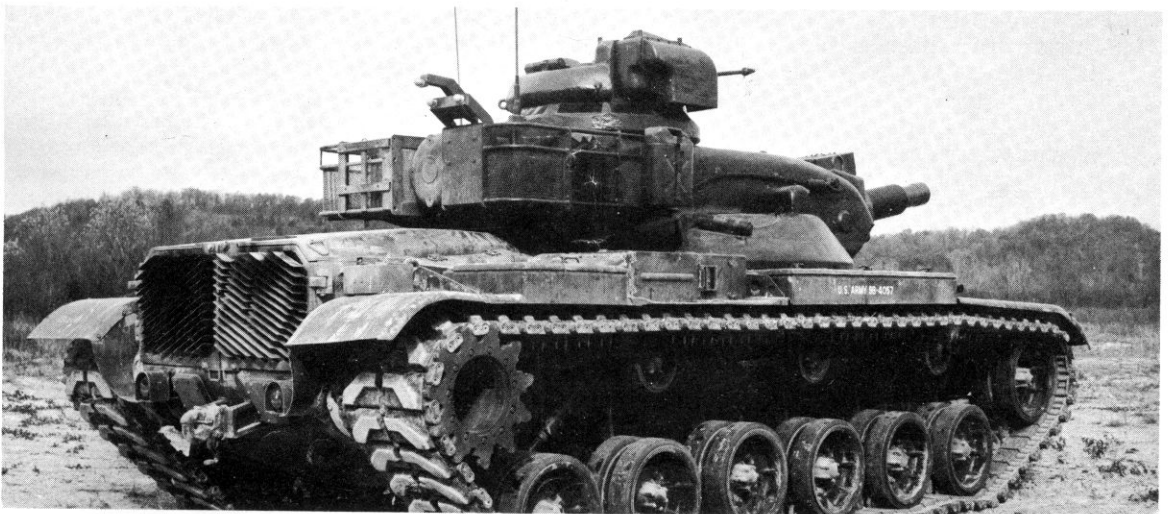
This three-quarter rear view of the M60A1E2 shows the vision riser below the cupola and the unusual turret bustle. Photo—U.S. Army
