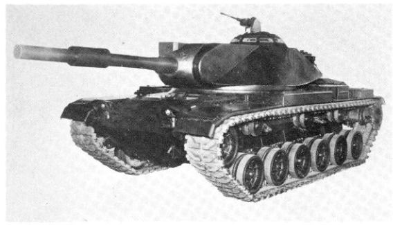
Project K, the redesigned M60A1 with longer Shillelegh mounted in a new armor plate turret of improved ballistic design. Photo—Courtesy Defense Operations Division Chrysler Corporation.
