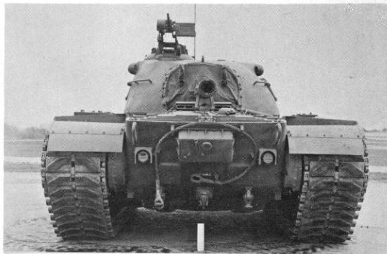
The production T48 with gun secured in the travel lock and turret to the rear, showing blackout lights and telephone box.
