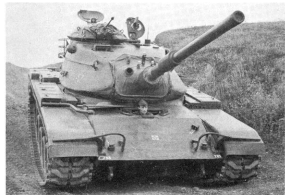
The M60A1 as used in Austria shows the change made in the glacis and the simplified supports for the fenders.
