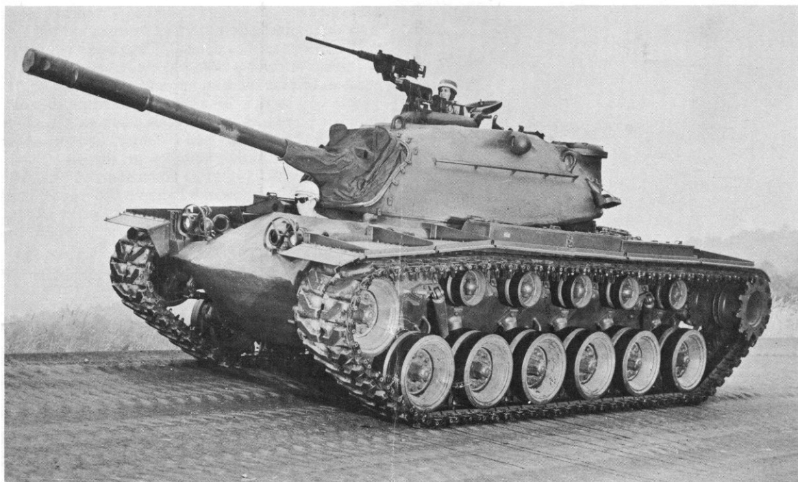
T 48 Prototype with original cupola and A/A machine-gun and with original 90-mm. gun, showing details of suspension. Photo:—Courtesy Chrysler Corporation
