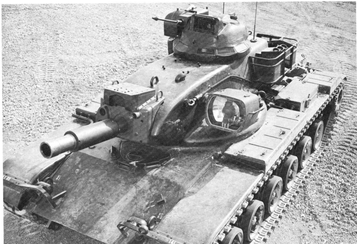
M60A1E2 main battle tank—vision devices are provided for all crew members.
