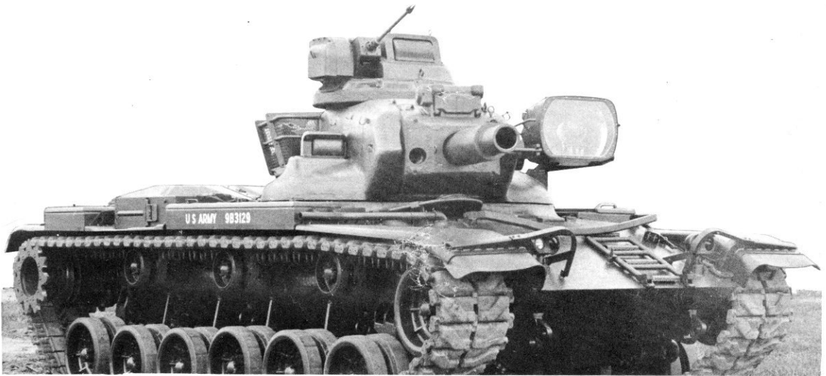
Three-quarter front view of the M60A1E1 shows the unusual turret design, the gun depression limit bar and the crew ladder on the left glacis. Photo—U.S. Army
