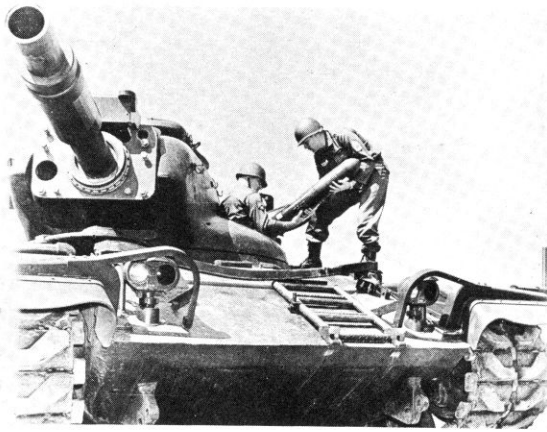
Loading Shilleagh projectile through loader's hatch in the M60A1E1 medium tank. Photo—U.S. Army
