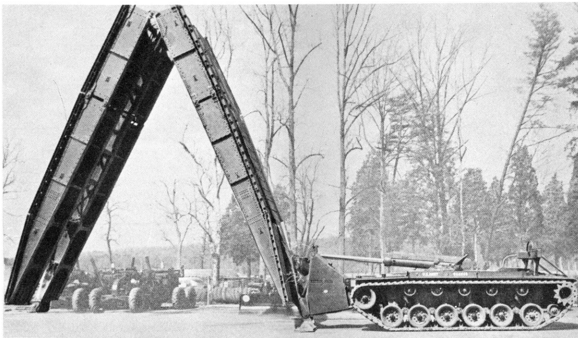
The AVLB scissors type bridging vehicle increased the operating range of its companion M48 and M60 main battle tanks.
