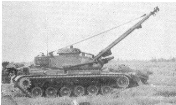
The T118E1 Armoured Engineer Vehicle was a general purpose vehicle armed with a 165-mm. assault gun. Photo: Courtesy J. W. Loop
