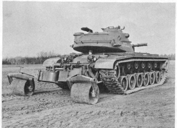
Expendable roller mine clearing device developed for use with standard M48 tanks.
