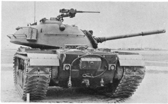
Rear view of the T48 with turret transversed to the right. In this view the engine compartment louvers and exhausts are clearly visible.
