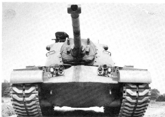
The flame gun on the M67 flame tank was a close replica of the 90-mm. gun on the standard tank. Photo—Chemical Warfare Service
