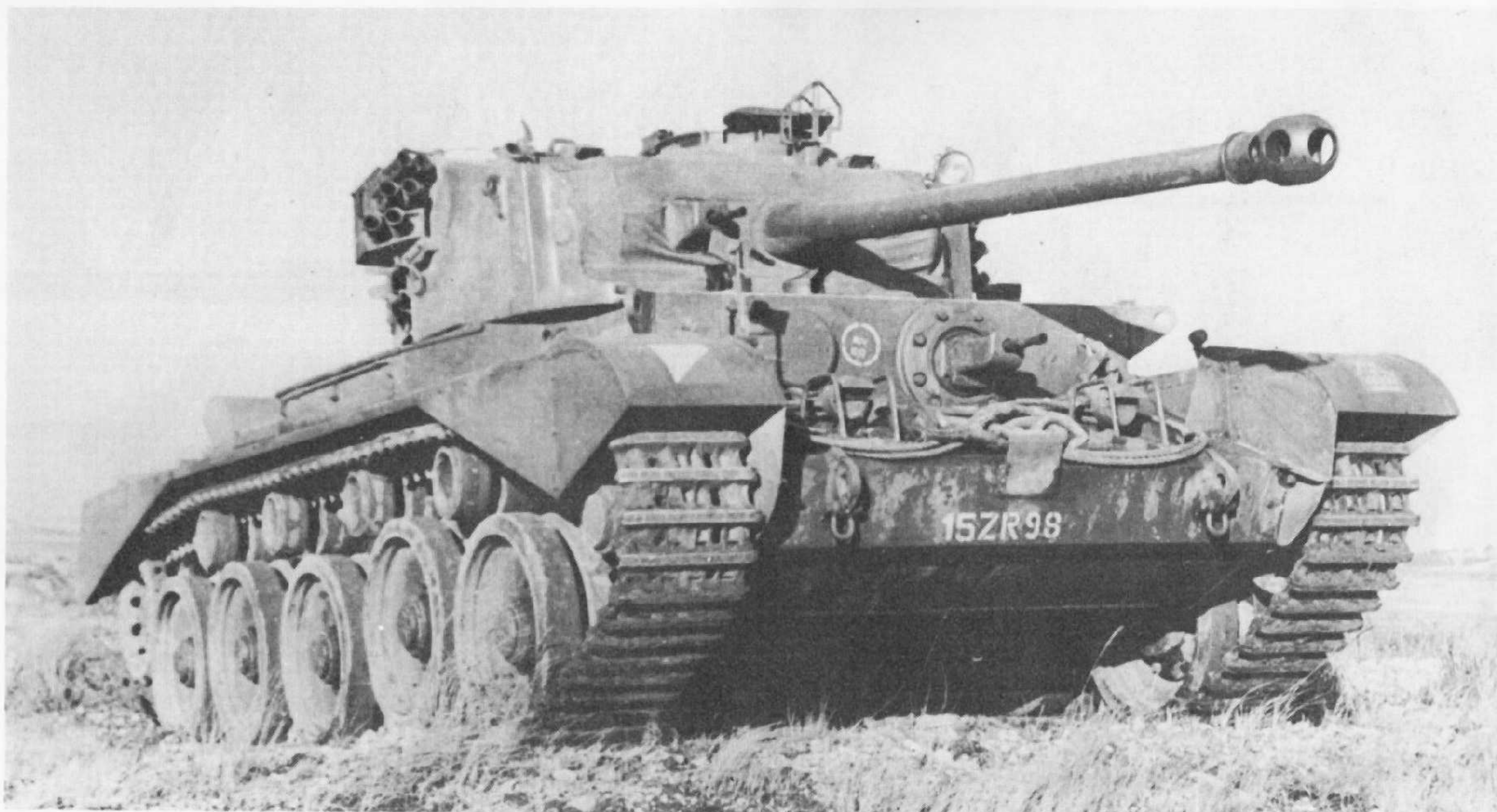
Multi-barrel smoke dischargers were fitted after the War, as on other armoured vehicles, arranged in three pairs on each side of the turret. This Comet tank has been renumbered in the new system. (Photo: R.A.C. Tank Museum)
