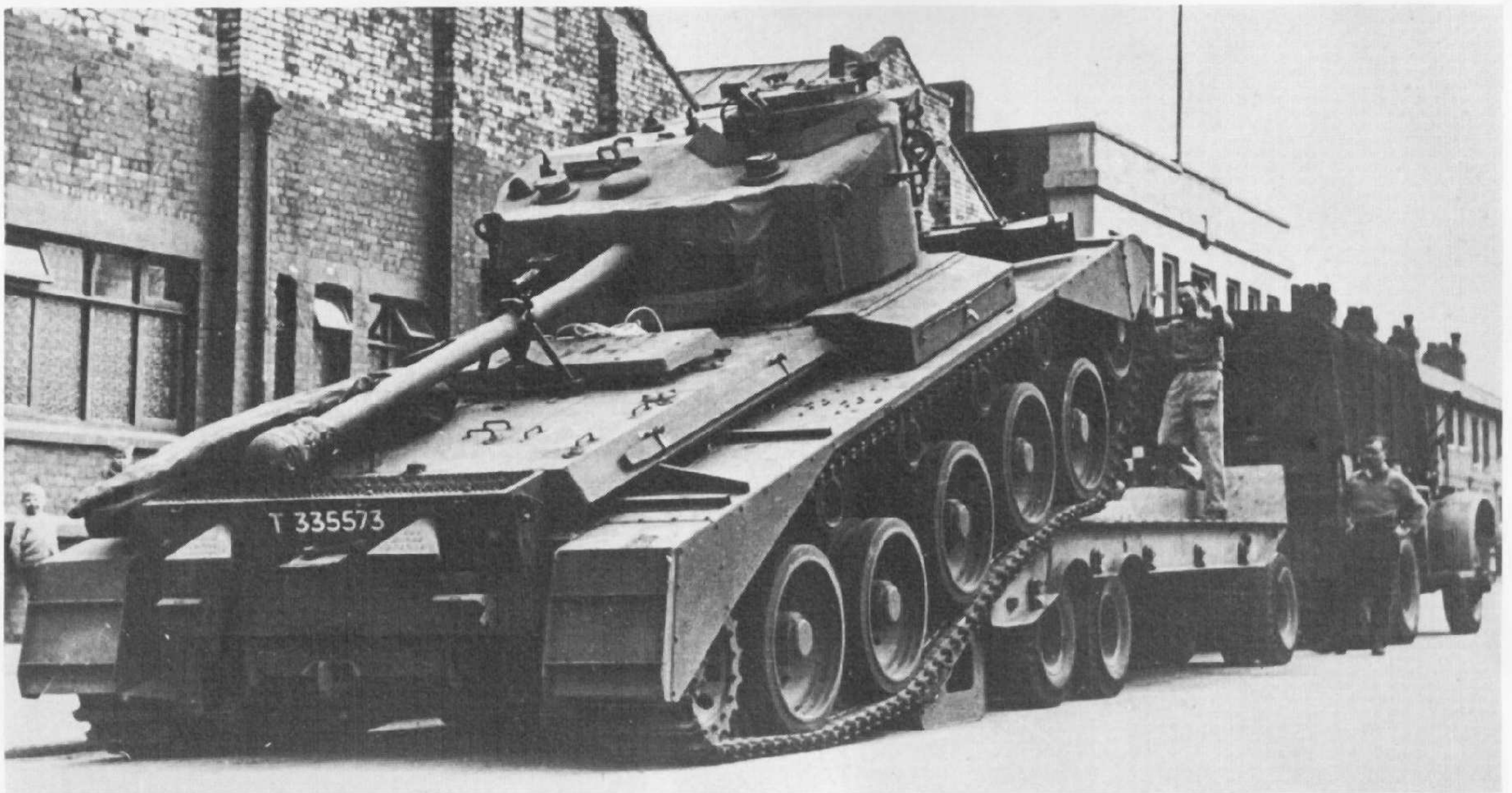
Above: Leading on to a transporter, a Comet Type B clearly shows the fittings on the engine deck and the turret top, including the armoured deflector shield in front of the commander's cupola. (Photo: R.A.C. Tank Museum)
