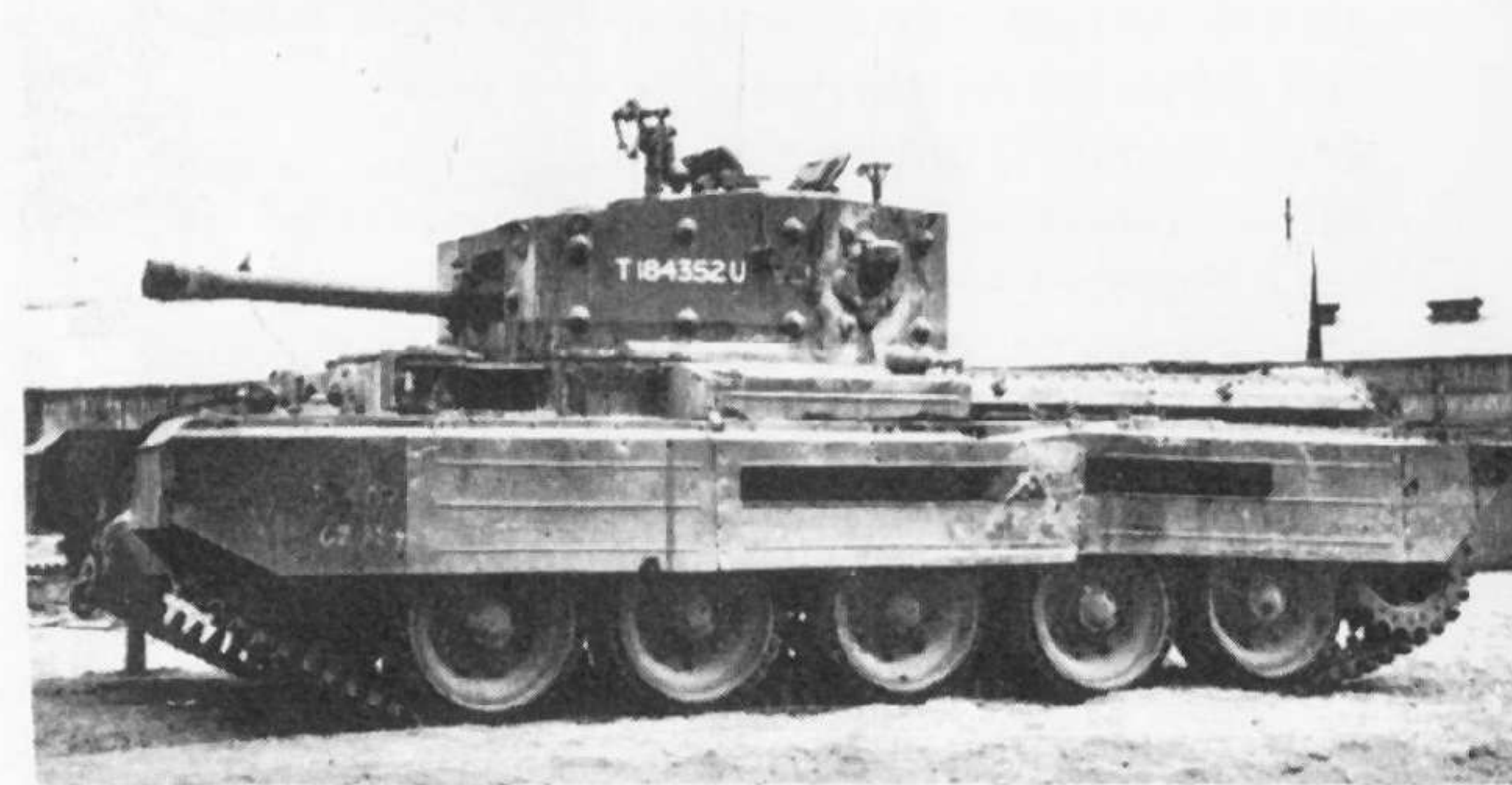
Cromwell III D—sub-mark indicated by hull gunner's side opening hatch. This vehicle was fitted with track sand shields for Middle East trials. (Photo: Imperial War Museum)
