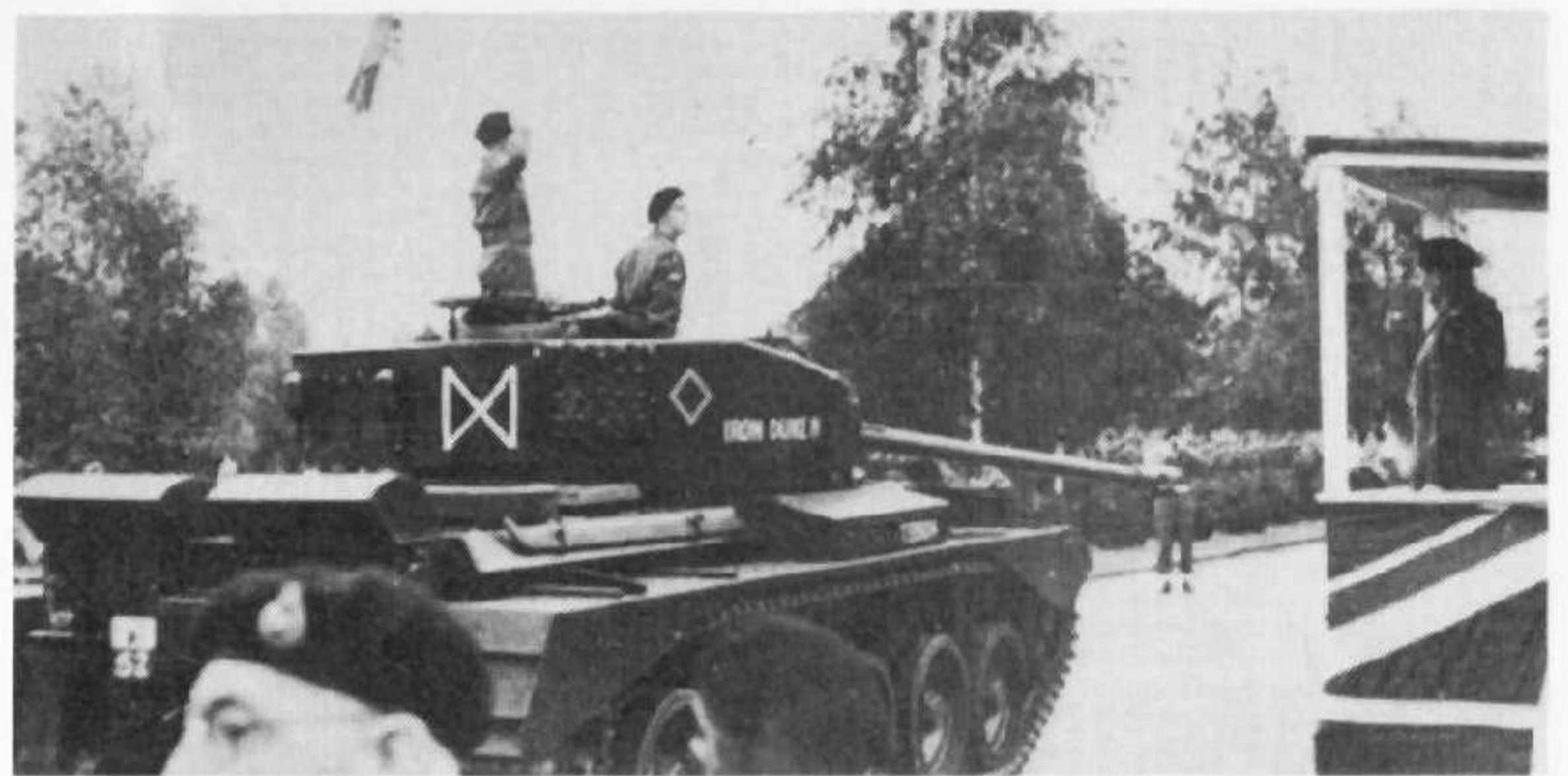
Above: Leading on to a transporter, a Comet Type B clearly shows the fittings on the engine deck and the turret top, including the armoured deflector shield in front of the commander's cupola. (Photo: R.A.C. Tank Museum)
