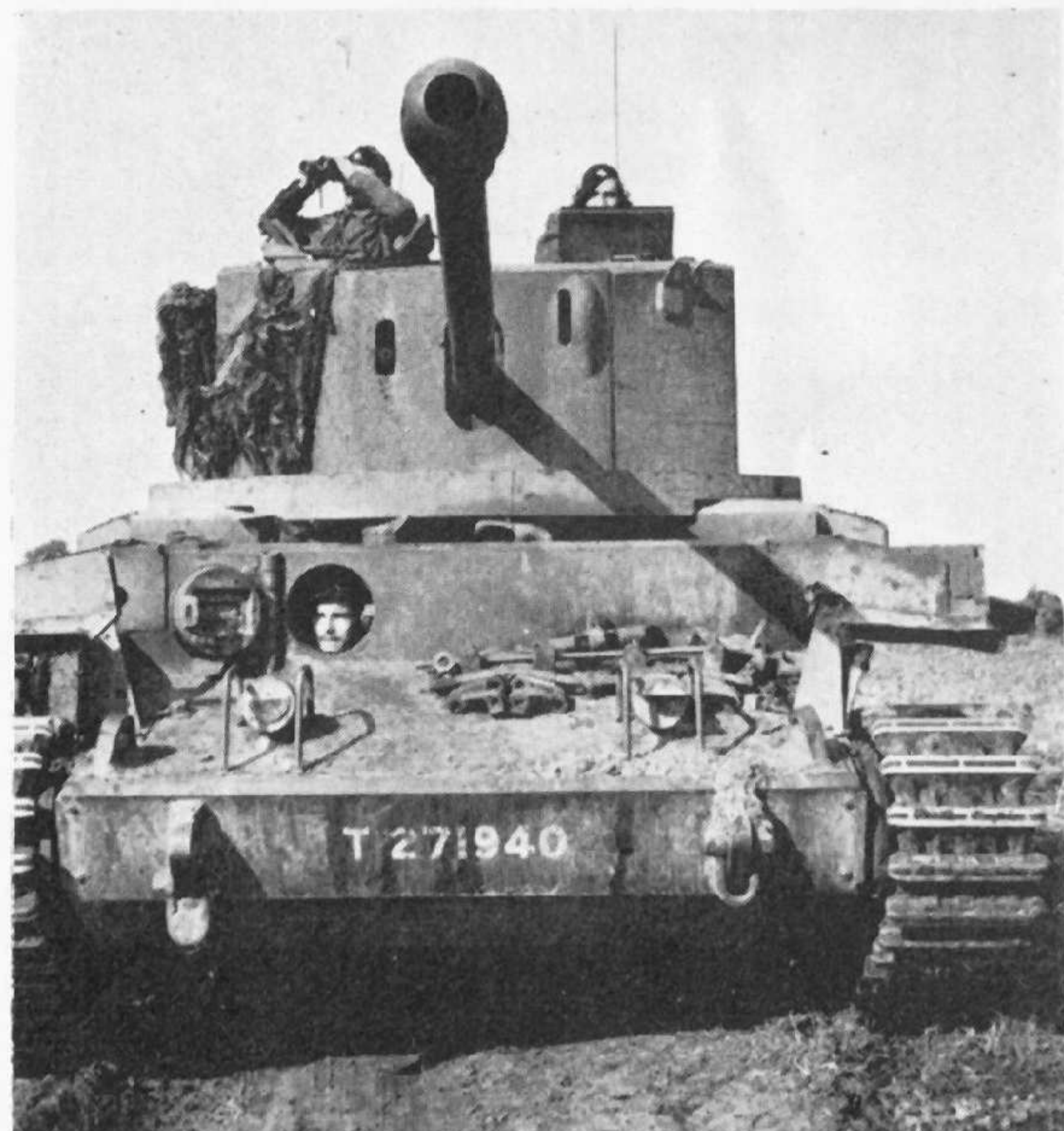
A.30 Challenger Tank Destroyer mounted the 17-pdr. (76.2-mm.) gun on a lengthened Cromwell chassis.
