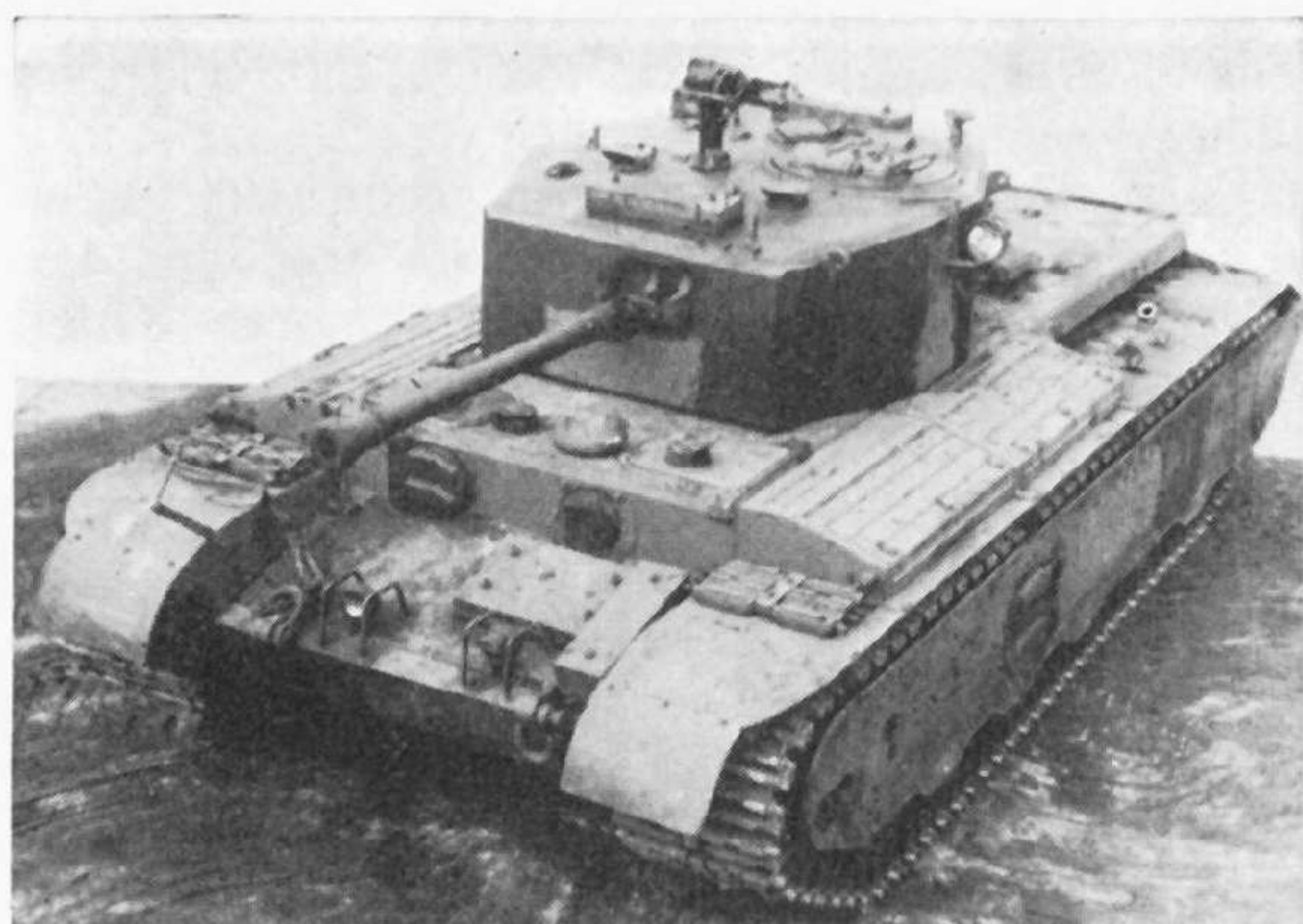
A.33(1) Assault Tank—this version used the U.S. T.1 track. (Photo: Imperial War Museum)
