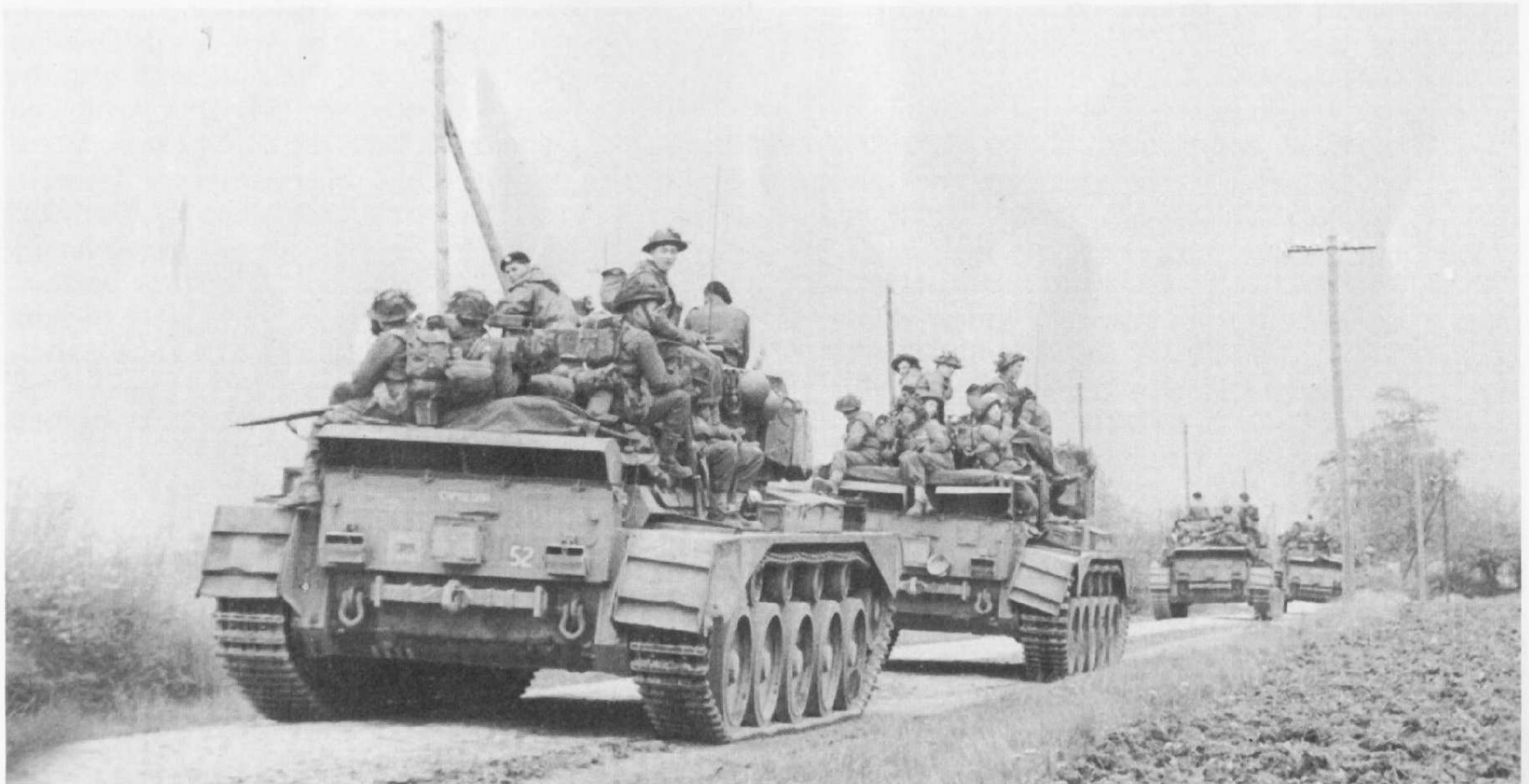
Soldiers of the 1st Bn. Herefordshire Regiment being carried forward on Comets of the 3rd Royal Tank Regiment. The nearest tank has the Cromwell exhaust cowl, with no space in the centre for the gun when in the travelling position in the gun crutch. (Photo: Imperial War Museum)
