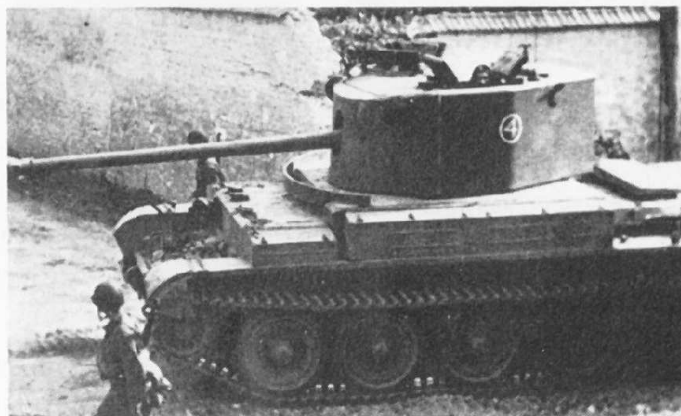
Above left and right: A.30 Challenger Tank Destroyer mounted the 17-pdr. (76.2-mm.) gun on a lengthened Cromwell chassis. Note six road wheels and characteristic high turret.
