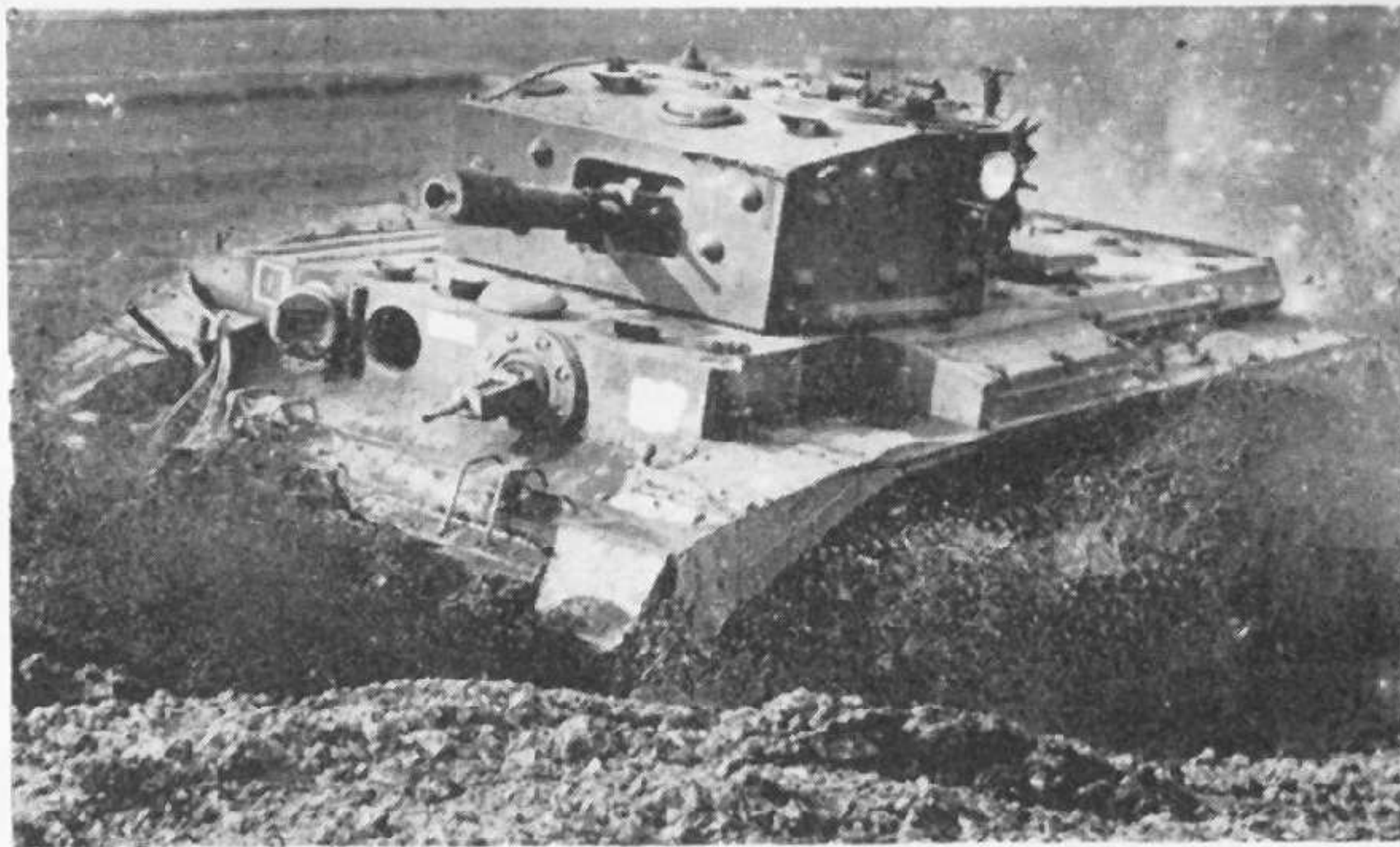
Cromwell VI 95-mm. howitzer close support tank. Cromwell VIII was similar but with additional armour on hull front and wider tracks.
