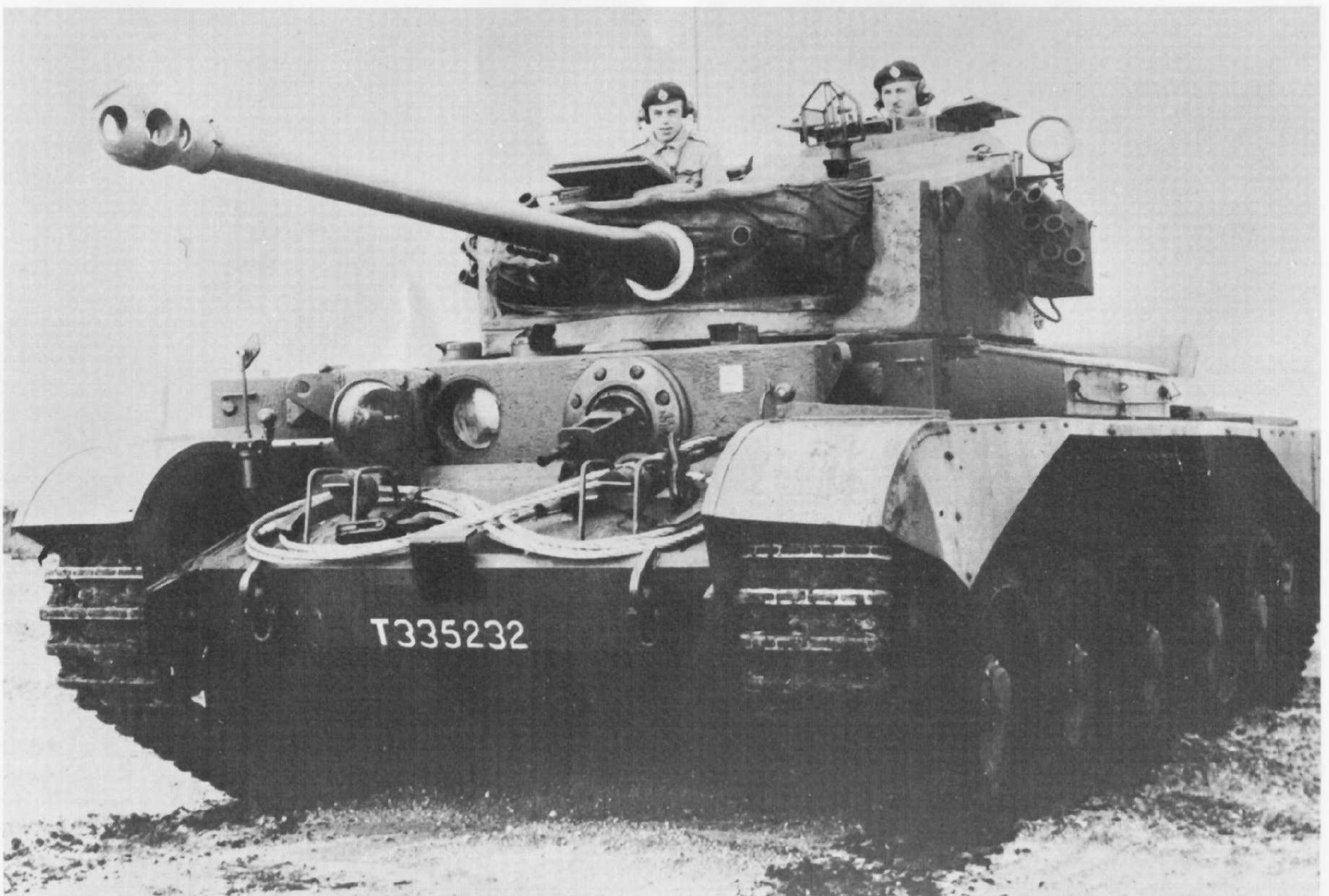
Below: A post-war Comet Type A—with exhaust cowl—showing clearly the blade vane sight on the turret roof for the commander. Also shown is the protection piece welded on to the glacis plate to protect the join with the vertical front plate. (Photo: R.A.C. Tank Museum)
