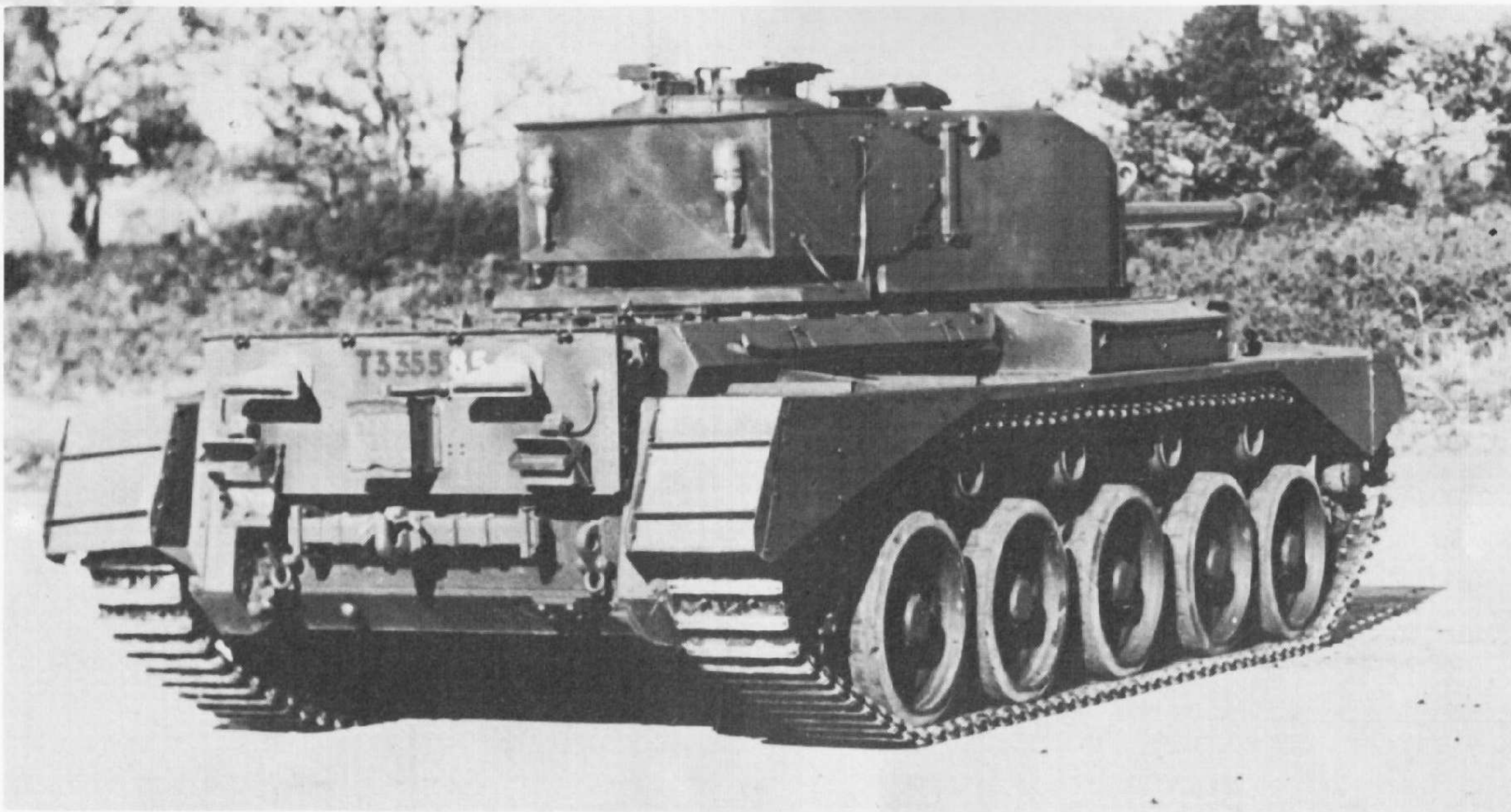
The Comet Type B, in which the exhaust pipes have been led to twin armoured fishtails mounted on the rear armoured plate. Note that the top of the armoured plate has been raised to the level of the engine deck. (Photo: R.A.C. Tank Museum)
