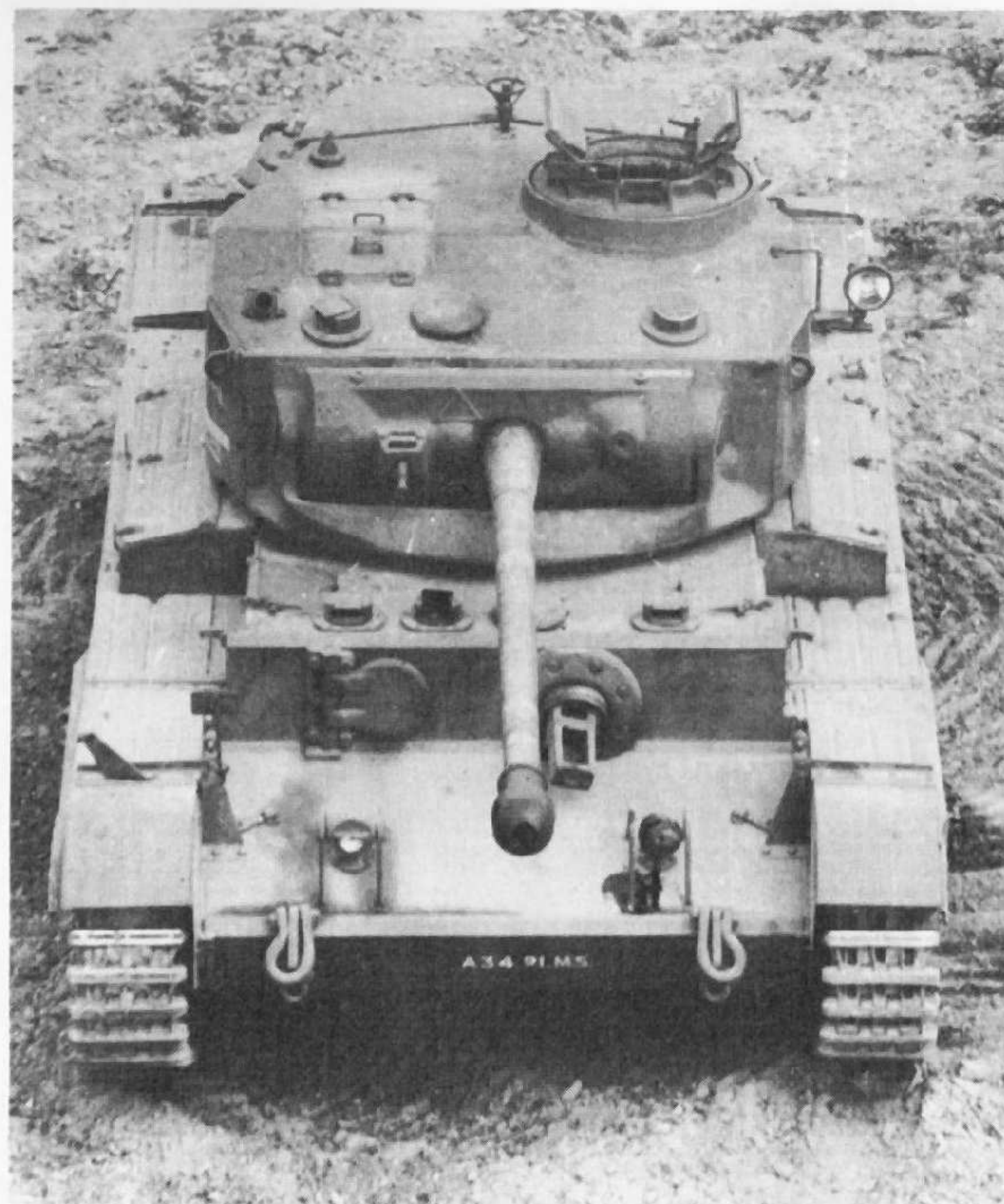
Above: The first A34 Prototype, in mild steel. Side-opening roof doors for both driver and front gunner were fitted on all Comets, as on the later types of Cromwell. This meant that both could get out, whatever the position of the turret.
