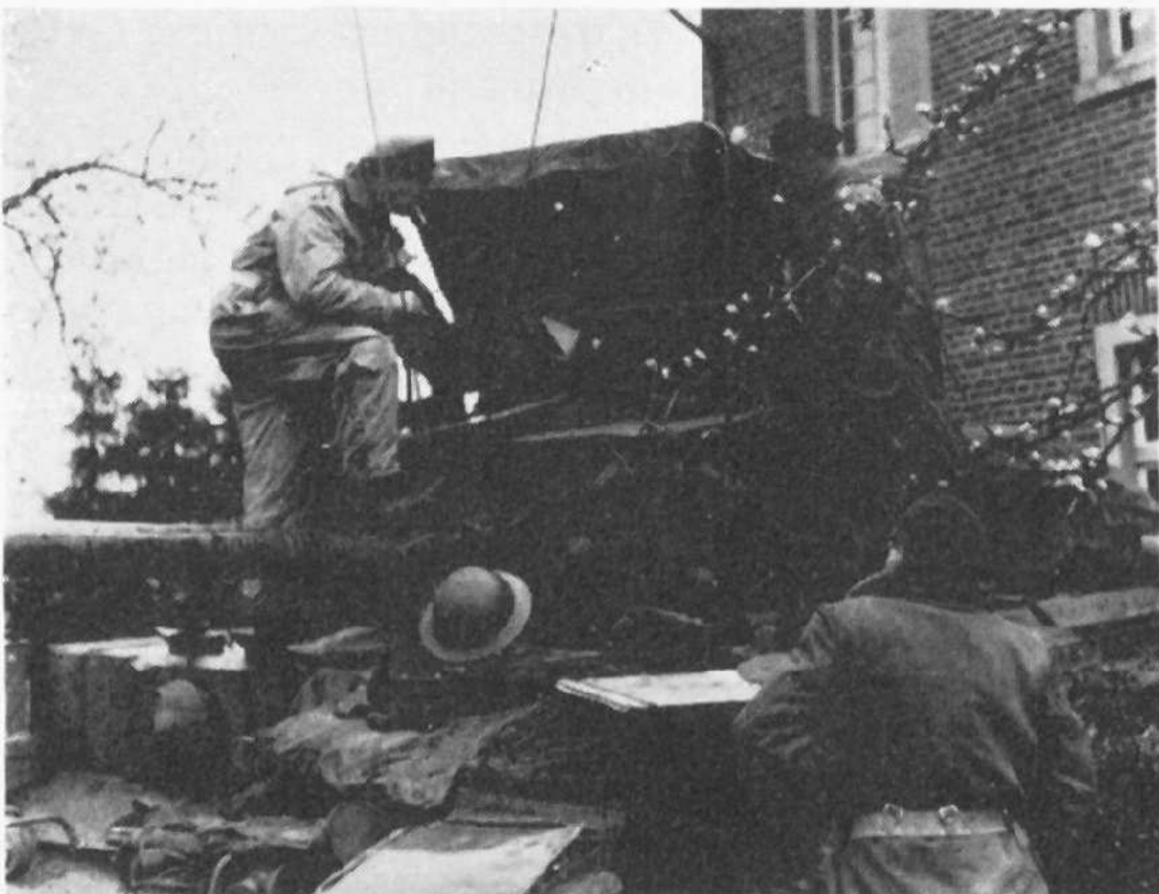
Cromwell IV adapted as Brigade HQ tank. The vehicle carries additional aerials, collapsible hood and brackets for mounting map boards.
