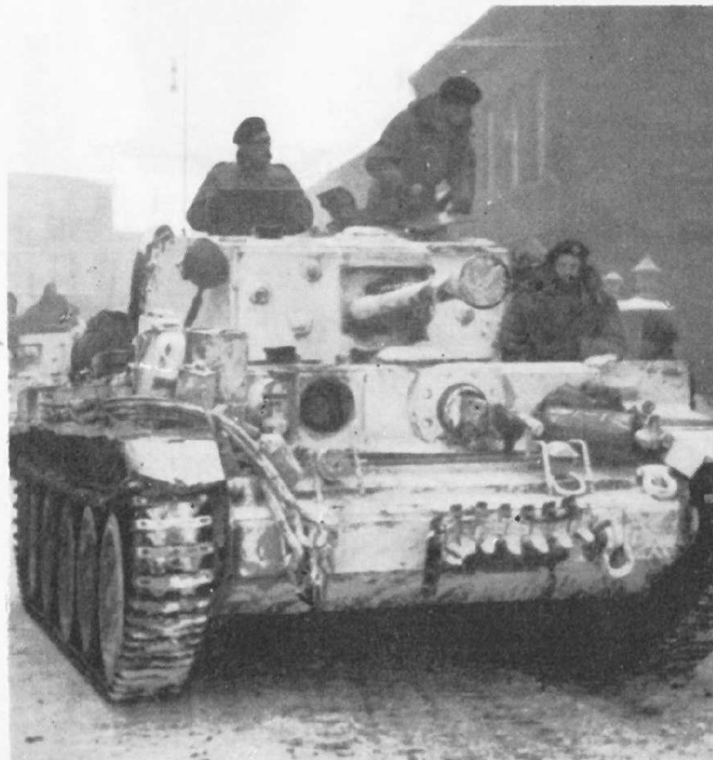
Snow camouflage—used for the first time by British armour—assists identification of additional armour plates welded on nose and hull front which characterize this Mk. VII photographed near Sittard, Holland, January 16, 1945.
