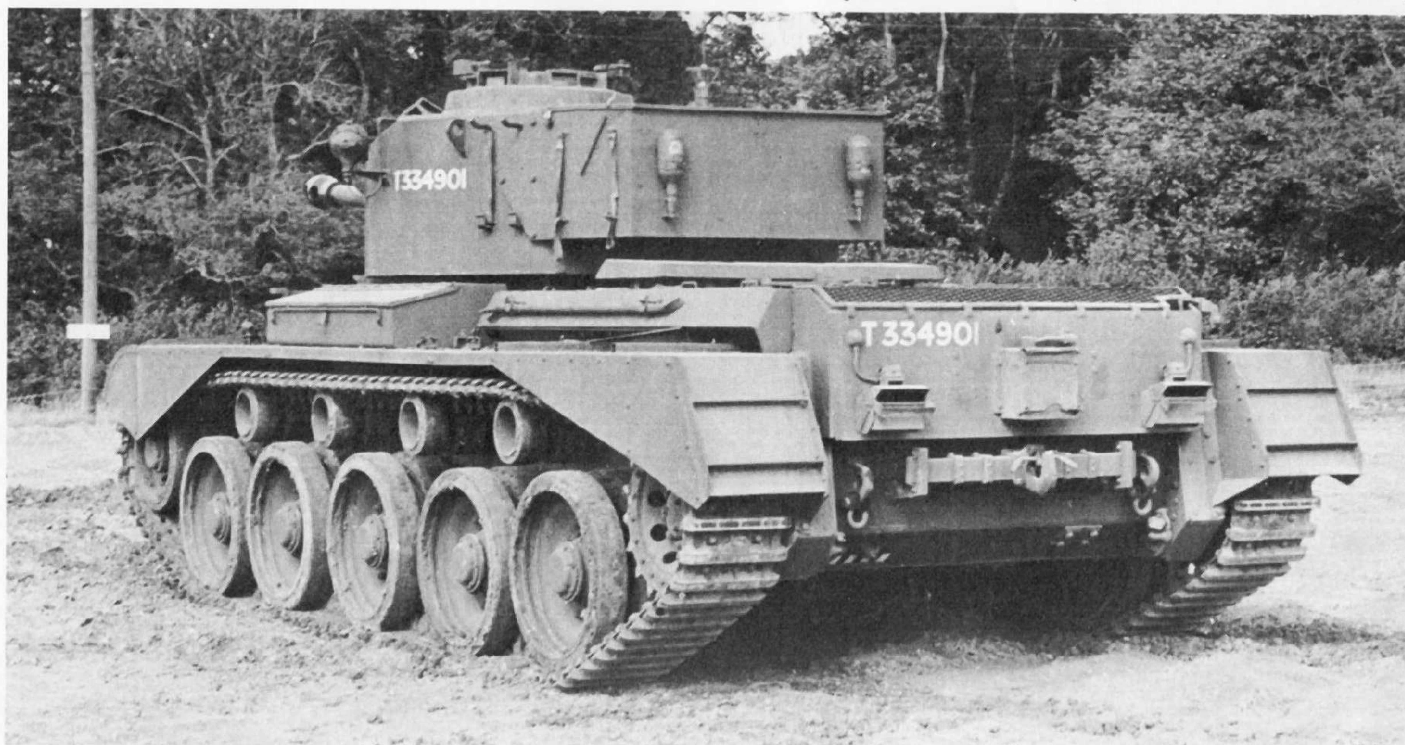
Below: Rear of the Comet Type A, which retained the Cromwell exhaust system. A cowl was normally fitted over the back end for concealment and protection against exhaust flames projected upwards. Note the addition of the 17-pdr. tow bar, which has caused the two smoke dischargers to be moved up on to the rear armoured plate.
