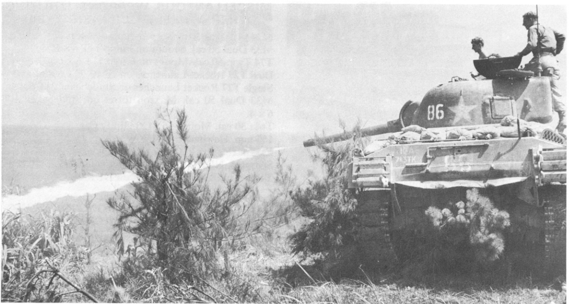
POA-CWS 75H-1 flamethrower tank, one of several varieties built in Hawaii for island operations.
