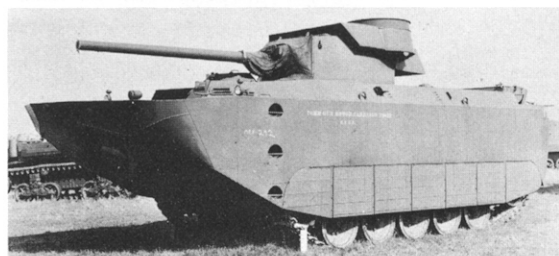
The T86E1 amphibious gun motor carriage created from the M18 by the National Defense Research Council. Photo—Courtesy C. J. Nuttall
