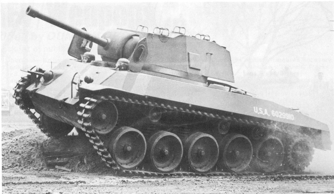
The T49 high speed gun motor carriage with 57-mm. gun and bow machine-gun had coil spring suspension.
