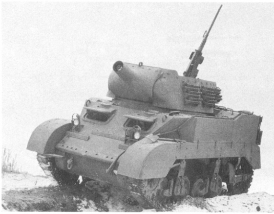
M8 howitzer motor carriage based on M5A1 light tank chassis. Photo—Cadillac Motor Car Division, General Motors Corporation
