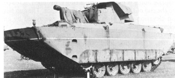
The T87 amphibious howitzer motor carriage carried the heavier 105-mm. howitzer but was lighter than the T86. Photo—Courtesy G. B. Jarrett
