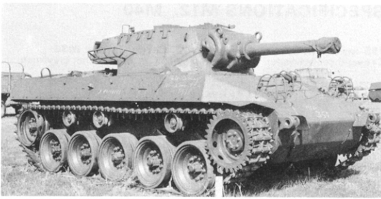
The T88 gun motor carriage was an experimental M18 carrying a 105-mm. Howitzer. Photo—U.S. Ordnance Dept.
