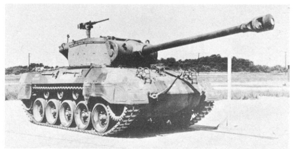
No "T" number was assigned to the informal experimental mounting of the M36 turret and gun on an M18 chassis. Photo—U.S. Ordnance Dept.
