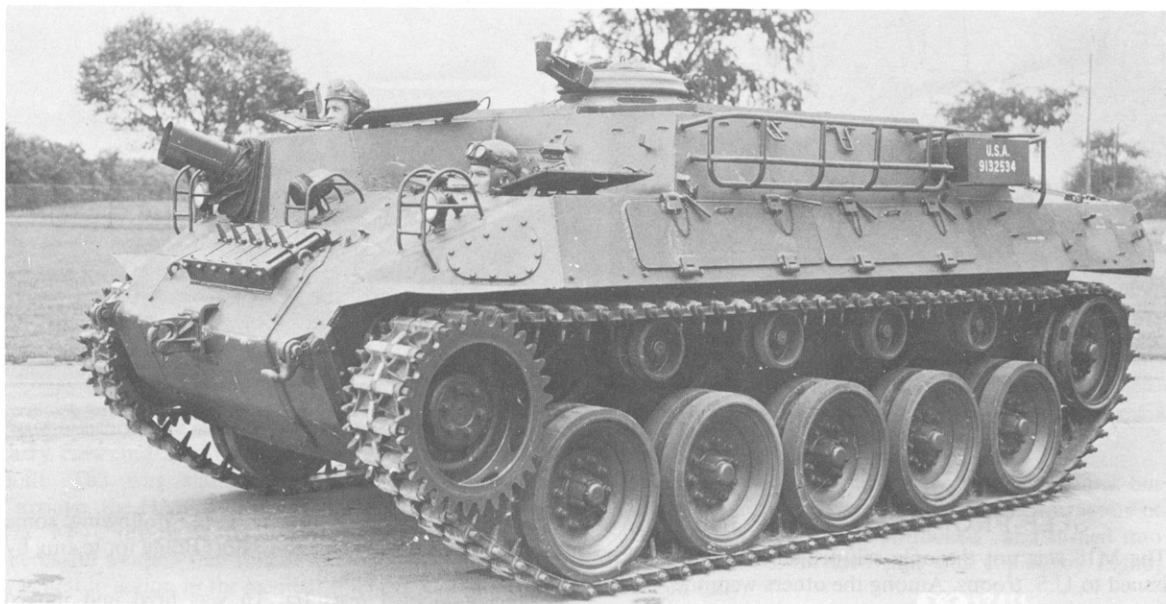
The T65 flame tank was a modified M18 with commander's cupola replacing turret and the hull modified to mount an Iroquois flame gun.
