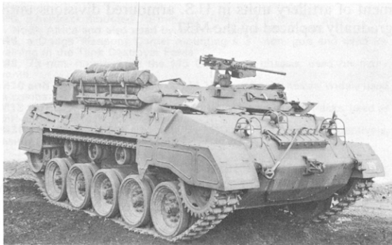
The M39 armoured utility vehicle was used as an armoured personnel carrier and as a command vehicle. Photo—U.S. Ordnance Dept.
