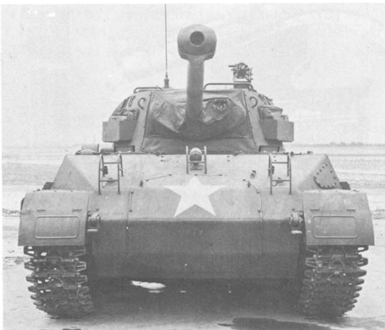
M18 gun motor carriage showing armor bevels and model equipped with gun with muzzle brake and T85E1 tracks. Photo—U.S. Ordnance Dept.
