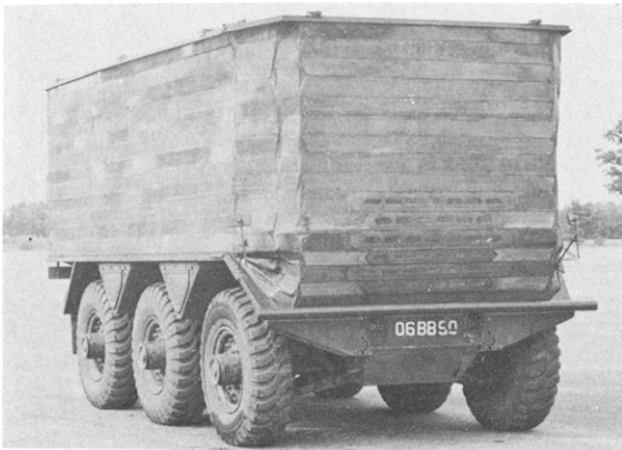
"Swimming" Saladin with rubberised screen raised. (Alvis Ltd.)
