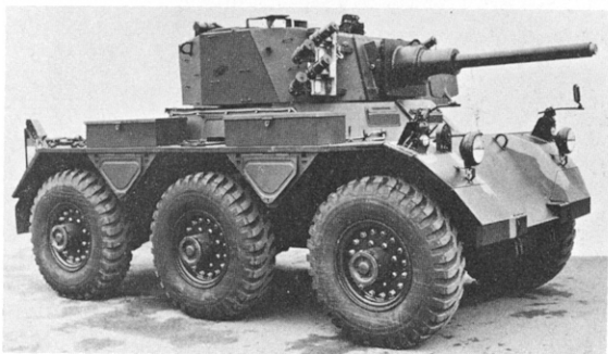
The FV 601(D) variant. Note the German smoke grenade dischargers among other detailed changes. (Alvis Ltd.)
