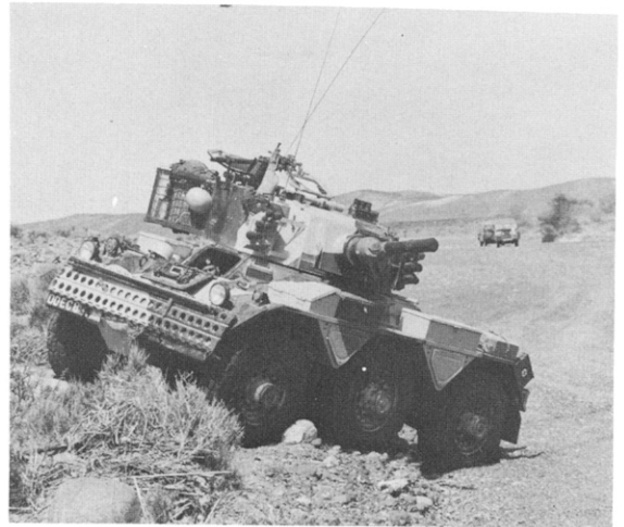
Saladin of 3rd Royal Tank Regiment leaves a desert track to cross rough terrain during a training exercise in Eastern Arabia. Sand channels are stowed on the glacis plate. (CCR BIS)
