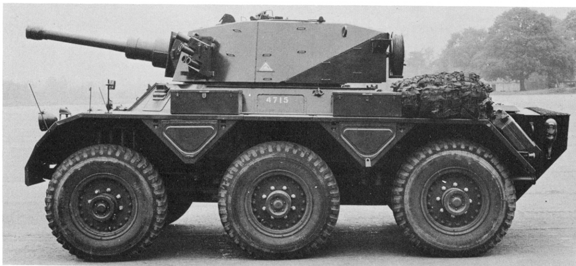
Side view of the first pre-production version of FV 601(B) (Saladin Mark I). The triangular plate on the turret warns that the vehicle is not built of armoured plate. (CCR MVEE)
