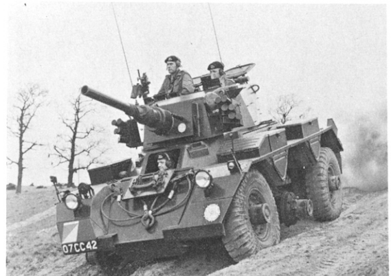
Saladin of The Queen's Own Hussars with its RH front and LH centre wheels removed moving across rough ground to demonstrate how the effect of mines can be minimised. (CCR BIS)
