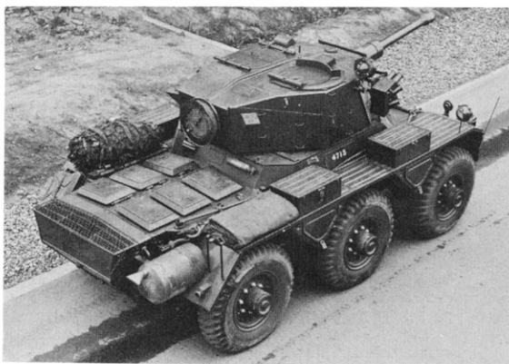
Three-quarter rear view of FV 601(B) showing the tapered and faired rear of the turret, and the periscope in the rear of the fighting compartment hull for driving rearwards in an emergency. (CCR MVEE)
