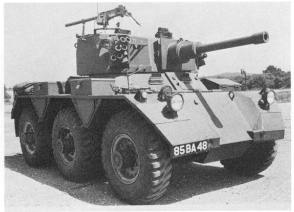
Saladin Mark 2 (FV 601(C)) showing gun barrel with counterbalance collar at muzzle. This feature was not retained in series production. (CCR MVEE)
