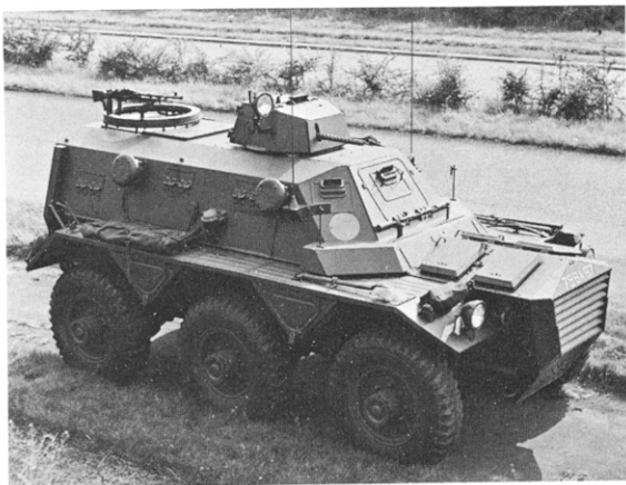
Saracen Armoured Personnel Carrier. The small turret for the commander mounts a 0.30-in. Browning MG. (Alvis Ltd.)
