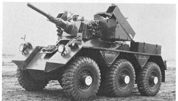
Standard Saladin Mark 2 modified to carry the BAC Swingfire anti-tank GW system. Two missiles are carried in the "ready-to-fire" position on the sides of the turret, and a further two on the rear wheelguards. (Alvis Ltd.)
