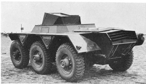
Three-quarter rear view of FV 601 prototype. The earlier grille over the engine has been replaced by six separate and liftable armoured covers. (CCR MVEE)
