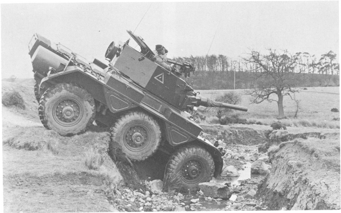
Saladin of The Queen's Own Hussars demonstrates its capability of crossing a deep and wide gully.
