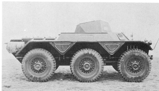
Side view of FV 601 prototype built for automotive trials. (CCR MVEE)
