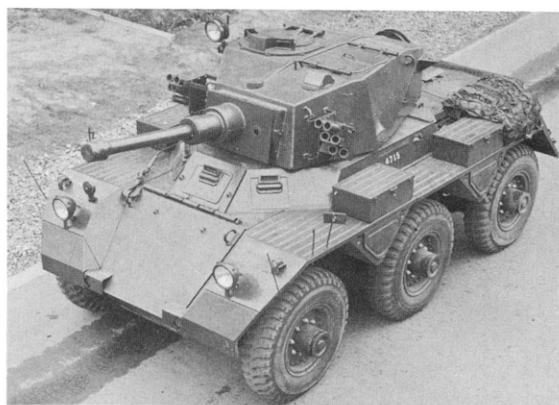
Three-quarter front view of Saladin Mark I (FV 601(B)) showing the original sighting and observation equipment. (CCR MVEE)
