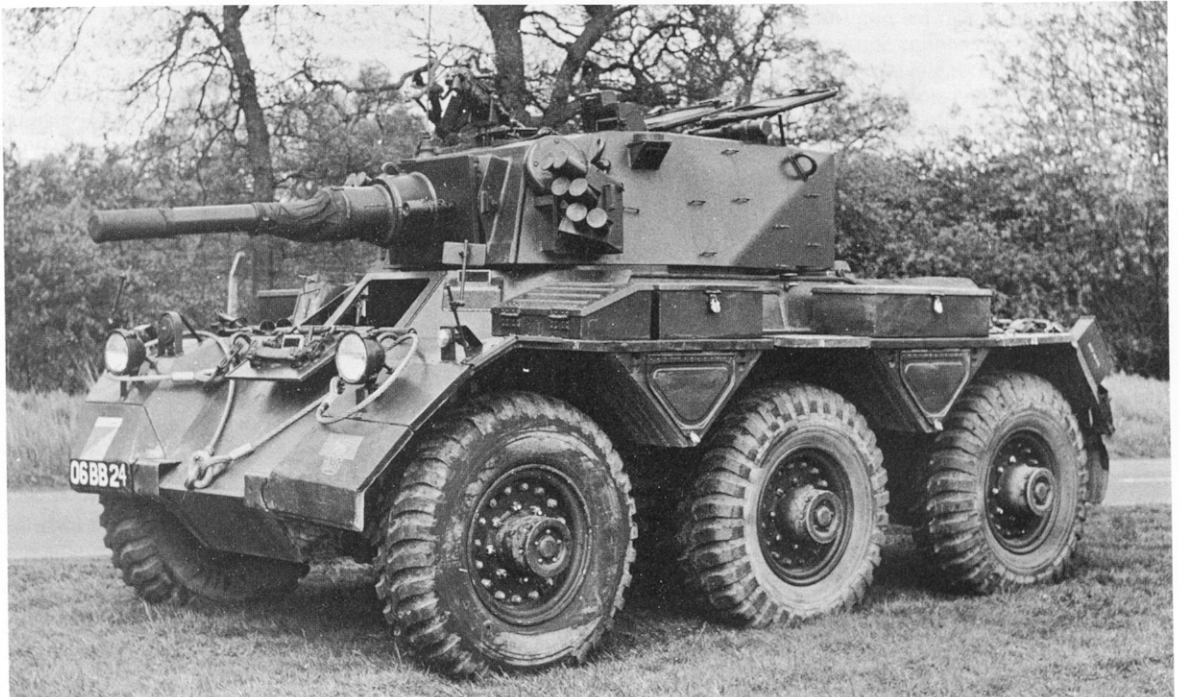
8 to 15 inclusive: Production versions of Saladin Mark 2 (FV 601(C)). Note changes from Mark 1 in turret shape, hatches, and sighting and observation equipment, including disappearance of rear view driving periscope below turret ring. The circular object on the left of the turret adjacent to the smoke grenade dischargers conceals an extractor fan to remove toxic fumes from the coaxial MG. (Alvis Ltd.)
