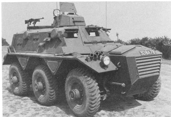
Saracen Armoured Personnel Carrier with various ports and hatches open and smoke grenade dischargers uncovered. (CCR MVEE)
