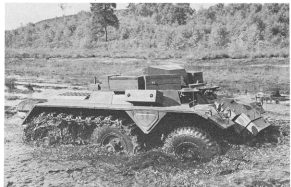
Early FV 601 prototype ballasted to simulate the expected all-up weight of the completed vehicle and with a light track fitted to the rear two pairs of wheels to enhance movement over difficult going. The track was very liable to shedding when steering and the idea was abandoned.
