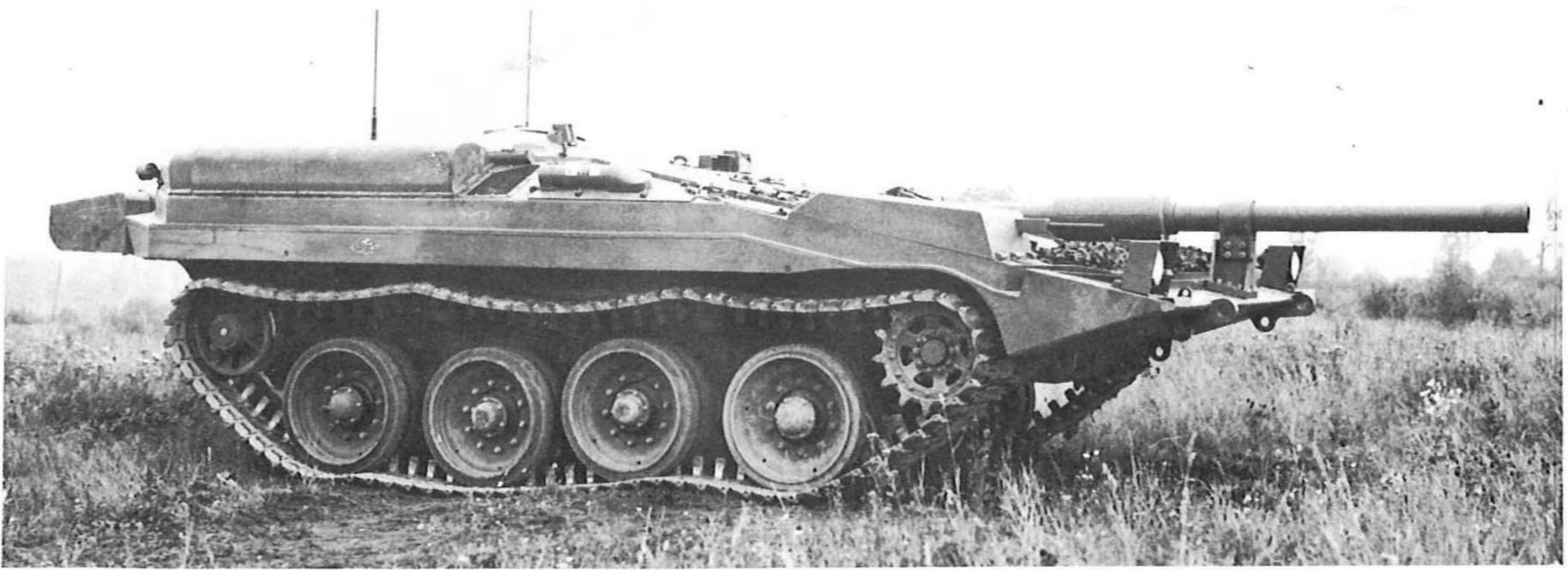
Pre-production version of the S-tank with a 12.7-mm. ranging machine-gun in the right hand machine-gun box.
