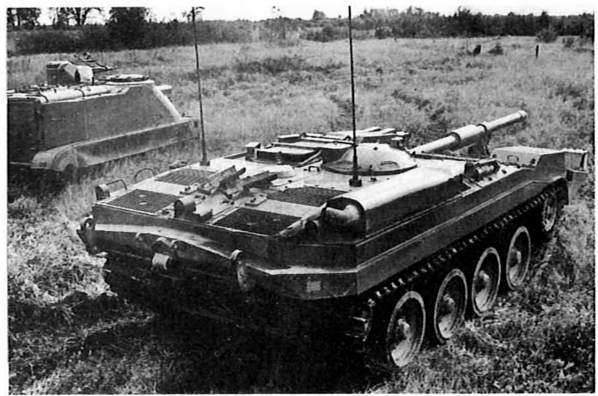
Rear view of an S-tank pre-production model which shows the location of the radiator louvres.
