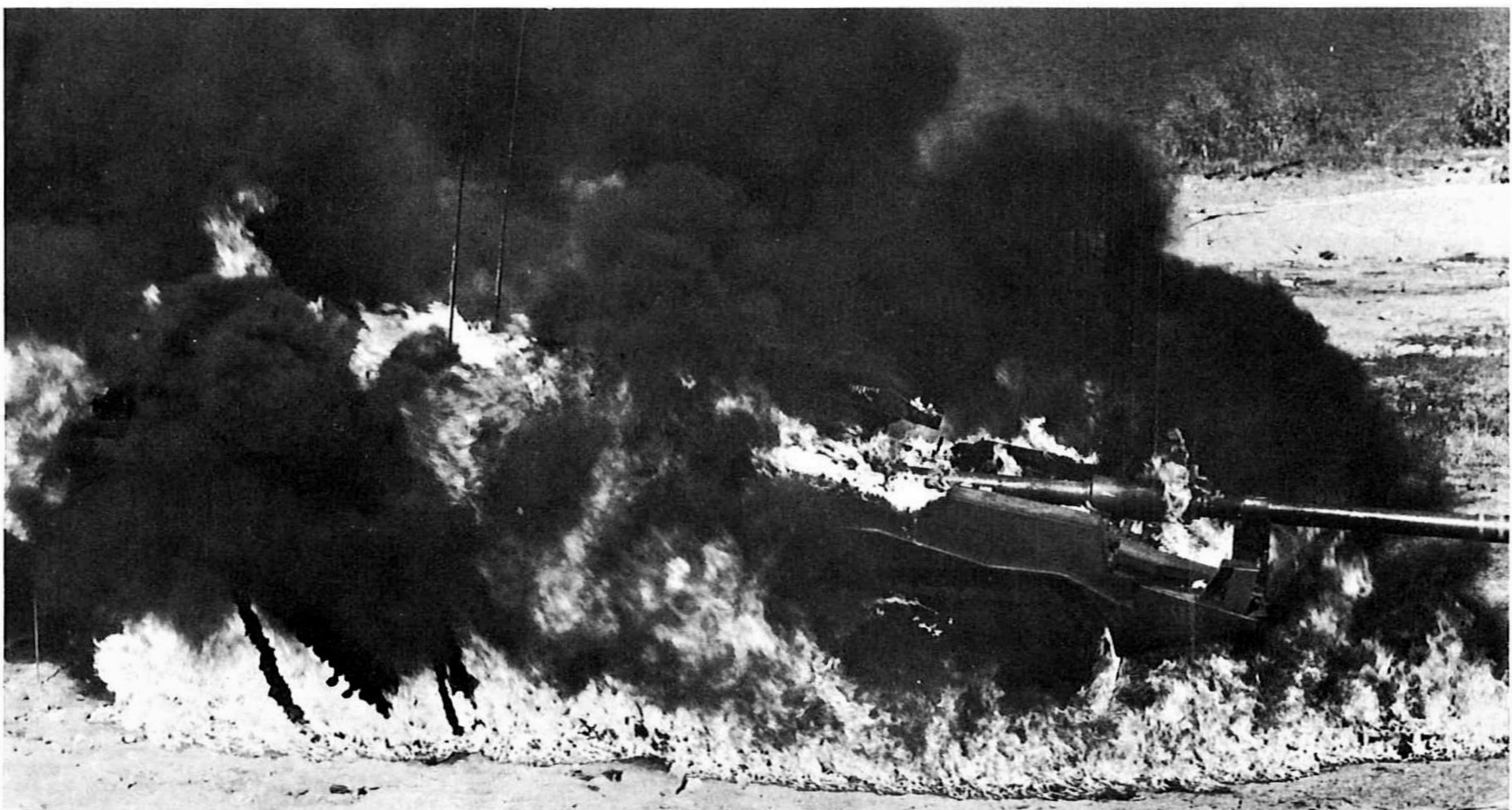
Contents of a napalm bomb burning around an S-tank which only required a few minutes' cleaning of optics to be fit for action again.
