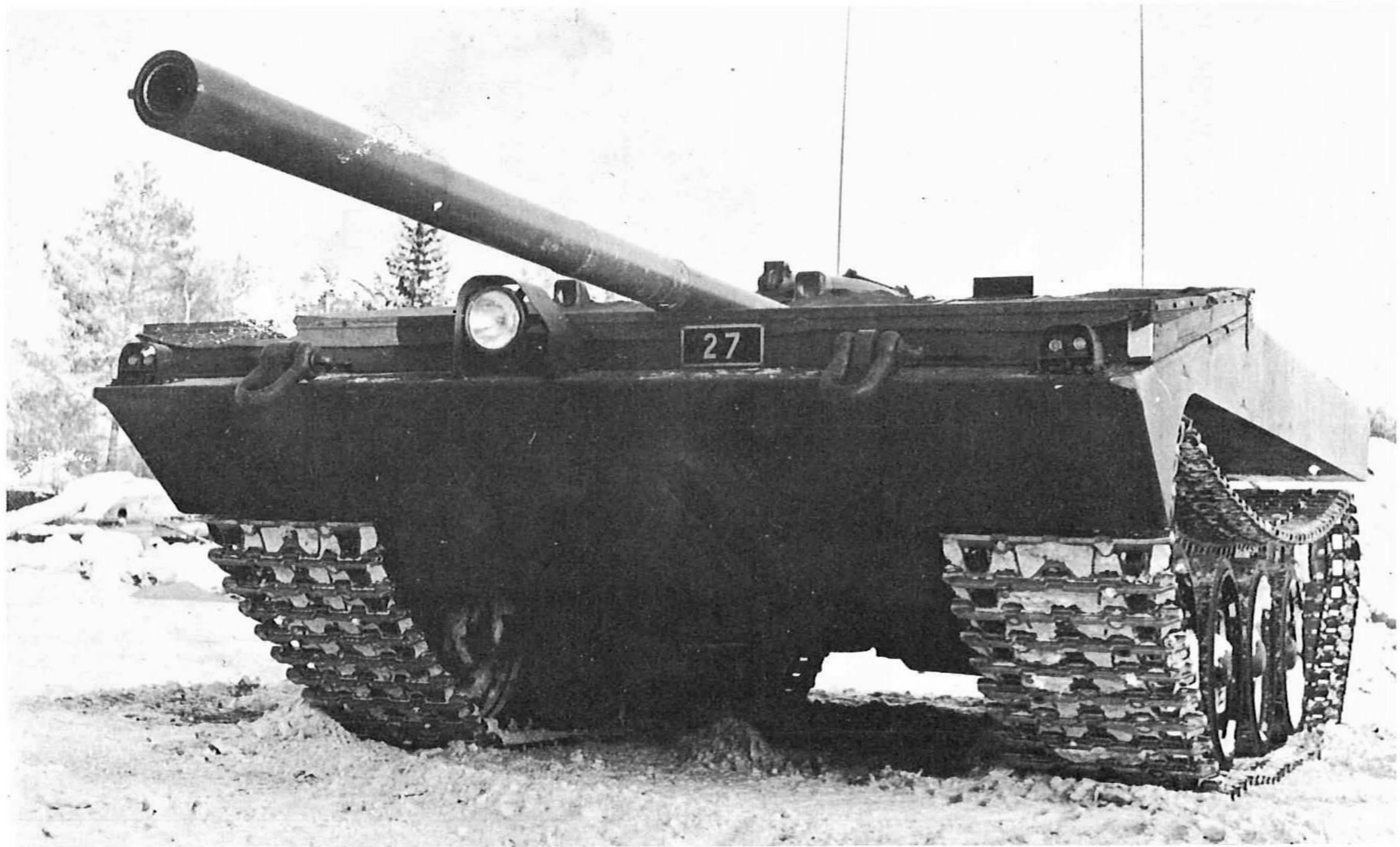
S-tank prototype with the original all-steel track.
