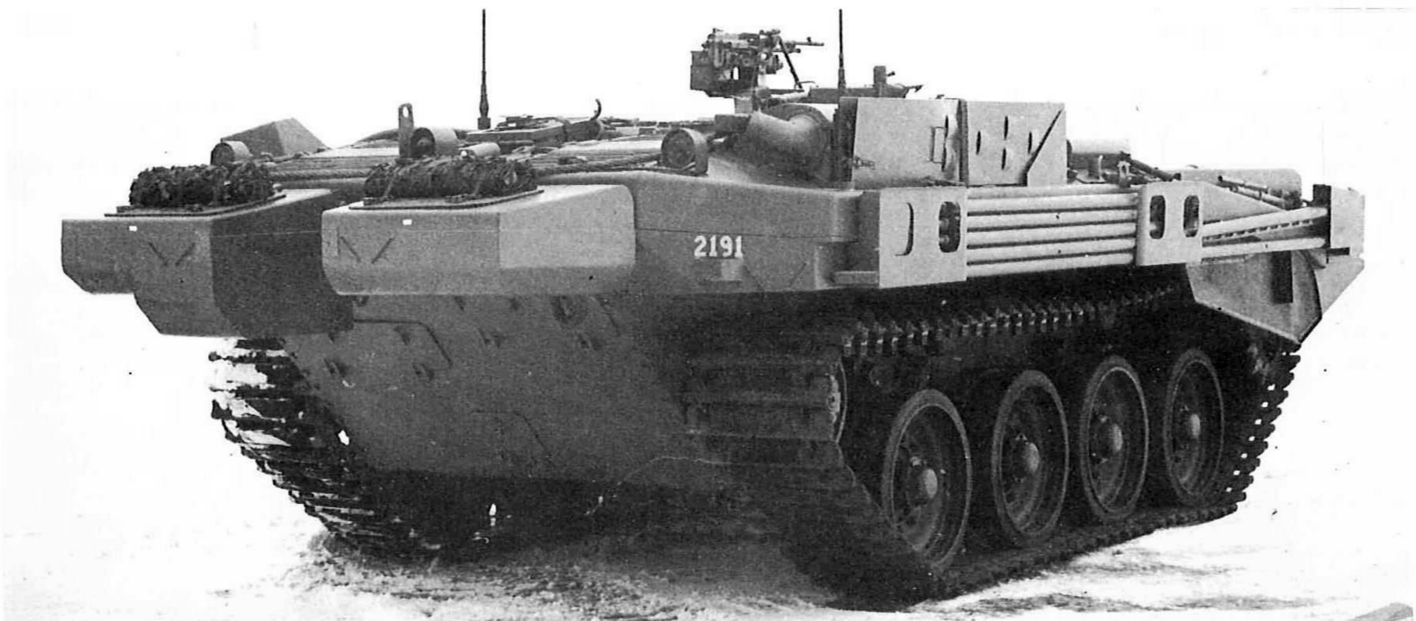
Rear view of an S-tank Type B with flotation equipment.
