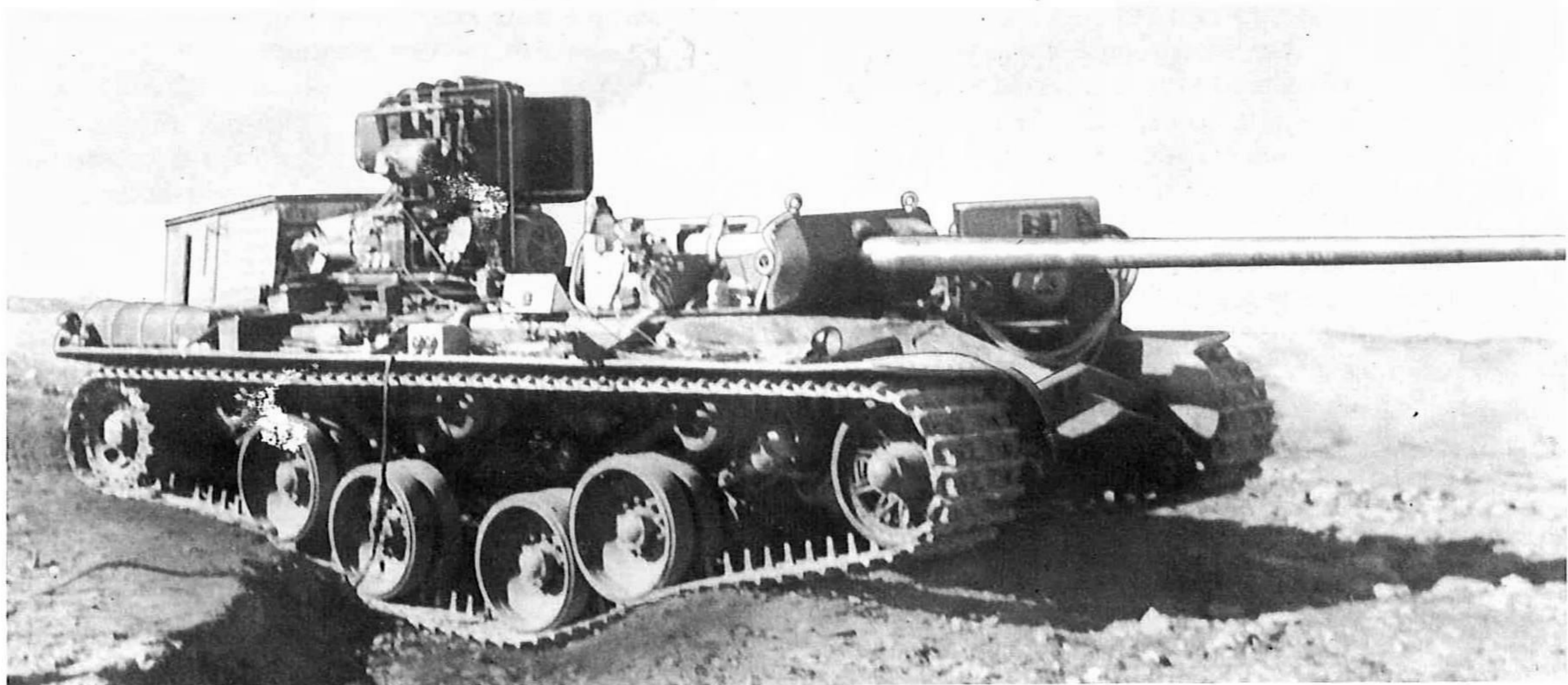
Test rig based on the KRV chassis fitted with a 83.4-mm. 20-pounder of the Centurion.
