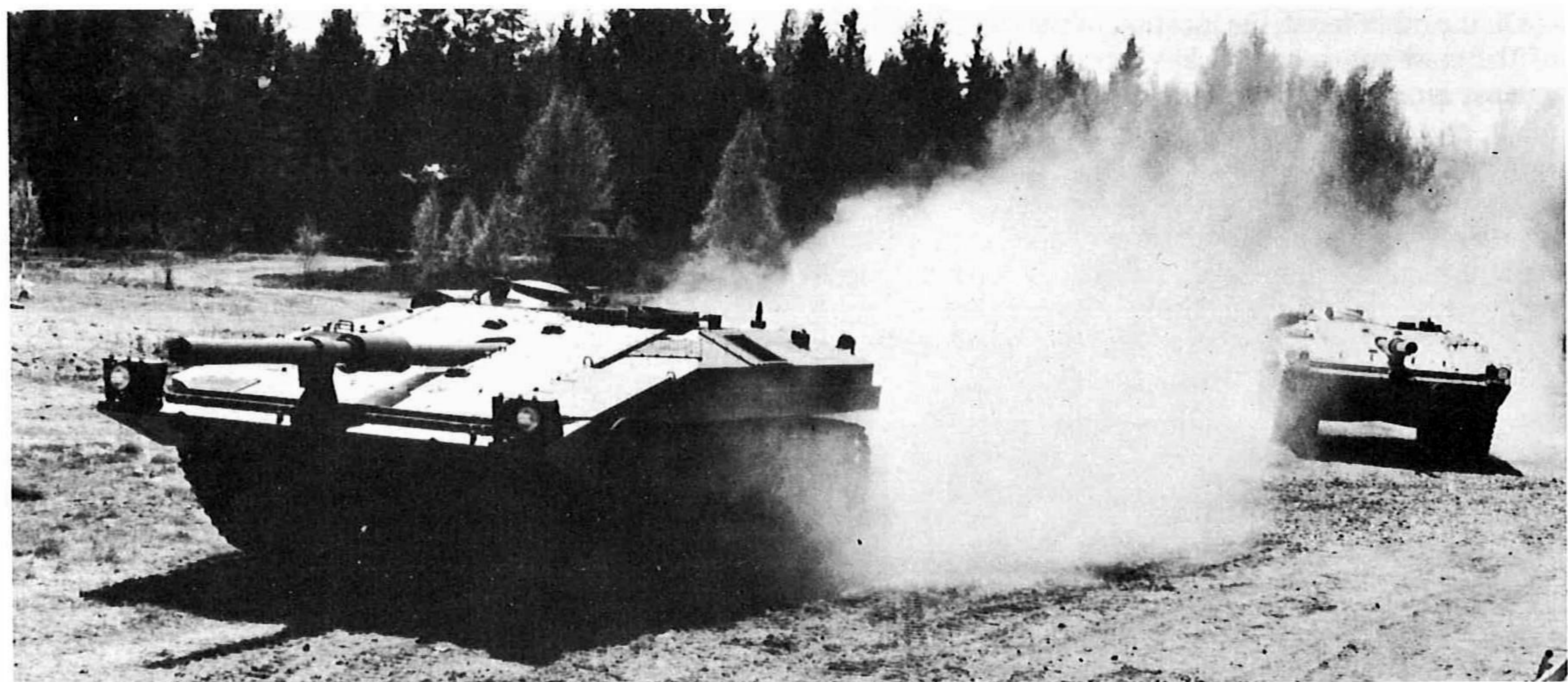
Pre-production models of the S-tank during trials: note the absence of the machine-gun boxes.
