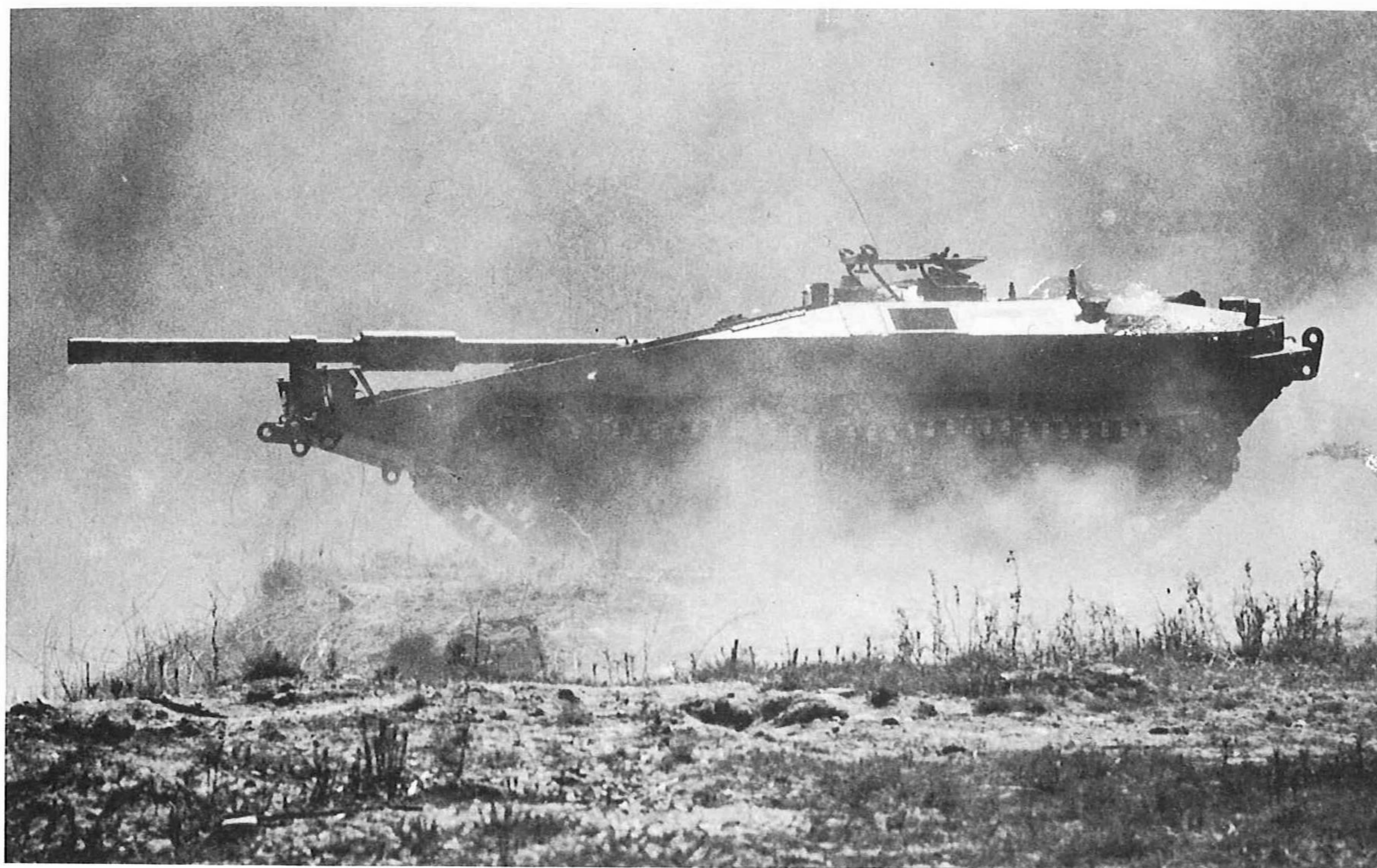
Side view of S-tank pre-production model without machine-gun boxes.
