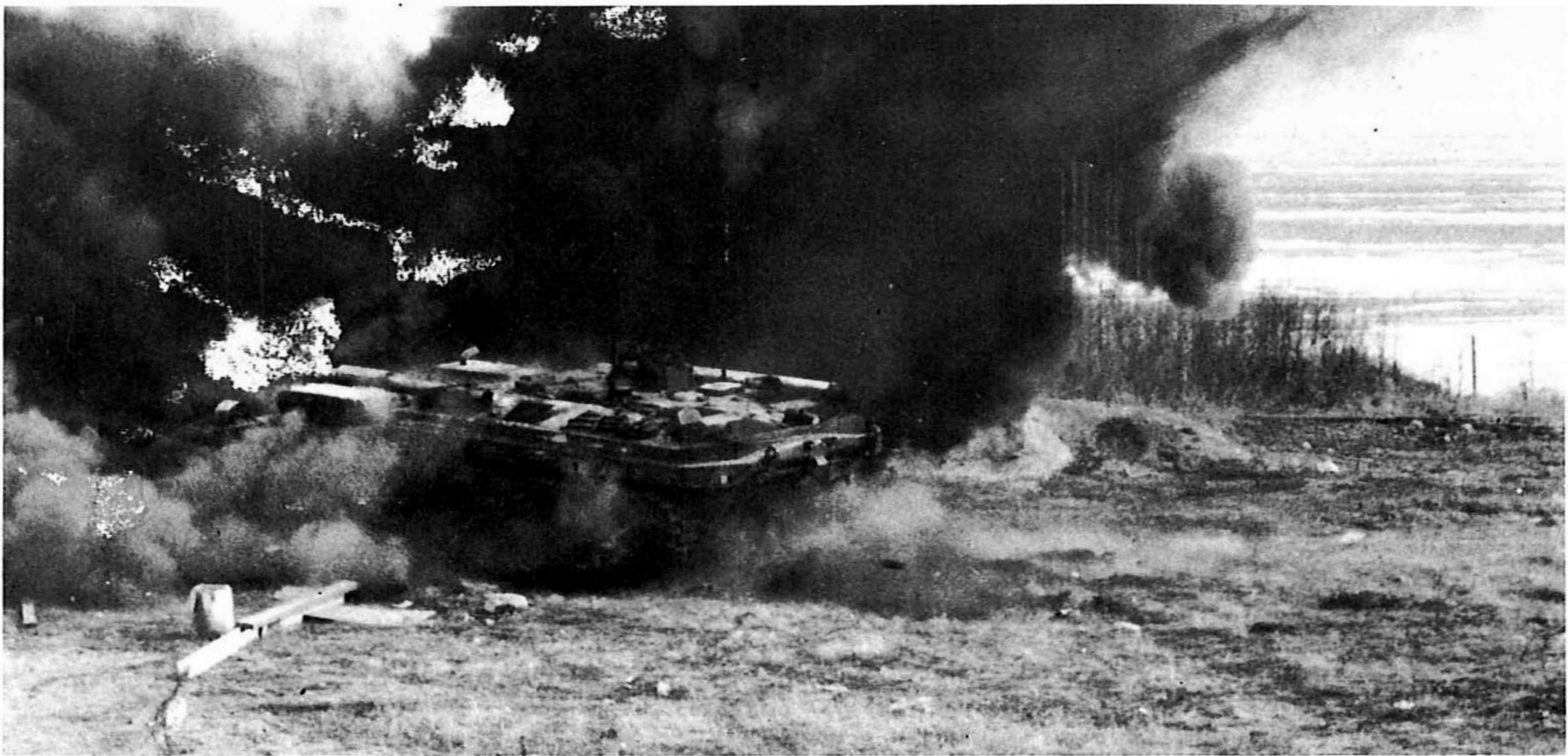
An S-tank with a mine exploding under one of its tracks during immunity trials; damage to the running gear could be repaired by the crew in about 3 hours.
