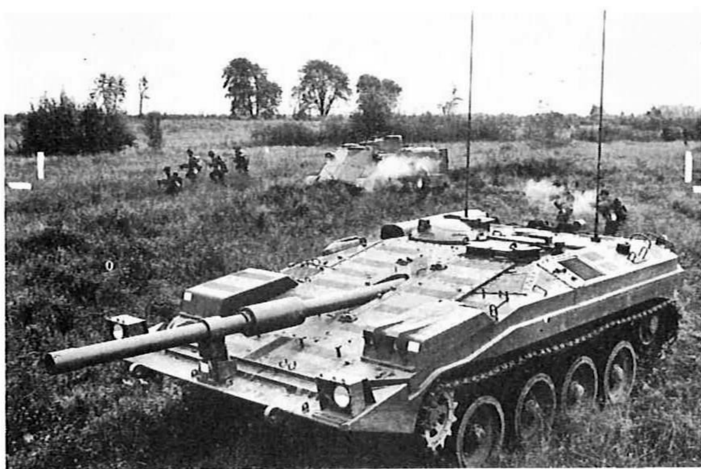
S-tank pre-production model with the original, domed commander's cupola.
