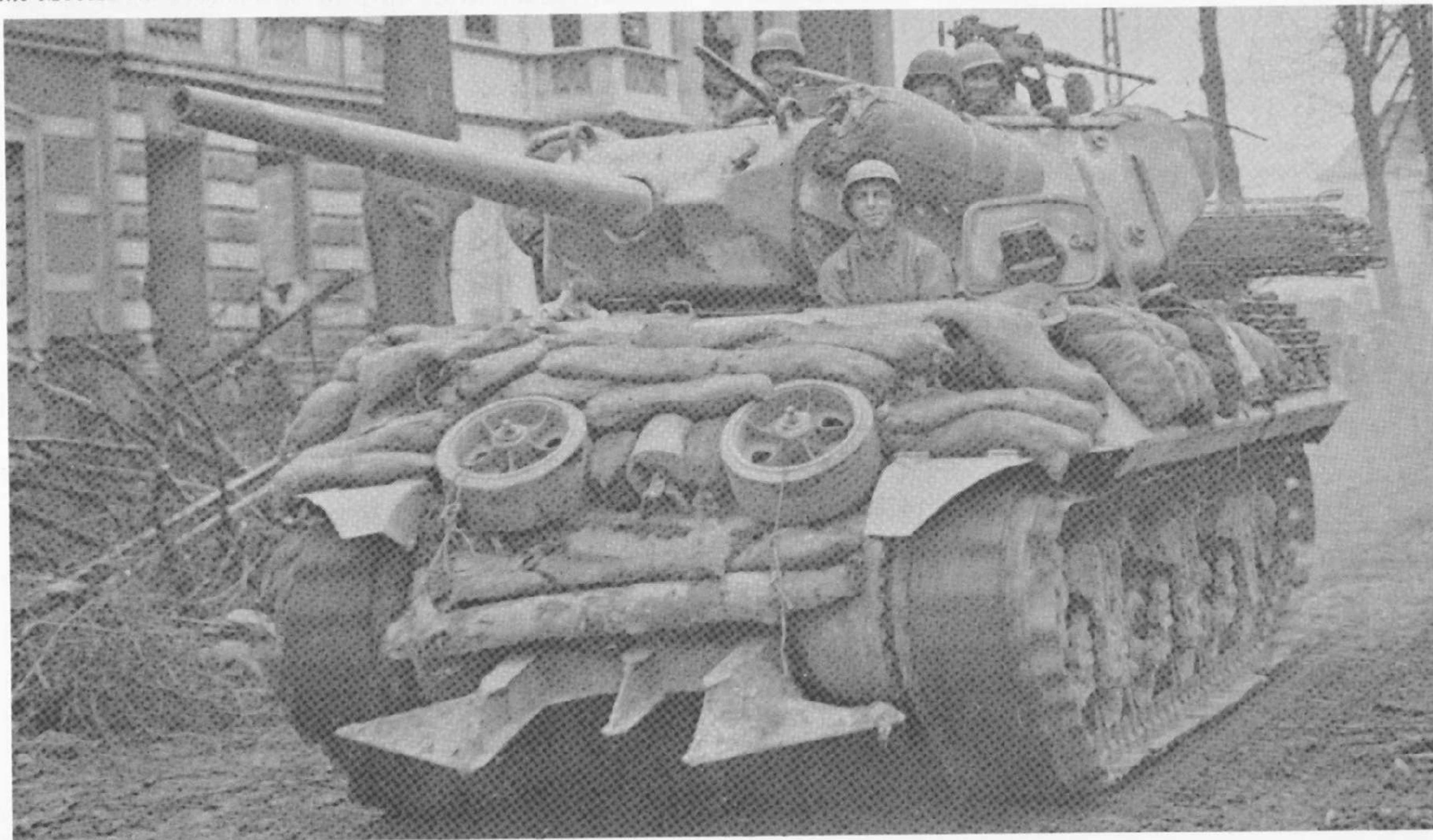
M10 GMC Tank Destroyer fitted with a Cullin Hedgerow device, Normandy 1944. The M10 was built on an adapted M4A2 chassis, the M10A1 on the M4A3 chassis. Both had a 3-inch gun.
