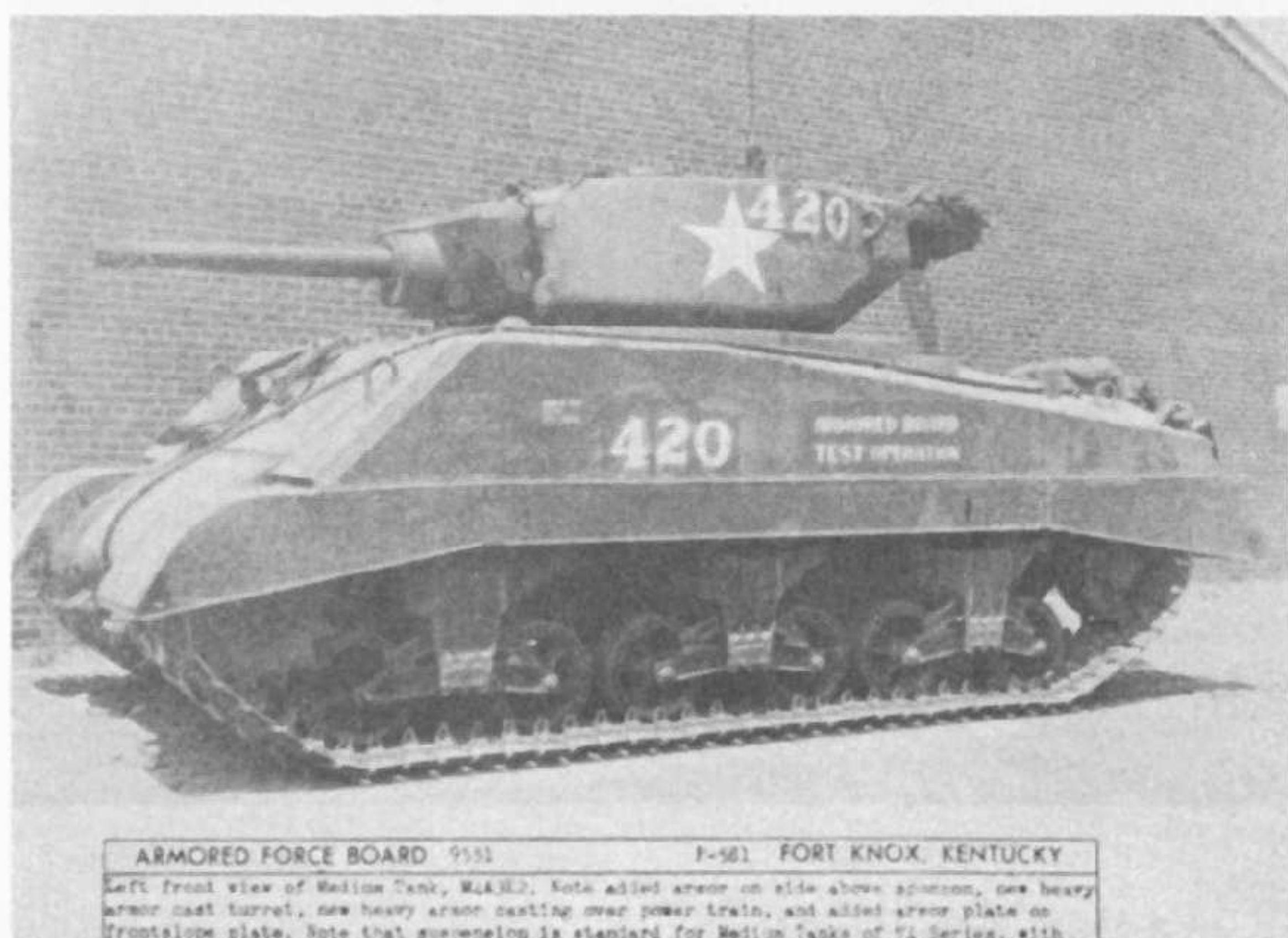
M4A3E2 "Jumbo" was a special assault tank built for the invasion of N.W. Europe to make good the American deficiency in heavy tanks. A new cast turret was made, plus a new heavy cast nose. Rest of hull was thickened with additional armor sheets, clearly visible in the front view. Grousers were a permanent fitting because of the extra weight.
