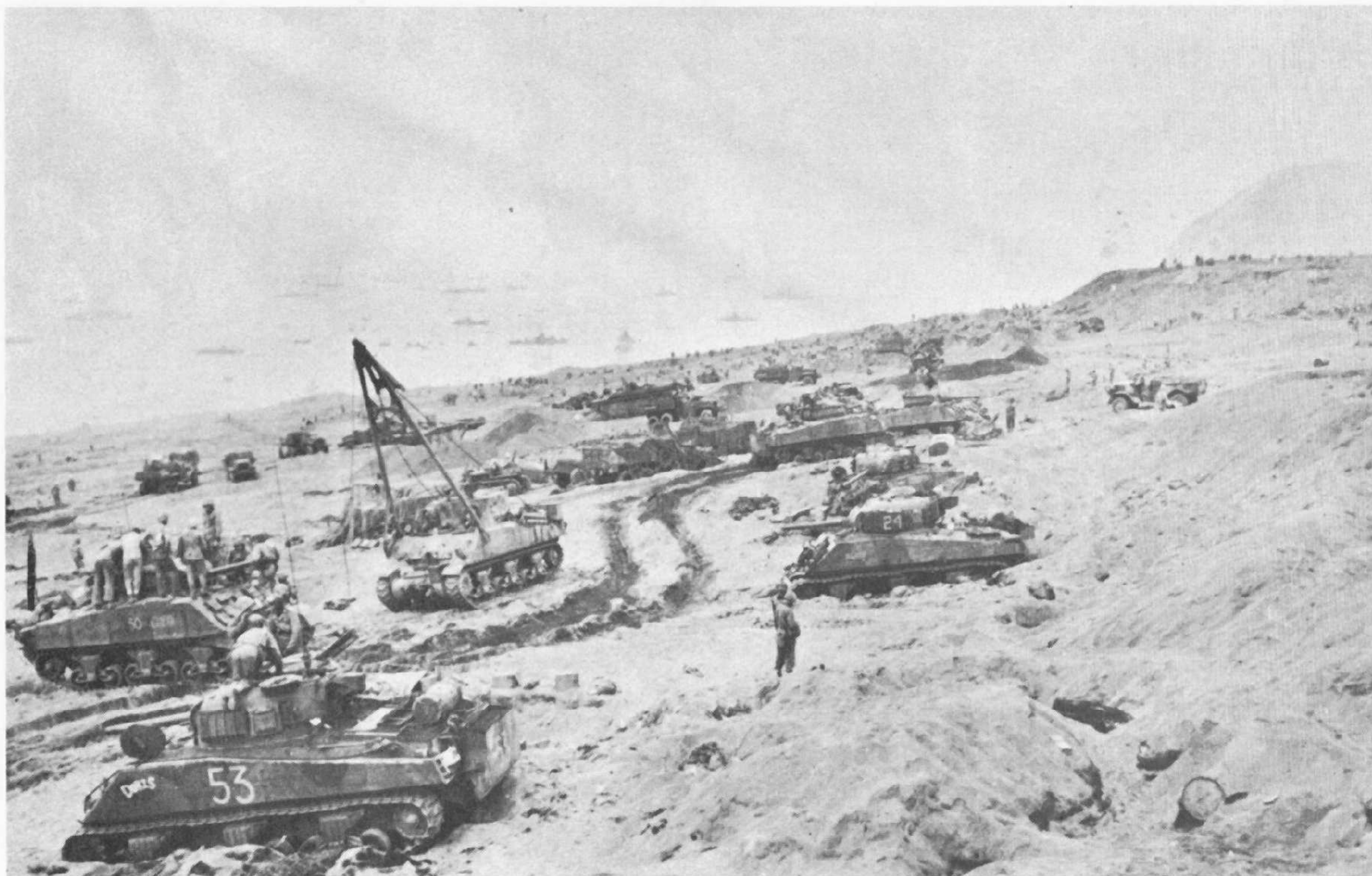
U.S. Marines on Iwo Jima, March 1945. In the foreground late production M4A3s (75mm) wet stowage, and M32 Tank Recovery Vehicle.
