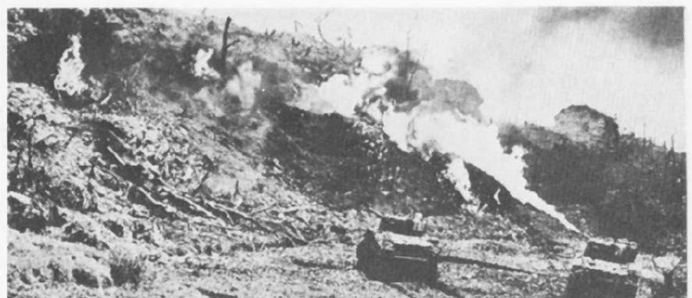
POA-CWS75 H1 Flamethrower on U.S. Marine Corps M4A2 in action against Japanese cave defensive positions on Okinawa, 1945.
