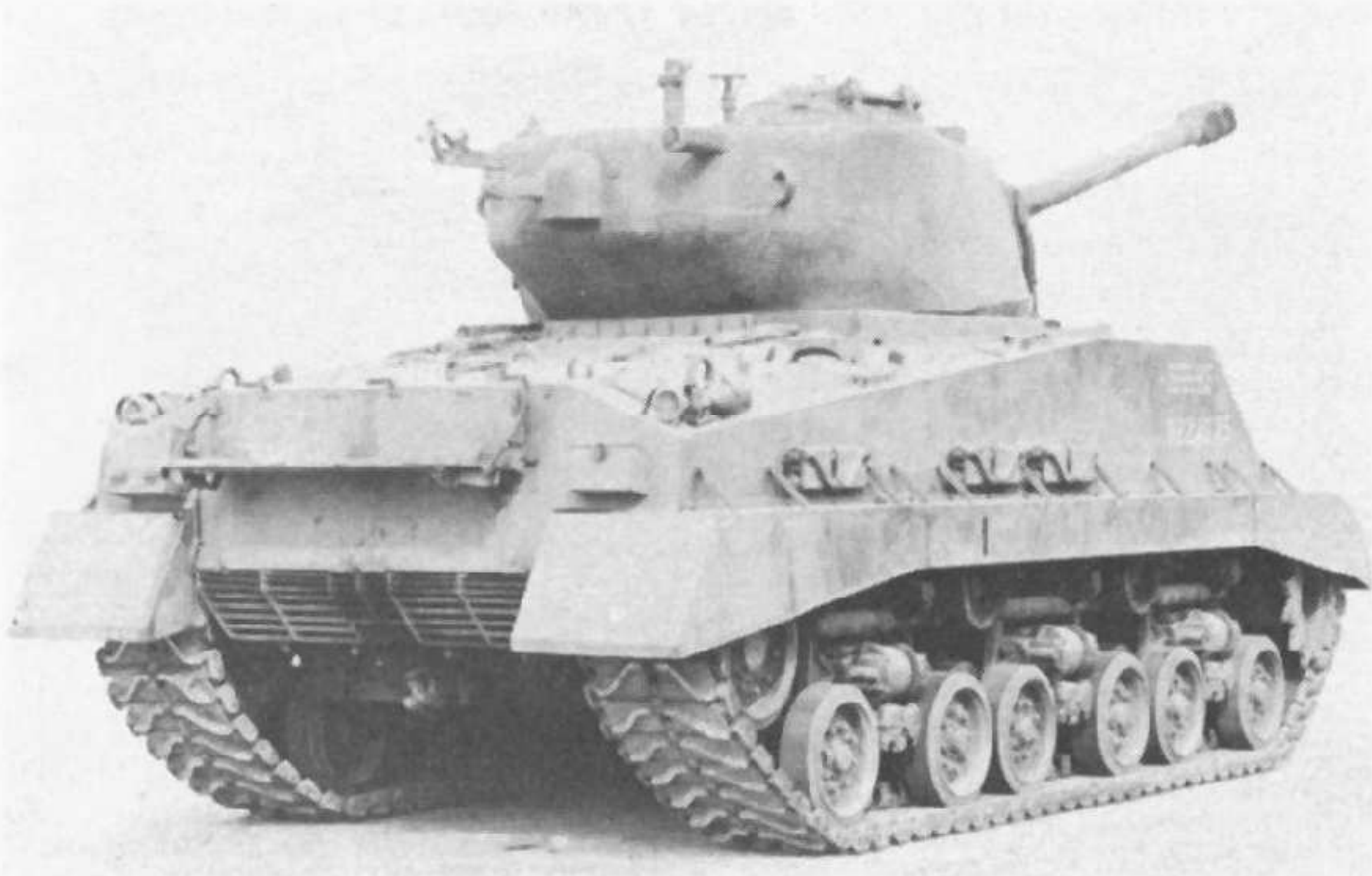
A small number of Shermans with HVSS were delivered to the British in 1945. This is a late production M4A2 (76mm) HVSS, designated Sherman IIIAY by the British (A = 76mm gun; Y = wide tracks). Note the stowage rack at rear and the grilles over the rear exhaust outlets, a feature of late M4 series vehicles.
