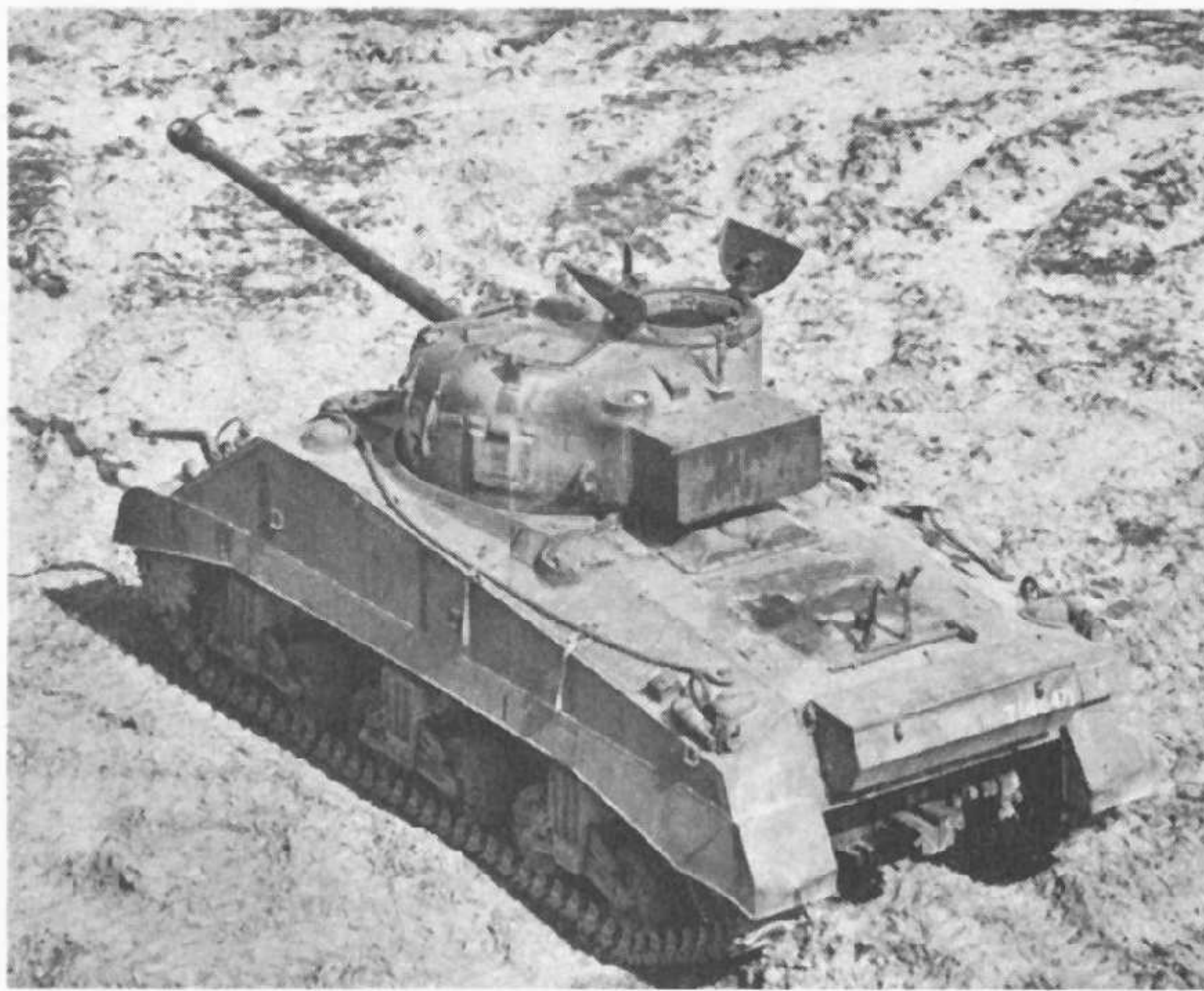
Loader's hatch and counterweight on turret rear were major additions to the "Firefly", shown clearly on this Mark VC. Note barrel clamp on rear decking.
