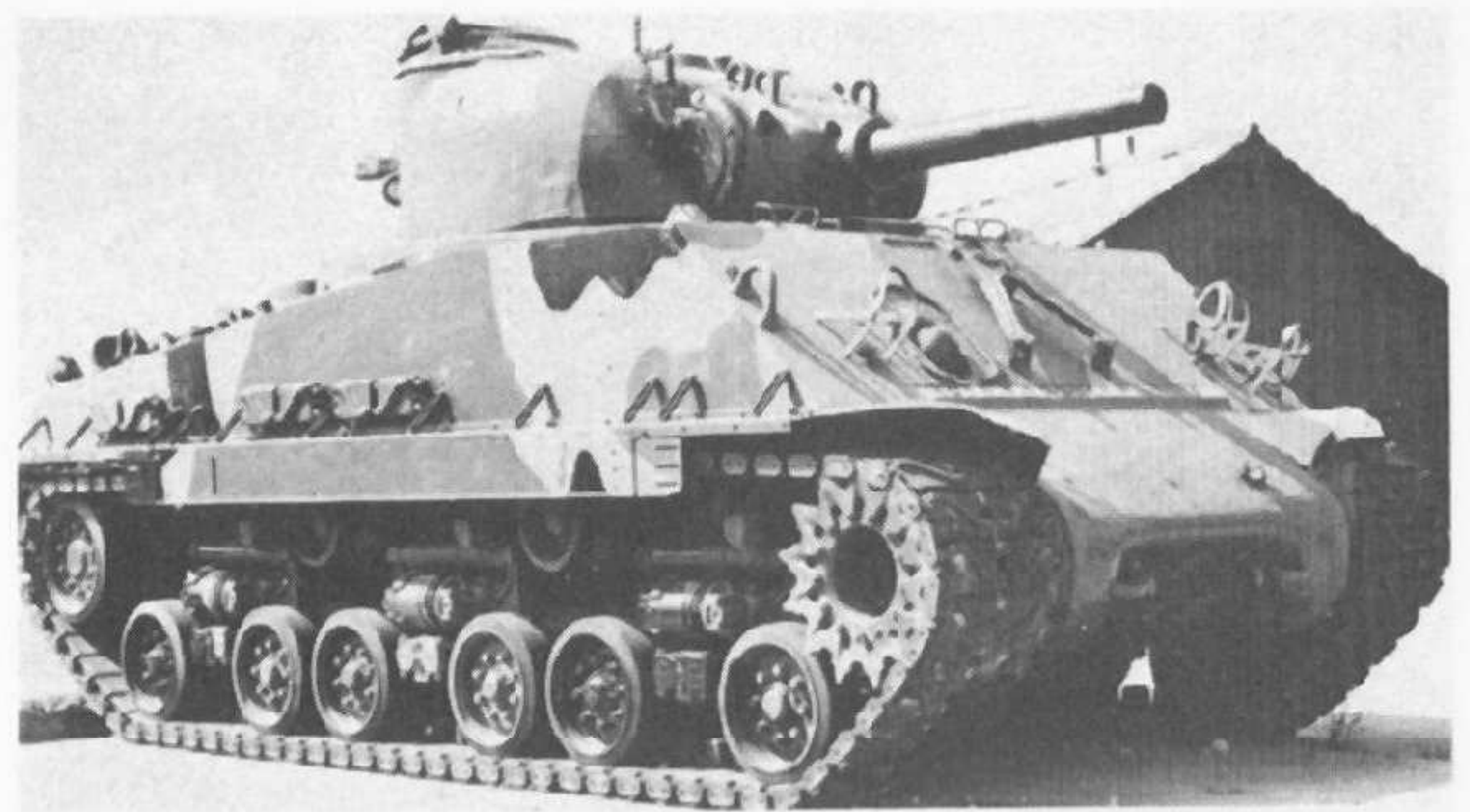
A late production M4 (105mm) with the 47 degree hull front and HVSS. Some of these served with the British Army, 1945-47, under the designation Sherman IBY (B=105mm howitzer, Y=wide tracks).
