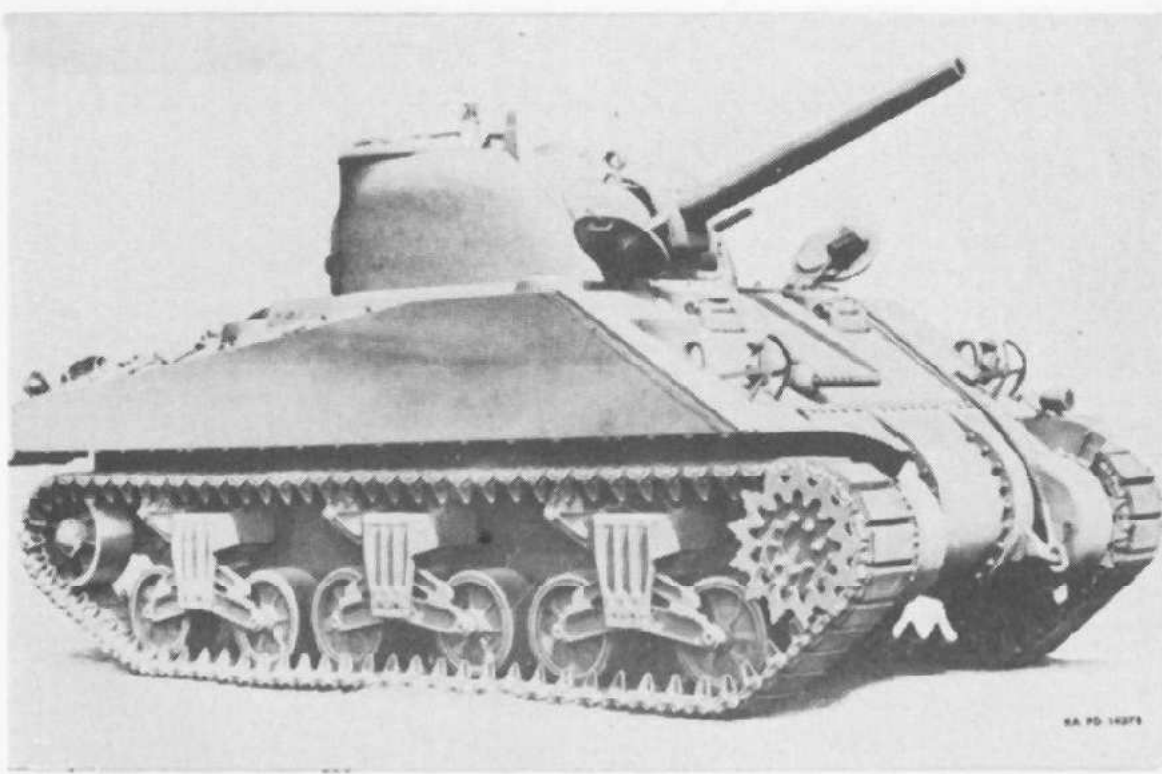
Early production M4 with M34 Combination Gun Mount, "second type" suspension (trailing return rollers), three-piece nose, and vision slots in hull front.
