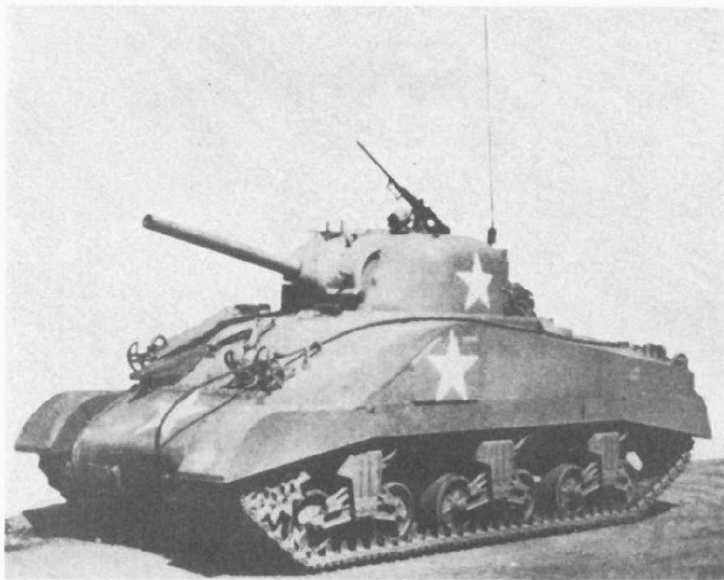
Very few M4A6s were built; they had a combination of cast nose and welded hull and were lengthened like the M4A4 to accommodate a Caterpillar diesel engine.
