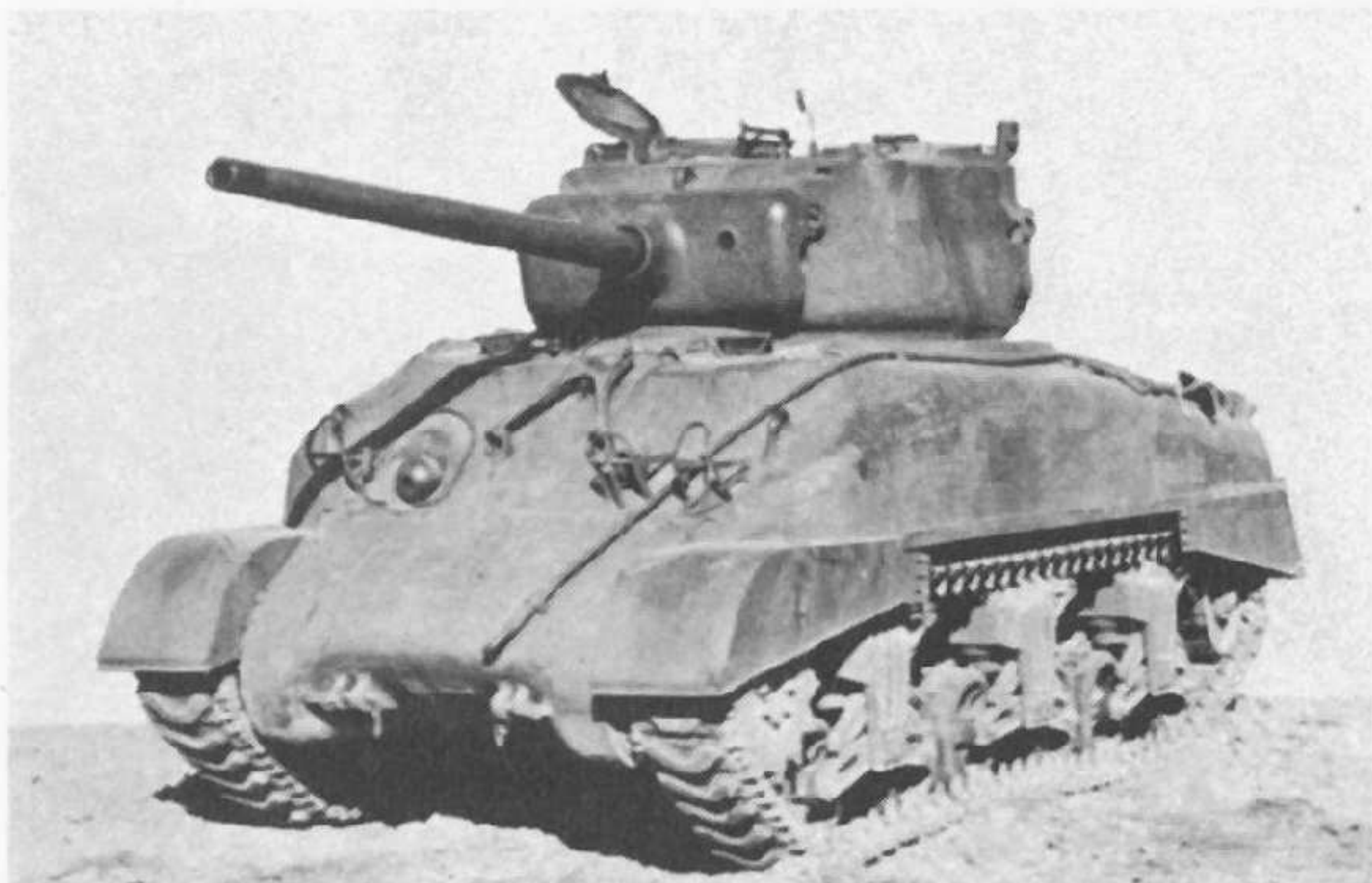
The later M4 series changes are well illustrated in these views of an early (1944) and late (1945) M4A1 (76mm). Vehicle on left has the M1A1 76mm gun.
