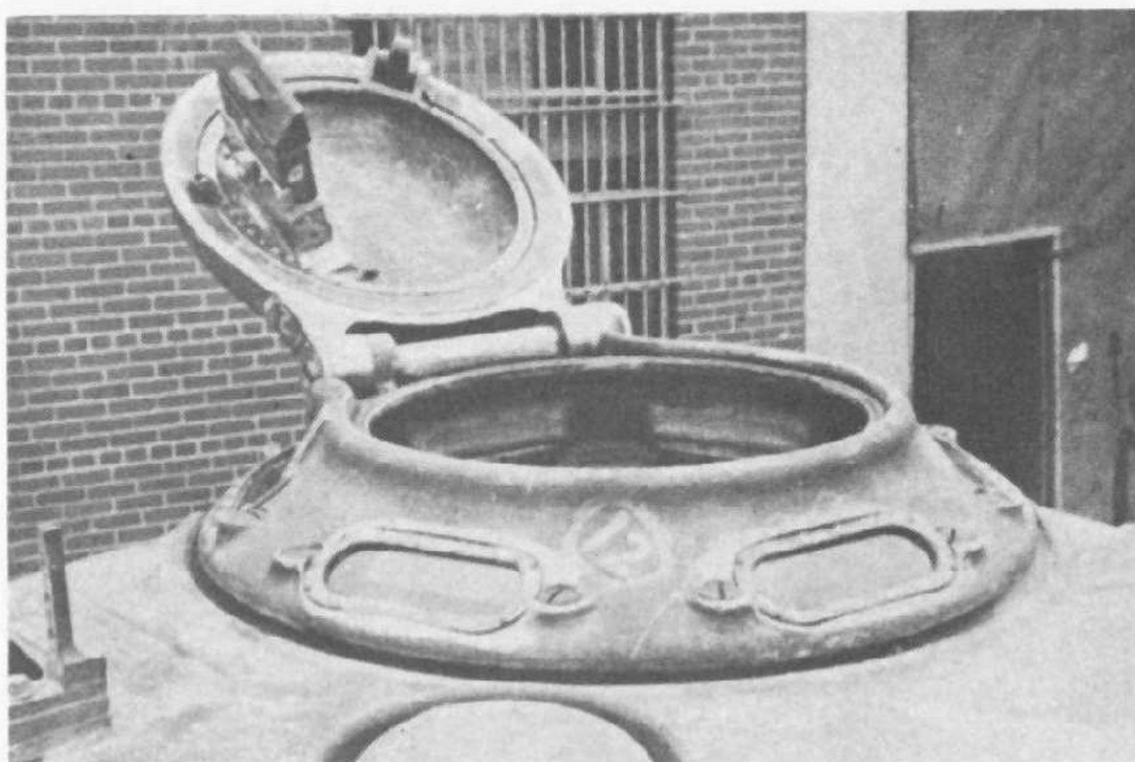
A close view of the all-round view vision cupola fitted to later variants of the M4 series. In the foreground is the "mushroom" ventilator in the turret top. (Picture sources for this Profile are U.S. Official, Canadian Official, and Imperial War Museum.)
