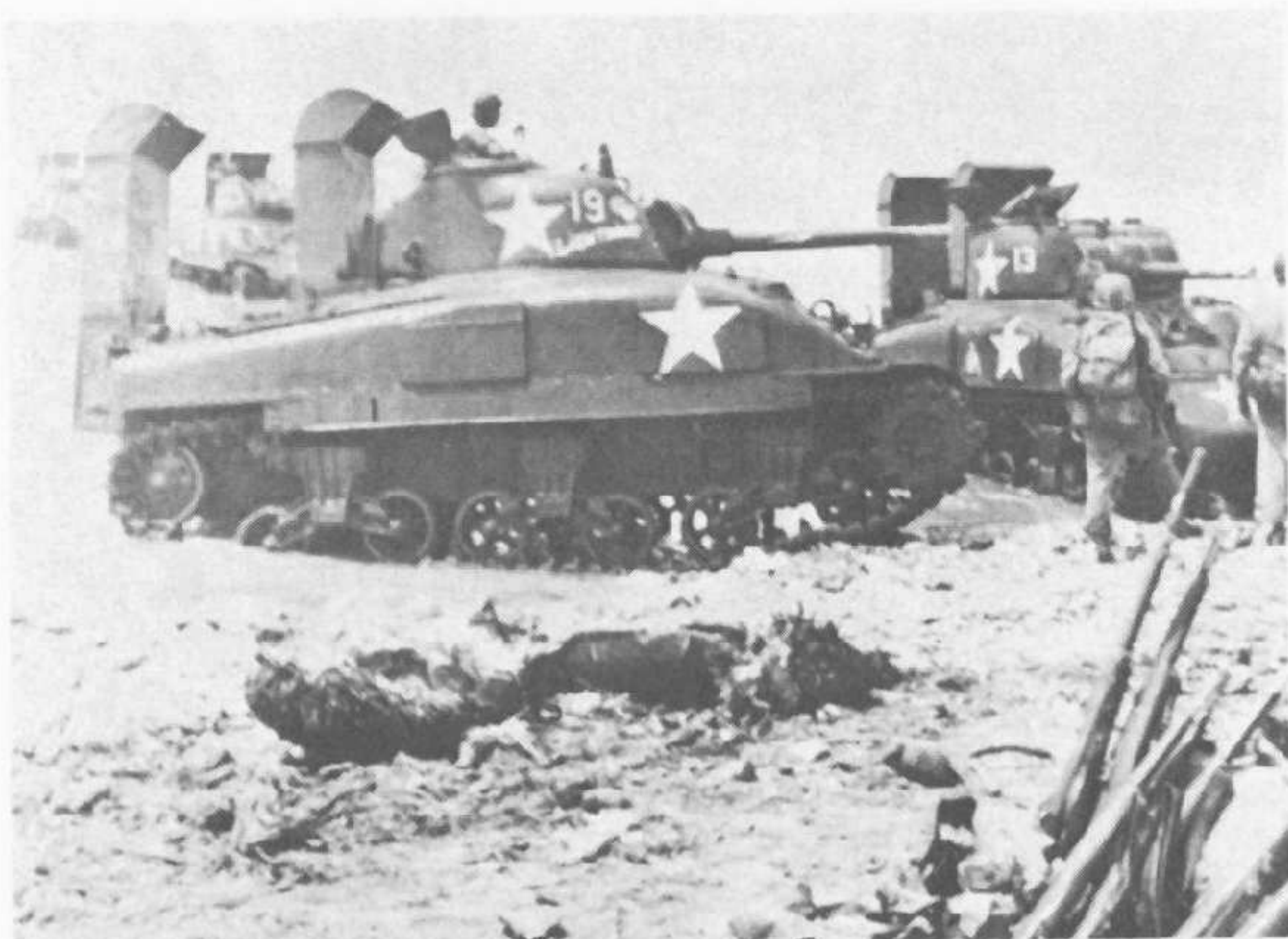
M4A1s of the U.S. Marines landing at Kwajalein. Full wading equipment is fitted, the trunking coming as a kit of parts for each vehicle.
