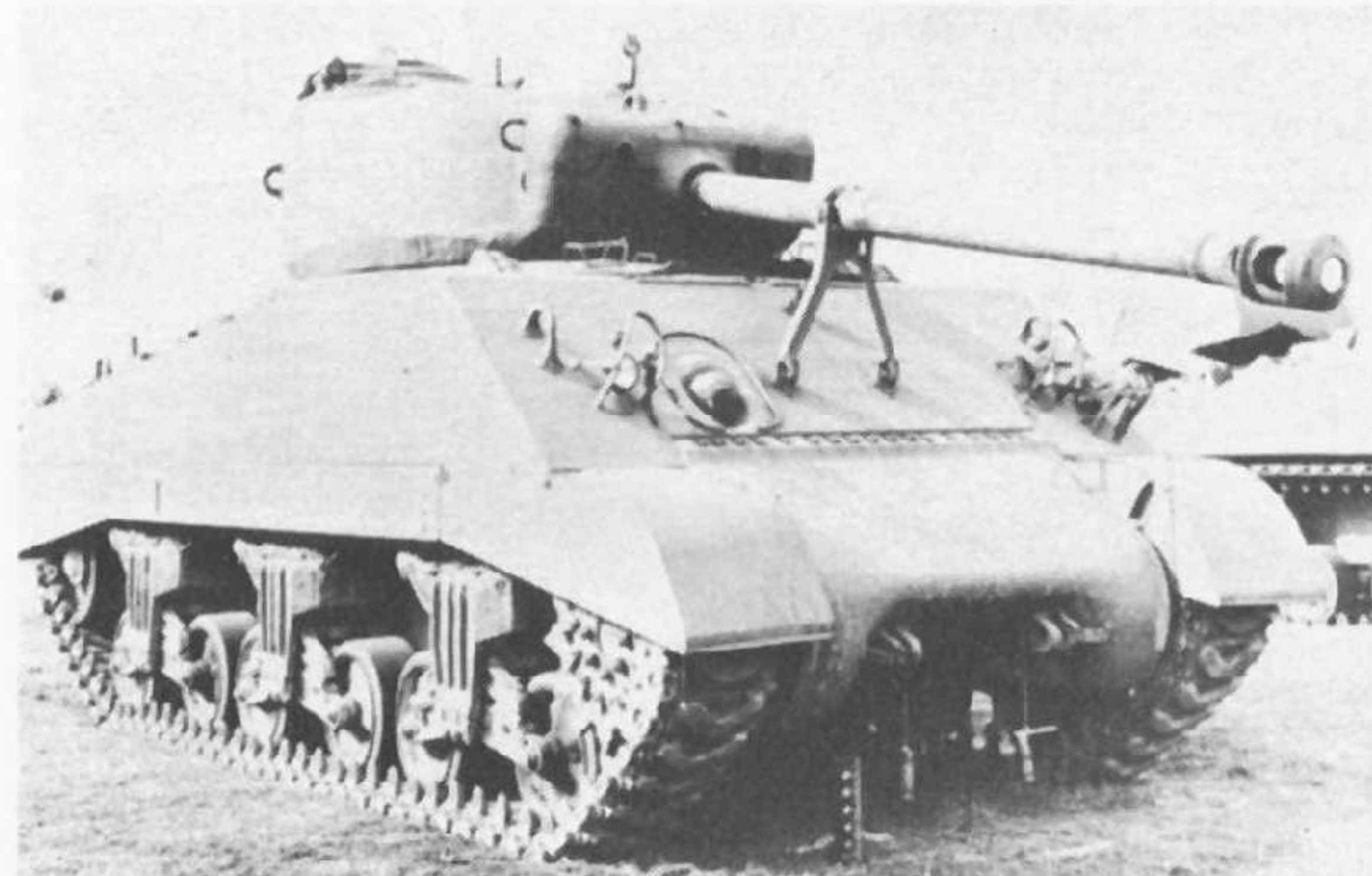
The penultimate production version of the Sherman was the M4A3 (76mm) with vertical volute suspension. The gun is the M1A1C version with muzzle brake.
