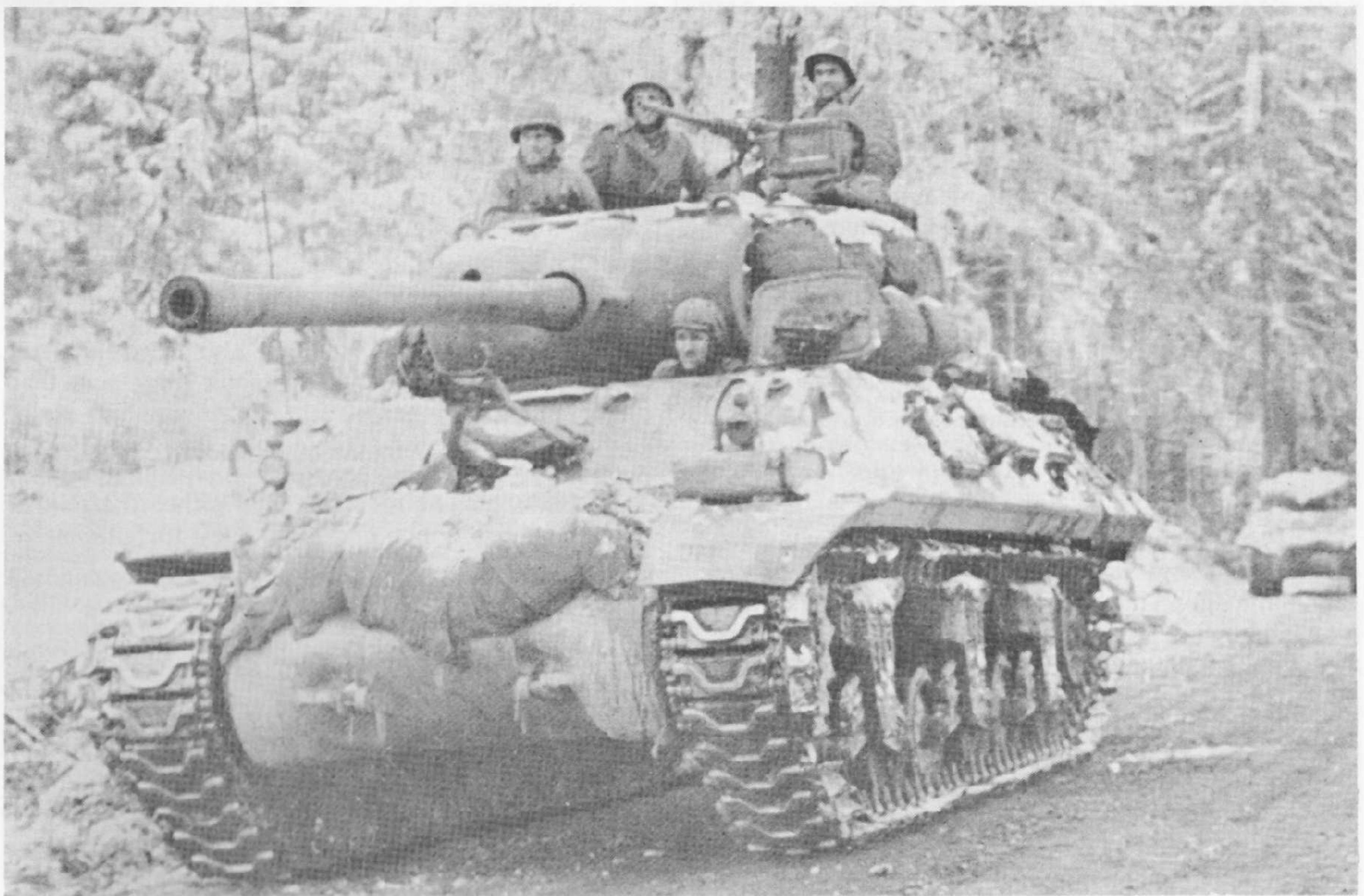
Standard M36 GMC Tank Destroyer on M4A3 chassis, Battle of the Bulge, Ardennes, January 1945. The M36 had a 90mm gun.
