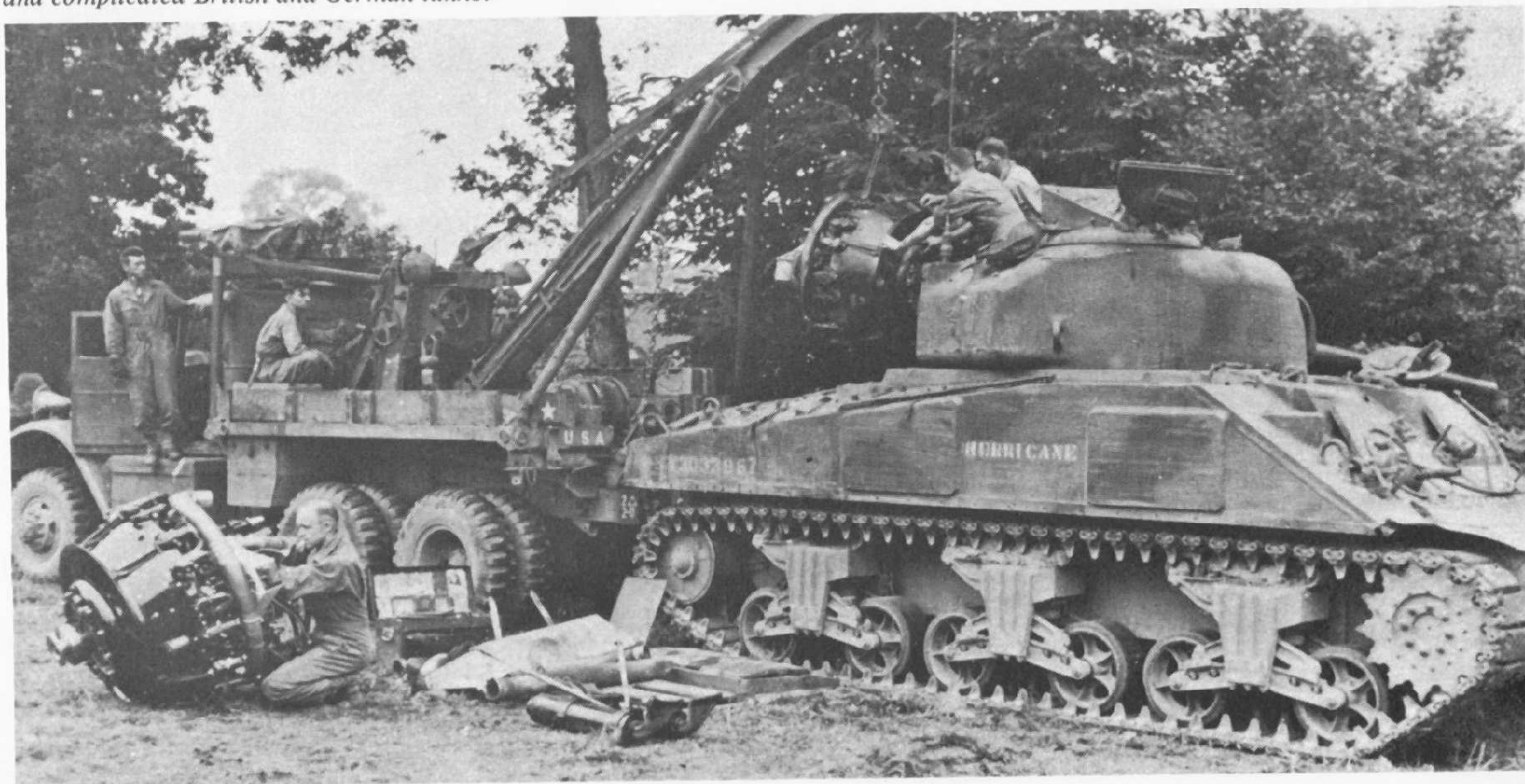
The original M4 had a Wright radial engine developed from the Continental aero engine. The rapid engine change in the field shown in this picture demonstrates a major advantage of the design—ease and speed of maintenance—compared with more sophisticated and complicated British and German tanks.
