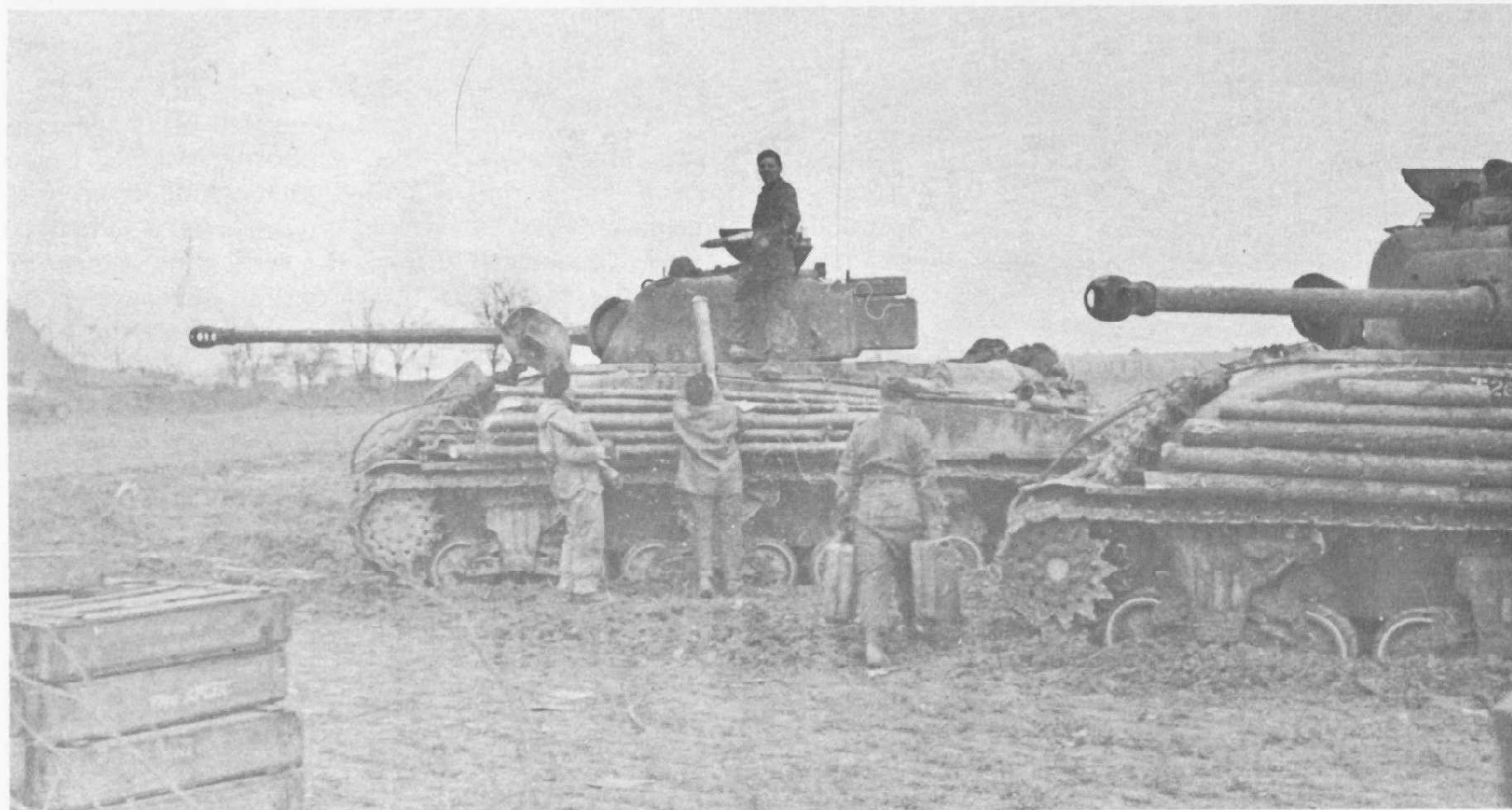
Two "Fireflies" of a Canadian regiment replenishing their ammunition, Germany, March 1945. Note the size of the 17-pdr. AP round. Logs are used here for added side protection.
