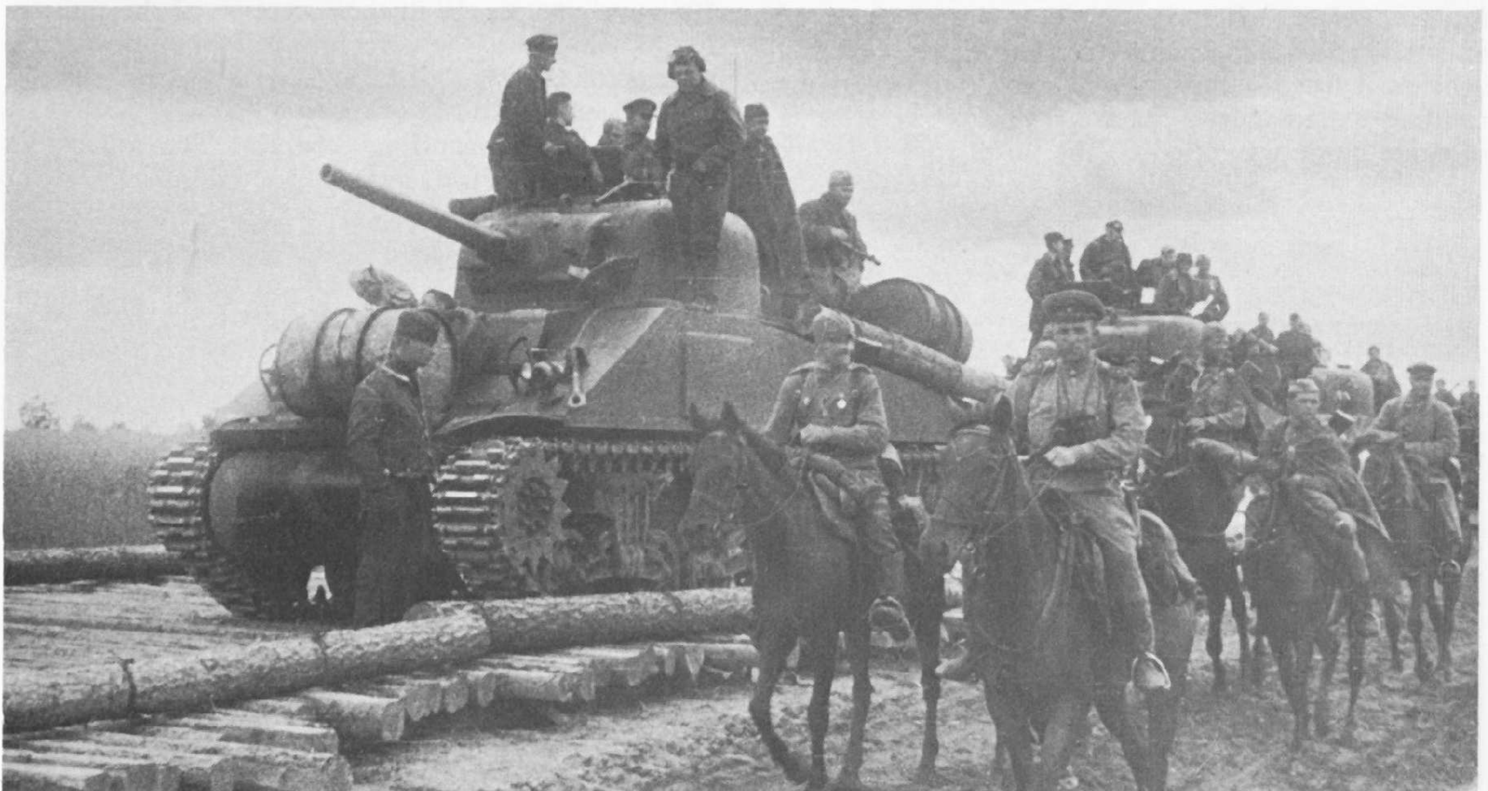
Though little publicised by the Russians, several thousand Shermans (M4A2) were delivered to the Soviet Army on Lease-Lend in 1942. Here cavalry pass new Russian Shermans near Kharkov. Note typical Soviet features including the log for unditching, and the extra fuel tanks. Front vehicle has all-steel tracks.
