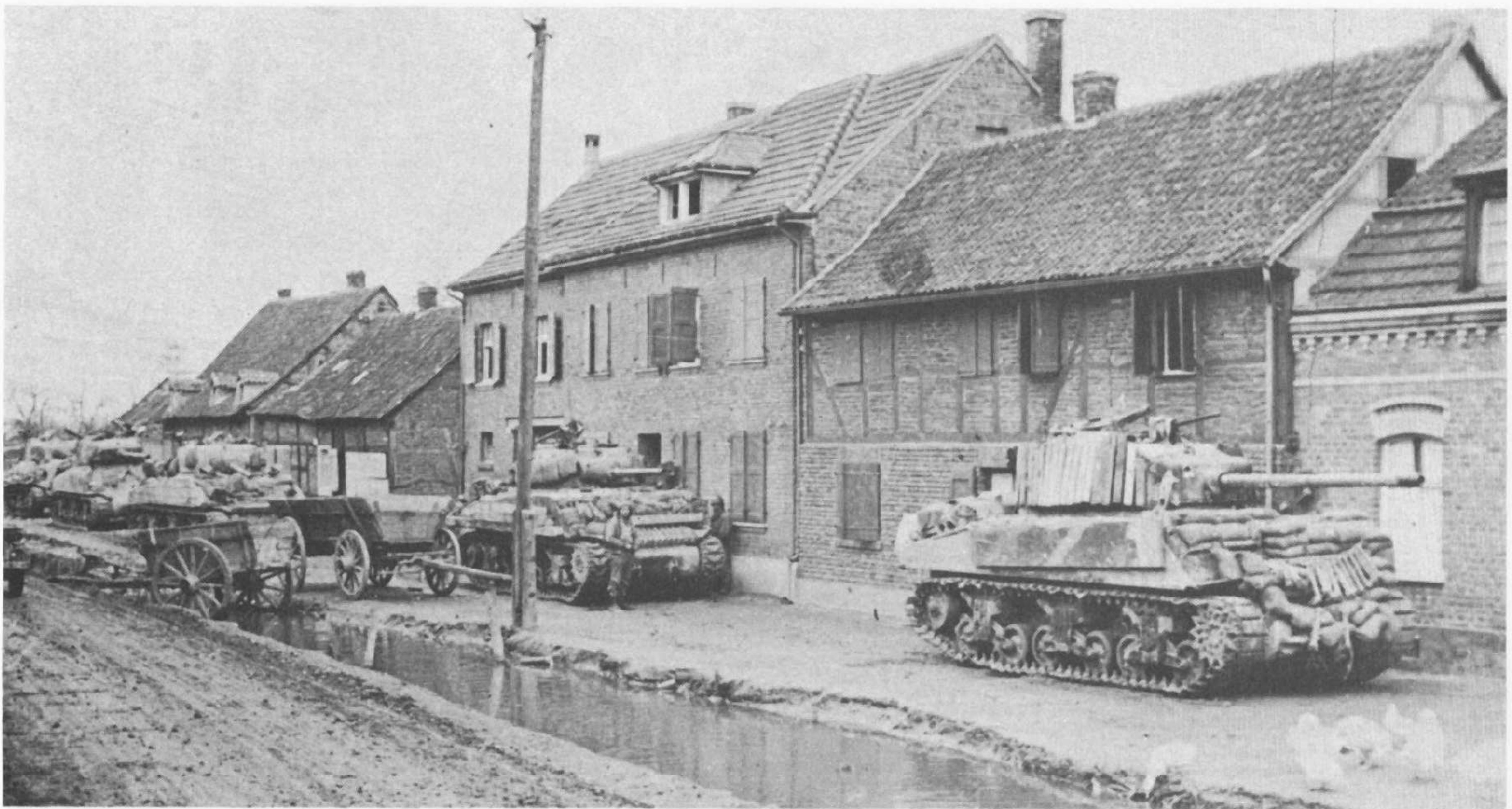
M4A3 (76mm) with a M4A3 and other Shermans behind it line a street in Bergerhausen, Germany. The tanks are of U.S. 8th Armored Division (nicknamed "Thundering Herd") which took part in the battle for Cologne which fell on March 6, 1945. Note extemporised protection of wood and sandbags.
