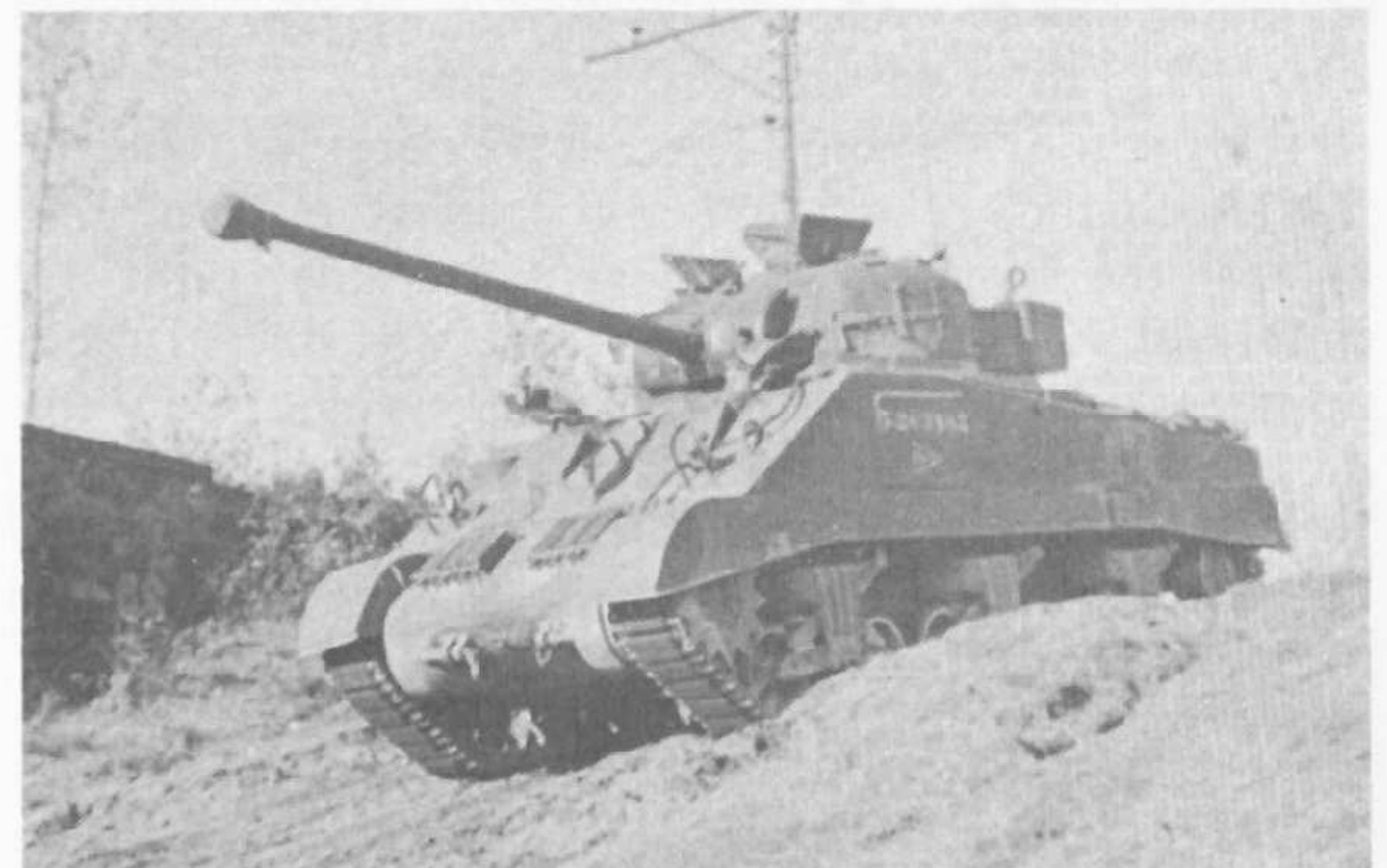
Sherman "Firefly". The British re-armed many Shermans, mainly Mark I (M4), Mark II (M4A1), Mark III (M4A2), and Mark V (M4A4), with the 17-pdr. gun to produce the most effective tank in Allied use when France was invaded in 1944. Shown here is a Mark IC (C=17-pdr. gun). Popular name for the conversion was "Firefly".
