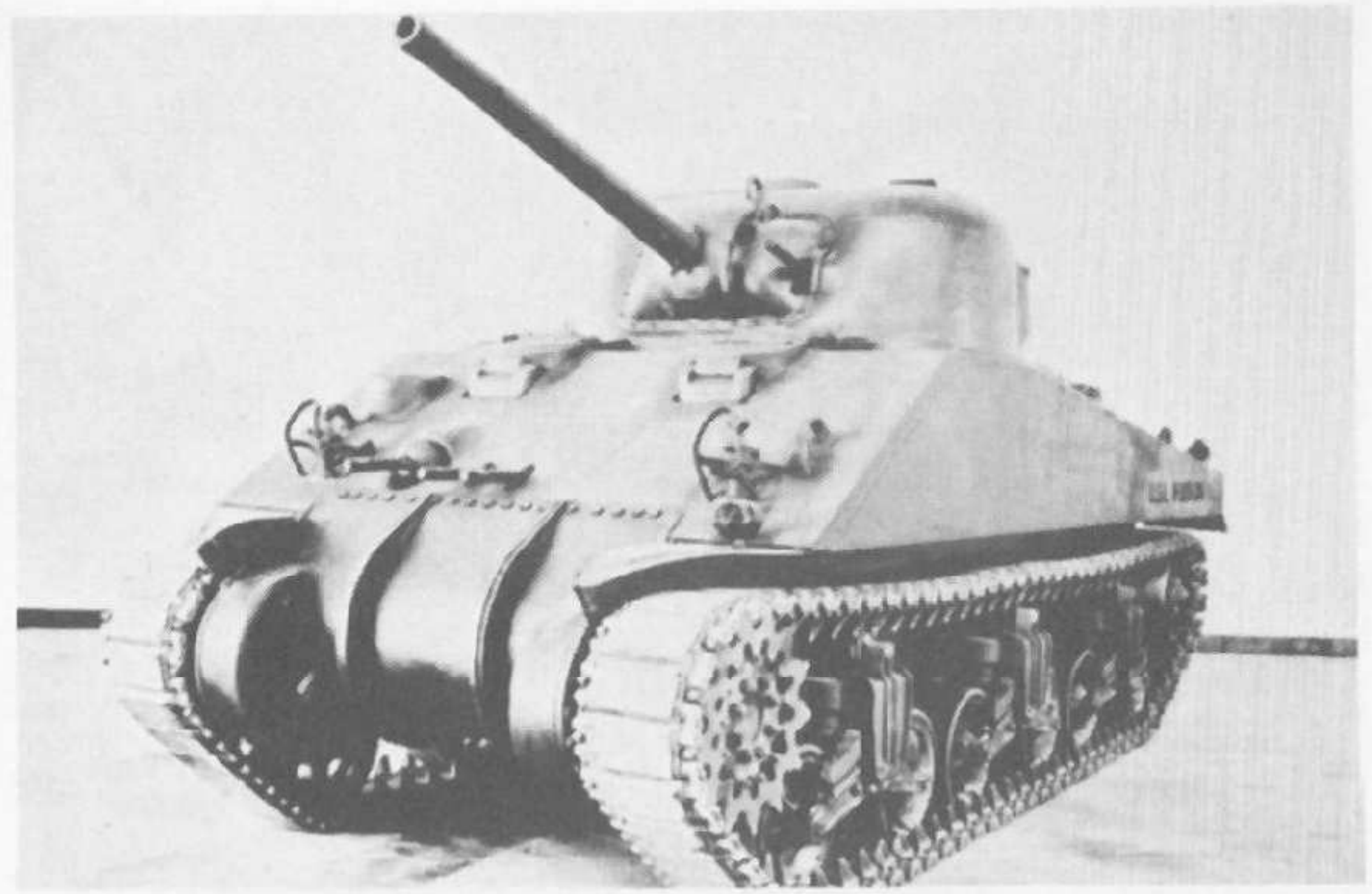
Early production M4A2 with M34 Combination Gun Mount, "first type" suspension (vertical return rollers), vision slots in hull front and fixed nose machine-guns.
