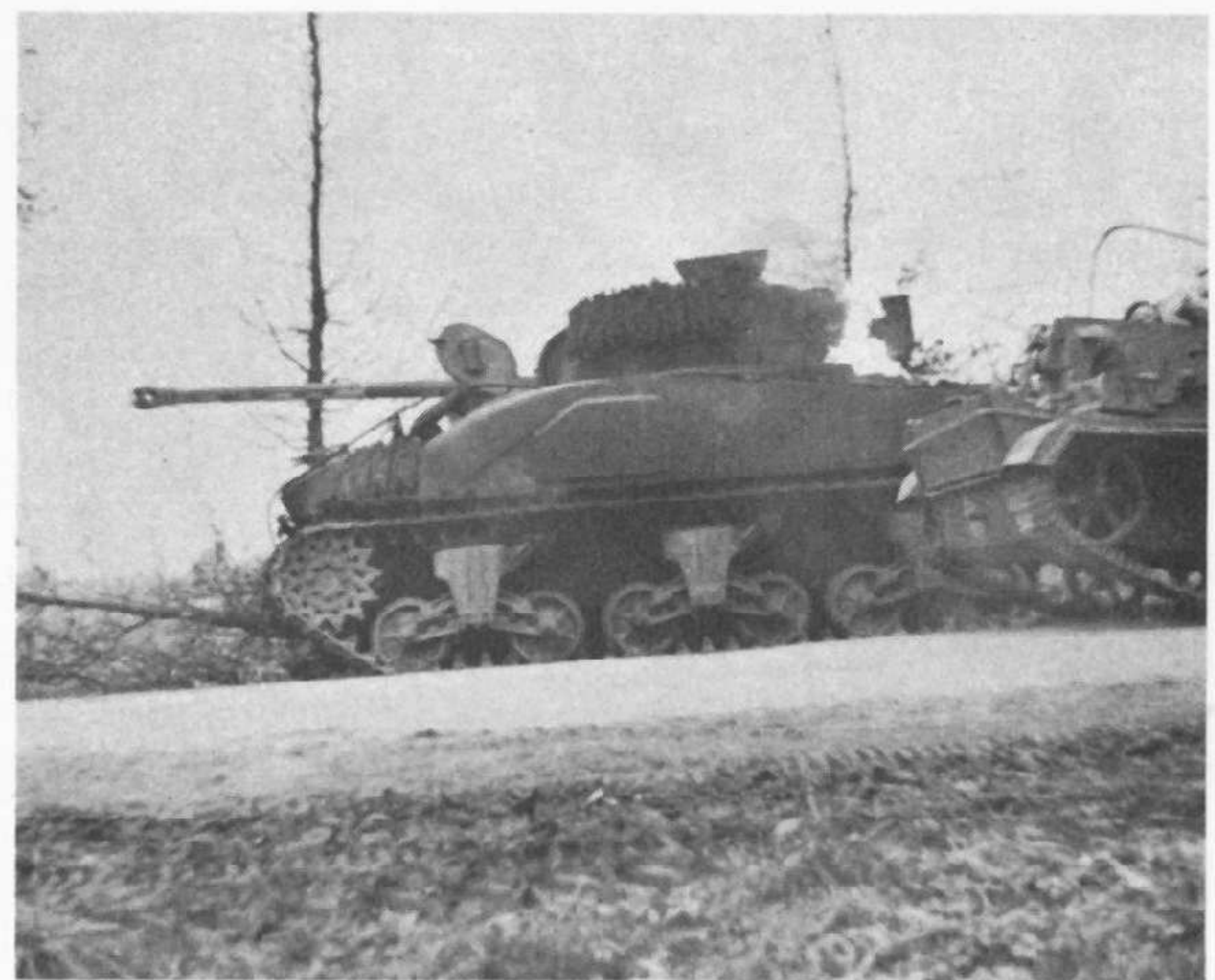
Late production M4s had the hull fronts originally produced for the cancelled M4A6 i.e. combination cast/rolled. They were known to the British as Sherman Hybrids. This one seen in Holland in 1945 has been converted to "Firefly" standards as a Sherman IC.
