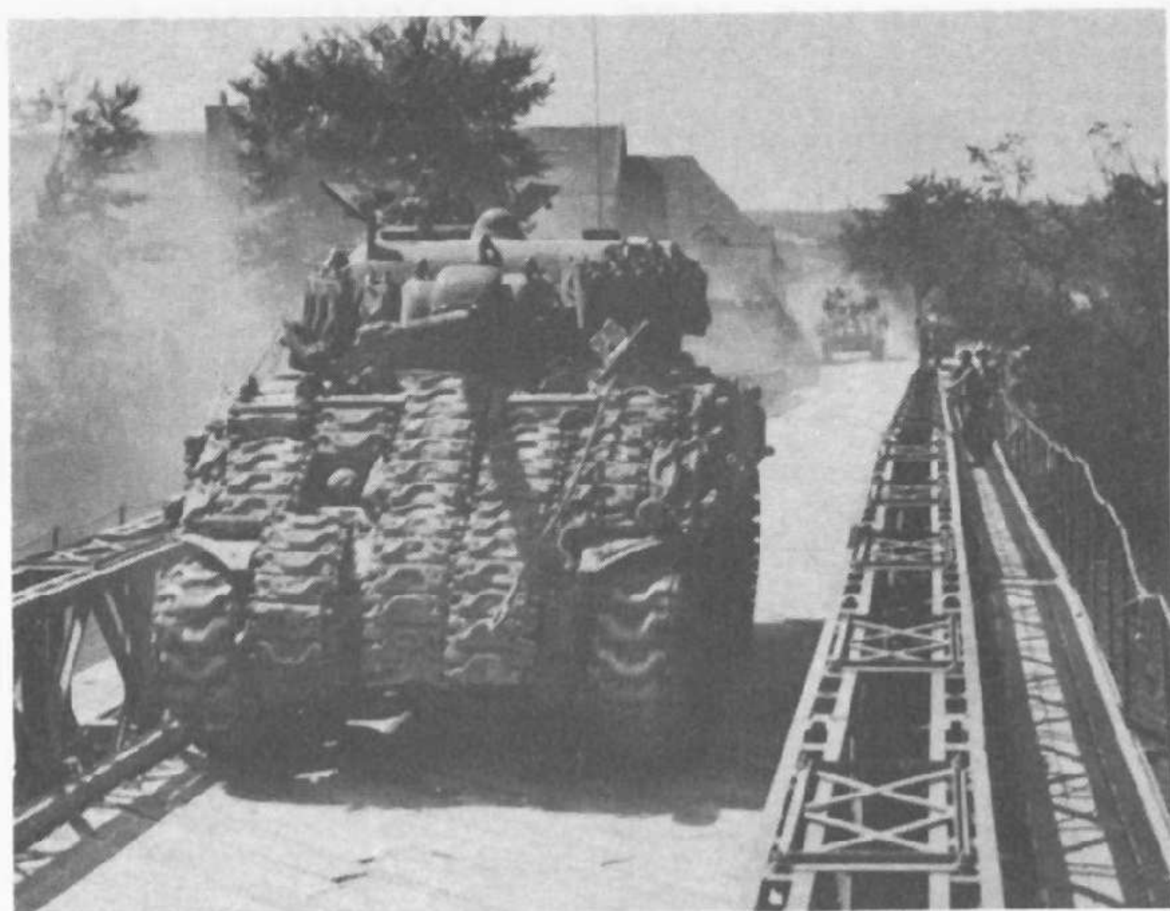
Extensive application of spare track shoes was another way of improving the Sherman's protection. This vehicle is crossing the Orne near Caen in August 1944.
