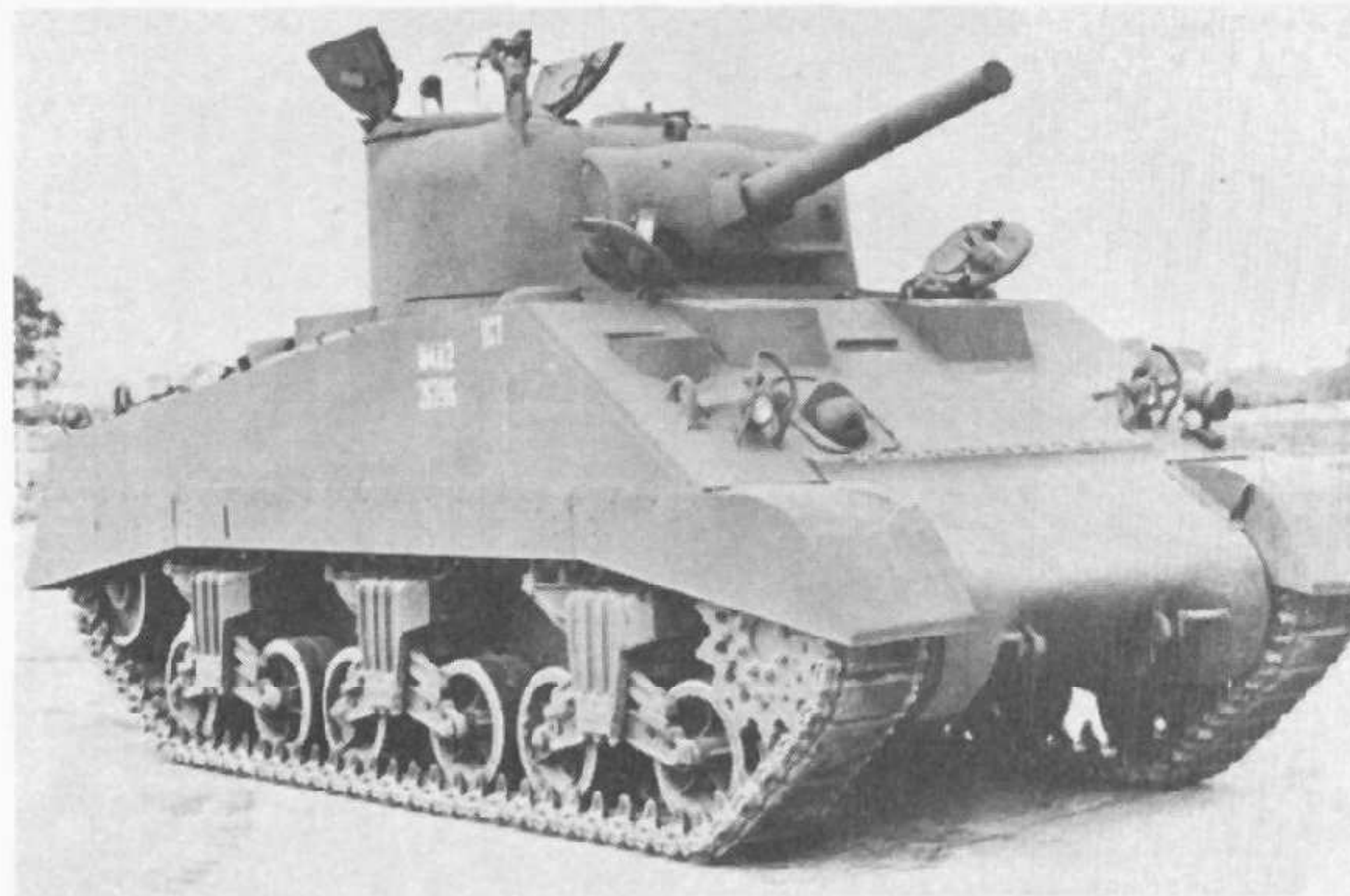
1943 production M4A2 with cast nose, M34A1 Combination Gun Mount, sandshields, and no vision slots.
