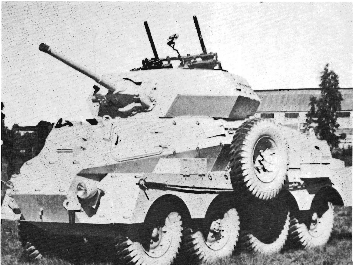
South African Armoured Reconnaissance Car, Mark VI—Armoured Car, Marmon-Herrington, Mark VI. This car, the first model, with 2-pdr. as the main armament, is in the Royal Armoured Corps Tank Museum at Bovington, Dorset.
