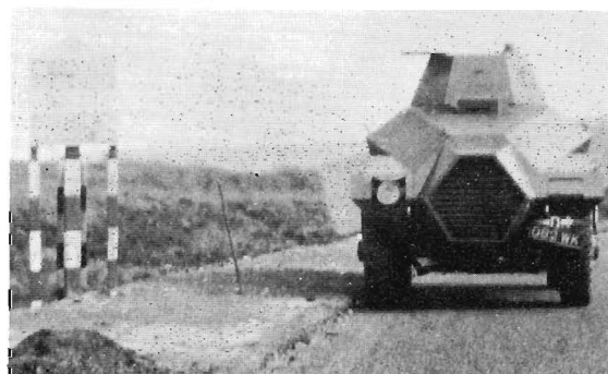
Rear view of the Alvis-Straussler Type A.C.3D showing the hexagonal radiator grille. The vehicle is on test in Britain. It is at Carter Bar on the border between England and Scotland. (Photo: Alvis Ltd.)
