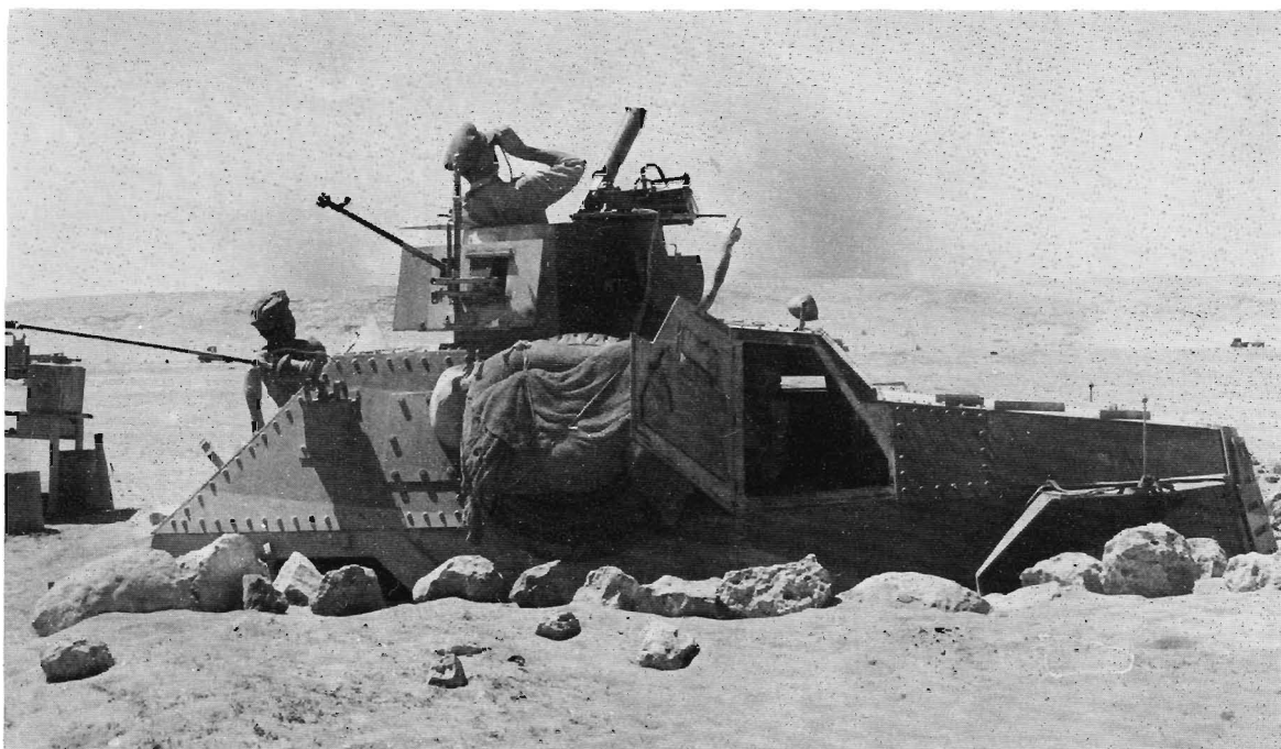
Armoured car of C Squadron, King's Dragoon Guards, dug in at Tobruk, September 1941. This is an example of the early riveted-hull version of the South African Reconnaissance Car, Mark II. (Photo: Imperial War Museum)
