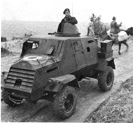
Car, 4 x 4, Light Reconnaissance, Canadian G.M. Mark I, Otter I, of 4th Canadian Reconnaissance Regiment in Italy.
