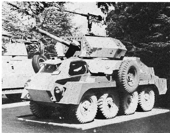
South African Armoured Reconnaissance Car, Mark VI, second model. This has a 6-pdr. as its main armament, and a co-axial 7.92-mm Besa, and a single 0.5-in. Browning for anti-aircraft use. This car is in the South African National War Museum.
