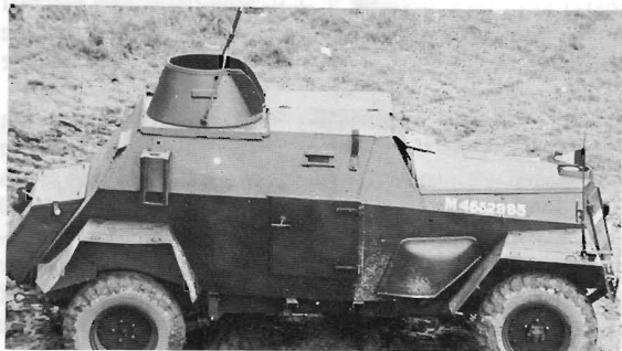
Three views of Car, 4 × 4, Light Reconnaissance Humber Mark III, which, with Mark IIIA, was the car of this class most widely used by the Reconnaissance Corps in action. Dimensions are: Wheelbase 9 ft. 3½ in., track 5 ft. 1 in., length overall 14 ft. 2½ in., width overall 6 ft. 3 in., height to top of turret 6 ft. 11 in., tyres 9.25 in. × 16 in. (Photo: R.A.C. Tank Museum)
