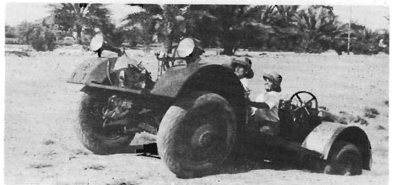
The curved armoured body of the A.C.2 could easily be removed in one piece. Note rear driving position. (Photo: Alvis Ltd.)
