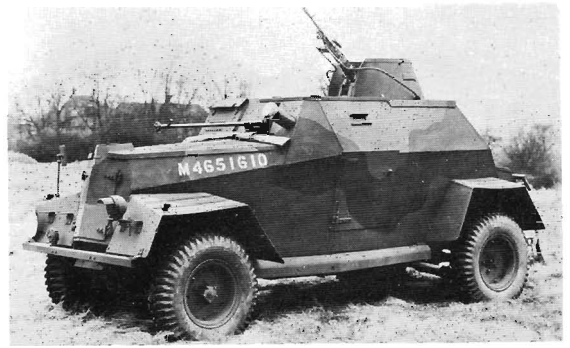
Car, 4 × 4, Light Reconnaissance, Humber Mark III, with radiator doors closed (operated from driver's seat). Boys anti-tank rifle in hull front, Bren gun in turret, and smoke discharger. Driver's visor closed.
