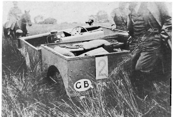
Straussler's "Hefty" tractor seen here on test in Belgium. The position of the tractor shows how the front and rear halves were able to pivot independently. (Photo: Alvis Ltd.)
