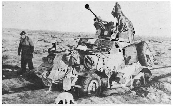
Marmon-Herrington, Mark III, stuck in soft sand. This is a late version (Mark IIIA) with "solid" front armour, absence of square headlamp covers, and spare wheel on left hand side of hull. The turret is fitted with a captured German 28/20-mm. tapered anti-tank gun. (Photo: K.D.G. History)
