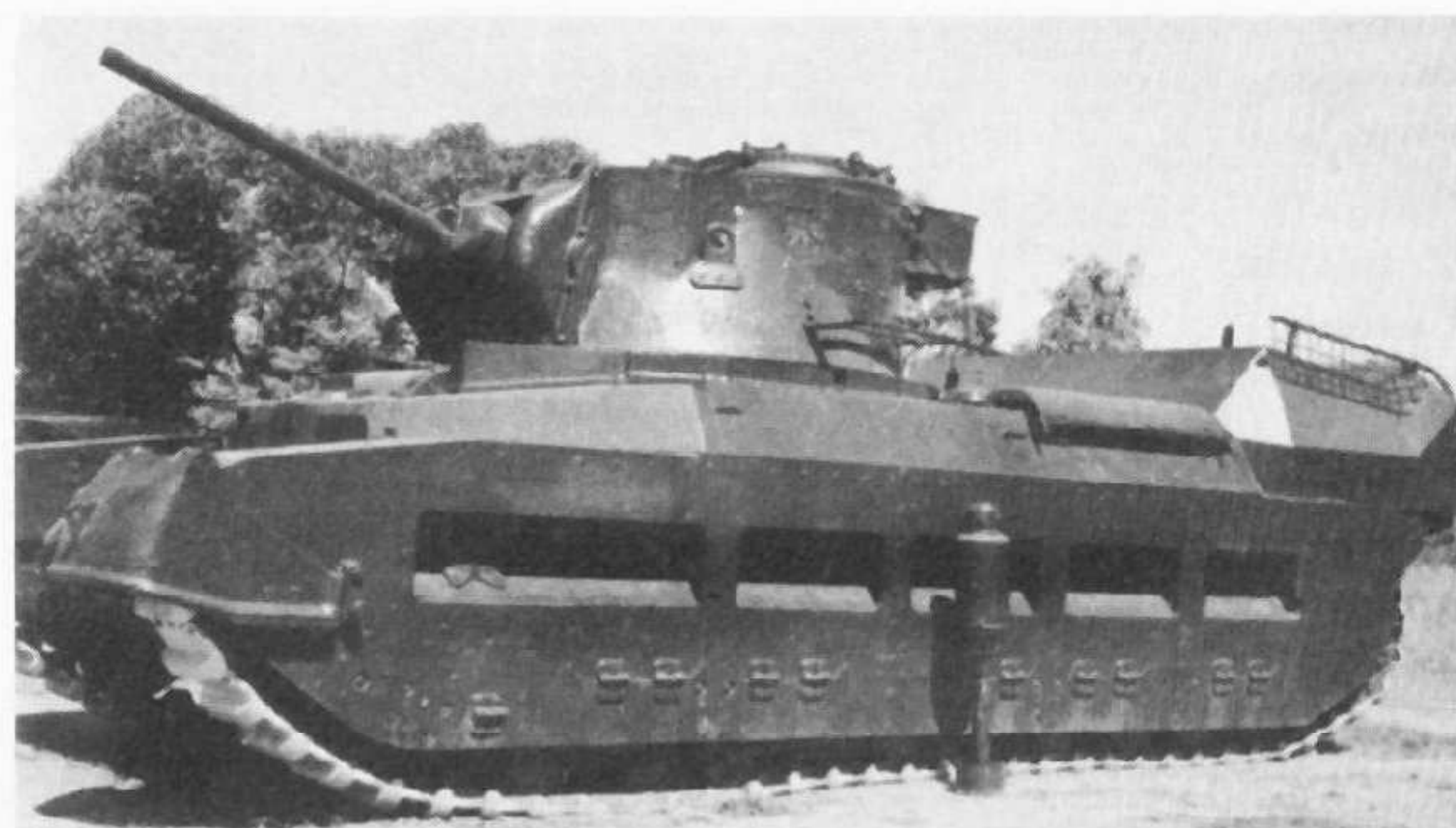
Matilda Hedgehog with the projector, over the rear of the engine compartment, lowered in the travelling position. The Hedgehog bomb, standing at the side, weighed 63 lb. (Photo: R.A.A.C. A.F.V. Museum)
