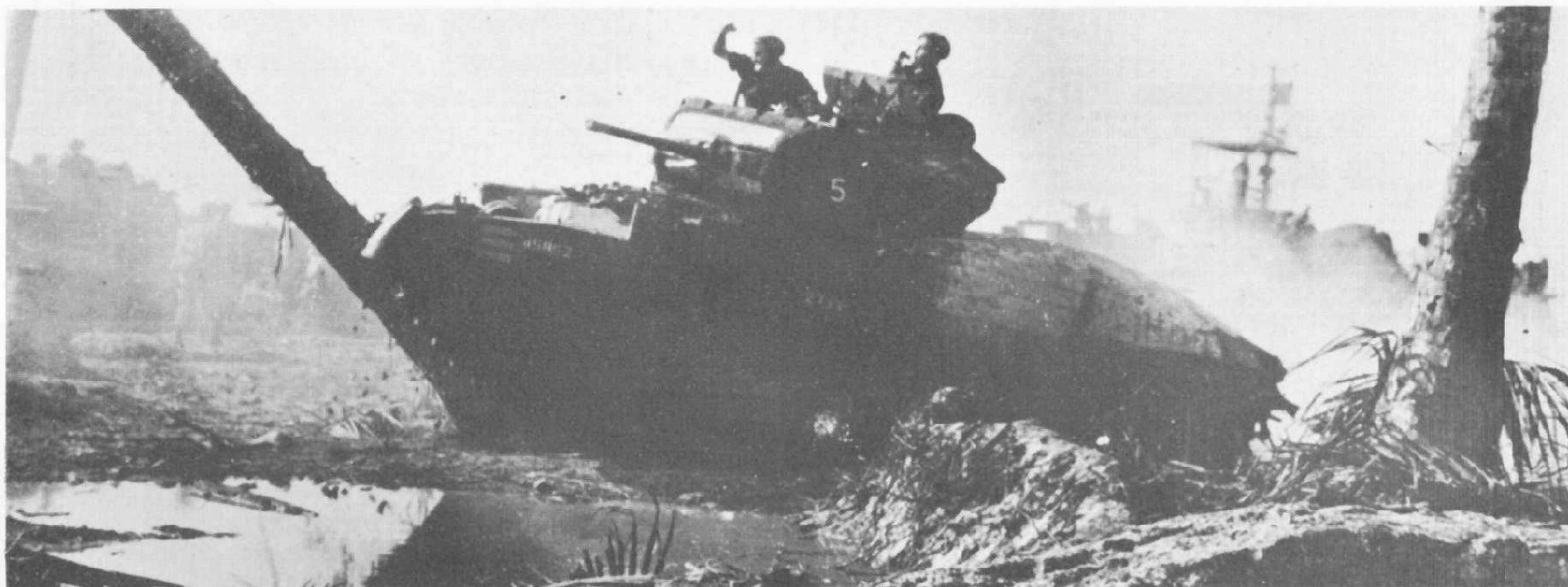
Knocking down a coconut palm after landing at Balikpapan, July 1945, where the tanks waded through 3 ft. 6 in. surf with ease. On this tank the canvas water-proofing screens over the gun mantlet and sides of the engine compartment have not yet been blown away.
