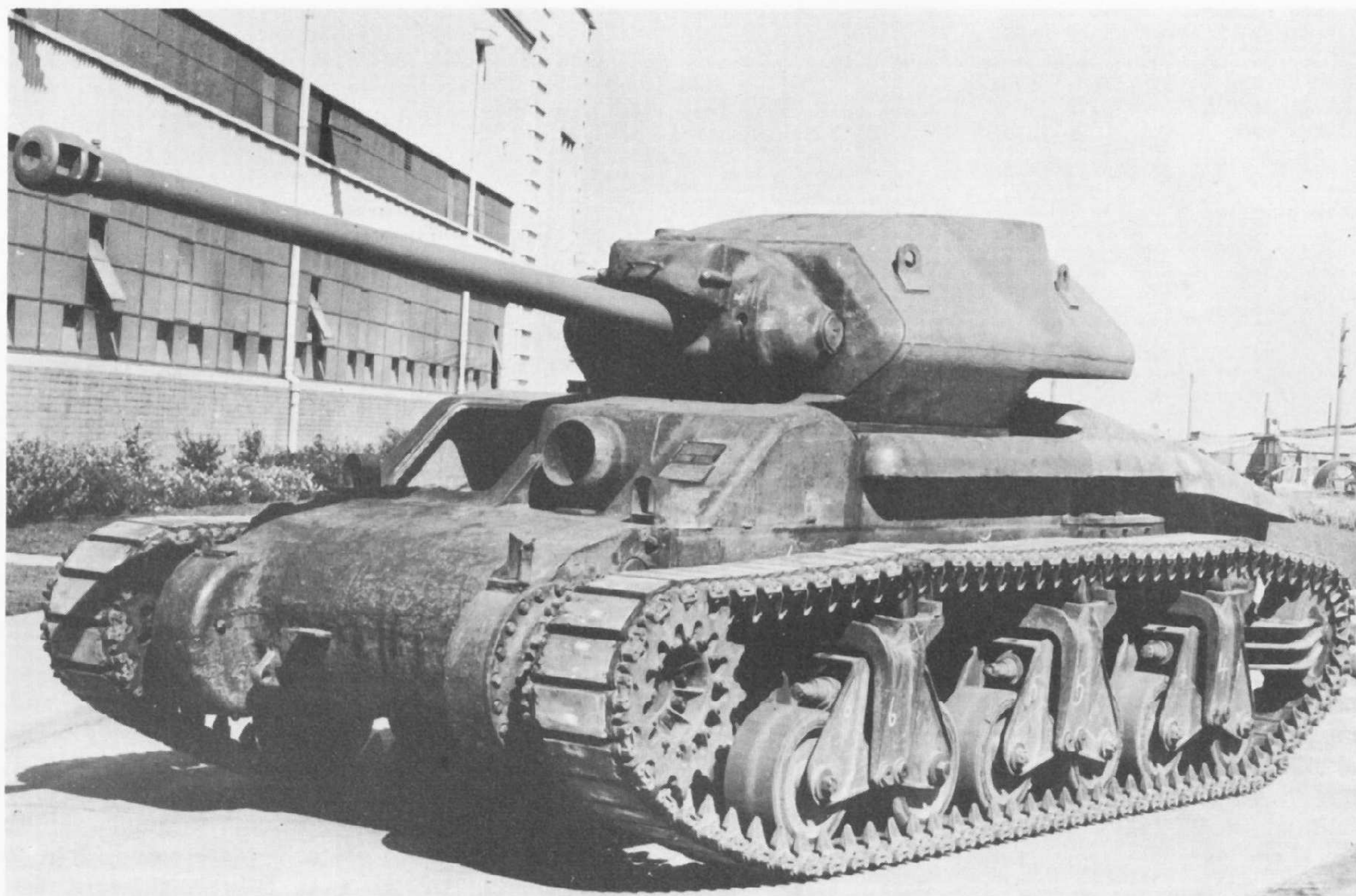
The 17-pdr. and turret mounted on an AC1 test vehicle.
