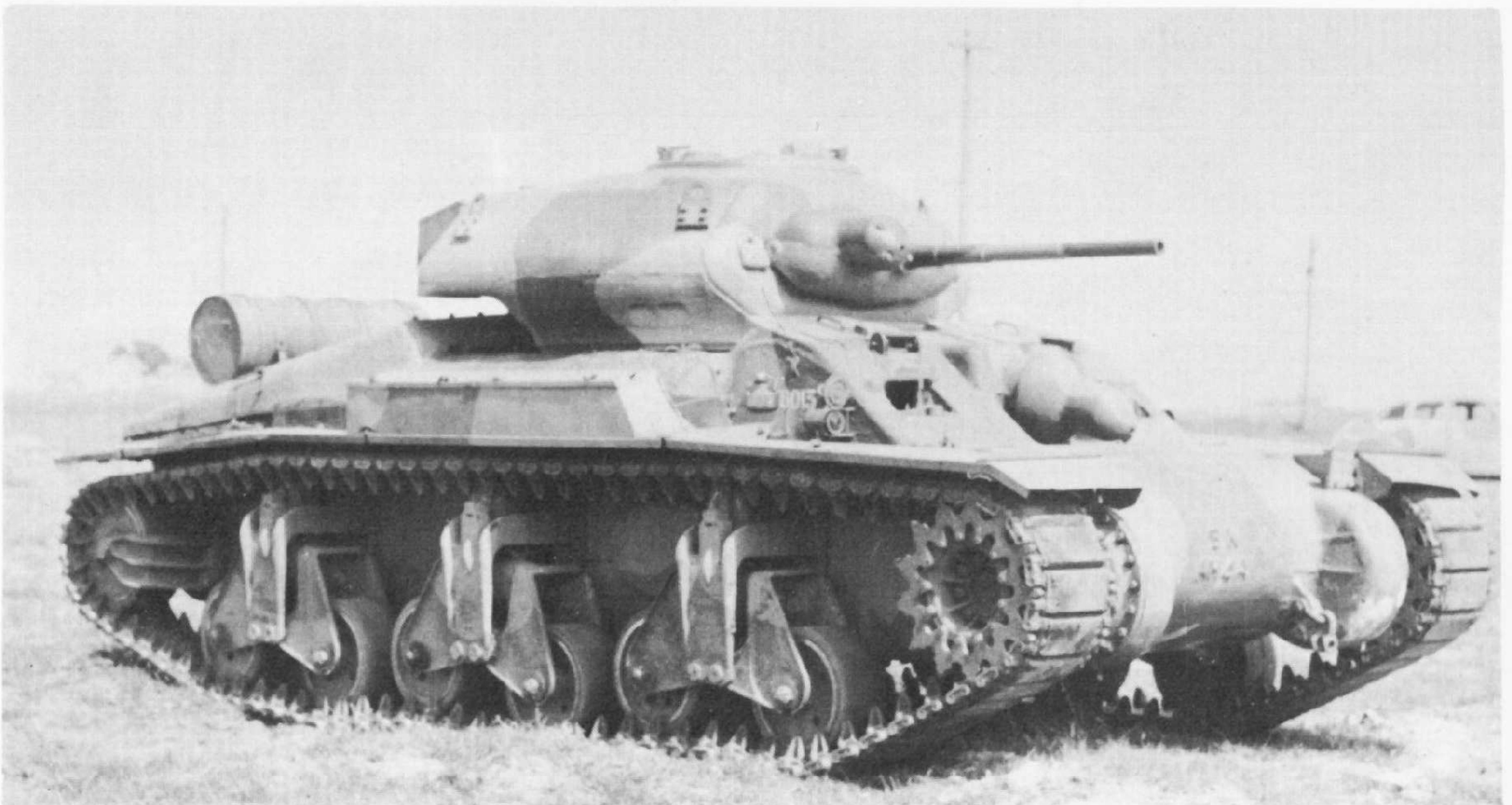
The Sentinel in camouflage paint, mounting a bin on the back of the turret and a jettison tank. (Photo: R.A.A.C. A.F.V. Museum)
