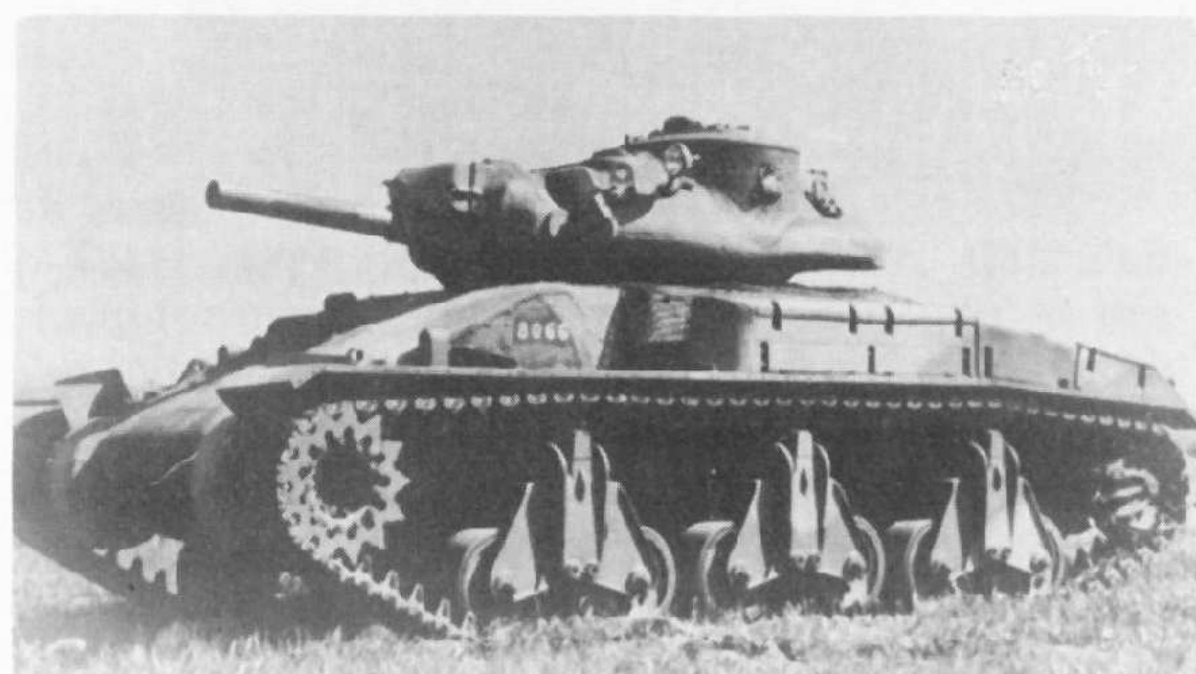
The AC3 mounting 25-pdr. and co-axial Vickers machine-gun. Note the difference from the AC1 in the new, sharply sloping hull front and the changed aspect of the hull top. (Photo: R.A.A.C. A.F.V. Museum)
