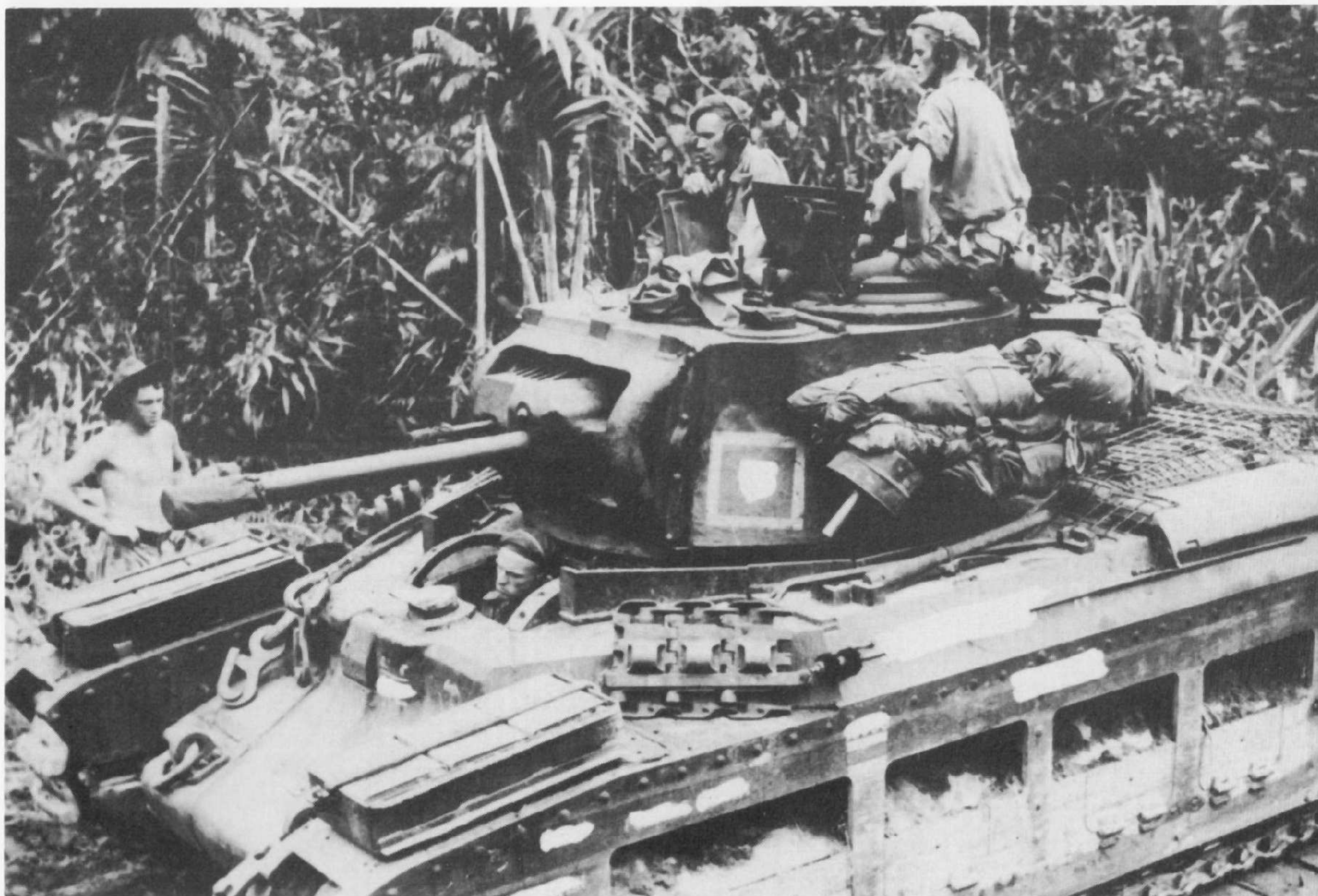
Special bridges had to be built to enable the tanks to move forward. The armoured shield to protect the turret ring, and the anti-magnetic mine screen over the engine louvres are fitted to this tank on Bougainville. (Photo: Australian War Memorial)
