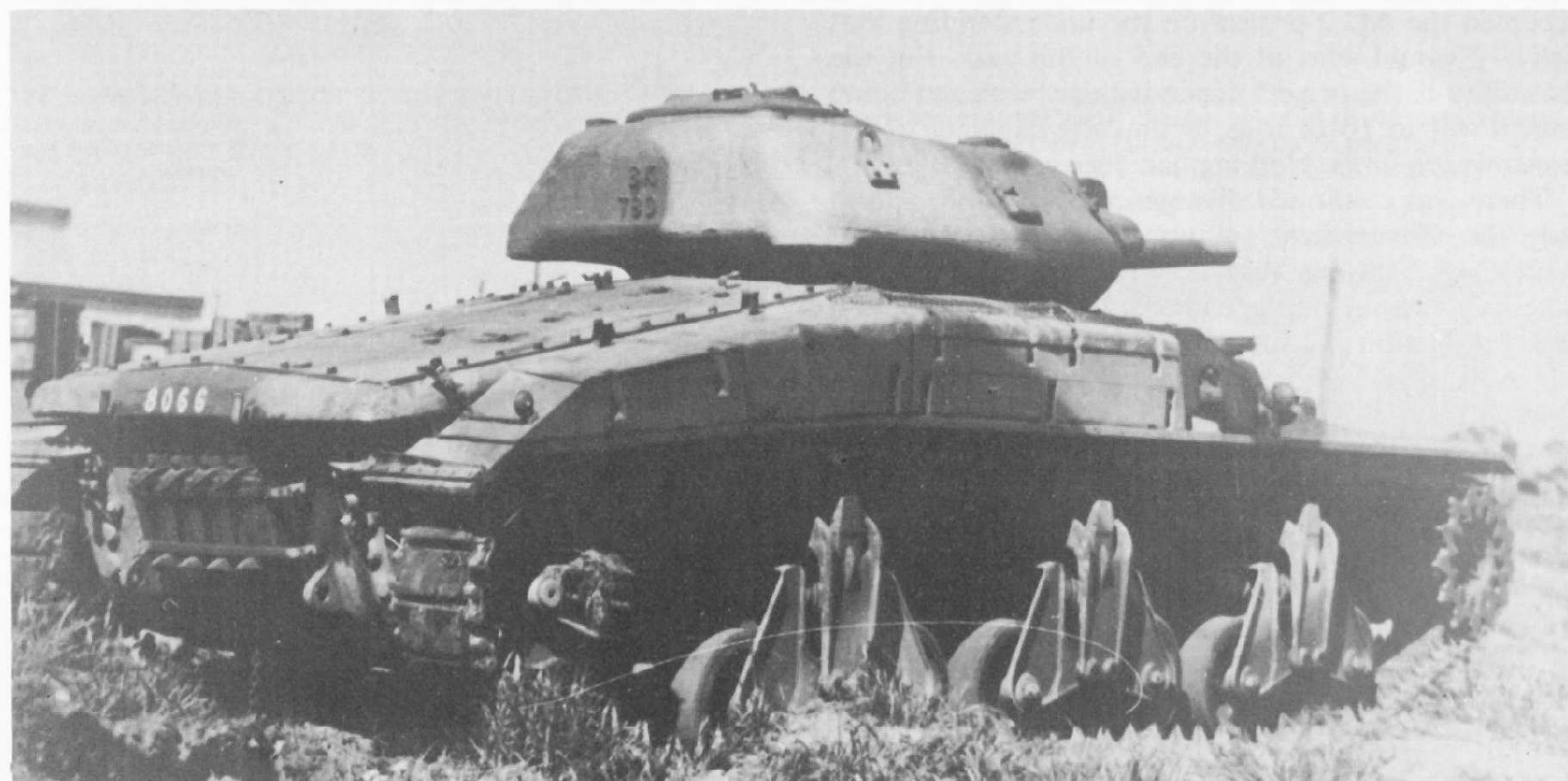
Rear view of AC3. The power unit cover plate on AC1 was similar, giving access to engines, radiators and fuel tanks through hatches. (Photo: R.A.A.C. A.F.V. Museum)
