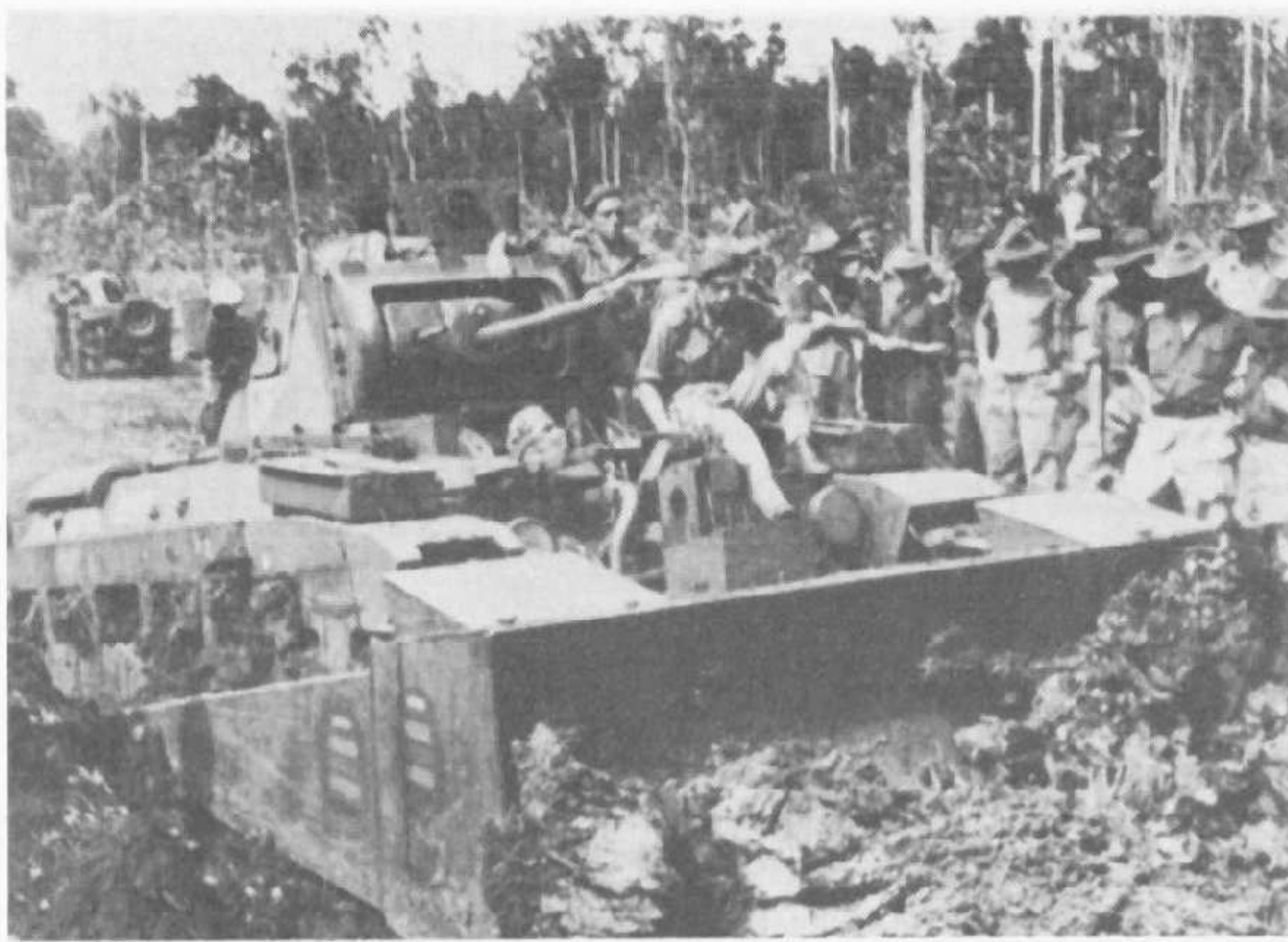
Matilda Dozer in use in New Guinea. This is an early version in which the blade is controlled by winch and cable mounted on the hull front. (Photo: Australian War Memorial)
