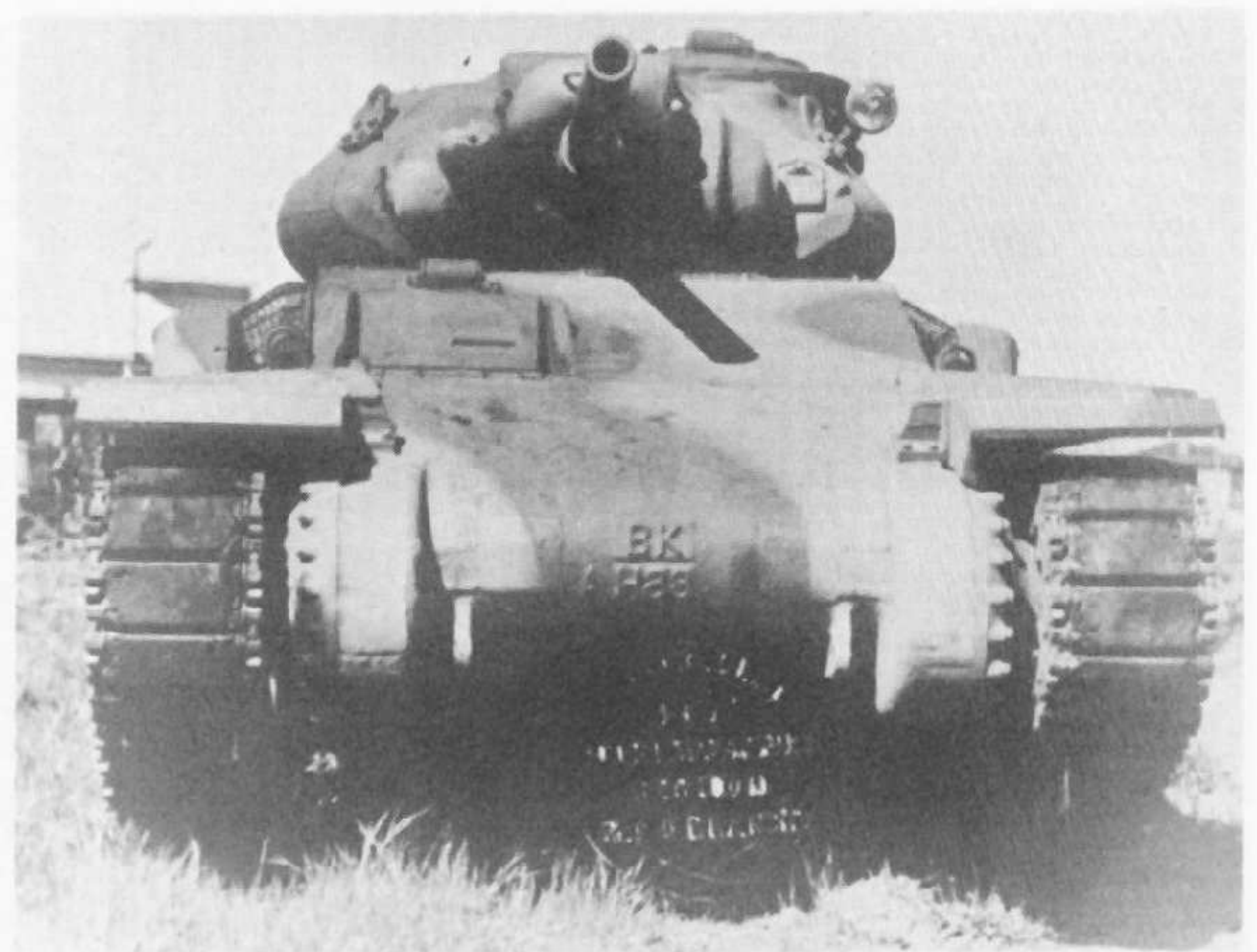
The AC3. The co-axial Vickers machine-gun was retained within an armoured shield beside the 25-pdr.
