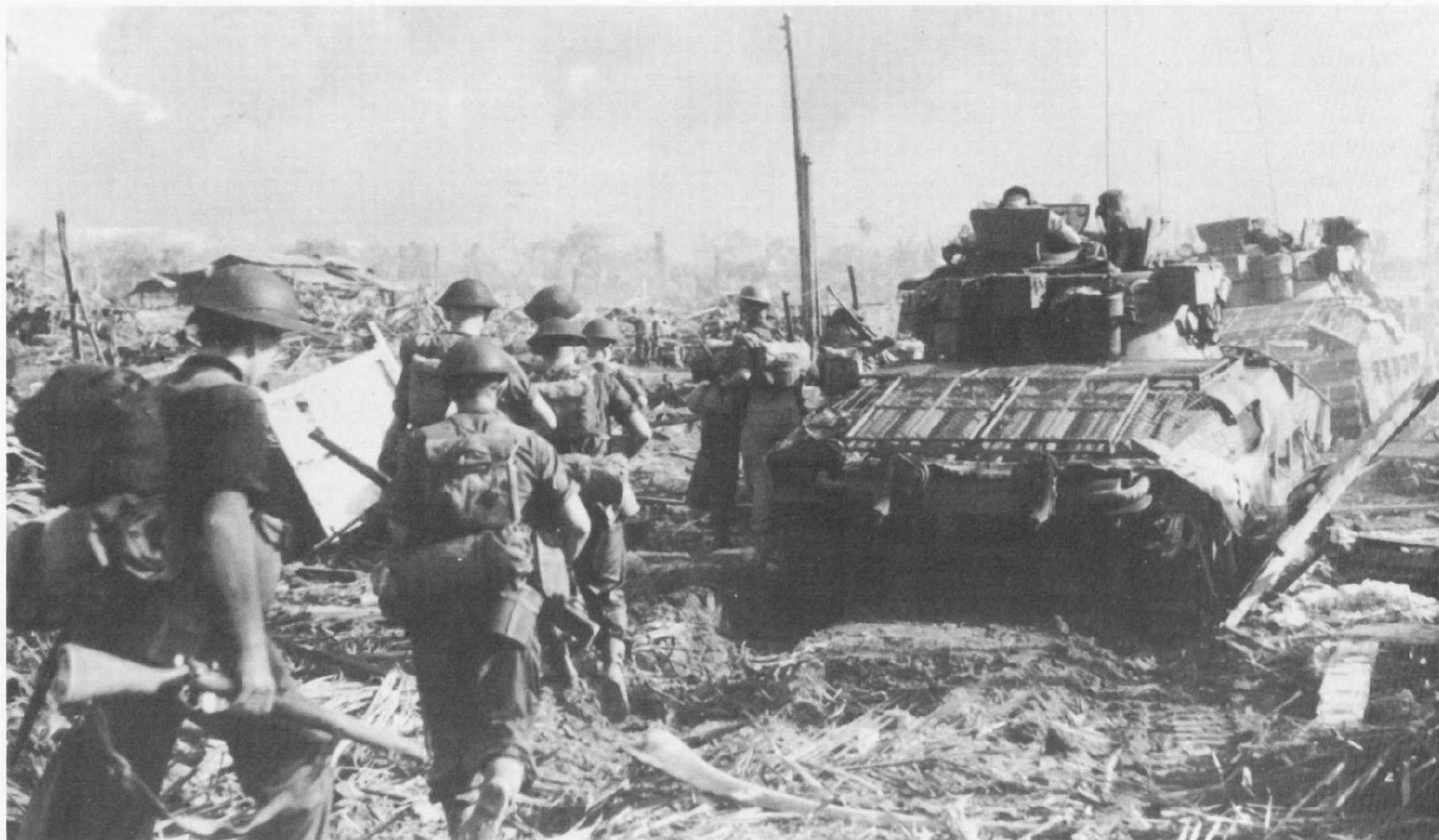
Tanks of 1st Armoured Regiment advancing inland at Balikpapan, July 1945. The wire mesh screen over engine louvres can be seen on the tank, as well as canvas water-proofing (already blown away) hanging from the side. (Photo: Australian War Memorial)
