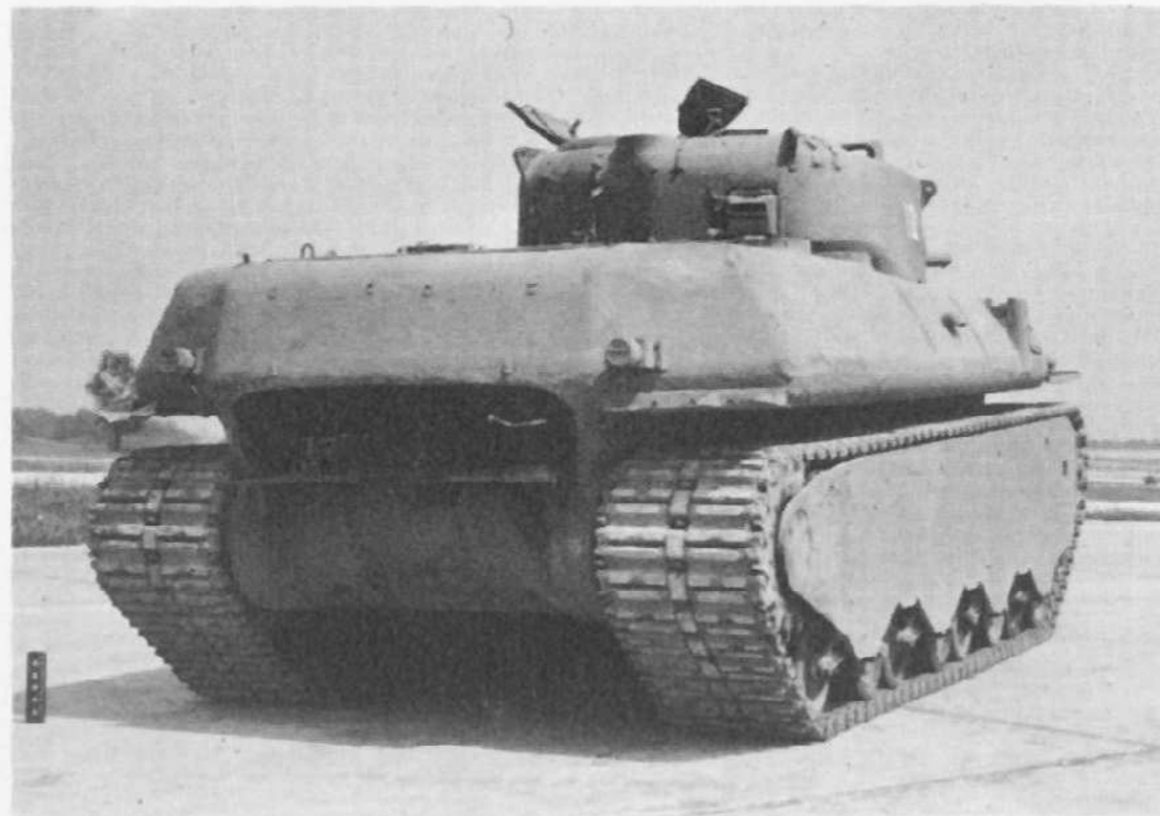
Rear view of the T1E1 illustrates its clean lines, rear turret protectoscope, and turret antenna base in the turret, which had no anti-aircraft gun or cupola. (U.S. Ordnance Department)
