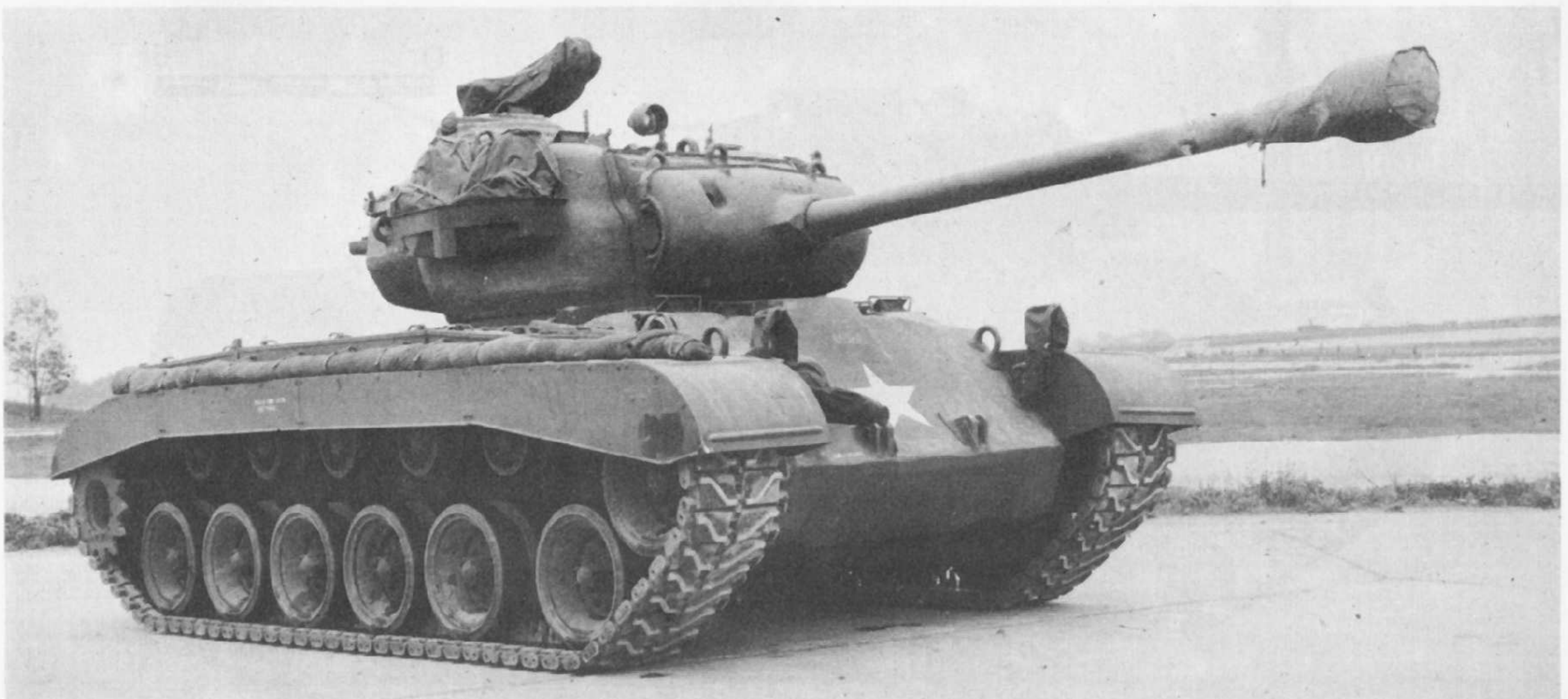
Three quarter right front view of T26E3 Medium tank showing canvas covers and tarpaulin and with T80E1 steel track.
