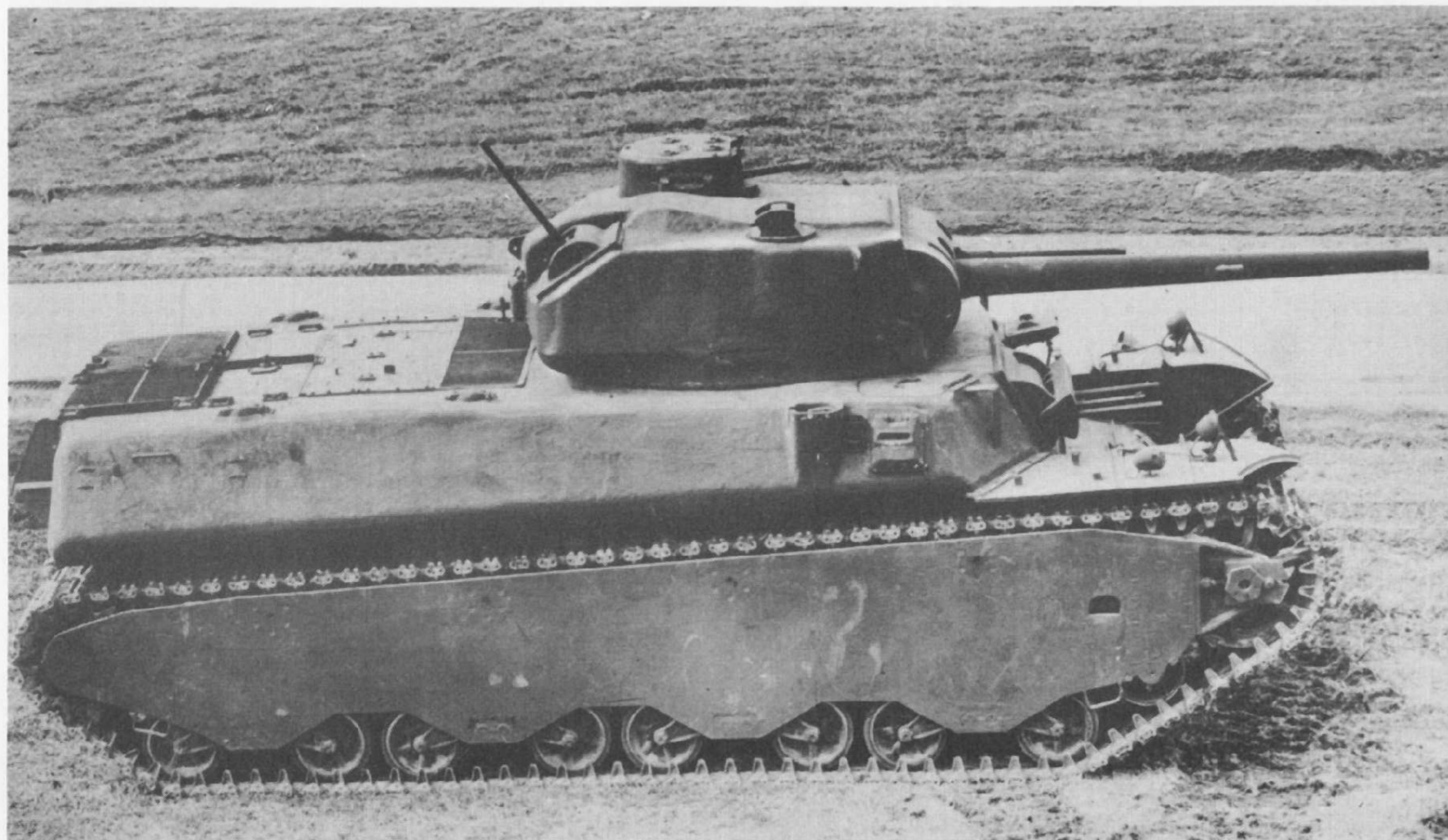
This view of the T1E2 or M6 clearly shows the cupola and turret machine-guns and the front plate mount for the bow machine-guns.
