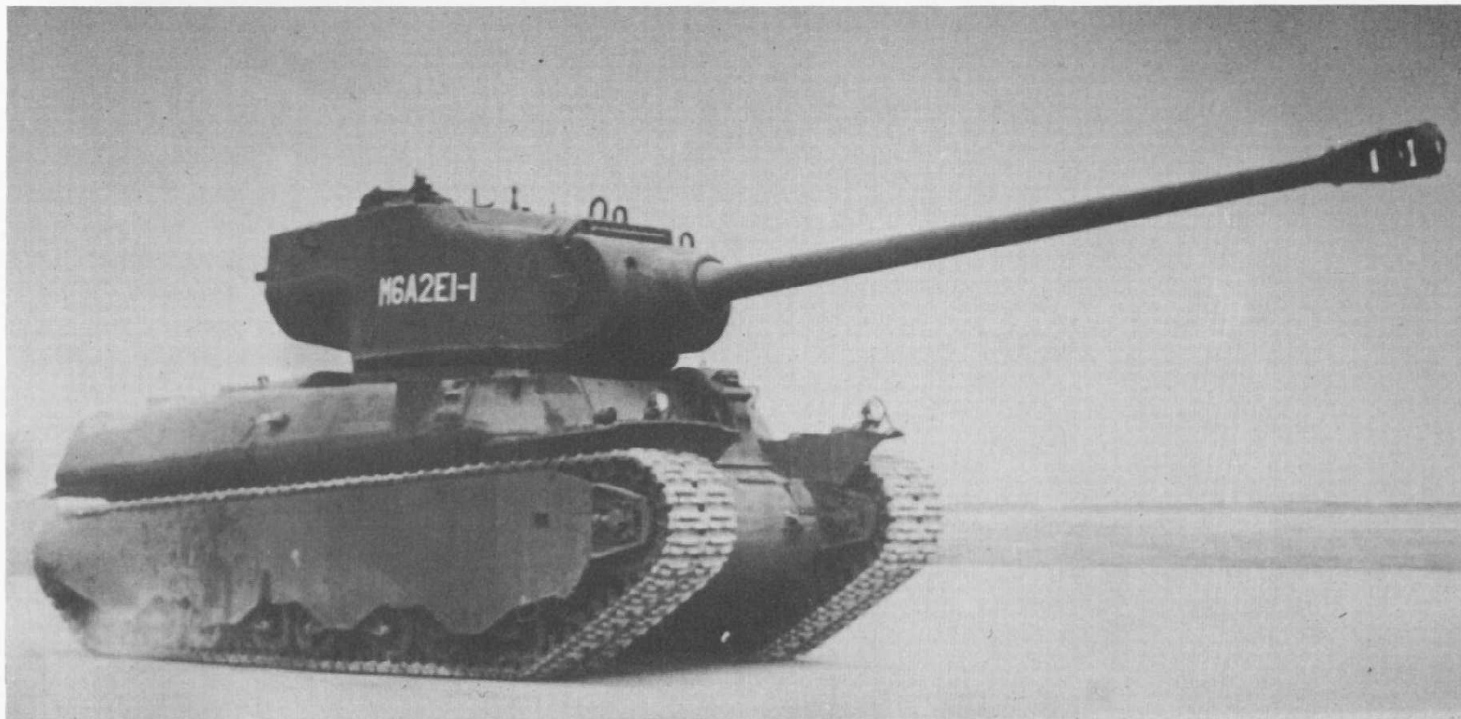
The M6A2E1 with its specially designed turret for the 105-mm gun became a somewhat massive vehicle.
