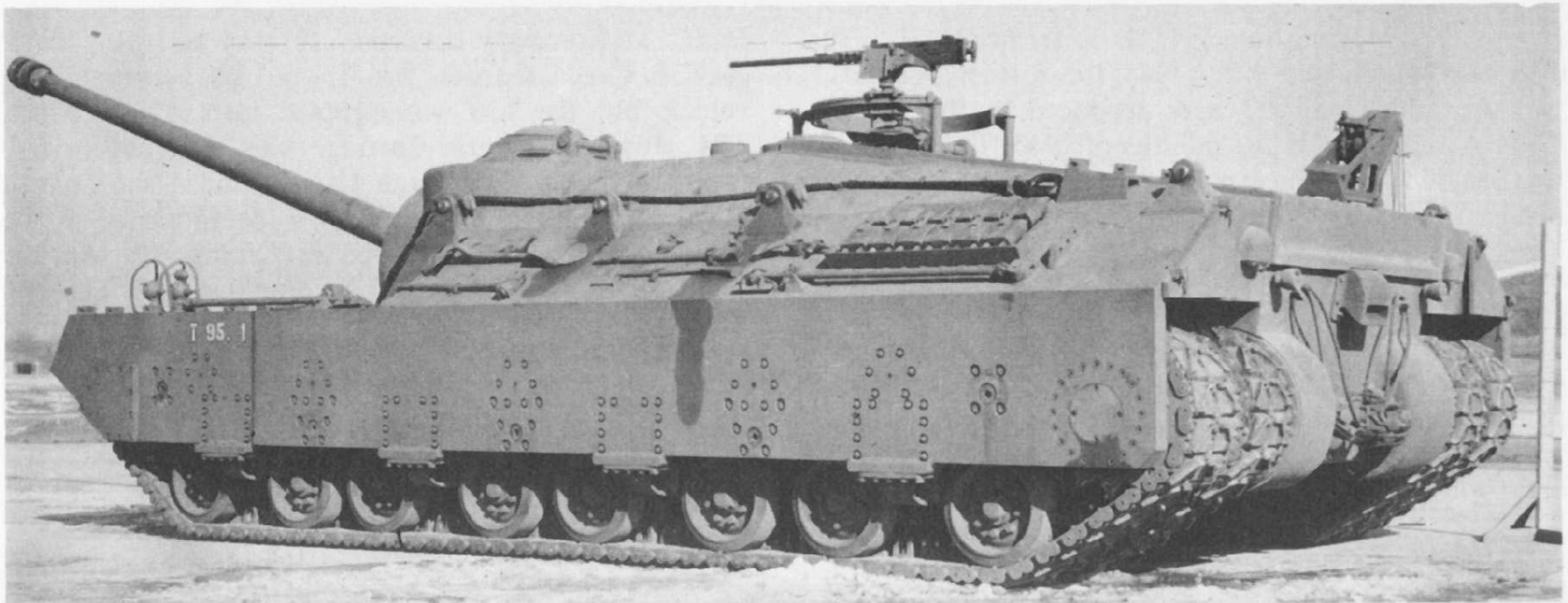
T95 Gun Motor Carriage which utilized many M26 tank components with track skirts and outer track sets removable for rail shipment. The T95 GMC was originally designated T28 Heavy Tank. (U.S. Ordnance Department)
