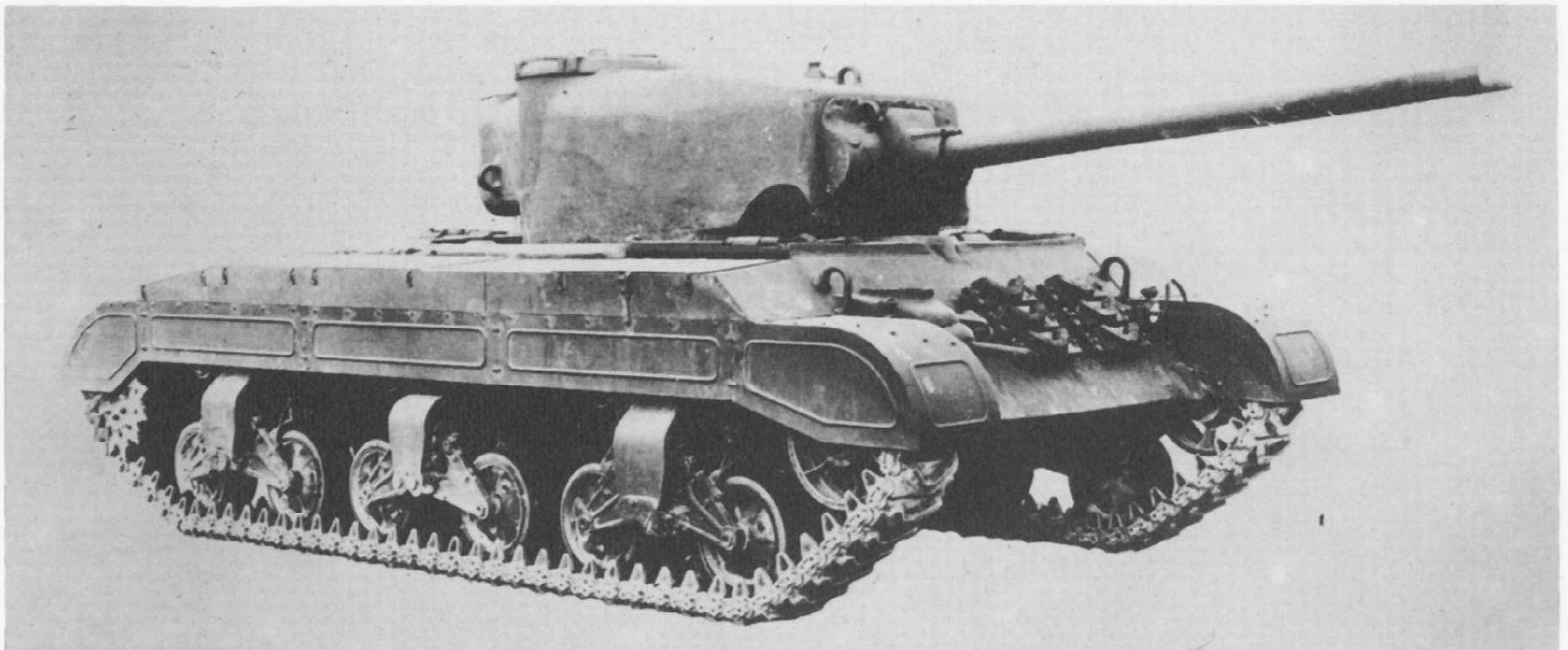
Medium Tank T22 equipped with early type of horizontal volute spring suspension and rubber chevron tracks.
