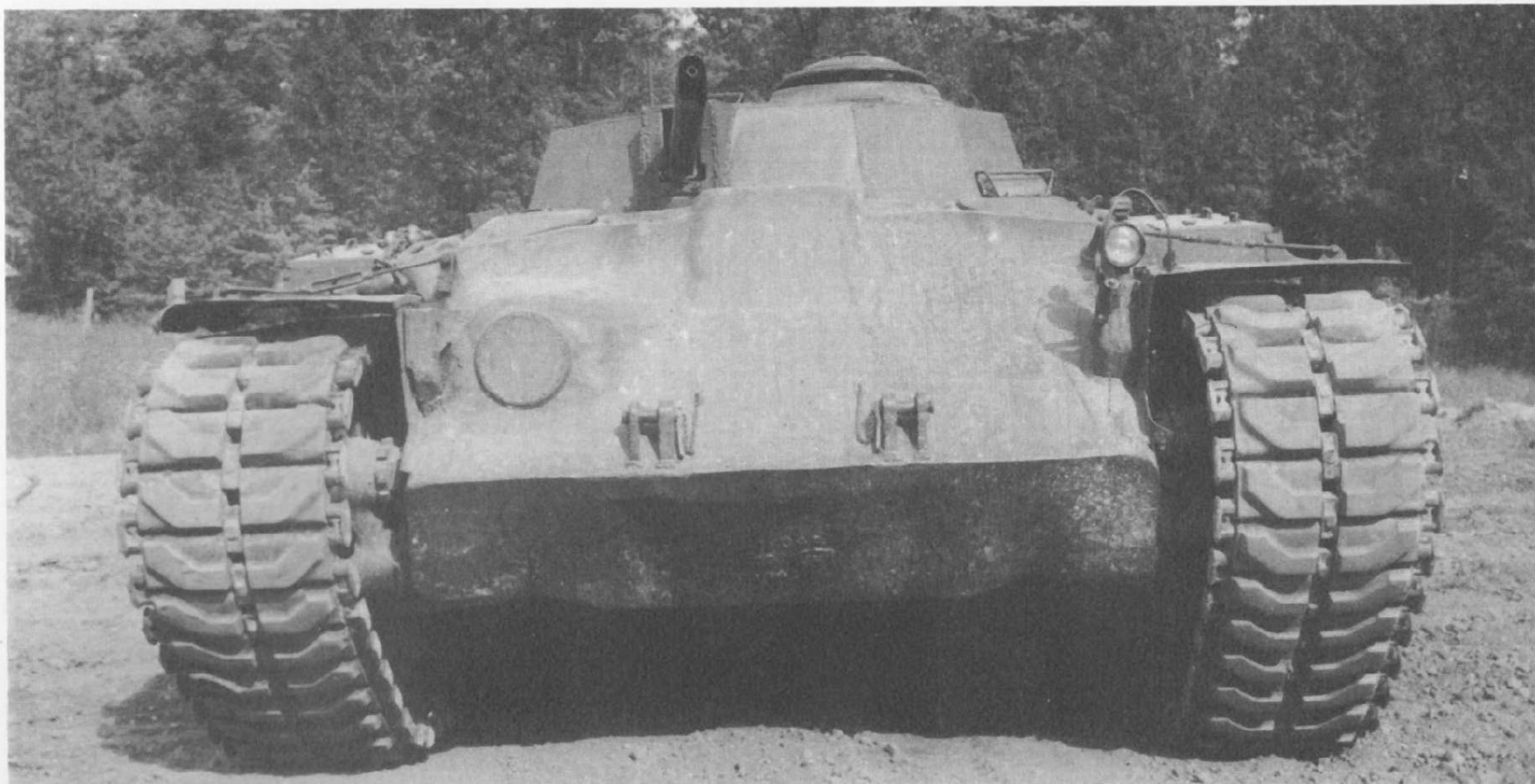
Canadian Iroquois flame gun in T35 Flame tank, a de-turreted M26 tank with special turret and T84E1 rubber tracks.
