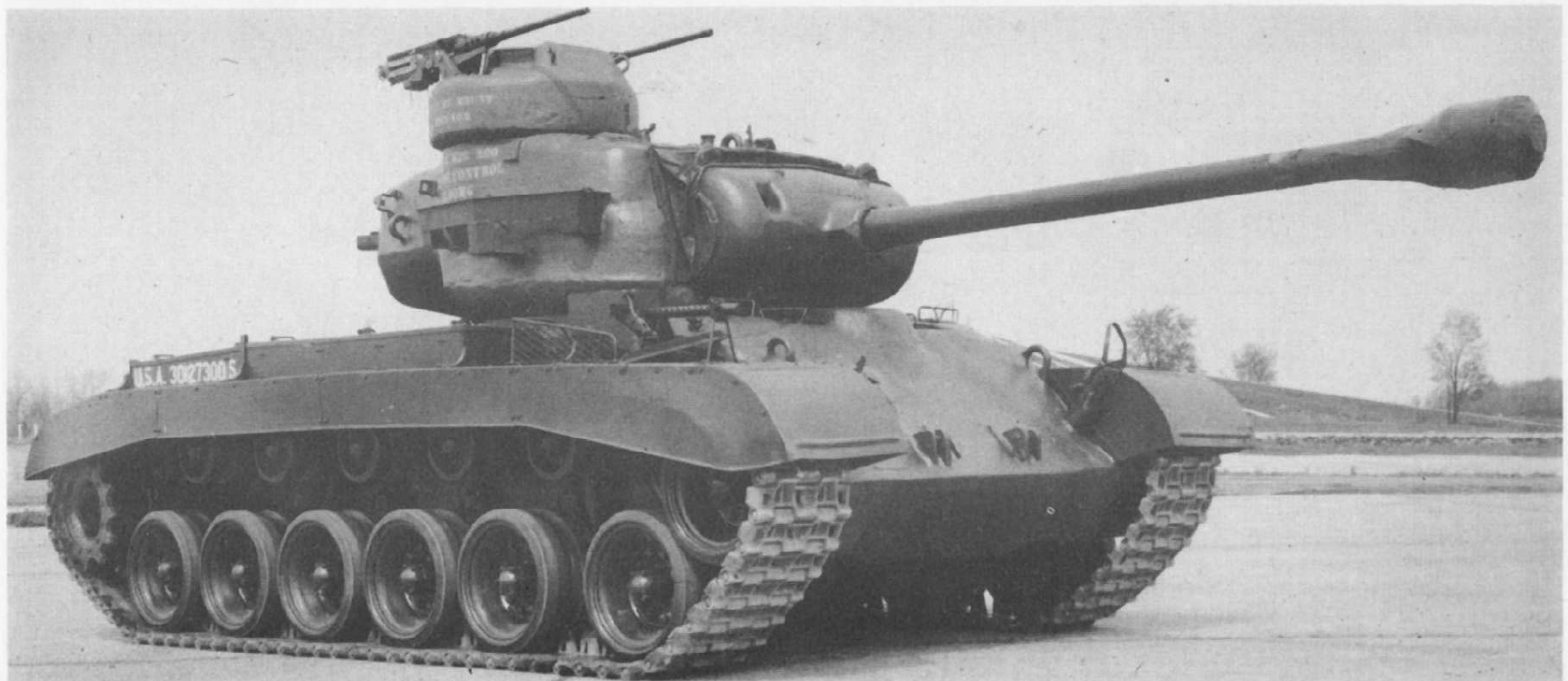
Experimental remote controlled machine-gun fender kit and experimental T121 remote controlled machine-gun cupola mounted on M26 Medium tank with T81 tracks. (U.S. Ordnance Department)
