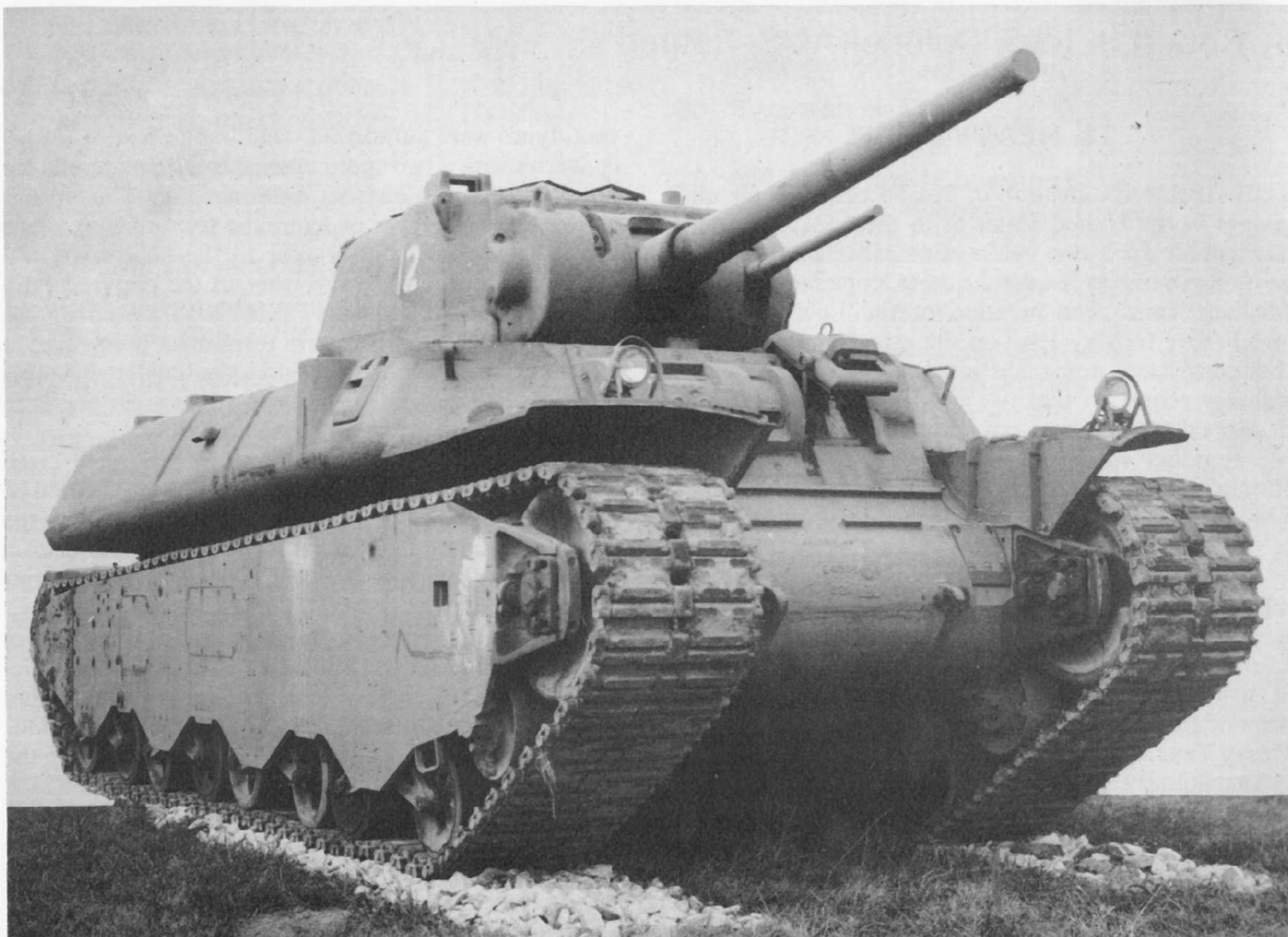
The T1E1 or M6A2 showing protectoscopes and radio antenna base on right side of hull.
