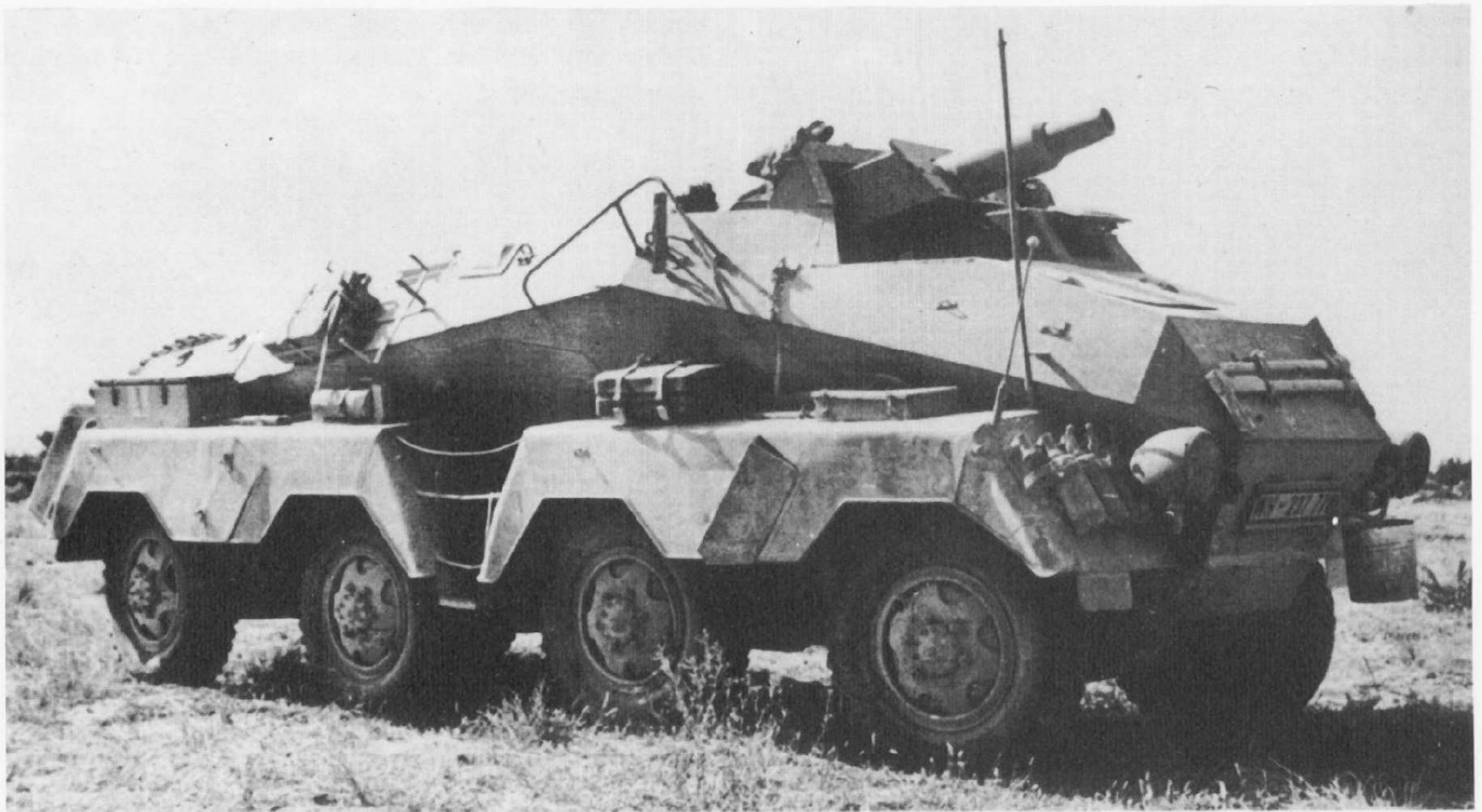
Schwerer Panzerspähwagen (8 Rad) Sd Kfz 233 had an open superstructure in which was mounted a 7.5 cm StuK (SturmKanone) L/24. The 233's assault gun was intended to provide supporting fire for the more lightly-armed 8 Rad 231 and 232 cars. (RAC Tank Museum)
