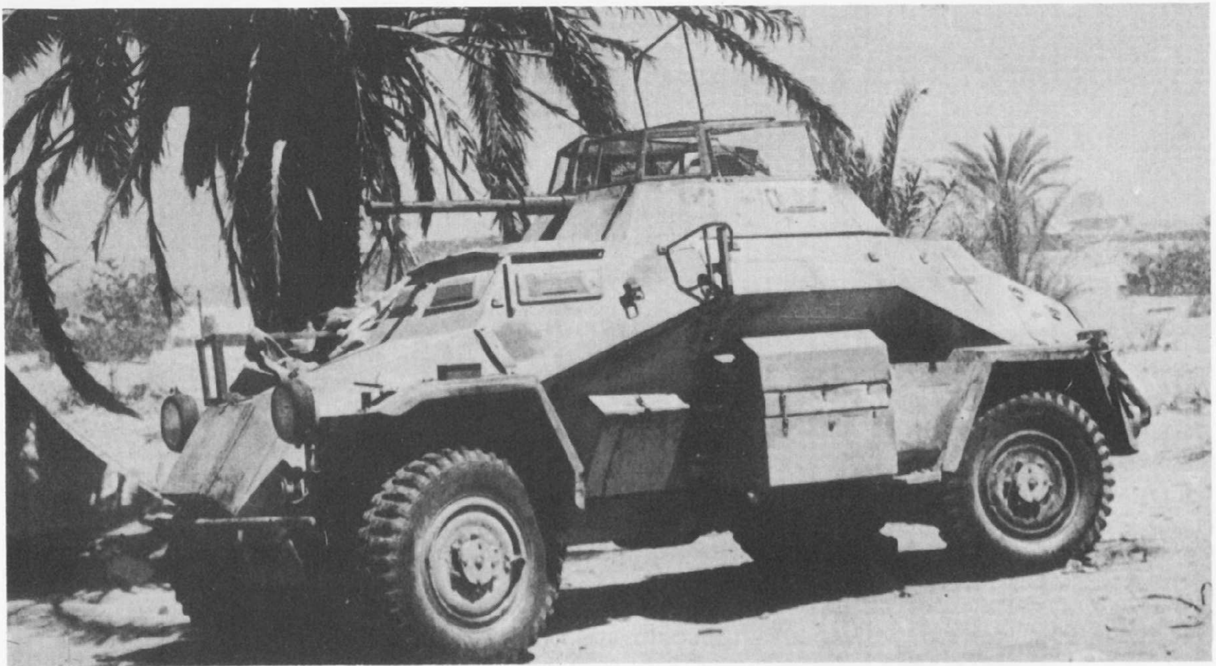
Leichter Panzerspähwagen Sd Kfz 222 in North Africa. The 222 had a 2 cm KwK (KraftwagenKanone) L/55 as its main armament, with a 7.92 mm coaxial machine-gun. Overhead protection in the turret was given by a hinged wire grille. (RAC Tank Museum)
