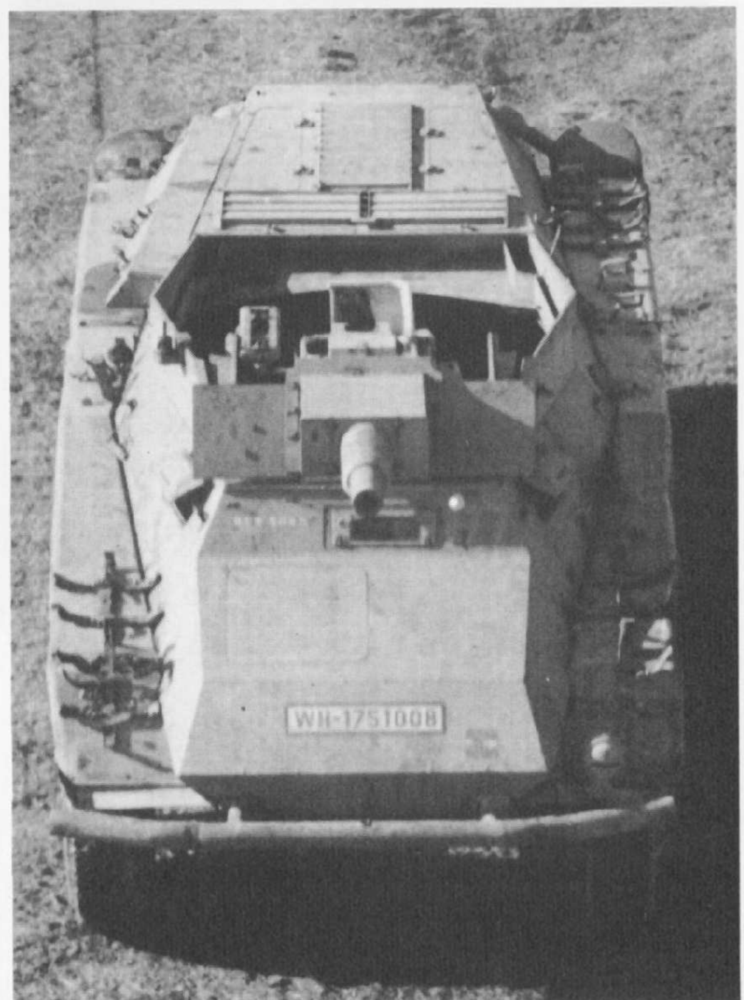
Schwerer Panzerspähwagen Sd Kfz 234/3 was a close support armoured car mounting a 7.5 cm StuK L/24 in an open body. (RAC Tank Museum)
