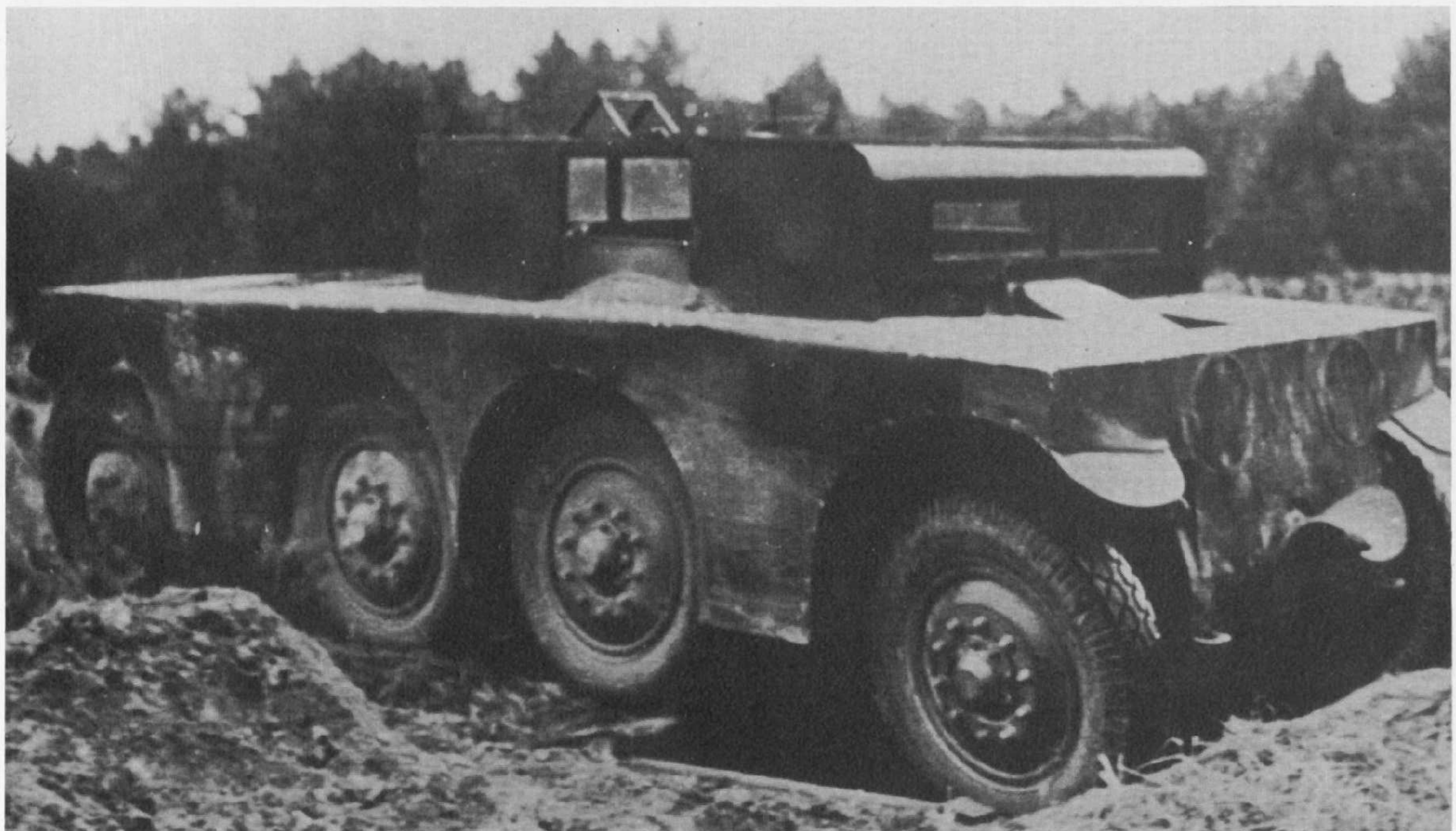
Three-quarter front view of the Daimler-Benz 8-wheeled ARW/MTW 1 (Achtradwagen/Mannschaftstransportwagen) during development. The vehicle, which was amphibious, had a chassis-less construction. (via RAC Tank Museum)
