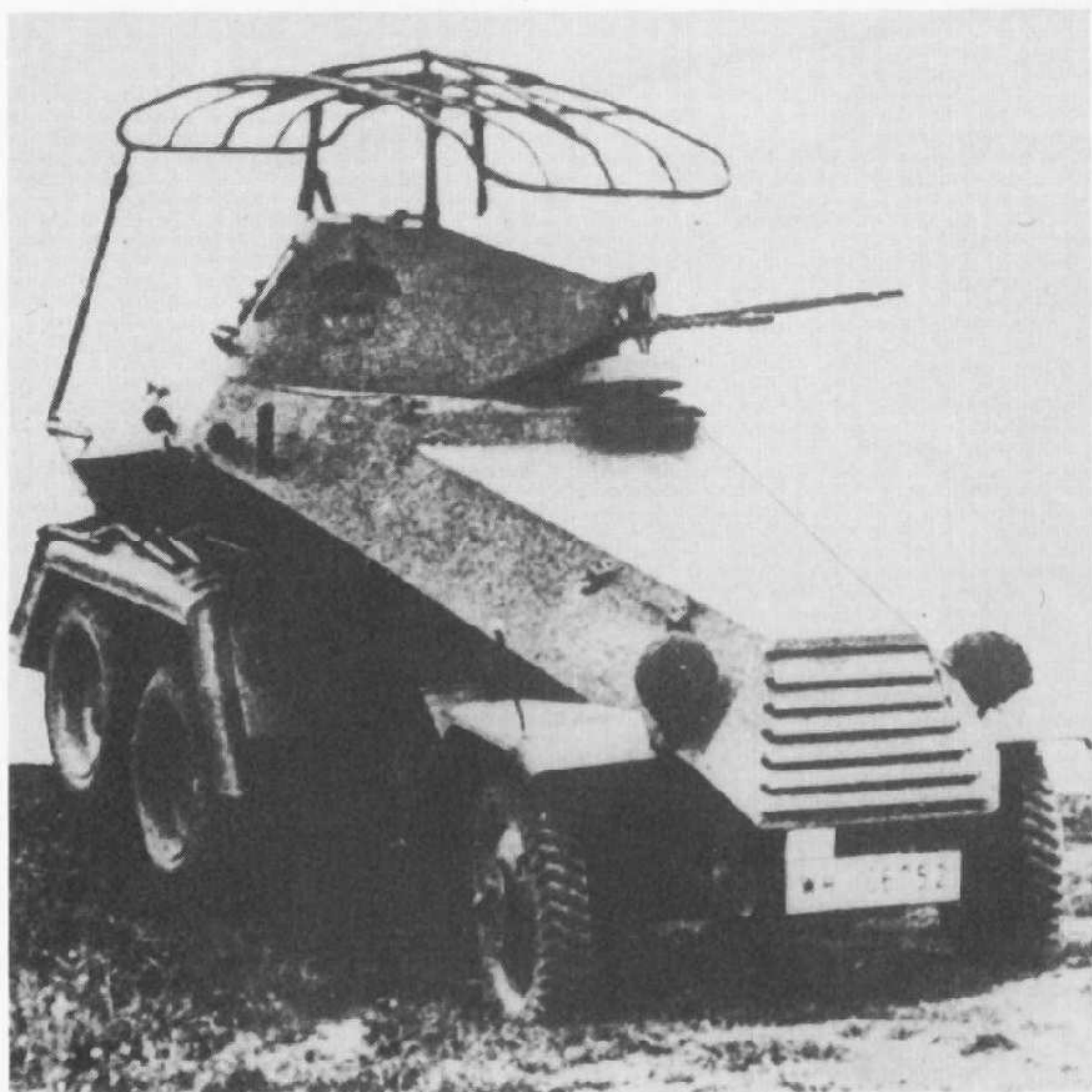
Schwerer Panzerspähwagen (6 Rad) Sd Kfz 232: the wireless-equipped version of the Sd Kfz 231, showing the turret swung beneath the frame aerial. (via RAC Tank Museum)
