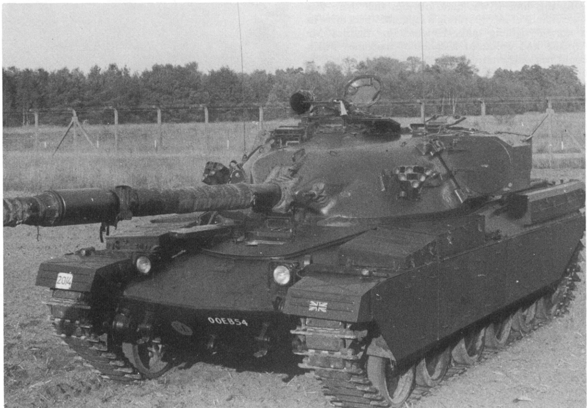
Chieftain with detachable rubber pads which reduce plate wear in tracks. (Photo: Profile Publications)
