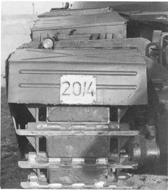
Close-up of Chieftain track with rubber pads for reducing plate wear. (Photo: Profile Publications)
