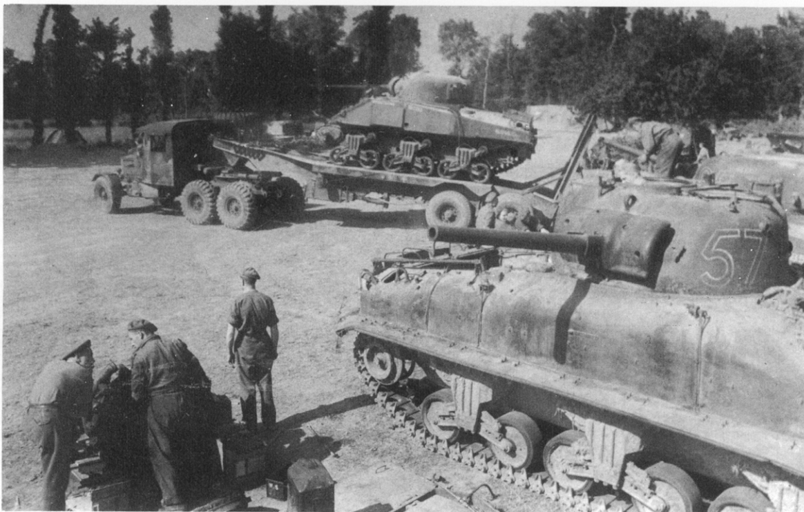
Scammell 30-ton Semi-Trailer Recovery Tank Transporter bringing a damaged Sherman into a R.E.M.E. tank repair workshop in Normandy, July 1944. Powered by a 6-cyl. Gardner engine with 6F and 1R gears, the tractor had a cab large enough for seven men. The two ramps were lowered by small hand winches to give a ramp angle of 18 degrees. Two hydraulic jacks support the rear of the semi-trailer during loading and can be used in wheel-changing and in detaching the semi-trailer from the tractor. (Photo: Scammell Lorries Ltd.)
