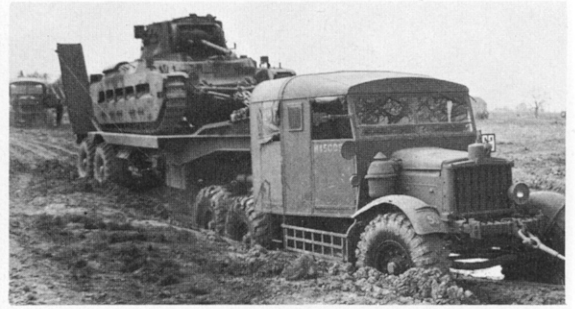
Scammell 30-ton Semi-Trailer Recovery Tank Transporter with Matilda on board. Length 49 ft. 8 in. (tractor and trailer with ramps raised). Width 8 ft. 7 in. (tractor), 9 ft. 5½ in. (semi-trailer). Height 10 ft. 11 in. (top of raised ramps), 9 ft. 5 in. (top of cab). Weight unladen 19 tons 18 cwt. gross, weight laden (with Matilda) 49 tons 16 cwt. gross. (Photo: Imperial War Museum)
