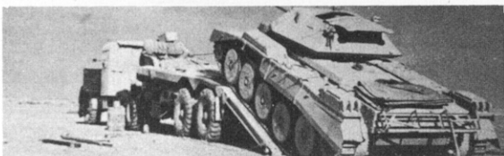
Crusader (Cruiser Tank Mark VI) on the ramps of a Scammell 30-ton Semi-Trailer Recovery Tank Transporter in the Western Desert.
