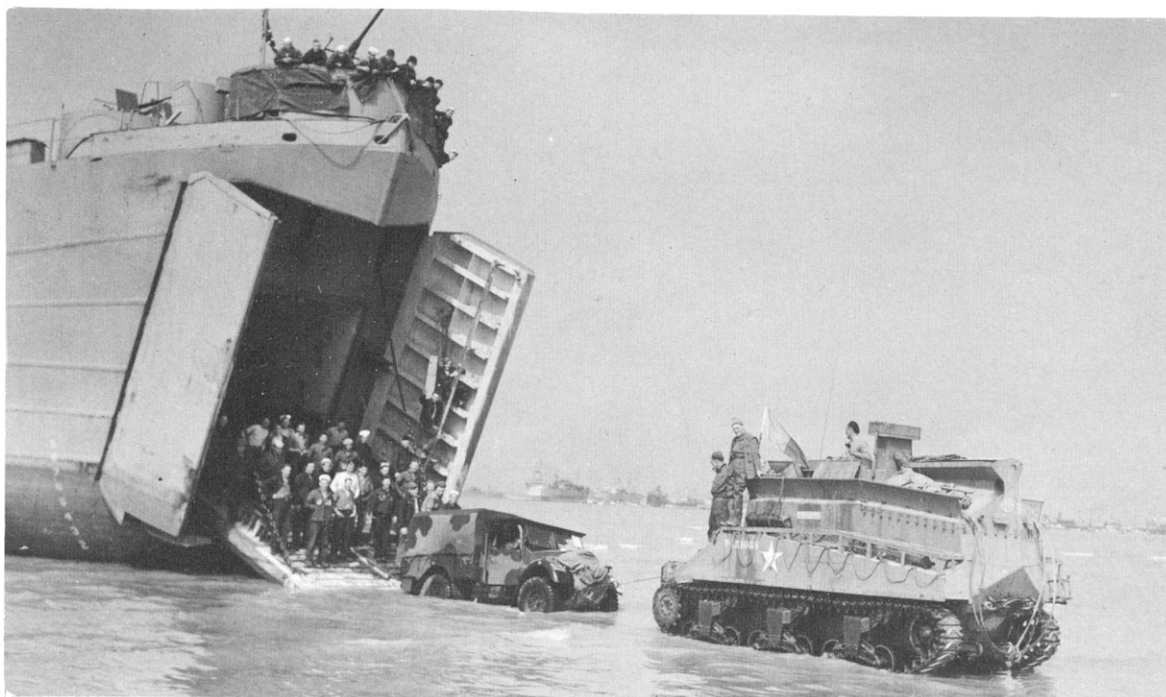
Sherman Beach Armoured Recovery Vehicle towing a truck ashore in Normandy, June 1944.
