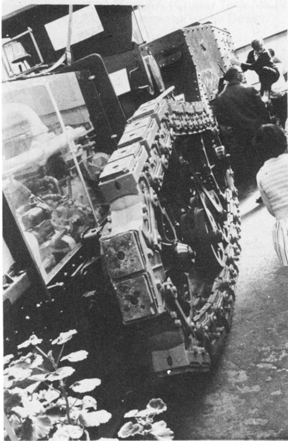
Very early type of track on a Ruston-Hornsby tractor, dating from before World War 1 now in the Royal Armoured Corps Tank Museum, Bovington. (Photo: Duncan Crow)
