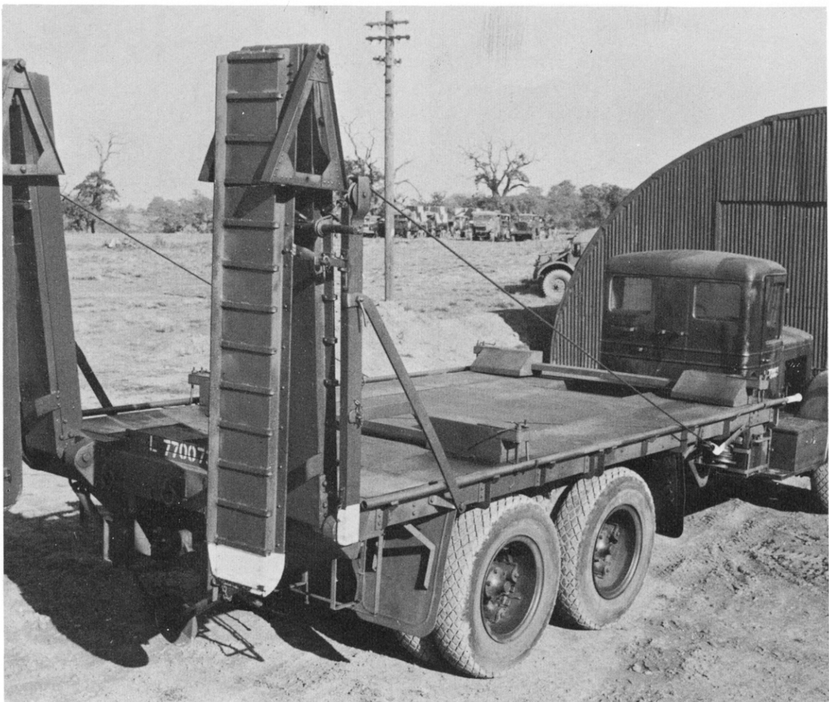
Mack "EXBX" 18-ton Tank Transporter (W.D. No. L770073). Weight unladen 11 tons 1 cwt. gross, weight laden 29 tons 10 cwt. gross (18 ton tank). (Photo: Imperial War Museum)
