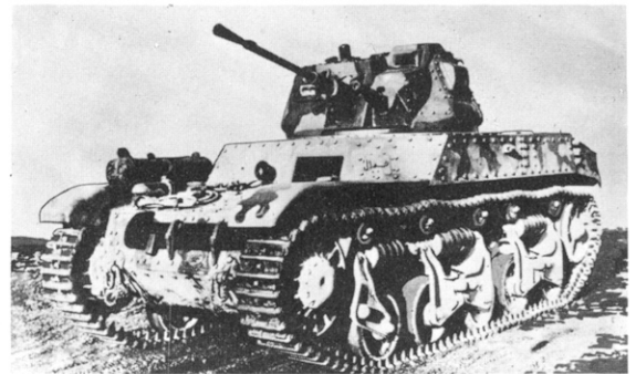
The A.M.C. Renault 35 ACG 1 appeared in two forms, differing only in the armament; here shown with the 25mm gun and 7.5mm machine-gun.
