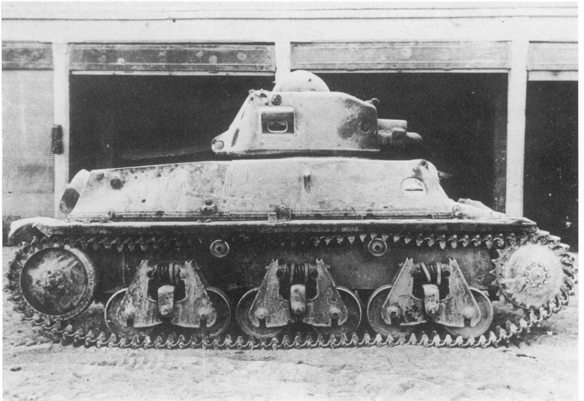
Hotchkiss H39, still mounting the short-barrelled 1918 model 37mm gun, but distinguished from the H35 by the almost horizontal engine deck, caused by the fitting of a larger engine.
