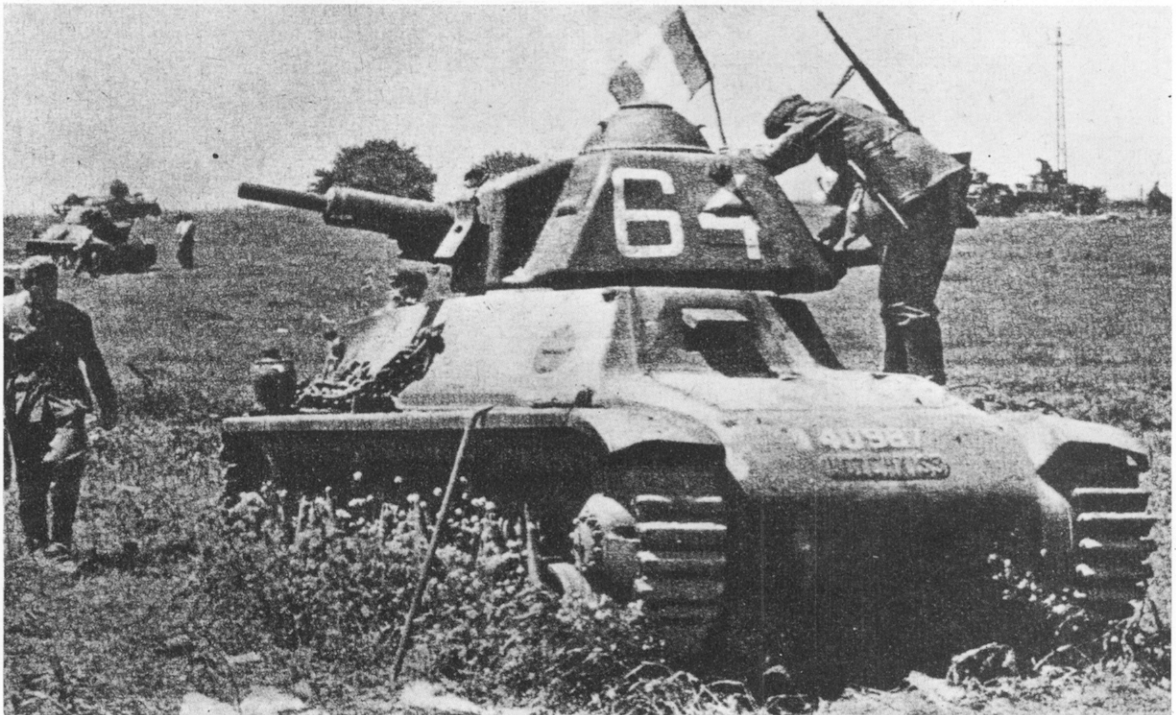
A captured H39 with long-barrelled 37mm gun in 1940. Note the vision slits in the turret in place of the earlier periscopic binoculars.
