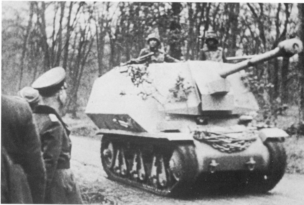
The H39 hull was used in a German conversion for a self-propelled 75mm anti-tank gun, known as the 7.5 cm PaK 40 L/48 auf Gw 39H (f) : 24 of these conversions were made.
