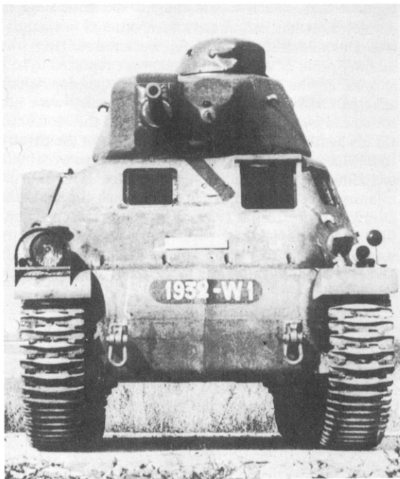
A prototype SOMUA S35 with the early, short pitch track plates. This picture shows how vision devices were mounted in separate frames inserted into the cast armour. Containers for stowage were sometimes strapped to the right side of the hull.
