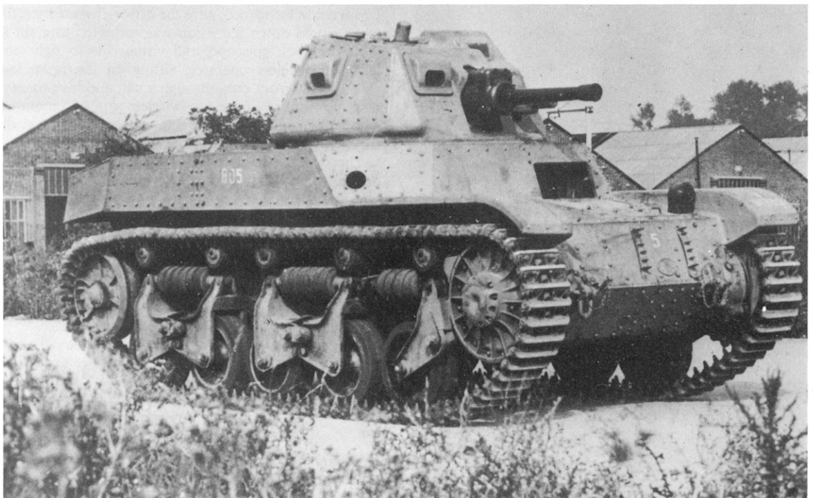
The suspension of the A.M.C. Renault 35 ACG 1 was similar to that of the Renault R35, but with five top rollers. Note the monocular periscope in the turret roof.
