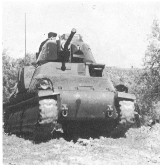
SOMUA S35 detail 6: the rear of the tank with its projecting towing hook. (RAC Tank Museum)
