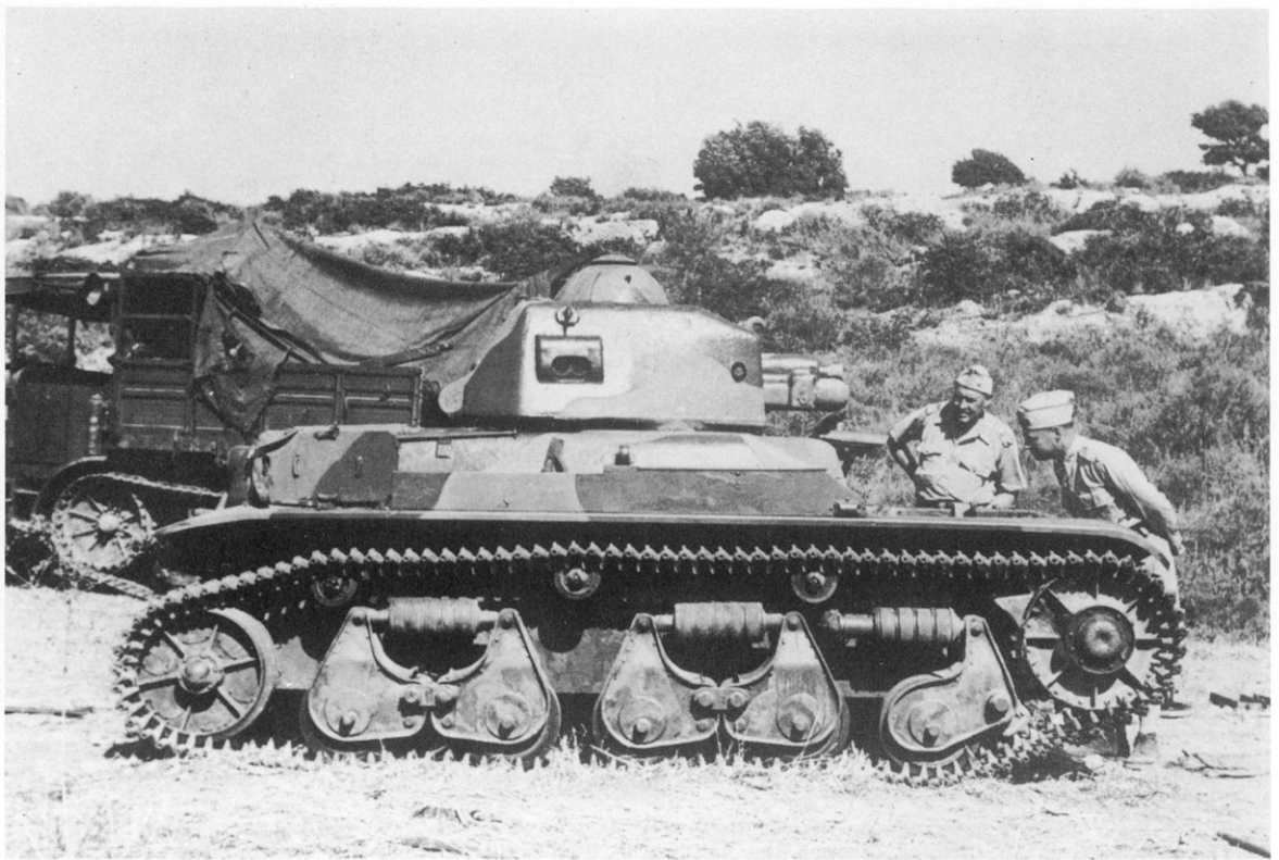
Renault R35, captured in Syria in 1941, being examined by American armour specialists. The R35 was of similar general shape to the H39 but distinguished chiefly by the suspension—five wheels compared with six.
