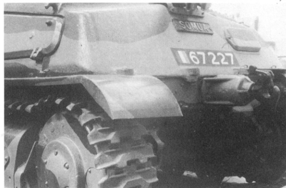
SOMUA S35 detail 6: the rear of the tank with its projecting towing hook. (RAC Tank Museum)
