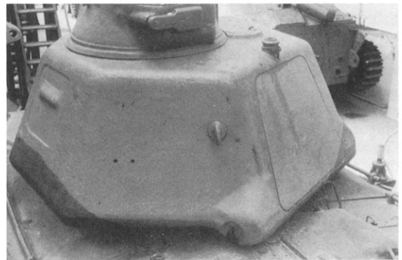
SOMUA S35 detail 2: APX 4 turret on the S35. Note the separate gun mantlets, with aperture for telescopic sight above the machine-gun; also the small blade vane sight in front of the cupola. (RAC Tank Museum)
