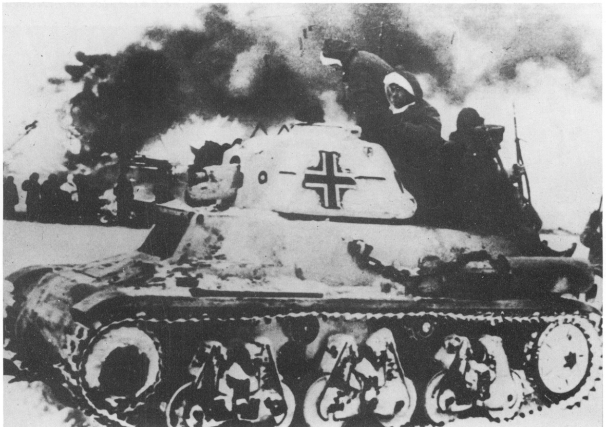
H39, still with short 37mm gun, in German service carrying infantry during winter operations.
