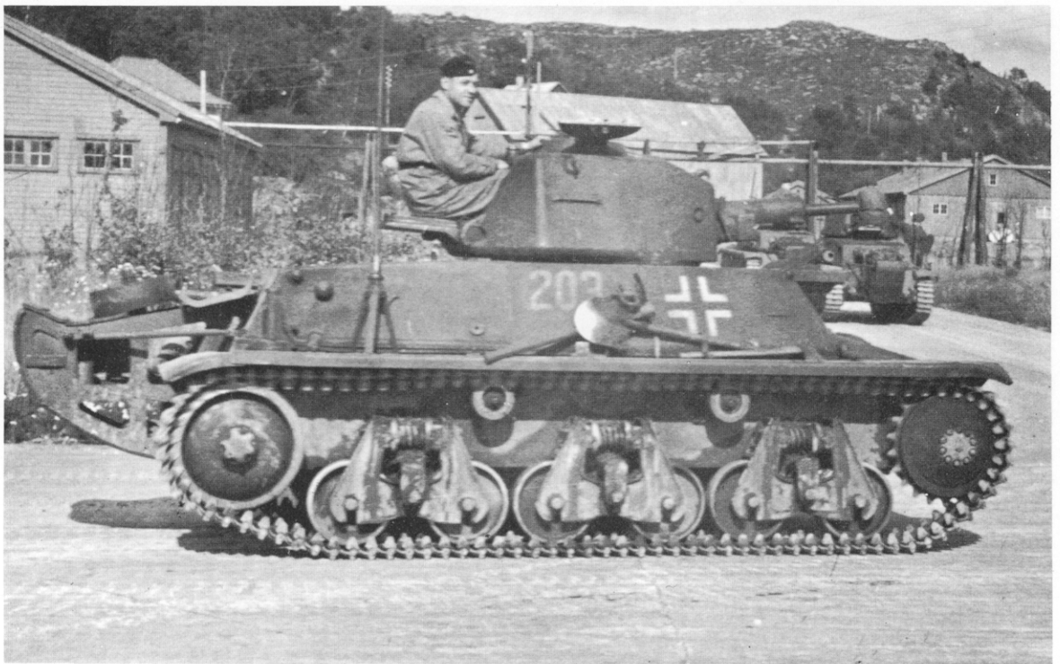
Another German modification on the H39 was the installation of a wireless set. Seen here is the aerial mounted in its base on the track guard. Note also the skid tail and the tank commander seated in a comfortable travelling position.
