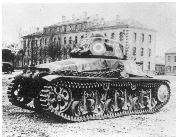
Abandoned in 1940, an H35. Note the commander's door at the rear of the turret, and the protrusions on the turret side to protect the periscopic binoculars.
