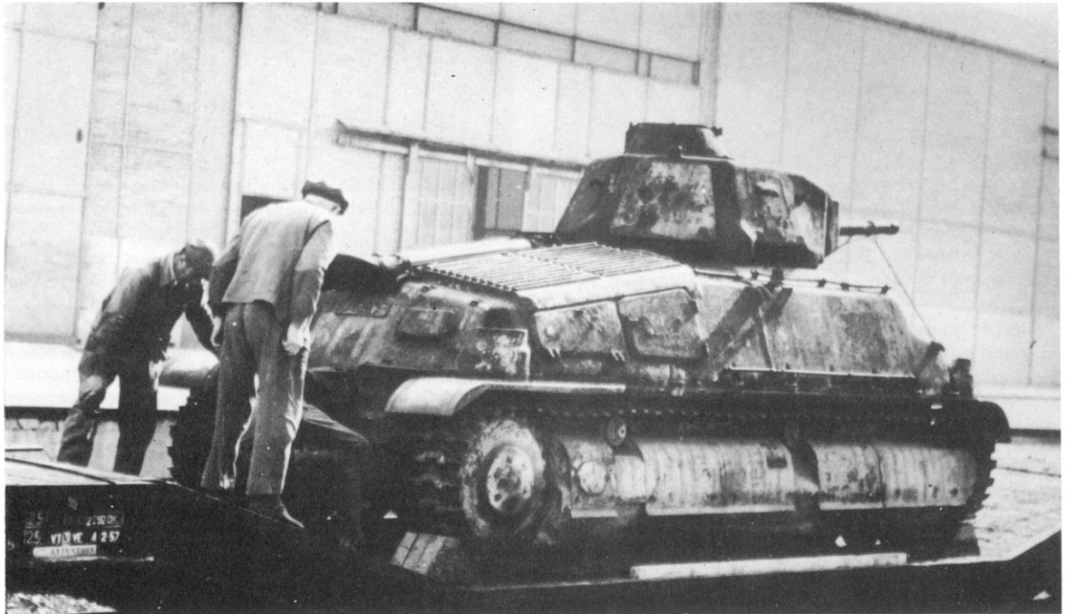
SOMUA S35. Note the round aerial base platforms moulded into the superstructure at the right front and rear corners; also, the additional aerial base bracket beside the turret; and the flat-topped cupola.
