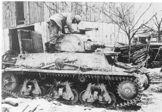
Re-captured—an American soldier examining an H39 with German markings taken during the winter 1944–45. This tank has the long-barrelled 37mm gun. Note the Panzerfaust projectile stowed on the hull side.
