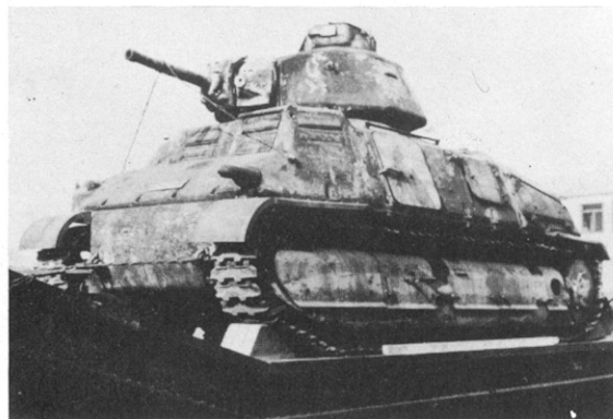
Three-quarter left front view of the SOMUA S35. The suspension was protected by armour plate; the curved, upper plates were hinged at the top and could be raised for access.
