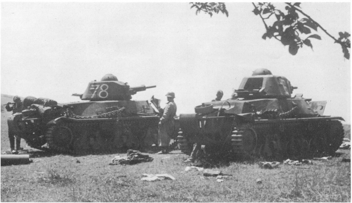
The H39 with detachable skid tail fitted to improve cross-country performance. An external fuel tank could be carried here on the tray in front of the spare bogie wheel.
