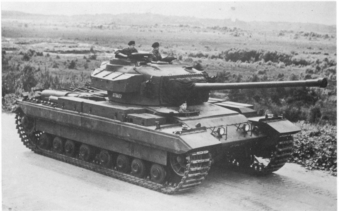
An FV 221 Caernarvon mounting a Centurion turret. The basic similarity to A45 is apparent. The tracks of this vehicle are untypically slack.
