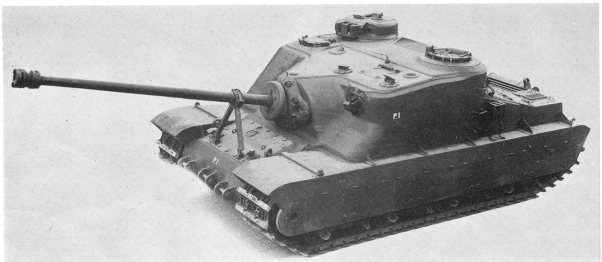
The first pilot model of the A39 Tortoise. Secondary armament was three Besa 7.92 mm. machine-guns, two in an independent turret on the roof for AA defence and the third to the left of the 32-pdr. The Besas are not mounted in this picture but their locations can be seen. Tortoise's huge superstructure was cast in one piece and its armour thickness was proof against any known German anti-tank gun of the period. It had a crew of seven.
