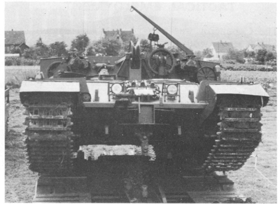
Front view of FV 219 ARV Mark 1 driving on to a transporter. Note driver's three periscopes as in Conqueror 1.
