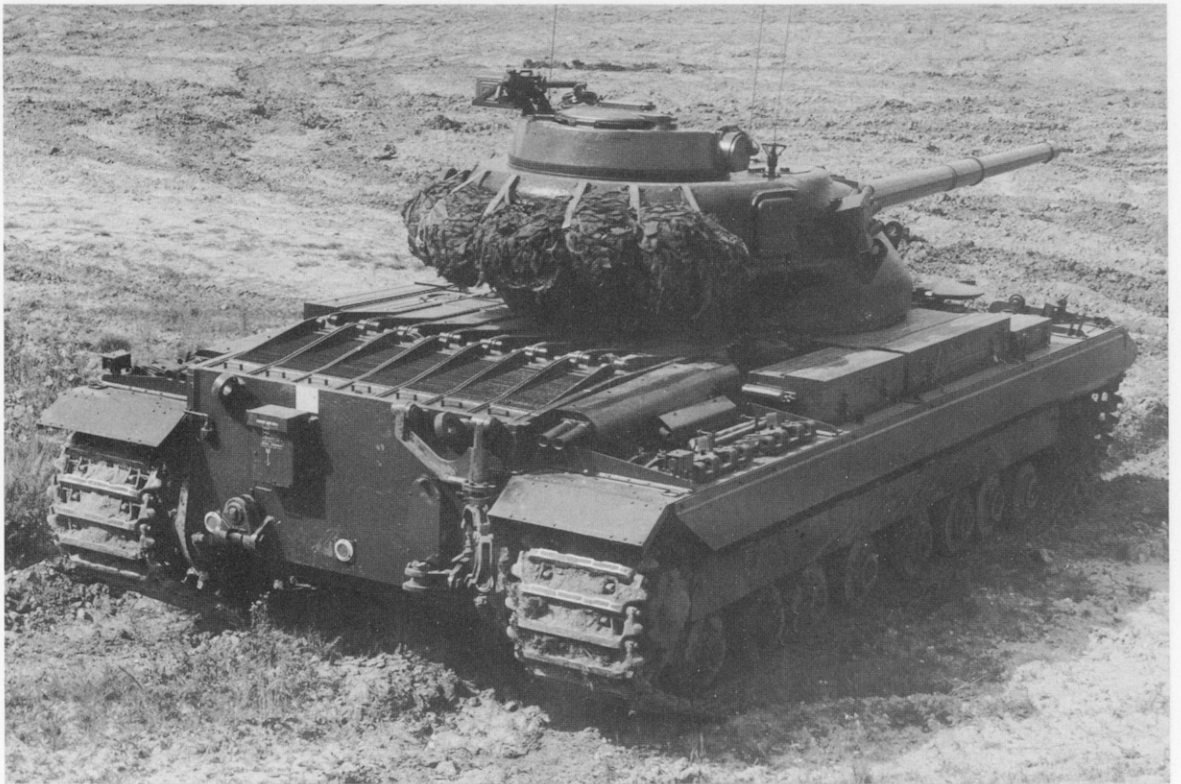
Conqueror 1. Note the vertical rear plate of the hull with the gun travelling clamp folded down on the right-hand side, the twin exhaust pipes, the camouflage net secured to the rear of the turret by straps before the introduction of a rack, and the armoured cowl for the rangefinder window on the right of the fire control turret.
