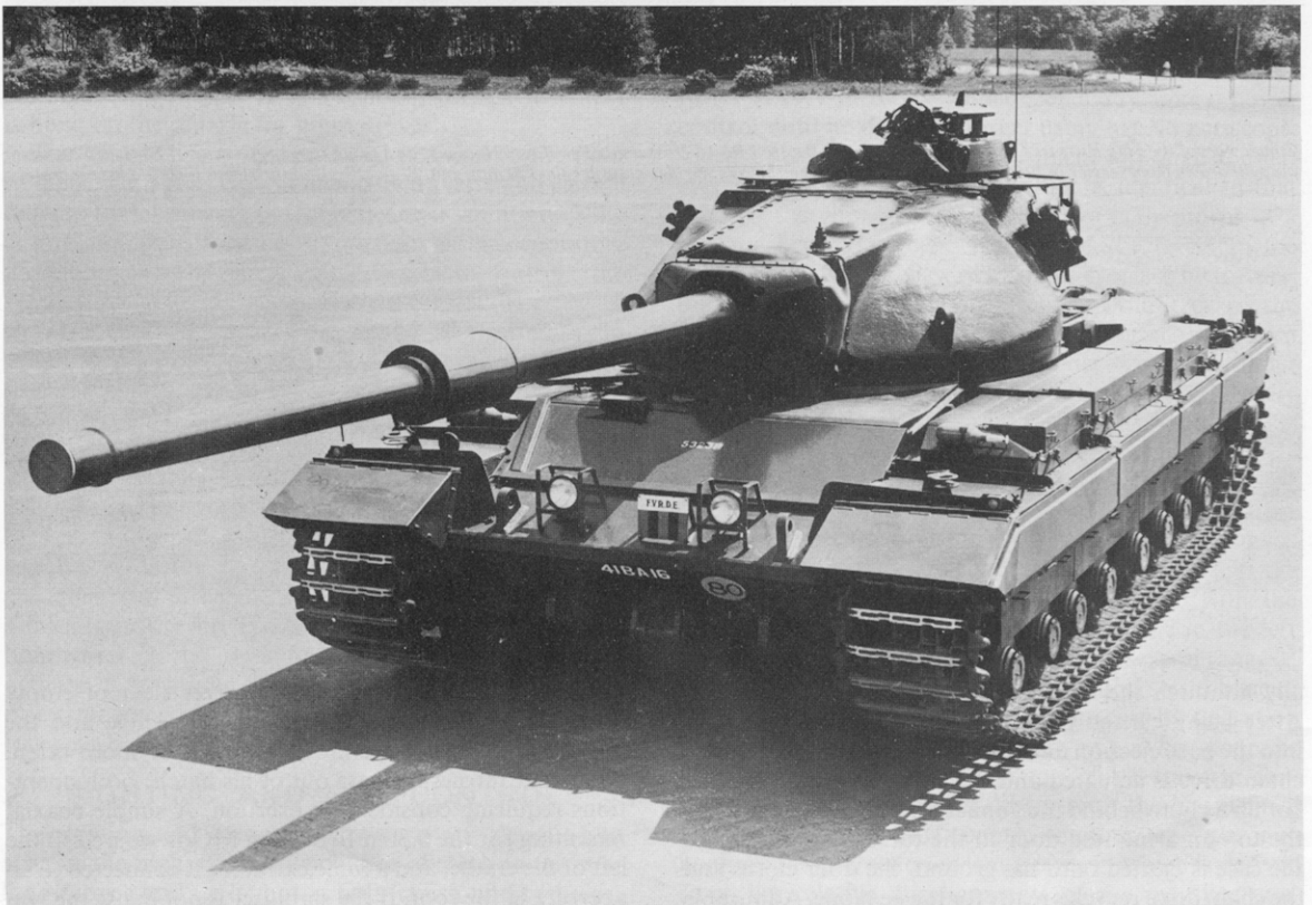
Conqueror Mark 2, showing the revised layout of the front hull armour with a single periscope for the driver. The gun has a fume extractor fitted and the fire control turret is traversed at 90° right to the turret axis.
