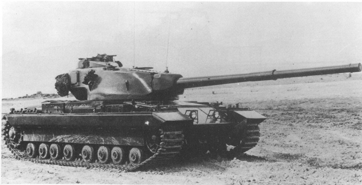
The first Conqueror. A protective counter-weight has been fitted on the 120 mm. barrel in lieu of the fume extractor. The armoured door for the case ejection chute is visible behind the smoke dischargers on the turret side.
