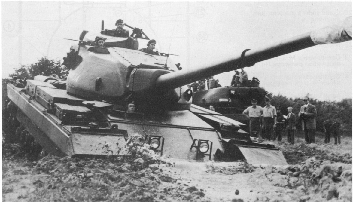
Two views of a Conqueror Mark 1, with a crew of The Queen's Own Hussars, in heavy going. Mark 1 can be distinguished from Mark 2 by the three driver's periscopes (instead of one) and by the prominent joint between the glacis and hull plates.
