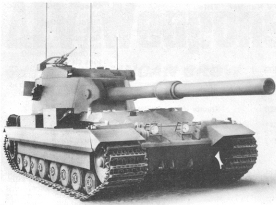
The wooden mock-up of FV 215b, the Heavy Anti-Tank SP mounting a 180 mm. gun.
