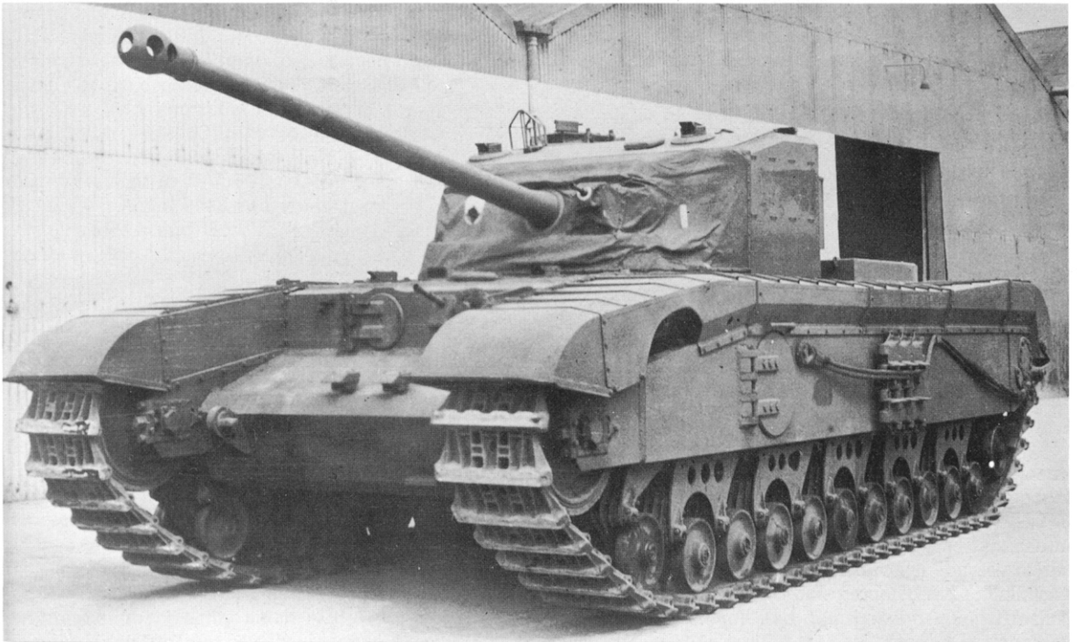
The A43 Black Prince, sometimes known as the "Super Churchill", was essentially similar to Churchill VII, but scaled up and with wider turret to take a 17-pdr. gun.
