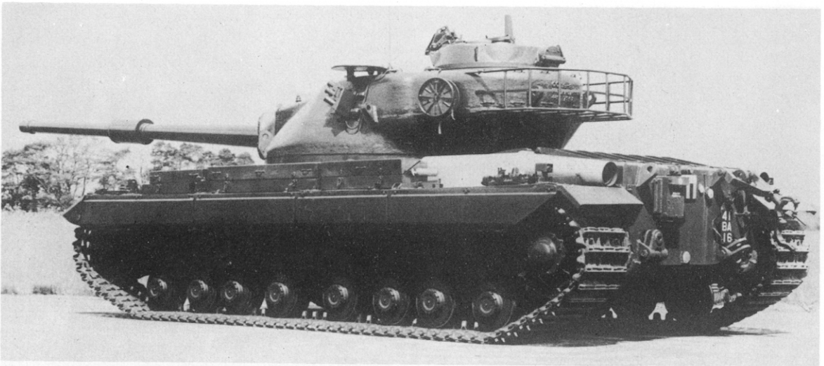
Conqueror 2 showing the stowage rack on the rear of the turret which was fitted as a retrospective modification. The circular object is the cable reel for remote communication.
