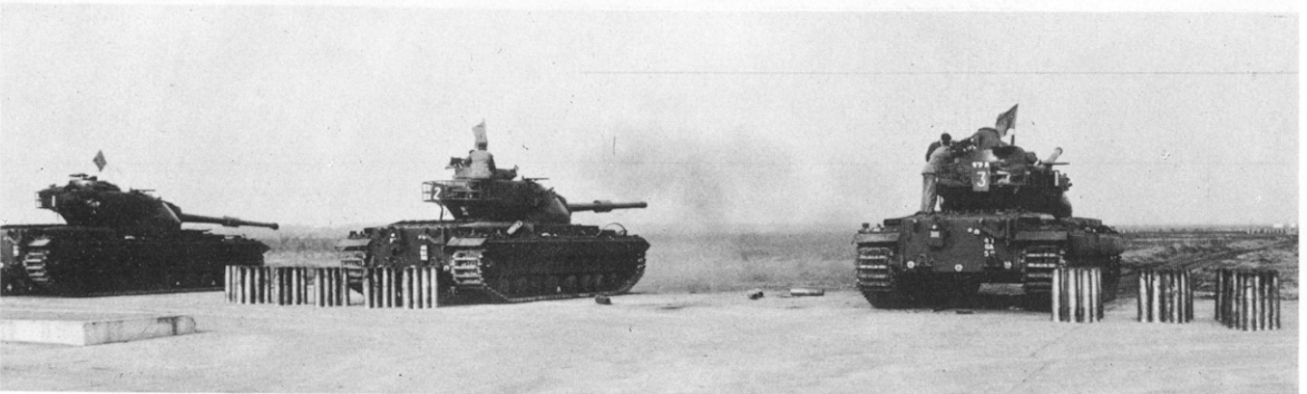
Conquerors of the 11th Hussars (now amalgamated with the 10th Royal Hussars as The Royal Hussars) on a firing range in Germany. The last Conqueror was withdrawn from service in 1966. Note the size of the sealed brass cartridge cases for the 120 mm. gun. Projectiles and cartridges were loaded separately.
