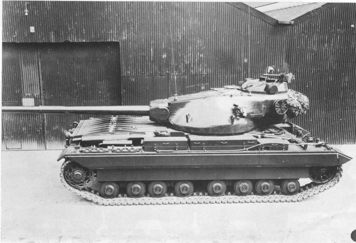
Conqueror Mark I, with turret reversed, showing the distinctive design of the turret and the arrangement of the four paired-wheel suspension units on each side.
