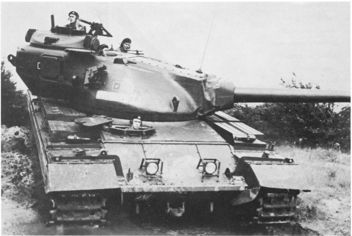
Two views of a Conqueror Mark 1, with a crew of The Queen's Own Hussars, in heavy going. Mark 1 can be distinguished from Mark 2 by the three driver's periscopes (instead of one) and by the prominent joint between the glacis and hull plates.
