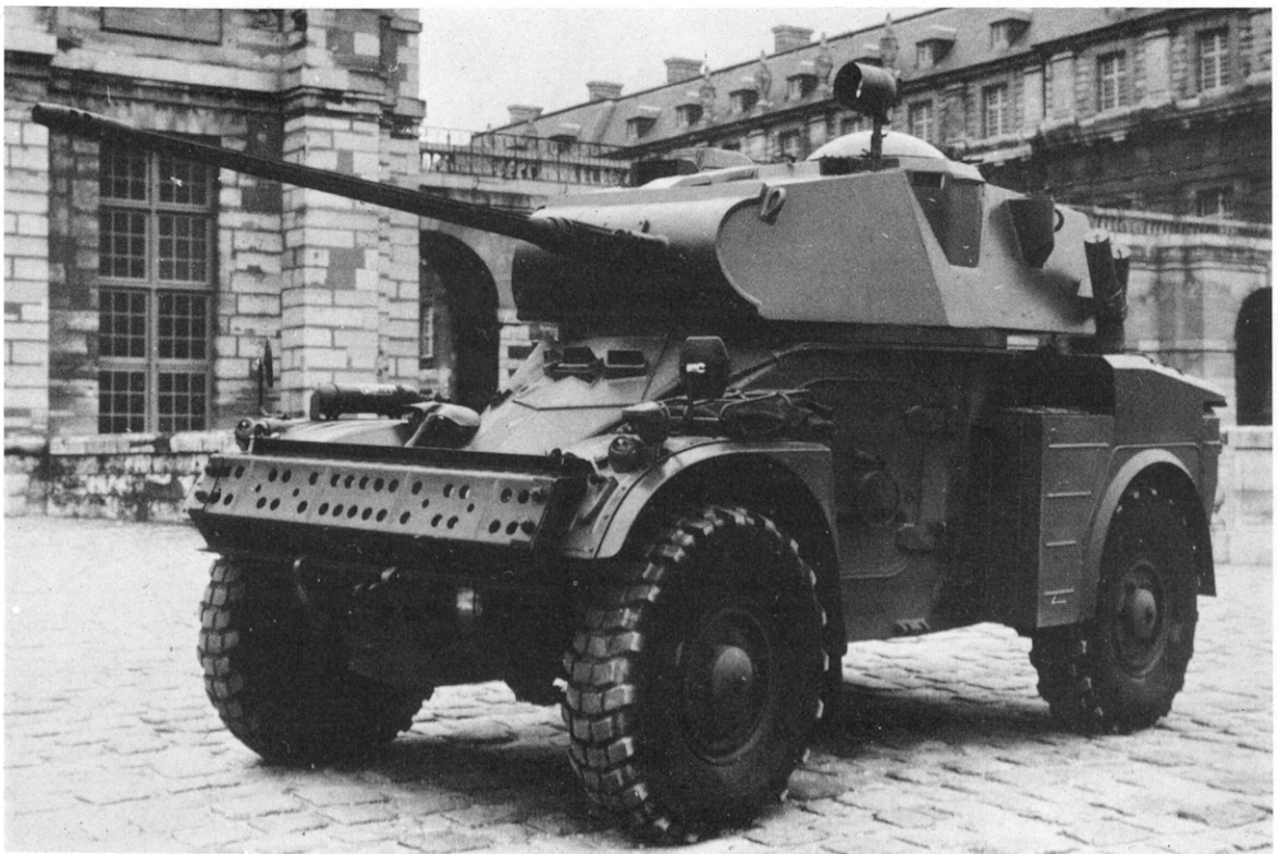
A.M.L. with H.30 turret mounting a 30mm gun.
