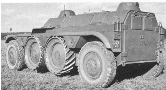
Rear view of the E.B.R.-E.T.T., an experimental armoured personnel carrier version of the E.B.R.
