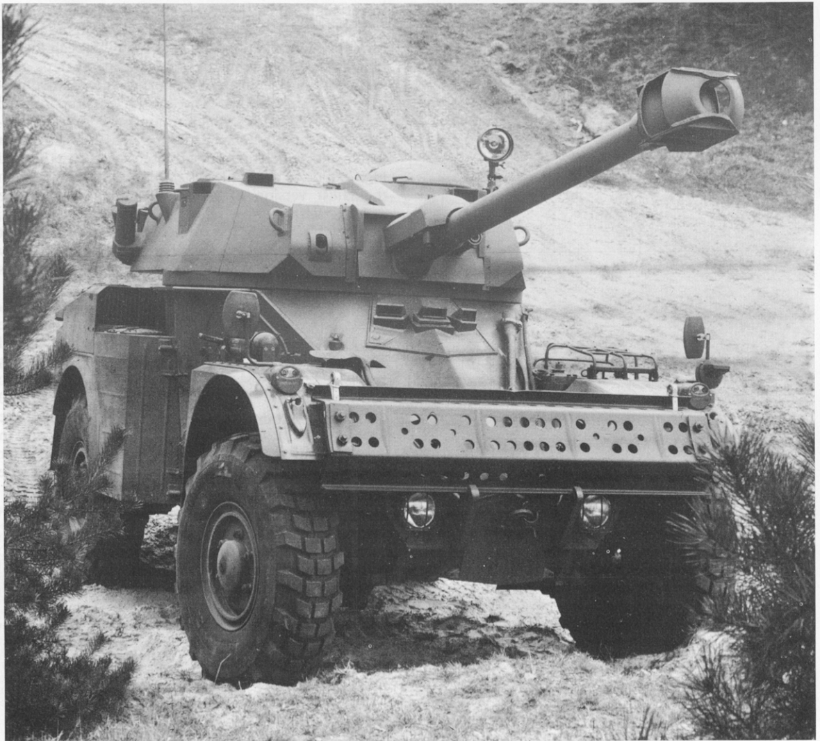
A.M.L. with H.90 turret mounting a 90mm anti-tank gun.
