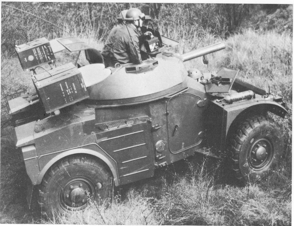
A.M.L. with HE.60 turret and S.A.M.O. 1160 launcher with Entac anti-tank guided missiles.
