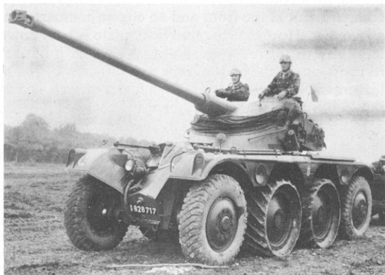
Service version of E.B.R. with F.L. 10 turret.
