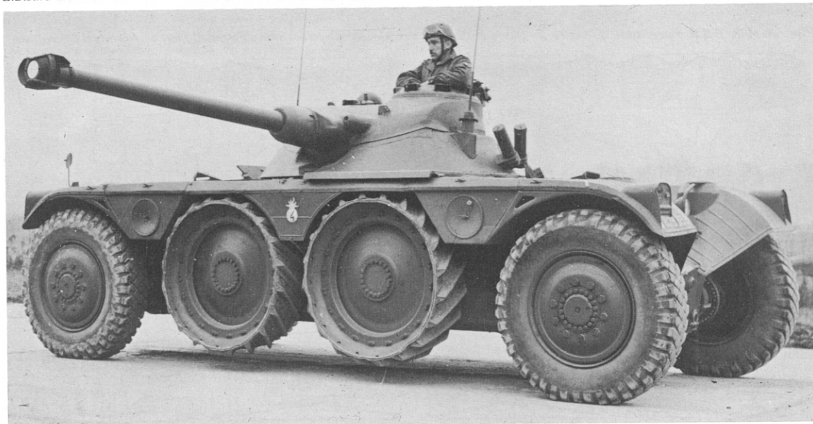
E.B.R.75 with F.L. 11 turret: the two centre wheels are raised for road operation.
