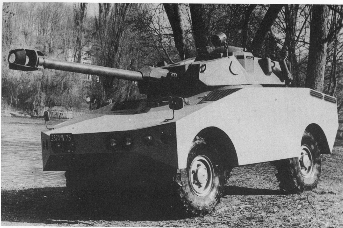
Amphibious version of the A.M.L. with H.90 turret.
