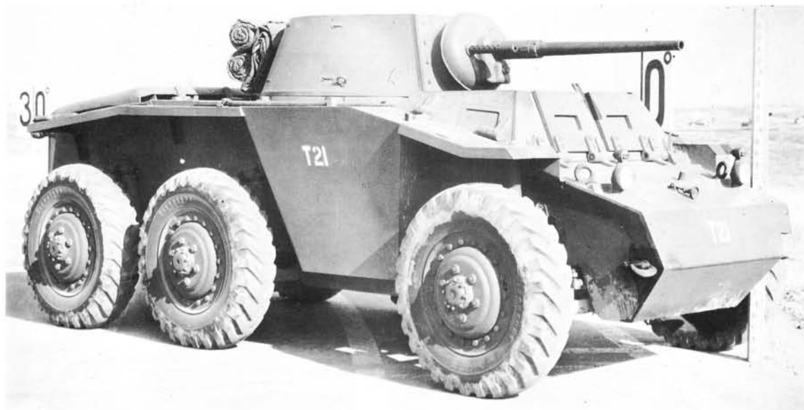
The T21 armored car, like the T22 and T23, was armed with the 37mm gun and co-axial 30 cal machine-gun. (U.S. Ordnance Dept.)
