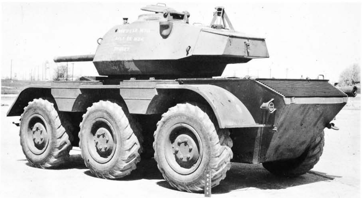
Three-quarter left rear view of the M38 light armored car (Wolfhound) after substitution of the M24 light tank turret. (U.S. Ordnance Dept.)
