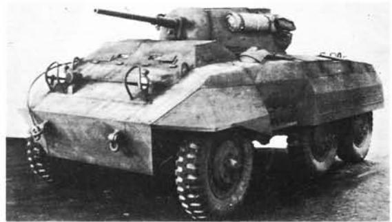
The T22E2 was the T22 with modifications, including addition of radio sponson, improvements in the turret and addition of sandshields. The T22E2 was standardized as the M8 armored car. (U.S. Ordnance Dept.)
