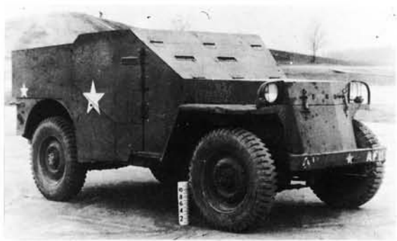
The ubiquitous jeep in the T25E2 scout car version was overloaded with armor. (Courtesy R. P. Hunnicutt)
