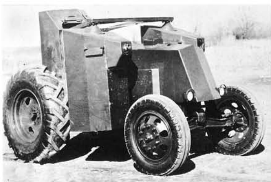
A John Deere standard farm tractor with modified front axle and wheels as a machine-gun unit. (U.S. Ordnance Dept.)
