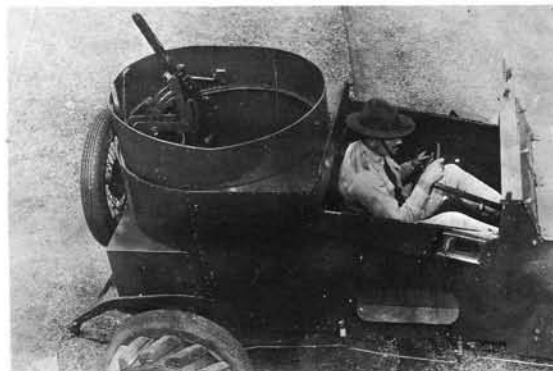
The T10 armored car showing run-flat rear grouser and vision protectors in hinged-down side armor.
