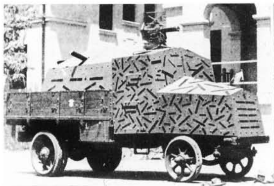
Armored car improvised on a World War I Liberty truck by the 15th Infantry in Tientsin, China, in 1930. (The Infantry Journal)
