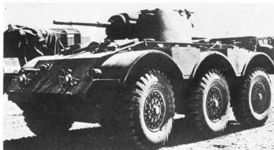
The T19E1 with a lighter, lower turret than the T19 and mounting a 37mm gun. (U.S. Ordnance Dept.)
