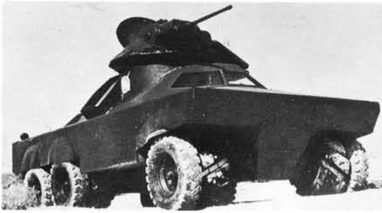
The AAI scout car, with squat centrally-placed turret, has inner run-flat grousers. (Courtesy AAI Corporation)
