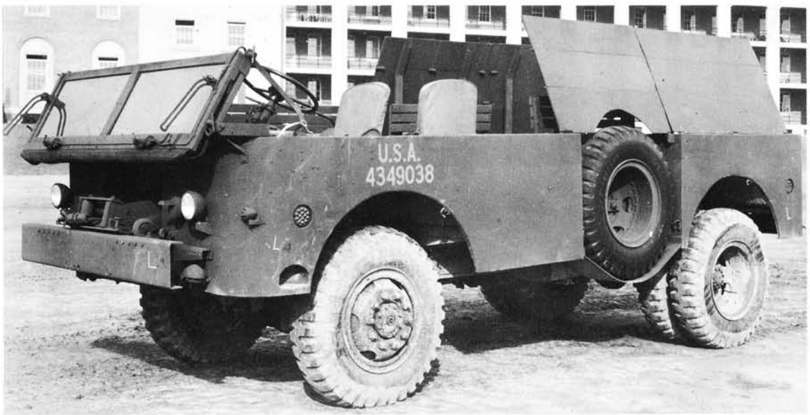
The experimental Reo 4 × 4 personnel carrier 3-ton version was a little known vehicle.
