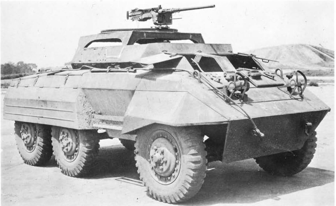
The prototype T26 armored utility vehicle with modified upper hull showing details of hull hatches. The T26 was eventually standardized as the M20 armored utility car. (U.S. Ordnance Dept.)
