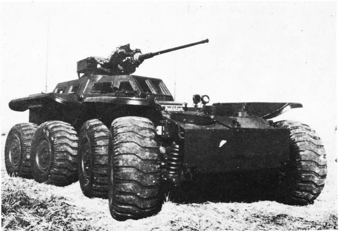
The XM808 armored car based on the well-tested articulated Lockheed Twister chassis.
