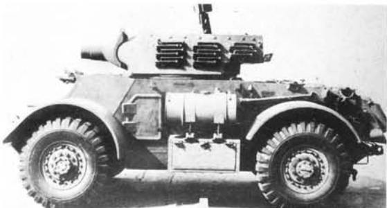
The T17E3 had a 75mm howitzer turret from an M8 Howitzer Motor Carriage. It was developed for British use but never put into production. (U.S. Ordnance Dept.)
