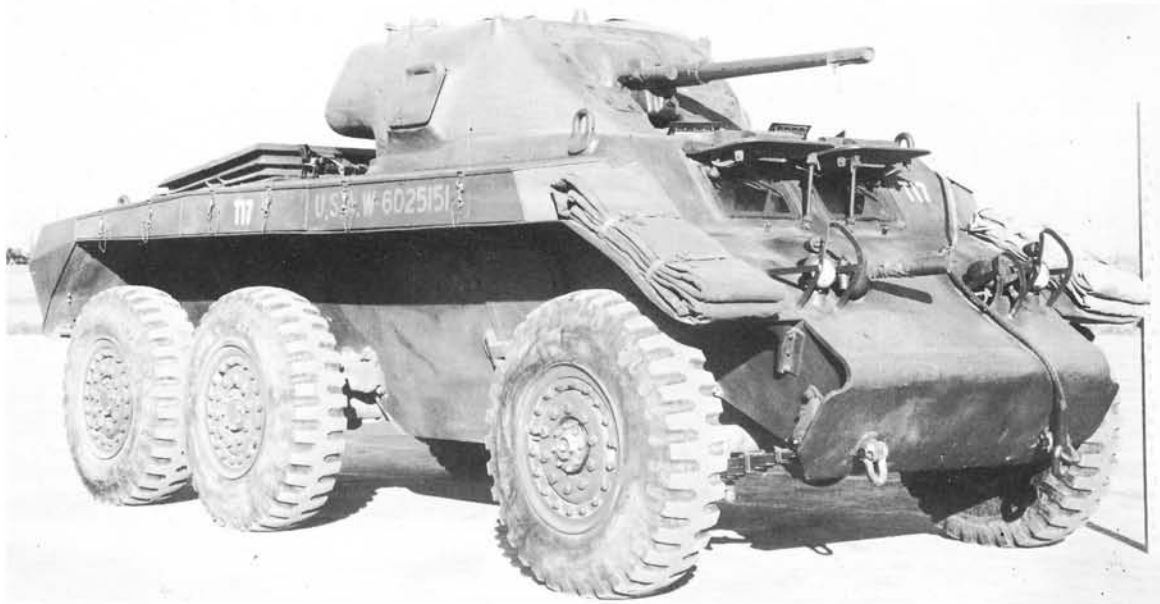
A production model of the 6 × 6 T17 armored car with bow machine-gun and standard turret armament of 37mm M6 gun and co-axial .30 cal machine-gun. (U.S. Ordnance Dept.)
