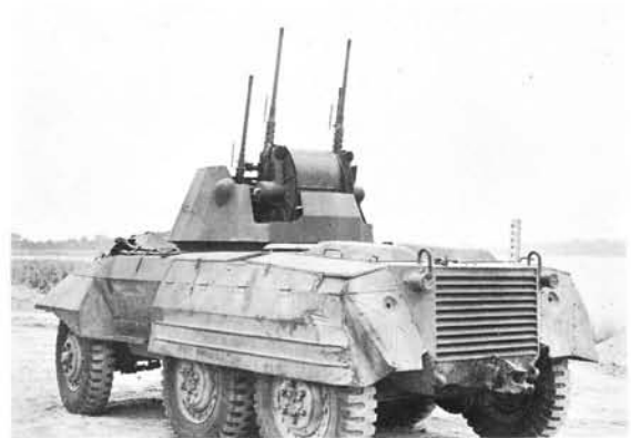
Three-quarter left rear view of the T69 Multiple Gun Motor Carriage with its Quad 50 cal machine-guns at full elevation. The T69 had the M8 armored car chassis. (U.S. Ordnance Dept.)
