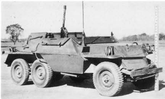
The T24 scout car utilized standard quarter-ton truck (Jeep) components to become a 6 × 6 vehicle.
