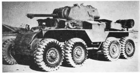
The T18 8 x 8 heavy armored car modified with a 57mm gun and larger turret instead of a 37mm light tank turret and gun was the T18E2, known to the British as the Boarhound. This is the first T18E2 pilot model. (U.S. Ordnance Dept.)
