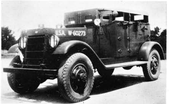
The T7 scout car was beginning to take the form which led eventually to the design of the M3A1 scout car. (U.S. Ordnance Dept.)
