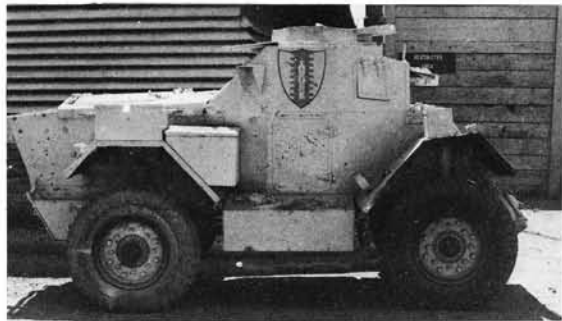
Daimler Dingo re-armored by U.S. troops in Vietnam with superstructure and cupola. Badge on superstructure side is of 4th Cavalry. (Courtesy J. W. Loop)
