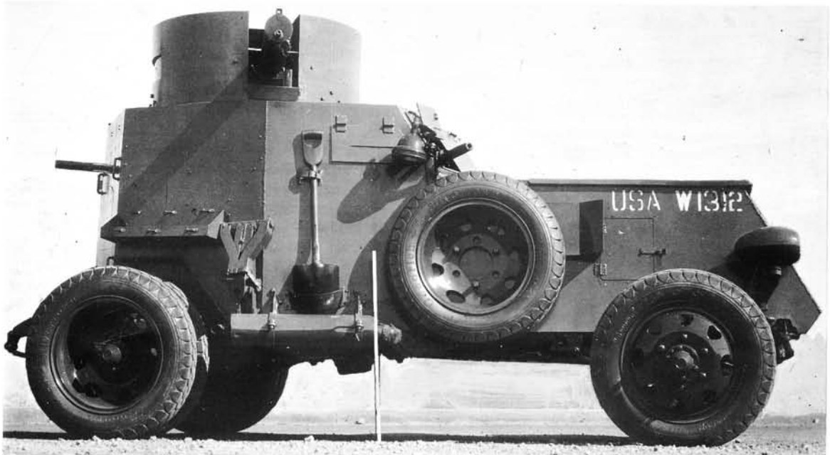
The T7 armored car built at Holabird Quartermaster Depot had a hull interchangeable with a cargo truck body. (Courtesy D. H. Unger)
