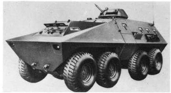
The Chrysler SWAT (Special Warfare Armored Transporter) is an 8 x 8 armored personnel carrier. (Courtesy J. W. Loop)
