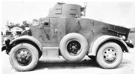
The T11E2 armored car with engine in rear gave the crew much better forward vision. (U.S. Ordnance Dept.)
