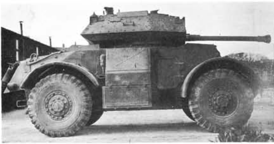
The British Staghound Mark III had a Crusader tank turret with 75mm gun. It had no bow machine-gun. (Courtesy G. M. Ross)
