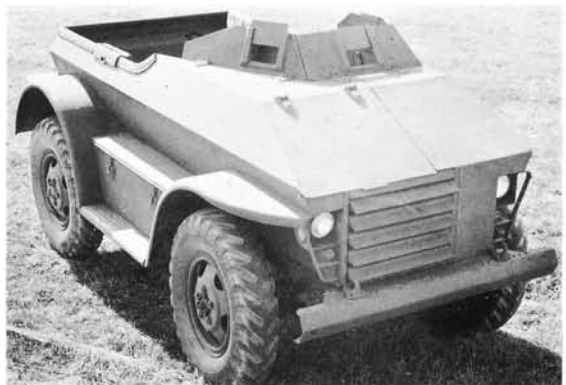
The O.P. tender T2 was a small 4 × 4 liaison vehicle type for the artillery, dropped after partial testing.
