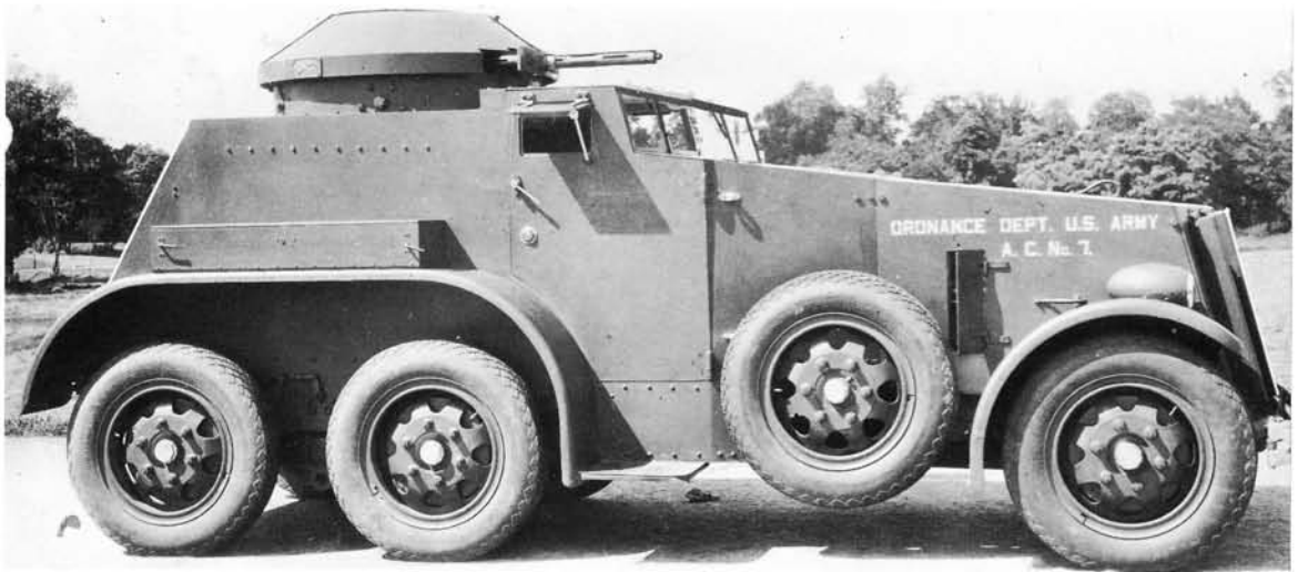
A production model of the M1 armored car which was the first U.S. armored car built as such rather than armoring a commercial vehicle. (Courtesy R. E. Jones)
