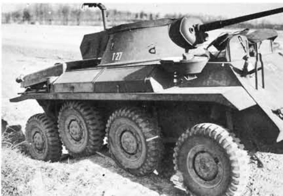
The Studebaker T27 armored car suspension system followed ground conformation closely.
