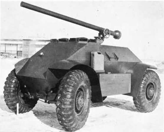
The T115 four-man wheeled carrier (Bat weapon version) was a 1956 experimental anti-tank vehicle. (U. S. Army)
