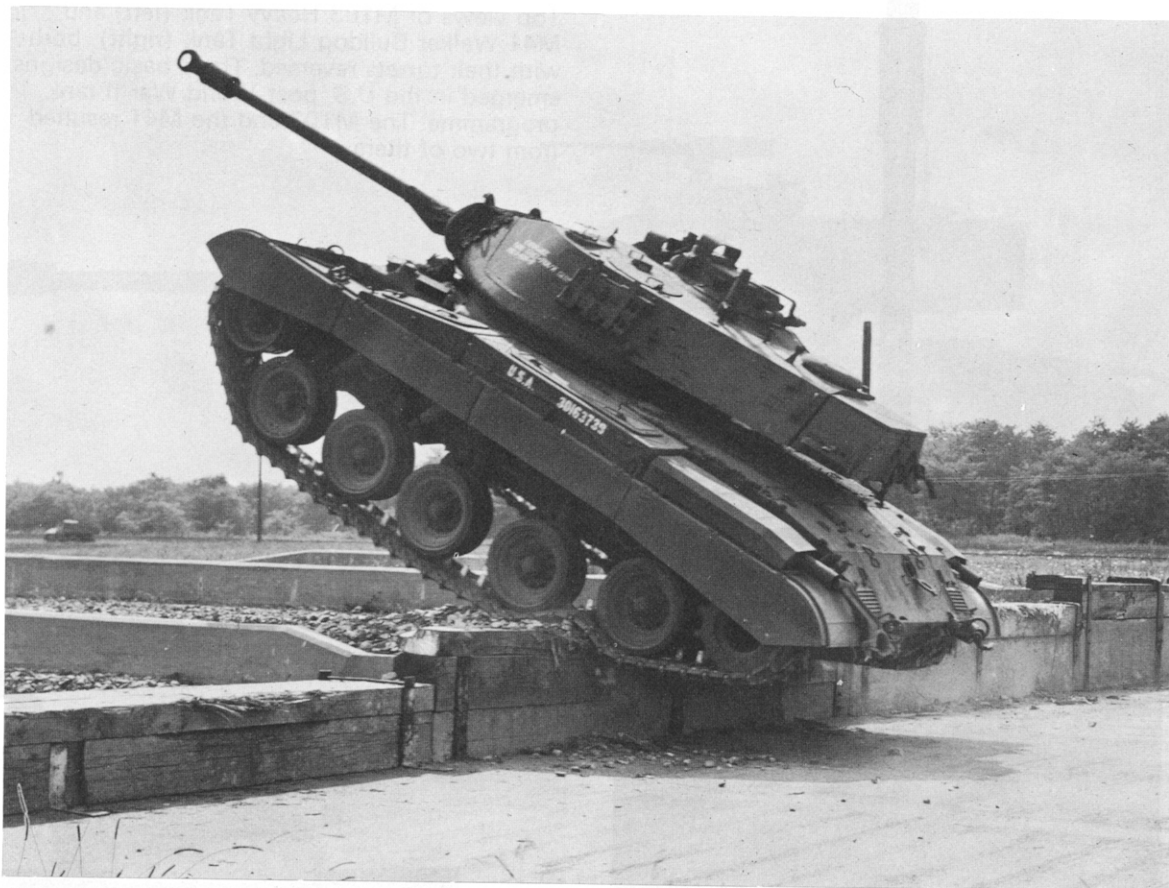
The T41E1 surmounts a vertical obstacle while undergoing proving ground tests. (U.S. Ordnance Corps)
