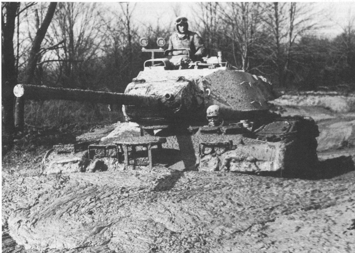
Controlled mud at the Cleveland Tank Arsenal proving ground provided ample testing of M41 Light Tank engine and transmission. (Courtesy Cadillac Motor Car Company)
