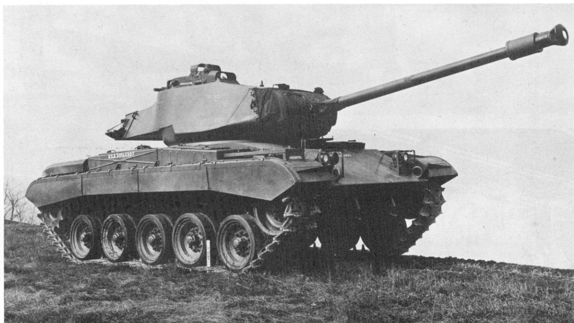
The T41E2 which became the M41A1 had an improved turret which was both welded and cast. (Courtesy Cleveland Tank Arsenal)
