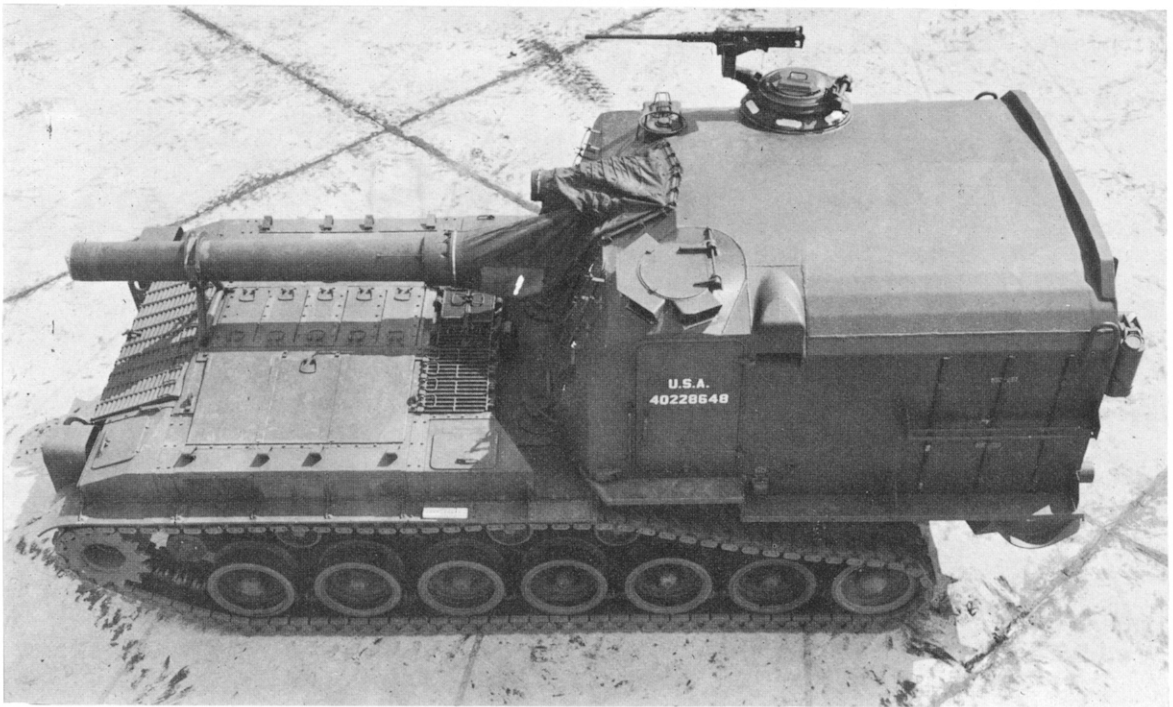
Top view of the 8-inch Howitzer Motor Carriage M55E1 illustrates the chassis common to the M53, also built with M41 Light Tank components. (U.S. Ordnance Corps)
