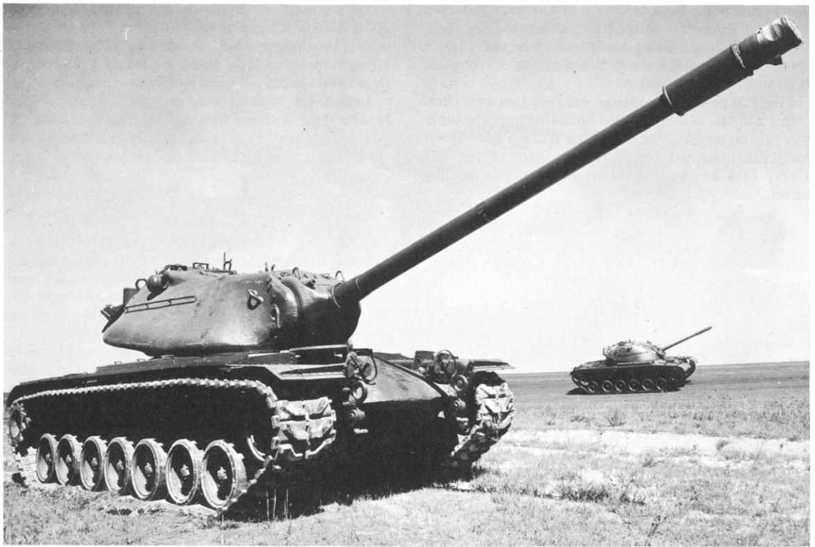
T43E1 Heavy Tank was standardized as the M103 shown here with a T48 Medium Tank in the background. (Courtesy Chrysler Corporation)
