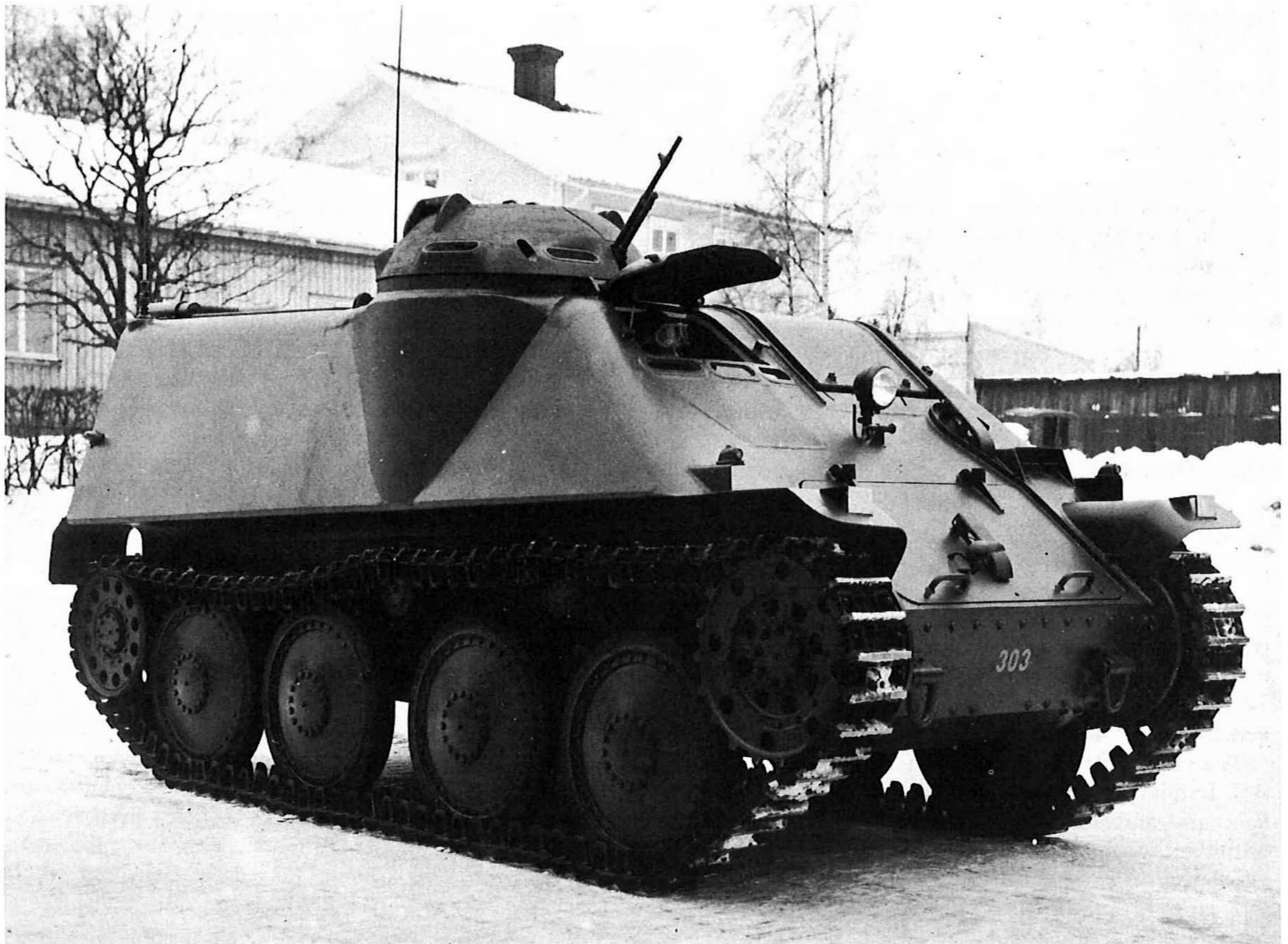
Prototype of Pbv 301 with a mock-up of a conventional, domed turret.
