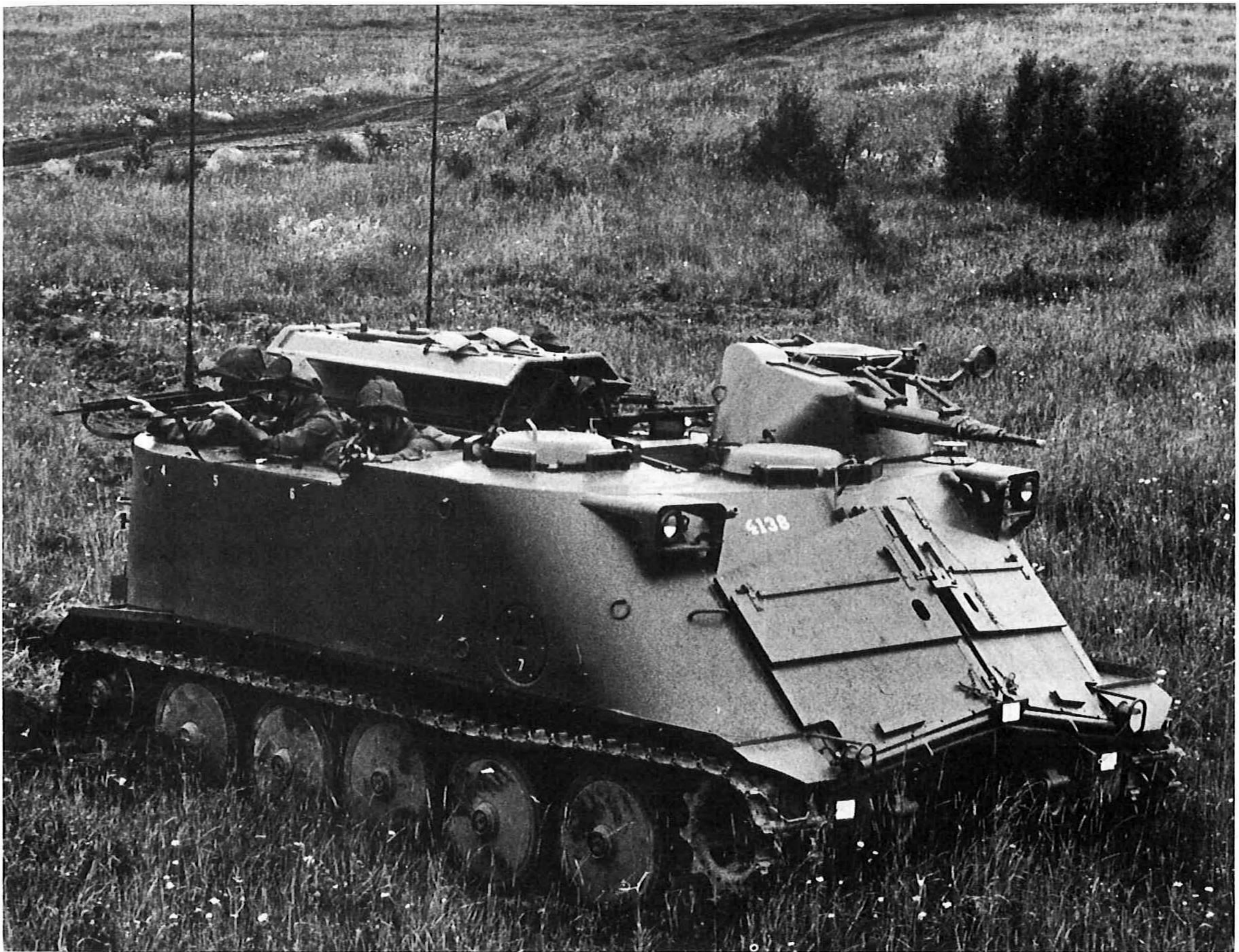
Early production version of Pbv 302 with troops firing out of the roof hatches.
