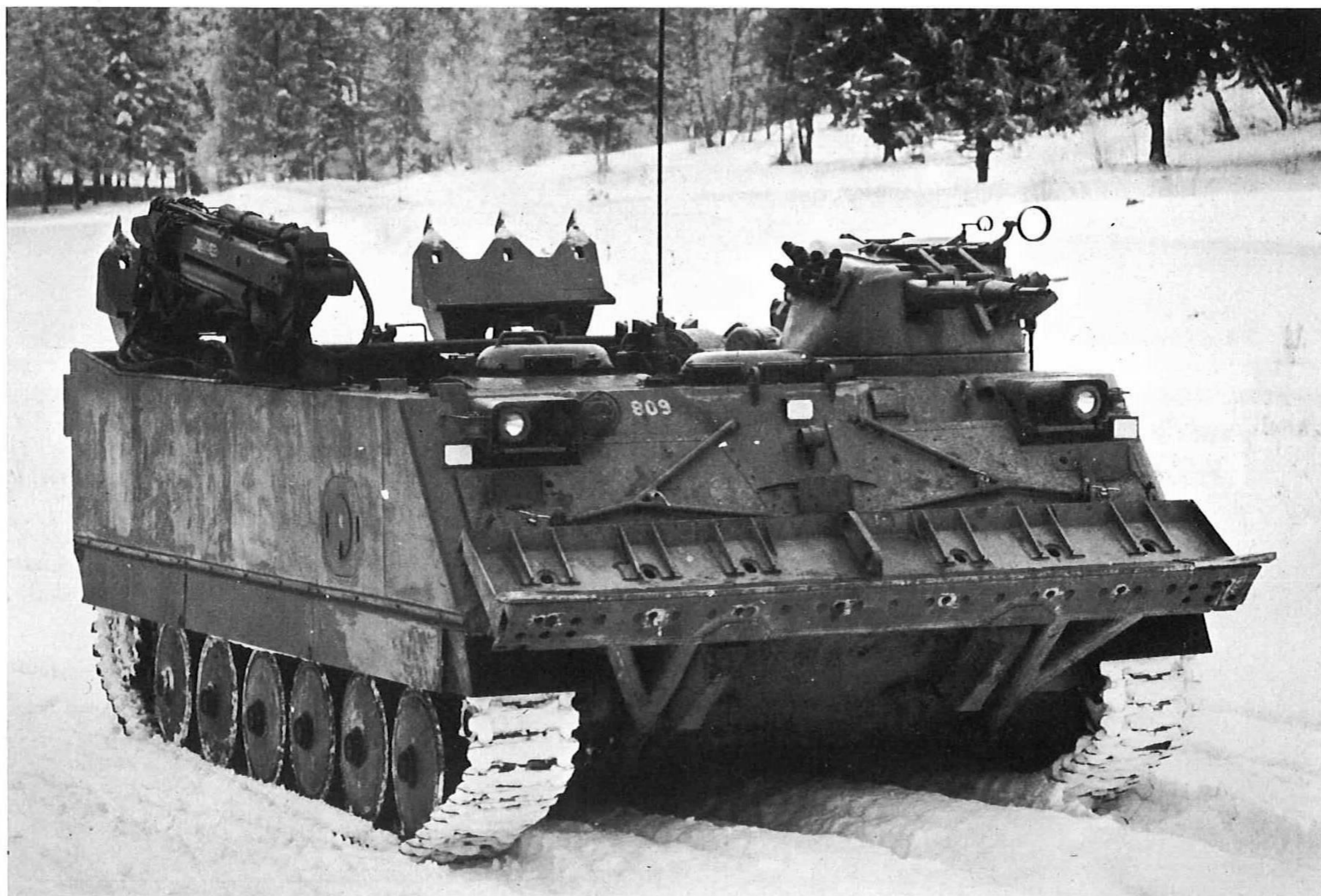
Prototype of Bgbv 82, the armoured recovery vehicle derived from the Pbv 302.
