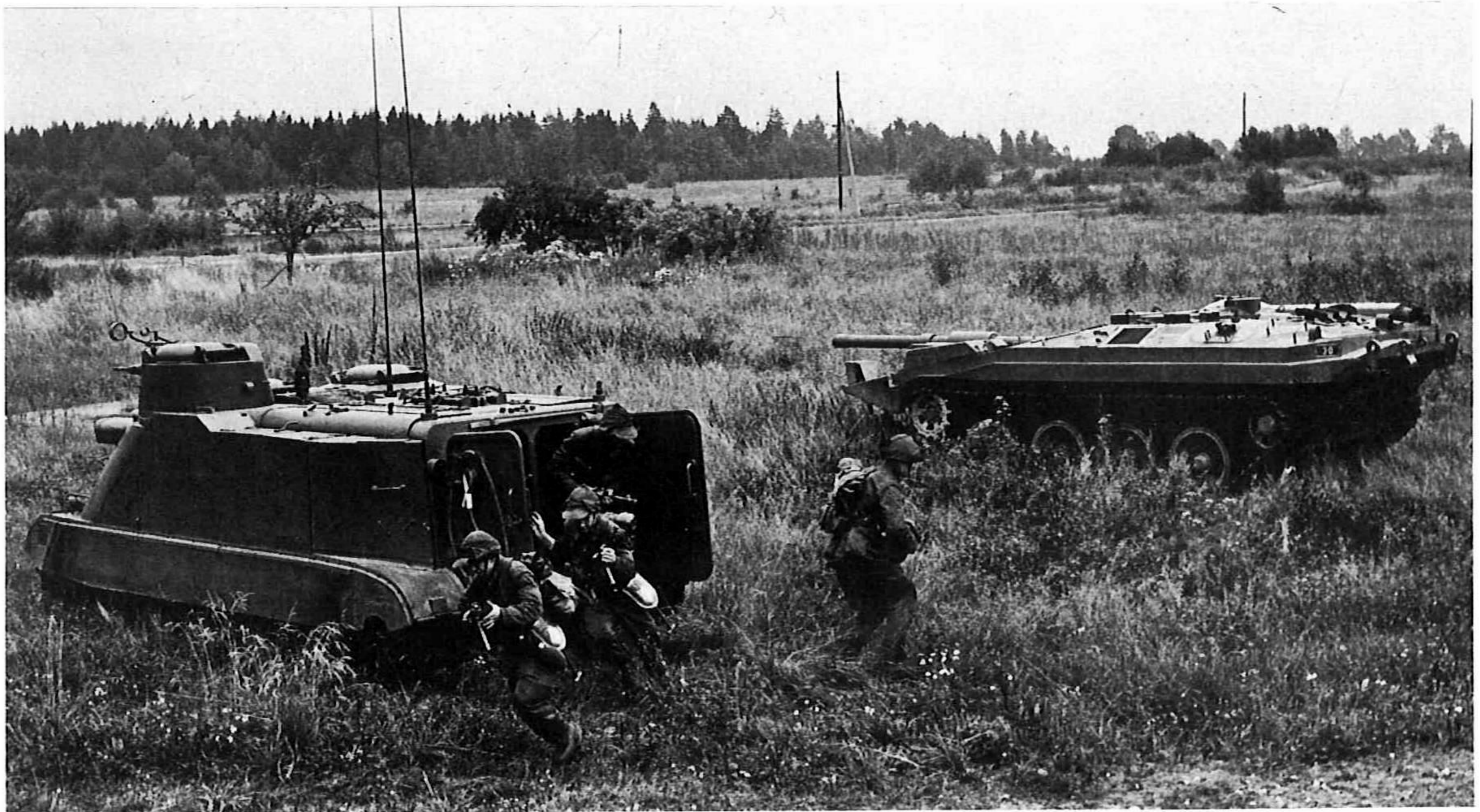
Prototypes of Pbv 302 and of the S-tank at a demonstration in September 1965.
