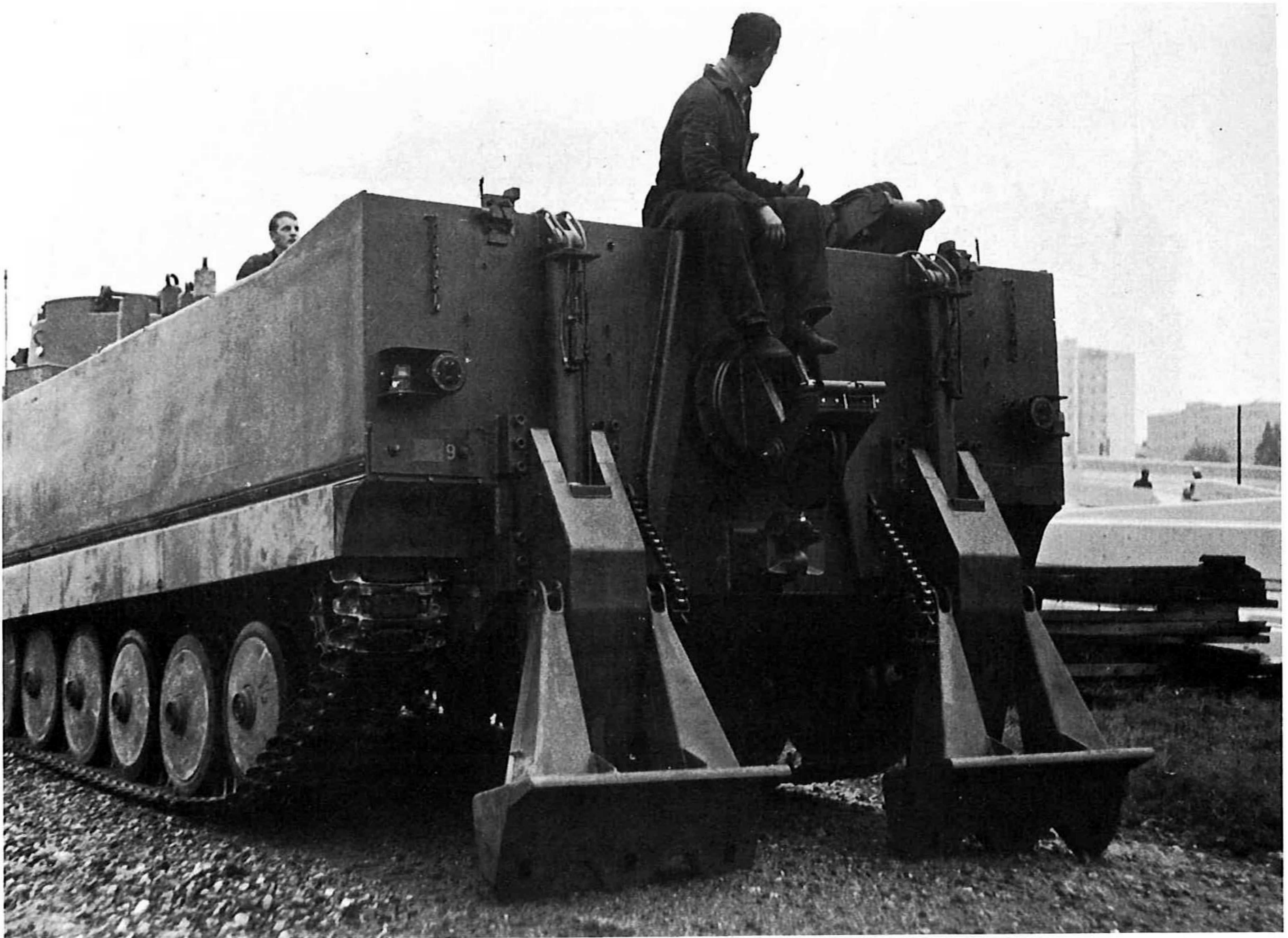
Bgbv 82 with its ground anchor spades lowered on to the ground.
