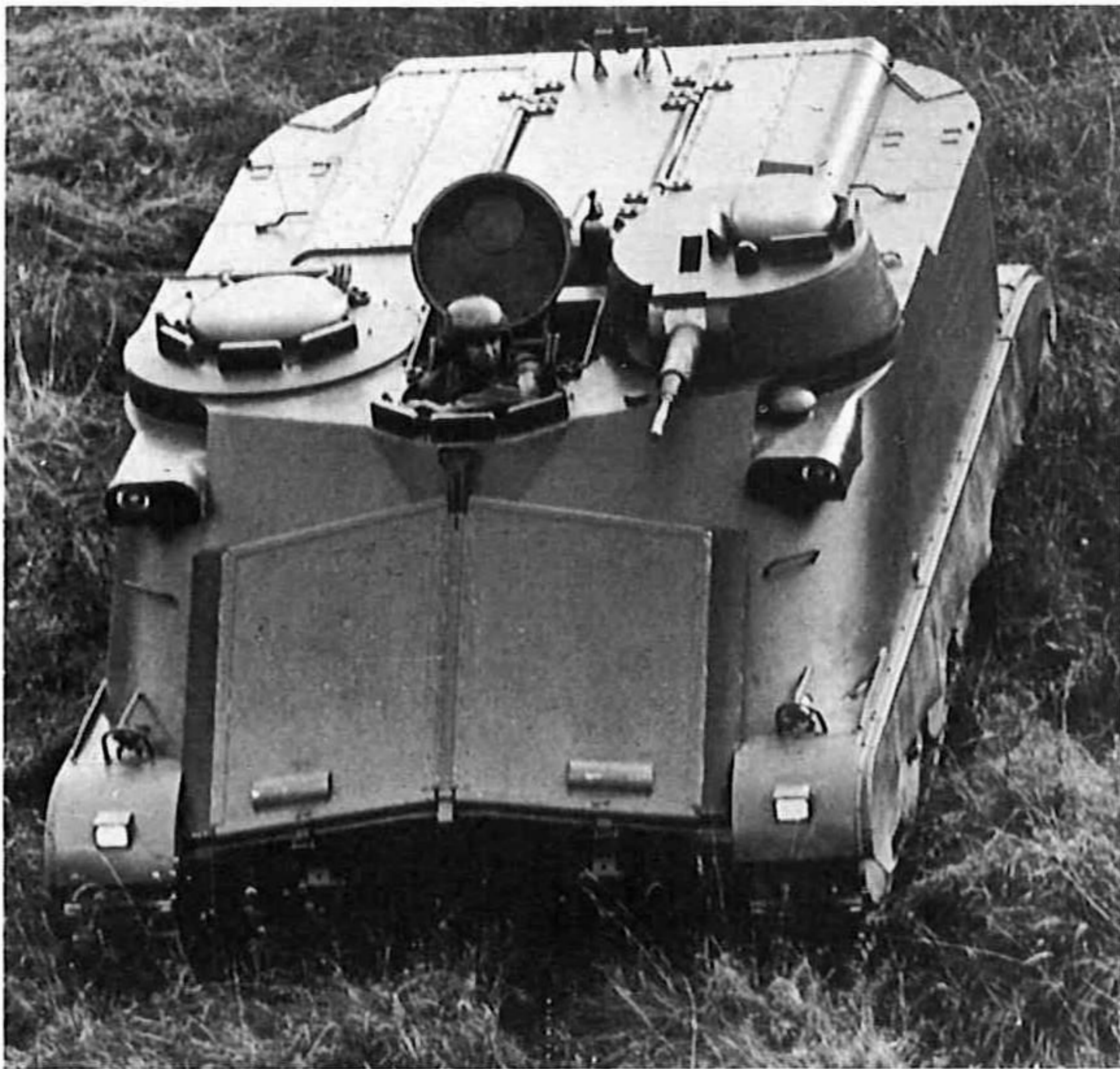
Pbv 302 prototype showing the driver's position between the gun turret and the commander's cupola. (Hägglund)
