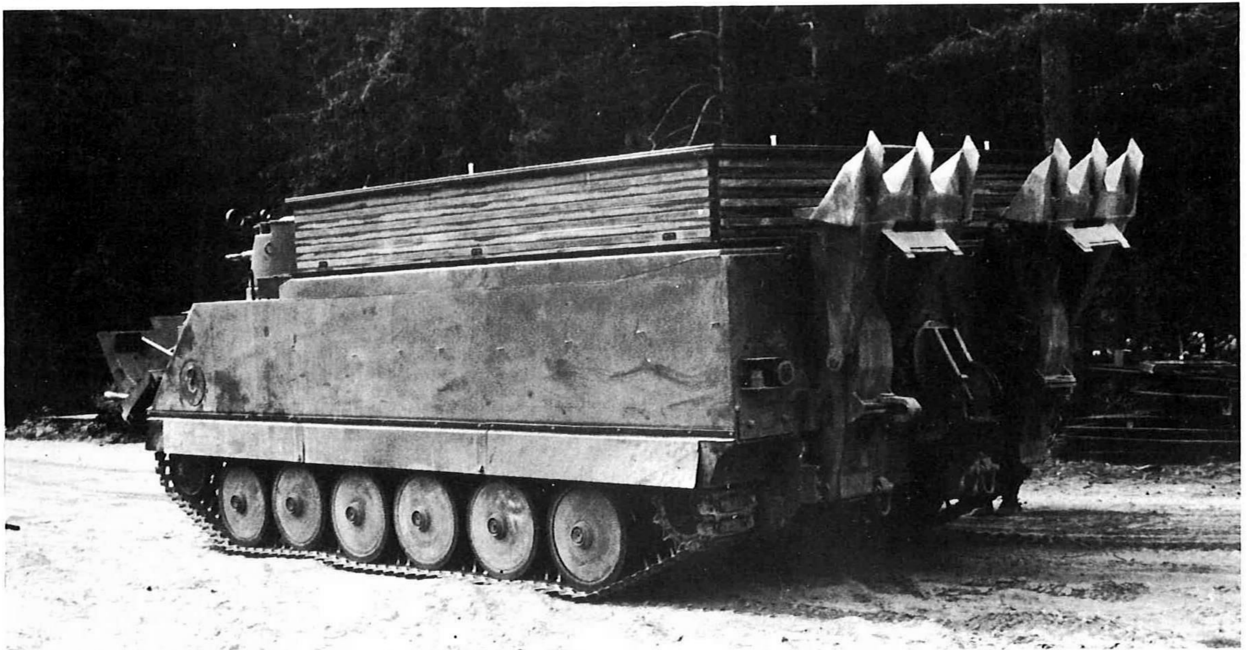
Pre-production version of Bgbv 82 with a collapsible flotation screen added to increase the freeboard.
