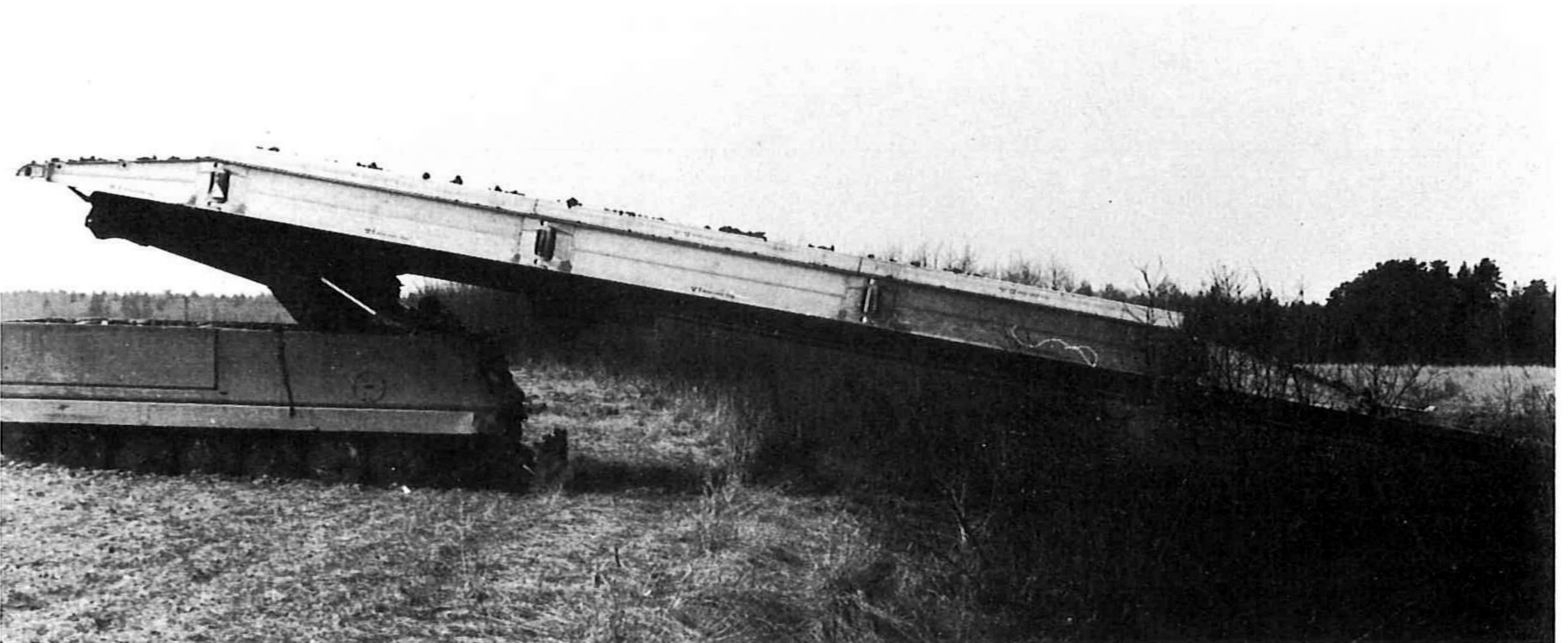
Sequence of three photographs showing the laying of a bridge by the Brobv 941: (top) bridgelaying extending its telescopic beam over the obstacle; (centre) bridge being slid over the extended beam; (bottom) with the beam retracted the bridgelaying is lowering the bridge on to the ground. (Hägglund)
