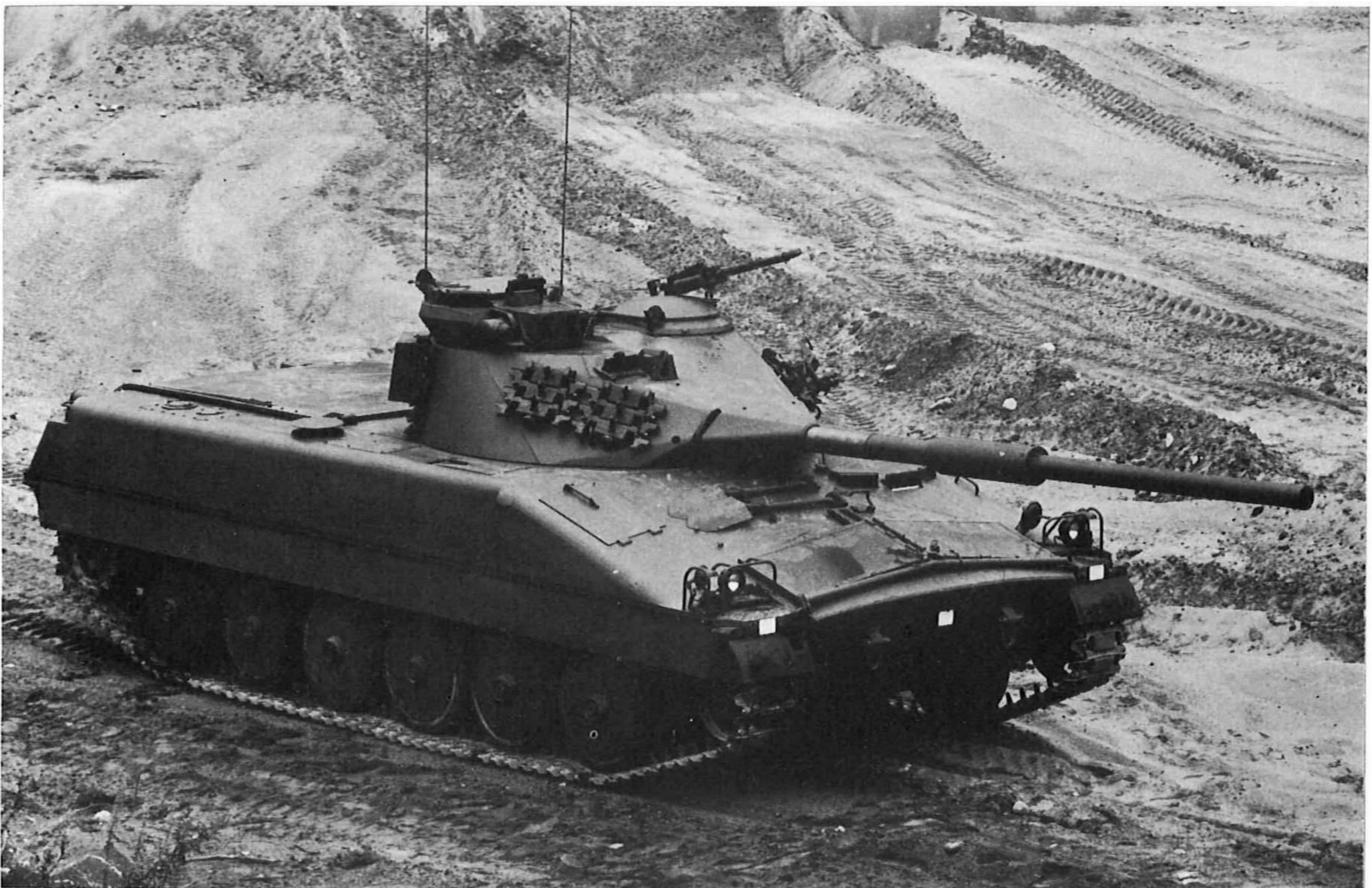
View of Ikv 91 showing the commander's rotating cupola with rangefinder and the loader's hatch.
