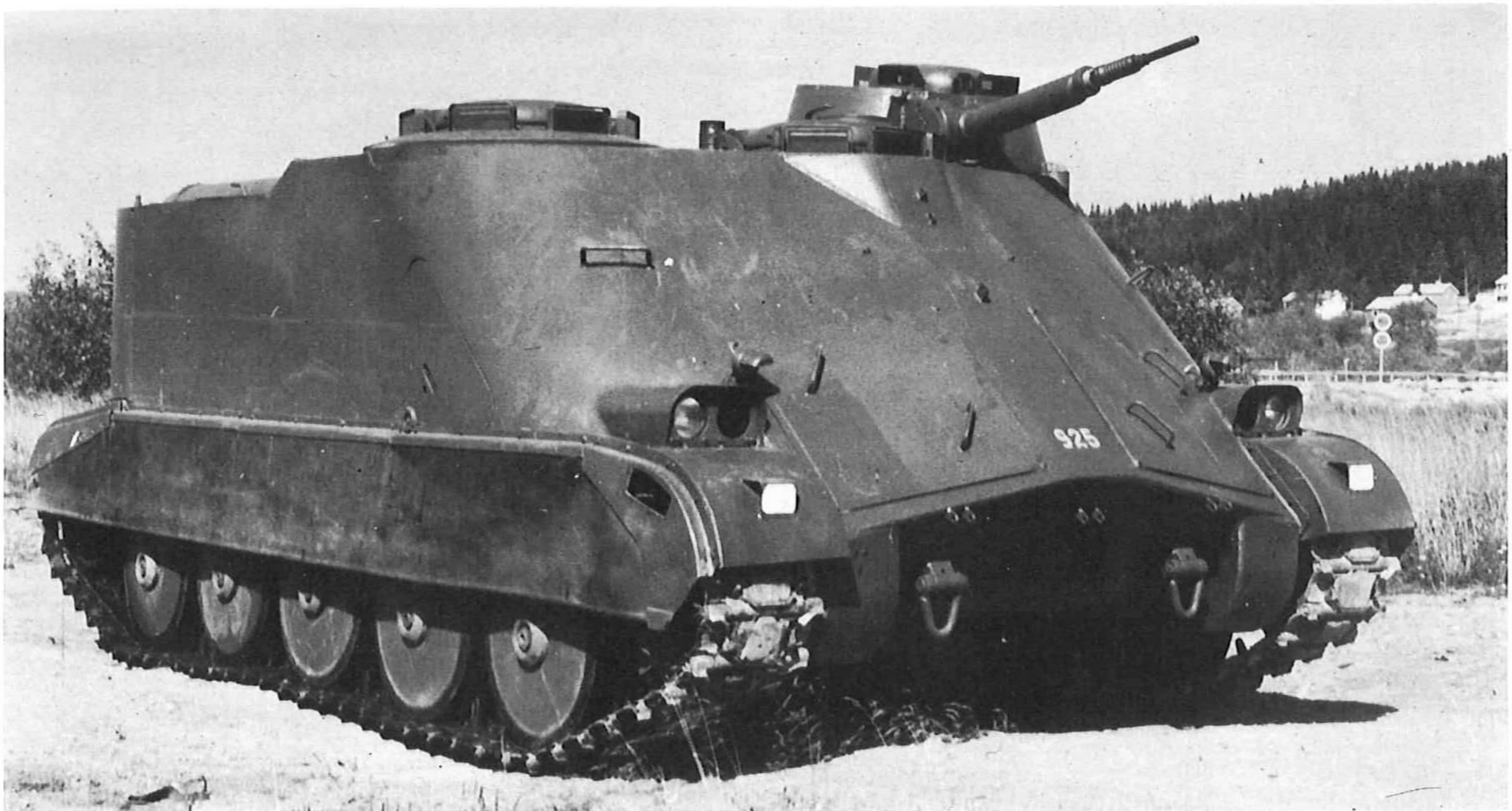
No. 1 prototype of Pbv 302 without its trim vane.
