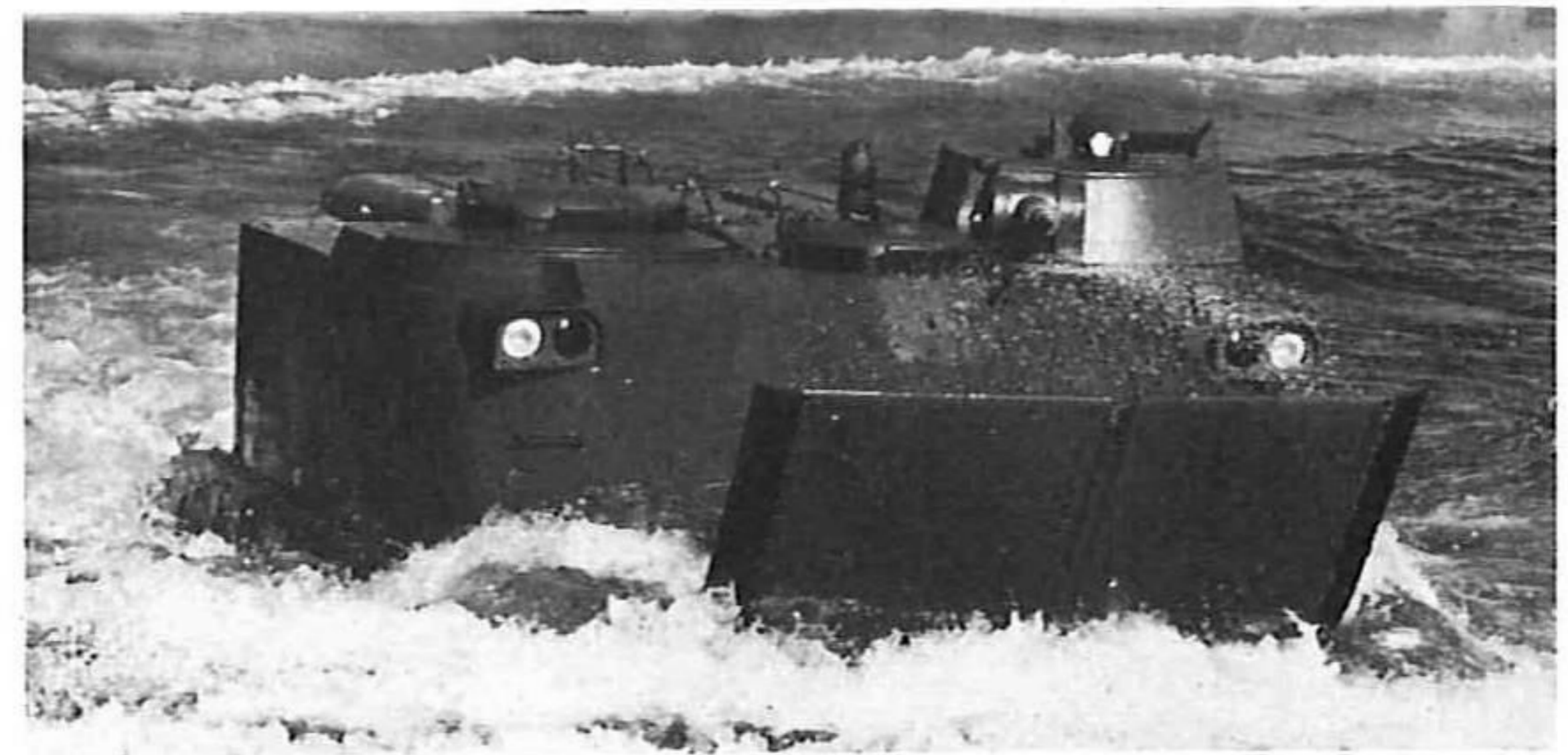
Pbv 302 prototype with its trim vane hinged forward. (Hägglund)
