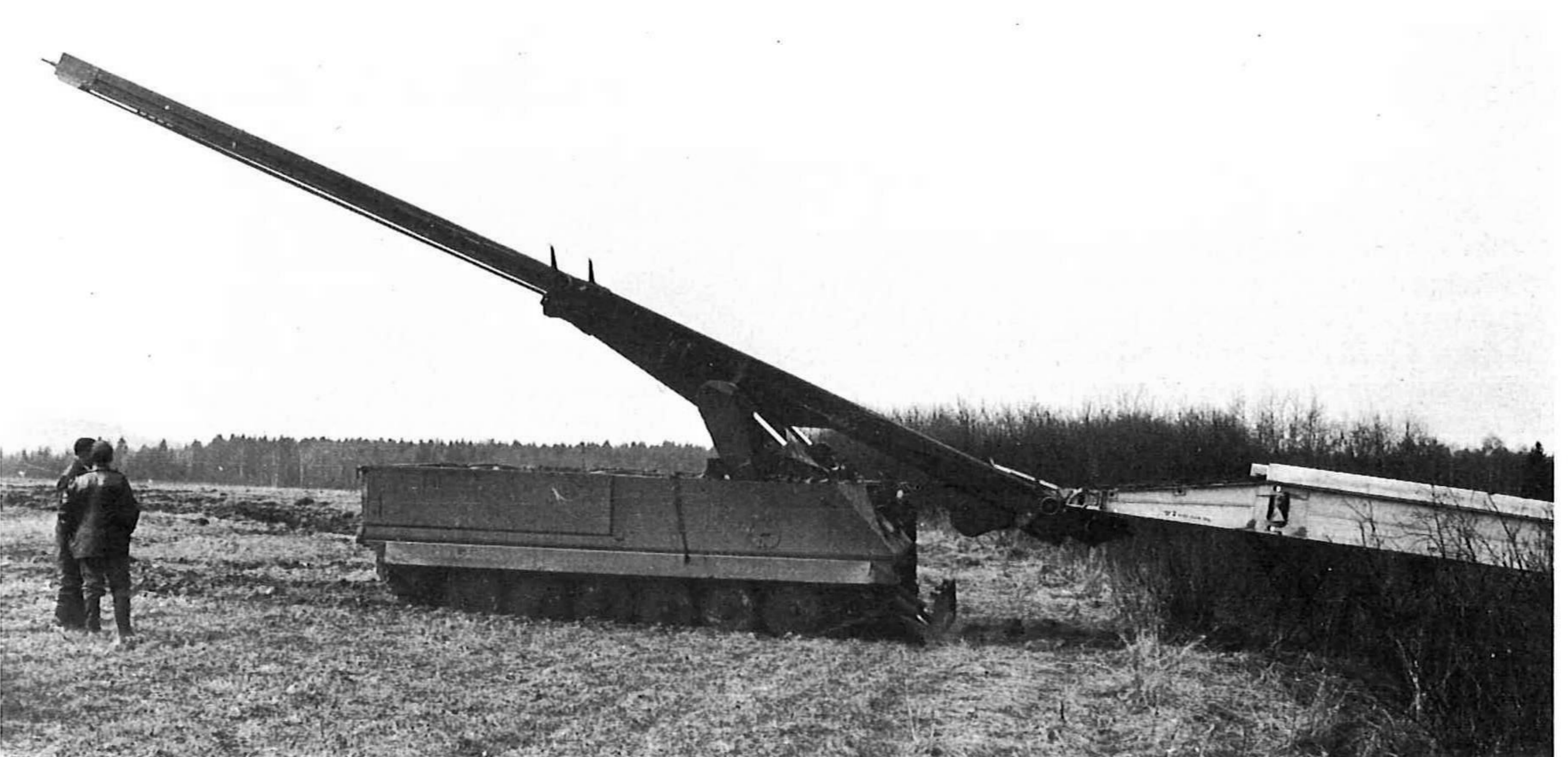
Sequence of three photographs showing the laying of a bridge by the Brobv 941: (top) bridgelaying extending its telescopic beam over the obstacle; (centre) bridge being slid over the extended beam; (bottom) with the beam retracted the bridgelaying is lowering the bridge on to the ground. (Hägglund)
