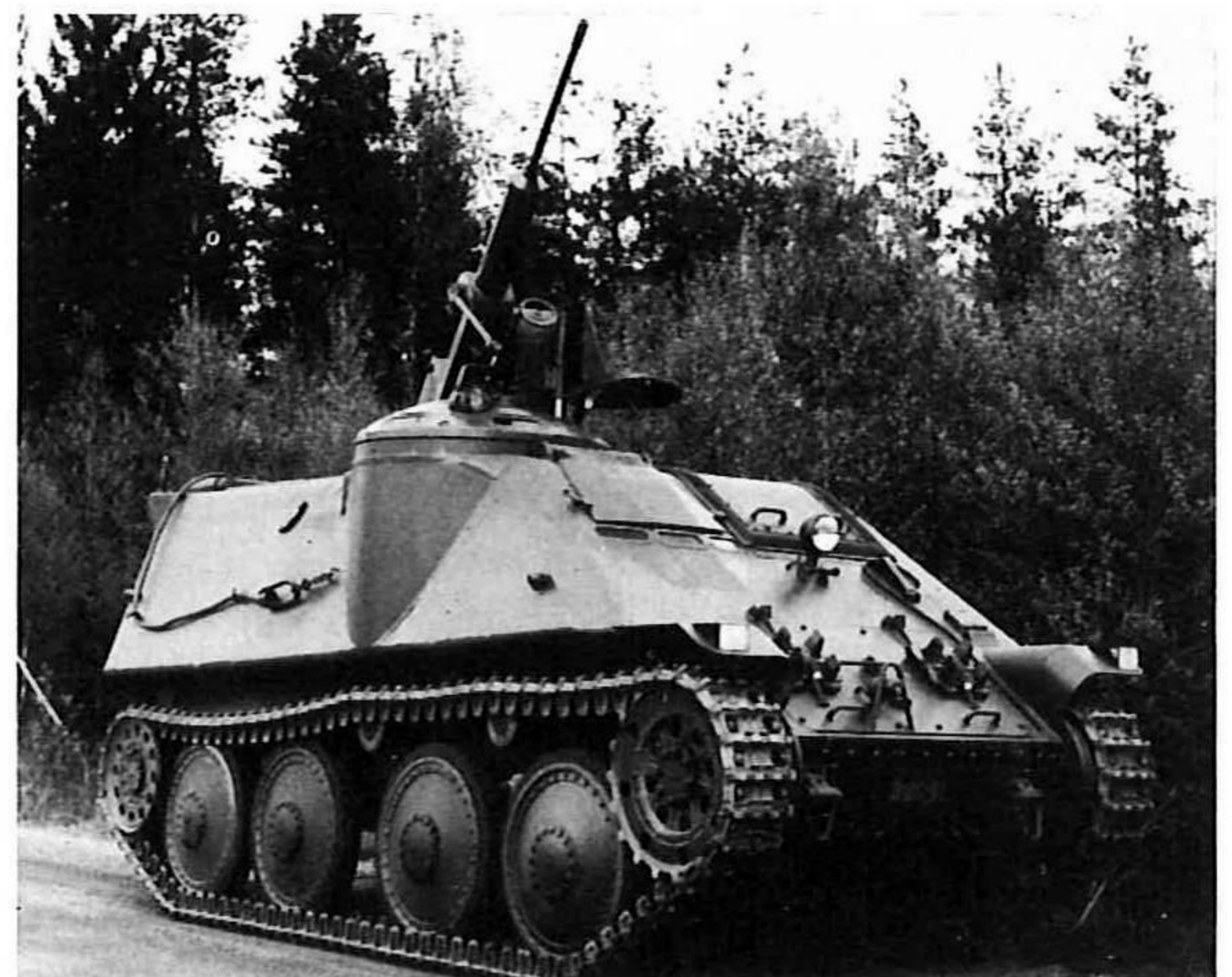
Pbv 301 with its 20mm gun elevated for anti-aircraft fire. (Bofors)
