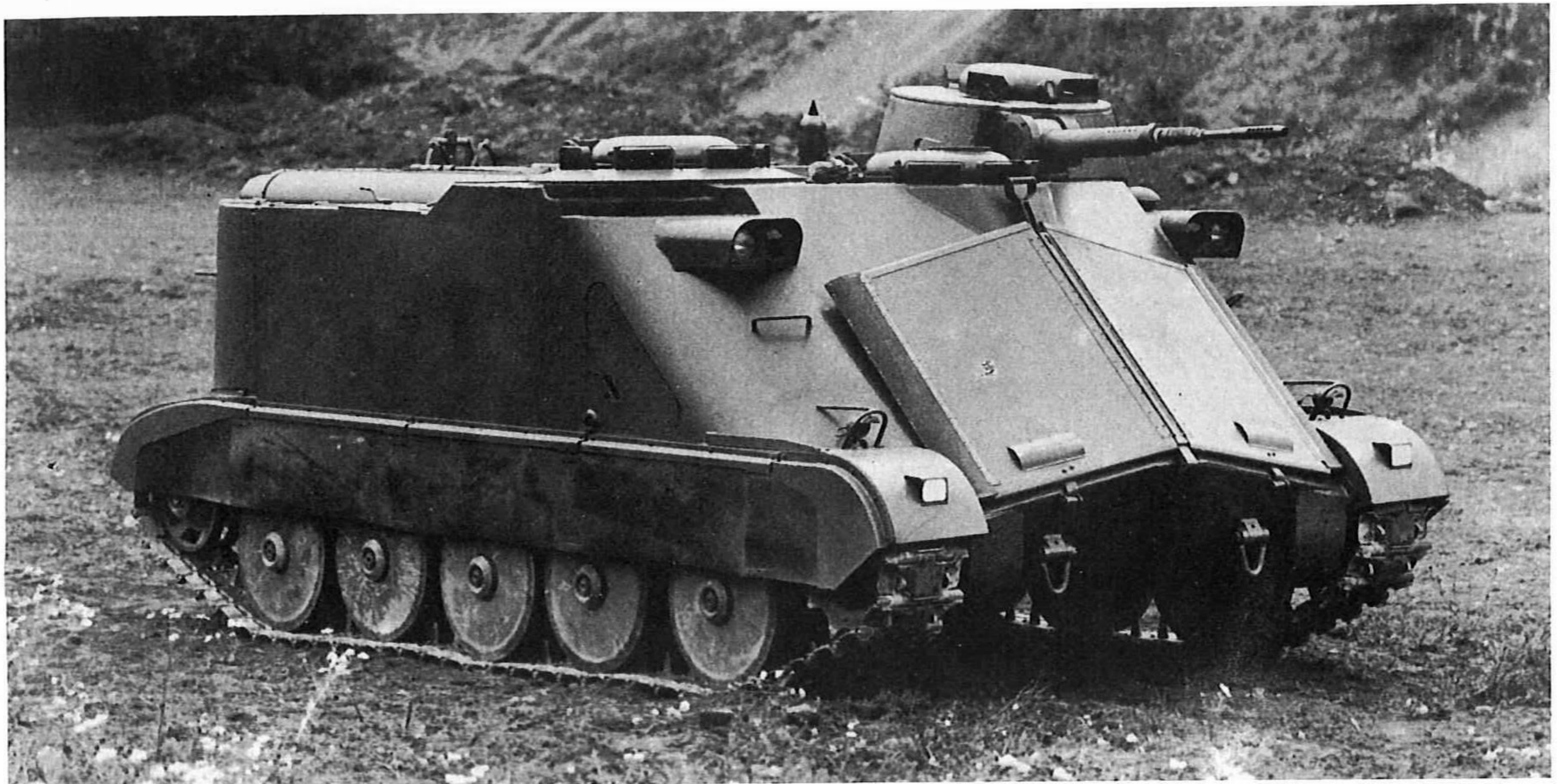
Prototype of Pbv 302, the amphibious armoured personnel carrier built by AB Hägglund & Söner.
