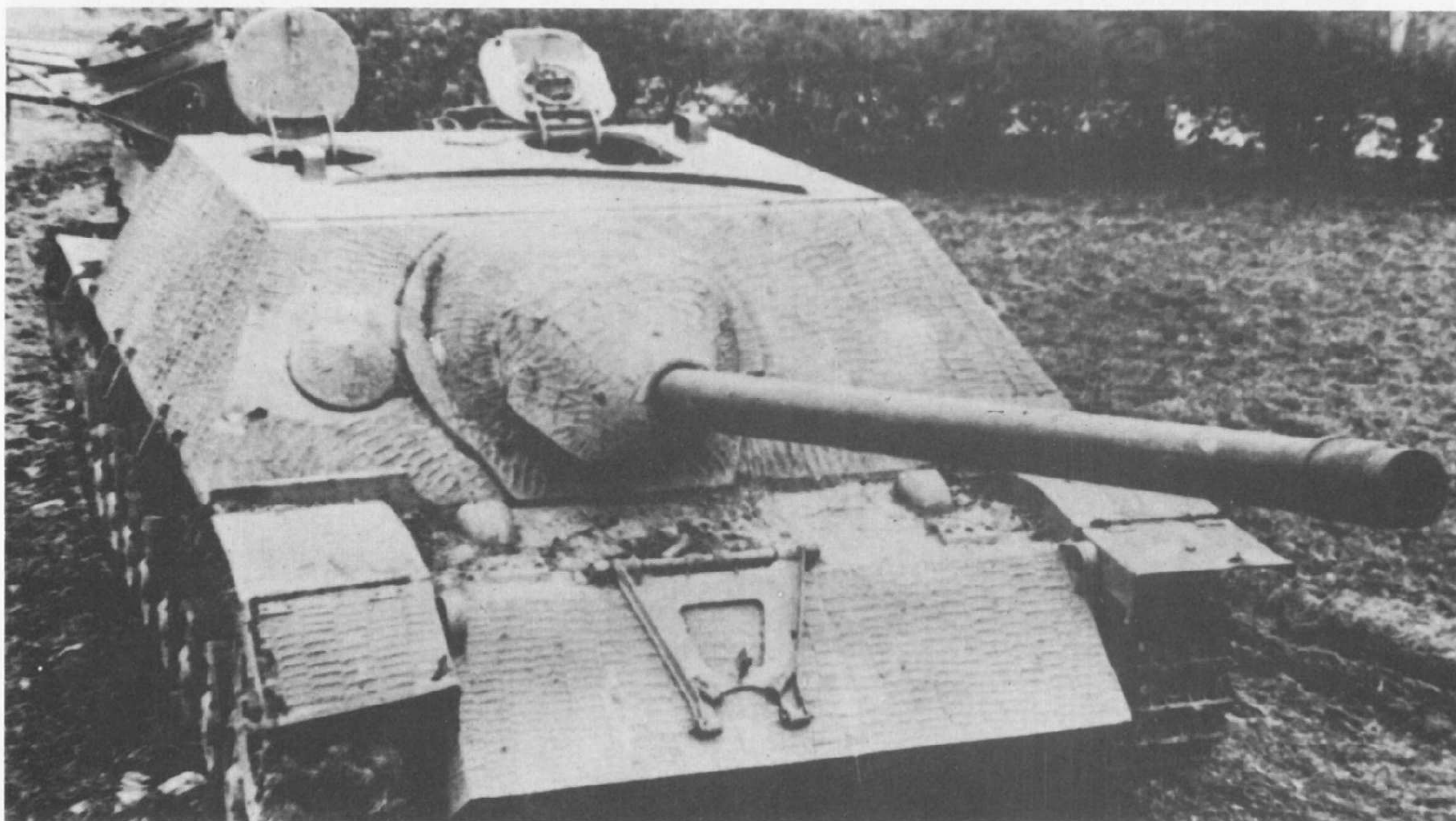
Panzer IV Ausf. F chassis were used for fully enclosed Jagdpanzer IV tank destroyers which mounted a 7.5 cm. PaK 39 L/48. Late models of SdKfz 162, one of which is shown here with Zimmerit anti-magnetic mine paste, had no port on left hand side of front plate and no muzzle brake.
