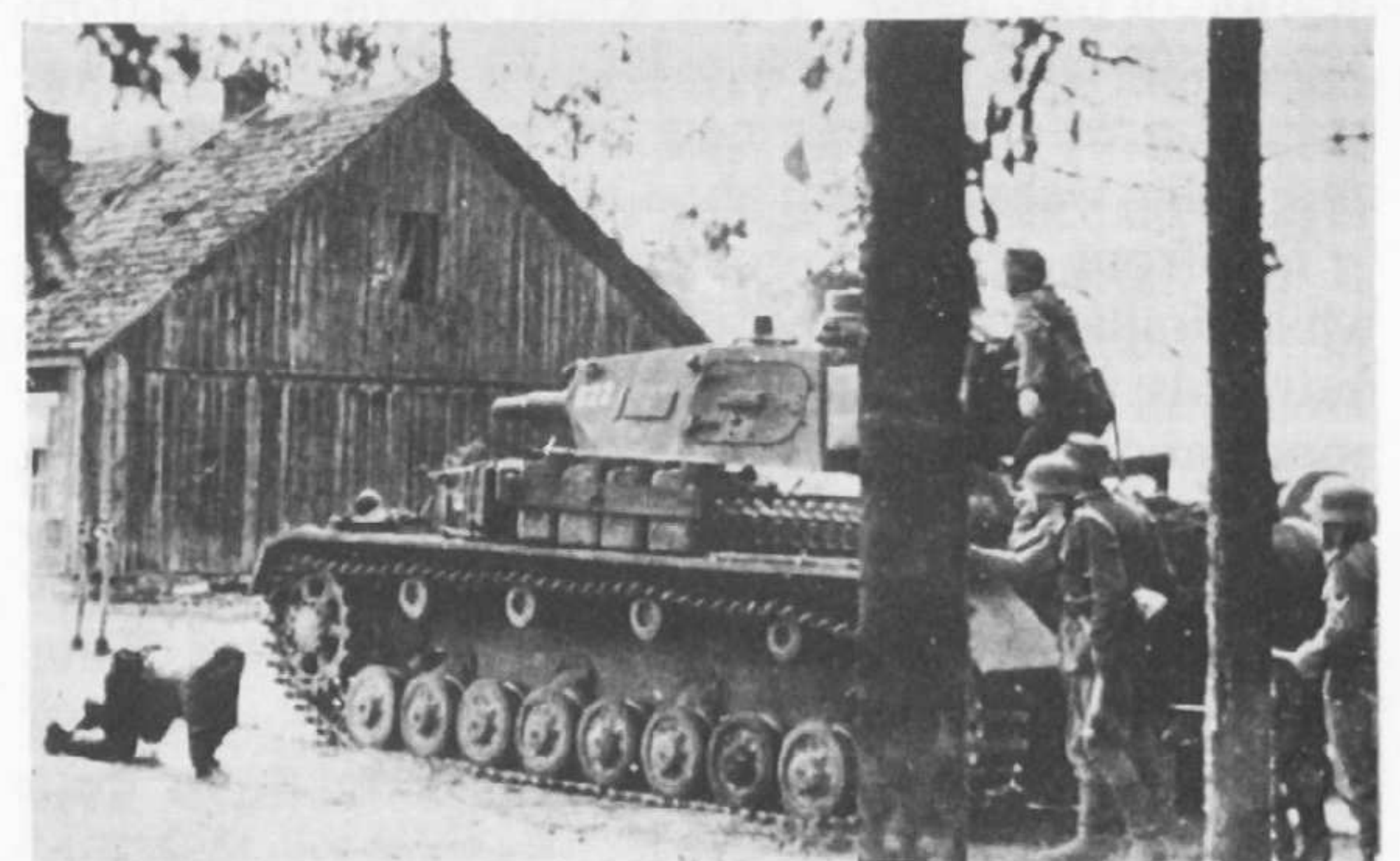
Panzer IV in action in Russia supporting infantry: Ausf. B, C, or D. Note fuel cans on side.
