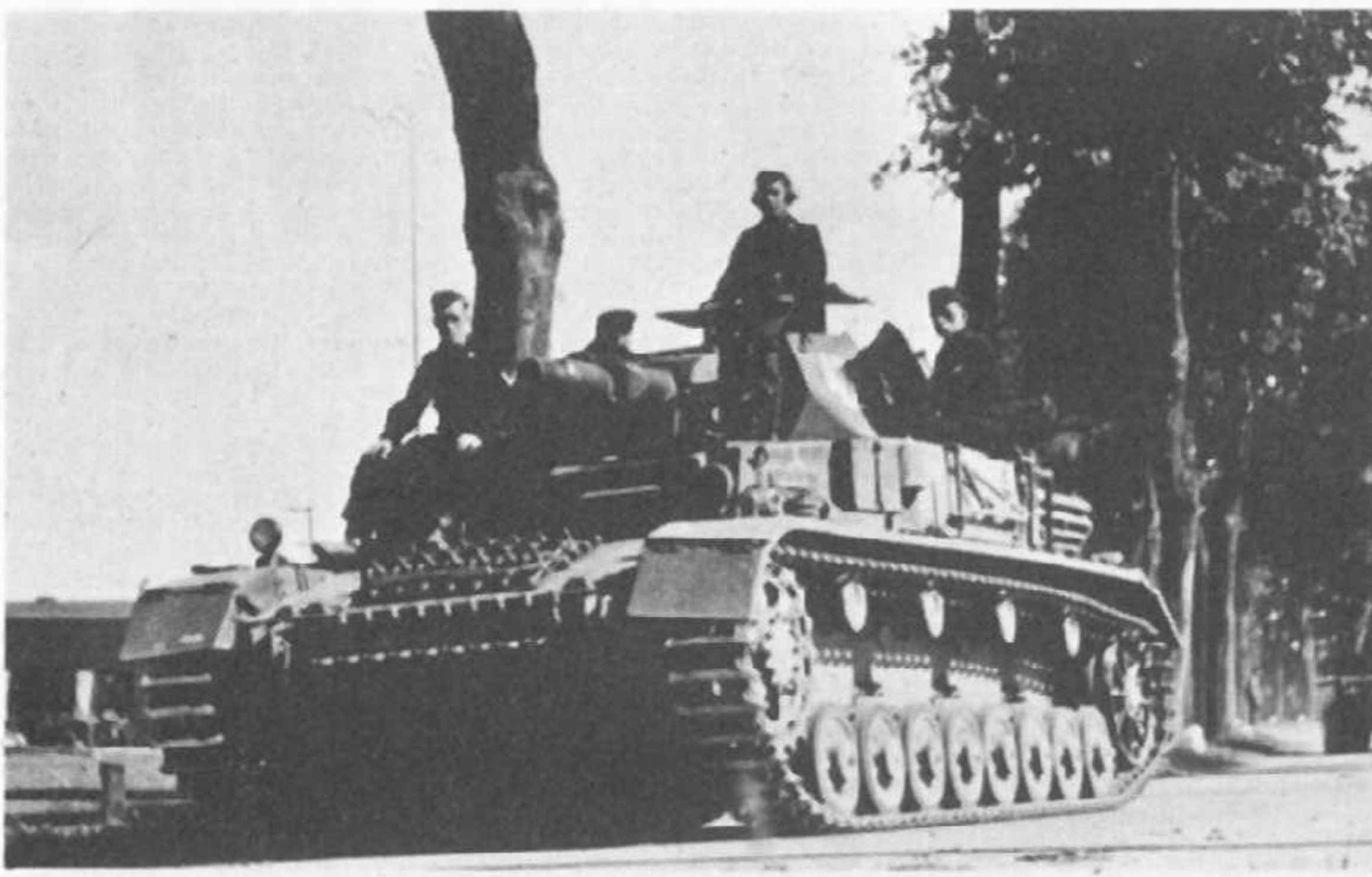
Panzer IV Ausf. A of 1st Panzer Division, only 35 of this model were built. Ausf. A had stepped front plate with driver's position protruding at left, round bow machine-gun mount at right. Driver had single centre vision slit and rectangular side view opening in front plate.
