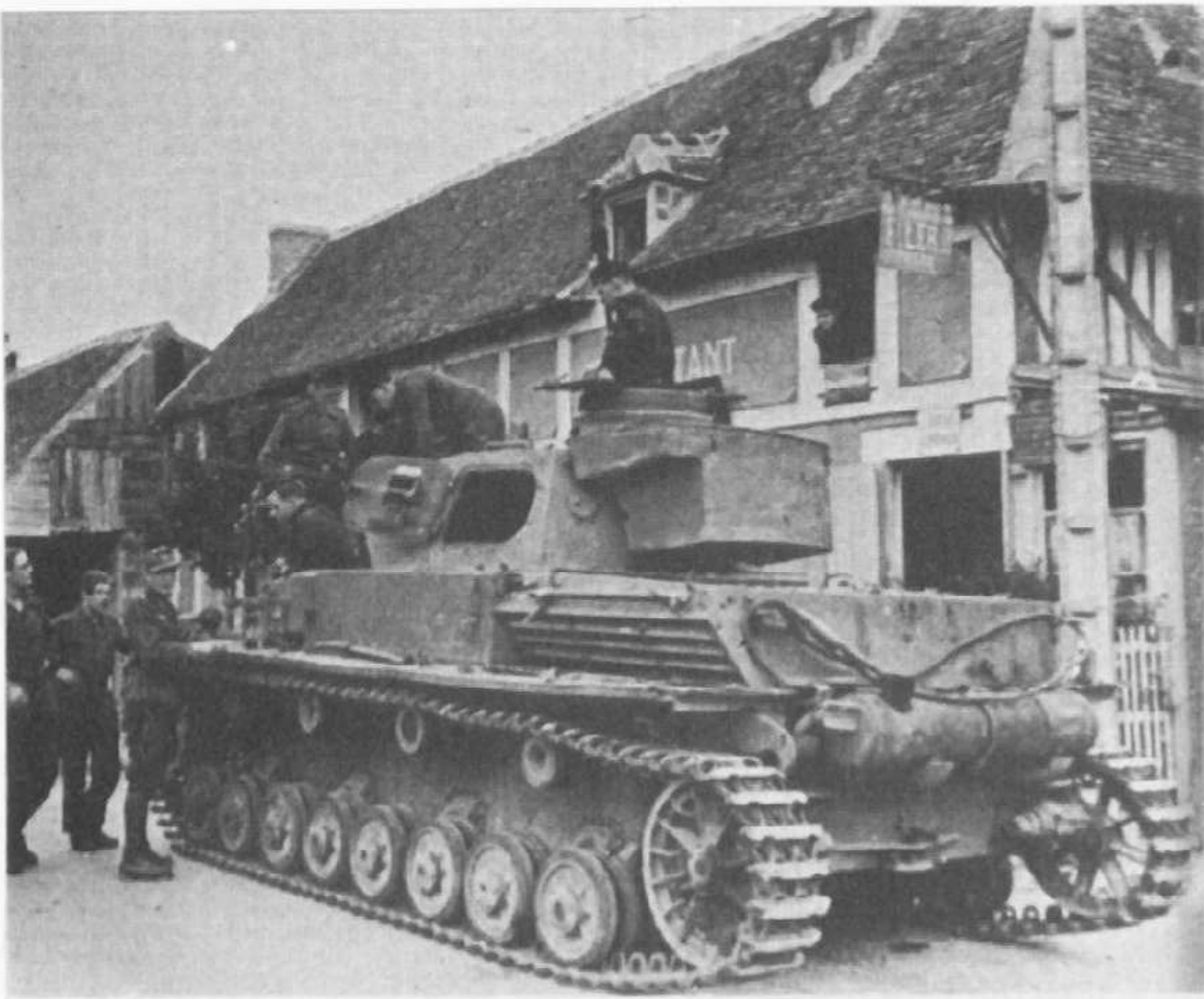
This three-quarter rear view of Ausf. B or C in France shows the single hatch door on the turret sides. Double doors were not substituted until Ausf. F. Exhaust configuration and track tensioning device are typical of all Panzer IV vehicles. Weight of Ausf. B was 17.7 tons, of Ausf. C 20 tons.
