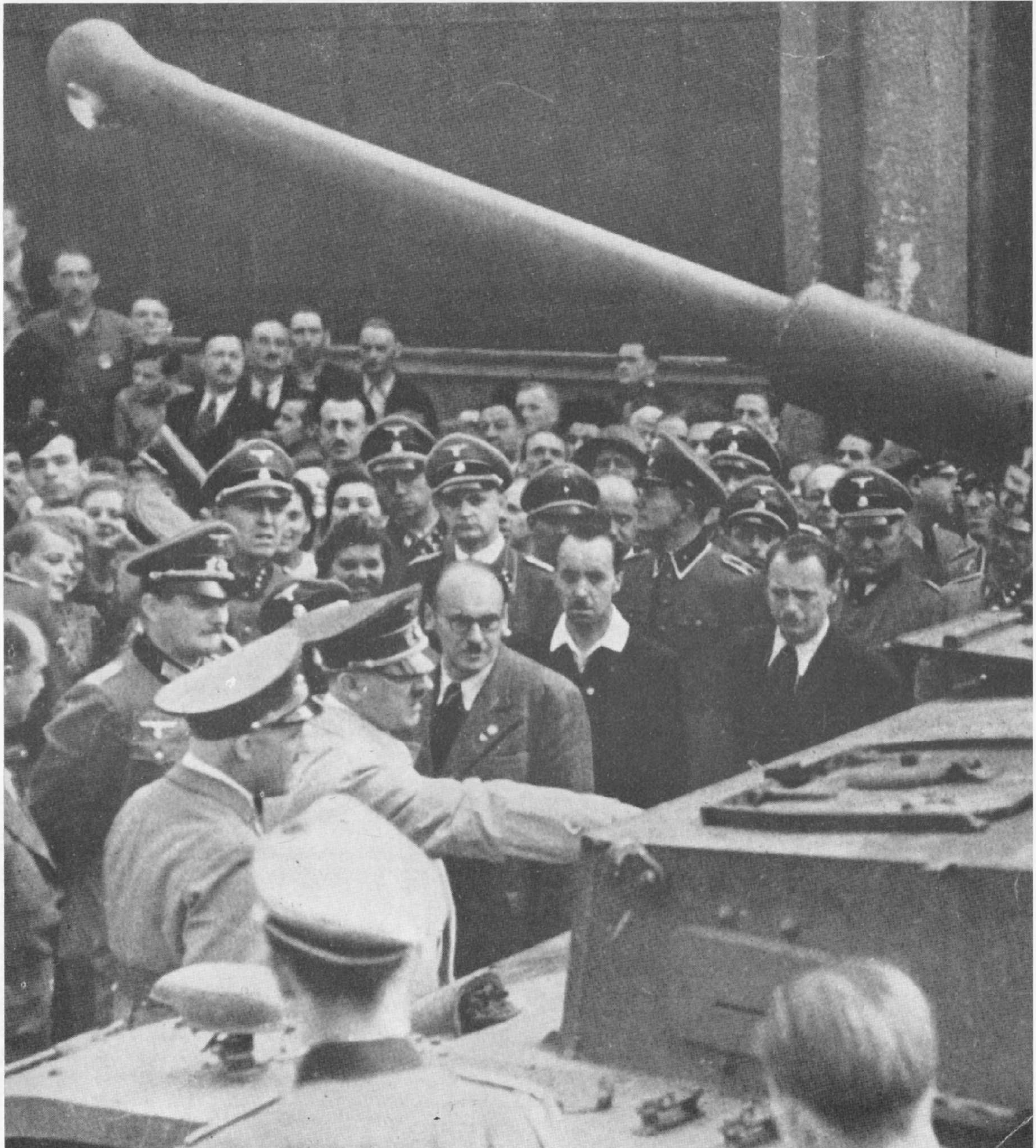
Hitler, surrounded by a ring of SS men with a single Army officer in attendance, inspects the first prototype PzKpfw IV F2, with the long-barrelled 7.5 cm. gun, at Krupp's Magdeburg factory early in 1942: note the ball-shaped, single-baffle muzzle brake of the early version.
