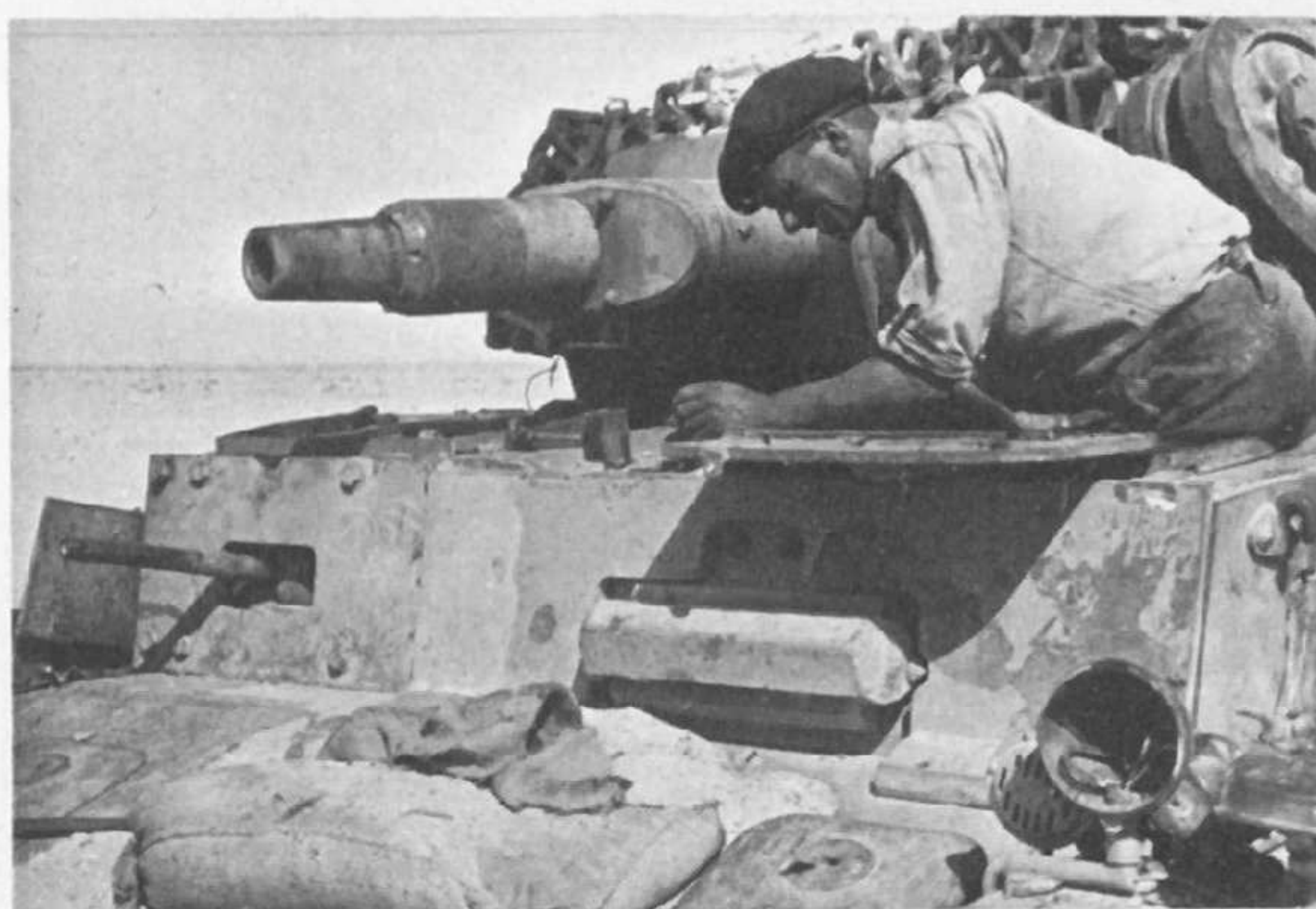
Close up of front plate of Ausf. E showing the new driver's visor with single hinged flap and the modified bow machine-gun mount.
