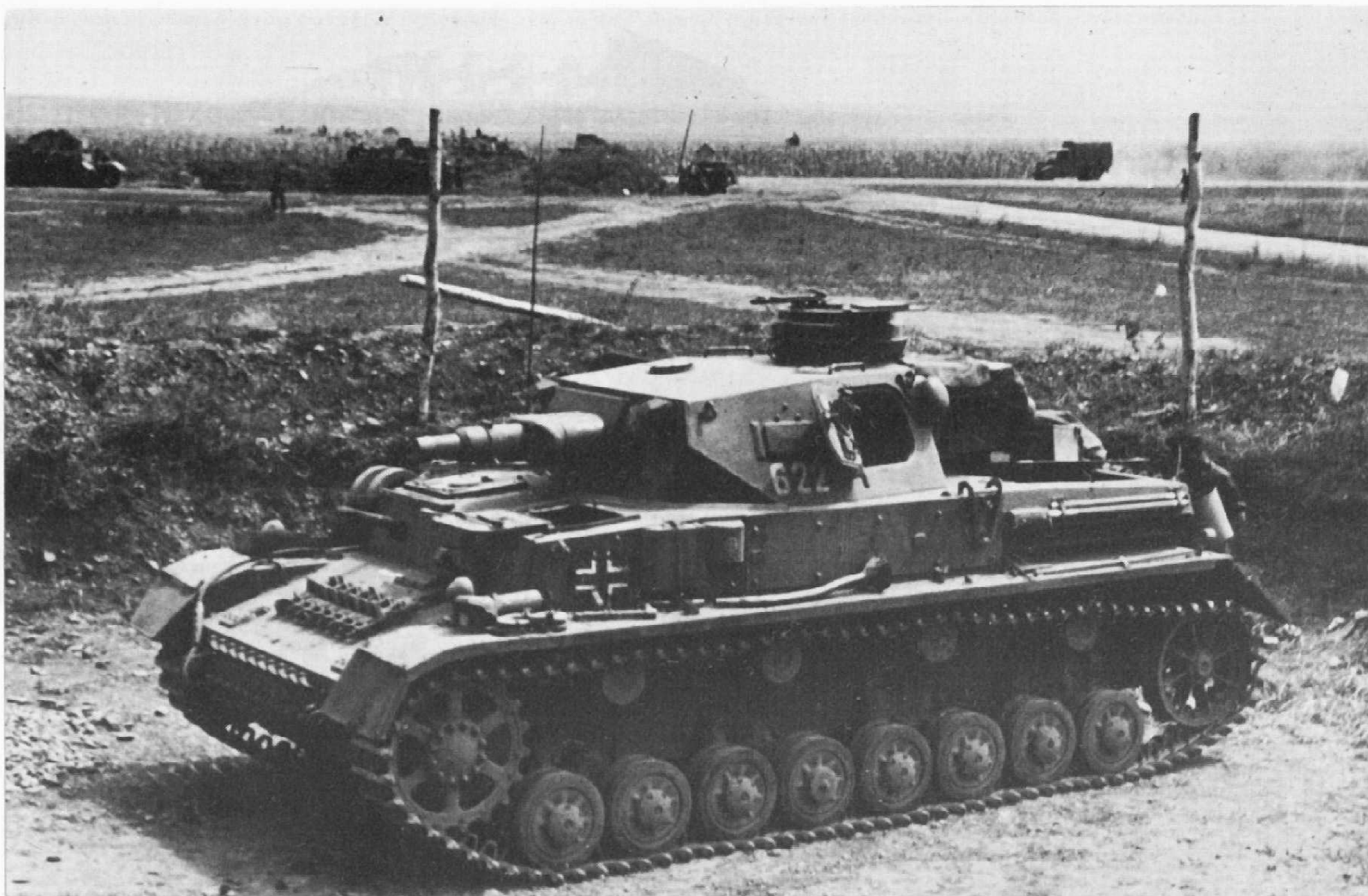
Ausf. E of 13th Panzer Division early in the Russian campaign, 1941. This model still had the stepped front plate, although with modifications to the driver's visor and the bow machine-gun mount. Other changes included: modified commander's cupola installed further forward so that it no longer protruded from the back plate of the turret which was now unbroken; increased armour on nose plate, bolted on armour for hull to improve fighting compartment protection (see picture), spaced armour in front of bow machine-gun and sometimes in front of driver's position; replacement of rectangular ventilator flap on turret roof by fan ventilator, and removal of cone-shaped single port flap which was replaced by a flat lid (see picture: the new ventilator is half-way along the turret roof in front of the cupola).
