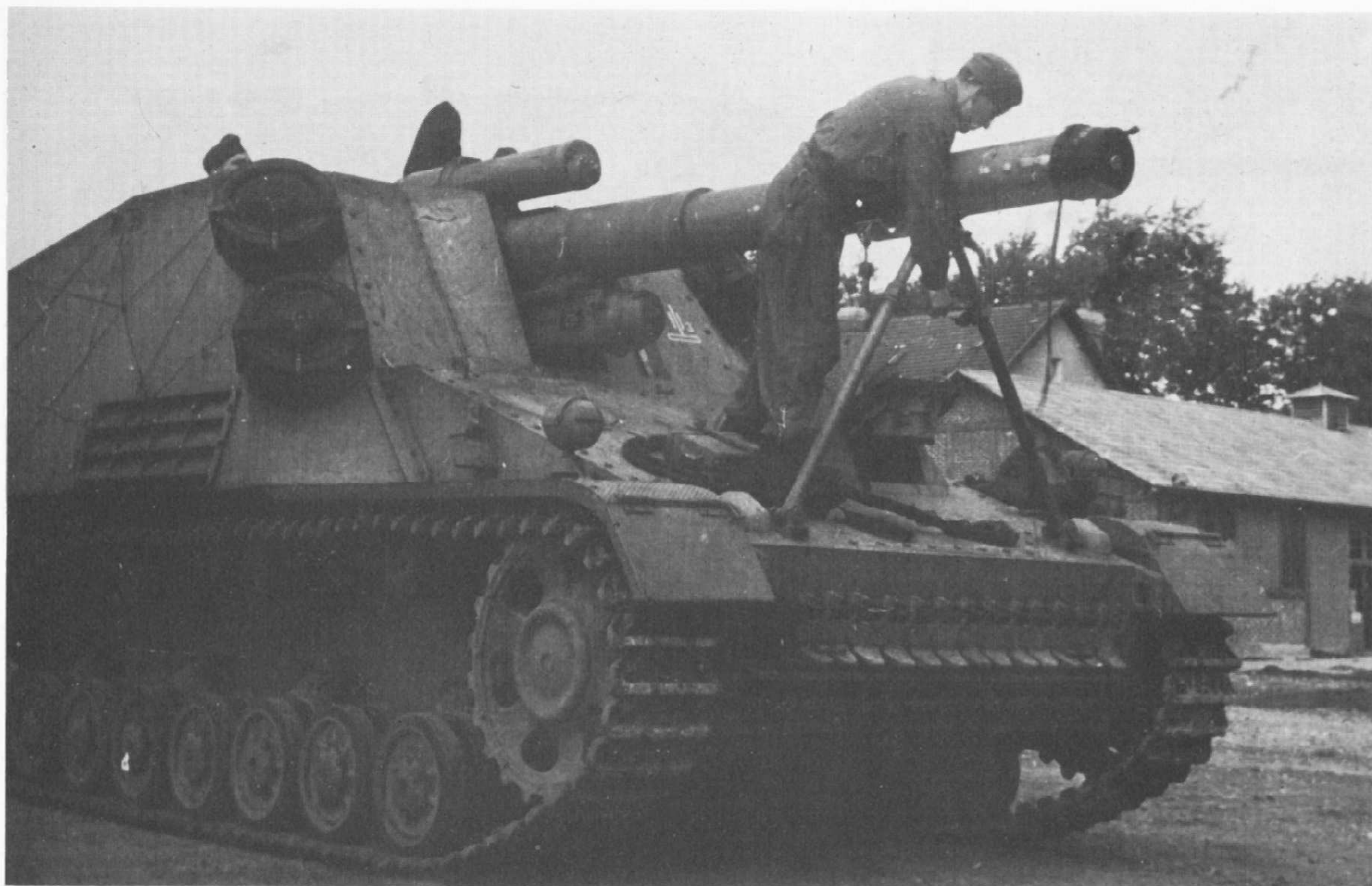
Built on a similar chassis to the Nashorn, the self-propelled 15 cm. howitzer Hummel (Bumble-bee) was a highly successful piece of Panzerartillerie.
