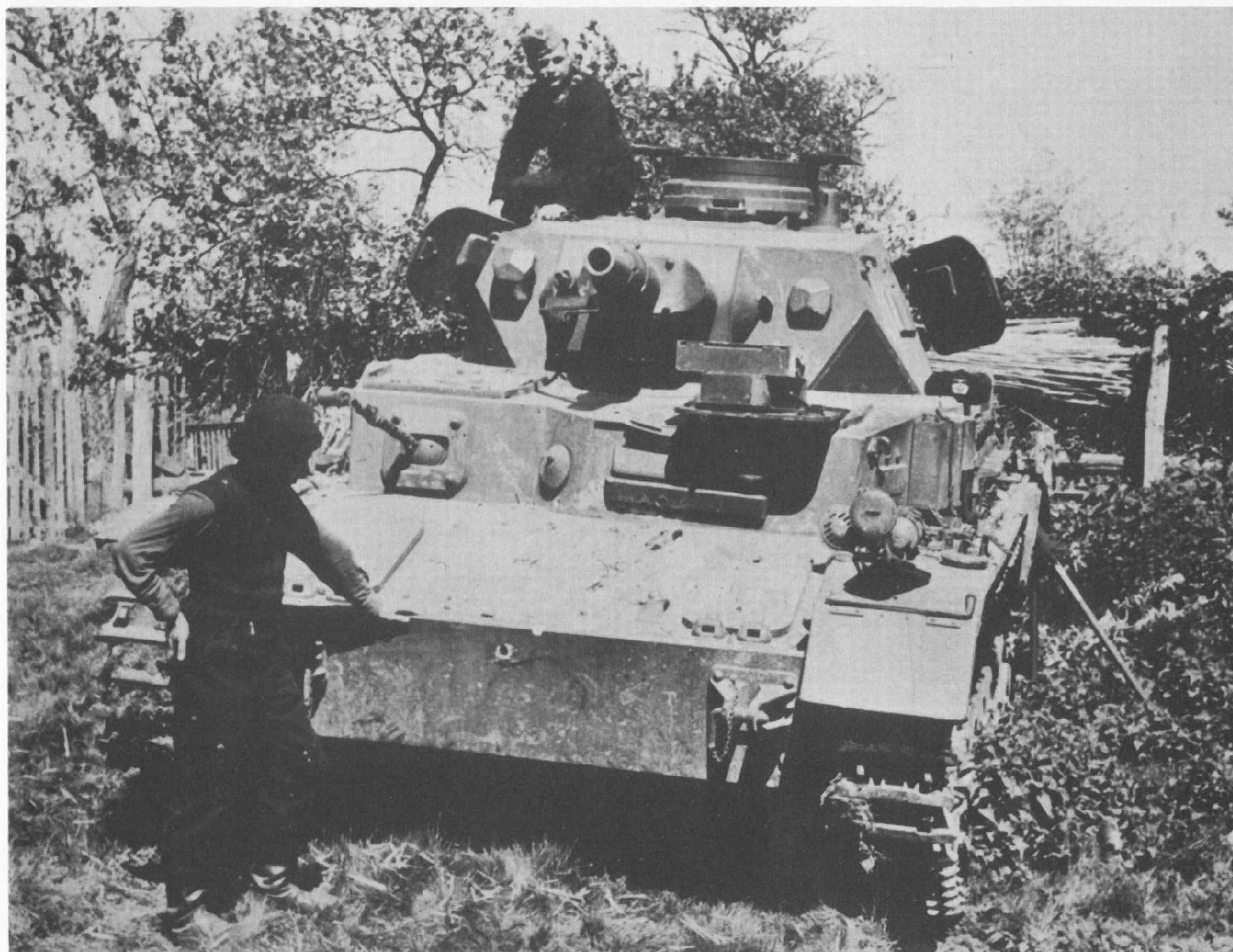
Ausf. D again had a stepped front plate like Ausf. A, but the bow machine-gun for the radio operator was now in a square shaped mount with internal ball. The driver had a side opening for a sub-machine-gun. The mantlet for the main armament was external, as opposed to the internal mantlet on all earlier models.
