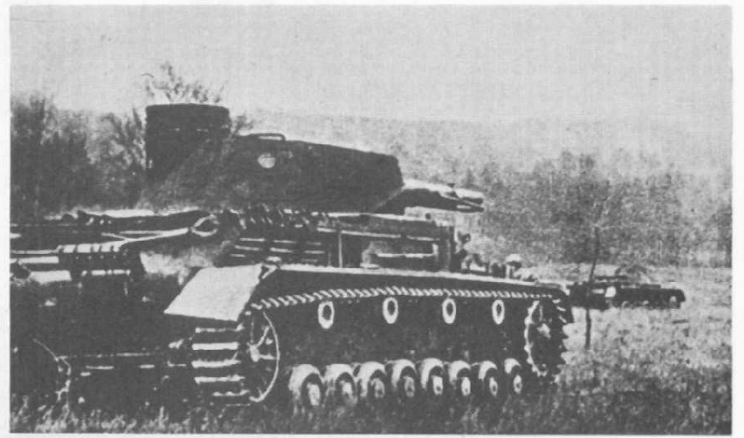
Another recognition feature of Ausf. A was the drum-shaped commander's cupola protruding through rear plate of turret. Engine was Maybach HL 108. Weight 17.3 tons.
