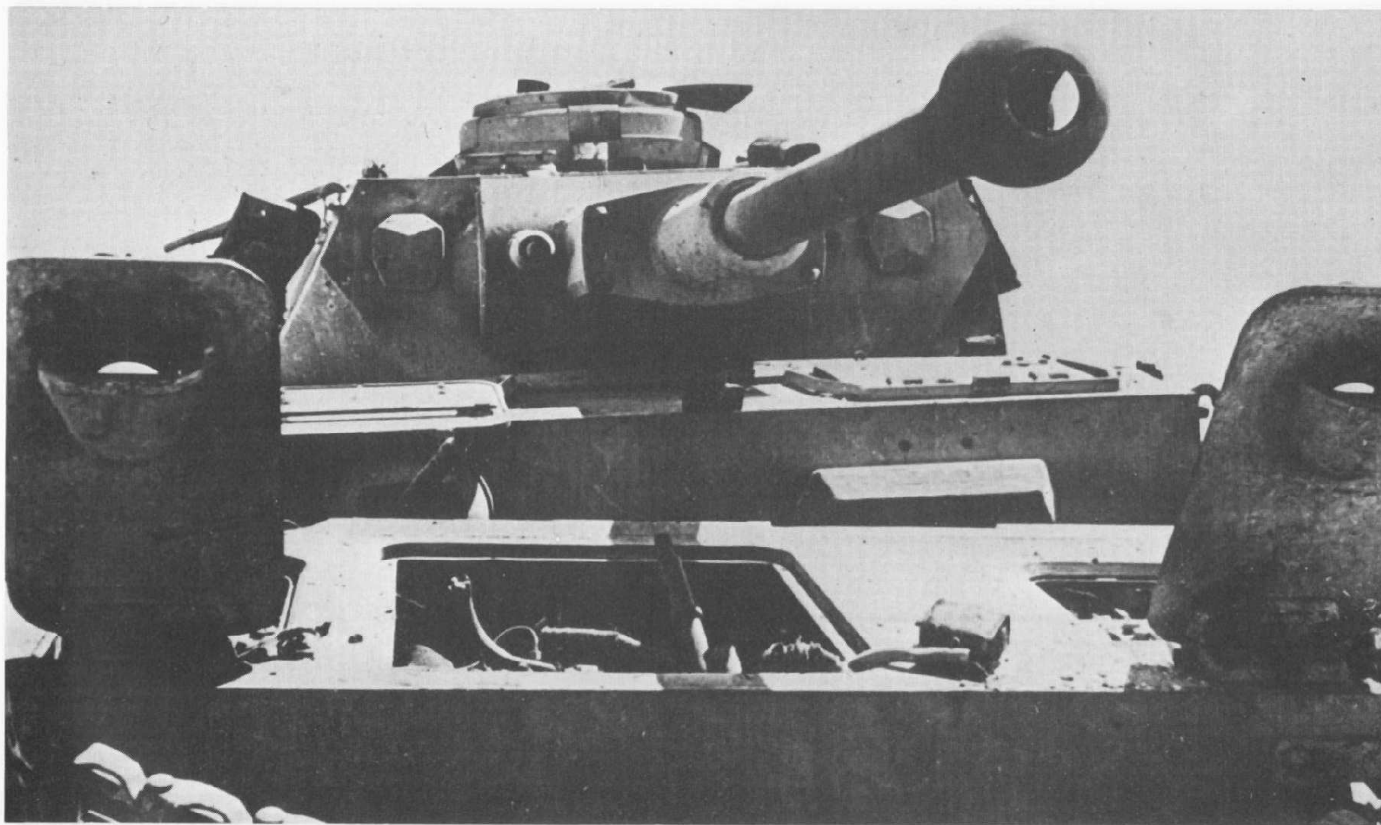
Ausf. F2 destroyed by its own crew in the Libyan desert; numbers of tanks had to be abandoned as fuel and spare parts shortages increased under British blockade. Note the raised glacis plate access doors; these were changed from earlier models, each door having an air intake cowl.
