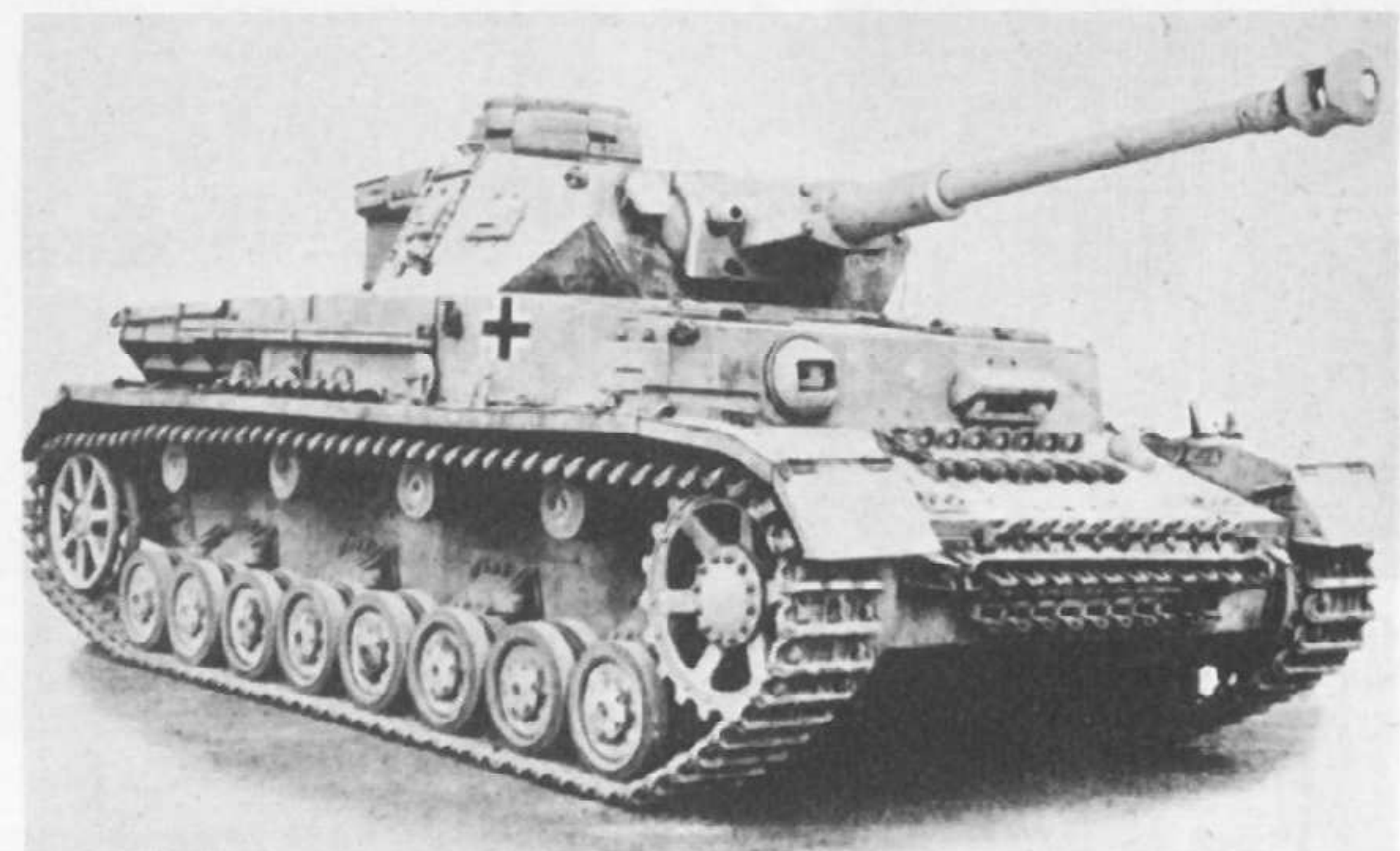
Ausf. G had a double-baffle muzzle brake on its KwK 40 L/43. In other respects it was similar in appearance to Ausf. F2. Its side armour, however, was 30 mm. compared with 20 mm. + 20 mm.
