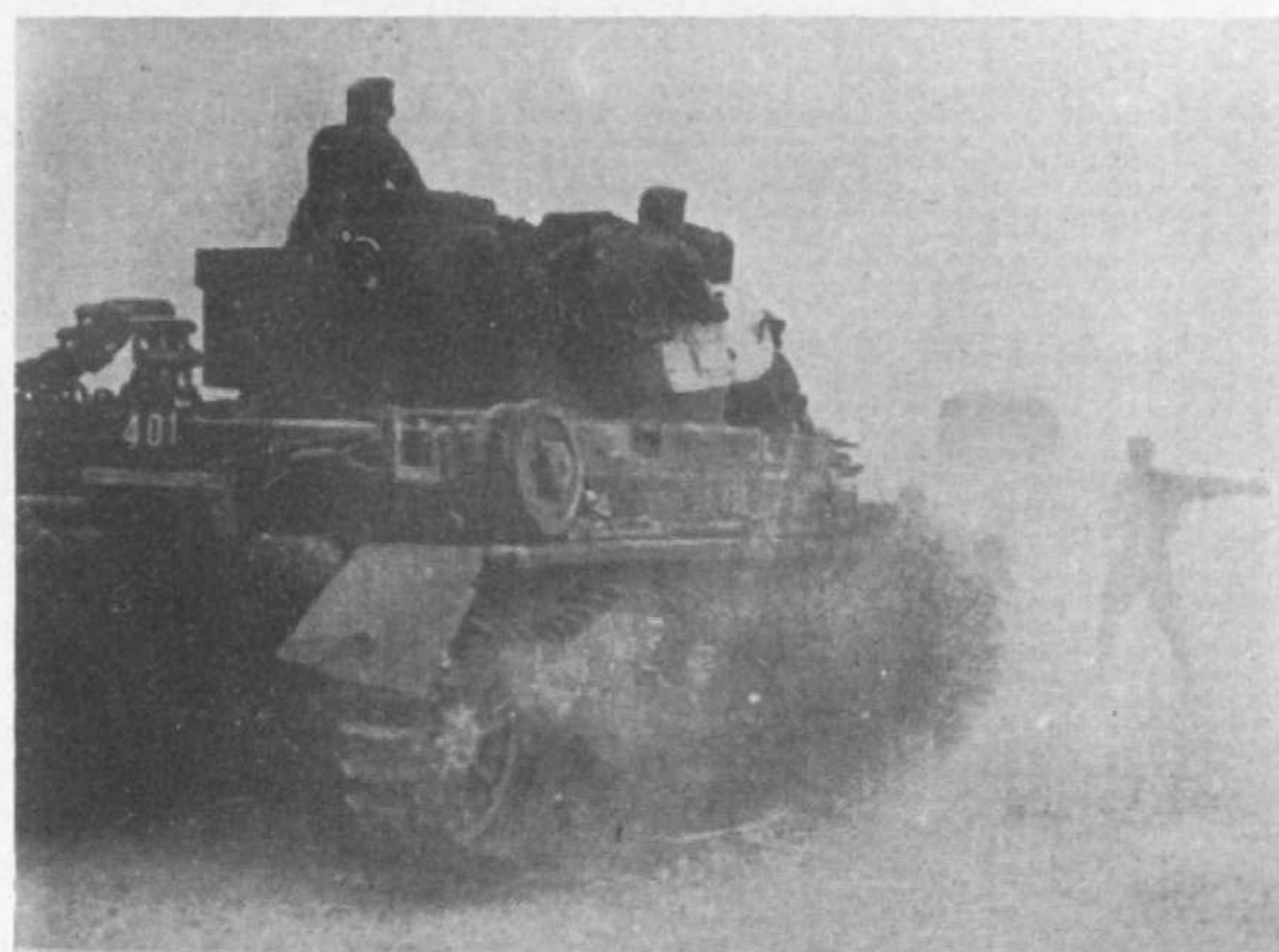
Ausf. E moving up for action in North Africa. Chassis numbers of this model were 80801 to 82000. Weight was 21 tons.
