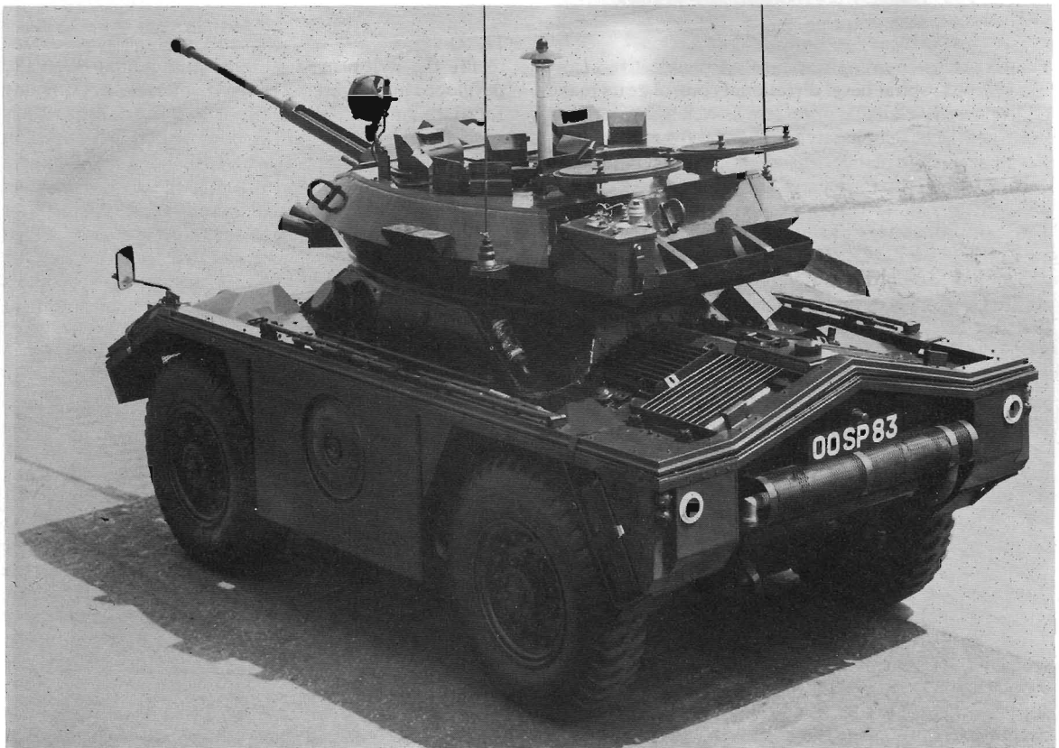
Rear view of a Fox prototype with Radiac mast on the turret.
