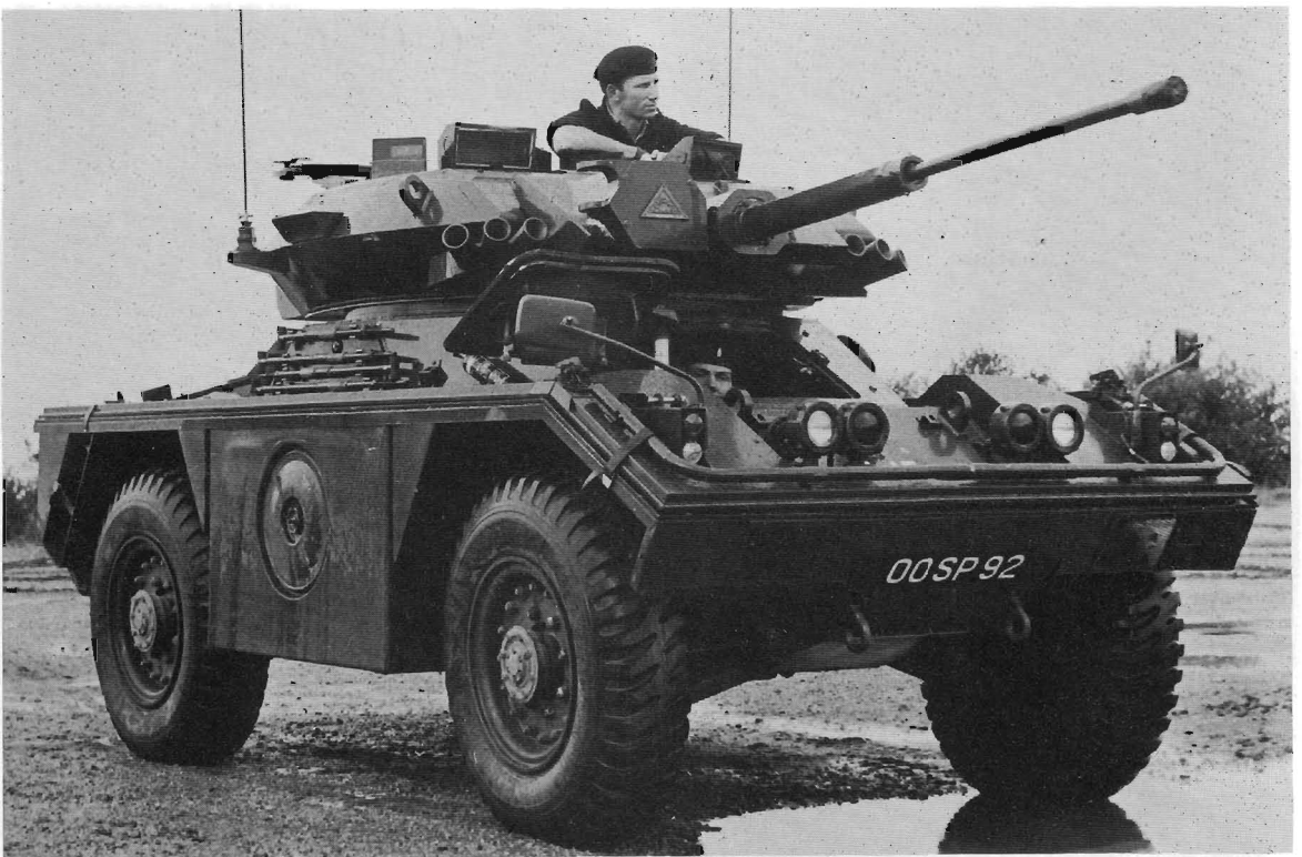
Prototype of the Fox with turret mounting a 30 mm. Rarden gun.
