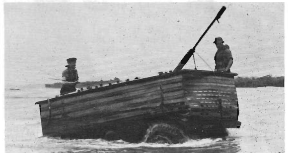
Fox coming ashore with its flotation screen erected. (MVEE)
