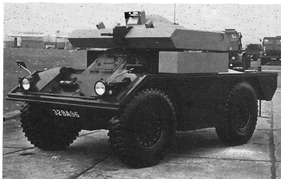
Ferret Mark 5 with mock-up turret for Swingfire missiles. (British Aircraft Corp.)
