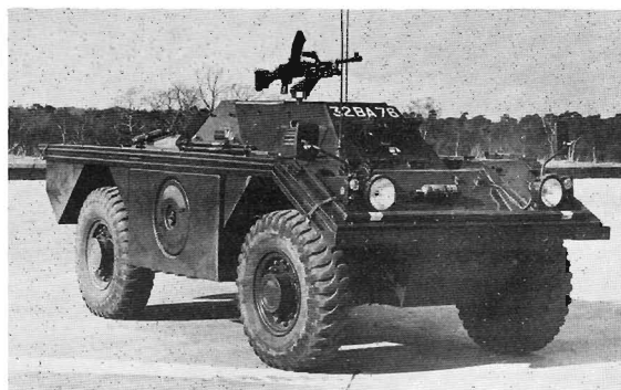
Ferret Mark 1/3 with flotation screen.
