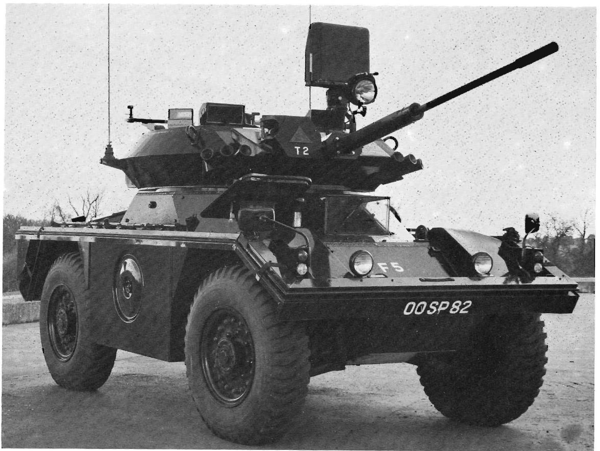
Late development version of the Fox with surveillance radar.
