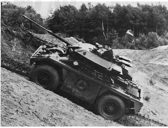
A Fox prototype demonstrating its ability to climb a steep slope. (Alvis)
