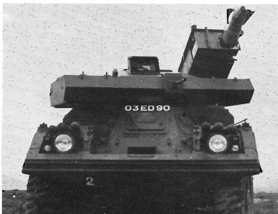
Ferret Mark 5 with a Swingfire missile emerging out of its container/launcher. (British Aircraft Corp.)
