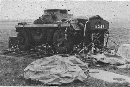
Ferret Mark 1 mounted on a platform on which it was dropped by parachute. (MVEE)
