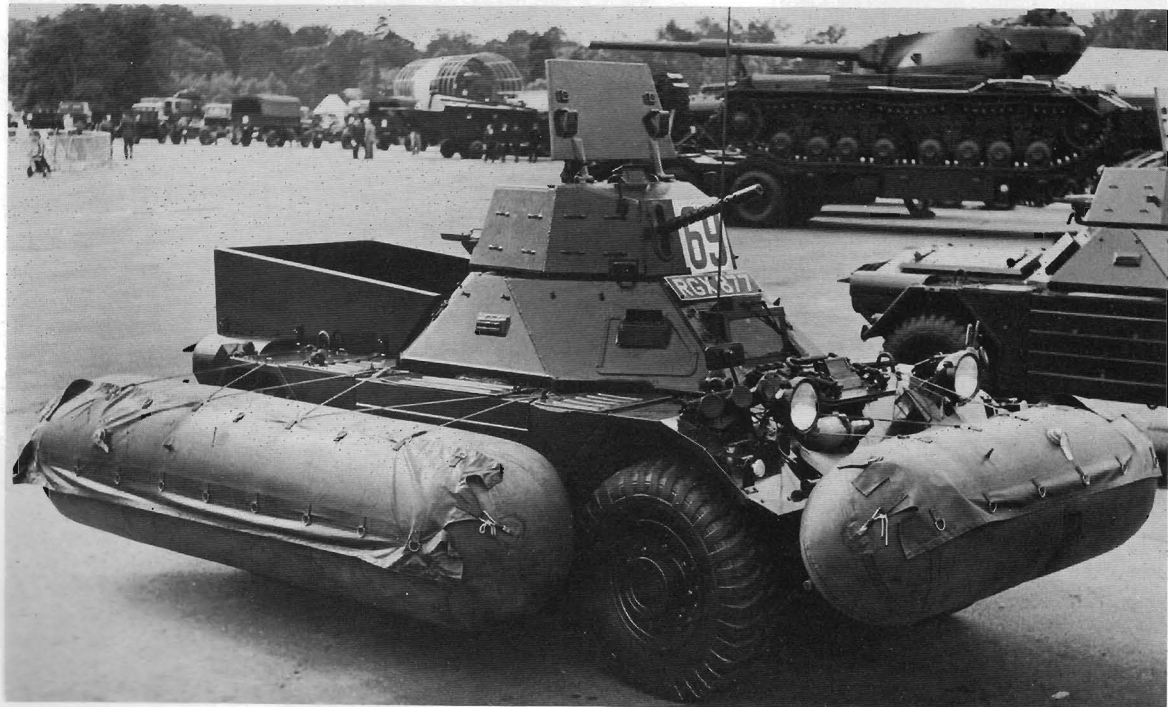
Ferret Mark 2 with inflatable buoyancy bags.
