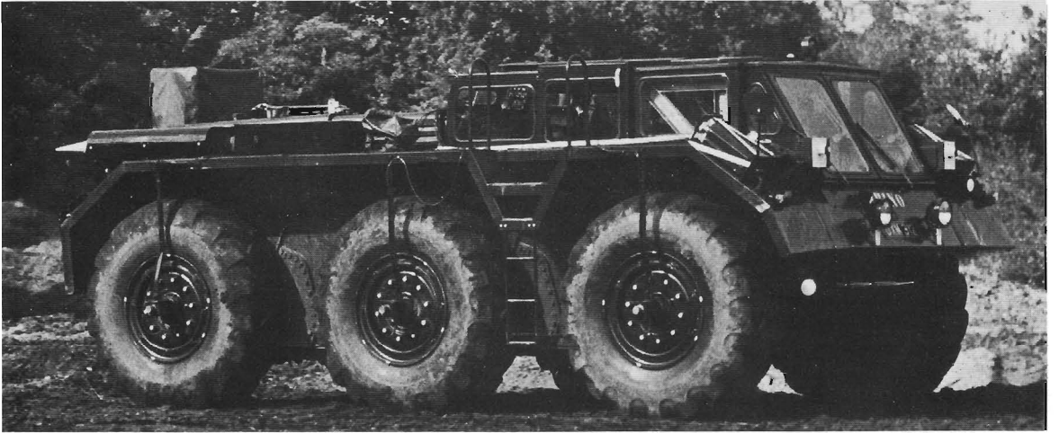
TV 1000 test vehicle with skid-steering.
