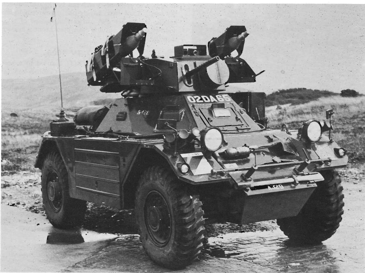
Ferret Mark 2/6 with Vigilant anti-tank guided missiles. (MVEE)
