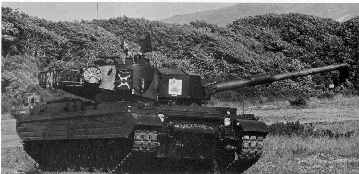
Mark I showing its rubber padded tracks.
