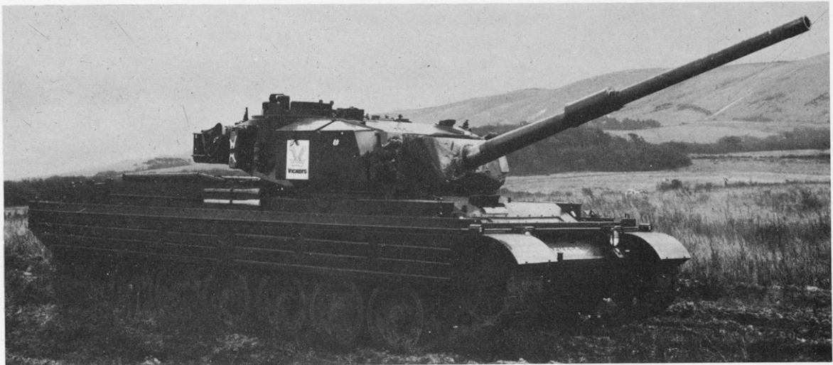
Vickers battle tank Mark 1 with trough for flotation screen.
