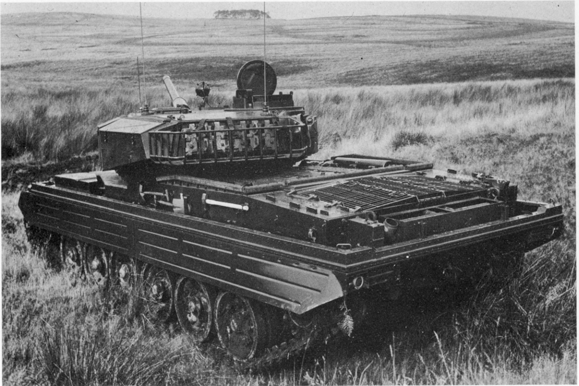
Rear view showing the louvres over the engine compartment.
