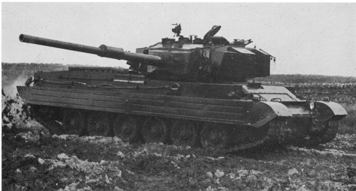
Vickers battle tank moving at speed: note the absence of the trough for the flotation screen.
