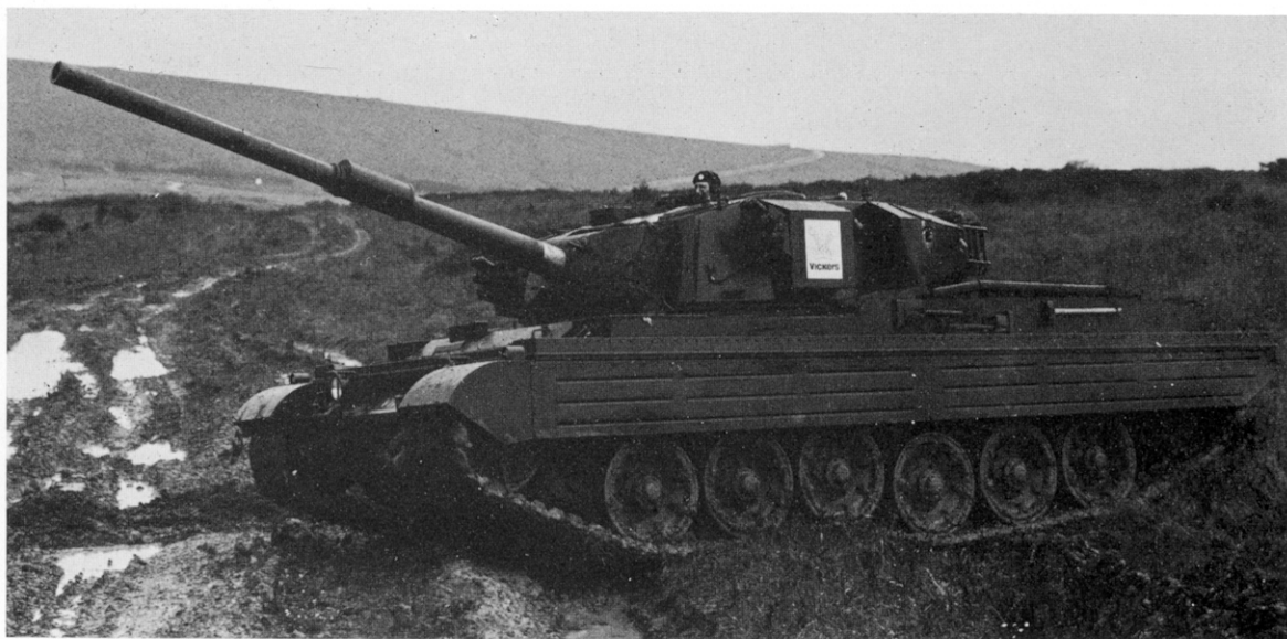
View showing the independently sprung road wheels.
