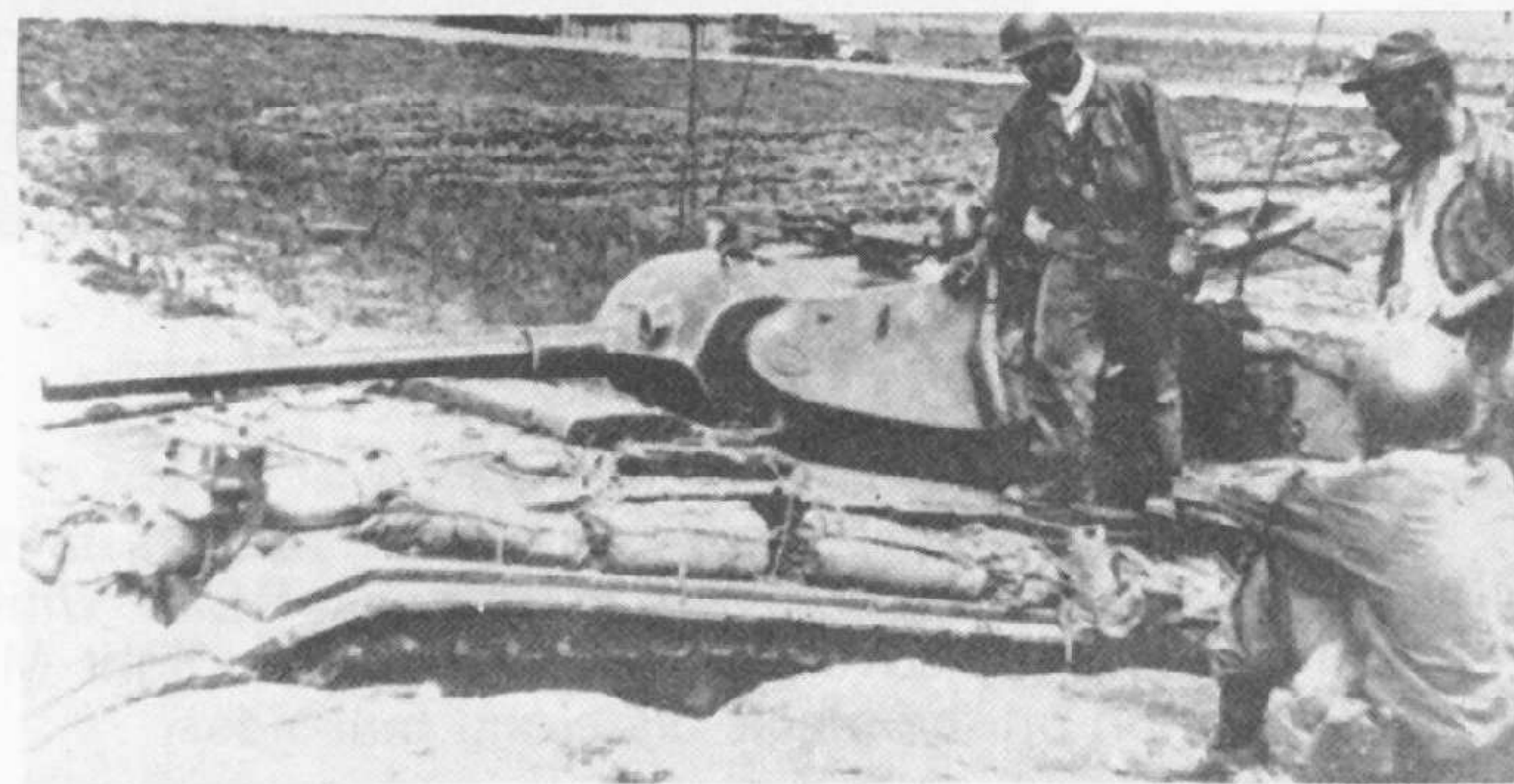
An M.24 light tank in dug-in position in Korea with 75 mm. gun facing rear permitting rear guard defence to make a rapid getaway. (U.S. Army photo)
