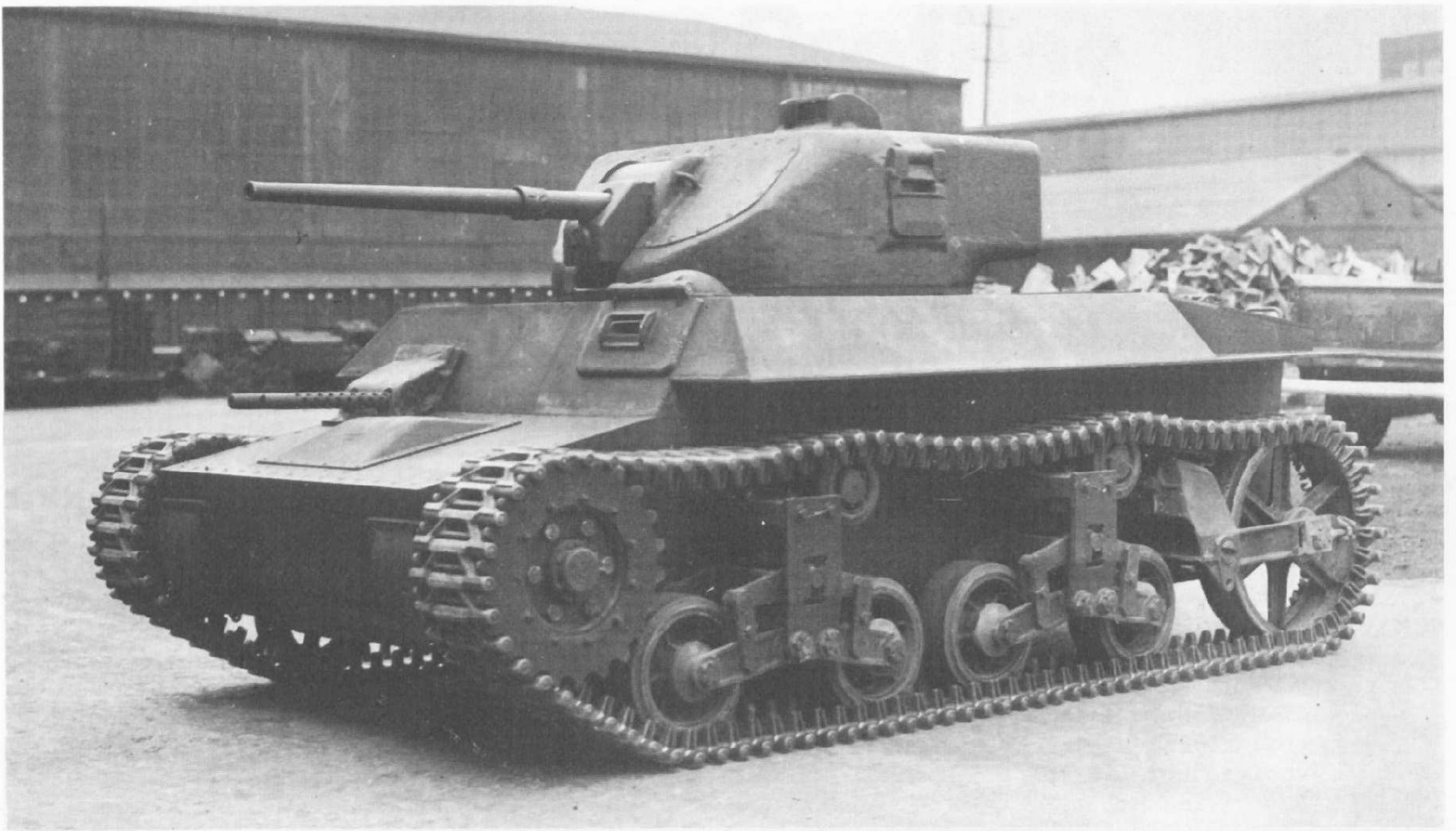
The T9 with original suspension, turret, bow, dual bow guns, and driver's hatch.
