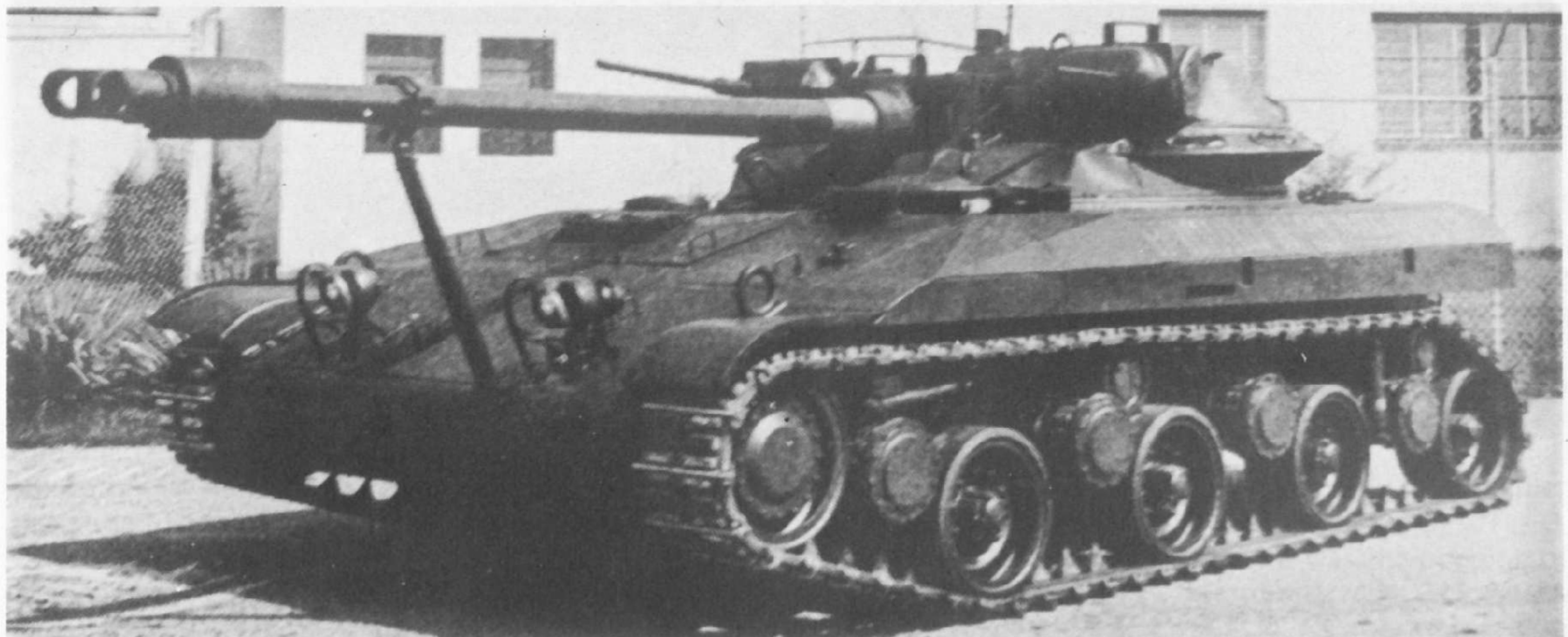
Above: The T92 Airborne Light Tank built by Aircraft Armaments Inc. had its gun in a cleft turret. Prototypes were built in 1956 and 1957 but the T92 was not adopted. (Aircraft Armaments Inc.)
