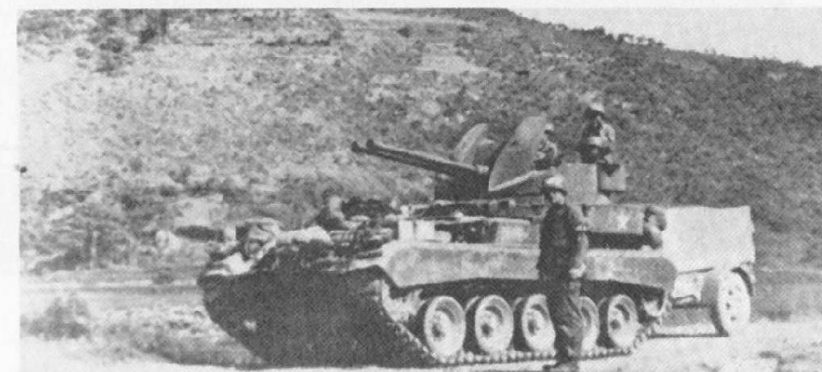
A multiple gun motor carriage M.19 mounting twin 40 mm. guns and towing an extra ammunition trailer preparing to move forward near Yongsan on 18th August 1950. (U.S. Army photo)
