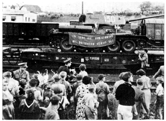
T-34/85 loaded on a rail flat preparatory to the Soviet withdrawal from Austria in August 1955. The forward-mounted turret ventilator can be clearly seen. The banner reads "Long live the Soviet Union that freed Austria." (Keystone)
