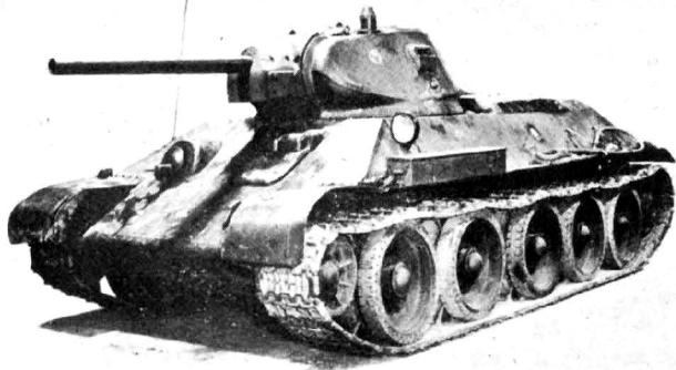
A representative T-34/76B with "long" 76.2-mm. gun, 41.2 calibres. Armour thickness is improved but standard turret fittings of the "A" model are retained including side episcopes, pistol ports, back plate and single, forward opening roof hatch. (Imperial War Museum)
