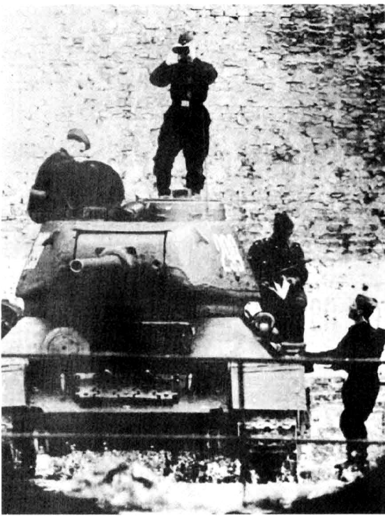
Maintaining a watch on West Berlin from a T34 during the uprising in the Soviet sector in June 1953. The Christie-type of track plate is unmistakable. (Keystone)
