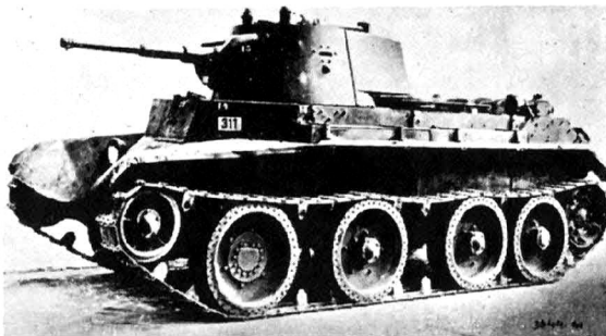
BT-7—an improved version of the Christie-type BT-5 retaining wheel-and-track feature. First introduced in 1935 with 45-mm. gun and 400 h.p. engine, it was up-gunned with a 76.2-mm. gun in 1938 and subsequently served as a test vehicle for the V2 500 h.p. diesel engine as installed in T-34 and later Soviet tanks. Weight: 13.8 tons (original vehicle), 14.6 tons (improved version). (Imperial War Museum)
