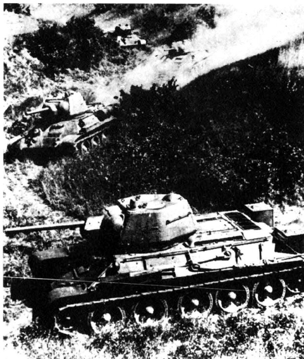
In action on the Eastern Front 1943, these T-34/76B's show the modified turret with twin hatches for commander/gunner and loader. Note absence of pistol ports in turret sides, also non-standard stowage bins at rear. The grab rails on turret and hull sides (for infantry) were also a modification. (RAC Tank Museum)
