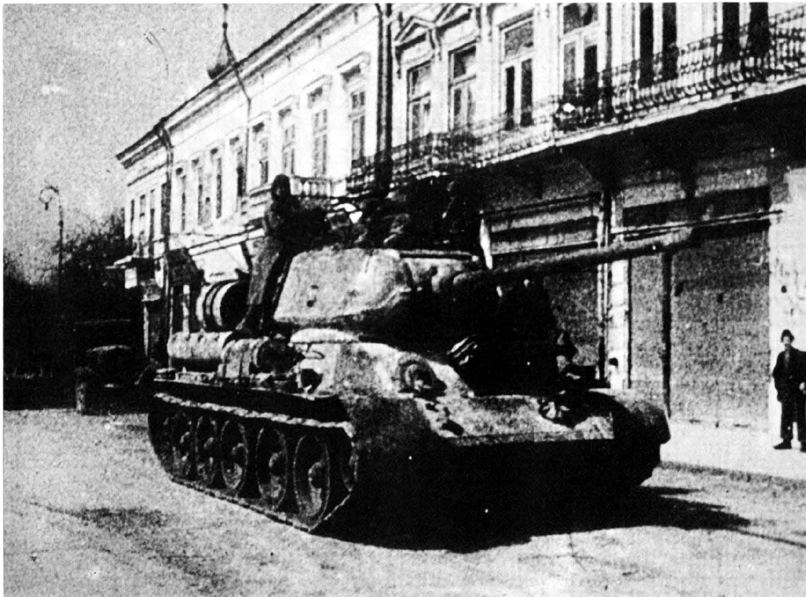
T-34/85 moving through a town in Poland. Extra fuel drums are carried on the rear deck because of the shortage of logistic transport. (RAC Centre)
