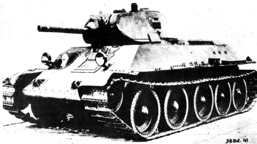
T-34/76A—the first of the famous series, put into production in June 1940. "Short" 76.2-mm. gun, 30.5 calibres; weight: 26 tons. Note very narrow (and consequently cramped) two-man turret.
