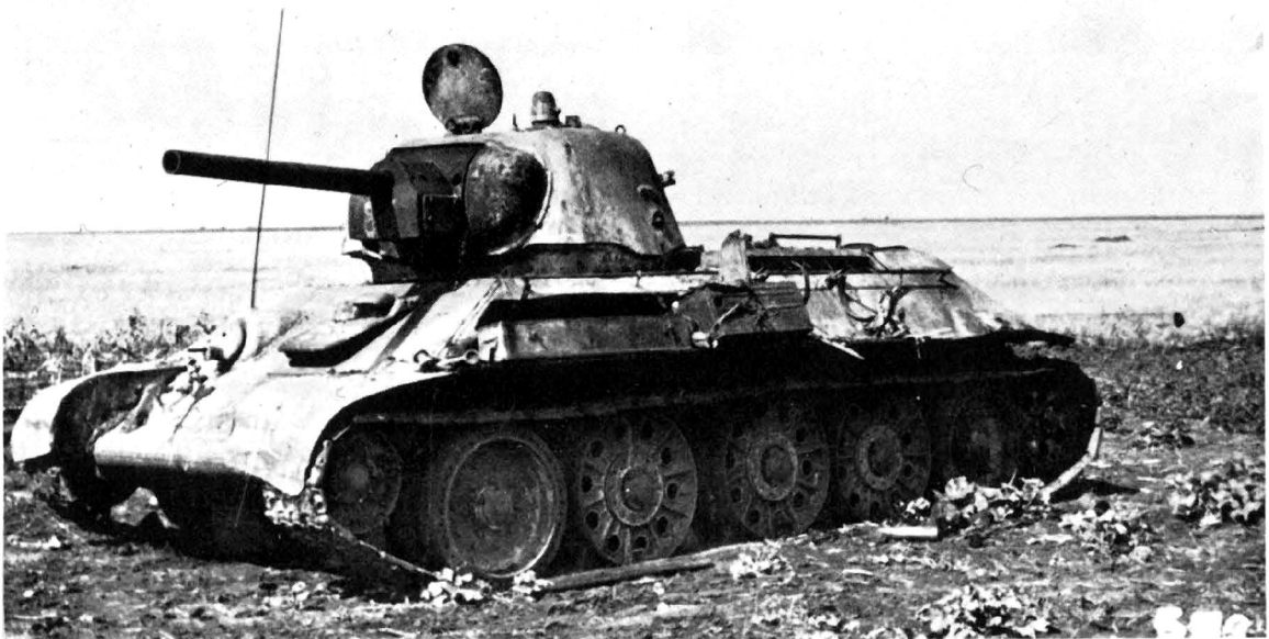
This T-34/76 with modified turret shows an odd combination of early type of perforated steel-tired wheels with the final rubber-tired disc type. There was no doubt a spares problem in the field. (Warpics)
