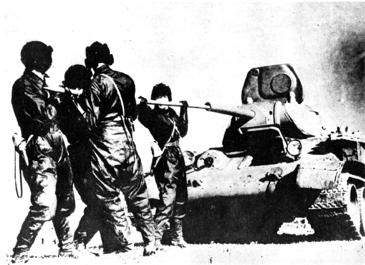
T-34/76A with original turret. Note clumsy one-piece turret hatch (also used on later models)—and crew overalls.
