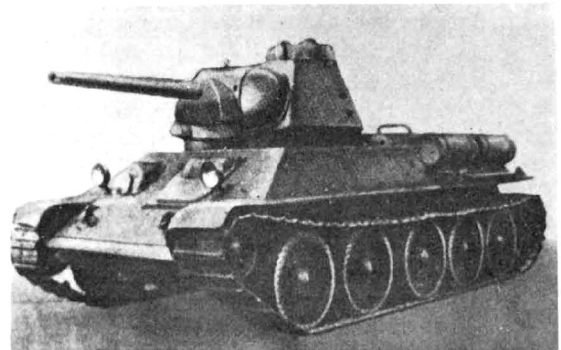
T-34/76C with commander’s cupola and welded turret. (F. M. von Senger und Etterlin)
