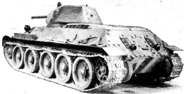
A representative T-34/76B with "long" 76.2-mm. gun, 41.2 calibres. Armour thickness is improved but standard turret fittings of the "A" model are retained including side episcopes, pistol ports, back plate and single, forward opening roof hatch. (Imperial War Museum)
