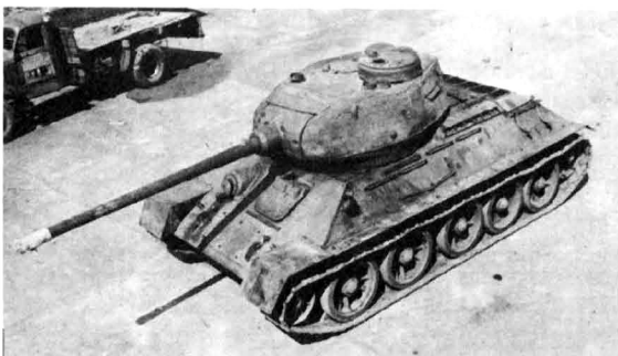
Four views of a T-34/85 captured in Korea and now in the Royal Armoured Corps Tank Museum, Bovington, Dorset. Noteworthy features are the poor ballistic shape of the turret base, the handrails for the supporting infantry, the brackets for the external fuel tanks, the well-sloped hull armour, and the wide tracks. (CCR MVEE)
