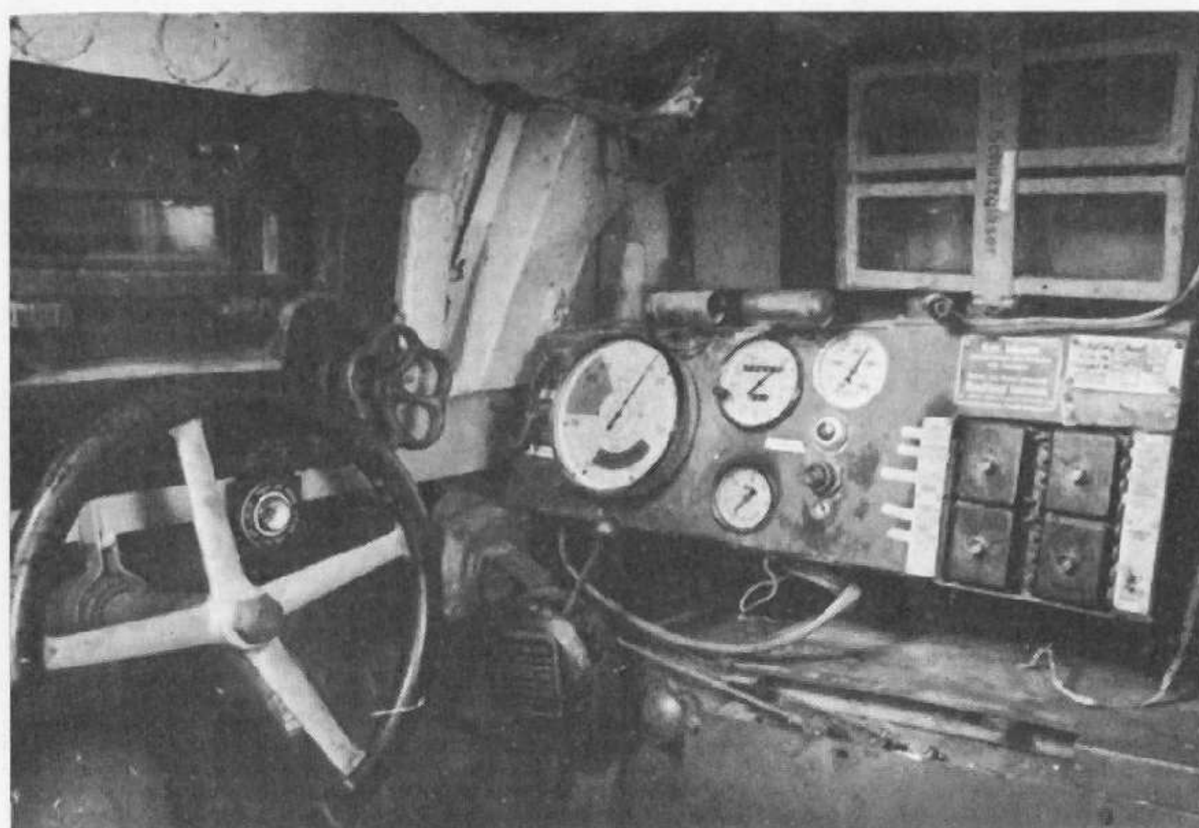
Driver's compartment of Tiger Ausf. H (Ausf. E) showing steering wheel, visor, and instrument panel. (Imperial War Museum)
