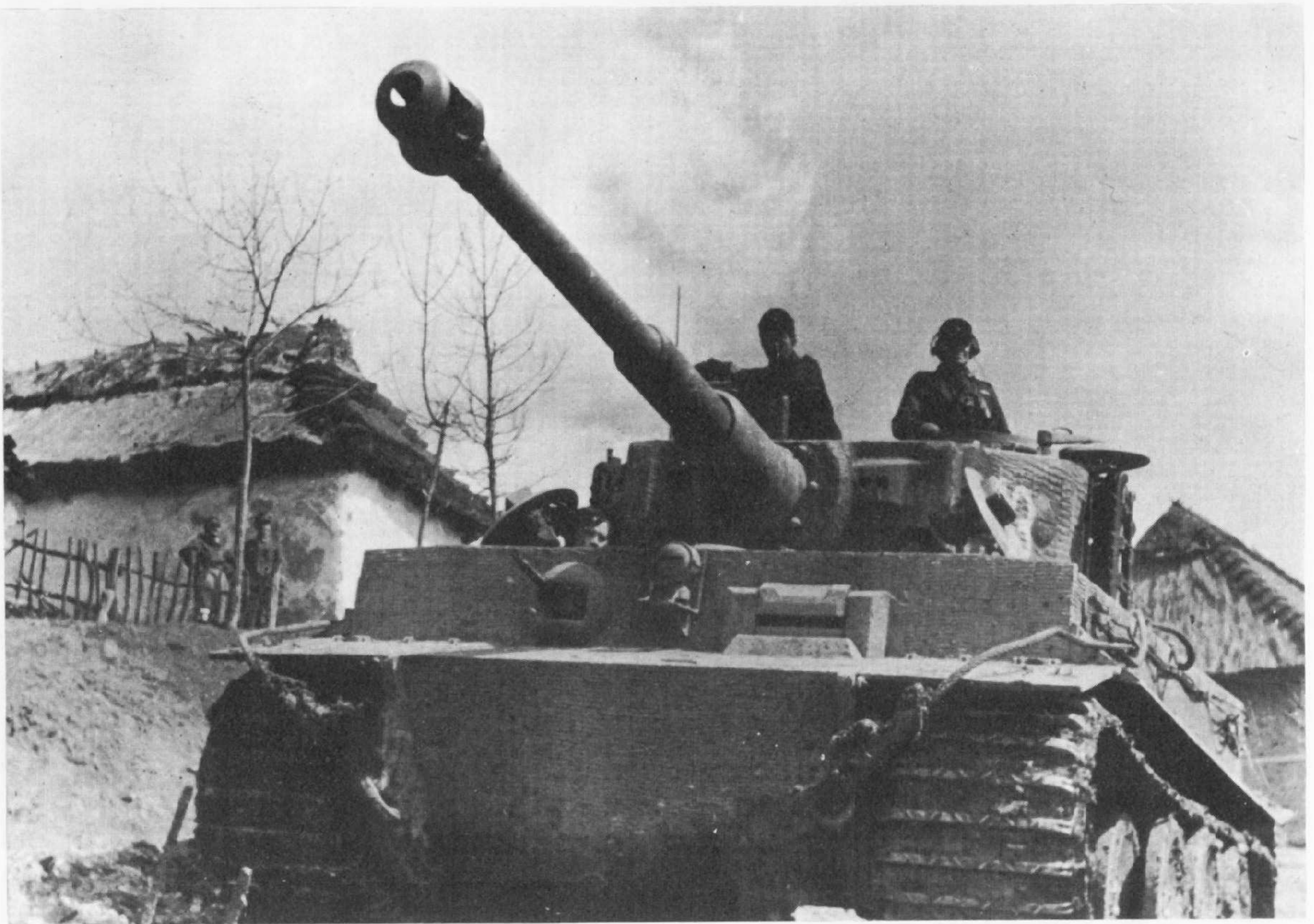
A late production Tiger Ausf. E on the Russian front, summer 1944; note episcopa-fitted cupola and "Zimmerit" anti-magnetic plaster ripple coating. (Chamberlain Collection)
