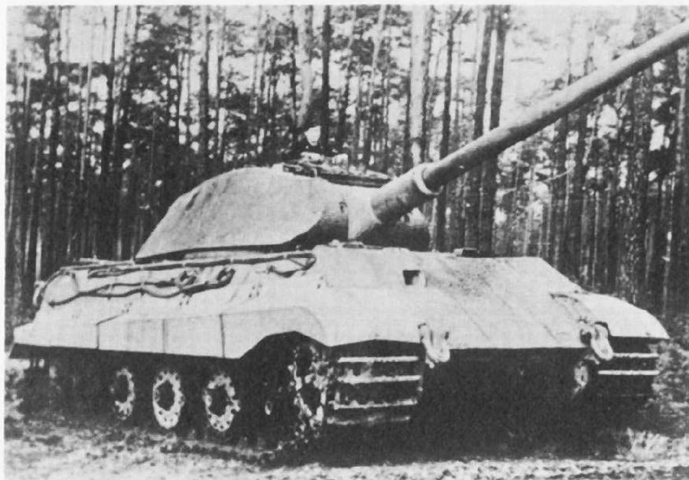
Three-quarter right front view of Koenigtiger with Porsche turret, showing the curved front gun mantlet and monobloc gun barrel.
