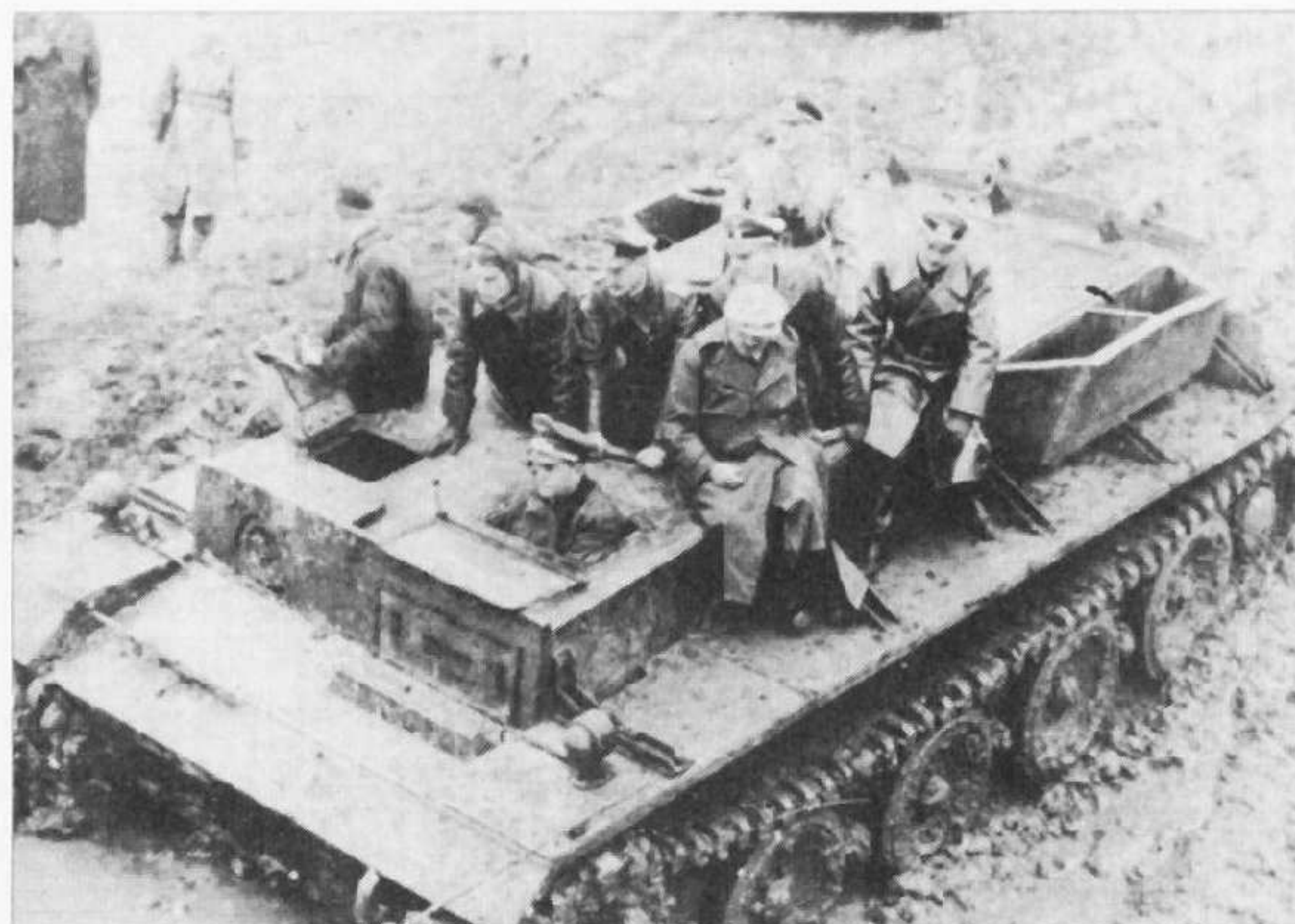
(Below) Henschel's VK.3601(H) prototype for a 36-ton tank specified by Hitler in 1941. It was followed by VK.4501(H), the Tiger prototype demonstrated to Hitler on April 20, 1942. (Chamberlain Collection/Col. R. J. Icks)
