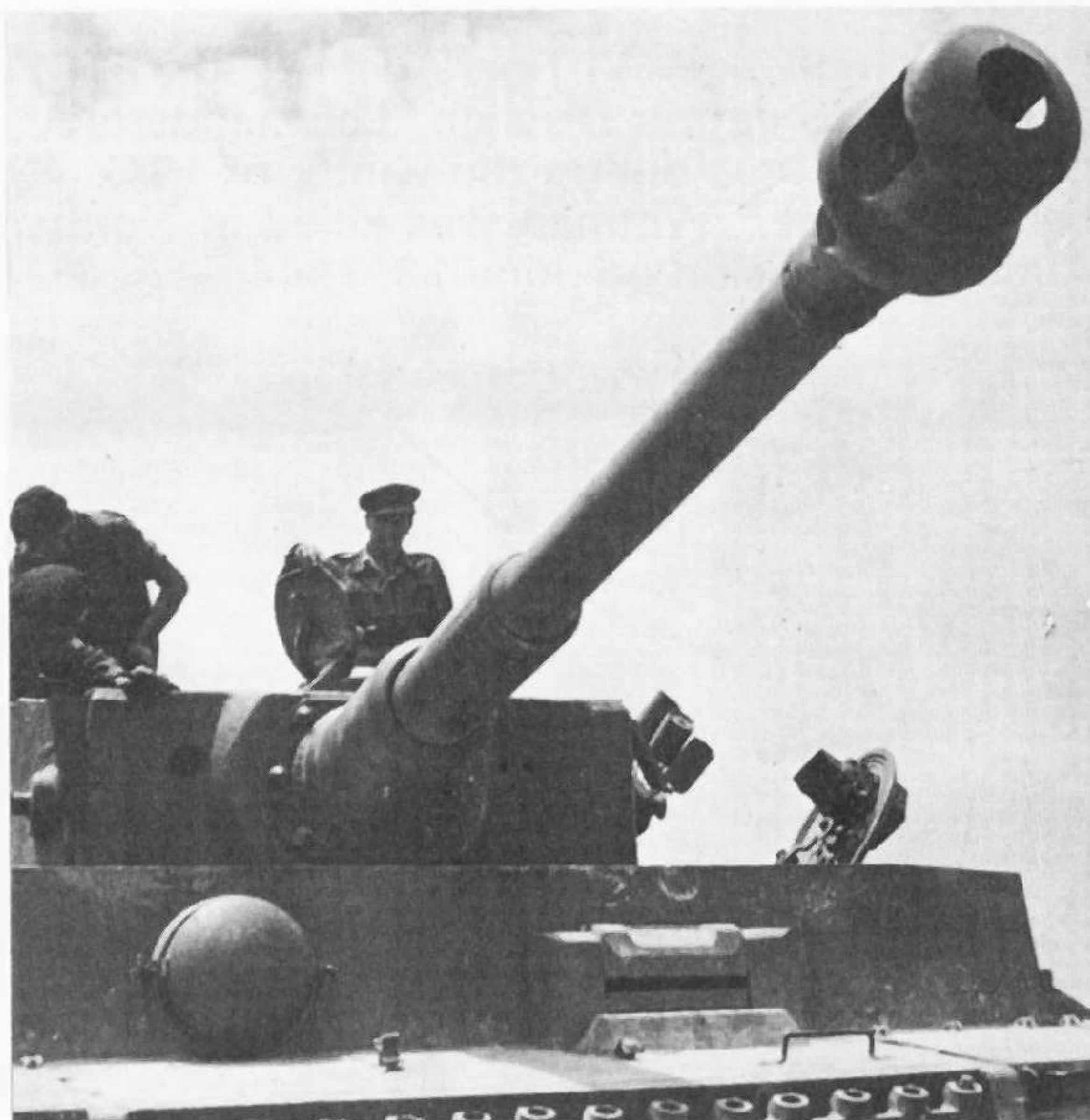
Note the rubber sealing plug over the hull machine-gun ball mount on this Tiger Ausf. E captured in Tunisia—part of the rig for deep wading. (Imperial War Museum)
