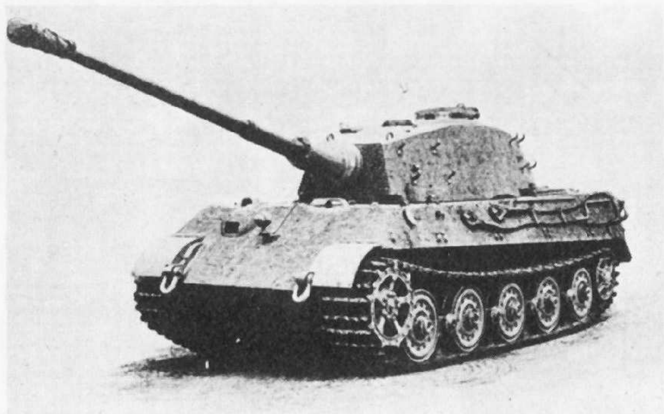
Royal Tiger with Henschel turret and two-piece gun barrel. This vehicle is equipped with transport tracks.
