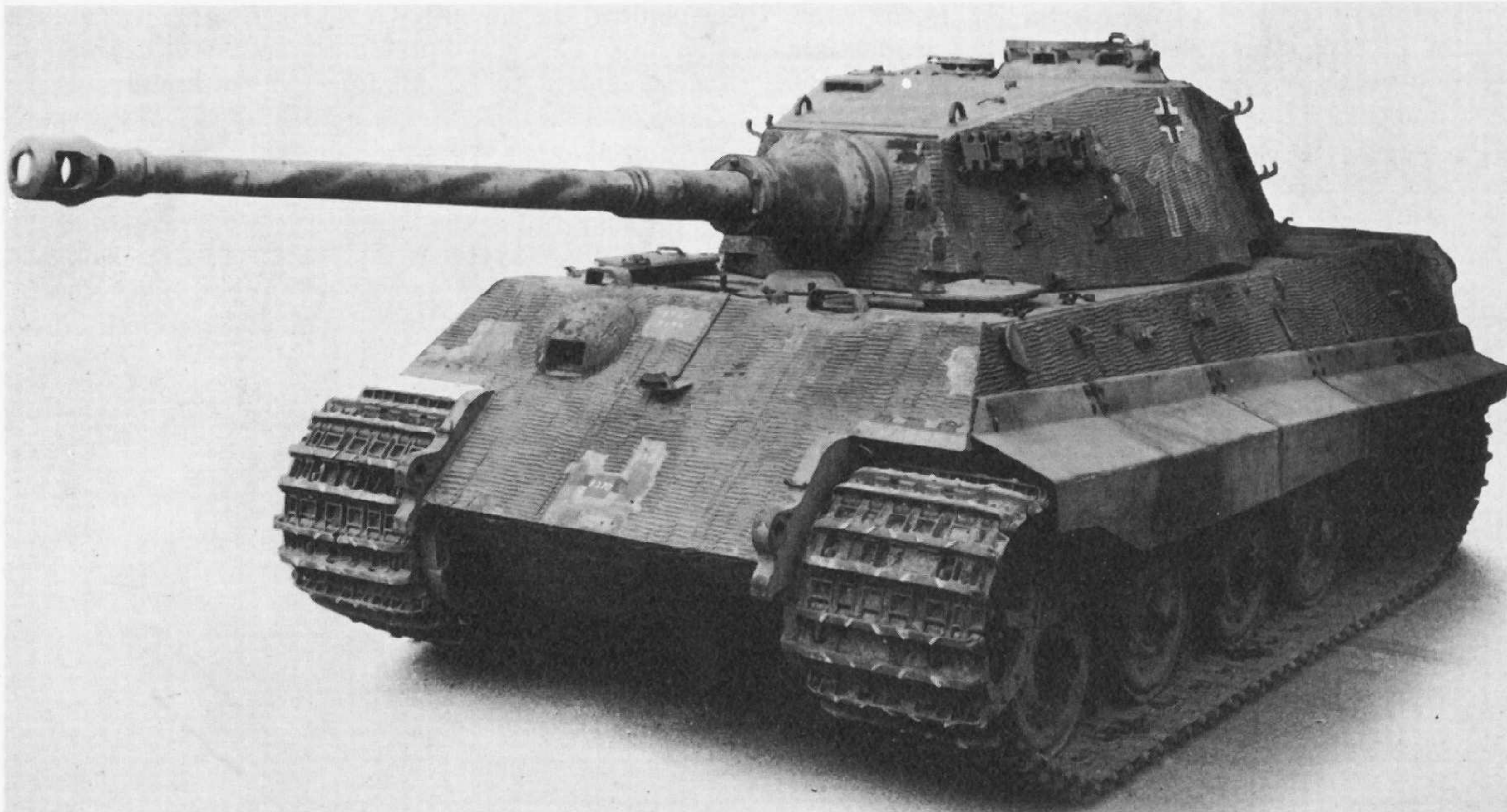
Henschel-turret Tiger Ausf. B with battle tracks and armoured skirting. The tank is covered with Zimmerit to prevent the attachment of magnetic mines.
