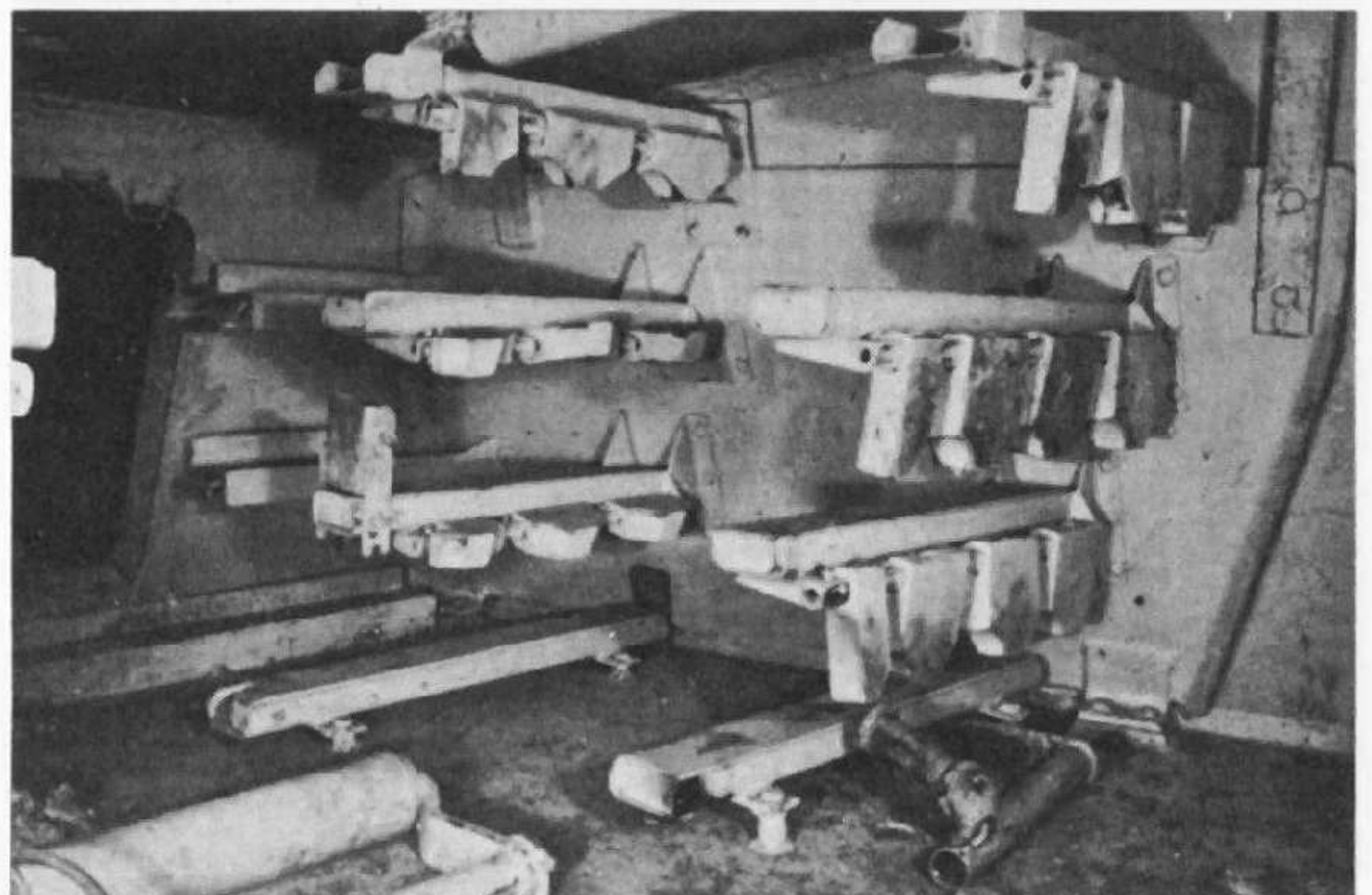
Nearside rear corner of turret showing ammunition racks. The roller on the turret floor (left) was to carry the gun when it was withdrawn from the mounting.
