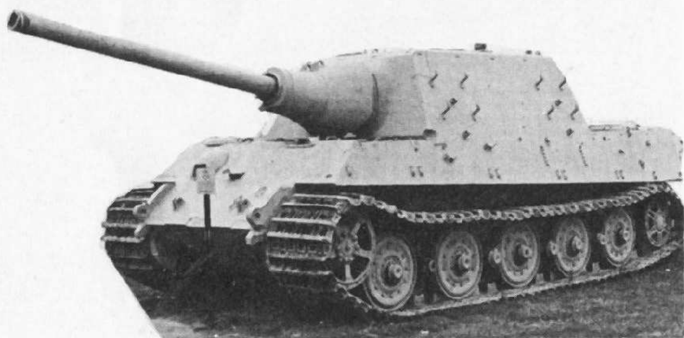
Jagdtiger, showing the hull and suspension of the Royal Tiger. At 70 tons this was the heaviest armoured vehicle to see service in World War II.
