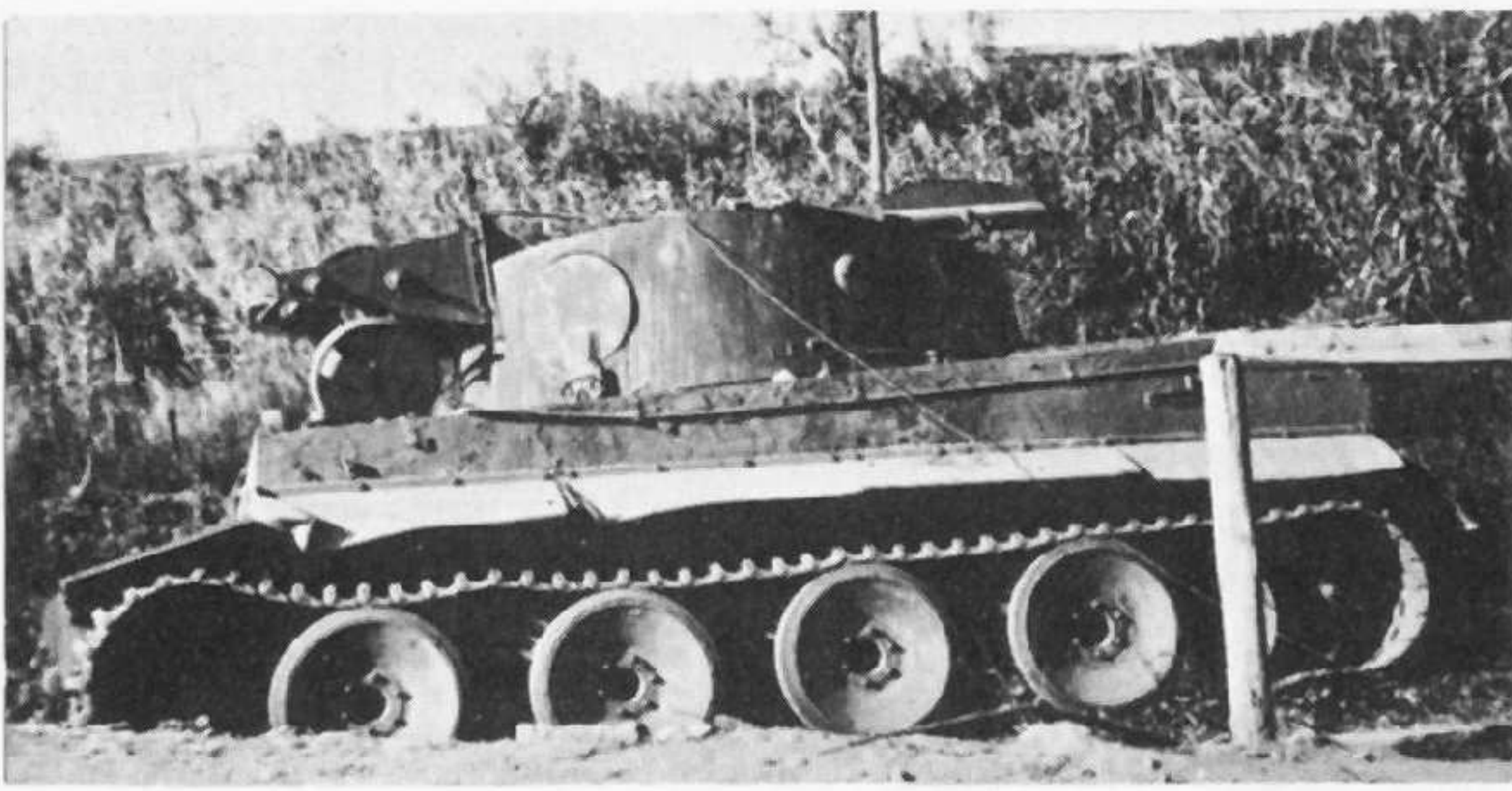
Side view of Tiger recovery vehicle ( Berge PzWg Tiger ), showing hand-operated winch and wire rope guide. The wire rope can be seen lying on the side of the vehicle. (Imperial War Museum)
