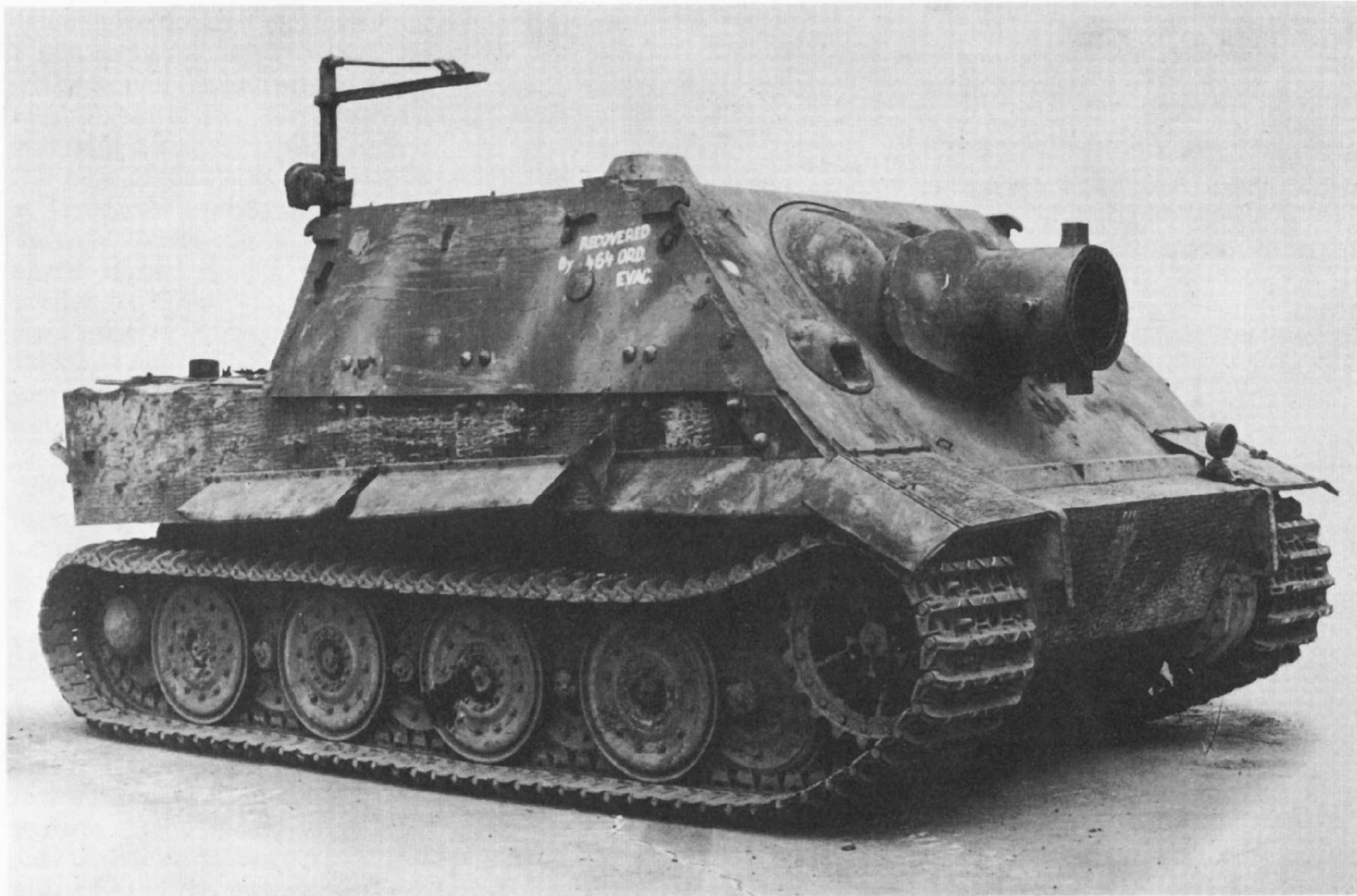
Three-quarter right front view of Sturmpanzer showing the ammunition loading crane. On the off-side front of the roof plate is the electric fan extractor. (Imperial War Museum)
