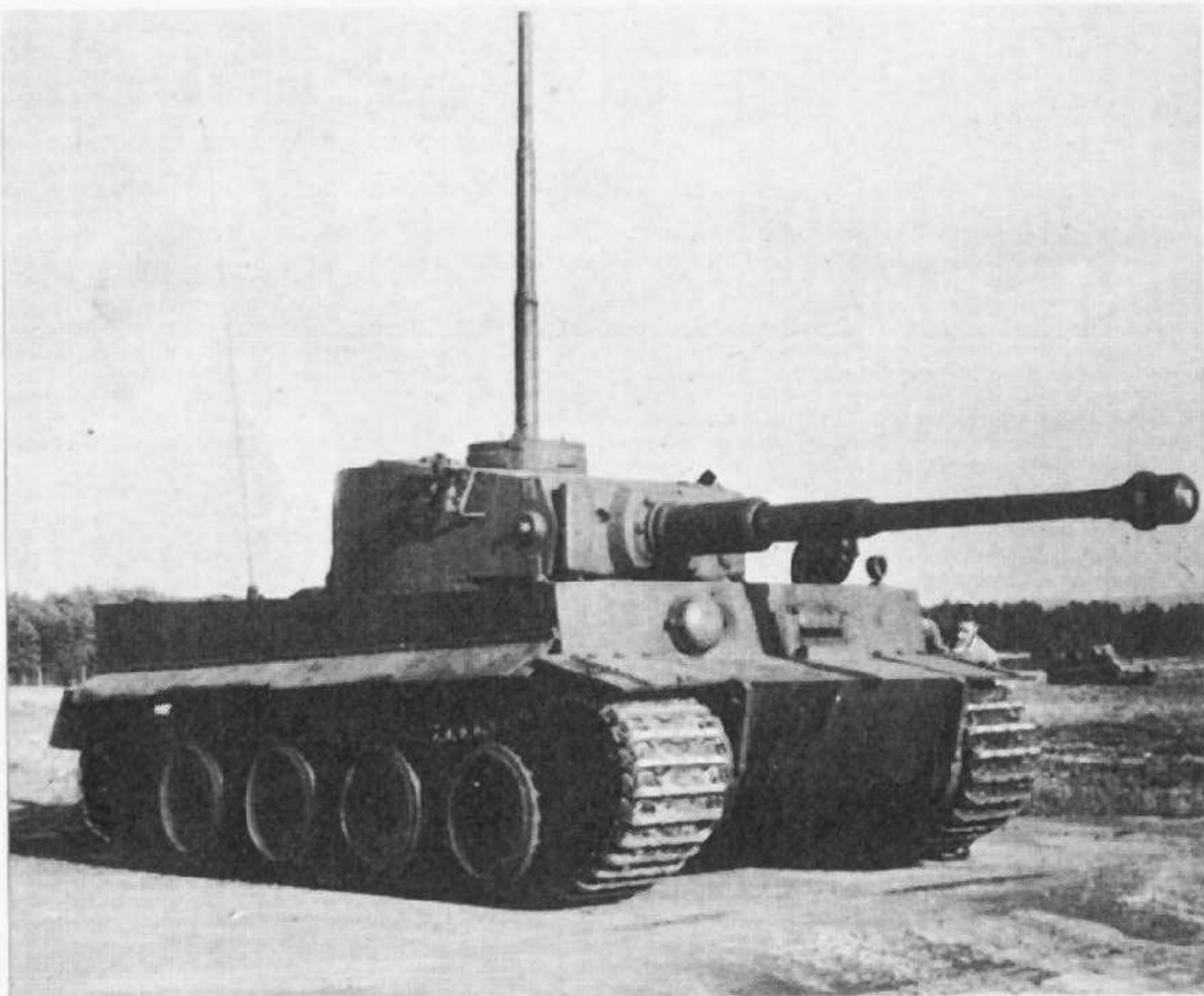
Late production Tiger Ausf. E with Panther type cupola which has fitting for anti-aircraft machine-gun (Fliegerbeschuss-gerät). Tank has steel-tired wheels. Note absence of Feifel on this late model. (Chamberlain Collection)
