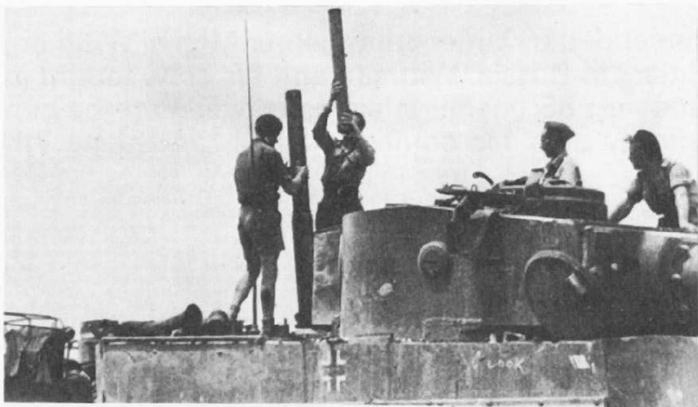
British troops erecting the three-piece Snorkel tube on an early production Tiger Ausf. E captured by the British in Tunisia, 1943. (Imperial War Museum)
