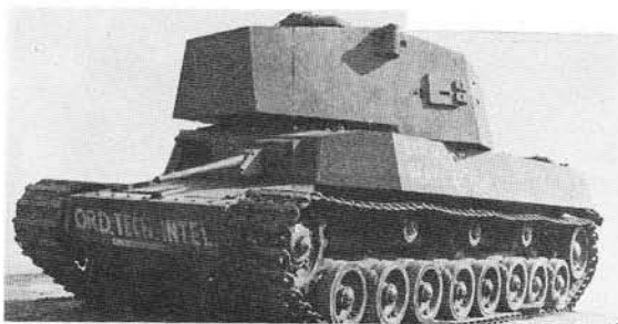
Type 5 Medium Tank (CHIRI). Three-quarter left front view with turret reversed. As well as its Type 4 75 mm. tank gun in the turret the CHIRI had a Type 1 37 mm. tank gun (seen here) mounted forward in a fixed position. It also had two machine-guns. CHIRI did not progress beyond the prototype stage.
