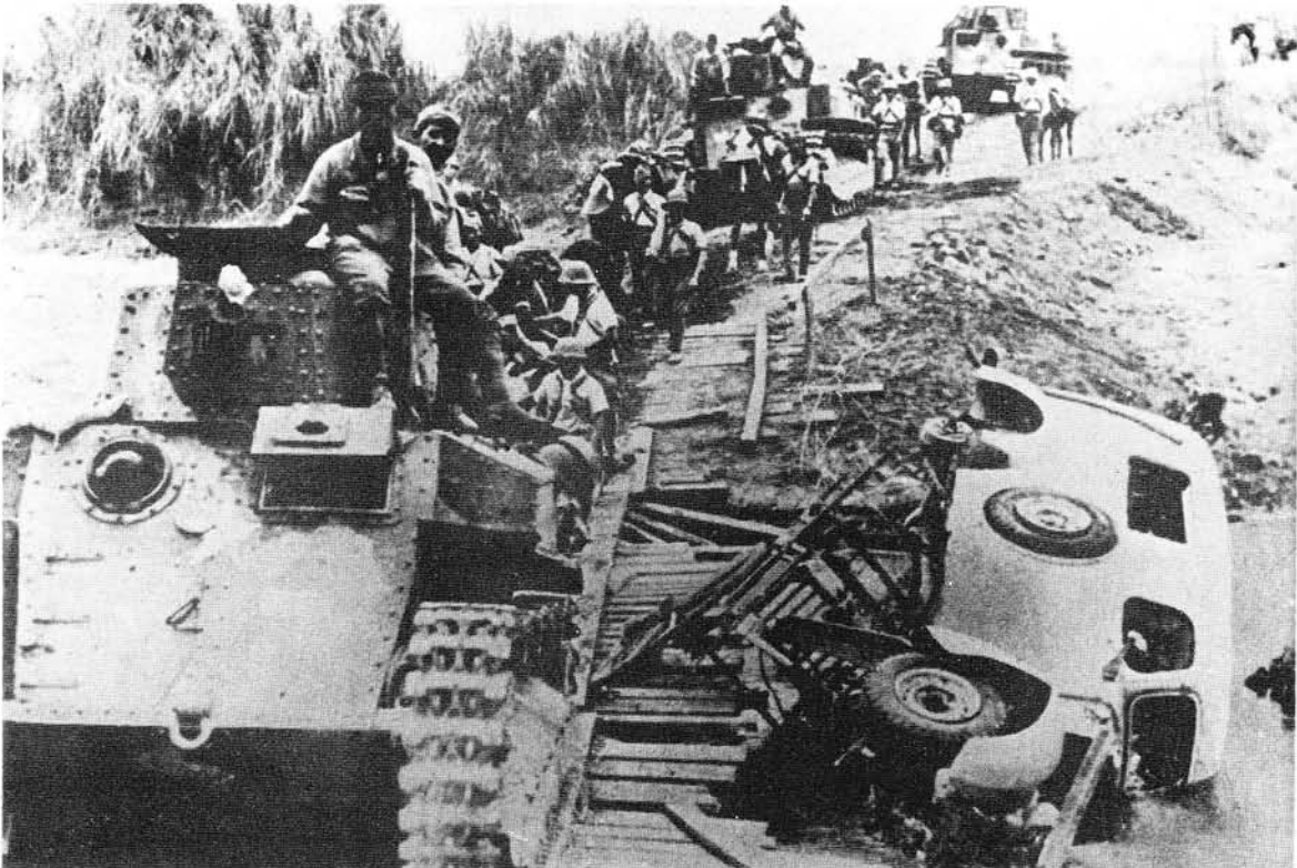
Column of Type 89 Medium Tanks with infantry moving forward after an attack. Of three tanks that are visible all have the modified suspension system with four return rollers and no girder, and all have the single sloping front plate. But whereas the front tank has the driver on the left the rear two have him on the right.
