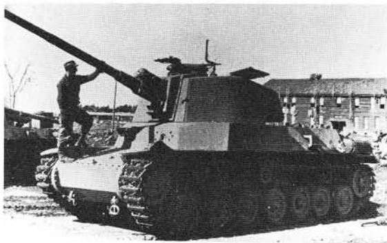
Three-quarter left front view of Type 4 Medium Tank (CHITO) which was the most powerful tank produced for the Imperial Japanese Army during World War II. It was armed with a 75 mm. gun of the anti-aircraft class and two machine-guns.
