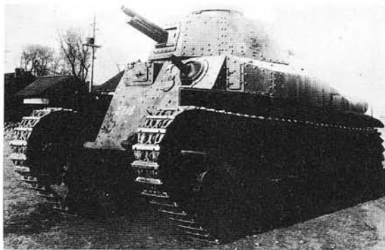
Type 89 "B" Medium Tank with single sloping front plate, driver's position on right and bow machine-gun on left, four return rollers, girder removed, flattish cupola with split lid. The Type 89 "B" had a diesel engine, the Type 89 "A" had a petrol (gasoline) engine.
