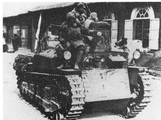
Type 89 "A" Medium Tank with short front plate and vertical front plate above this. There is a door on the right of the lower plate with a bow machine-gun above it. The driver's position was on the left. Note opened "saucepan" cupola behind the shoulder of the left-hand crew member. There are five small return rollers mounted along a girder.
