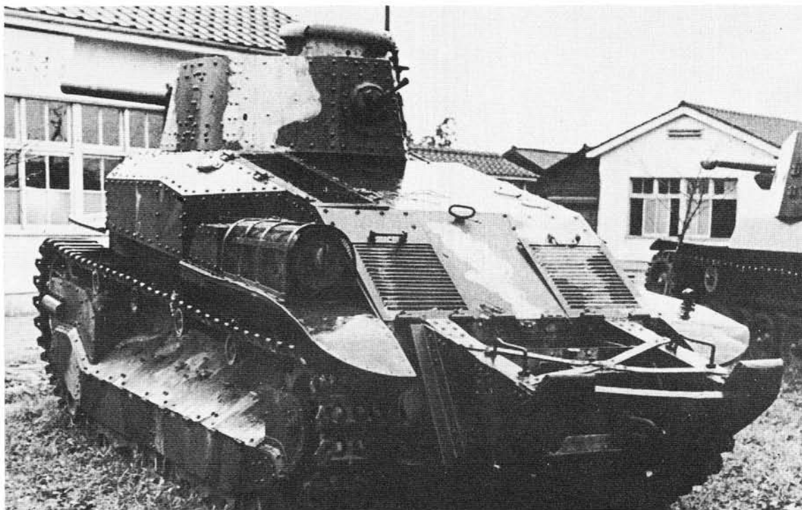
Three-quarter left rear view of Type 89 "B" Medium Tank with ditching tail. Fuel tanks were over the tracks.
