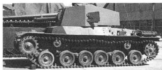
Type 3 Medium Tank (CHINU) at Mitsubishi Heavy Industries Ltd. The tank is armed with a long-barreled 75 mm. gun of the Type 90 field artillery class. Welded structure.
