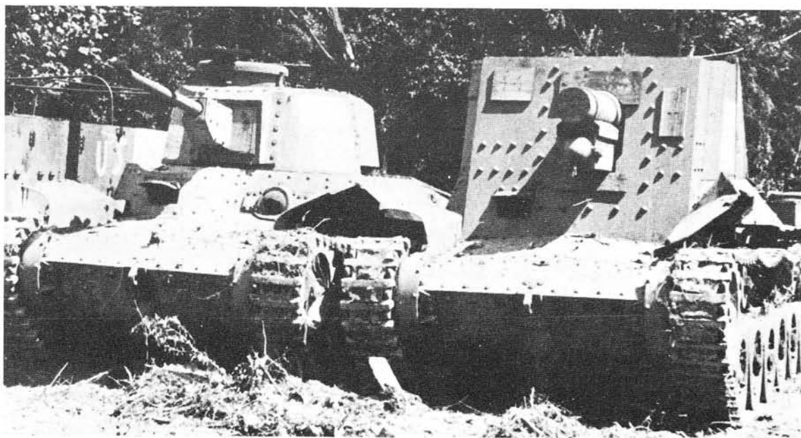
Type 97 Medium Tank—Modified (left) with Type 4 (15 cm.) self-propelled gun (HORO). The HORO with its Type 38 15 cm. howitzer was one of several self-propelled weapons based on the CHIHA chassis. These are described in a separate Profile.
