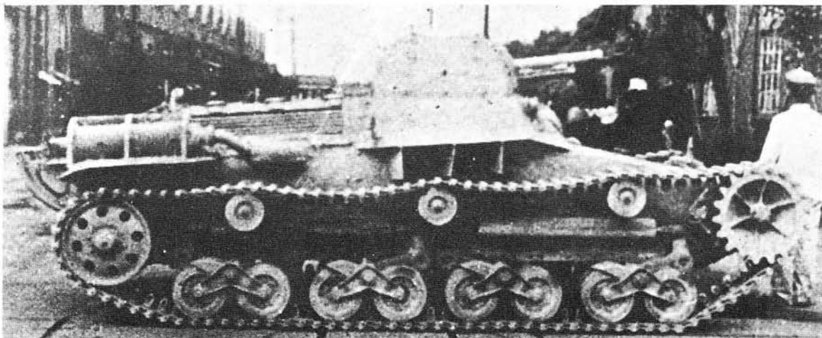
Type 97 Medium Tank, Second Plan (CHINI), which was not adopted. In the author's opinion it should not have been totally rejected but should have been adopted as a light tank.
