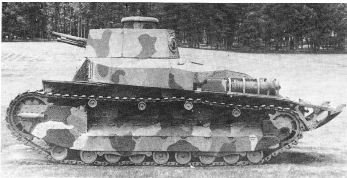
Type 89 "B" Medium Tank with ditching tail added. Note flattish cupola, four return rollers and absence of girder. This model has been referred to sometimes as Type 94 Medium Tank.
