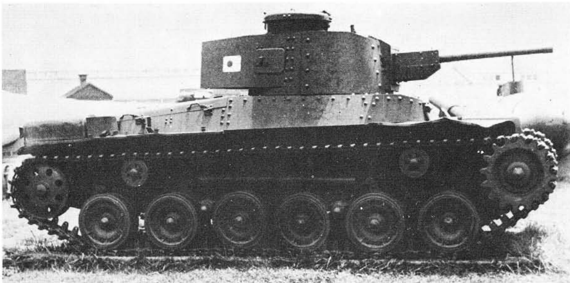
Type 97 Medium Tank—Modified (new turret CHIHA). The CHIHA'S turret was changed to allow the mounting of the long-barreled Type 1 47 mm. gun instead of the 57 mm. gun. CHIHA also had two machine-guns.
