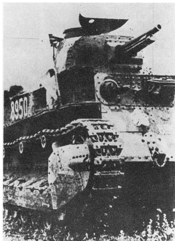
Type 89 Medium Tank with short front plate and vertical front plate above it, but with flattish type cupola and no girder under the return rollers. The gun mount has also been modified with external mantlet.
