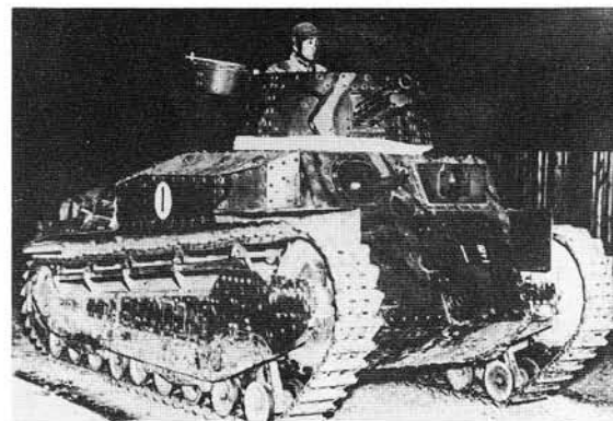
Type 89 Medium Tank with single sloping front plate and "saucepan" cupola. This model has been referred to sometimes as Type 92 Medium Tank.
