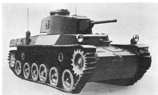
Type 1 Medium Tank (CHIHE). This was the Type 97 Medium Tank with a Type 1 47 mm. gun and other modifications including a Type 100 standardized diesel engine. Note the welded structure which was another feature of this tank. CHIHE had two machine-guns.
