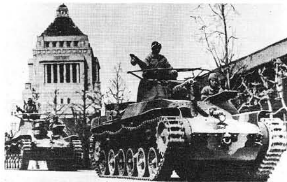
Type 97 Medium Tanks with radio antennae round turret tops. The cupola hatch was of a most unusual design. It had two flaps, one shaped like a crab's claw which fitted round the other when the hatch was closed.
