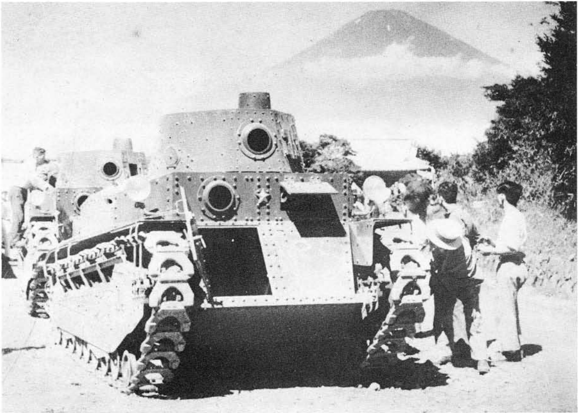
Original model of Type 89 Medium Tank during road tests near Mount Fuji, which is seen in the background. Note the caterpillar shoe.
