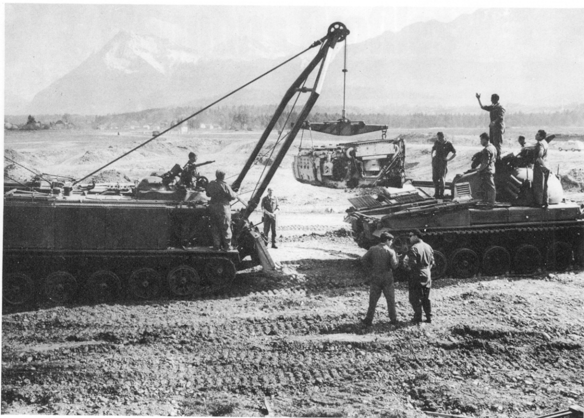
Entp. Pz.65 lowering an engine-transmission assembly into a Pz.61 battle tank.
