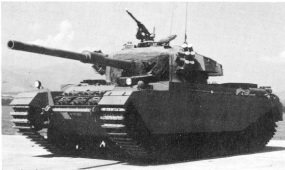
British-built Centurion tank with 105mm gun.
