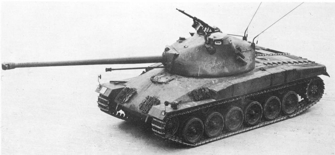
Another view of Pz.58 which shows its 20mm coaxial gun.
