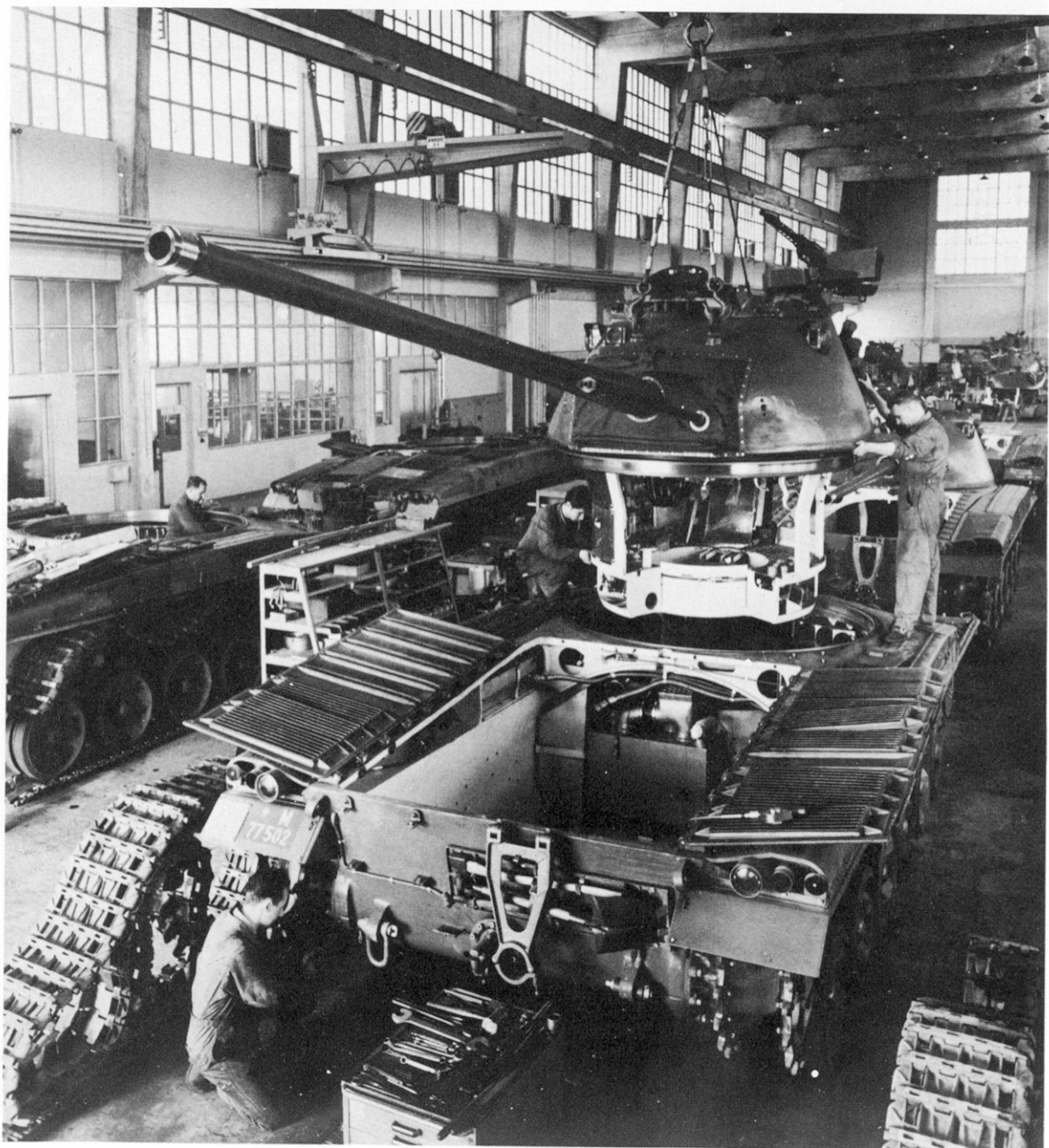
Turret being lowered onto the hull of a Pz.58 whose engine compartment awaits the installation of the engine-transmission assembly.
