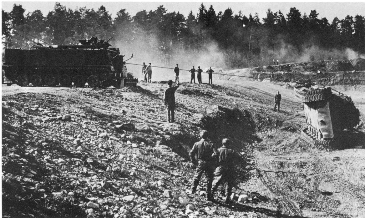
Entp. Pz.65 with its bulldozer blade used as a ground anchor pulling an overturned battle tank.
