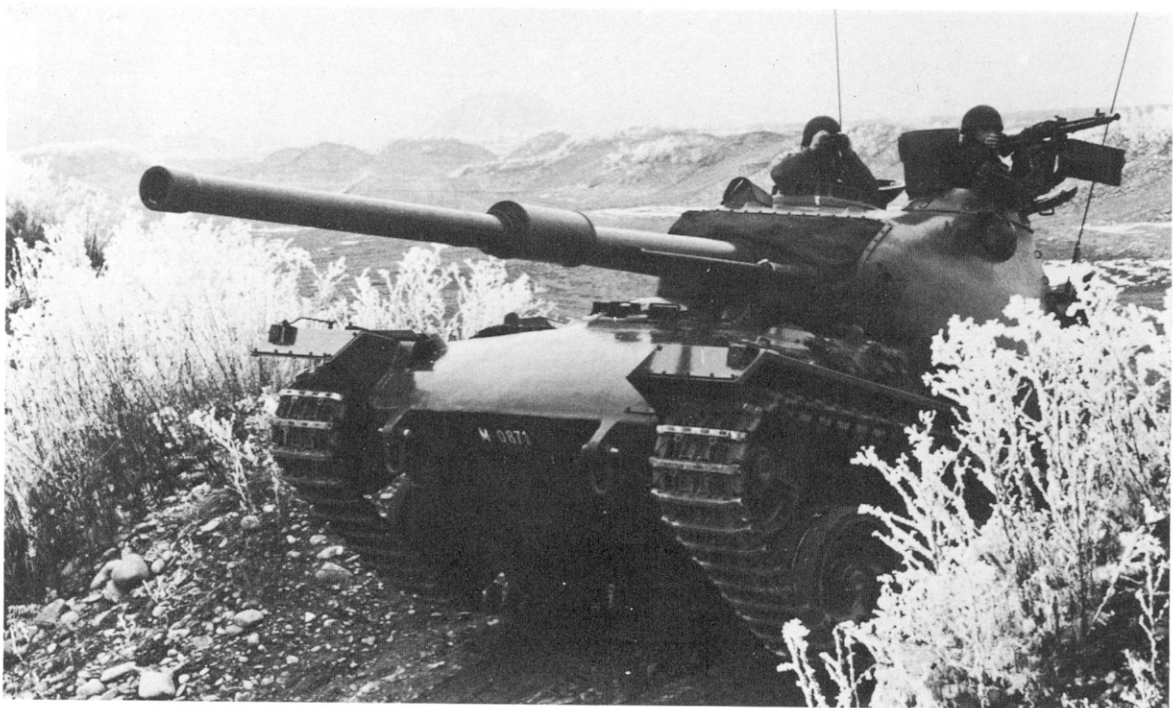
Pz.61 with its turret-mounted 7.5mm machine-gun manned by the loader.
