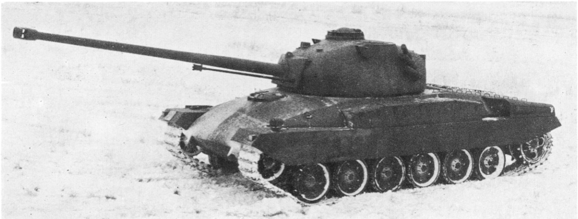
First prototype of Pz.58, the forerunner of the Pz.61, armed with a 90mm gun.
