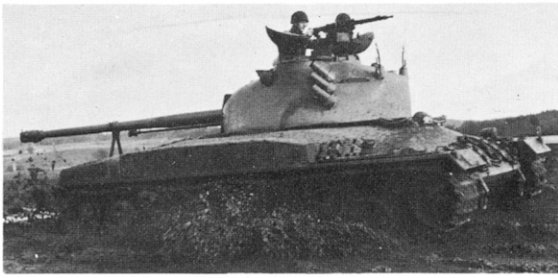
Pz.58 with its turret traversed to the rear successfully negotiating muddy terrain.
