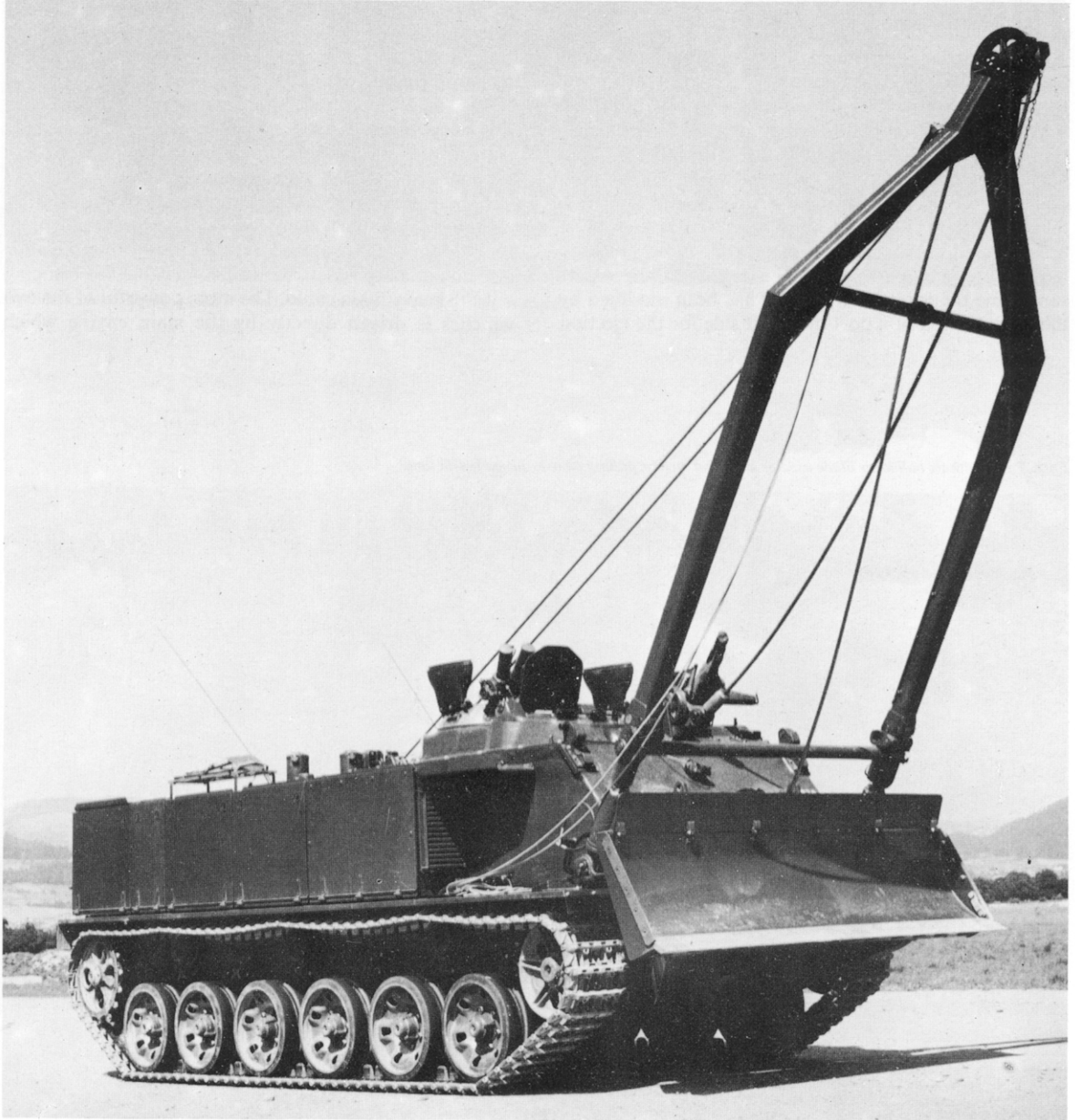
Entp. Pz.65, the armoured recovery vehicle based on the Pz.61, with its jib raised into the working position.
