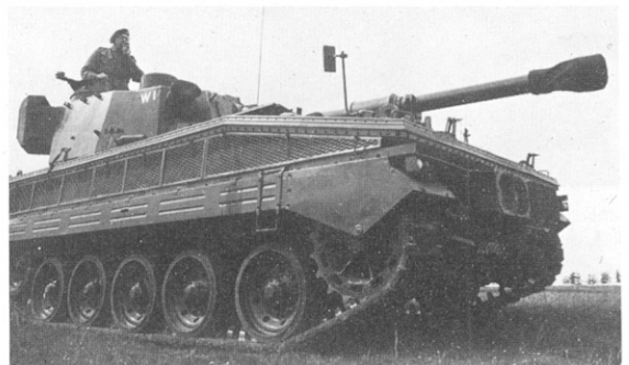
Abbot prototype after being fitted with production type flotation screen. (CCR BIS)
