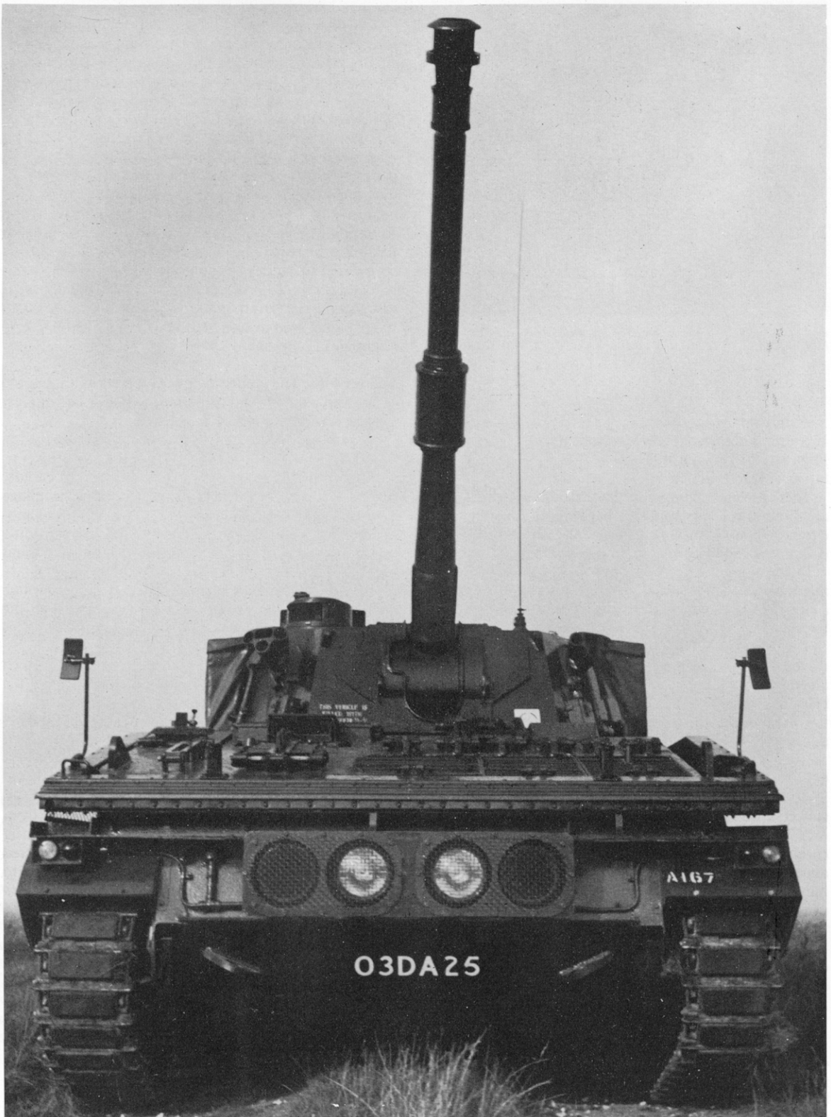
Abbot prototype, note that the outer headlamps are infra-red.
