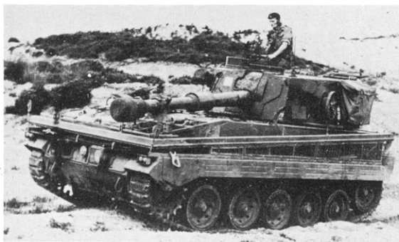
The fifth Abbot prototype, note the original position of the exhaust pipe on left hull top (centre). (RAC Tank Museum)
