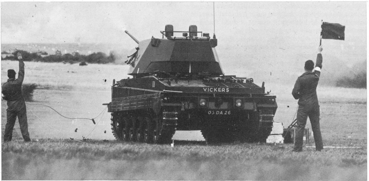
Falcon firing its two 30mm Hispano Suiza HSS 831L guns with turret traversed to rear.
