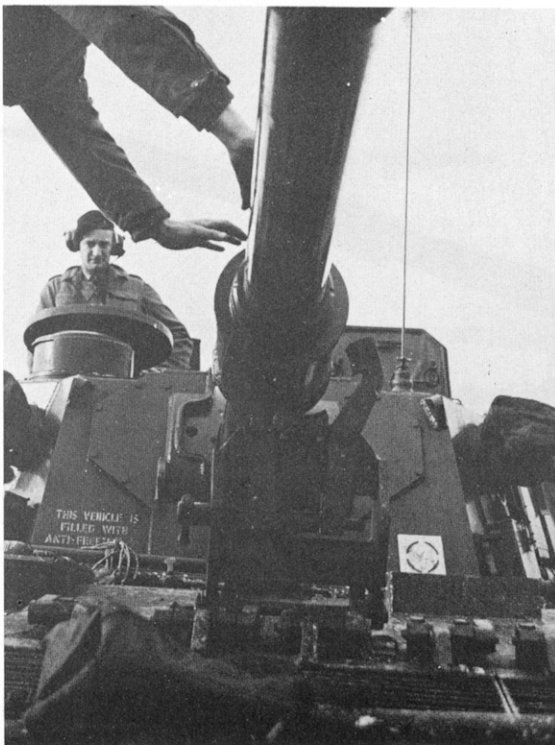
Close up showing Abbot gun lock.
