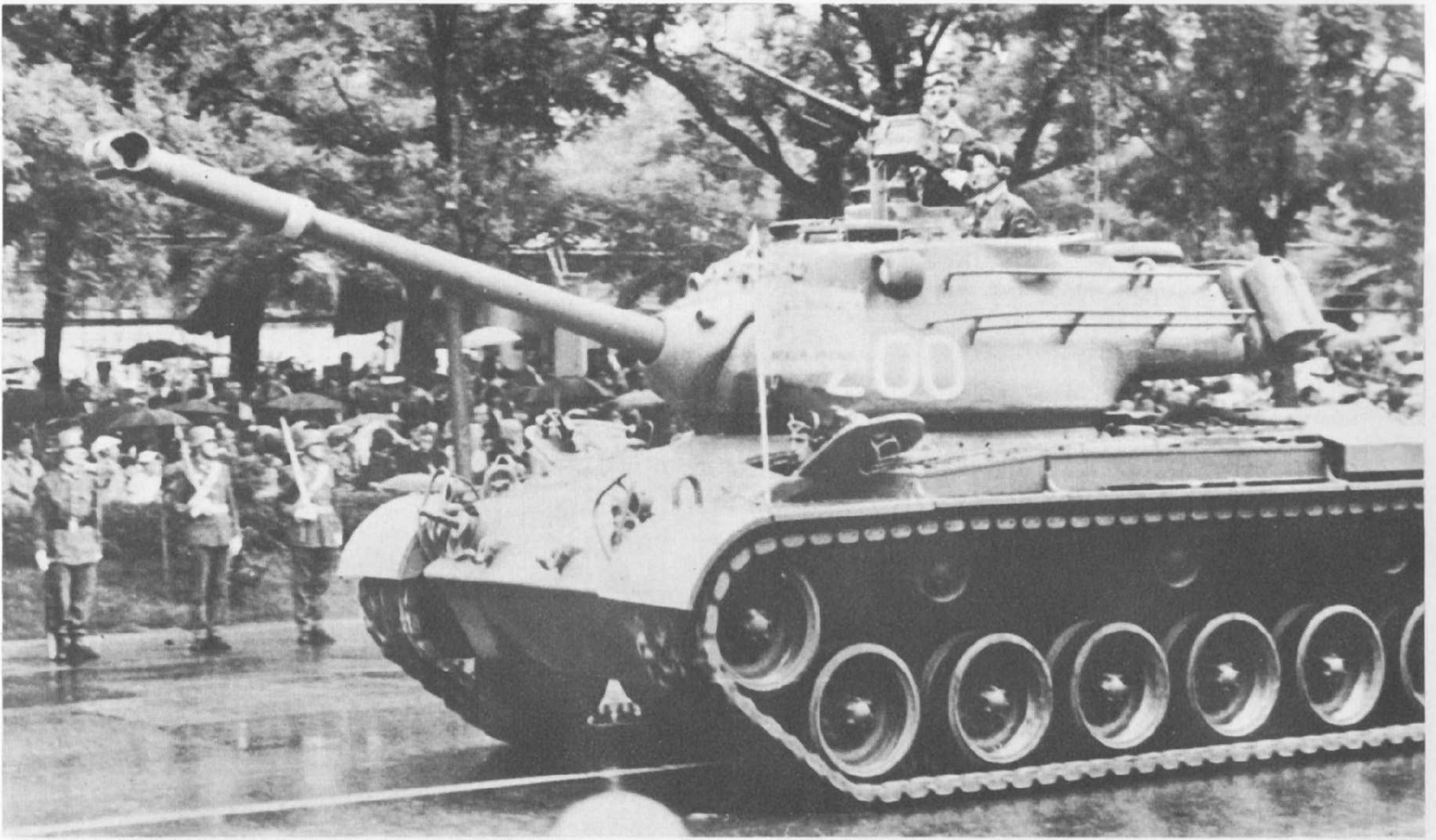
An M47 Medium Tank with T-head blast deflector, in a military parade in Madrid in May 1967.
