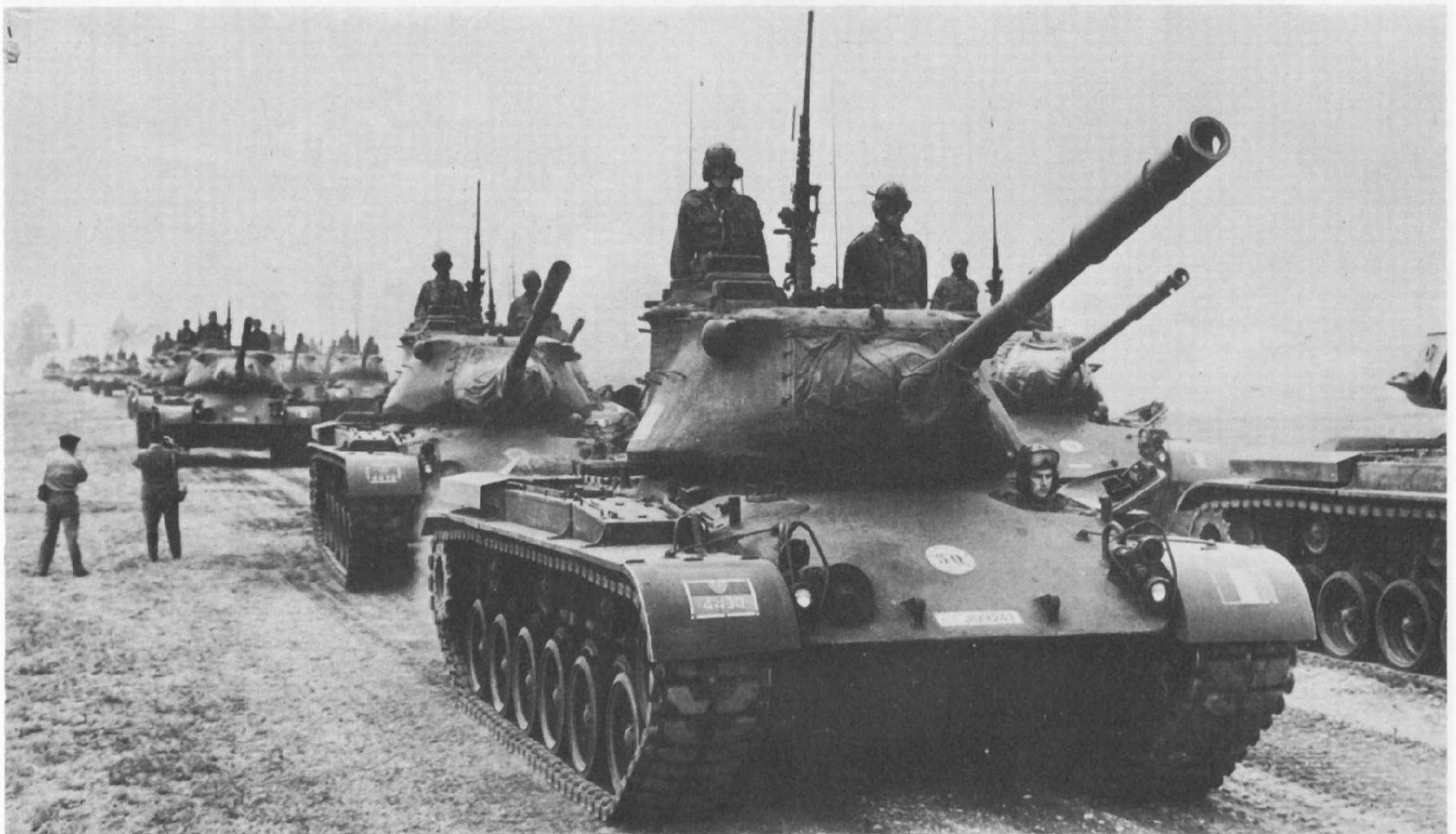
M.47 Medium Tanks in an Italian Army military parade, all but the co-driver's hatch open, showing tool boxes over fenders.
