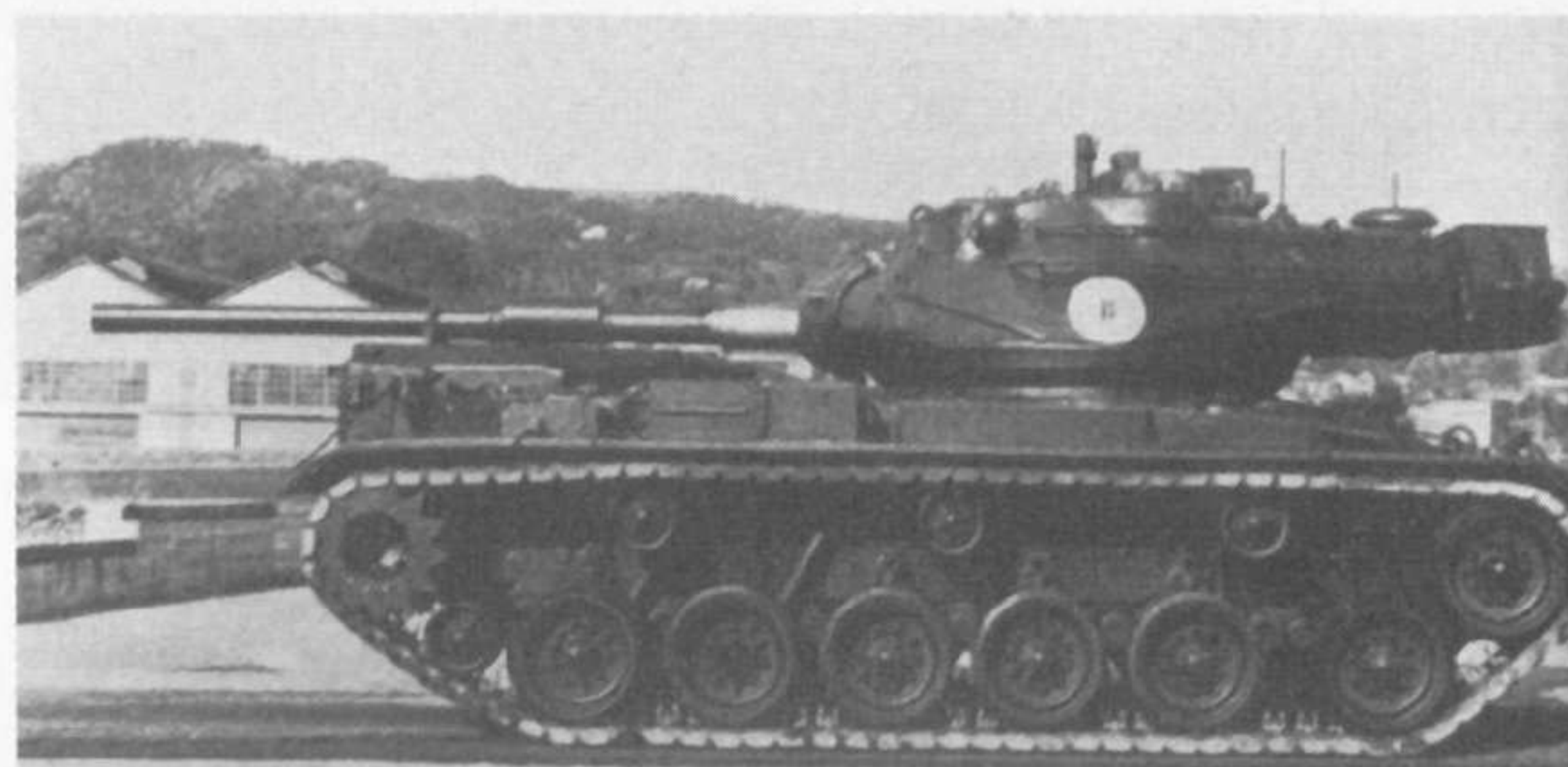
Side view of M.47 with diesel engine and 105 mm. gun made by OTO-Melara.
