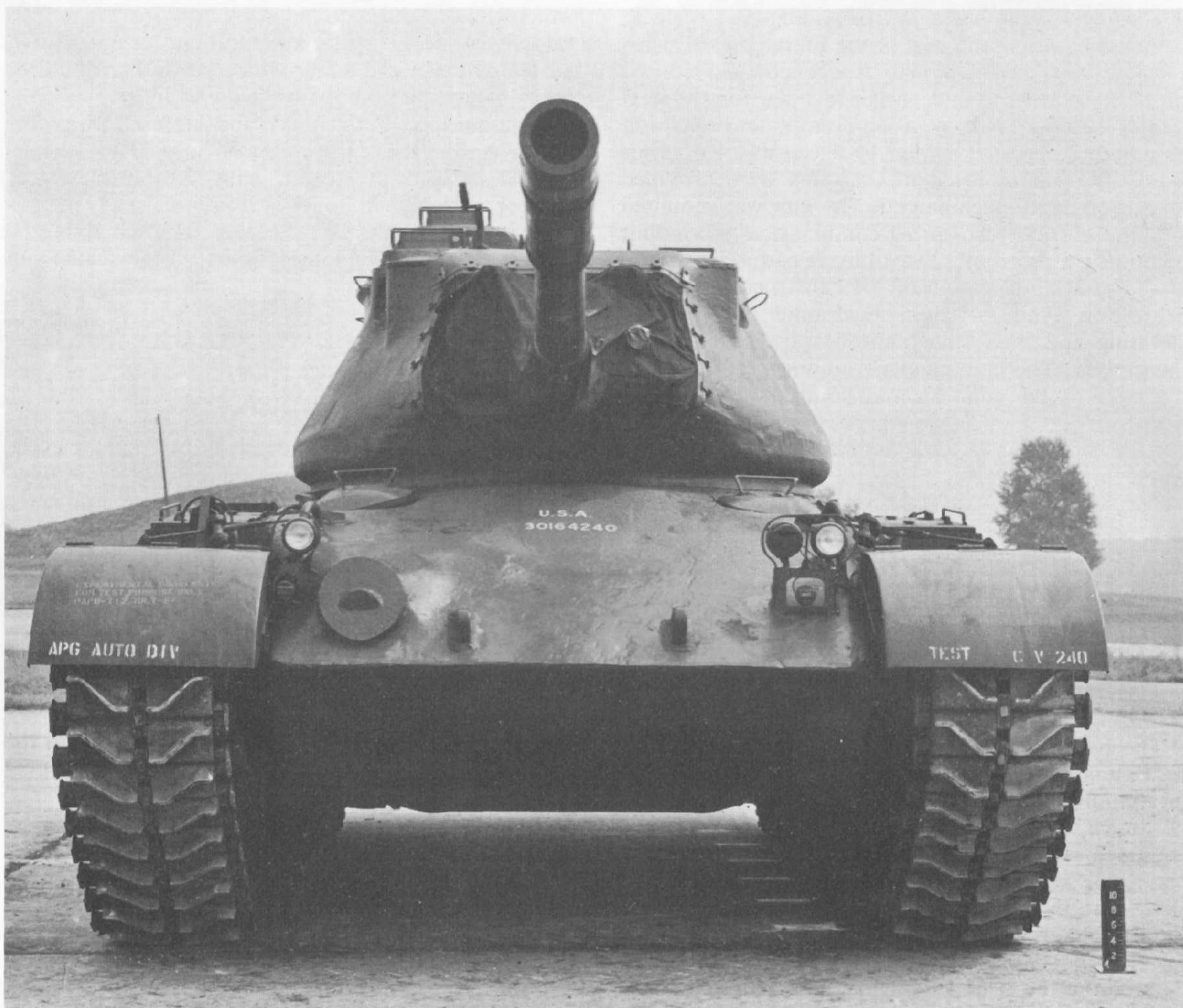
Front view of early M.47 Medium Tank without rangefinder or bow machine-gun, with driver and co-driver hatches closed and equipped with steel grouser tracks. (U.S. Ordnance Dept.)
