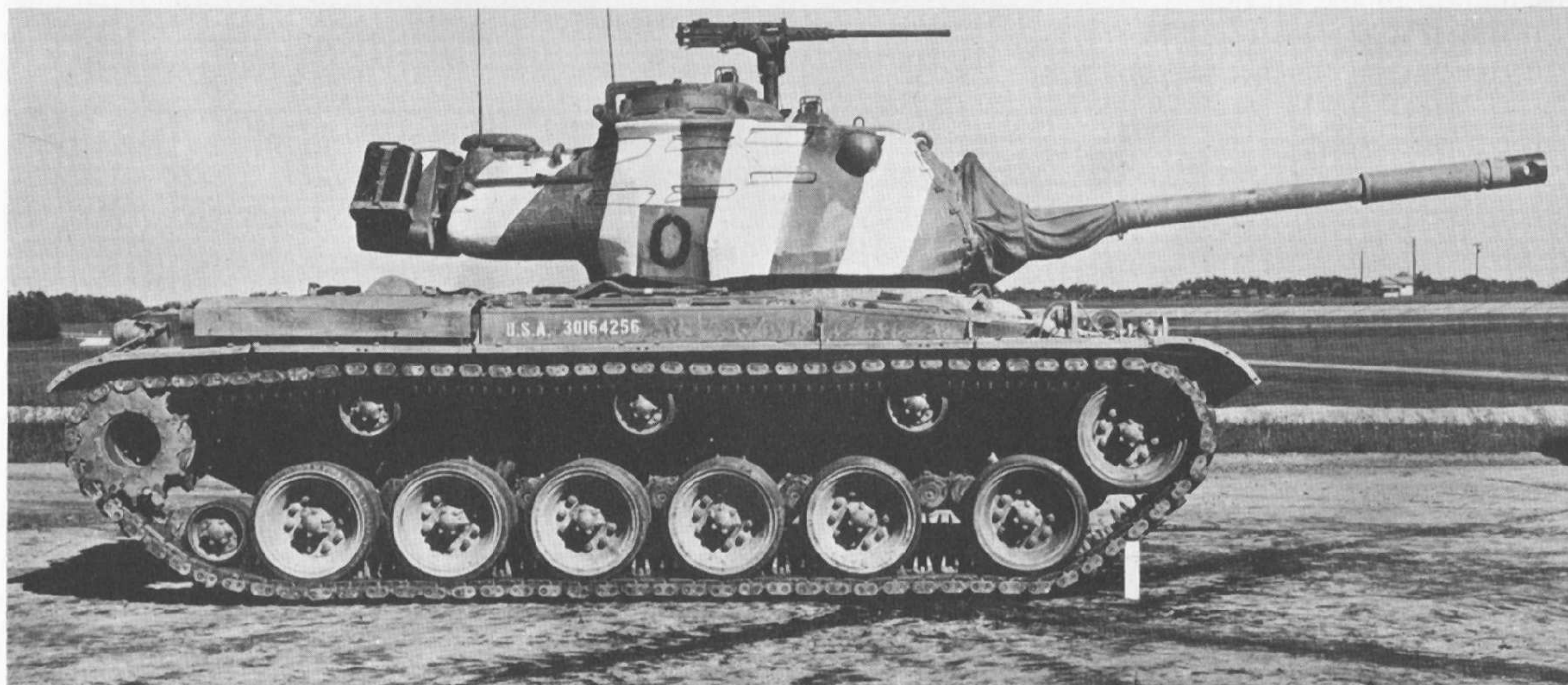
M.47 Medium Tank showing suspension details, characteristic turret bustle and original type of welded-on turret stowage brackets.
