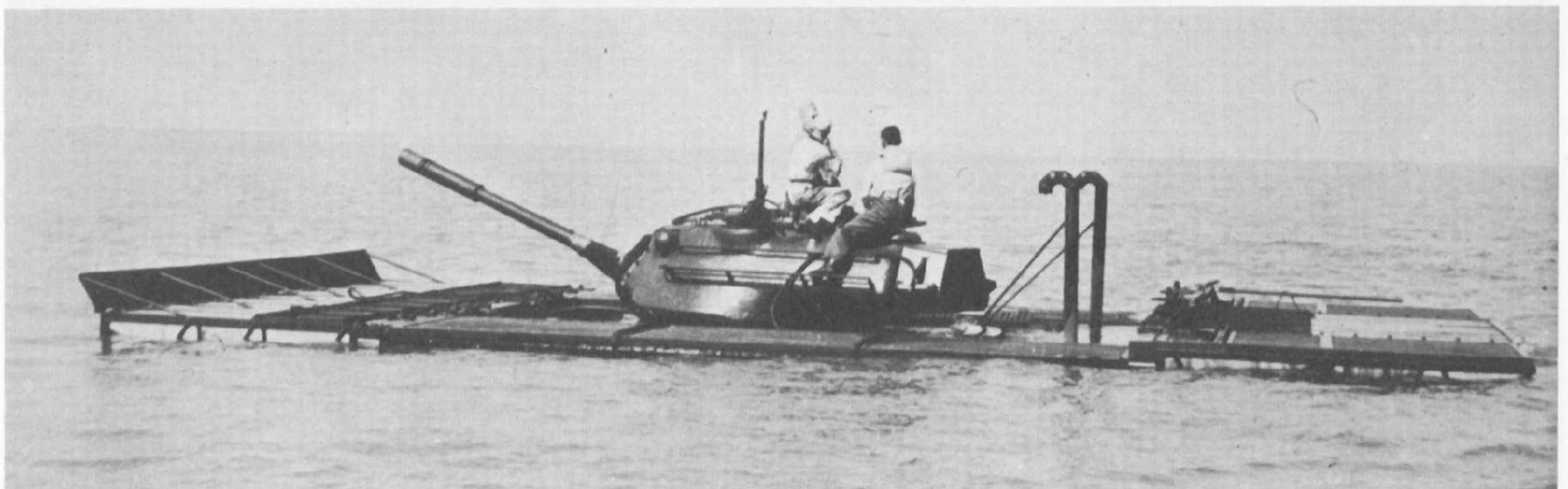
M.47 tank fitted with T.15 flotation device operating in a calm sea, showing the two engine ventilation snorkels for rougher seas.
