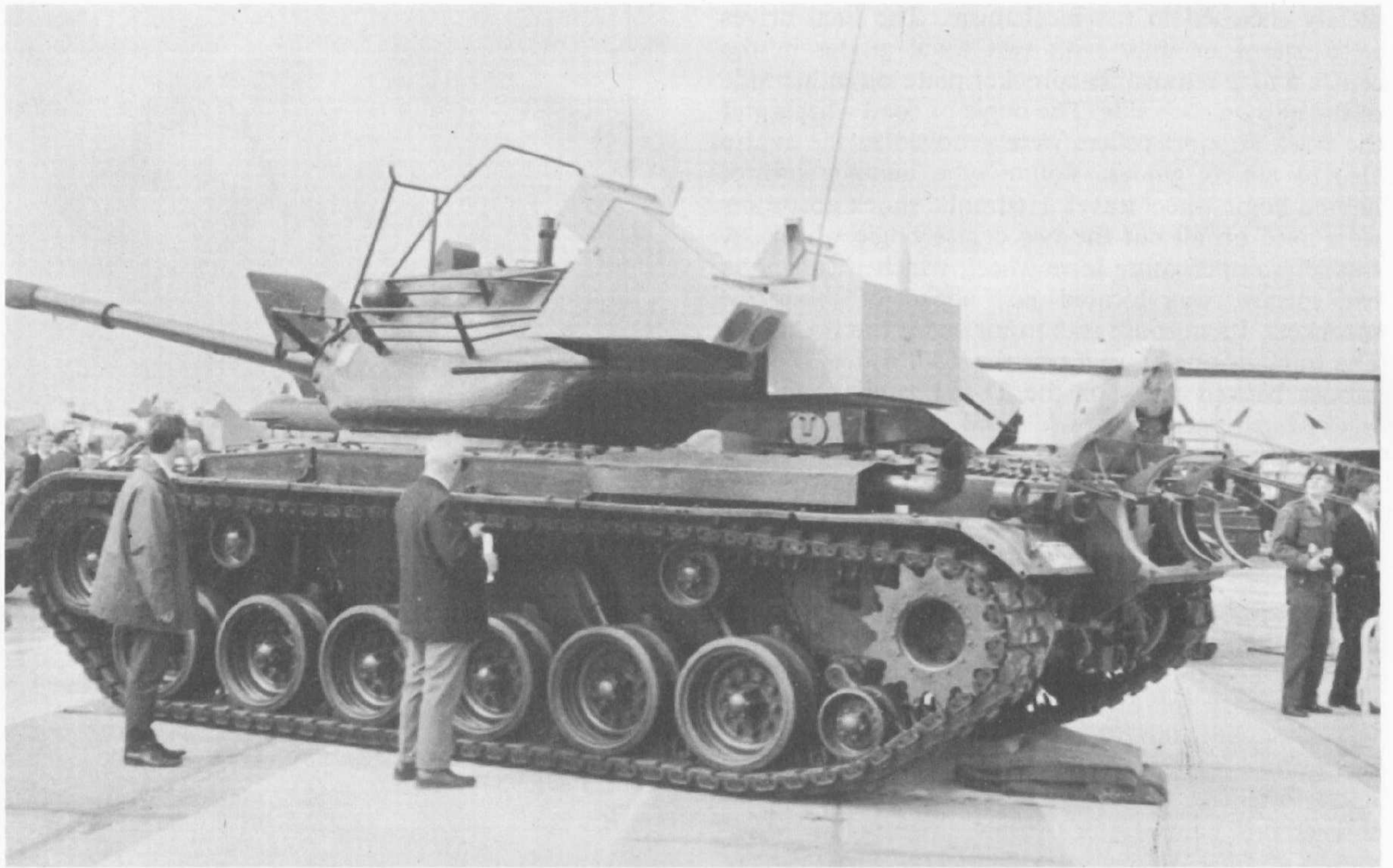
An M.47 tank equipped with British Aircraft Corporation Swingfire missile projectors being shown at Farnborough Air Show in 1967. (B. H. Vanderveen)
