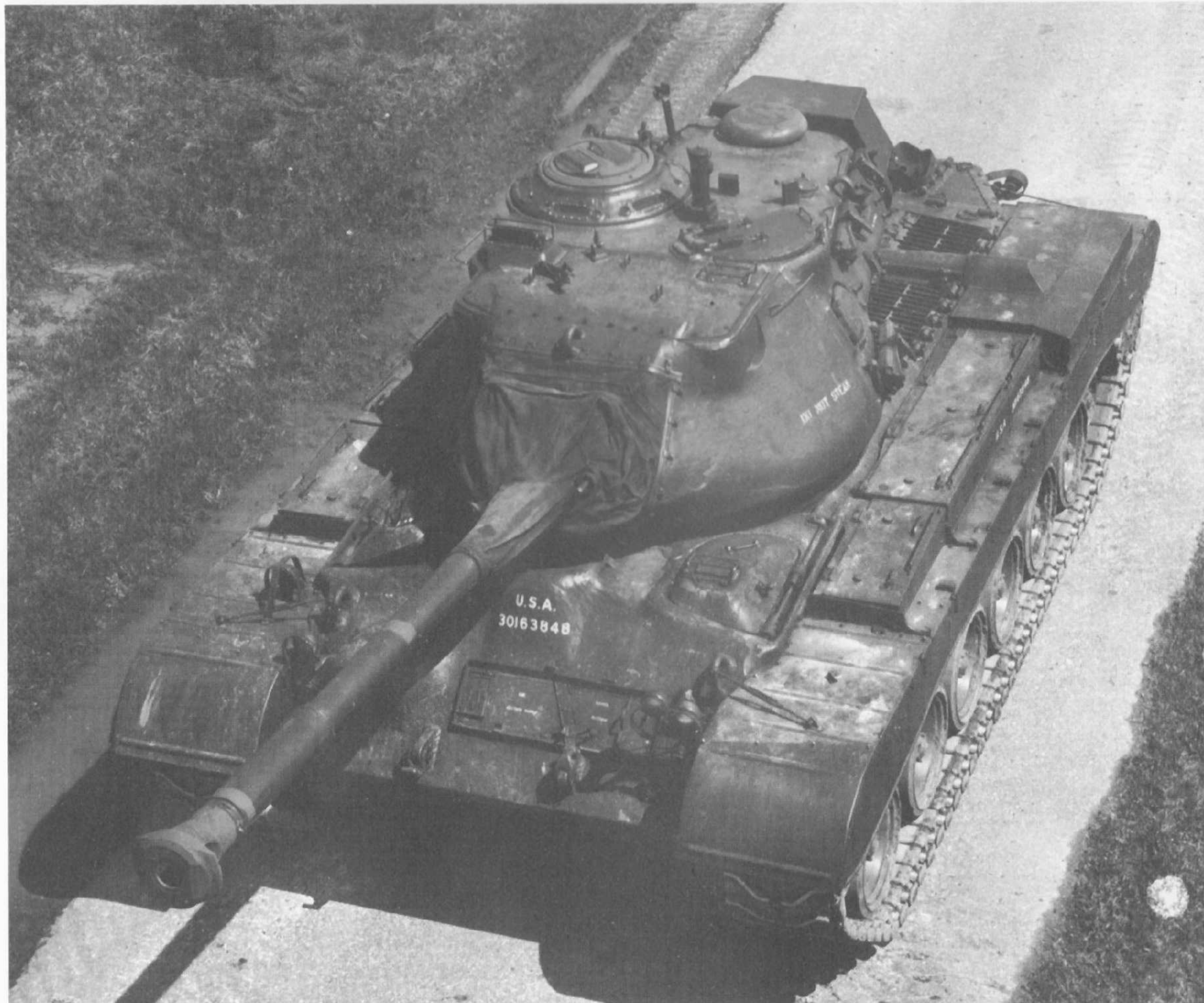
M.46 E1 (M.46 A1) Medium Tank with T.42 tank turret, M.46 Medium Tank gun, new ignition harness, fire extinguishers and brake control.
