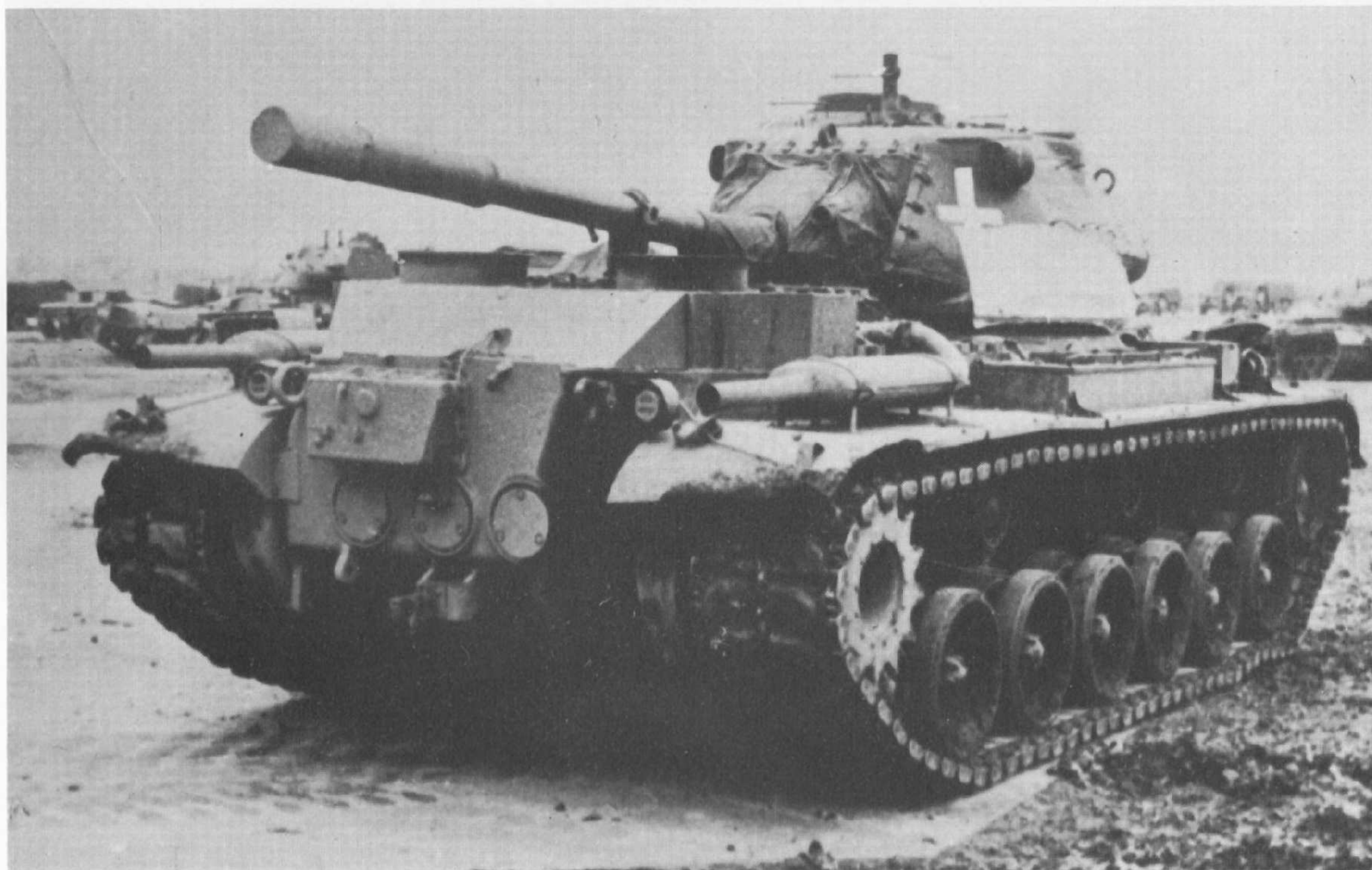
West German M.47 tank with engine compartment modifications necessitated by installation of a Daimler-Benz MB 837a 600 h.p. 8-cylinder multi-fuel engine. (Courtesy W. J. Spielberger)
