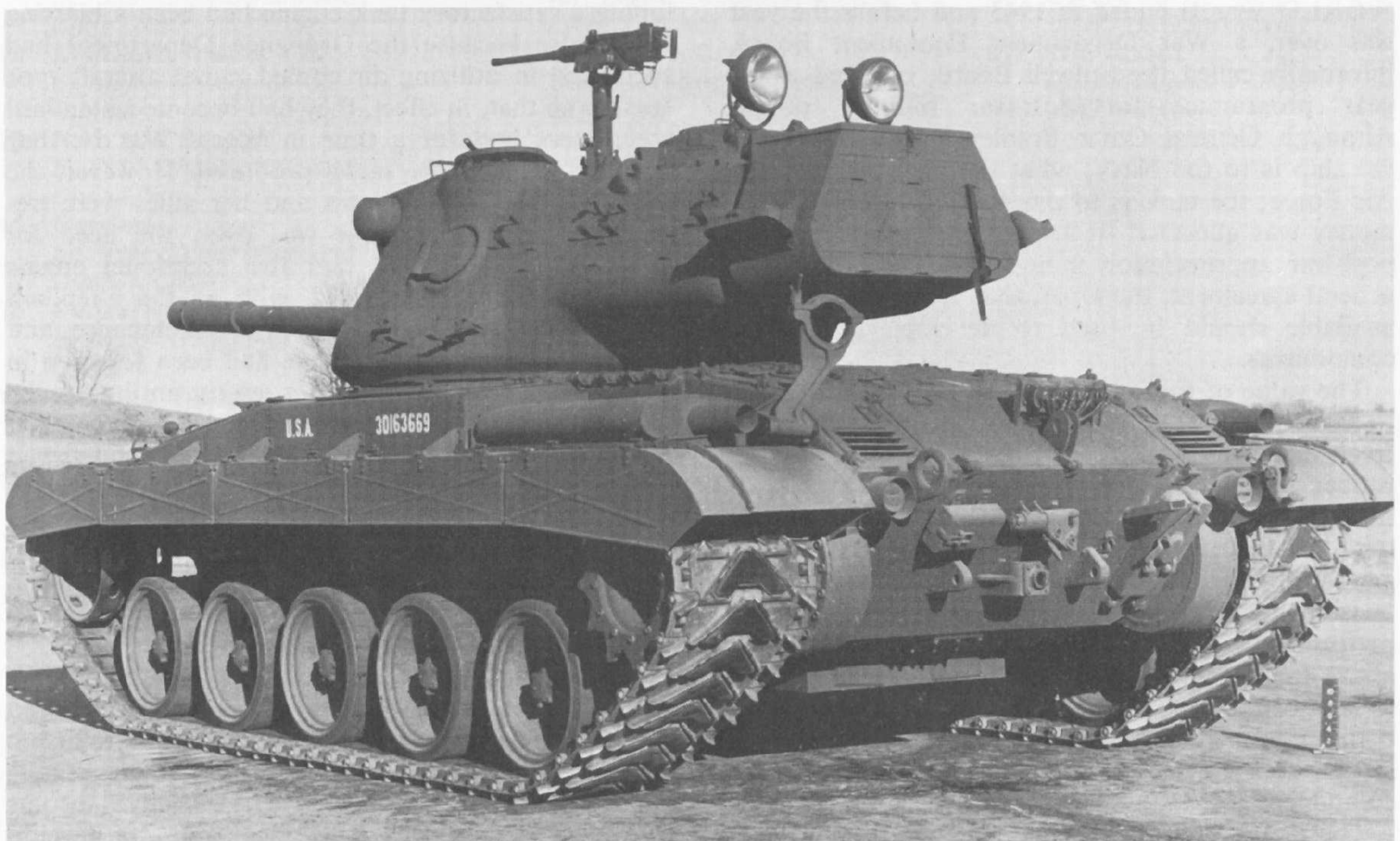
Three-quarter left rear view of the T.42 medium tank showing rangefinder turret, with pistol port and steel tracks with detachable pads.
