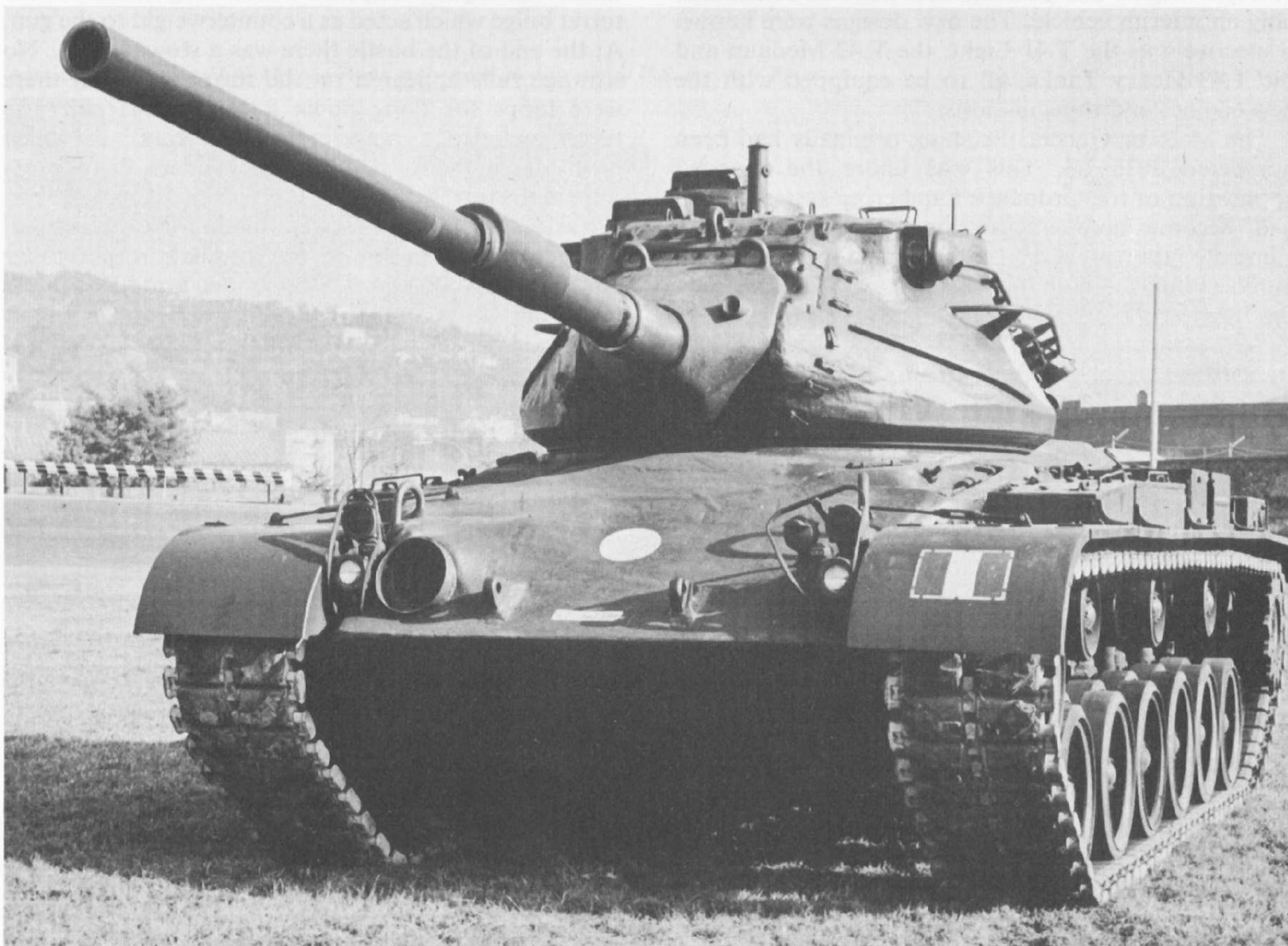
The M.47.R modified by OTO-Melara in Italy and offered commercially had a new diesel engine and new transmission and was armed with the British 105 mm. gun. (Photo courtesy OTO-Melara)
