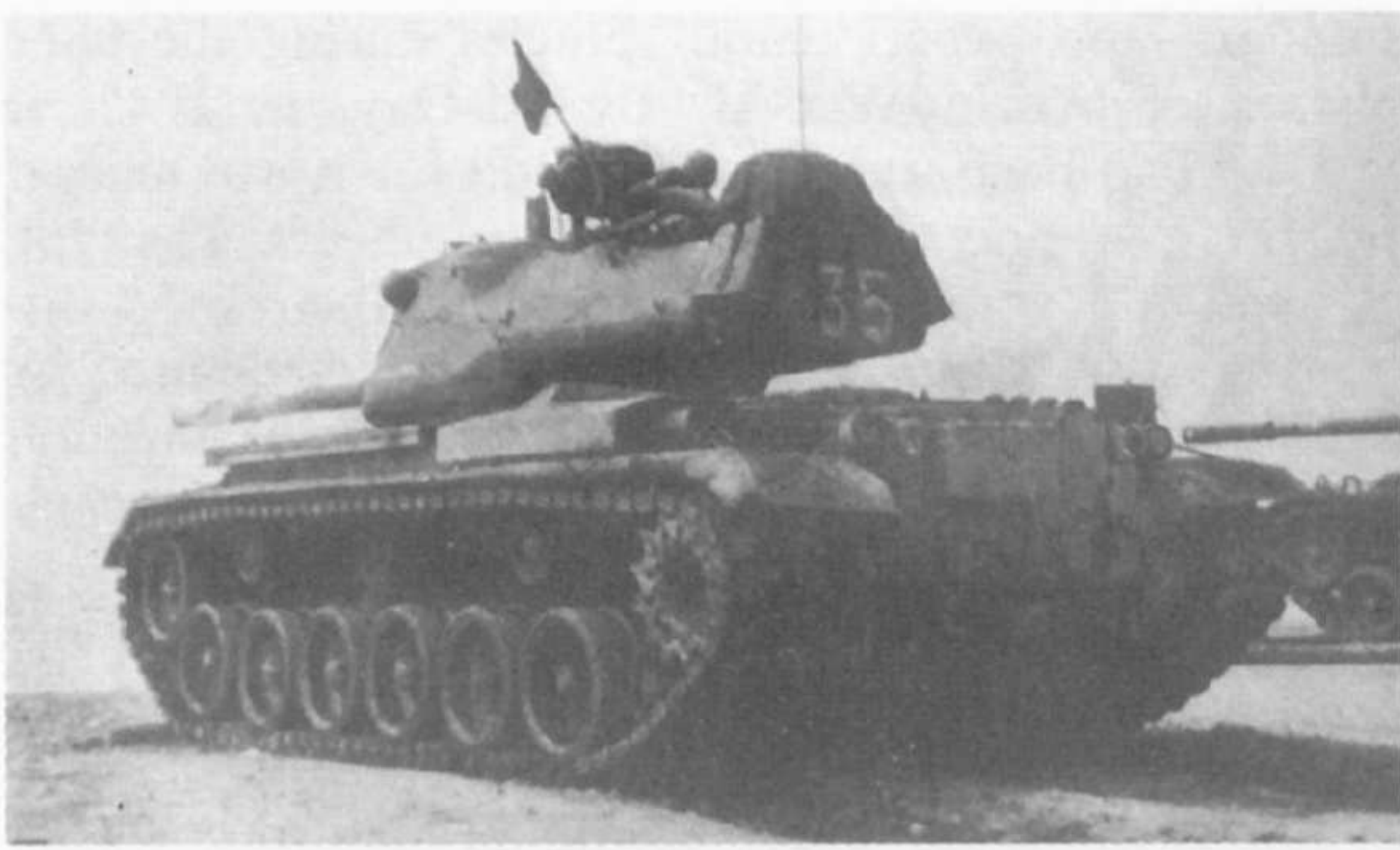
M.47 of U.S. Forces in Germany firing on a range, 1955. Compare this picture with that of the T.42 Medium. Note the three round inspection plates at the rear of the hull, characteristic of early M.47s which had modified M.46 hulls. Later hulls may not have these.
