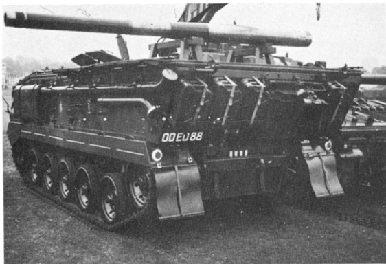
Three-quarter left rear view of FV434 with Abbot 105 mm barrel across rear load compartment. (C. F. Foss)
