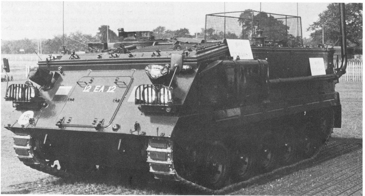
FV432 with FACE. Note wire rack over hatch and exhaust extension pipe fitted.
