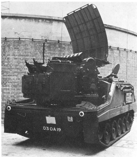
FV436 with Green Archer Mortar Locating Radar. (EMI Electronics Limited)
