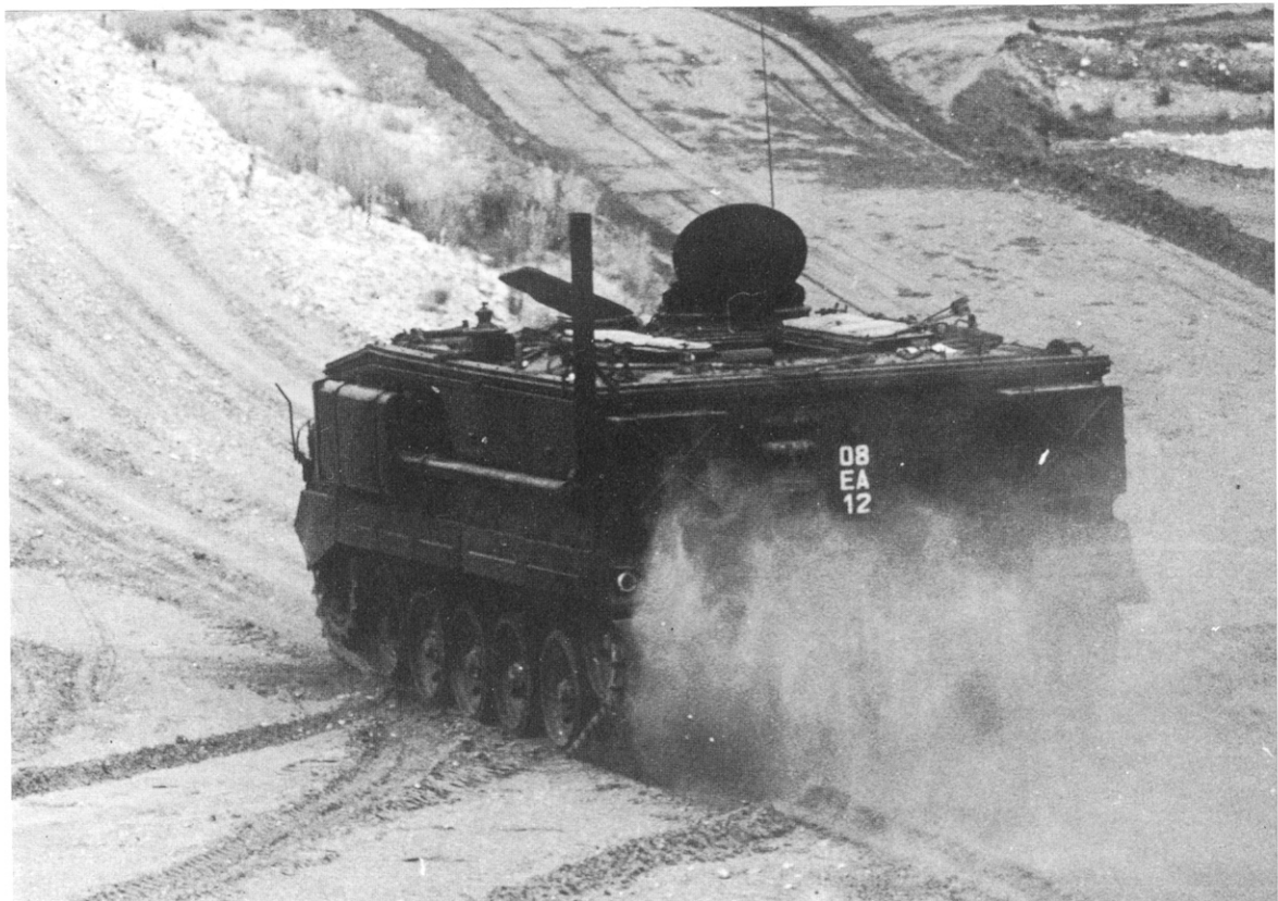
Three-quarter left rear view of FV432 with extension fitted to exhaust pipe. (C. F. Foss)
