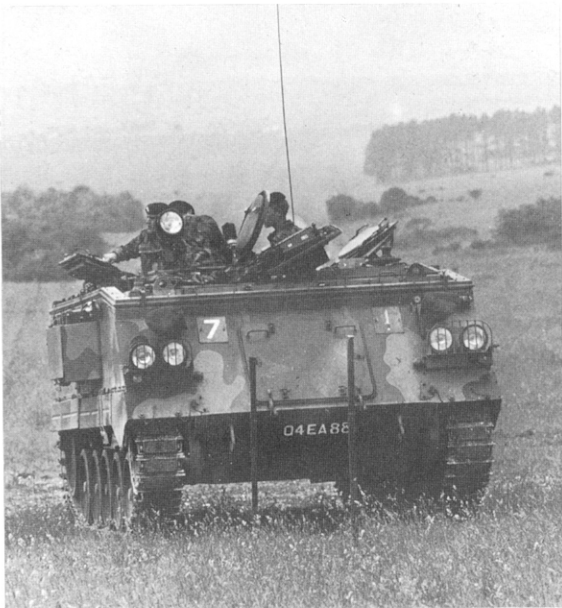
Front view of FV432 with no trim board on front of vehicle. (Sperry Rand Limited)
