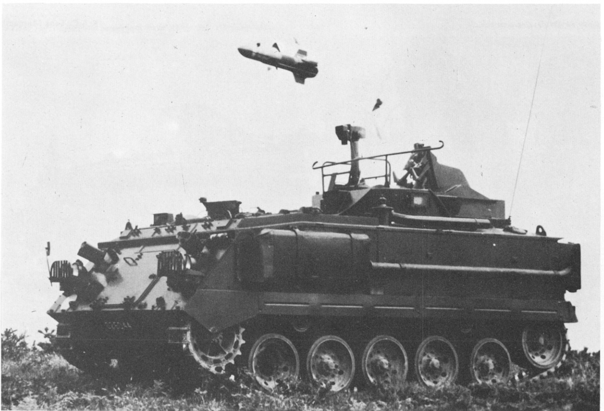
Swingfire missile being launched from FV438. (British Aircraft Corporation (Guided Weapons Division))
