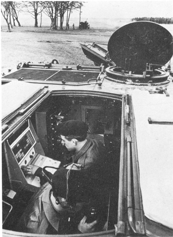
Interior view of FV432 with FACE showing part of installation. Note FV433 Abbot Self-Propelled Gun firing in background. (Marconi Space and Defence Systems Limited)
