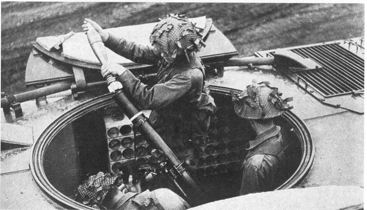
FV432 in its mortar rôle with 81 mm mortar firing through the roof of the vehicle.
