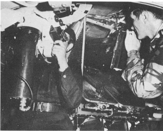
Inside an FV438: commander (left) searches for target while Swingfire missile is loaded (right). (British Aircraft Corporation (Guided Weapons Division))
