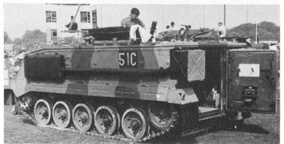
Three-quarter left rear view of FV432 with 81 mm mortar.
