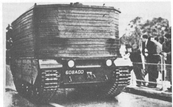
FV401 Cambridge (also known as the Carrier, Universal No. 4) with flotation screen erected.
